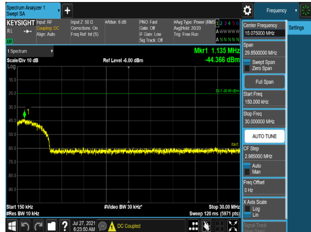
Plot 7-766. Conducted Spurious Emission Plot 150 kHz to 30 MHz (B13_5M+NB-lot(IB)_1C_QPSK – Middle Channel, Port 1)
