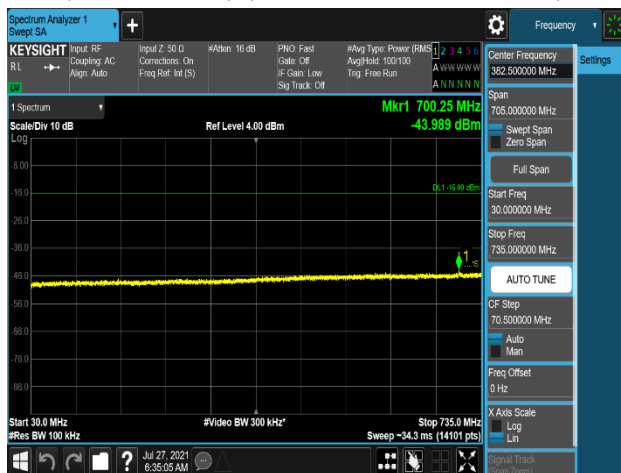
Plot 7-767. Conducted Spurious Emission Plot 30 MHz to 735 MHz (B13_5M+NB-lot(IB)_1C_QPSK – High Channel, Port 0)
