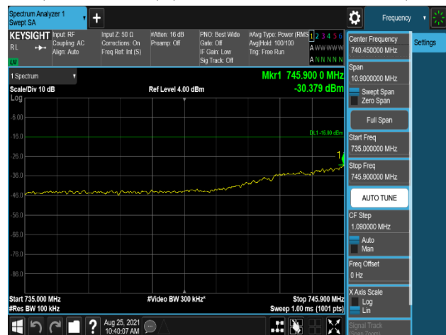
Plot 7-768. Conducted Spurious Emission Plot 735 MHz to 745.9 MHz (B13_5M+NB-lot(IB)_1C_QPSK – Low Channel, Port 1)
