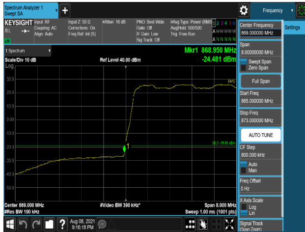
Plot 7-655. Band Edge Emission (868MHz to 869MHz) Plot (B5_10M(DSS)+5M_2C_16QAM - Low Channel, Port 2)
