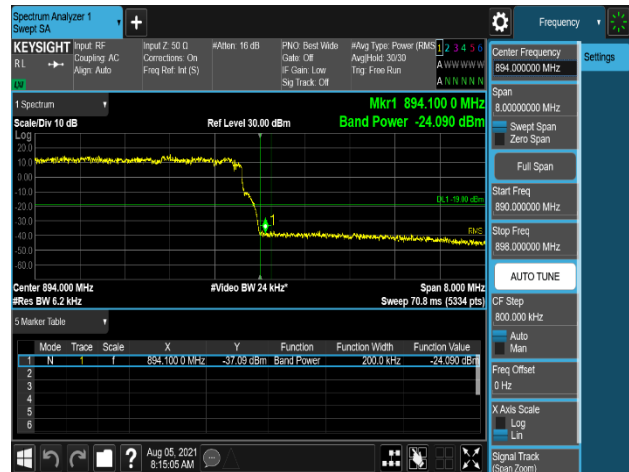
Plot 7-646. Band Edge Emission (894MHz to 895MHz) Plot Integration method Plot (B5_10M(DSS)+10M_2C_64QAM - High Channel, Port 2)
