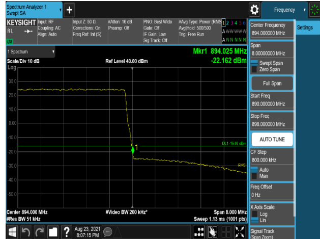
Plot 7-660. Band Edge Emission (894MHz to 895MHz) Plot (B5_10M(DSS)+5M_2C_256QAM - High Channel, Port 1)
