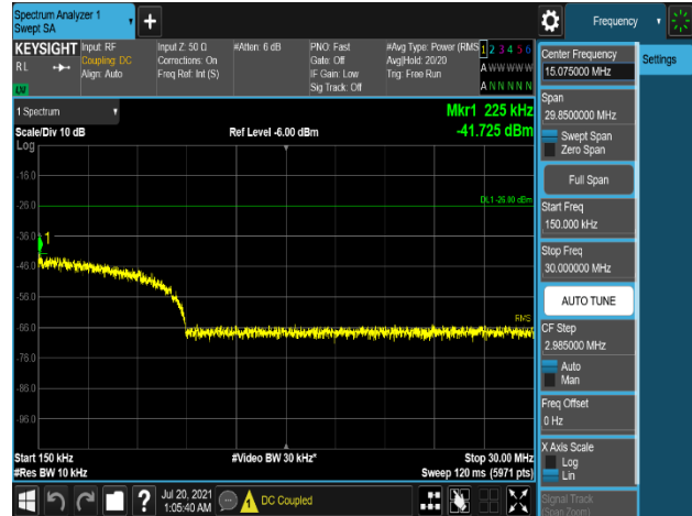
Plot 7-670. Conducted Spurious Emission Plot 150 kHz to 30 MHz (B5_10M_1C_2T_16QAM - Low Channel, Port 1)
