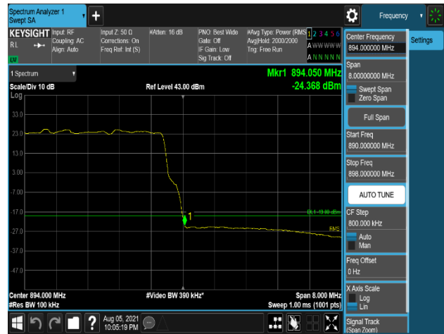
Plot 7-658. Band Edge Emission (894MHz to 895MHz) Plot (B5_10M(DSS)+10M_2C_16QAM - High Channel, Port 2)
