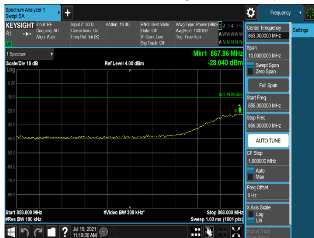
Plot 7-666. Conducted Spurious Emission Plot 858 MHz to 868 MHz (B5_5M_1C_2T_QPSK - Low Channel, Port 1)
