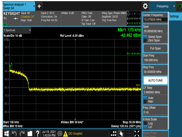
Plot 7-664. Conducted Spurious Emission Plot 150 kHz to 30 MHz (B5_5M_1C_2T_256QAM - High Channel, Port 1)
