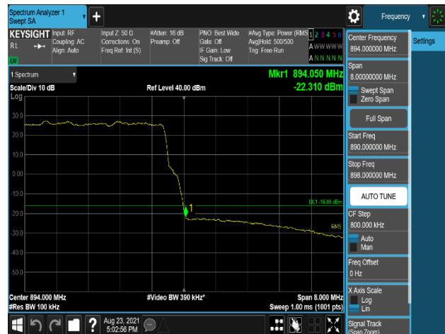
Plot 7-662. Band Edge Emission (894MHz to 895MHz) Plot (B5_10M(DSS)+10M_2C_16QAM - High Channel, Port 0)
