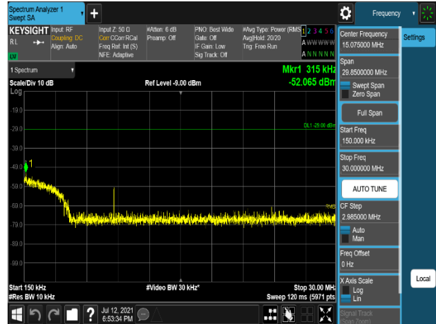
Plot 7-676. Conducted Spurious Emission Plot 150 kHz to 30 MHz (B5_5M_1C_64QAM - Middle Channel, Port 0)
