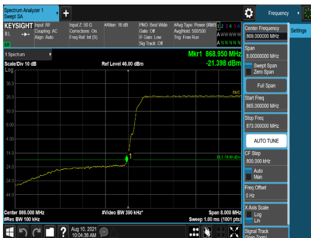
Plot 7-639. Band Edge Emission (868MHz to 869MHz) Plot (B5_10M(DSS_7:3)_1C_QPSK - Low Channel, Port 2)
