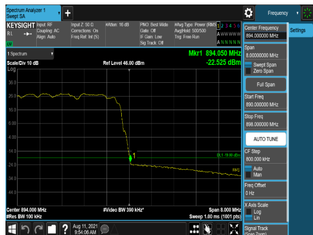
Plot 7-640. Band Edge Emission (894MHz to 895MHz) Plot (B5_10M(DSS_7:3)_1C_256QAM - Low Channel, Port 2)
