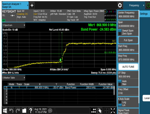
Plot 7-651. Band Edge Emission (868MHz to 869MHz) Plot Integration method Plot (B5_10M(DSS)+10M_2C_64QAM - Low Channel, Port 0)
