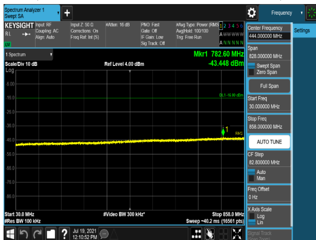
Plot 7-665. Conducted Spurious Emission Plot 30 MHz to 858 MHz (B5_5M_1C_2T_QPSK - Middle Channel, Port 0)
