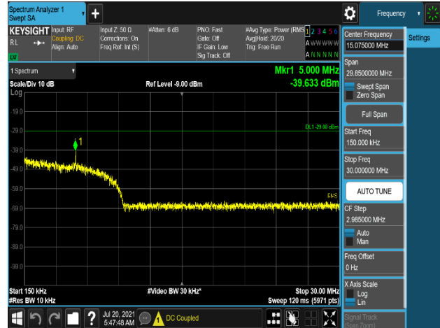
Plot 7-688. Conducted Spurious Emission Plot 150 kHz to 30 MHz (B5_5M+5M_2C_2T_16QAM - High Channel, Port 0)
