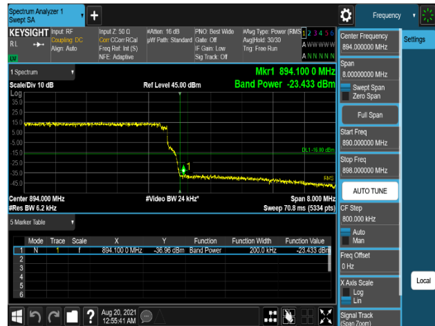
Plot 7-652. Band Edge Emission (894MHz to 895MHz) Plot Integration method Plot (B5_10M(DSS)+10M_2C_QPSK - High Channel, Port 0)
