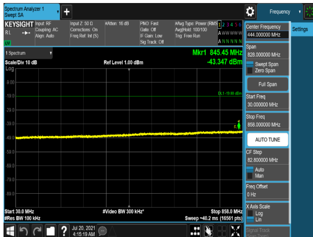
Plot 7-689. Conducted Spurious Emission Plot 30 MHz to 858 MHz (B5_5M+5M_2C_2T_QPSK - Low Channel, Port 1)
