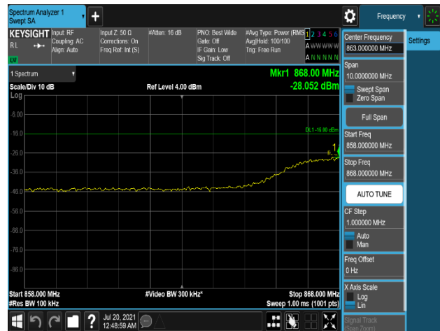
Plot 7-672. Conducted Spurious Emission Plot 858 MHz to 868 MHz (B5_10M_2T_1C_QPSK - Low Channel, Port 1)
