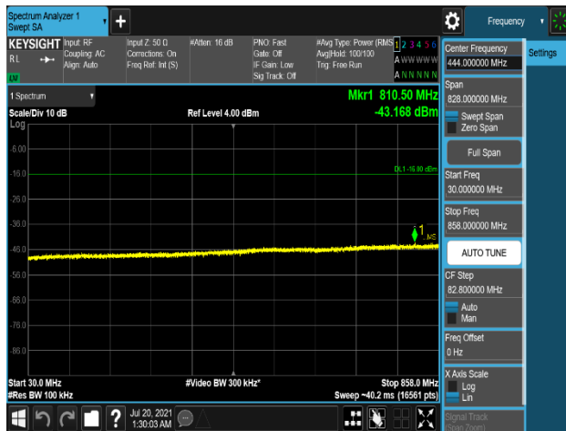
Plot 7-671. Conducted Spurious Emission Plot 30 MHz to 858 MHz (B5_10M_1C_2T_256QAM - Low Channel, Port 0)
