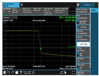
Plot 7-602. Band Edge Emission (756MHz to 756.1MHz) Plot (B13\_5M\_1C\_64QAM - High Channel, Port 3)
