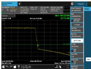
Plot 7-578. Band Edge Emission (894MHz to 895MHz) Plot (B5\_5M\_1C\_64QAM - High Channel, Port 2)
