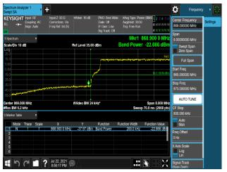
Plot 7-594. Band Edge Emission (868MHz to 869MHz) Plot (B5\_10M+10M\_2C\_64QAM\_Non-contiguous - Low Channel, Port 0)
