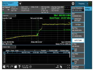
Plot 7-583. Band Edge Emission (868MHz to 869MHz) Plot (B5\_10M+10M\_2C\_16QAM - Low Channel, Port 1)
