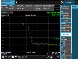
Plot 7-636. Band Edge Emission (756MHz to 756.1MHz) Plot (B13 10M+Low NB-lot(IB)+Low NB-lot(IB) 1C - Port 2)
