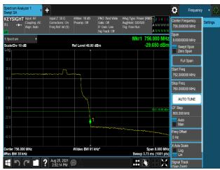
Plot 7-616. Band Edge Emission (756MHz to 756.1MHz) Plot (B13 10M+Low NB-lot(IB)+High NB-lot(IB) 3C - Port 1)
