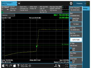
Plot 7-607. Band Edge Emission (745.9MHz to 746MHz) Plot (B13\_5M+5M\_2C\_QPSK - Low Channel, Port 1)
