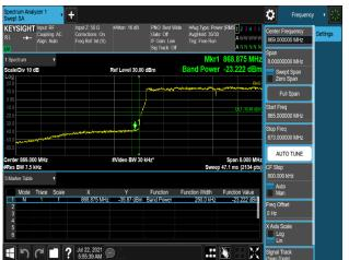
Plot 7-589. Band Edge Emission (868MHz to 869MHz) Plot (B2\_5M+10M+10M\_3C\_16QAM - Low Channel, Port 0)
