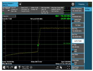
Plot 7-601. Band Edge Emission (745.9MHz to 746MHz) Plot (B13\_5M\_1C\_256QAM - Low Channel, Port 1)
