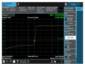
Plot 7-605. Band Edge Emission (745.9MHz to 746MHz) Plot (B13\_5M+5M\_2C\_16QAM - Low Channel, Port 1)
