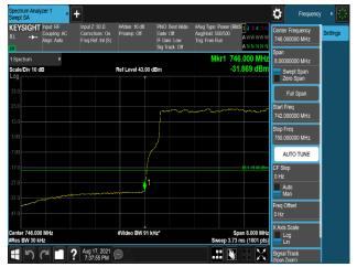
Plot 7-603. Band Edge Emission (745.9MHz to 746MHz) Plot (B13\_10M\_1C\_16QAM - Low Channel, Port 3)
