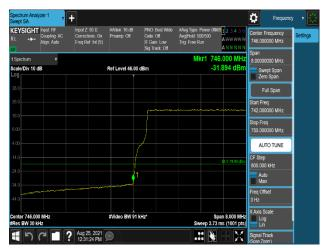
Plot 7-625. Band Edge Emission (745.9MHz to 746MHz) Plot (B13\_10M+High\_NB-lot(IB)+High\_NB-lot(IB)\_1C - Port 0)
