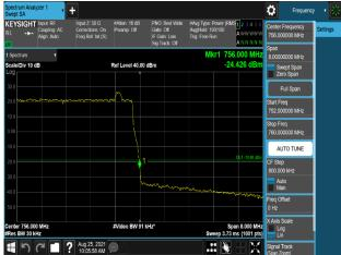
Plot 7-613. Band Edge Emission (745.9MHz to 746MHz) Plot (B13\_5M+NB-lot(IB)\_ 2C - Port 1)
