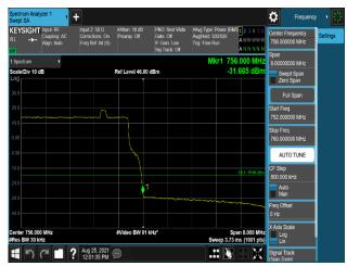
Plot 7-622. Band Edge Emission (756MHz to 756.1MHz) Plot (B13 10M+Low NB-lot(IB)+High NB-lot(IB) 1C - Port 3)
