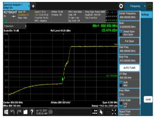
Plot 7-579. Band Edge Emission (868MHz to 869MHz) Plot (B5\_10M\_1C\_256QAM - Low Channel, Port 1)
