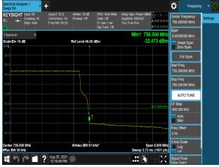
Plot 7-624. Band Edge Emission (756MHz to 756.1MHz) Plot (B13 10M+Low NB-lot(IB)+Low NB-lot(IB) 1C - Port 3)
