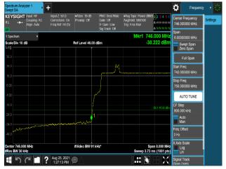
Plot 7-637. Band Edge Emission (745.9MHz to 746MHz) Plot (B13\_10M+High\_NB-lot(IB)+High\_NB-lot(IB)\_1C - Port 2)
