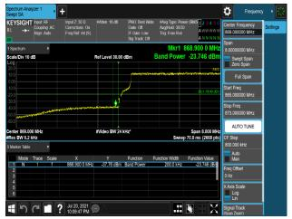
Plot 7-587. Band Edge Emission (868MHz to 869MHz) Plot (B5\_10M+10M\_2C\_64QAM - Low Channel, Port 3)
