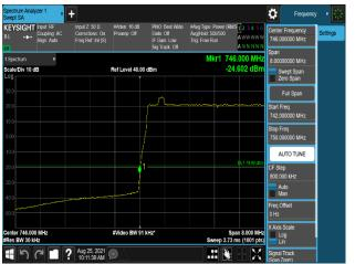
Plot 7-611. Band Edge Emission (745.9MHz to 746MHz) Plot (B13\_5M+NB-lot(IB)\_ 2C - Port 1)
