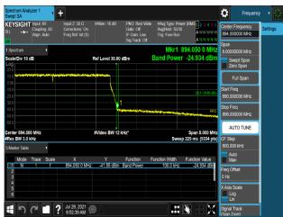
Plot 7-586. Band Edge Emission (894MHz to 895MHz) Plot (B5\_5M+5M\_2C\_64QAM - High Channel, Port 3)
