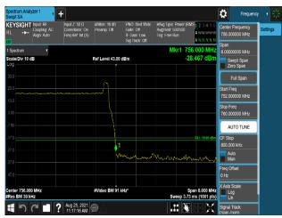
Plot 7-634. Band Edge Emission (756MHz to 756.1MHz) Plot (B13\_10M+Low\_NB-lot(IB)+High\_NB-lot(IB)\_1C - Port 2)
