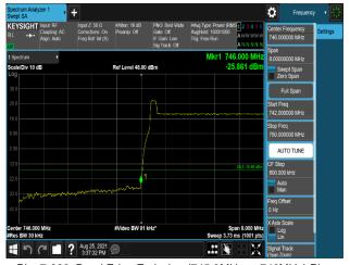
Plot 7-629. Band Edge Emission (745.9MHz to 746MHz) Plot (B13\_10M+Low\_NB-lot(IB)+Low\_NB-lot(IB)\_1C - Port 0)
