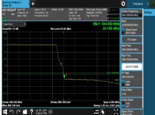
Plot 7 860. Band Edge Emission (894MHz to 895MHz) Plot (B5\_10M+10M\_2C\_256QAM\_Non-contiguous - High Channel, Port 3)
