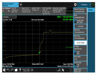
Plot 7-615. Band Edge Emission (745.9MHz to 746MHz) Plot (B13\_10M+Low\_NB-lot(IB)+High\_NB-lot(IB)\_3C - Port 0)
