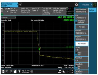
Plot 7-598. Band Edge Emission (756MHz to 756.1MHz) Plot (B13\_5M\_1C\_256QAM - High Channel, Port 1)
