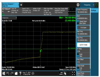
Plot 7-597. Band Edge Emission (745.9MHz to 746MHz) Plot (B13\_5M\_1C\_QPSK - Low Channel, Port 1)
