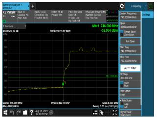
Plot 7-623. Band Edge Emission (745.9MHz to 746MHz) Plot (B13 10M+Low NB-lot(IB)+Low NB-lot(IB) 1C - Port 0)
