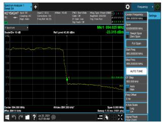
Plot 7 860. Band Edge Emission (894MHz to 895MHz) Plot (B5\_5M+5M\_2C\_16QAM\_Non-contiguous High Channel, Port 2)
