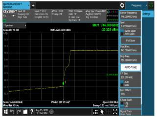
Plot 7-619. Band Edge Emission (745.9MHz to 746MHz) Plot (B13\_10M+High\_NB-lot(IB)+High\_NB-lot(IB)\_1C - Port 0)
