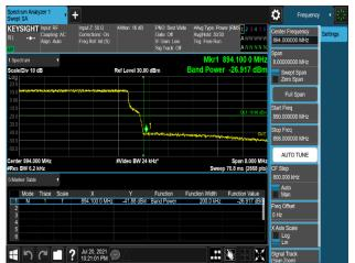
Plot 7-588. Band Edge Emission (894MHz to 895MHz) Plot (B5\_10M+10M\_2C\_QPSK - High Channel, Port 0)
