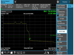
Plot 7-626. Band Edge Emission (756MHz to 756.1MHz) Plot (B13\_10M+High\_NB-lot(IB)+High\_NB-lot(IB)\_1C - Port 3)
