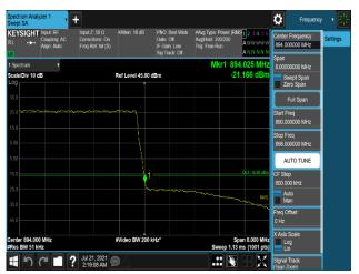
Plot 7 860. Band Edge Emission (894MHz to 895MHz) Plot (B5\_5M+5M\_2C\_256QAM\_Non-contiguous High Channel, Port 1)
