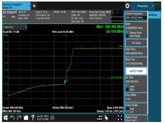
Plot 7-596. Band Edge Emission (868MHz to 869MHz) Plot (B5\_10M+10M\_2C\_256QAM\_Non-contiguous - Low Channel, Port 3)
