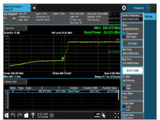
Plot 7-591. Band Edge Emission (868MHz to 869MHz) Plot (B2\_5M+10M+10M\_3C\_64QAM - Low Channel, Port 3)
