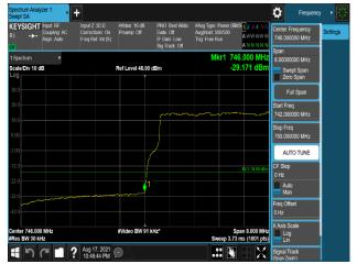
Plot 7-599. Band Edge Emission (745.9MHz to 746MHz) Plot (B13\_10M\_1C\_16QAM - Low Channel, Port 0)
