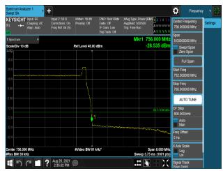
Plot 7-628. Band Edge Emission (756MHz to 756.1MHz) Plot (B13\_10M+Low\_NB-lot(IB)+High\_NB-lot(IB)\_1C - Port 1)
