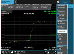
Plot 7-617. Band Edge Emission (745.9MHz to 746MHz) Plot (B13 10M+Low NB-lot(IB)+Low NB-lot(IB) 3C - Port 1)
