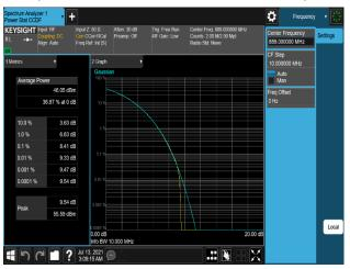
Plot 7-474. Peak To Average Power Ratio Plot (B5\_10M\_1C\_256QAM – High Channel, Port 1)
