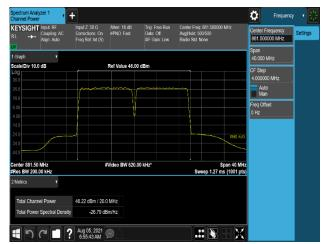
Plot 7-440. Conducted Average Output Power Plot (B5\_10M(DSS)+10M\_2C\_256QAM - Mid Channel, Port 3)
