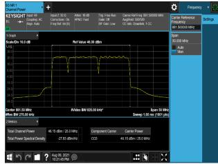
Plot 7-459. Conducted Average Output Power Plot (B5\_10M(DSS)+10M+5M\_3C\_16QAM - Port 2)
