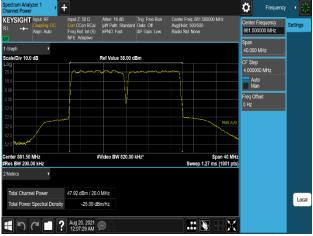
Plot 7-453. Conducted Average Output Power Plot (B5\_10M(DSS)+10M\_2C\_16QAM - Mid Channel, Port 0)
