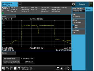
Plot 7-438. Conducted Average Output Power Plot (B5\_10M(DSS)+10M\_2C\_256QAM - Mid Channel, Port 1)
