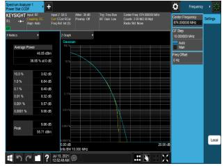
Plot 7-472. Peak To Average Power Ratio Plot (B5\_10M\_1C\_256QAM - Low Channel, Port 0)
