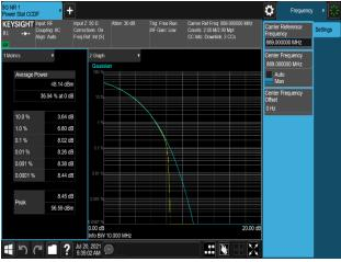
Plot 7-477. Peak To Average Power Ratio Plot (B5\_5M+5M\_2C\_QPSK - High Channel, Port 0)
