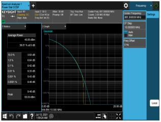
Plot 7-473. Peak To Average Power Ratio Plot (B5\_10M\_1C\_256QAM – Mid Channel, Port 0)
