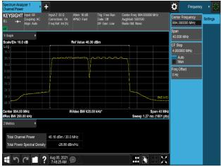
Plot 7-441. Conducted Average Output Power Plot (B5\_10M(DSS)+10M\_2C\_16QAM – High Channel, Port 0)
