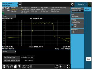
Plot 7-450. Conducted Average Output Power Plot (B5\_10M(DSS)+5M\_2C\_64QAM – High Channel, Port 1)
