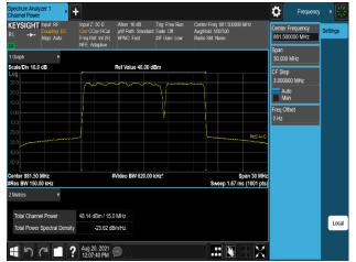
Plot 7-448. Conducted Average Output Power Plot (B5\_10M(DSS)+5M\_2C\_64QAM - Mid Channel, Port 1)
