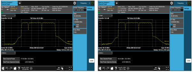
Plot 7-461. Conducted Average Output Power Plot (B5\_10M(DSS)+10M+5M\_3C\_16QAM - Port 0) Plot 7-462. Conducted Average Output Power Plot (B5\_10M(DSS)+10M+5M\_3C\_16QAM - Port 1)
