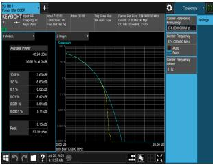
Plot 7-475. Peak To Average Power Ratio Plot (B5\_5M+5M\_2C\_QPSK - Low Channel, Port 1)
