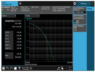
Plot 7-479. Peak To Average Power Ratio Plot (B5\_10M+10M\_2C\_16QAM – Mid Channel, Port 0)
