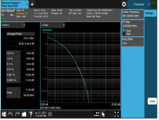
Plot 7-471. Peak To Average Power Ratio Plot (B5\_5M\_1C\_QPSK - High Channel, Port 1)
