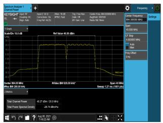
Plot 7-444. Conducted Average Output Power Plot (B5\_10M(DSS)+10M\_2C\_16QAM – High Channel, Port 3)
