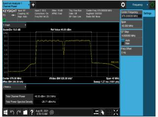
Plot 7-436. Conducted Average Output Power Plot (B5\_10M(DSS)+10M\_2C\_16QAM - Low Channel, Port 3)
