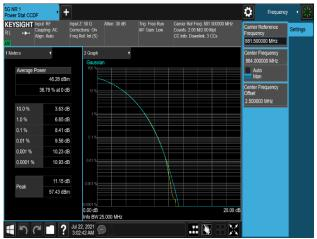
Plot 7-490. Peak To Average Power Ratio Plot (B5\_5M+10M+10M\_3C\_16QAM - Low Channel, Port 1)
