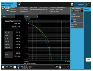
Plot 7-504. Peak To Average Power Ratio Plot (B5\_10M(DSS)\_1C\_256QAM - High Channel, Port 0)
