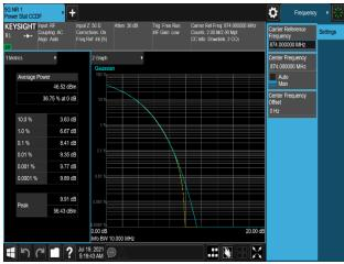
Plot 7-481. Peak To Average Power Ratio Plot (B5\_5M+5M\_2C\_64QAM - Low Channel, Port 1)
