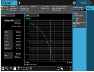
Plot 7-495. Peak To Average Power Ratio Plot (B5\_10M(DSS)\_1C\_64QAM - Low Channel, Port 0)
