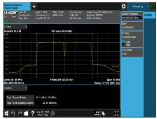
Plot 7-437. Conducted Average Output Power Plot (B5\_10M(DSS)+10M\_2C\_256QAM - Mid Channel, Port 0)
