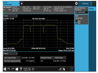
Plot 7-460. Conducted Average Output Power Plot (B5\_10M(DSS)+10M+5M\_3C\_16QAM - Port 3)
