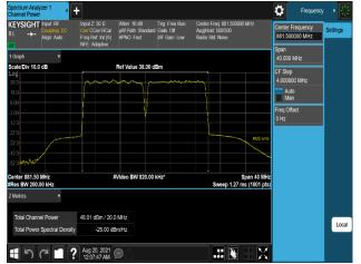
Plot 7-454. Conducted Average Output Power Plot (B5\_10M(DSS)+10M\_2C\_16QAM - Mid Channel, Port 1)
