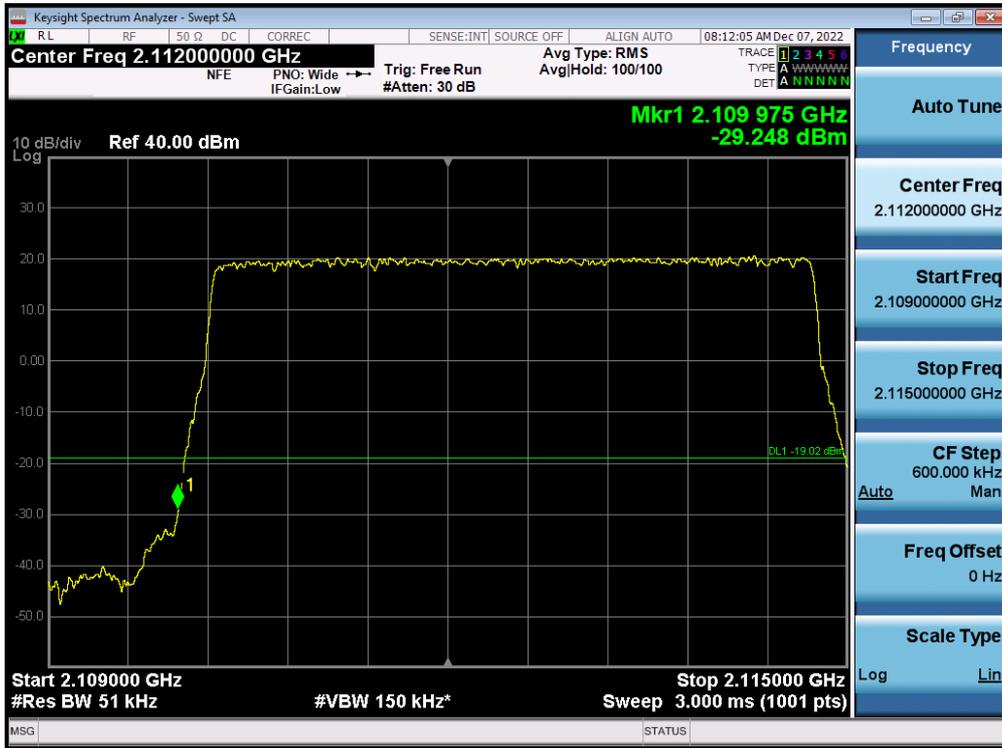
Antenna 1 / (4 Port) LTE B66 5 MHz 1 Carrier + 5G NR n66 5 MHz 1 Carrier + 5G NR n66 10 MHz 1 Carrier + 5G NR n66 20 MHz 1 Carrier [4 Carrier] / QPSK / High / Contiguous
