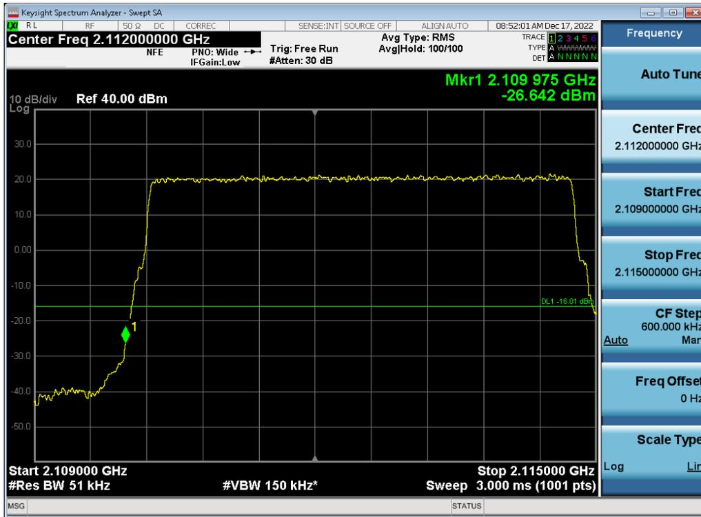
Antenna 0 / (2 Port) LTE B66 5 MHz 1 Carrier + 5G NR n66 5 MHz 1 Carrier + 5G NR n66 10 MHz 1 Carrier + 5G NR n66 20 MHz 1 Carrier [4 Carrier] / QPSK / High / Contiguous
