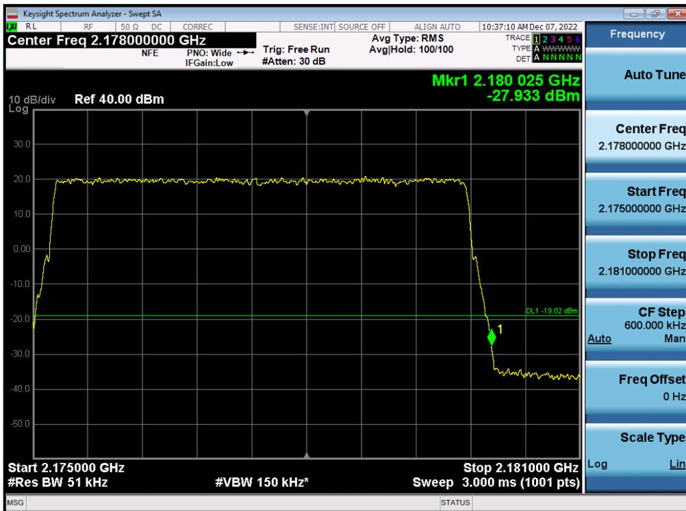
Antenna 3 / (4 Port) LTE B66 5 MHz 1 Carrier + 5G NR n66 5 MHz 1 Carrier + 5G NR n66 5 MHz 1 Carrier + DSS B66 10 MHz 1 Carrier [4 Carrier] / QPSK / Low / Contiguous
