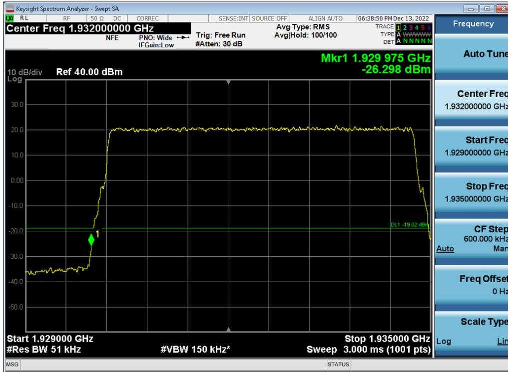
Antenna 0 / (4 Port) LTE B2 5 MHz 1 Carrier + 5G NR n2 5 MHz 1 Carrier + DSS B2 10 MHz 1 Carrier [3 Carrier] / 16QAM / High / Contiguous
