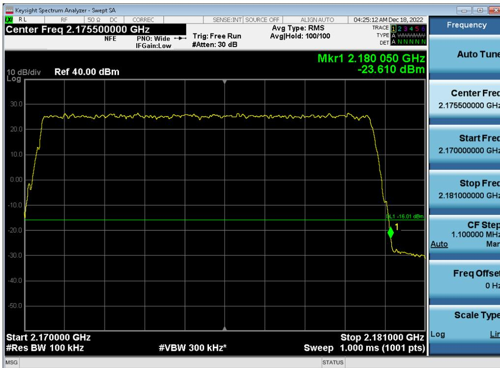
Antenna 1 / (2 Port) LTE B66 5 MHz 1 Carrier + 5G NR n66 5 MHz 1 Carrier + 5G NR n66 5 MHz 1 Carrier + DSS B66 10 MHz 1 Carrier [4 Carrier] [3C+1C] / 256QAM / Low / Non-Contiguous
