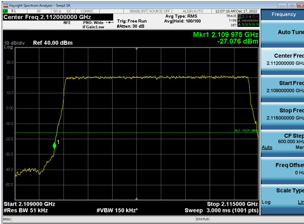
Antenna 0 / (2 Port) LTE B66 5 MHz 1 Carrier + LTE B66 5 MHz 1 Carrier + DSS B66 10 MHz 1 Carrier + DSS B66 20 MHz 1 Carrier [4 Carrier] / QPSK / High / Contiguous
