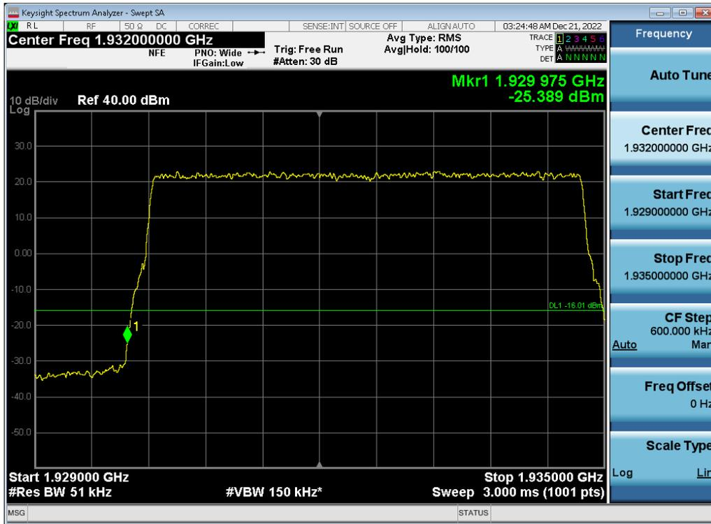
Antenna 1 / (2 Port) LTE B2 5 MHz 1 Carrier + 5G NR n2 5 MHz 1 Carrier + DSS B2 10 MHz 1 Carrier [3 Carrier] [2C+1C] / 256QAM / High / Non-Contiguous
