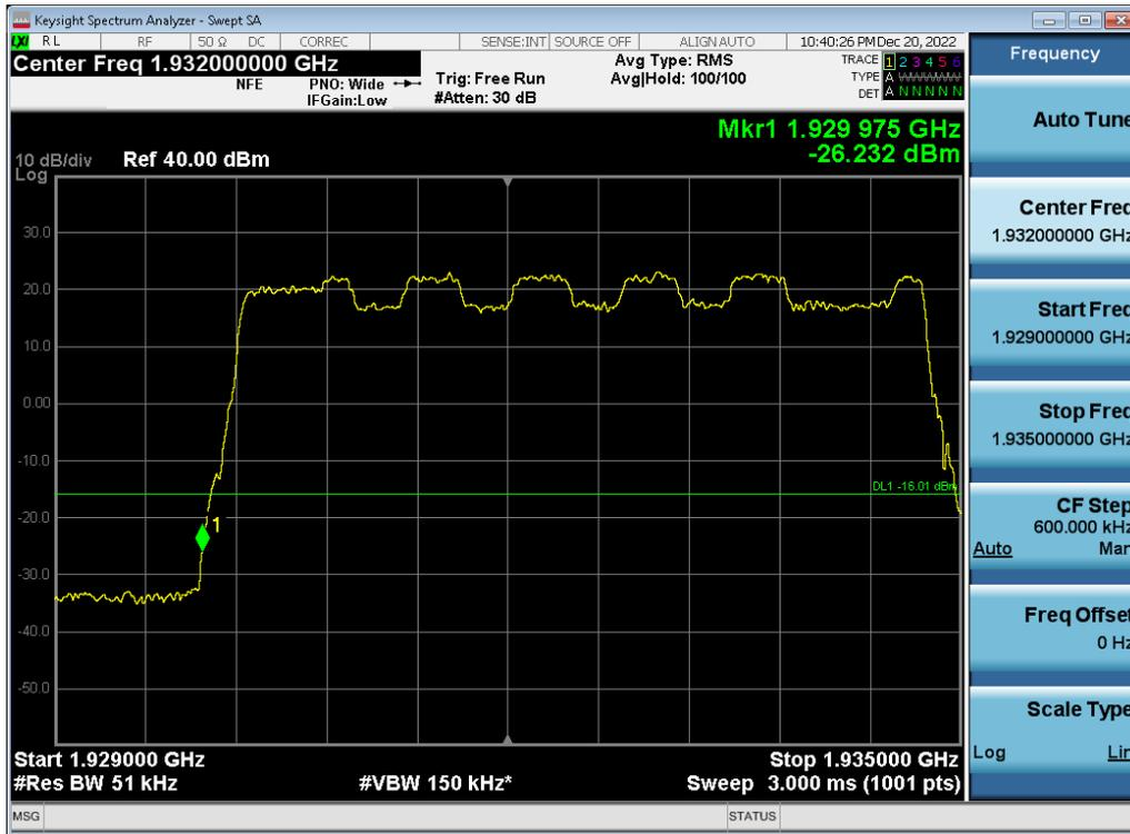
Antenna 0 / (2 Port) 5G NR n2 5 MHz 1 Carrier + 5G NR n2 5 MHz 1 Carrier + DSS B2 20 MHz 1 Carrier [3 Carrier] [2C+1C] / QPSK / High / Non-Contiguous
