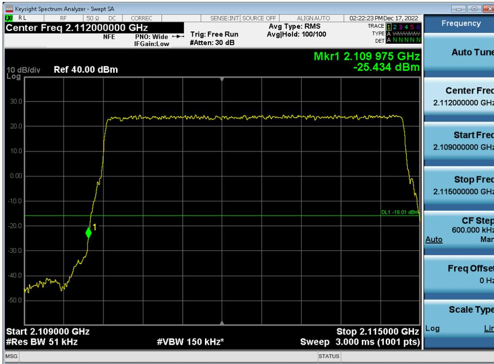
Antenna 0 / (2 Port) 5G NR n66 5 MHz 1 Carrier + 5G NR n66 5 MHz 1 Carrier + DSS B66 10 MHz 1 Carrier [3 Carrier] / 256QAM / High / Contiguous
