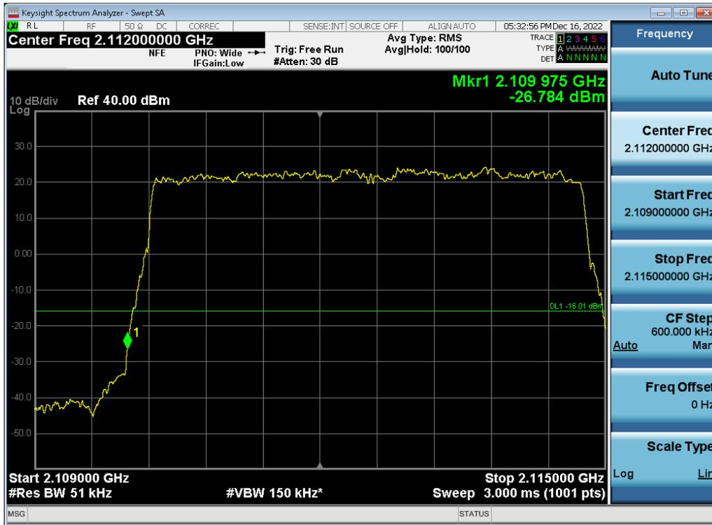
Antenna 1 / (2 Port) LTE B66 5 MHz 1 Carrier + LTE B66 5 MHz 1 Carrier + DSS B66 10 MHz 1 Carrier + DSS B66 10 MHz 1 Carrier [4 Carrier] / QPSK / High / Contiguous
