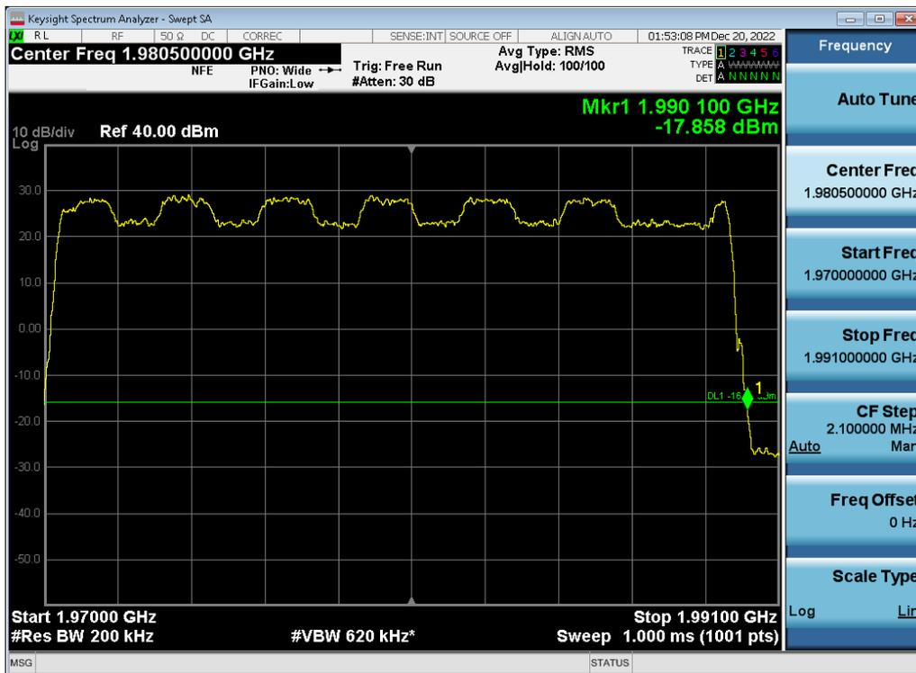
Antenna 0 / (2 Port) 5G NR n2 5 MHz 1 Carrier + 5G NR n2 5 MHz 1 Carrier + DSS B2 10 MHz 1 Carrier [3 Carrier] [1C+2C] / QPSK / Low / Non-Contiguous
