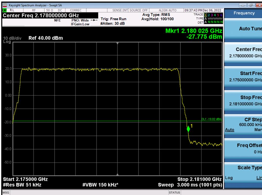
Antenna 1 / (2 Port) DSS B2 10 MHz 1 Carrier + DSS B2 10 MHz 1 Carrier [2 Carrier] / 64QAM / Low / Non-Contiguous
