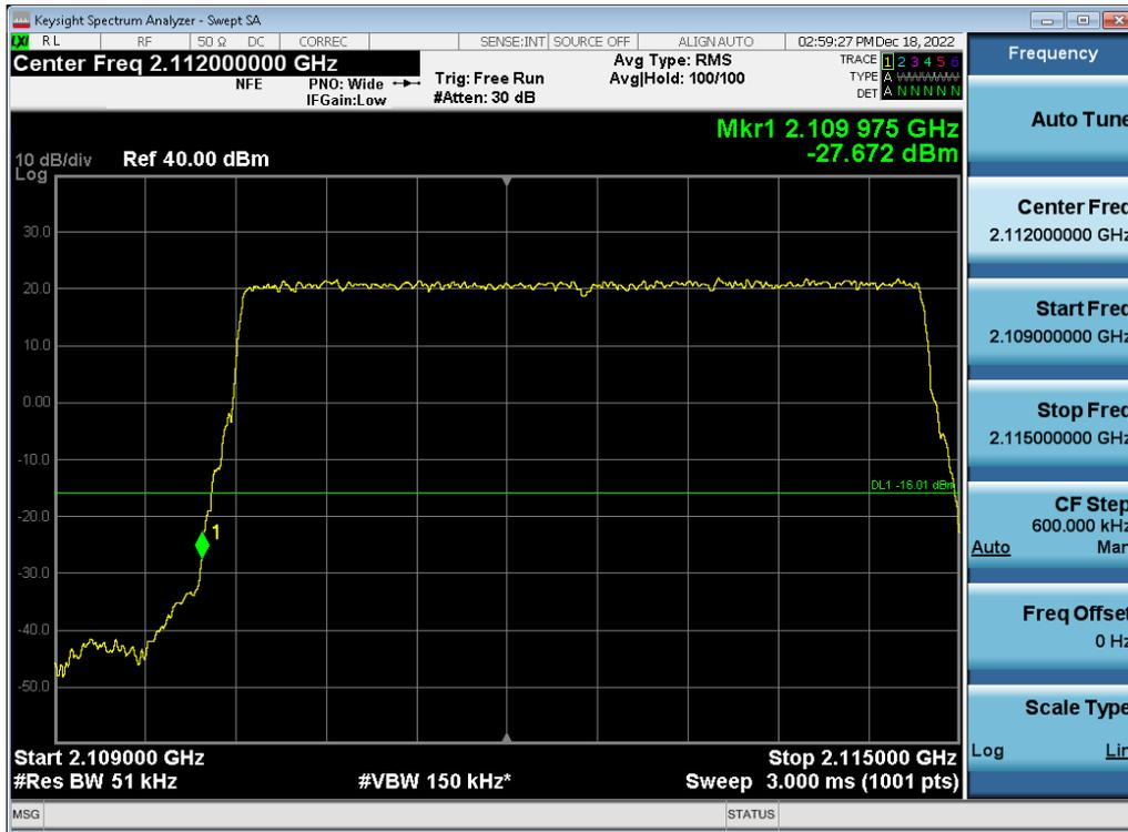
**Antenna 0 / (2 Port) LTE B66 5 MHz 1 Carrier + 5G NR n66 5 MHz 1 Carrier + DSS B66 10 MHz 1 Carrier + DSS B66 20 MHz 1 Carrier [4 Carrier] [1C+3C] / 64QAM / High / Non-Contiguous**
