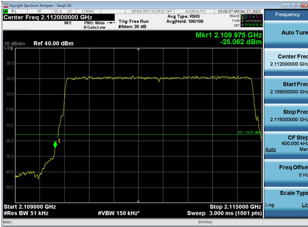
Antenna 0 / (2 Port) LTE B66 5 MHz 1 Carrier + LTE B66 5 MHz 1 Carrier + DSS B66 10 MHz 1 Carrier + DSS B66 20 MHz 1 Carrier [4 Carrier] [3C+1C] / 256QAM / High / Non-Contiguous
