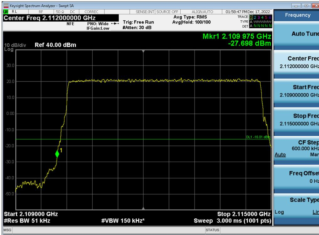
Antenna 1 / (2 Port) LTE B66 5 MHz 1 Carrier + 5G NR n66 5 MHz 1 Carrier + 5G NR n66 10 MHz 1 Carrier + 5G NR n66 20 MHz 1 Carrier [4 Carrier] [1C+3C] / 64QAM / High / Non-Contiguous
