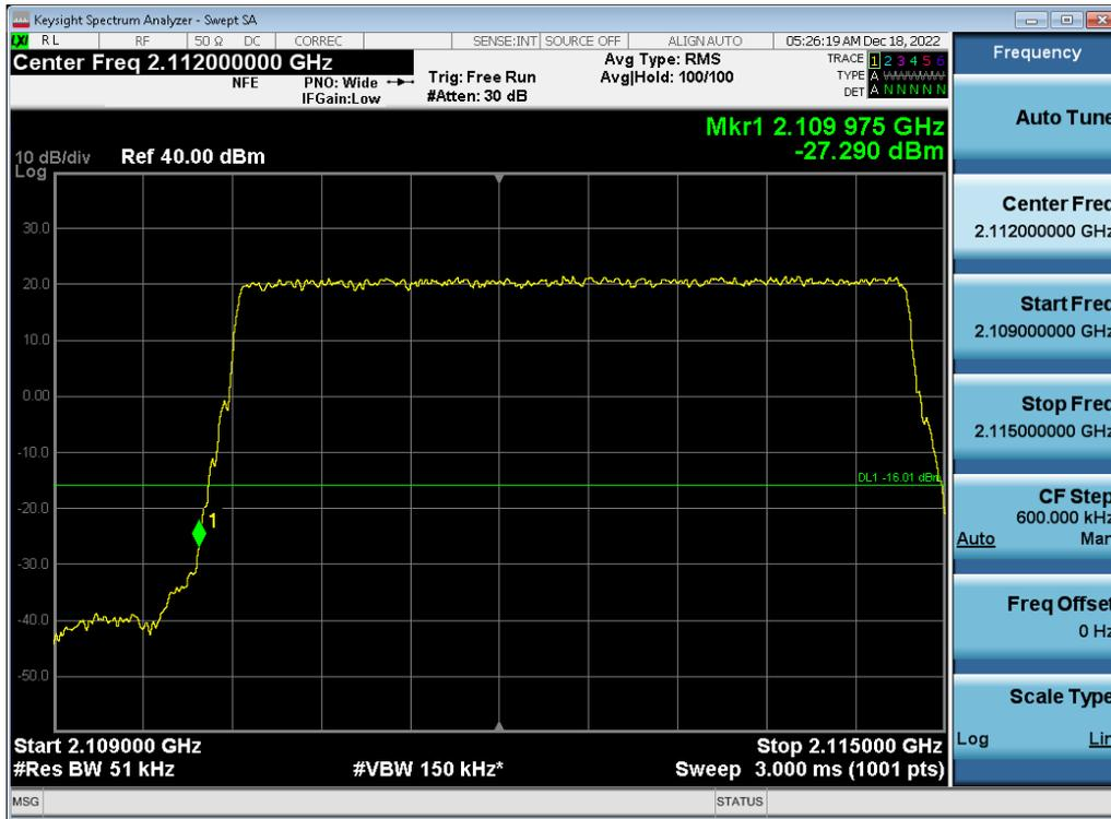
**Antenna 1 / (2 Port) LTE B66 5 MHz 1 Carrier + 5G NR n66 5 MHz 1 Carrier + DSS B66 10 MHz 1 Carrier + DSS B66 20 MHz 1 Carrier [4 Carrier] / 256QAM / High / Contiguous**
