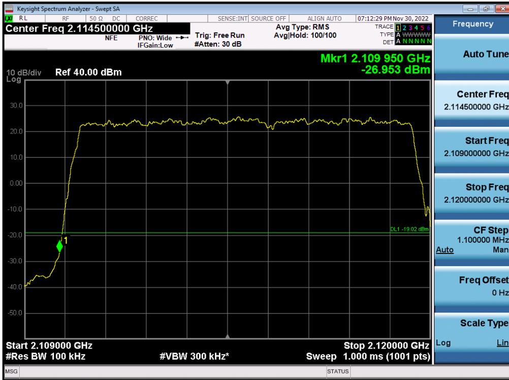
Antenna 2 / (4 Port) DSS B66 10 MHz 1 Carrier + DSS B66 10 MHz 1 Carrier + DSS B66 10 MHz 1 Carrier [3 Carrier] / QPSK / High / Contiguous
