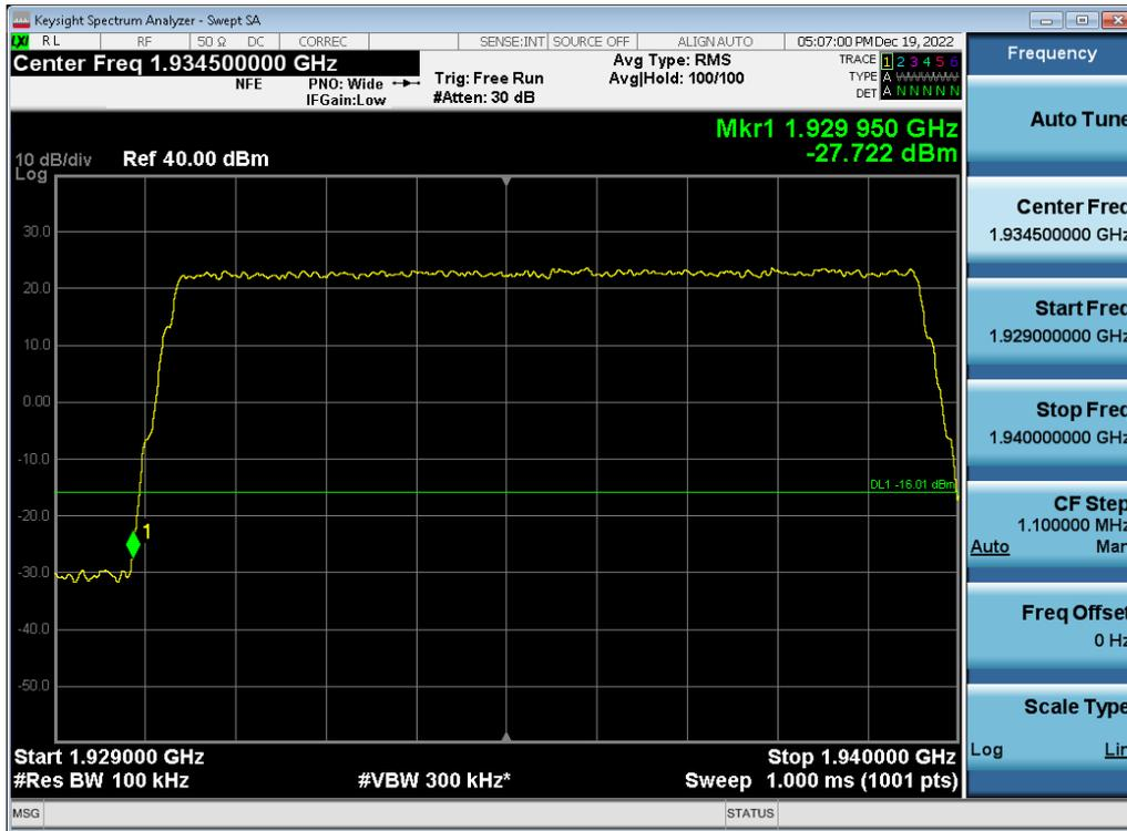
Antenna 1 / (2 Port) DSS B2 10 MHz 1 Carrier + DSS B2 10 MHz 1 Carrier + DSS B2 10 MHz 1 Carrier [3 Carrier] [2C+1C] / 64QAM / High / Non-Contiguous
