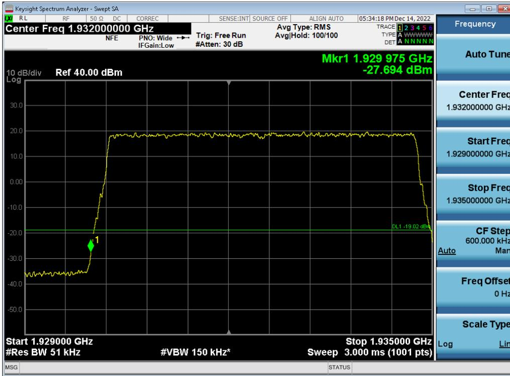
Antenna 3 / (4 Port) LTE B2 5 MHz 1 Carrier + 5G NR n2 5 MHz 1 Carrier + DSS B2 20 MHz 1 Carrier [3 Carrier] [1C+2C] / 16QAM / High / Non-Contiguous
