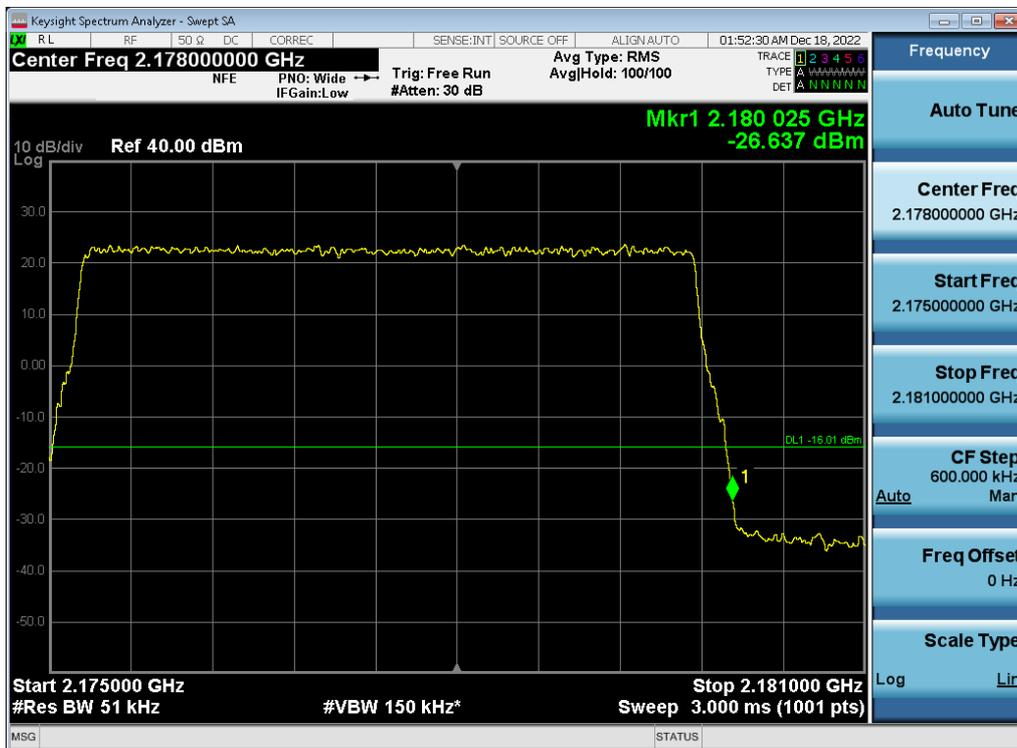
**Antenna 0 / (2 Port) LTE B66 5 MHz 1 Carrier + 5G NR n66 5 MHz 1 Carrier + DSS B66 10 MHz 1 Carrier + DSS B66 20 MHz 1 Carrier [4 Carrier] / 64QAM / Low / Contiguous**
