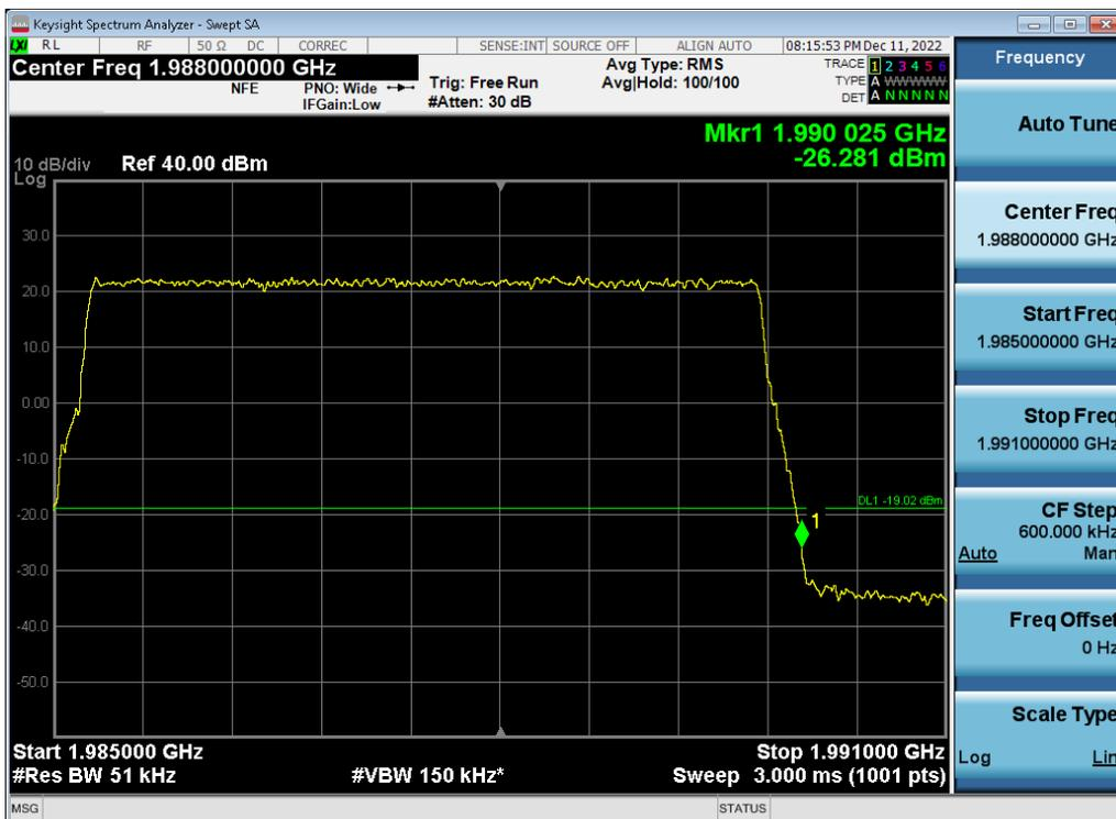
Antenna 0 / (4 Port) 5G NR n2 5 MHz 1 Carrier + 5G NR n2 5 MHz 1 Carrier + 5G NR n2 20 MHz 1 Carrier [3 Carrier] / 16QAM / Low / Contiguous
