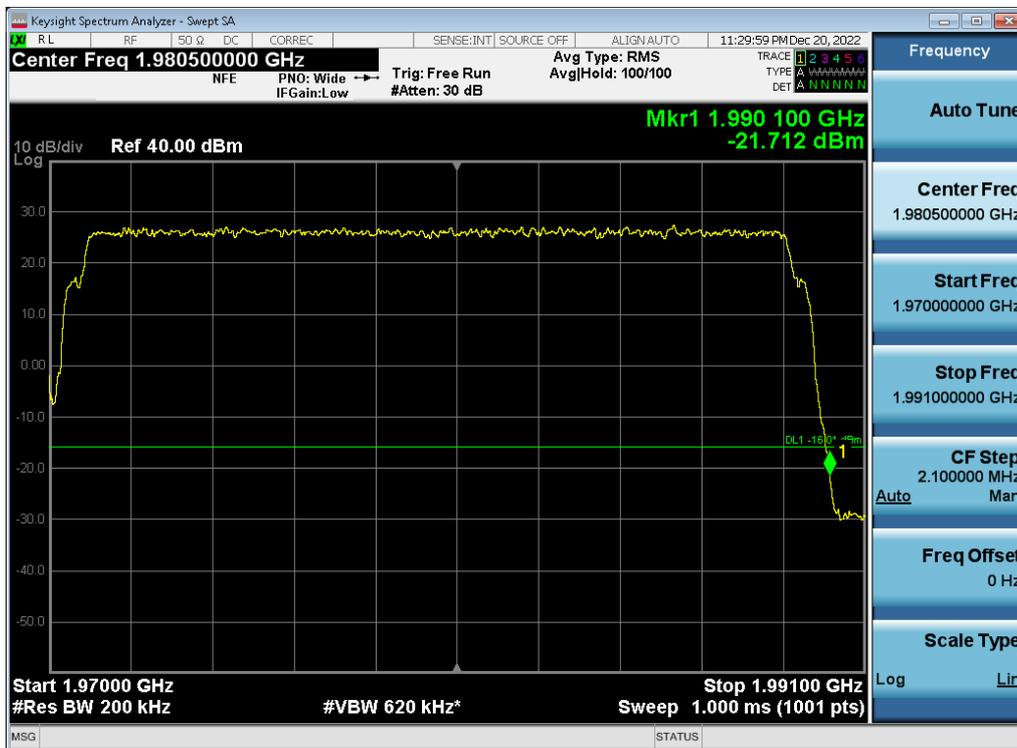
Antenna 1 / (2 Port) 5G NR n2 5 MHz 1 Carrier + 5G NR n2 5 MHz 1 Carrier + DSS B2 20 MHz 1 Carrier [3 Carrier] [2C+1C] / 16QAM / Low / Non-Contiguous
