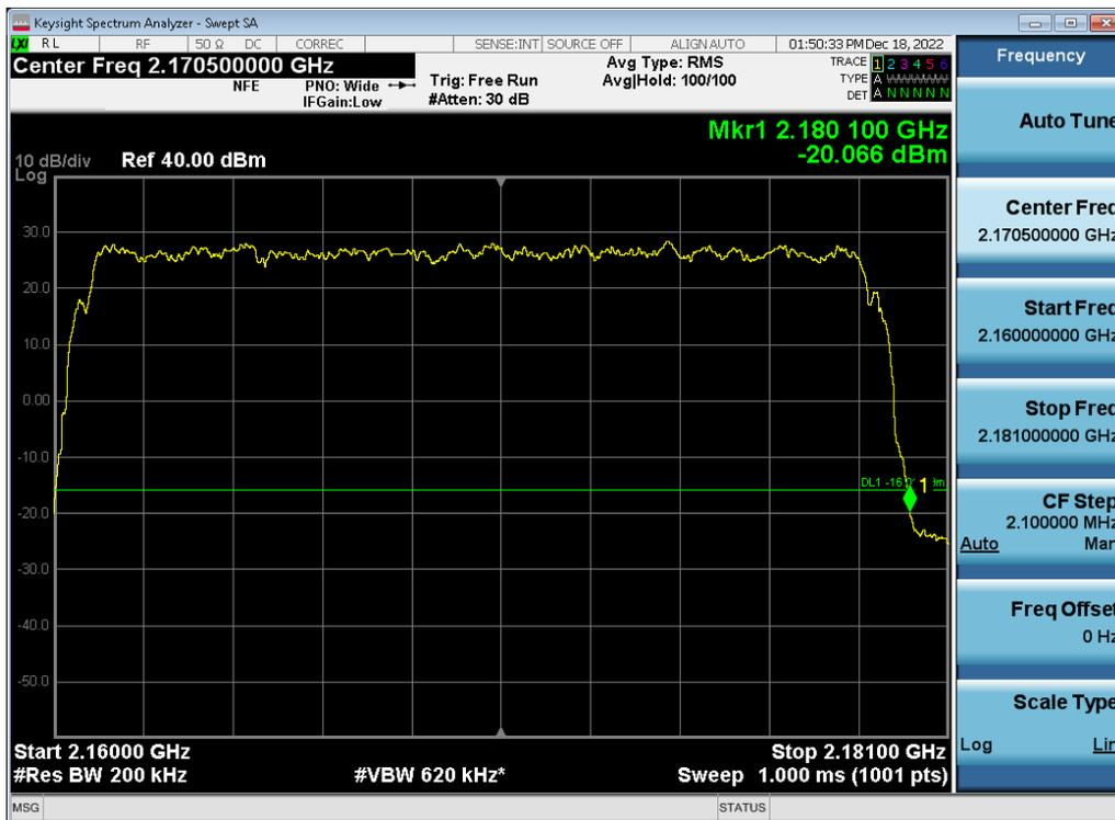
**Antenna 1 / (2 Port) LTE B66 5 MHz 1 Carrier + LTE B66 5 MHz 1 Carrier + DSS B66 10 MHz 1 Carrier + DSS B66 10 MHz 1 Carrier [4 Carrier] [1C+3C] / 64QAM / Low / Non-Contiguous**
