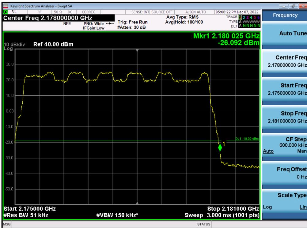
Antenna 0 / (4 Port) 5G NR n66 10 MHz 1 Carrier + 5G NR n66 20 MHz 1 Carrier + DSS B66 10 MHz 1 Carrier [3 Carrier] / 64QAM / Low / Contiguous
