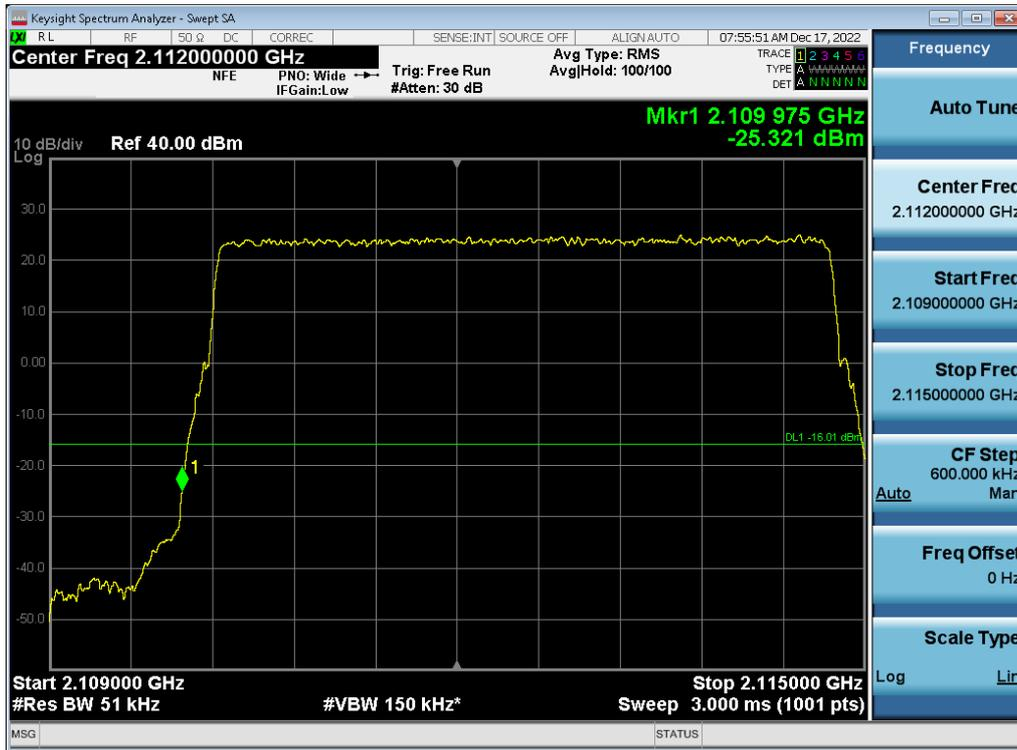
Antenna 1 / (2 Port) LTE B66 5 MHz 1 Carrier + 5G NR n66 5 MHz 1 Carrier + 5G NR n66 5 MHz 1 Carrier + 5G NR n66 5 MHz 1 Carrier [4 Carrier] [1C+3C] / 256QAM / High / Non-Contiguous
