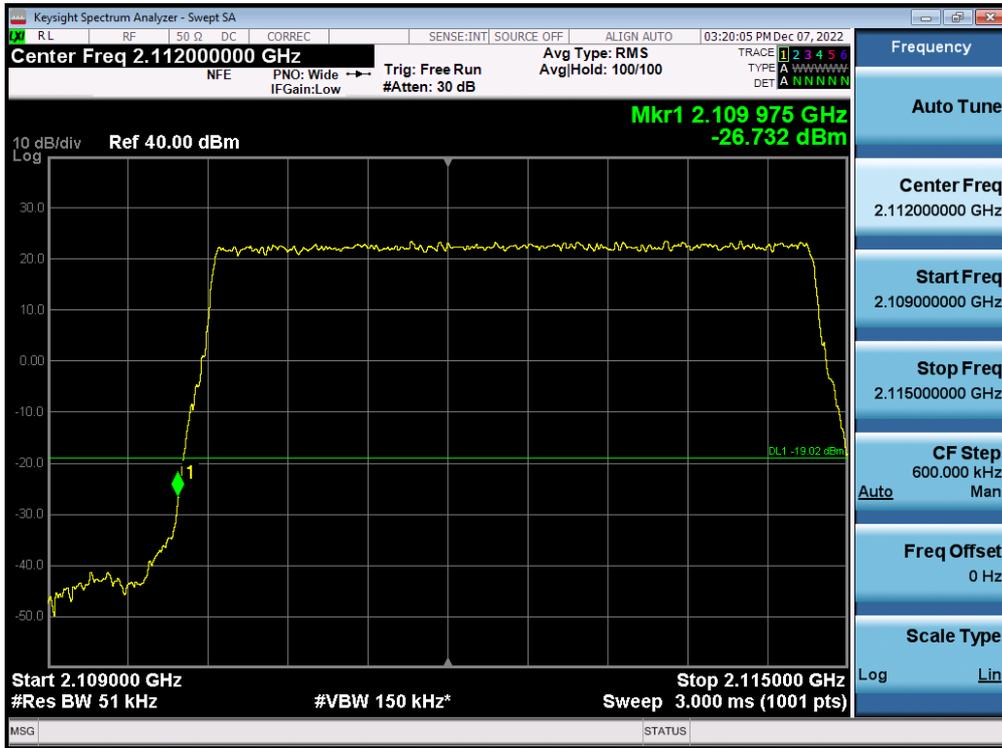
Antenna 0 / (4 Port) 5G NR n66 5 MHz 1 Carrier + 5G NR n66 5 MHz 1 Carrier + DSS B66 10 MHz 1 Carrier [3 Carrier] / 16QAM / High / Contiguous
