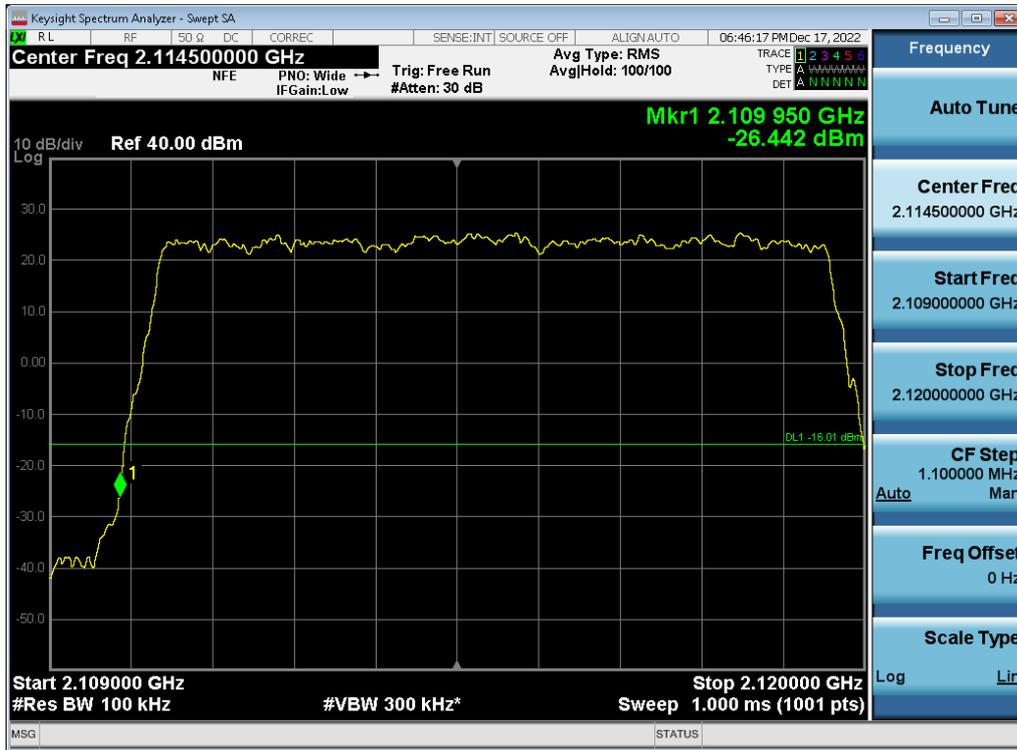
Antenna 0 / (2 Port) DSS B66 10 MHz 1 Carrier + 5G NR n66 10 MHz 1 Carrier + 5G NR n66 20 MHz 1 Carrier [3 Carrier] / QPSK / High / Contiguous
