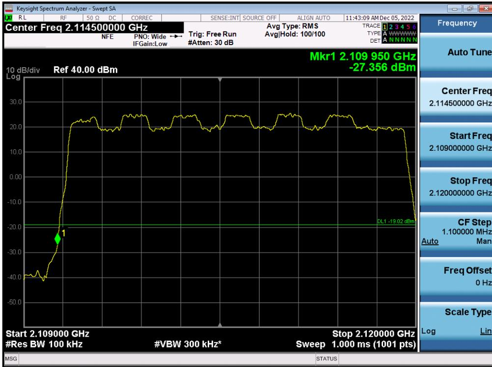
Antenna 3 / (4 Port) 5G NR n66 10 MHz 1 Carrier + 5G NR n66 10 MHz 1 Carrier + 5G NR n66 20 MHz 1 Carrier [3 Carrier] / 256QAM / High / Contiguous
