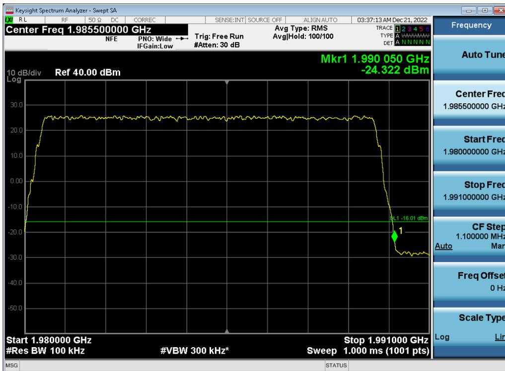
**Antenna 1 / (2 Port) LTE B2 5 MHz 1 Carrier + 5G NR n2 5 MHz 1 Carrier + DSS B2 20 MHz 1 Carrier [3 Carrier] [1C+2C] / 64QAM / Low / Non-Contiguous**
