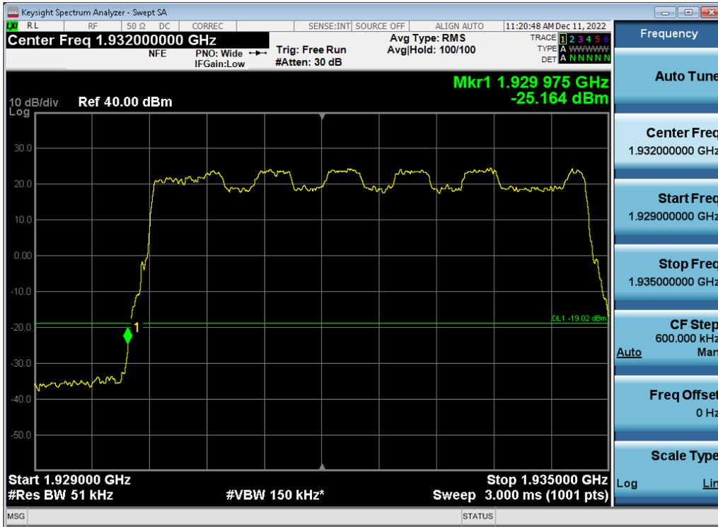
Antenna 2 / (4 Port) 5G NR n2 5 MHz 1 Carrier + 5G NR n2 5 MHz 1 Carrier + 5G NR n2 5 MHz 1 Carrier [3 Carrier] / 64QAM / High / Contiguous
