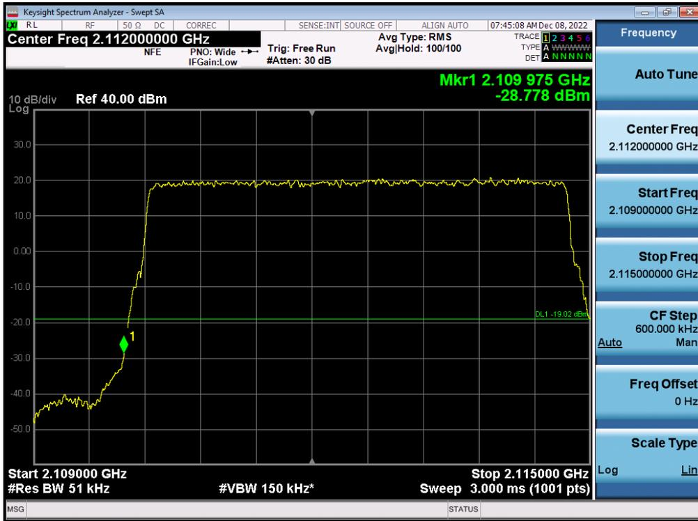
Antenna 0 / (4 Port) LTE B66 5 MHz 1 Carrier + 5G NR n66 5 MHz 1 Carrier + DSS B66 10 MHz 1 Carrier + DSS B66 20 MHz 1 Carrier [4 Carrier] / 256QAM / High / Contiguous
