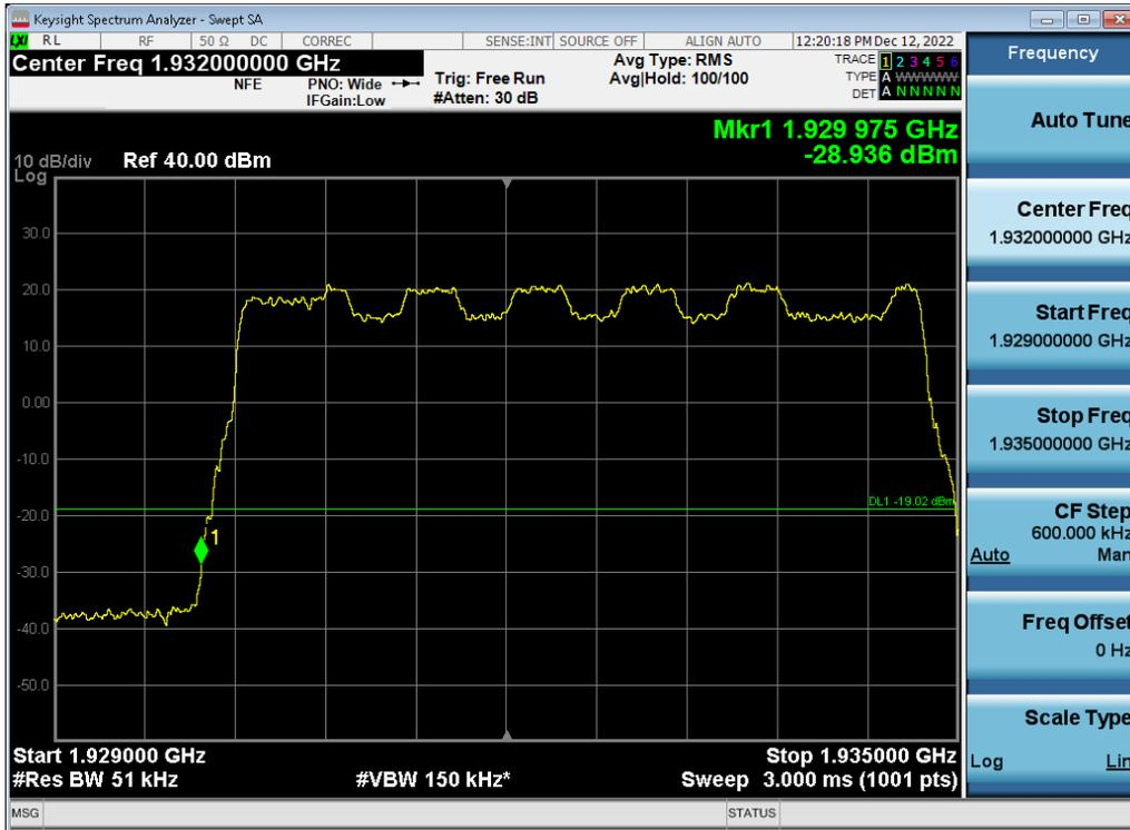
Antenna 2 / (4 Port) 5G NR n2 5 MHz 1 Carrier + 5G NR n2 5 MHz 1 Carrier + 5G NR n2 20 MHz 1 Carrier [3 Carrier] / 16QAM / High / Contiguous
