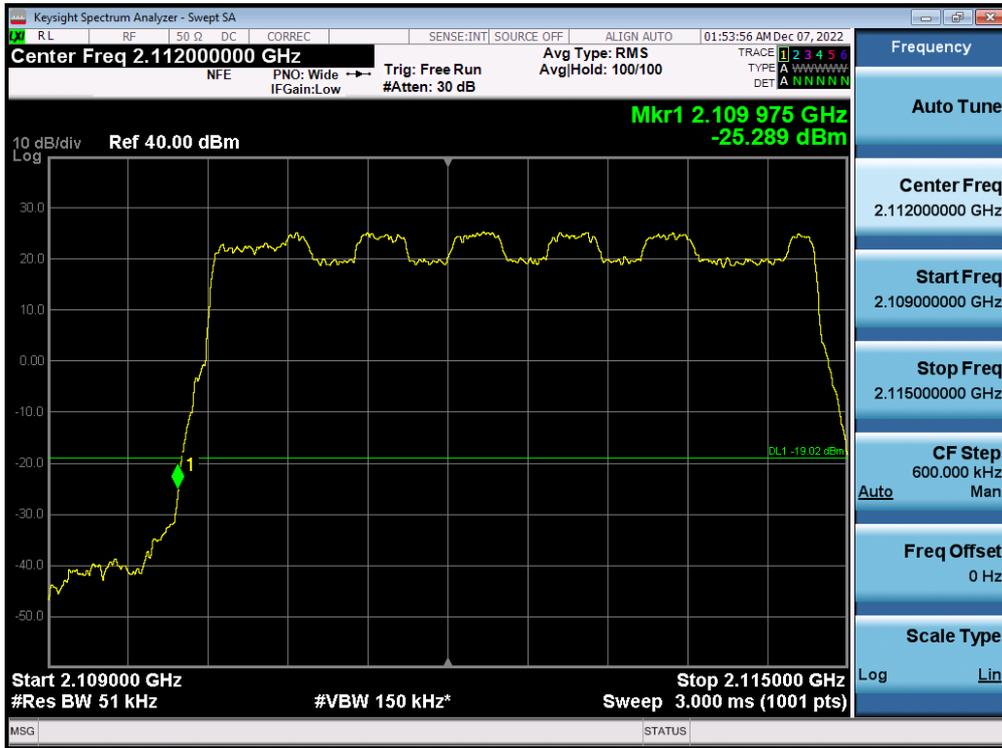
Antenna 1 / (4 Port) LTE B66 5 MHz 1 Carrier + 5G NR n66 5 MHz 1 Carrier + 5G NR n66 5 MHz 1 Carrier + 5G NR n66 5 MHz 1 Carrier [4 Carrier] / 64QAM / High / Contiguous
