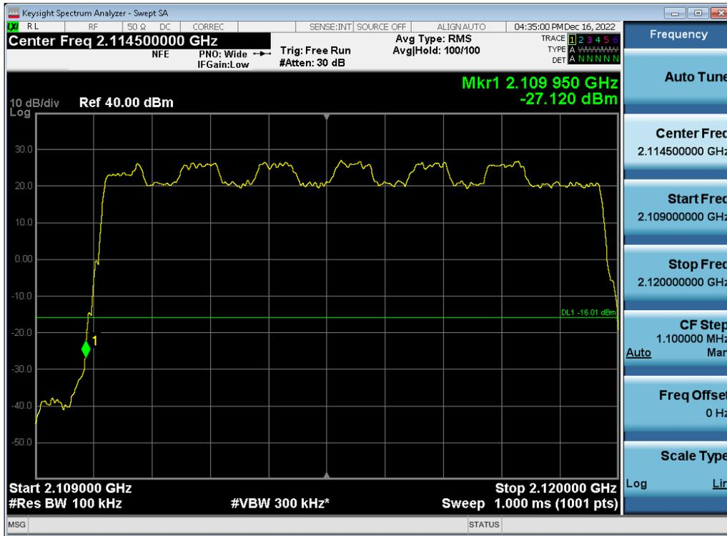
Antenna 1 / (2 Port) 5G NR n66 10 MHz 1 Carrier + 5G NR n66 10 MHz 1 Carrier + 5G NR n66 20 MHz 1 Carrier [3 Carrier]
