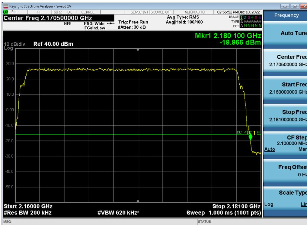
Antenna 1 / (2 Port) LTE B66 5 MHz 1 Carrier + 5G NR n66 5 MHz 1 Carrier + DSS B66 10 MHz 1 Carrier + DSS B66 20 MHz 1 Carrier [4 Carrier] [3C+1C] / QPSK / Low / Non-Contiguous
