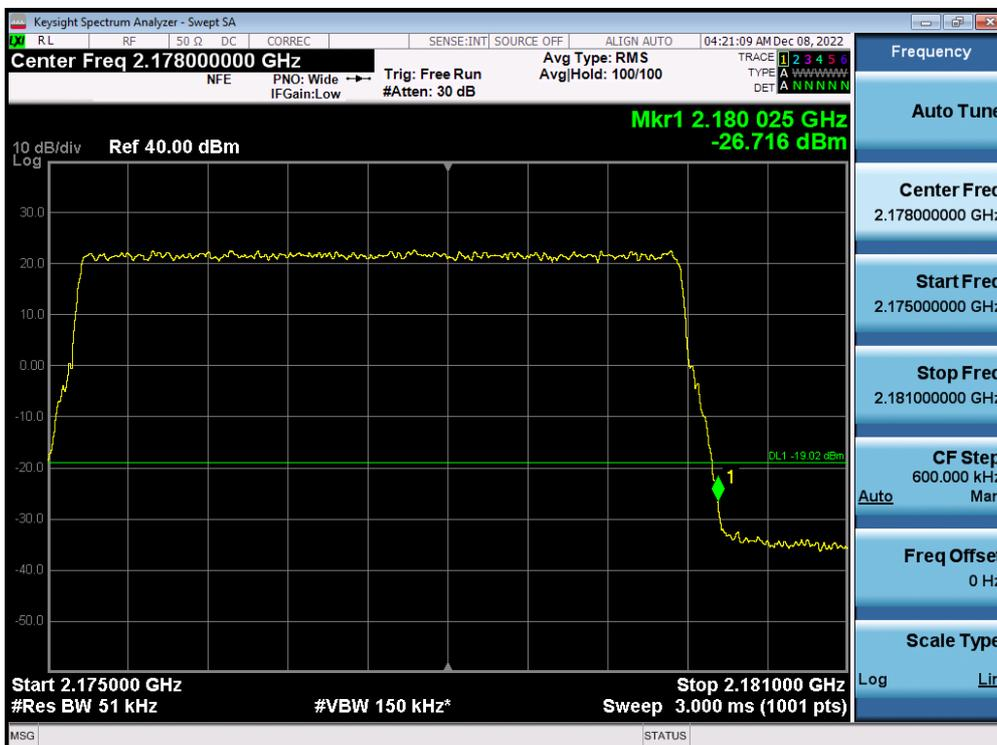
Antenna 0 / (4 Port) LTE B66 5 MHz 1 Carrier + 5G NR n66 5 MHz 1 Carrier + DSS B66 10 MHz 1 Carrier + DSS B66 20 MHz 1 Carrier [4 Carrier] / 64QAM / Low / Contiguous
