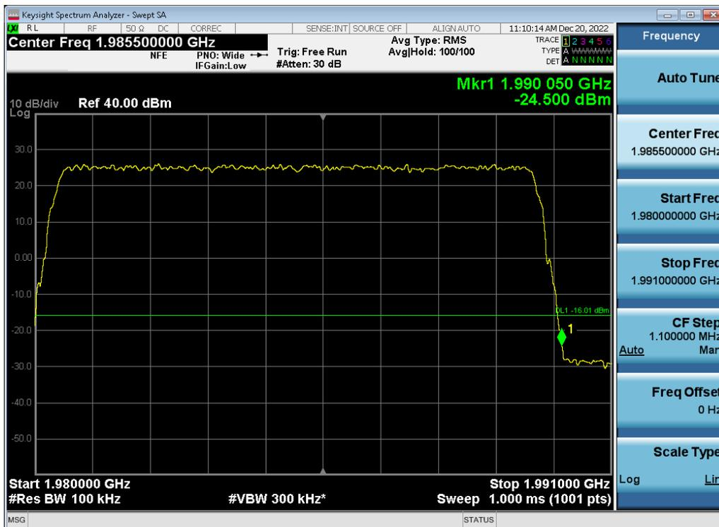
Antenna 0 / (2 Port) LTE B2 5 MHz 1 Carrier + 5G NR n2 5 MHz 1 Carrier + DSS B2 10 MHz 1 Carrier [3 Carrier] [1C+2C] / 64QAM / Low / Non-Contiguous
