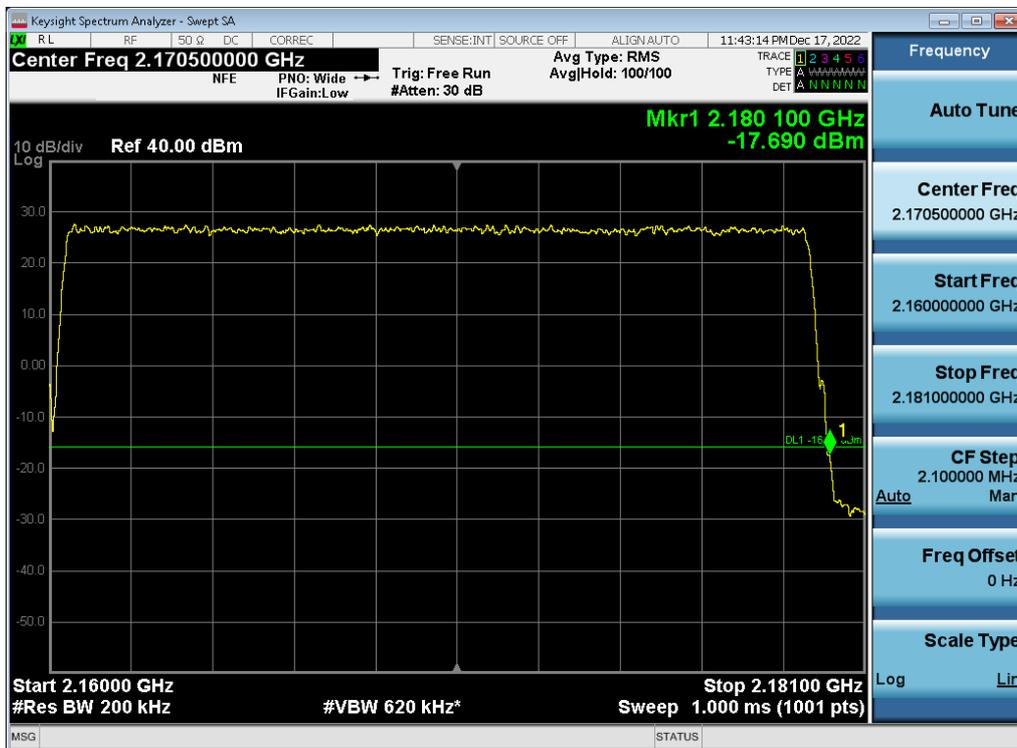
Antenna 0 / (2 Port) DSS B66 10 MHz 1 Carrier + 5G NR n66 10 MHz 1 Carrier + 5G NR n66 20 MHz 1 Carrier [3 Carrier]
