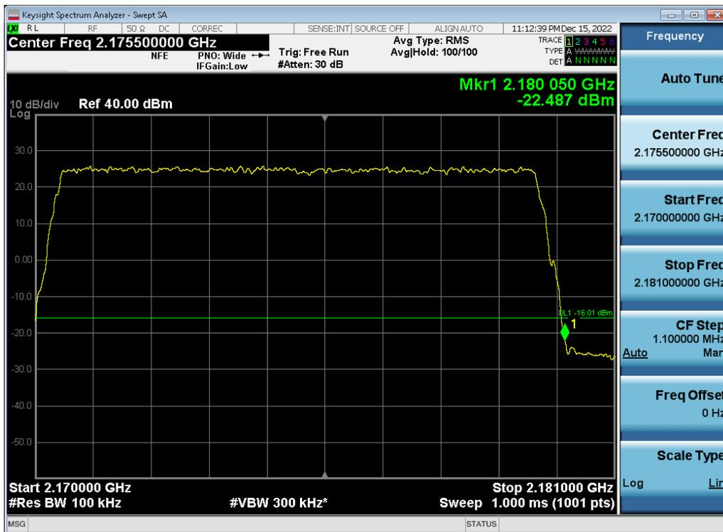
Antenna 0 / (2 Port) DSS B66 10 MHz 1 Carrier + DSS B66 10 MHz 1 Carrier + DSS B66 10 MHz 1 Carrier [3 Carrier]
