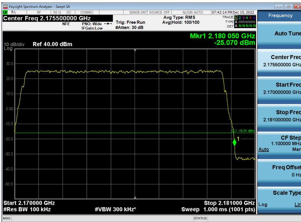
Antenna 1 / (2 Port) DSS B66 10 MHz 1 Carrier + DSS B66 10 MHz 1 Carrier + DSS B66 20 MHz 1 Carrier [3 Carrier] / 256QAM / Low / Contiguous
