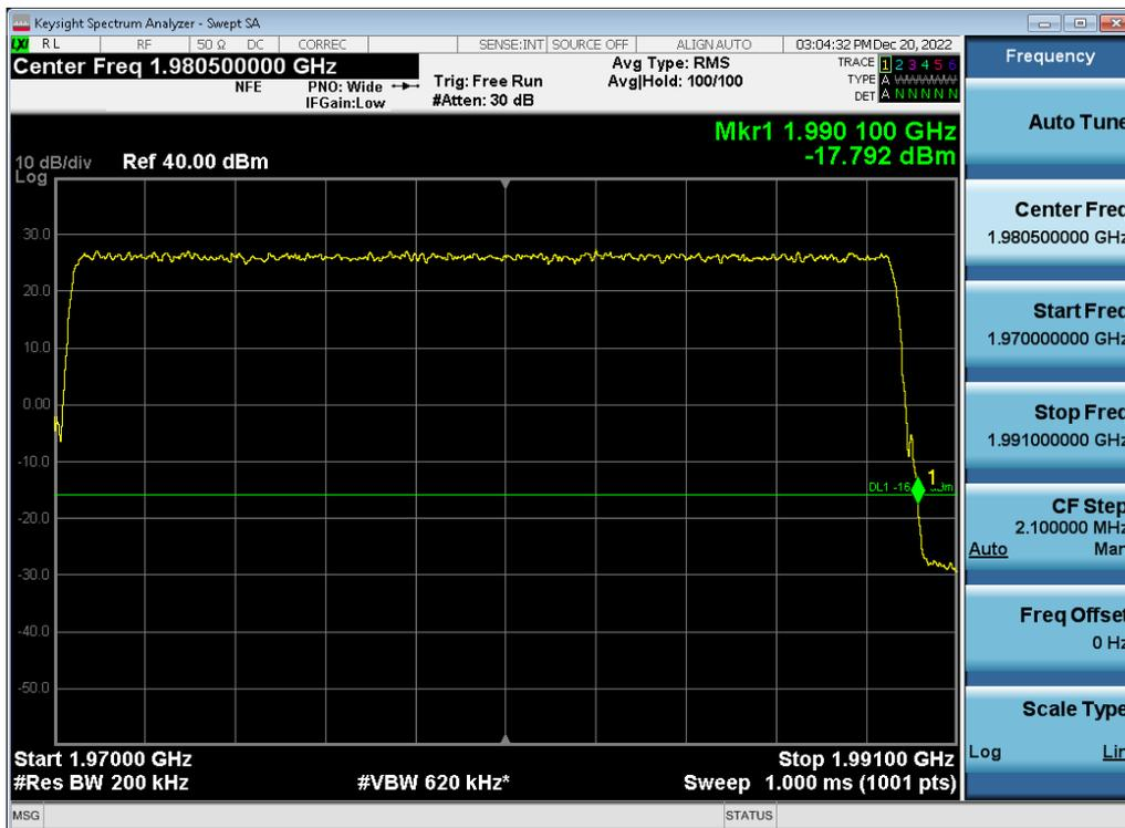
**Antenna 0 / (2 Port) 5G NR n2 5 MHz 1 Carrier + 5G NR n2 5 MHz 1 Carrier + 5G NR n2 20 MHz 1 Carrier [3 Carrier]
