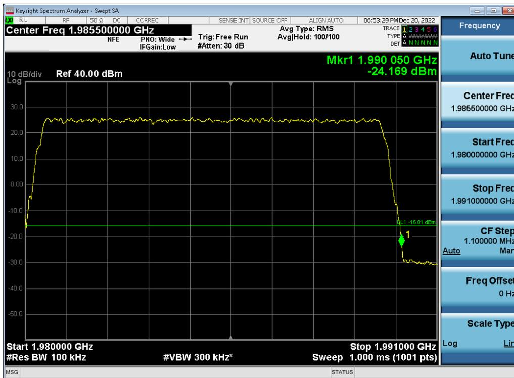
Antenna 0 / (2 Port) 5G NR n2 5 MHz 1 Carrier + 5G NR n2 5 MHz 1 Carrier + DSS B2 10 MHz 1 Carrier [3 Carrier] [2C+1C] / 16QAM / Low / Non-Contiguous
