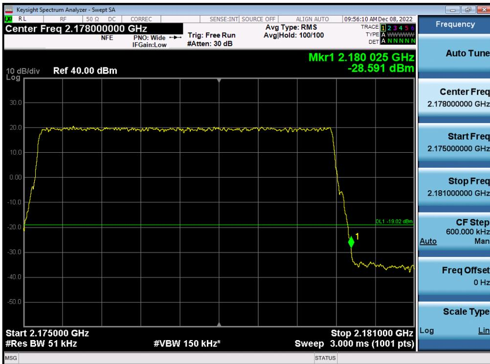
Antenna 1 / (4 Port) LTE B66 5 MHz 1 Carrier + LTE B66 5 MHz 1 Carrier + DSS B66 10 MHz 1 Carrier + DSS B66 10 MHz 1 Carrier [4 Carrier] / QPSK / Low / Contiguous
