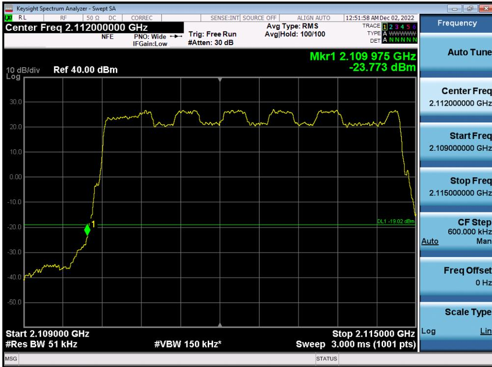
Antenna 3 / (4 Port) 5G NR n66 5 MHz 1 Carrier + 5G NR n66 5 MHz 1 Carrier + 5G NR n66 5 MHz 1 Carrier [3 Carrier] / QPSK / High / Contiguous
