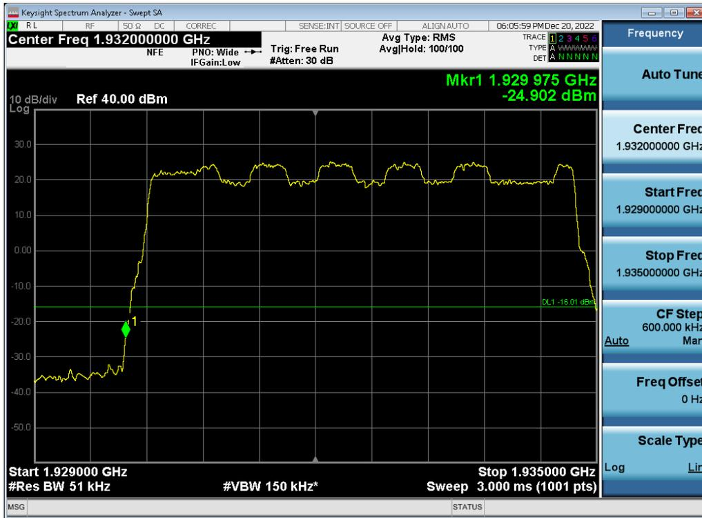
Antenna 1 / (2 Port) 5G NR n2 5 MHz 1 Carrier + 5G NR n2 5 MHz 1 Carrier + DSS B2 10 MHz 1 Carrier [3 Carrier] [2C+1C] / 256QAM / High / Non-Contiguous
