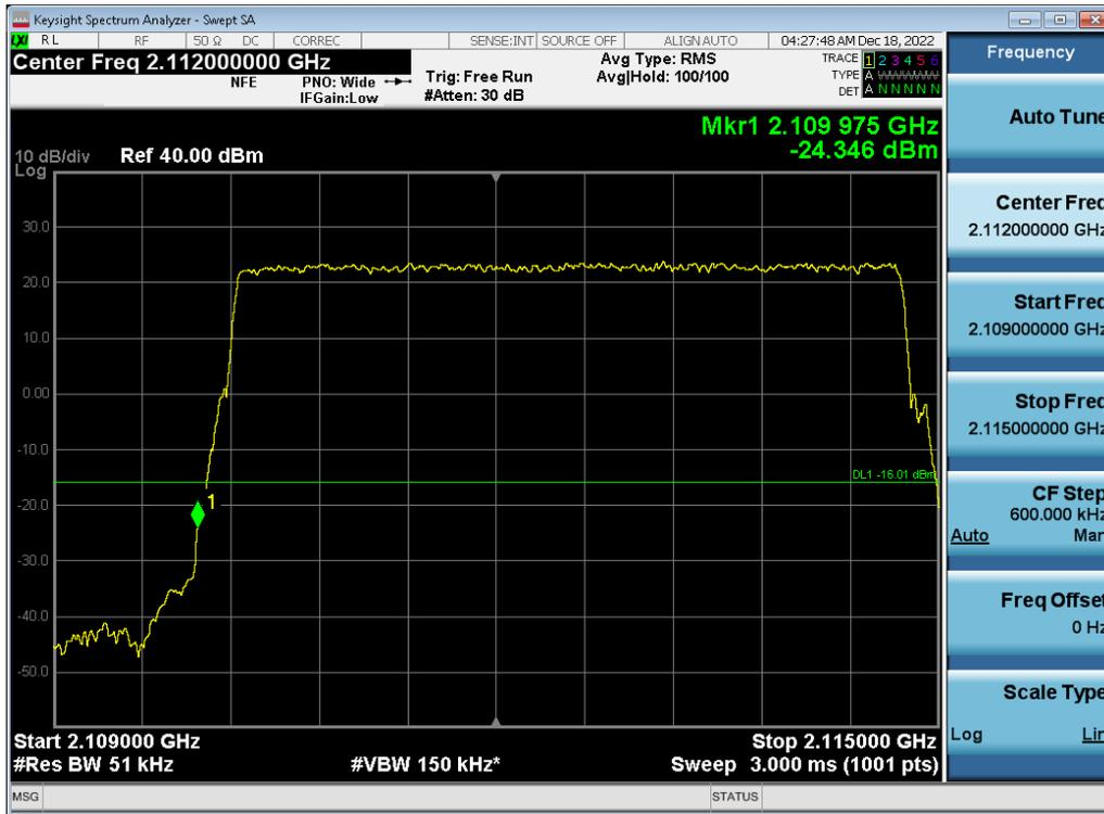
**Antenna 0 / (2 Port) LTE B66 5 MHz 1 Carrier + 5G NR n66 5 MHz 1 Carrier + 5G NR n66 5 MHz 1 Carrier + DSS B66 10 MHz 1 Carrier [4 Carrier] [1C+3C] / 64QAM / High / Non-Contiguous**
