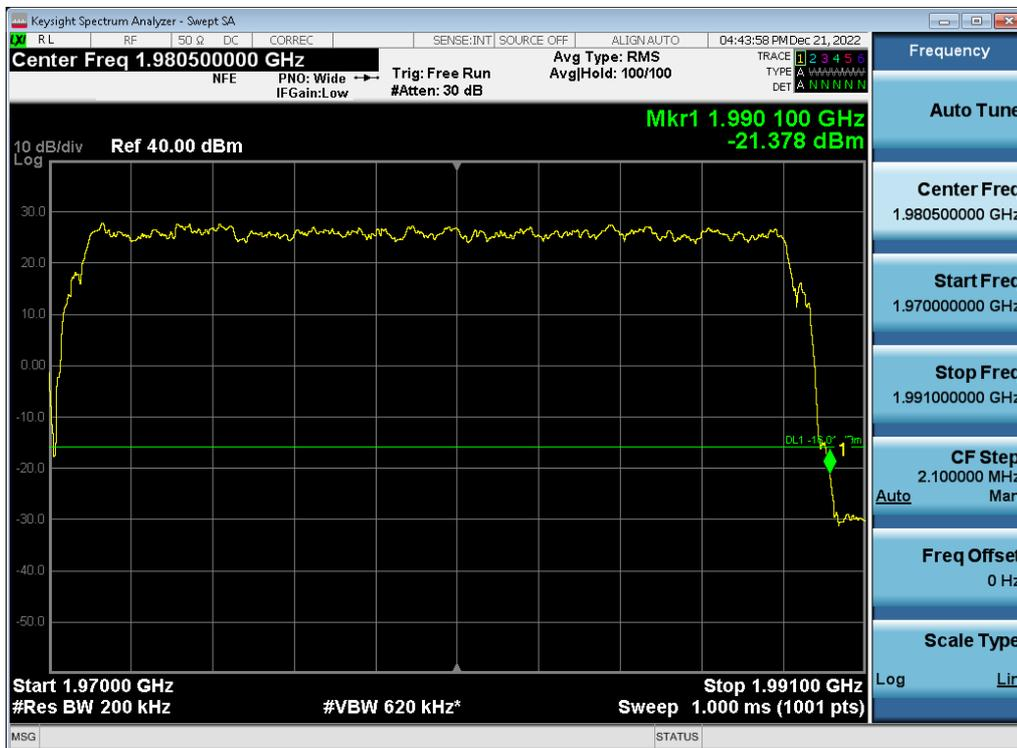
Antenna 1 / (2 Port) LTE B2 5 MHz 1 Carrier + 5G NR n2 5 MHz 1 Carrier + DSS B2 20 MHz 1 Carrier [3 Carrier] [2C+1C] / 256QAM / Low / Non-Contiguous
