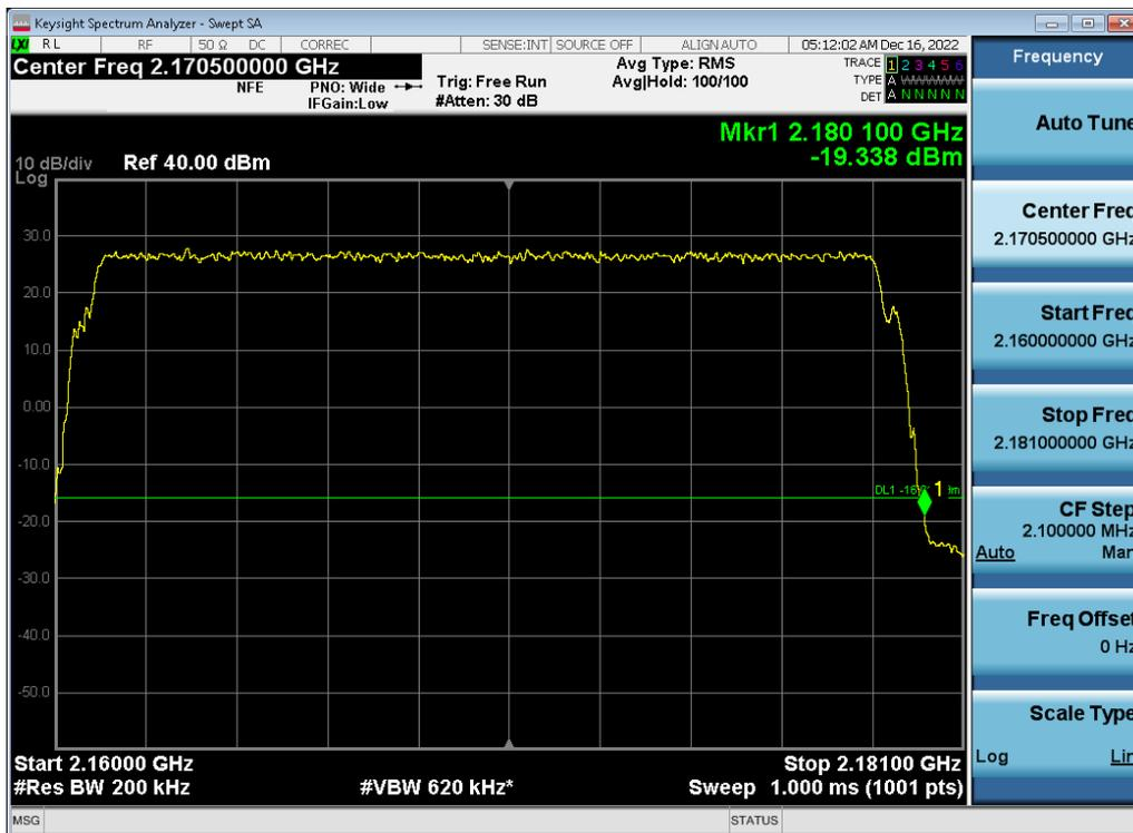
Antenna 1 / (2 Port) LTE B66 5 MHz 1 Carrier + 5G NR n66 5 MHz 1 Carrier + 5G NR n66 5 MHz 1 Carrier + 5G NR n66 5 MHz 1 Carrier [4 Carrier] [1C+3C] / QPSK / Low / Non-Contiguous
