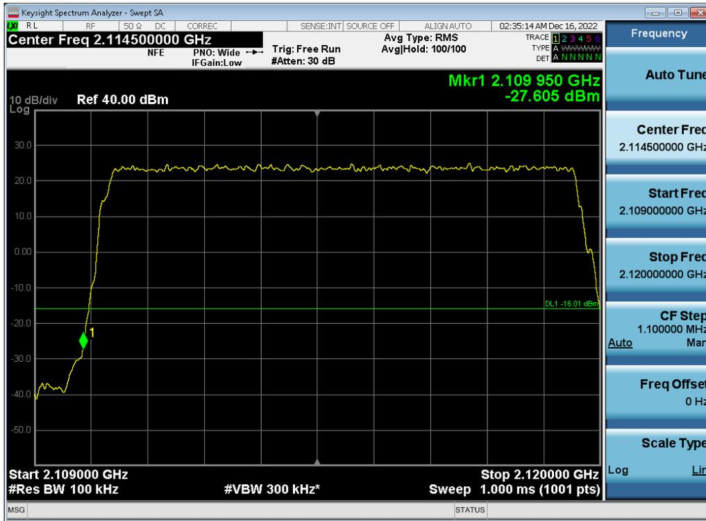
Antenna 1 / (2 Port) DSS B66 10 MHz 1 Carrier + DSS B66 10 MHz 1 Carrier + DSS B66 20 MHz 1 Carrier [3 Carrier] / 256QAM / High / Contiguous
