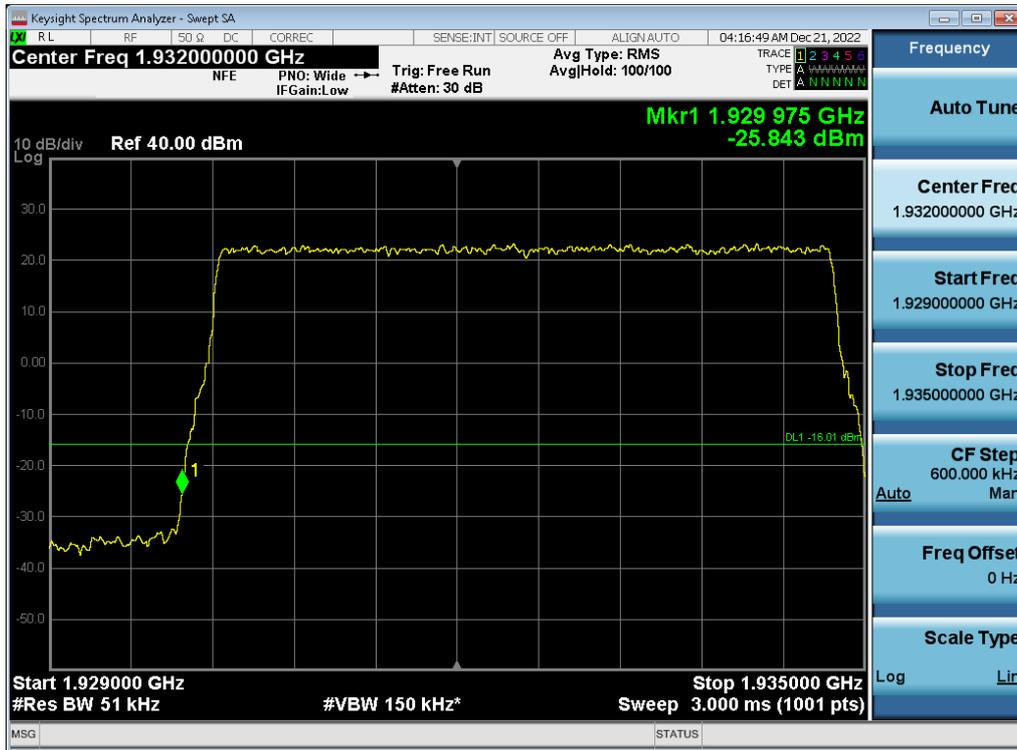
Antenna 1 / (2 Port) LTE B2 5 MHz 1 Carrier + 5G NR n2 5 MHz 1 Carrier + DSS B2 10 MHz 1 Carrier [3 Carrier] [1C+2C] / QPSK / High / Non-Contiguous
