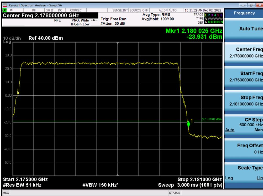
Antenna 1 / (4 Port) 5G NR n66 10 MHz 1 Carrier + 5G NR n66 10 MHz 1 Carrier + 5G NR n66 20 MHz 1 Carrier [3 Carrier] / 16QAM / Low / Contiguous
