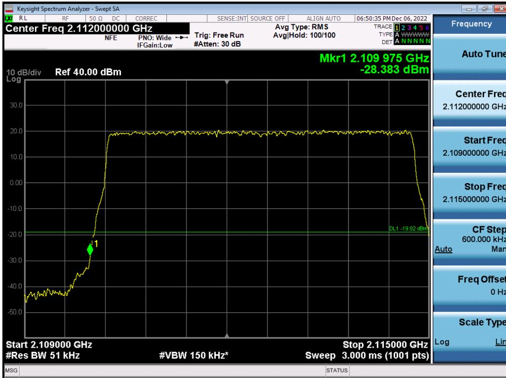
Antenna 1 / (4 Port) LTE B66 5 MHz 1 Carrier + LTE B66 5 MHz 1 Carrier + DSS B66 10 MHz 1 Carrier + DSS B66 20 MHz 1 Carrier [4 Carrier] / 256QAM / High / Contiguous
