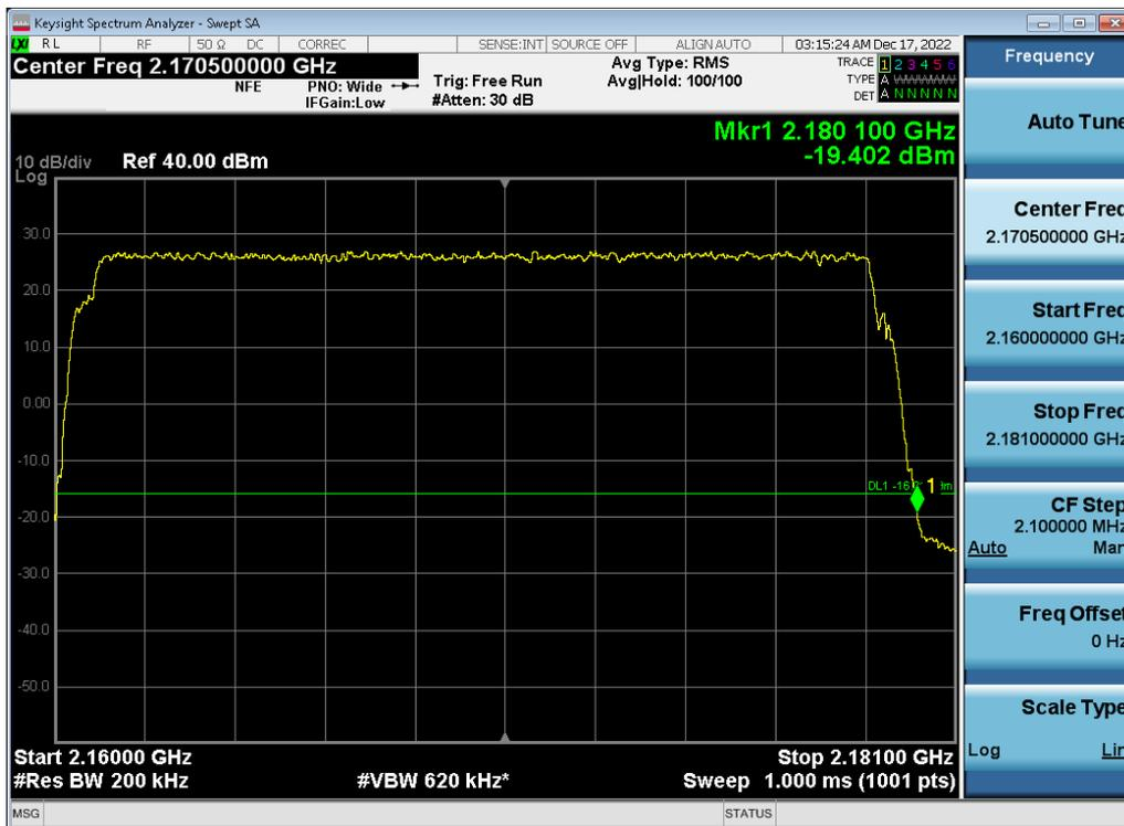
Antenna 3 / (4 Port) DSS B2 10 MHz 1 Carrier + DSS B2 10 MHz 1 Carrier [2 Carrier] / 16QAM / Low / Non-Contiguous
