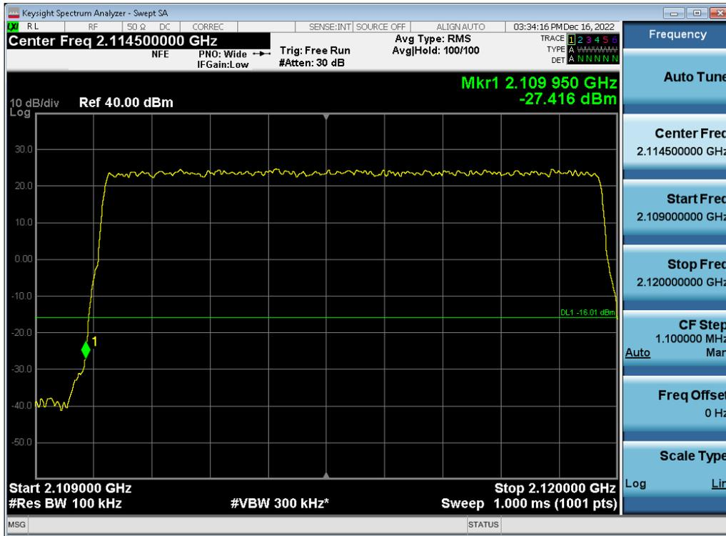
Antenna 0 / (2 Port) 5G NR n66 10 MHz 1 Carrier + 5G NR n66 10 MHz 1 Carrier + 5G NR n66 20 MHz 1 Carrier [3 Carrier]
