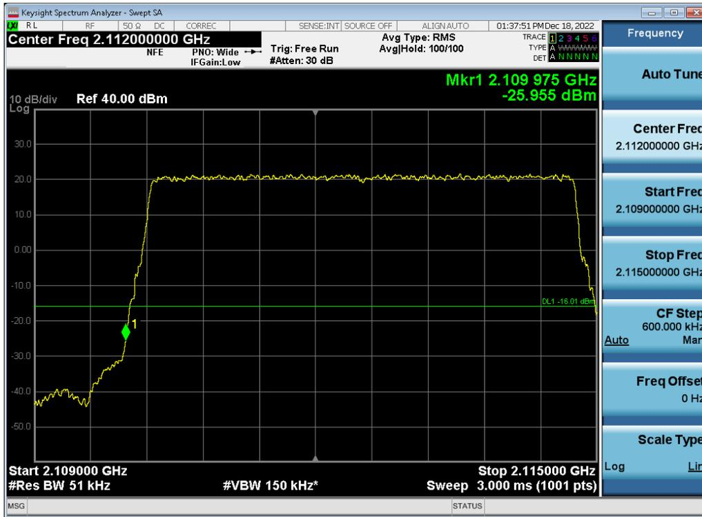
Antenna 1 / (2 Port) LTE B66 5 MHz 1 Carrier + 5G NR n66 5 MHz 1 Carrier + DSS B66 10 MHz 1 Carrier + DSS B66 20 MHz 1 Carrier [4 Carrier] [3C+1C] / 16QAM / High / Non-Contiguous
