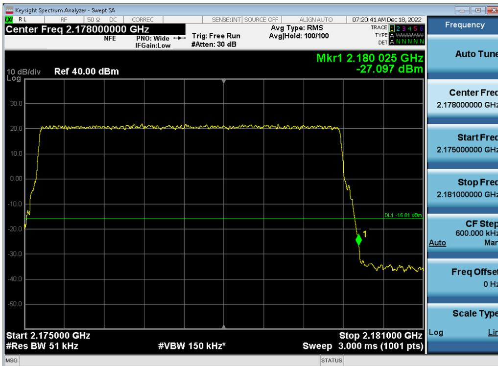
Antenna 1 / (2 Port) LTE B66 5 MHz 1 Carrier + LTE B66 5 MHz 1 Carrier + DSS B66 10 MHz 1 Carrier + DSS B66 10 MHz 1 Carrier [4 Carrier] / 16QAM / Low / Contiguous
