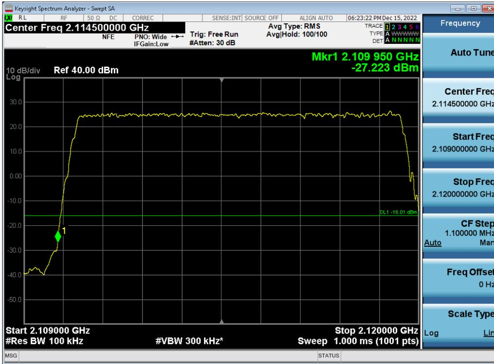
Antenna 1 / (2 Port) DSS B66 10 MHz 1 Carrier + DSS B66 10 MHz 1 Carrier + DSS B66 10 MHz 1 Carrier [3 Carrier] / QPSK / High / Contiguous
