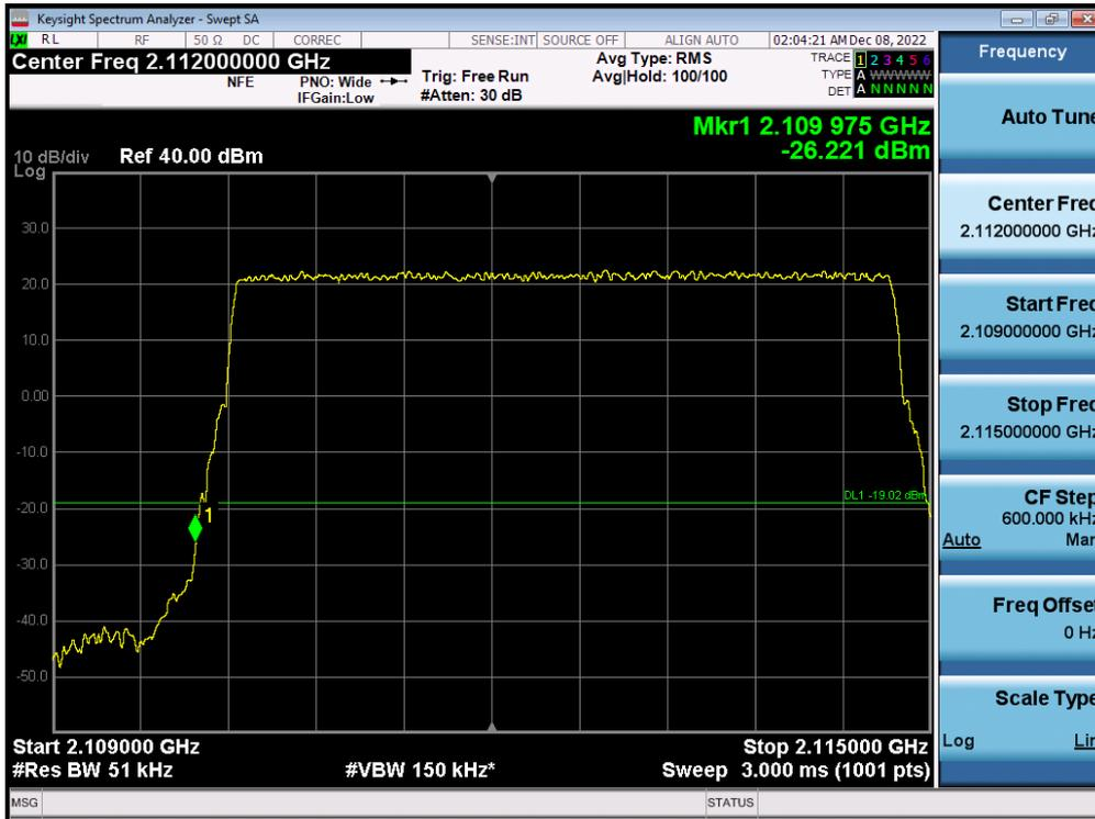
Antenna 0 / (4 Port) LTE B66 5 MHz 1 Carrier + 5G NR n66 5 MHz 1 Carrier + 5G NR n66 5 MHz 1 Carrier + DSS B66 10 MHz 1 Carrier [4 Carrier] / 64QAM / High / Contiguous
