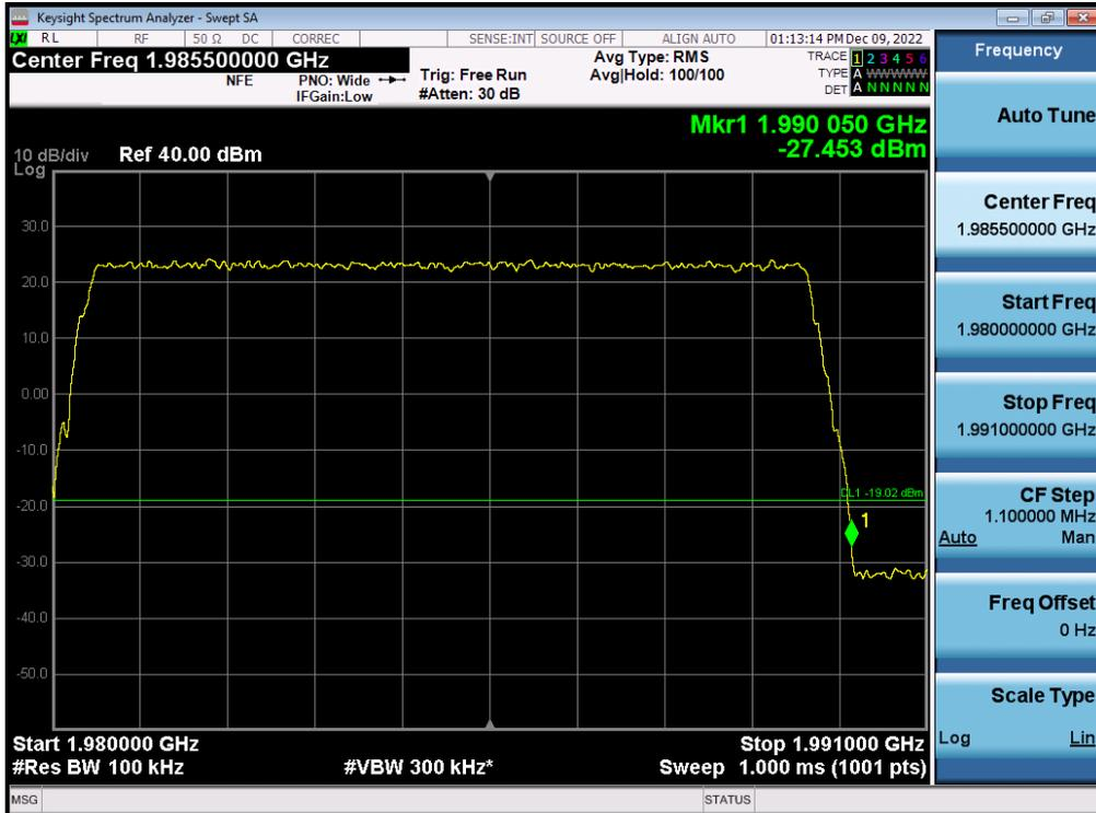
Antenna 3 / (4 Port) LTE B2 5 MHz 1 Carrier + 5G NR n2 5 MHz 1 Carrier + DSS B2 10 MHz 1 Carrier [3 Carrier] / QPSK / Low / Contiguous
