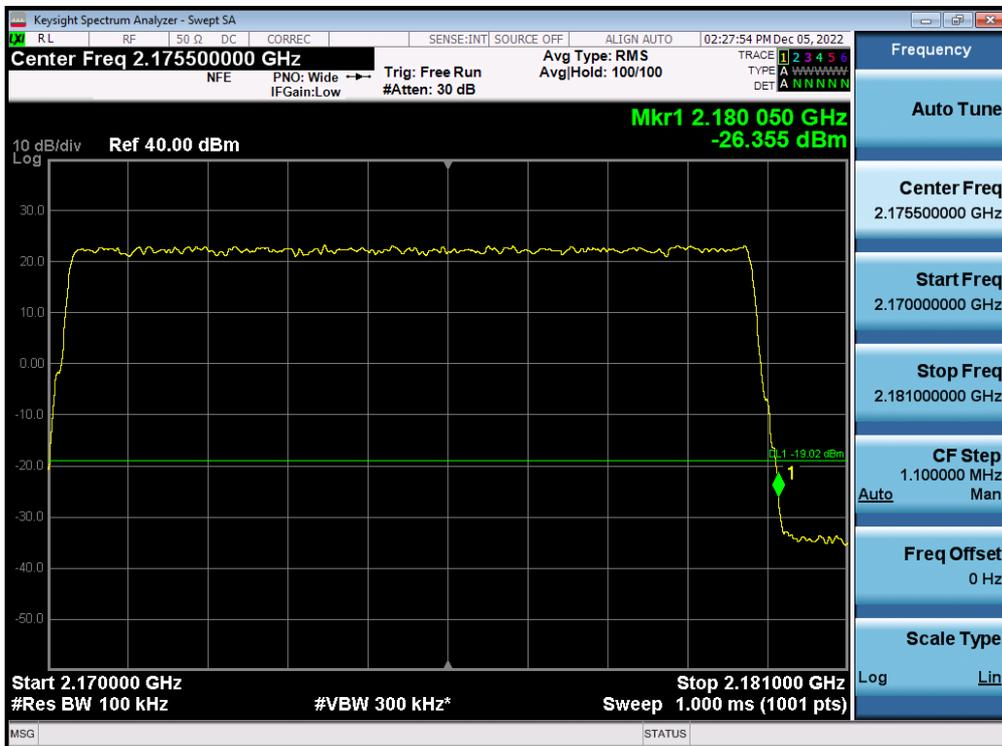
Antenna 0 / (4 Port) 5G NR n66 5 MHz 1 Carrier + 5G NR n66 5 MHz 1 Carrier + DSS B66 10 MHz 1 Carrier [3 Carrier] / 256QAM / Low / Contiguous
