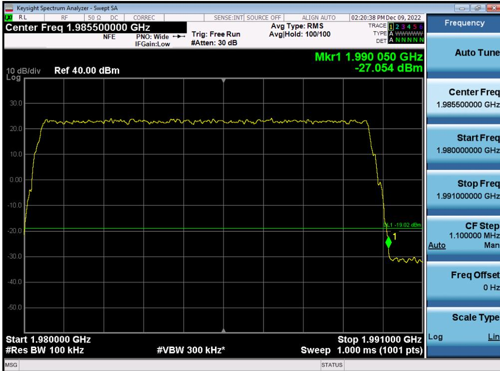
Antenna 3 / (4 Port) LTE B2 5 MHz 1 Carrier + 5G NR n2 5 MHz 1 Carrier + DSS B2 10 MHz 1 Carrier [3 Carrier] [1C+2C] / 256QAM / Low / Non-Contiguous
