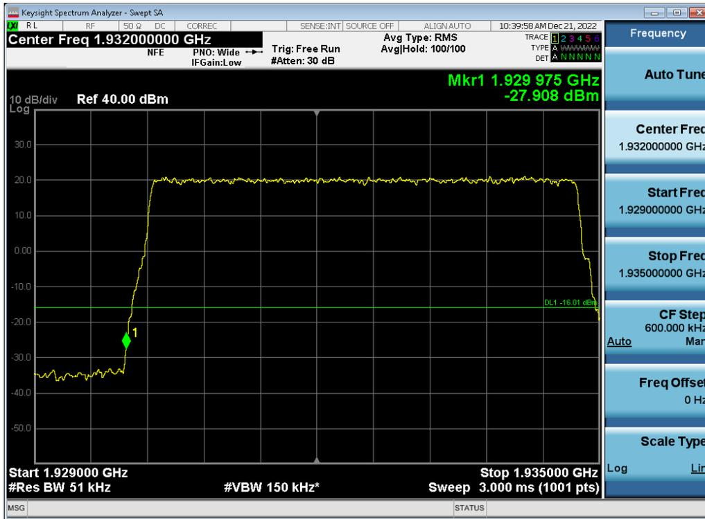
Antenna 1 / (2 Port) LTE B2 5 MHz 1 Carrier + 5G NR n2 5 MHz 1 Carrier + DSS B2 20 MHz 1 Carrier [3 Carrier] [2C+1C] / QPSK / High / Non-Contiguous
