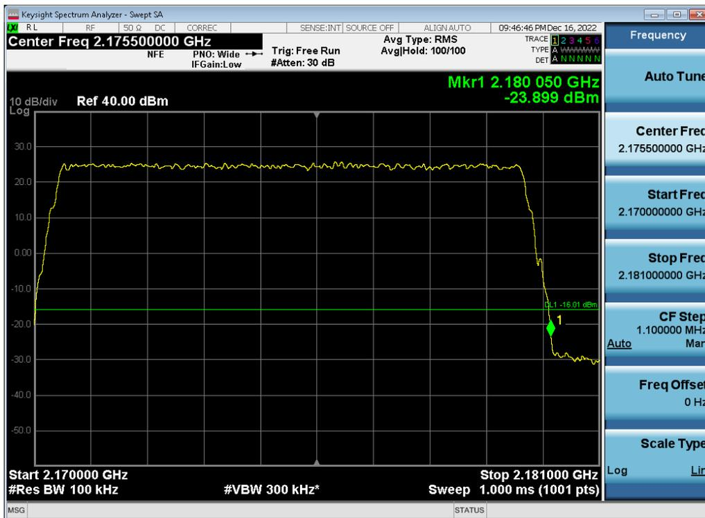
**Antenna 1 / (2 Port) LTE B66 5 MHz 1 Carrier + LTE B66 5 MHz 1 Carrier + DSS B66 10 MHz 1 Carrier + DSS B66 20 MHz 1 Carrier [4 Carrier] [1C+3C] / 64QAM / Low / Non-Contiguous**
