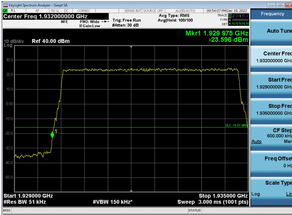
Antenna 1 / (2 Port) 5G NR n2 5 MHz 1 Carrier + 5G NR n2 5 MHz 1 Carrier + 5G NR n2 5 MHz 1 Carrier [3 Carrier] [2C+1C]
