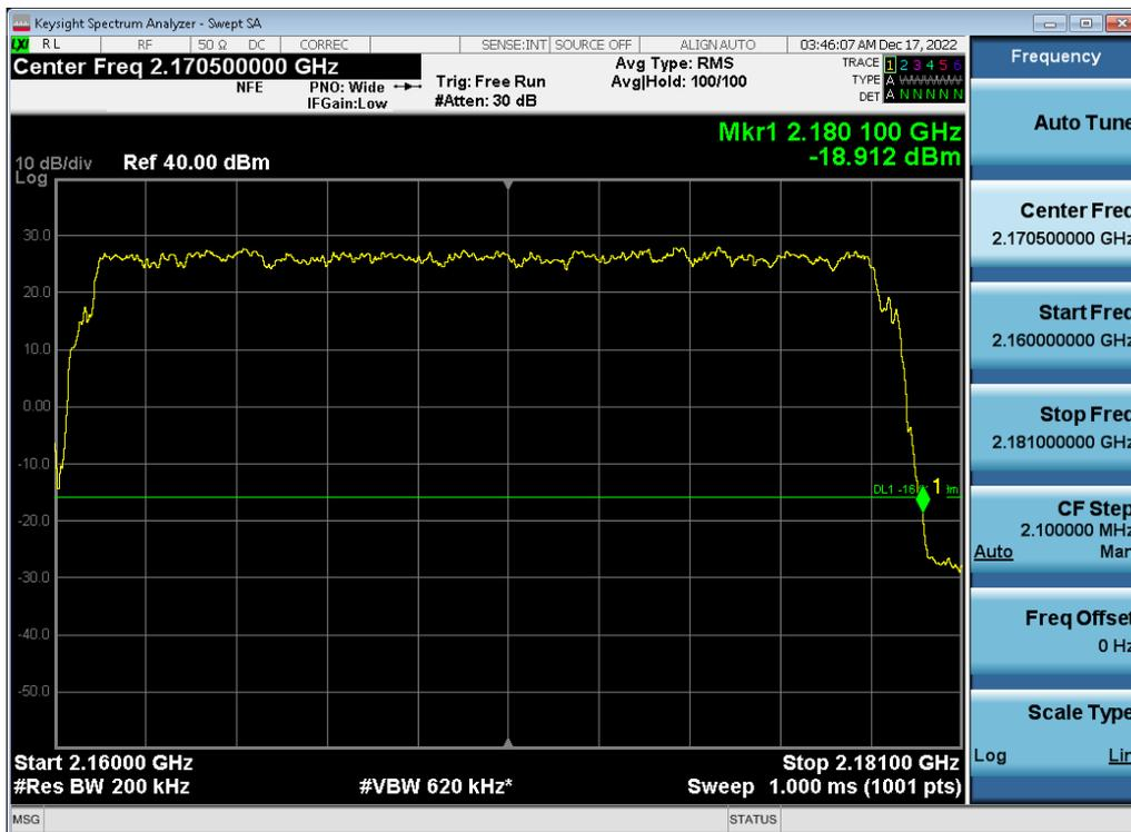
Antenna 1 / (2 Port) LTE B66 5 MHz 1 Carrier + LTE B66 5 MHz 1 Carrier + DSS B66 10 MHz 1 Carrier + DSS B66 20 MHz 1 Carrier [4 Carrier] [3C+1C] / 64QAM / Low / Non-Contiguous
