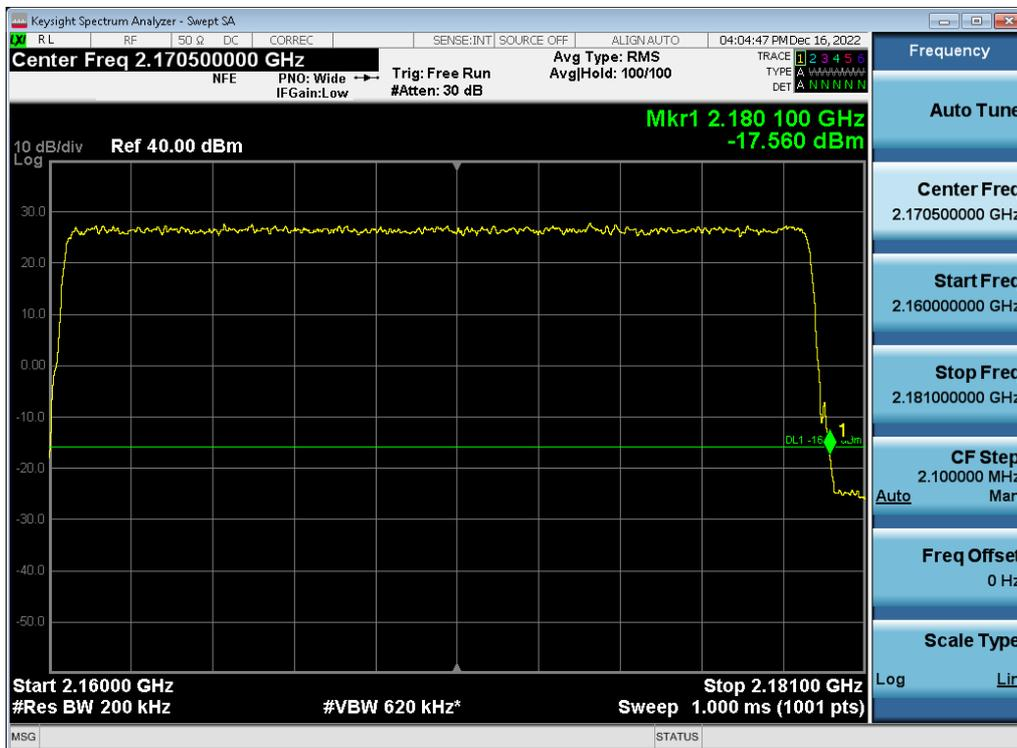
Antenna 0 / (2 Port) 5G NR n66 5 MHz 1 Carrier + 5G NR n66 5 MHz 1 Carrier + DSS B66 10 MHz 1 Carrier [3 Carrier]
