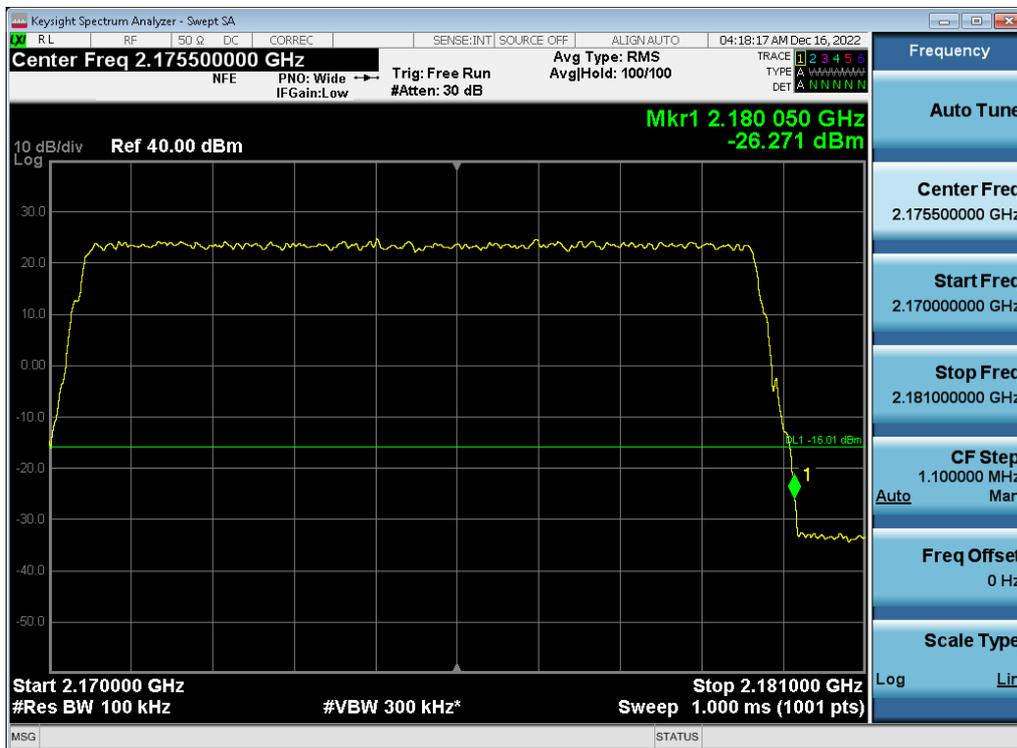
Antenna 1 / (2 Port) LTE B66 5 MHz 1 Carrier + 5G NR n66 5 MHz 1 Carrier + 5G NR n66 5 MHz 1 Carrier + 5G NR n66 5 MHz 1 Carrier [4 Carrier] / 16QAM / Low / Contiguous
