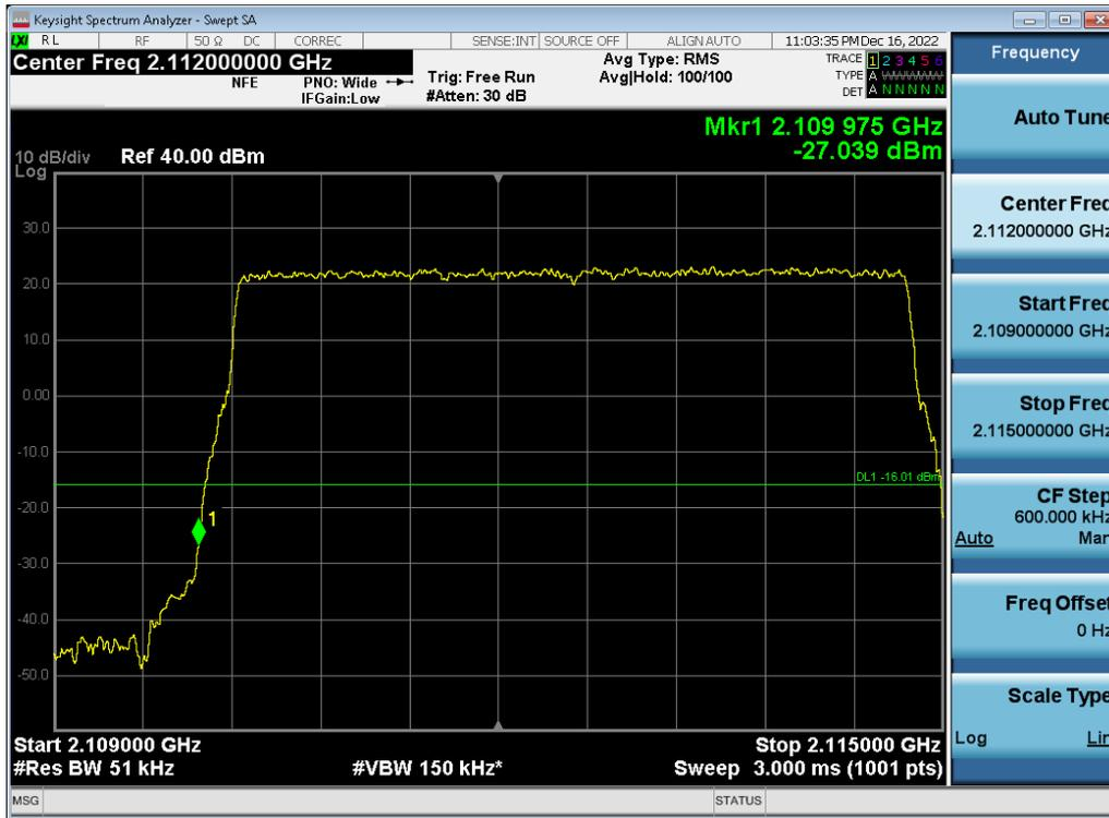
**Antenna 0 / (2 Port) LTE B66 5 MHz 1 Carrier + LTE B66 5 MHz 1 Carrier + DSS B66 10 MHz 1 Carrier + DSS B66 10 MHz 1 Carrier [4 Carrier] [1C+3C] / 256QAM / High / Non-Contiguous**
