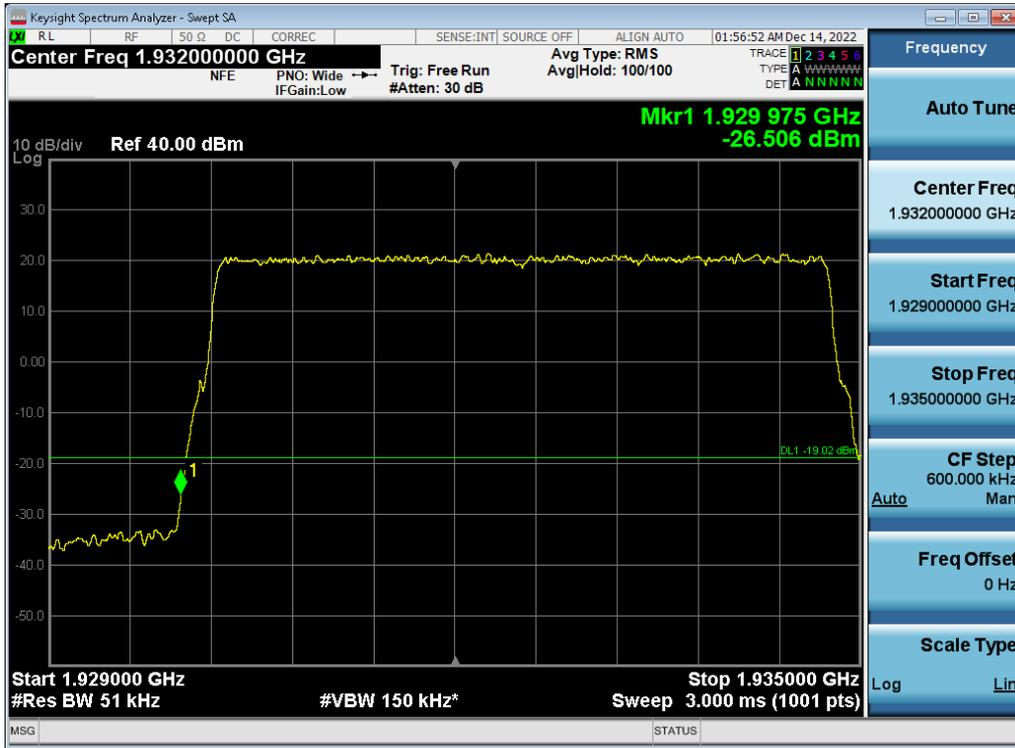
Antenna 0 / (4 Port) LTE B2 5 MHz 1 Carrier + 5G NR n2 5 MHz 1 Carrier + DSS B2 10 MHz 1 Carrier [3 Carrier] [2C+1C] / 64QAM / High / Non-Contiguous
