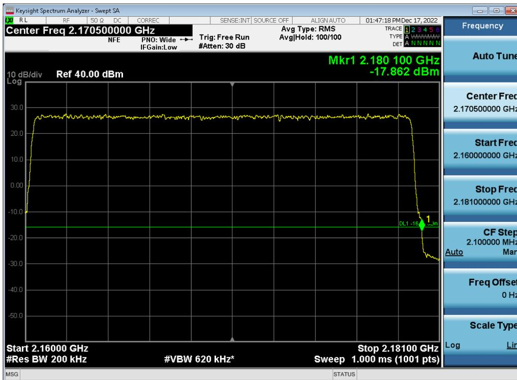
**Antenna 1 / (2 Port) LTE B66 5 MHz 1 Carrier + 5G NR n66 5 MHz 1 Carrier + 5G NR n66 10 MHz 1 Carrier + 5G NR n66 20 MHz 1 Carrier [4 Carrier] [3C+1C] / 64QAM / Low / Non-Contiguous**
