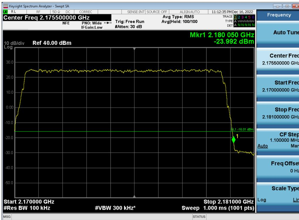
**Antenna 0 / (2 Port) LTE B66 5 MHz 1 Carrier + LTE B66 5 MHz 1 Carrier + DSS B66 10 MHz 1 Carrier + DSS B66 10 MHz 1 Carrier [4 Carrier] [3C+1C] / 64QAM / Low / Non-Contiguous**
