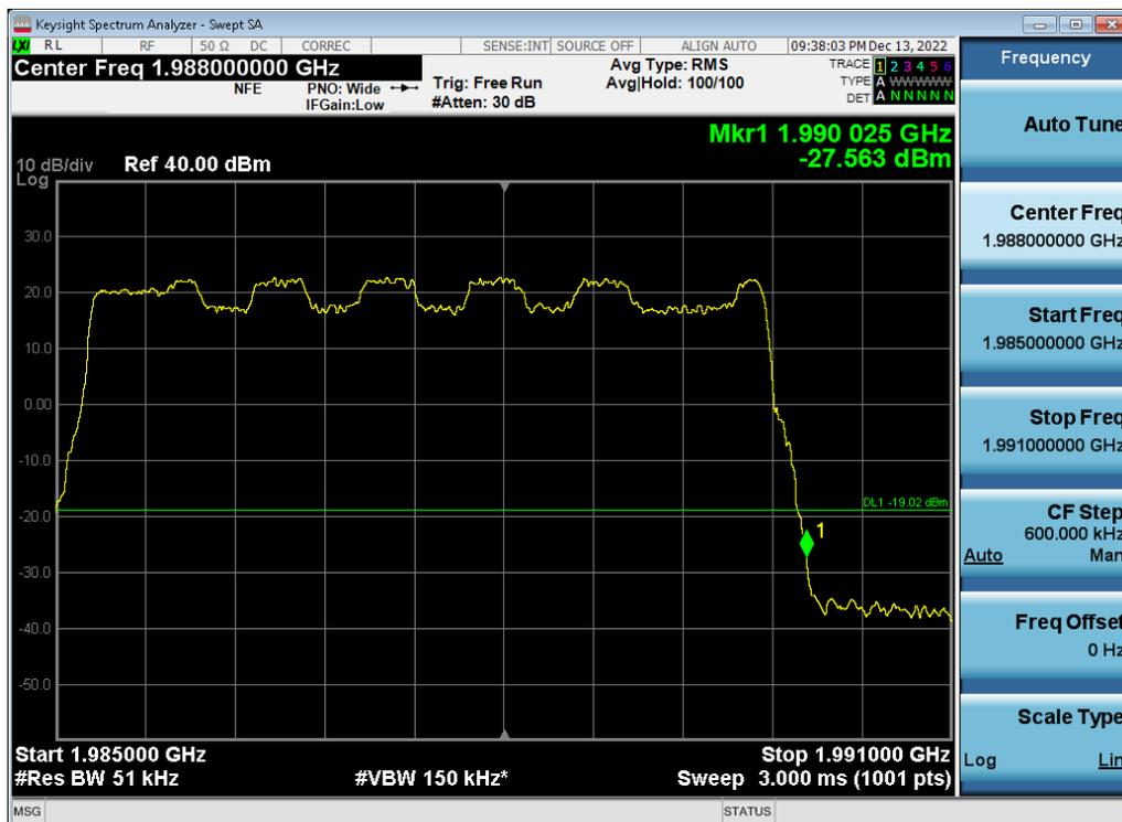
Antenna 3 / (4 Port) LTE B2 5 MHz 1 Carrier + 5G NR n2 5 MHz 1 Carrier + DSS B2 20 MHz 1 Carrier [3 Carrier] / 16QAM / Low / Contiguous
