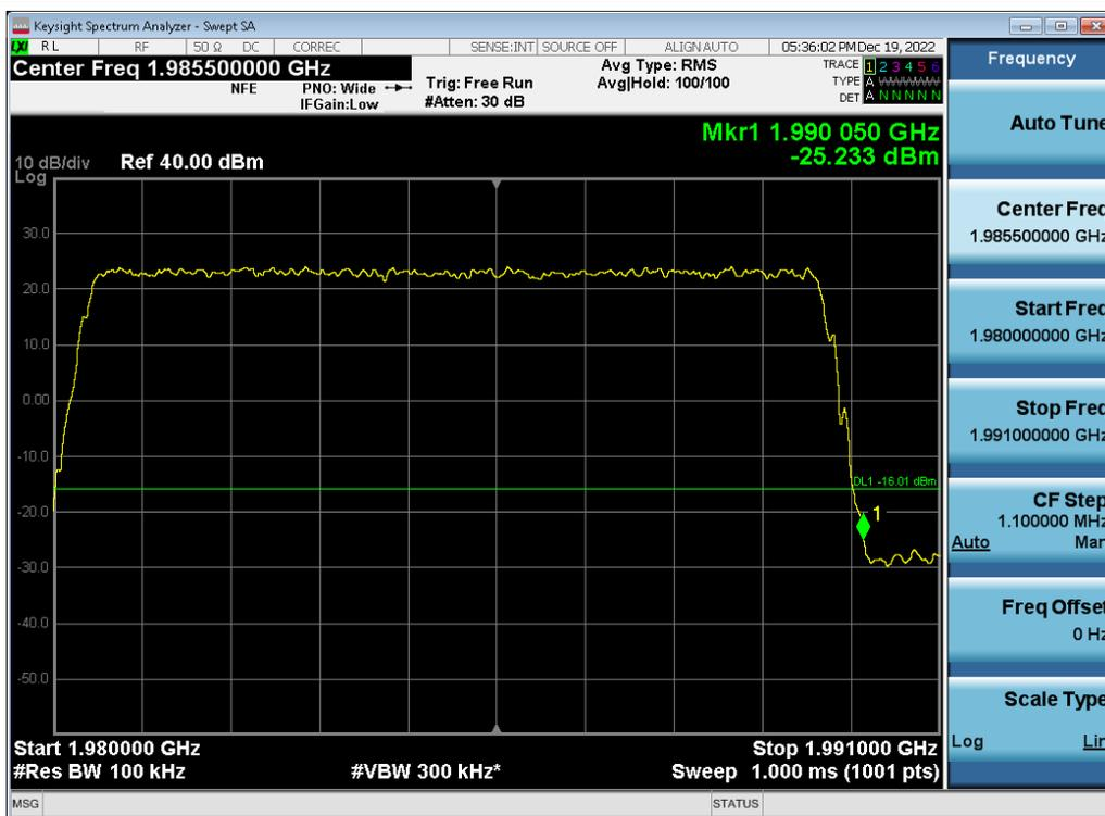
Antenna 1 / (2 Port) 5G NR n66 5 MHz 1 Carrier + 5G NR n66 5 MHz 1 Carrier + 5G NR n66 5 MHz 1 Carrier [3 Carrier]
