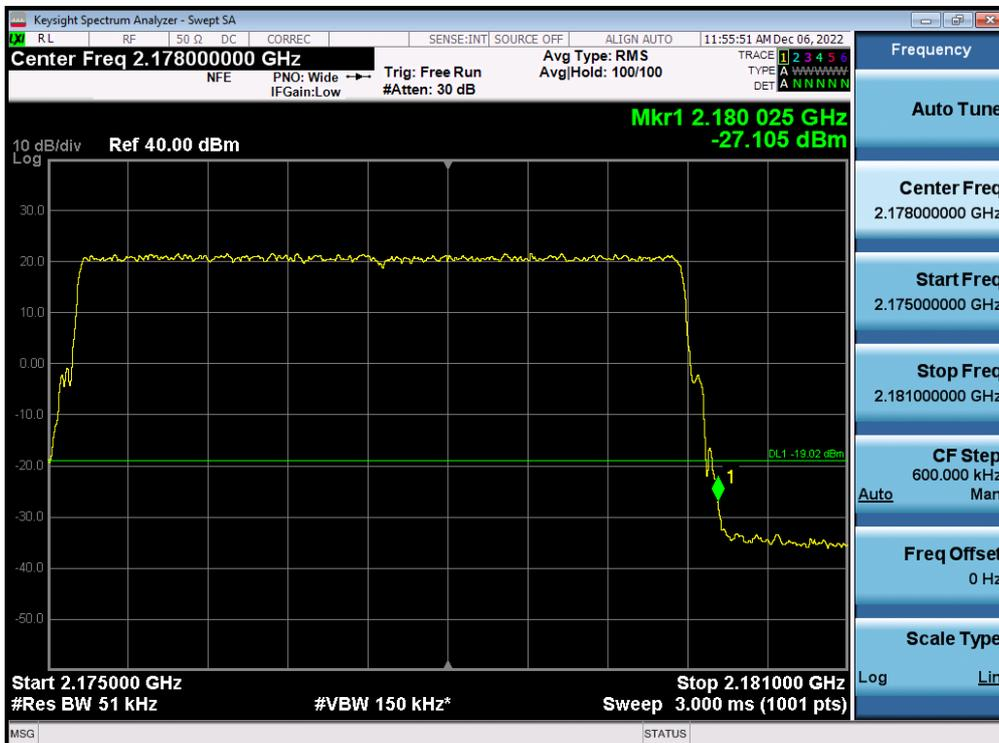
Antenna 1 / (4 Port) LTE B66 5 MHz 1 Carrier + LTE B66 5 MHz 1 Carrier + DSS B66 10 MHz 1 Carrier + DSS B66 20 MHz 1 Carrier [4 Carrier] / 64QAM / Low / Contiguous
