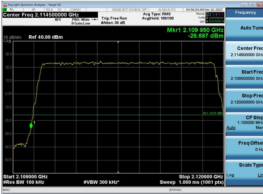
Antenna 1 / (2 Port) DSS B66 10 MHz 1 Carrier + DSS B66 10 MHz 1 Carrier + DSS B66 20 MHz 1 Carrier [3 Carrier]
