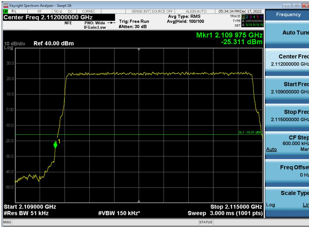
Antenna 1 / (2 Port) 5G NR n66 5 MHz 1 Carrier + 5G NR n66 5 MHz 1 Carrier + DSS B66 10 MHz 1 Carrier [3 Carrier]
