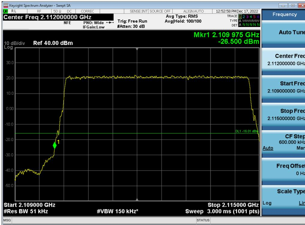
**Antenna 0 / (2 Port) LTE B66 5 MHz 1 Carrier + 5G NR n66 5 MHz 1 Carrier + 5G NR n66 10 MHz 1 Carrier + 5G NR n66 20 MHz 1 Carrier [4 Carrier] [3C+1C] / QPSK / High / Non-Contiguous**
