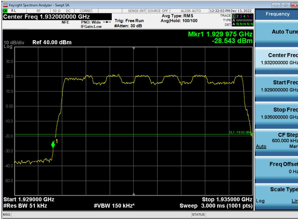
Antenna 2 / (4 Port) 5G NR n2 5 MHz 1 Carrier + 5G NR n2 5 MHz 1 Carrier + DSS B2 20 MHz 1 Carrier [3 Carrier] / 16QAM / High / Contiguous
