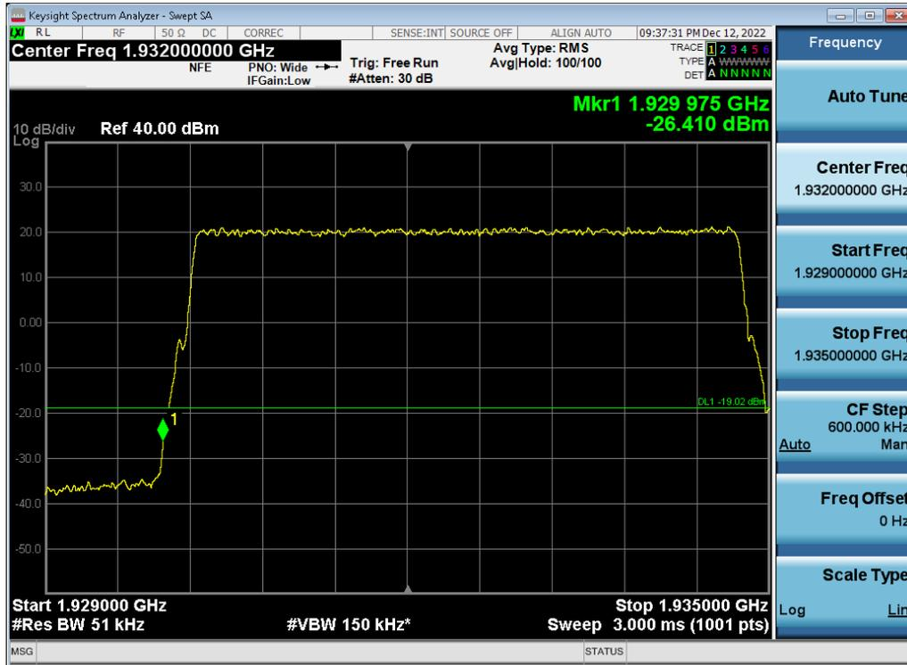
Antenna 0 / (4 Port) 5G NR n2 5 MHz 1 Carrier + 5G NR n2 5 MHz 1 Carrier + DSS B2 10 MHz 1 Carrier [3 Carrier] / 256QAM / High / Contiguous
