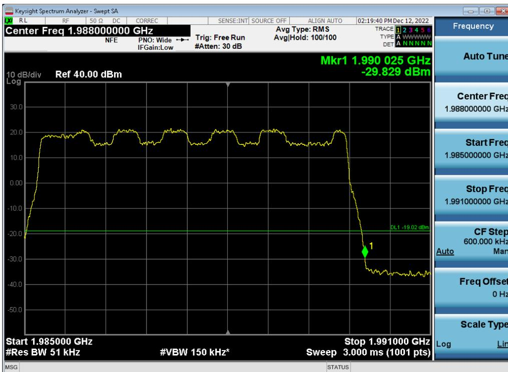
Antenna 2 / (4 Port) 5G NR n2 5 MHz 1 Carrier + 5G NR n2 5 MHz 1 Carrier + DSS B2 10 MHz 1 Carrier [3 Carrier] / 64QAM / Low / Contiguous
