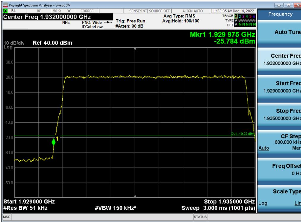
Antenna 3 / (4 Port) LTE B2 5 MHz 1 Carrier + 5G NR n2 5 MHz 1 Carrier + DSS B2 10 MHz 1 Carrier [3 Carrier] [1C+2C] / 64QAM / High / Non-Contiguous
