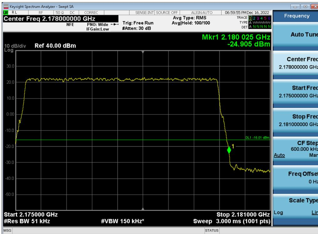
Antenna 0 / (2 Port) LTE B66 5 MHz 1 Carrier + LTE B66 5 MHz 1 Carrier + DSS B66 10 MHz 1 Carrier + DSS B66 20 MHz 1 Carrier [4 Carrier] / QPSK / Low / Contiguous
