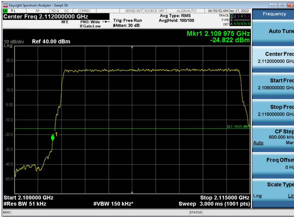
Antenna 0 / (2 Port) LTE B66 5 MHz 1 Carrier + 5G NR n66 5 MHz 1 Carrier + 5G NR n66 5 MHz 1 Carrier + 5G NR n66 5 MHz 1 Carrier [4 Carrier] [3C+1C] / 64QAM / High / Non-Contiguous
