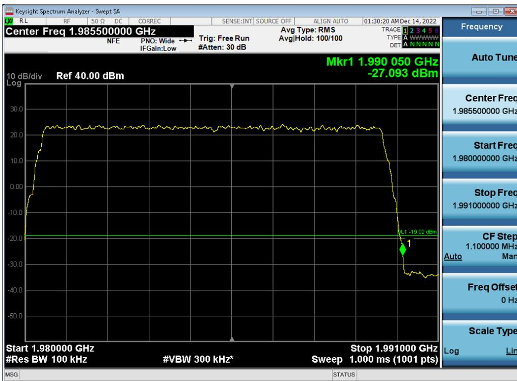
Antenna 3 / (4 Port) LTE B2 5 MHz 1 Carrier + 5G NR n2 5 MHz 1 Carrier + DSS B2 20 MHz 1 Carrier [3 Carrier] [1C+2C] / QPSK / Low / Non-Contiguous
