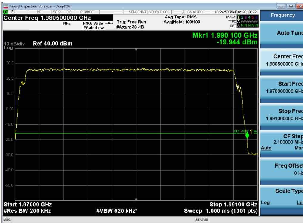
Antenna 1 / (2 Port) DSS B2 10 MHz 1 Carrier + DSS B2 10 MHz 1 Carrier + DSS B2 10 MHz 1 Carrier [3 Carrier] [1C+2C] / QPSK / Low / Non-Contiguous
