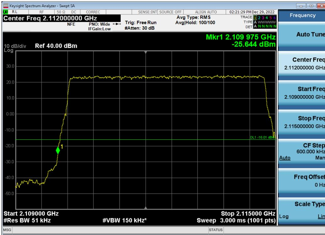
Antenna 1 / (2 Port) LTE B66 5 MHz 1 Carrier + 5G NR n66 5 MHz 1 Carrier + 5G NR n66 5 MHz 1 Carrier + DSS B66 10 MHz 1 Carrier [4 Carrier] [3C+1C] / QPSK / High / Non-Contiguous
