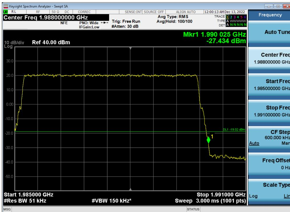
Antenna 2 / (4 Port) 5G NR n2 5 MHz 1 Carrier + 5G NR n2 5 MHz 1 Carrier + DSS B2 20 MHz 1 Carrier [3 Carrier] / 16QAM / Low / Contiguous
