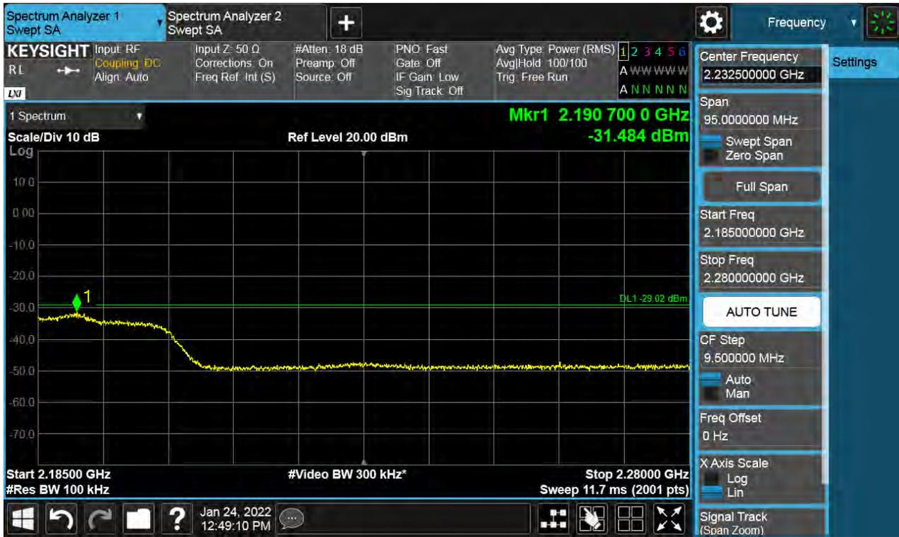
**Antenna 3 / High Edge + 100 MHz ~ 10 GHz / (4 Port) LTE B66 5 MHz 1 Carrier + LTE B66 5 MHz 1 Carrier + LTE B66 5 MHz 1 Carrier + 5G NR n66 5 MHz 1 Carrier [4 Carrier] (3C+1C) / Non-Contiguous / 256QAM**
