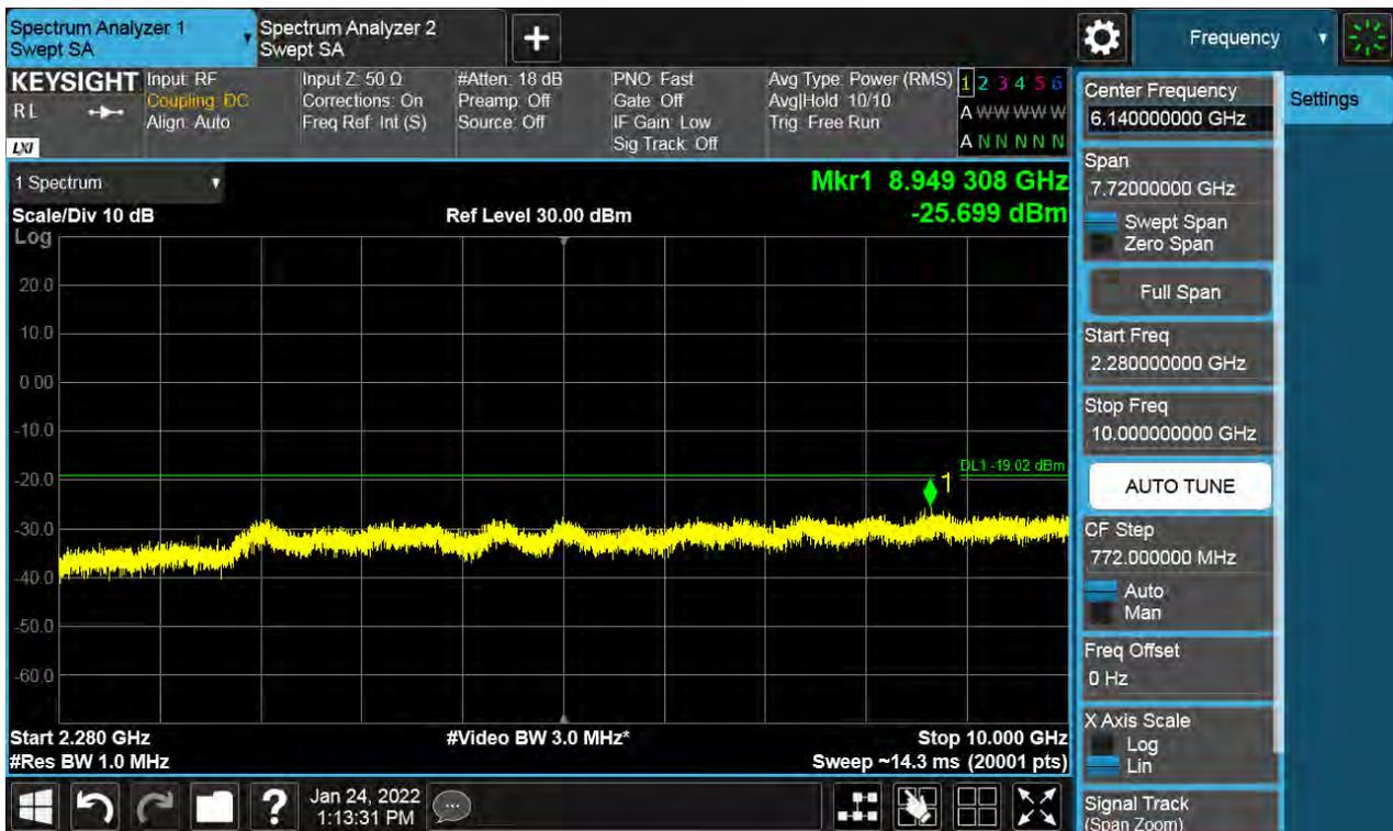
Antenna 2 / 10 GHz ~ 26.5 GHz / (4 Port) LTE B66 5 MHz 1 Carrier + LTE B66 5 MHz 1 Carrier + LTE B66 5 MHz 1 Carrier + 5G NR n66 5 MHz 1 Carrier [4 Carrier] (3C+1C) / Non-Contiguous / QPSK
