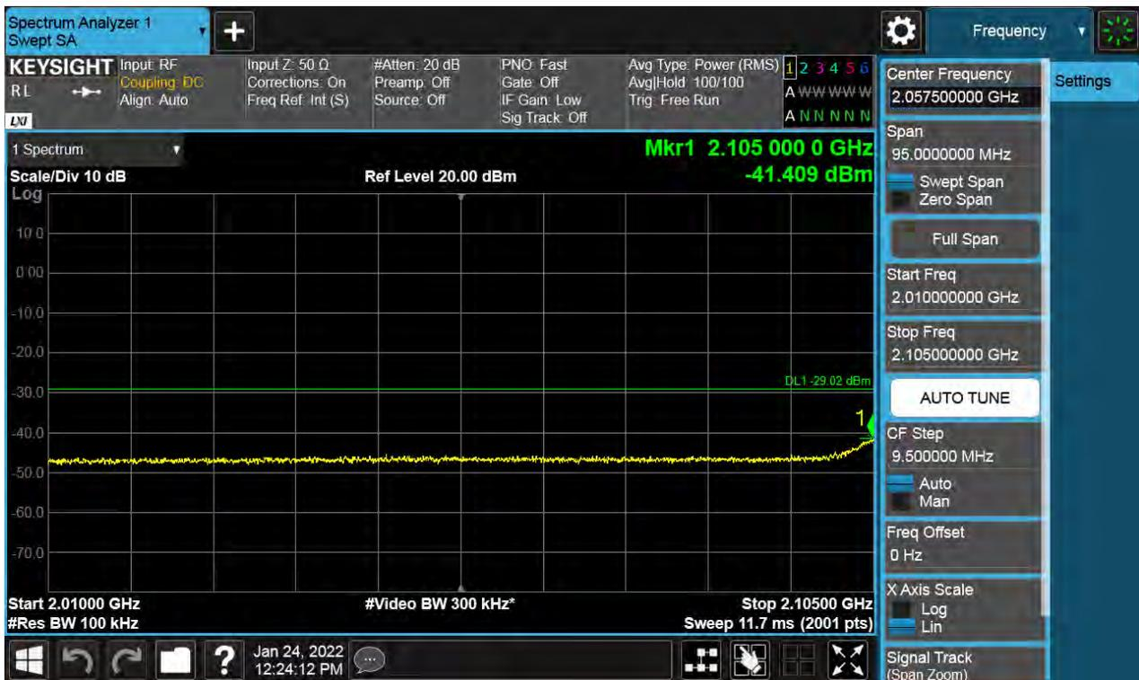
**Antenna 0 / High Edge ~ High Edge + 100 MHz / (4 Port) LTE B66 5 MHz 1 Carrier + LTE B66 5 MHz 1 Carrier + LTE B66 5 MHz 1 Carrier + 5G NR n66 5 MHz 1 Carrier [4 Carrier] (3C+1C) / Non-Contiguous / 64QAM**
