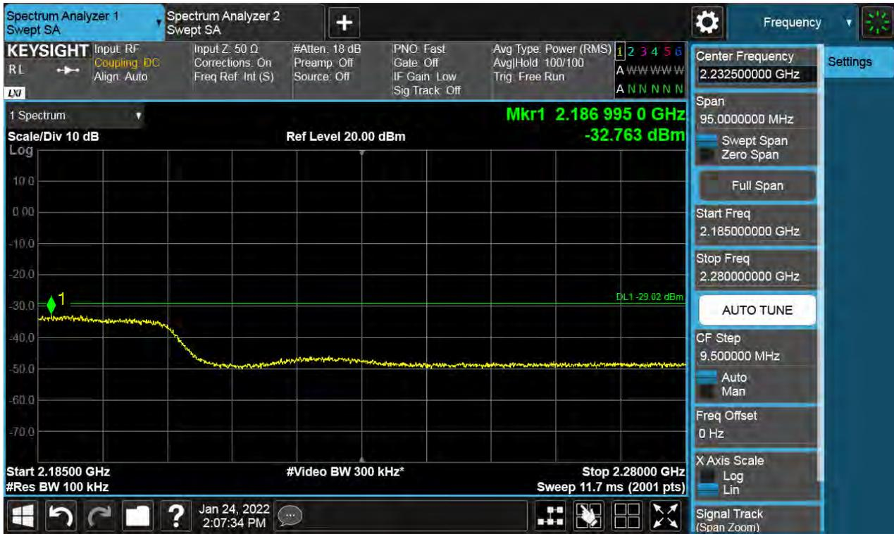
**Antenna 3 / High Edge + 100 MHz ~ 10 GHz / (4 Port) LTE B66 5 MHz 1 Carrier + LTE B66 5 MHz 1 Carrier + LTE B66 5 MHz 1 Carrier + 5G NR n66 5 MHz 1 Carrier [4 Carrier] (1C+3C) / Non-Contiguous / QPSK**
