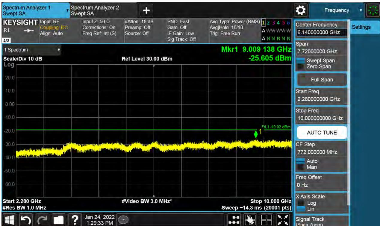
Antenna 2 / 10 GHz ~ 26.5 GHz / (4 Port) LTE B66 5 MHz 1 Carrier + LTE B66 5 MHz 1 Carrier + LTE B66 5 MHz 1 Carrier + 5G NR n66 5 MHz 1 Carrier [4 Carrier] (1C+3C) / Non-Contiguous / 64QAM
