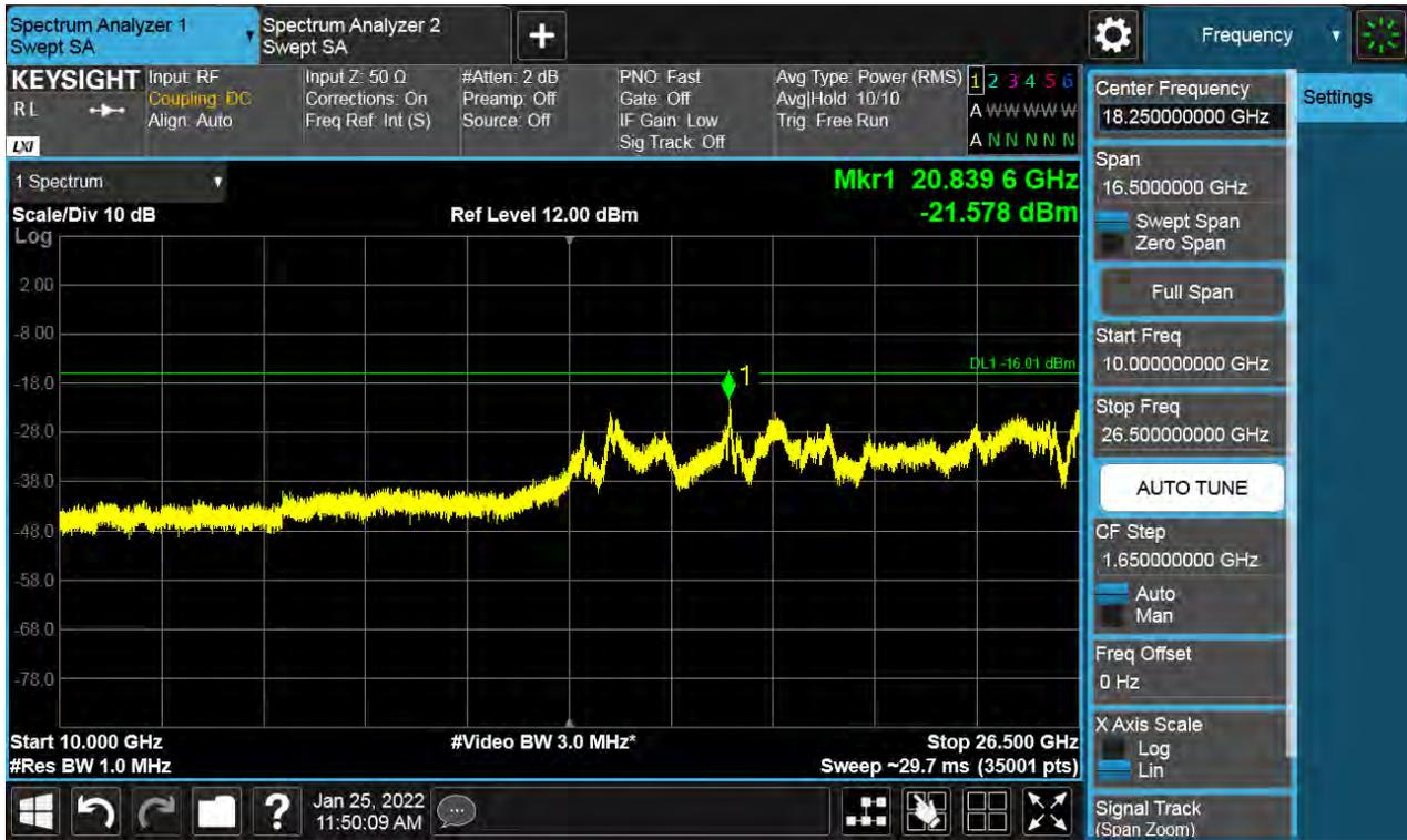
Antenna 0 / 9 kHz ~ 150 kHz / (4 Port) LTE B66 5 MHz 1 Carrier + LTE B66 5 MHz 1 Carrier + LTE B66 5 MHz 1 Carrier + 5G NR n66 5 MHz 1 Carrier [4 Carrier] (1C+3C) / Non-Contiguous / 16QAM
