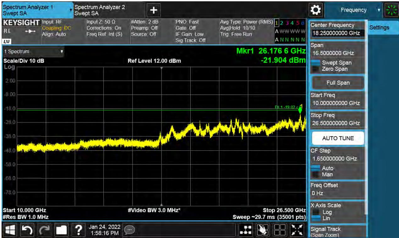
Antenna 0 / 9 kHz ~ 150 kHz / (4 Port) LTE B66 5 MHz 1 Carrier + LTE B66 5 MHz 1 Carrier + LTE B66 5 MHz 1 Carrier + 5G NR n66 5 MHz 1 Carrier [4 Carrier] (3C+1C) / Non-Contiguous / 16QAM
