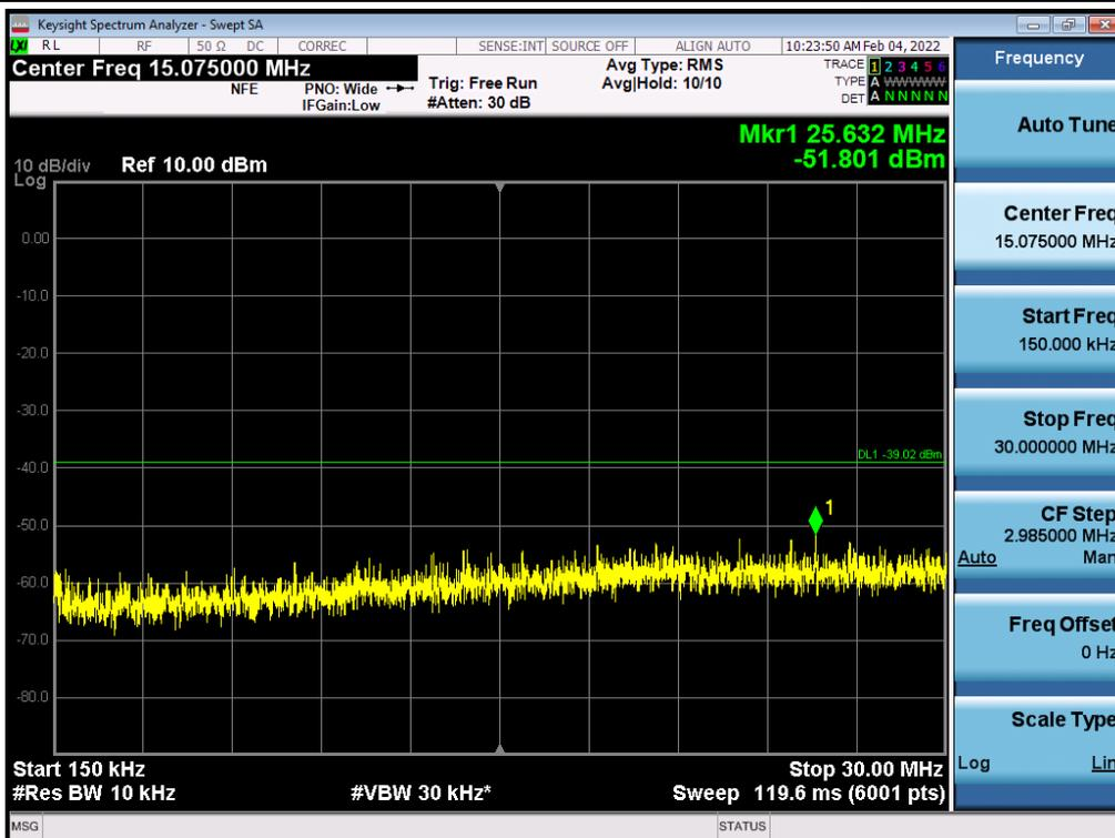
**Antenna 3 / 30 MHz ~ Low Edge - 100 MHz / (4 Port) LTE B66 5 MHz 1 Carrier + LTE B66 5 MHz 1 Carrier + LTE B66 10 MHz 1 Carrier + 5G NR n66 20 MHz 1 Carrier [4 Carrier] (1C+3C) / Non-Contiguous / 16QAM**
