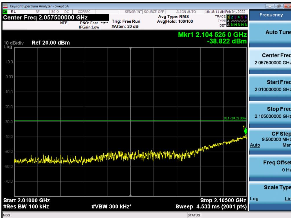
Antenna 0 / High Edge ~ High Edge + 100 MHz / (4 Port) LTE B66 5 MHz 1 Carrier + LTE B66 5 MHz 1 Carrier + LTE B66 10 MHz 1 Carrier + 5G NR n66 20 MHz 1 Carrier [4 Carrier] (1C+3C) / Non-Contiguous / 16QAM
