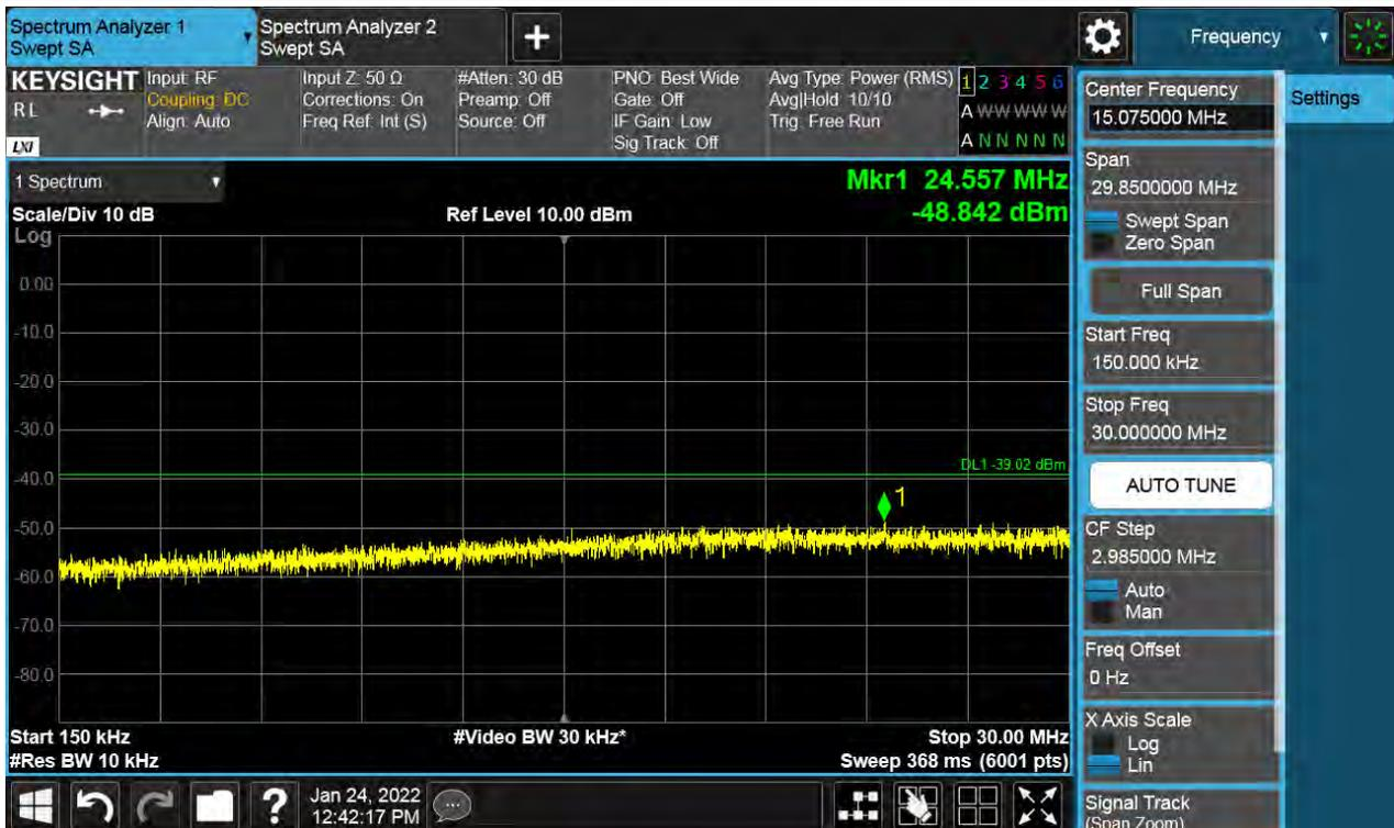
**Antenna 3 / 30 MHz ~ Low Edge - 100 MHz / (4 Port) LTE B66 5 MHz 1 Carrier + LTE B66 5 MHz 1 Carrier + LTE B66 5 MHz 1 Carrier + 5G NR n66 5 MHz 1 Carrier [4 Carrier] (3C+1C) / Non-Contiguous / 64QAM**
