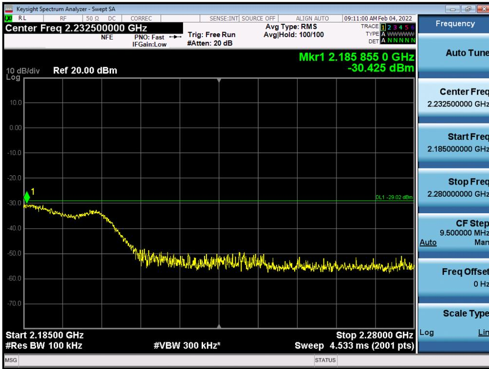
Antenna 3 / High Edge + 100 MHz ~ 10 GHz / (4 Port) LTE B66 5 MHz 1 Carrier + LTE B66 5 MHz 1 Carrier + LTE B66 10 MHz 1 Carrier + 5G NR n66 20 MHz 1 Carrier [4 Carrier] (3C+1C) / Non-Contiguous / 64QAM
