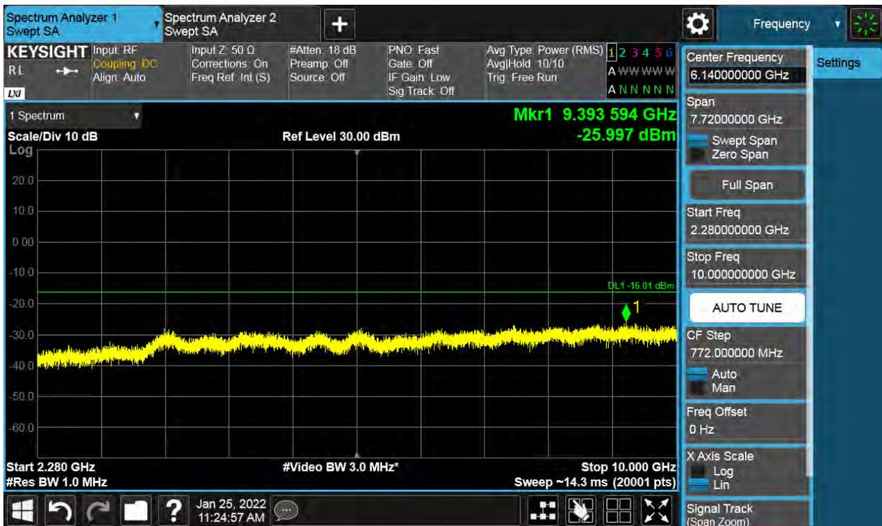
Antenna 1 / 10 GHz ~ 26.5 GHz / (2 Port) LTE B66 5 MHz 1 Carrier + LTE B66 5 MHz 1 Carrier + LTE B66 10 MHz 1 Carrier + 5G NR n66 20 MHz 1 Carrier [4 Carrier] (3C+1C) / Non-Contiguous / 64QAM
