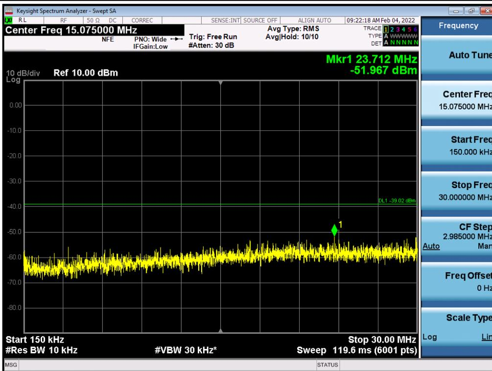
Antenna 3 / 30 MHz ~ Low Edge - 100 MHz / (4 Port) LTE B66 5 MHz 1 Carrier + LTE B66 5 MHz 1 Carrier + LTE B66 10 MHz 1 Carrier + 5G NR n66 20 MHz 1 Carrier [4 Carrier] (3C+1C) / Non-Contiguous / 64QAM
