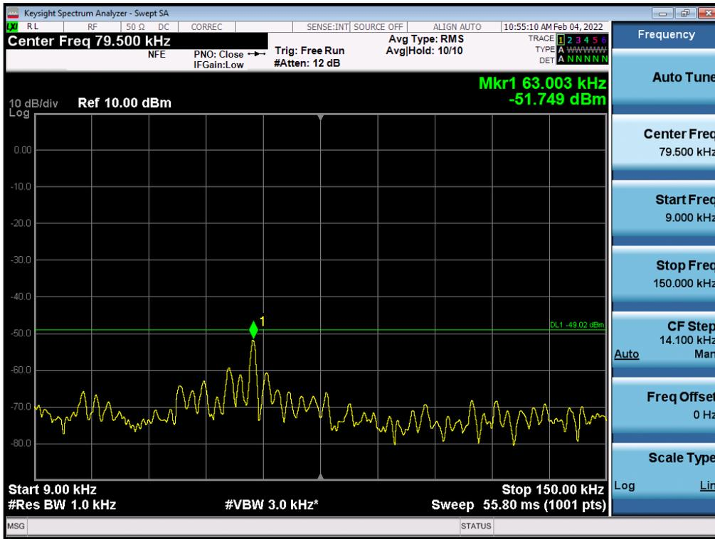
Antenna 3 / 150 kHz ~ 30 MHz / (4 Port) LTE B66 5 MHz 1 Carrier + LTE B66 5 MHz 1 Carrier + LTE B66 10 MHz 1 Carrier + 5G NR n66 20 MHz 1 Carrier [4 Carrier] (1C+3C) / Non-Contiguous / QPSK
