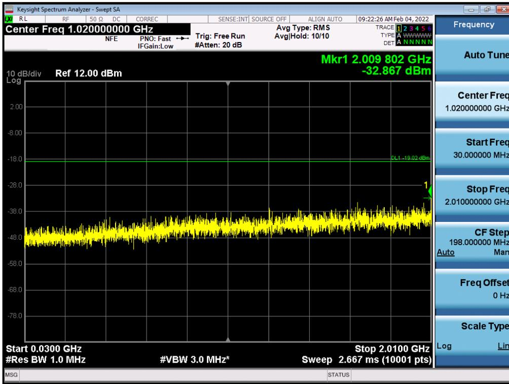
Antenna 2 / Low Edge - 100 MHz ~ Low Edge / (4 Port) LTE B66 5 MHz 1 Carrier + LTE B66 5 MHz 1 Carrier + LTE B66 10 MHz 1 Carrier + 5G NR n66 20 MHz 1 Carrier [4 Carrier] (3C+1C) / Non-Contiguous / QPSK
