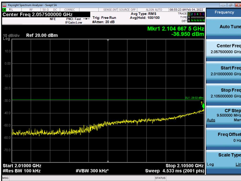
Antenna 1 / High Edge ~ High Edge + 100 MHz / (4 Port) LTE B66 5 MHz 1 Carrier + LTE B66 5 MHz 1 Carrier + LTE B66 10 MHz 1 Carrier + 5G NR n66 20 MHz 1 Carrier [4 Carrier] (3C+1C) / Non-Contiguous / 64QAM
