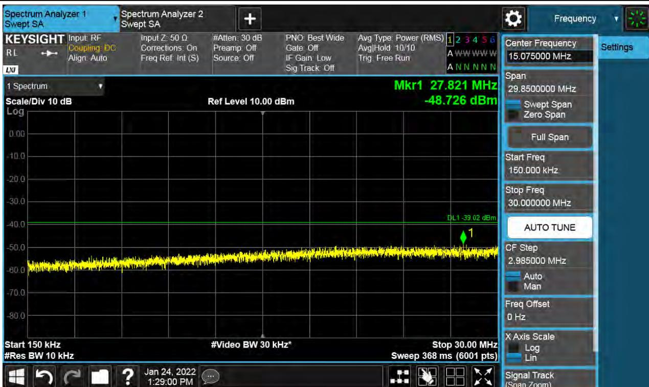
**Antenna 3 / 30 MHz ~ Low Edge - 100 MHz / (4 Port) LTE B66 5 MHz 1 Carrier + LTE B66 5 MHz 1 Carrier + LTE B66 5 MHz 1 Carrier + 5G NR n66 5 MHz 1 Carrier [4 Carrier] (1C+3C) / Non-Contiguous / 64QAM**
