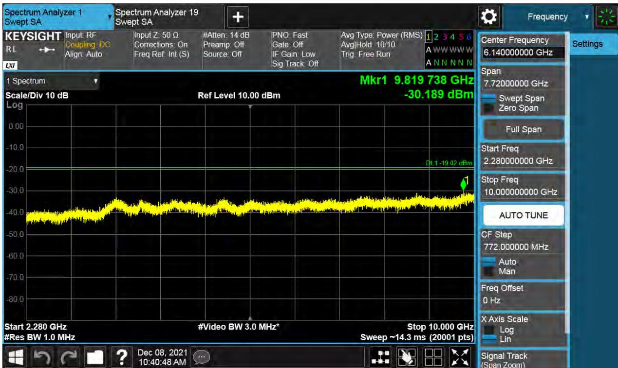
Antenna 1 / 10 GHz ~ 26.5 GHz / (4 Port) B66 DSS 20 MHz 9to1 1 Carrier + LTE B66 10 MHz 1 Carrier + LTE B66 5 MHz 1 Carrier + LTE B66 5 MHz 1 Carrier [4 Carrier] (3C+1C) / Non-Contiguous / 16QAM
