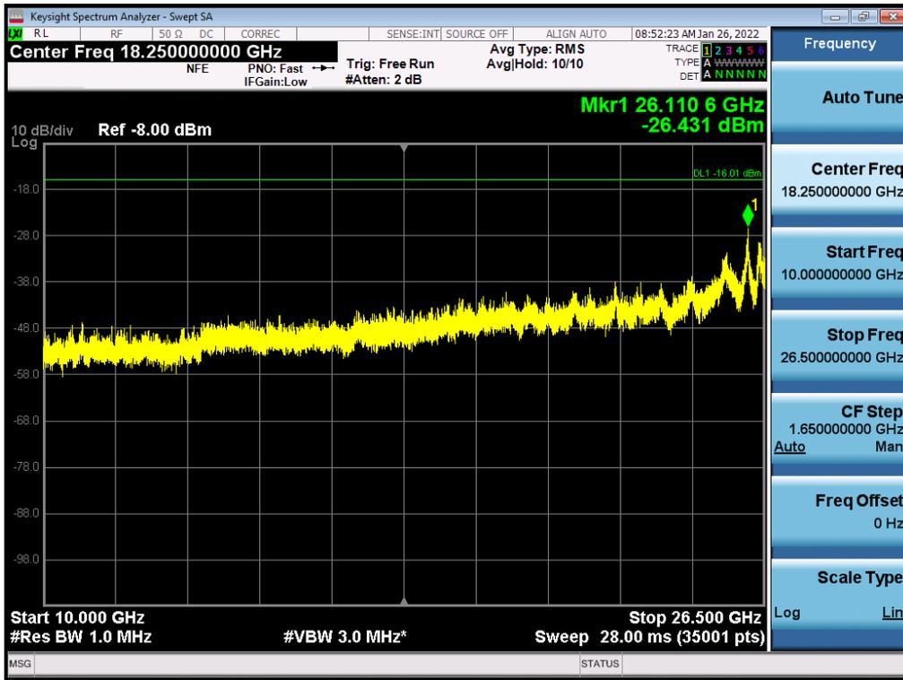
Antenna 0 / 9 kHz ~ 150 kHz / (2 Port) LTE B2 5 MHz 1 Carrier + LTE B2 5 MHz 1 Carrier + 5G NR n2 5 MHz 1 Carrier [3 Carrier] (2C+1C) / Non-Contiguous / 16QAM
