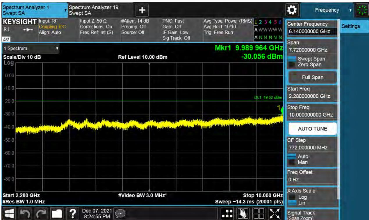
Antenna 1 / 10 GHz ~ 26.5 GHz / (4 Port) B66 DSS 20 MHz 9to1 1 Carrier + LTE B66 10 MHz 1 Carrier + LTE B66 5 MHz 1 Carrier + LTE B66 5 MHz 1 Carrier [4 Carrier] (1C+3C) / Non-Contiguous / QPSK
