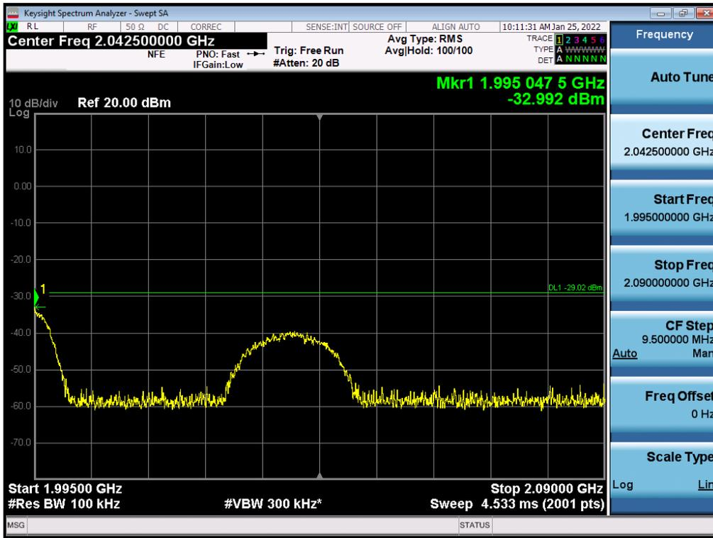
Antenna 0 / High Edge + 100 MHz ~ 10 GHz / (4 Port) LTE B2 5 MHz 1 Carrier + LTE B2 5 MHz 1 Carrier + 5G NR n2 5 MHz 1 Carrier [3 Carrier] (1C+2C) / Non-Contiguous / 64QAM
