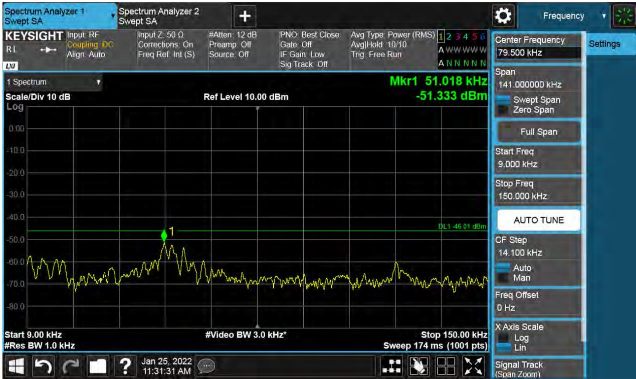
Antenna 1 / 150 kHz ~ 30 MHz / (2 Port) LTE B66 5 MHz 1 Carrier + LTE B66 5 MHz 1 Carrier + LTE B66 10 MHz 1 Carrier + 5G NR n66 20 MHz 1 Carrier [4 Carrier] (3C+1C) / Non-Contiguous / 256QAM
