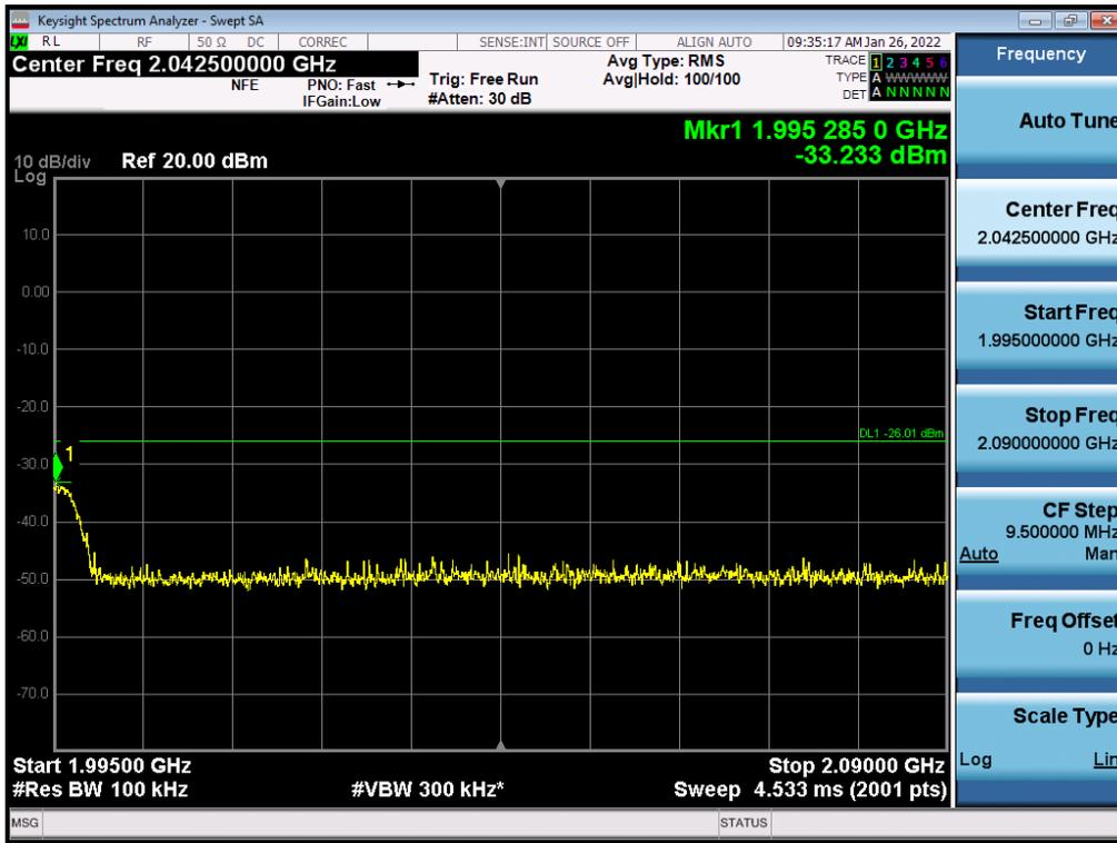
Antenna 0 / High Edge + 100 MHz ~ 10 GHz / (2 Port) LTE B2 5 MHz 1 Carrier + LTE B2 5 MHz 1 Carrier + 5G NR n2 5 MHz 1 Carrier [3 Carrier] (2C+1C) / Non-Contiguous / QPSK
