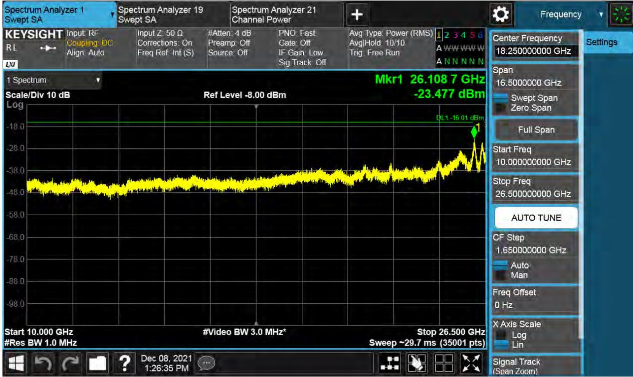
Antenna 1 / 9 kHz ~ 150 kHz / (2 Port) B66 DSS 20 MHz 9to1 1 Carrier + LTE B66 10 MHz 1 Carrier + LTE B66 5 MHz 1 Carrier + LTE B66 5 MHz 1 Carrier [4 Carrier] (3C+1C) / Non-Contiguous / 64QAM
