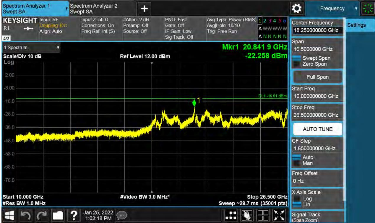
Antenna 0 / 9 kHz ~ 150 kHz / (2 Port) LTE B66 5 MHz 1 Carrier + LTE B66 5 MHz 1 Carrier + LTE B66 10 MHz 1 Carrier + 5G NR n66 20 MHz 1 Carrier [4 Carrier] (3C+1C) / Non-Contiguous / 16QAM
