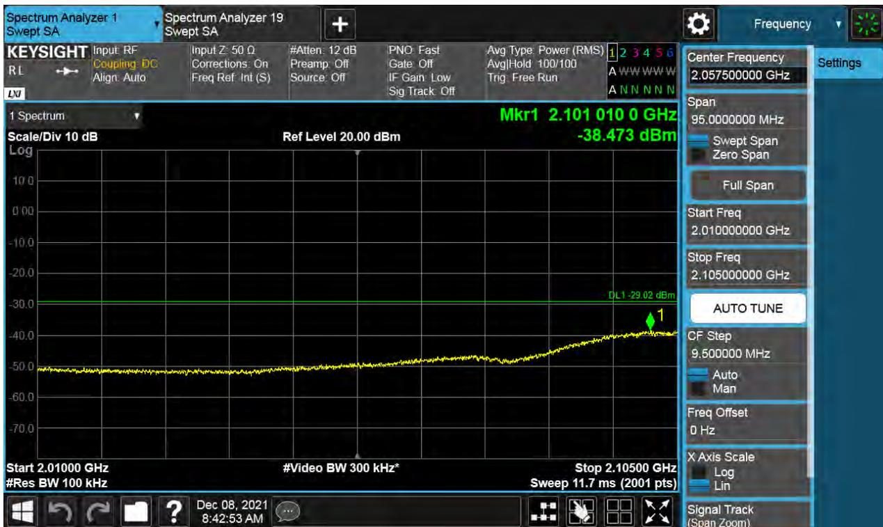
Antenna 0 / High Edge ~ High Edge + 100 MHz / (4 Port) B66 DSS 20 MHz 9to1 1 Carrier + LTE B66 10 MHz 1 Carrier + LTE B66 5 MHz 1 Carrier + LTE B66 5 MHz 1 Carrier [4 Carrier] (1C+3C) / Non-Contiguous / 256QAM
