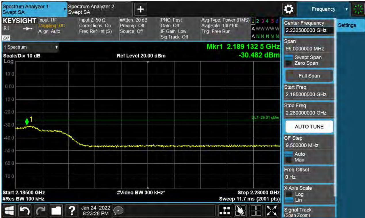
**Antenna 1 / High Edge + 100 MHz ~ 10 GHz / (2 Port) LTE B66 5 MHz 1 Carrier + LTE B66 5 MHz 1 Carrier + LTE B66 5 MHz 1 Carrier + 5G NR n66 5 MHz 1 Carrier [4 Carrier] (3C+1C) / Non-Contiguous / QPSK**
