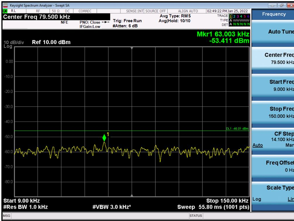
Antenna 0 / 150 kHz ~ 30 MHz / (2 Port) LTE B2 5 MHz 1 Carrier + LTE B2 5 MHz 1 Carrier + 5G NR n2 20 MHz 1 Carrier [3 Carrier] (2C+1C) / Non-Contiguous / 16QAM
