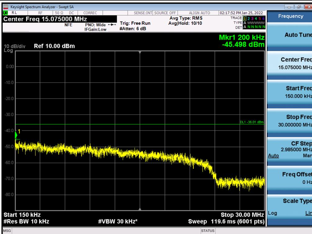
**Antenna 0 / 30 MHz ~ Low Edge - 100 MHz / (2 Port) LTE B2 5 MHz 1 Carrier + LTE B2 5 MHz 1 Carrier + 5G NR n2 20 MHz 1 Carrier [3 Carrier] (1C+2C) / Non-Contiguous / QPSK**
