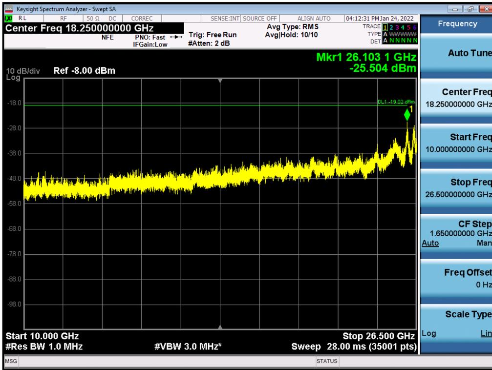
Antenna 1 / 9 kHz ~ 150 kHz / (2 Port) B66 DSS 20 MHz 9to1 1 Carrier + LTE B66 10 MHz 1 Carrier + LTE B66 5 MHz 1 Carrier + LTE B66 5 MHz 1 Carrier [4 Carrier] (1C+3C) / Non-Contiguous / 256QAM
