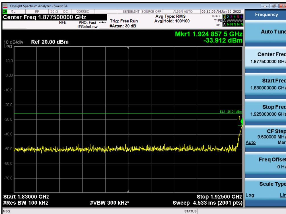
Antenna 1 / High Edge ~ High Edge + 100 MHz / (2 Port) LTE B2 5 MHz 1 Carrier + LTE B2 5 MHz 1 Carrier + 5G NR n2 5 MHz 1 Carrier [3 Carrier] (2C+1C) / Non-Contiguous / 256QAM
