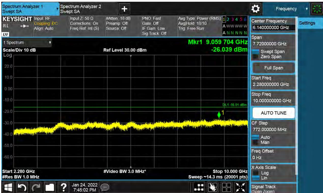
Antenna 1 / 10 GHz ~ 26.5 GHz / (2 Port) LTE B66 5 MHz 1 Carrier + LTE B66 5 MHz 1 Carrier + LTE B66 5 MHz 1 Carrier + 5G NR n66 5 MHz 1 Carrier [4 Carrier] (3C+1C) / Non-Contiguous / 64QAM
