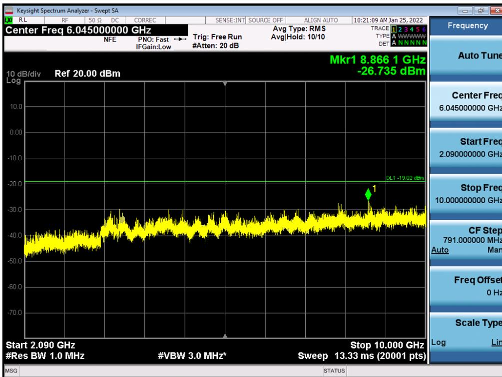
Antenna 2 / 10 GHz ~ 26.5 GHz / (4 Port) LTE B2 5 MHz 1 Carrier + LTE B2 5 MHz 1 Carrier + 5G NR n2 5 MHz 1 Carrier [3 Carrier] (1C+2C) / Non-Contiguous / 256QAM
