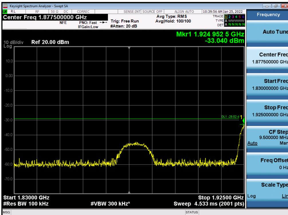
Antenna 1 / High Edge ~ High Edge + 100 MHz / (4 Port) LTE B2 5 MHz 1 Carrier + LTE B2 5 MHz 1 Carrier + 5G NR n2 5 MHz 1 Carrier [3 Carrier] (1C+2C) / Non-Contiguous / 16QAM
