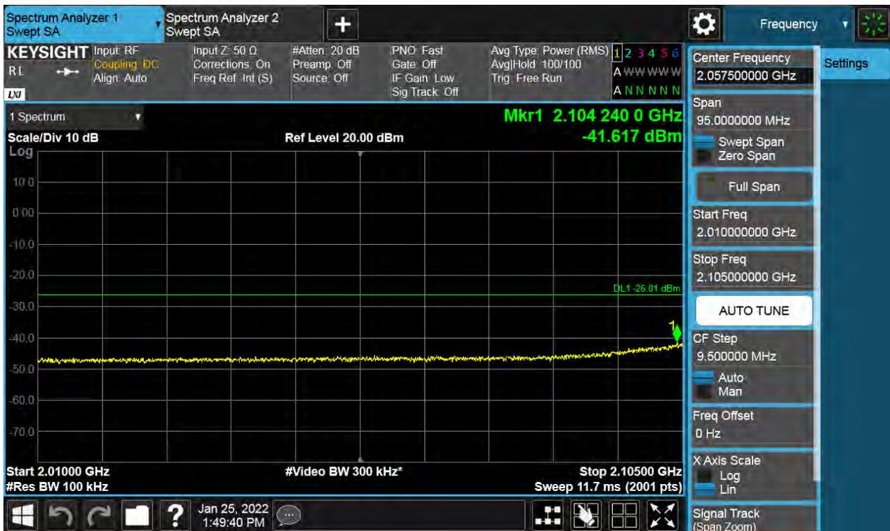
Antenna 1 / High Edge ~ High Edge + 100 MHz / (2 Port) LTE B66 5 MHz 1 Carrier + LTE B66 5 MHz 1 Carrier + LTE B66 10 MHz 1 Carrier + 5G NR n66 20 MHz 1 Carrier [4 Carrier] (1C+3C) / Non-Contiguous / 16QAM
