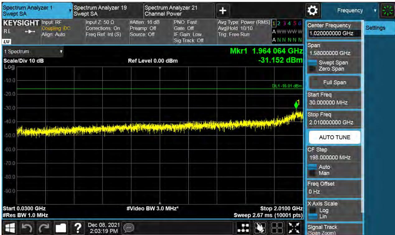
**Antenna 1 / Low Edge - 100 MHz ~ Low Edge / (2 Port) B66 DSS 20 MHz 9to1 1 Carrier + LTE B66 10 MHz 1 Carrier + LTE B66 5 MHz 1 Carrier + LTE B66 5 MHz 1 Carrier [4 Carrier] (3C+1C) / Non-Contiguous / 16QAM**
