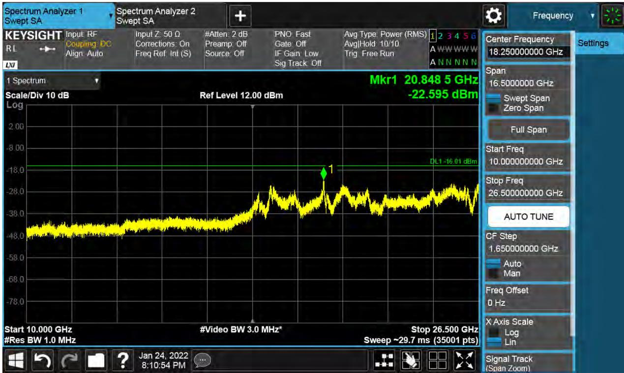
Antenna 1 / 9 kHz ~ 150 kHz / (2 Port) LTE B66 5 MHz 1 Carrier + LTE B66 5 MHz 1 Carrier + LTE B66 10 MHz 1 Carrier + 5G NR n66 20 MHz 1 Carrier [4 Carrier] (1C+3C) / Non-Contiguous / QPSK
