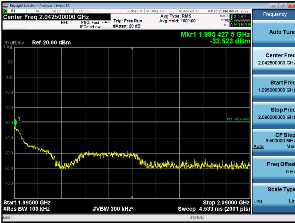
Antenna 2 / High Edge + 100 MHz ~ 10 GHz / (4 Port) LTE B2 5 MHz 1 Carrier + LTE B2 5 MHz 1 Carrier + 5G NR n2 20 MHz 1 Carrier [3 Carrier] (2C+1C) / Non-Contiguous / QPSK
