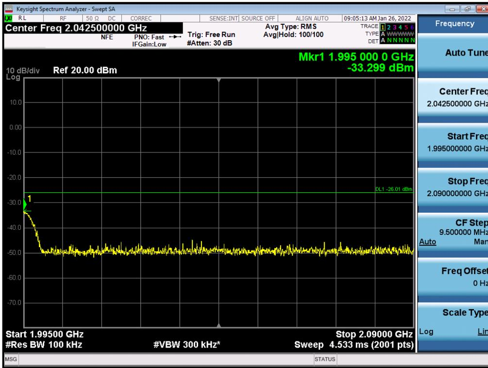
Antenna 1 / High Edge + 100 MHz ~ 10 GHz / (2 Port) LTE B2 5 MHz 1 Carrier + LTE B2 5 MHz 1 Carrier + 5G NR n2 5 MHz 1 Carrier [3 Carrier] (1C+2C) / Non-Contiguous / 16QAM
