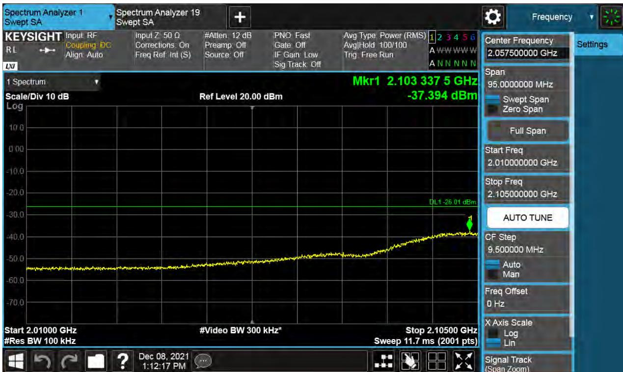
Antenna 0 / High Edge ~ High Edge + 100 MHz / (2 Port) B66 DSS 20 MHz 9to1 1 Carrier + LTE B66 10 MHz 1 Carrier + LTE B66 5 MHz 1 Carrier + LTE B66 5 MHz 1 Carrier [4 Carrier] (1C+3C) / Non-Contiguous / 256QAM
