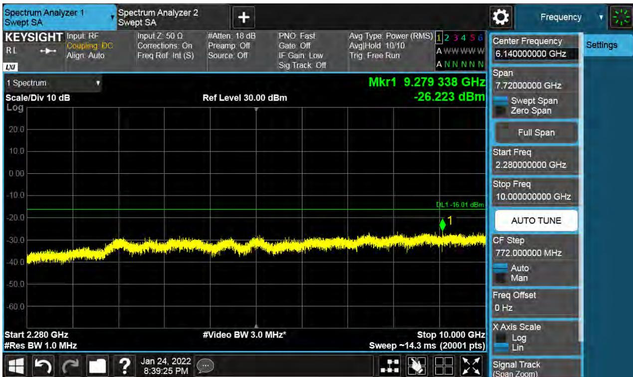
Antenna 1 / 10 GHz ~ 26.5 GHz / (2 Port) LTE B66 5 MHz 1 Carrier + LTE B66 5 MHz 1 Carrier + LTE B66 5 MHz 1 Carrier + 5G NR n66 5 MHz 1 Carrier [4 Carrier] (1C+3C) / Non-Contiguous / QPSK
