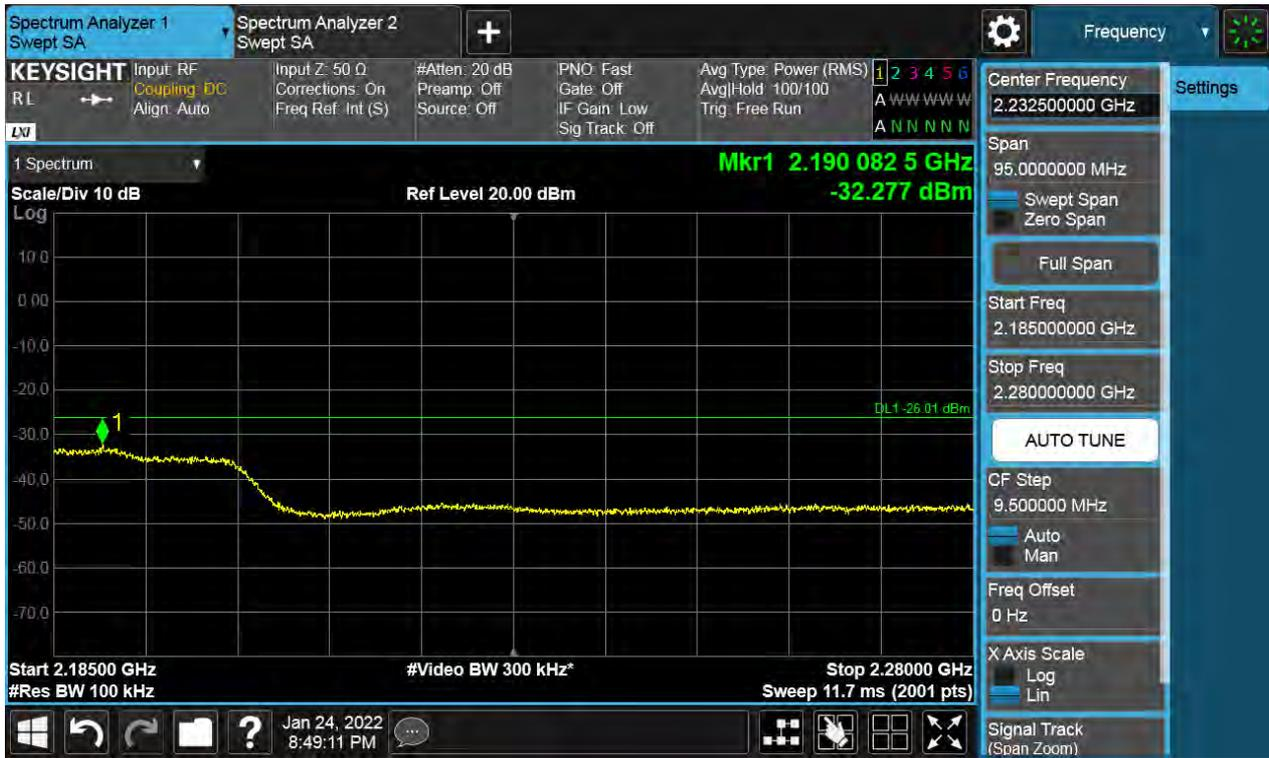
**Antenna 1 / High Edge + 100 MHz ~ 10 GHz / (2 Port) LTE B66 5 MHz 1 Carrier + LTE B66 5 MHz 1 Carrier + LTE B66 5 MHz 1 Carrier + 5G NR n66 5 MHz 1 Carrier [4 Carrier] (1C+3C) / Non-Contiguous / QPSK**
