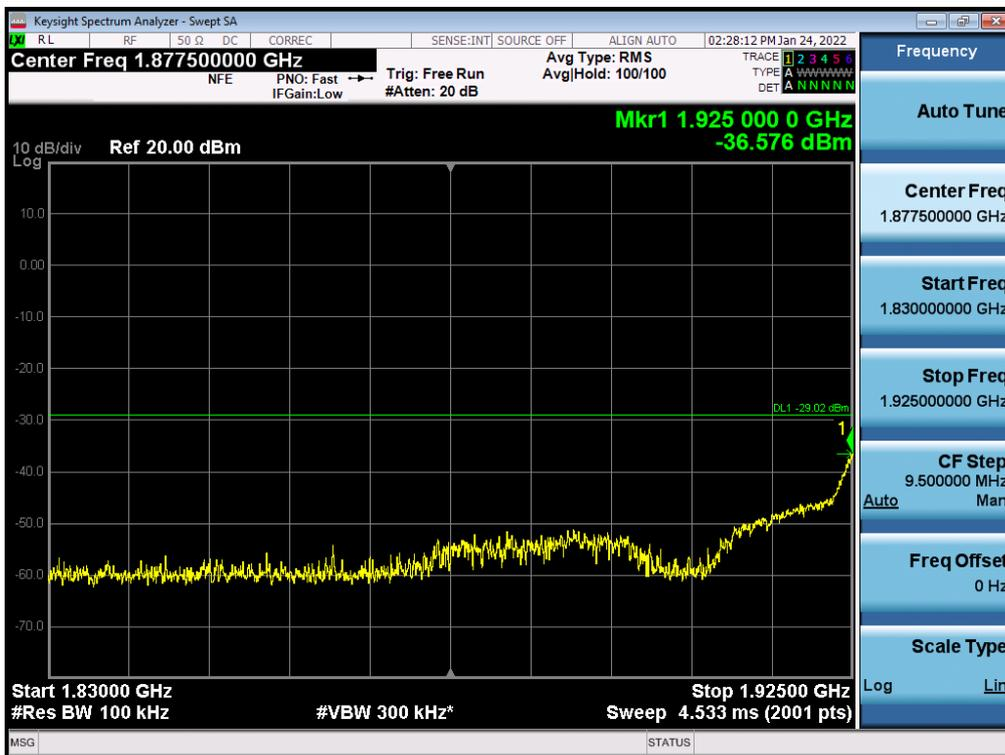
Antenna 1 / High Edge ~ High Edge + 100 MHz / (4 Port) LTE B2 5 MHz 1 Carrier + LTE B2 5 MHz 1 Carrier + 5G NR n2 20 MHz 1 Carrier [3 Carrier] (1C+2C) / Non-Contiguous / 256QAM
