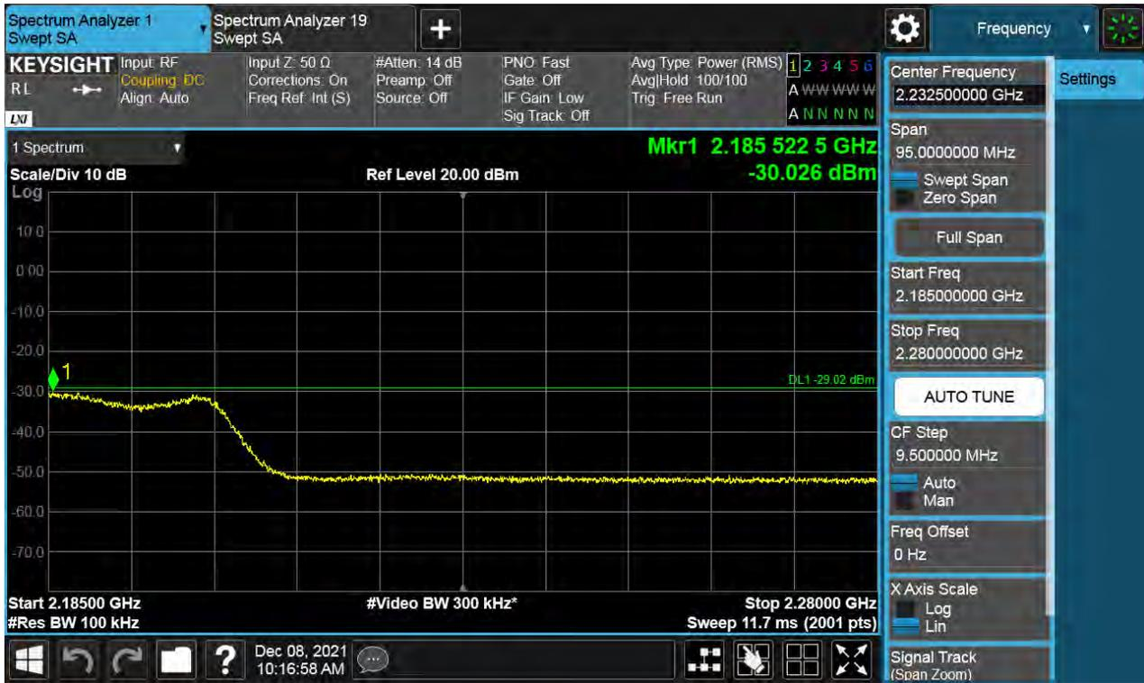
Antenna 0 / High Edge + 100 MHz ~ 10 GHz / (4 Port) B66 DSS 20 MHz 9to1 1 Carrier + LTE B66 10 MHz 1 Carrier + LTE B66 5 MHz 1 Carrier + LTE B66 5 MHz 1 Carrier [4 Carrier] (3C+1C) / Non-Contiguous / 16QAM
