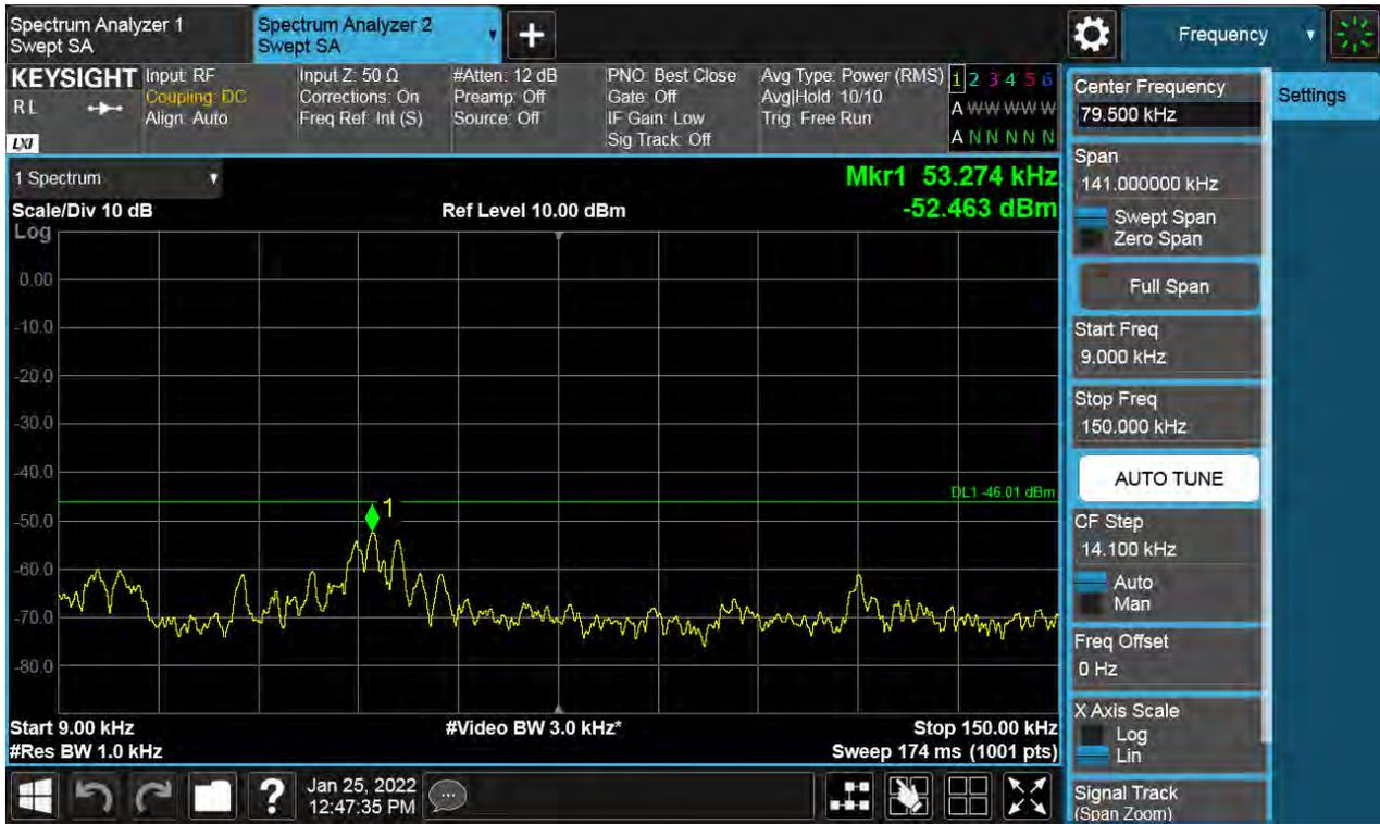
Antenna 1 / 150 kHz ~ 30 MHz / (2 Port) LTE B66 5 MHz 1 Carrier + LTE B66 5 MHz 1 Carrier + LTE B66 10 MHz 1 Carrier + 5G NR n66 20 MHz 1 Carrier [4 Carrier] (1C+3C) / Non-Contiguous / 256QAM
