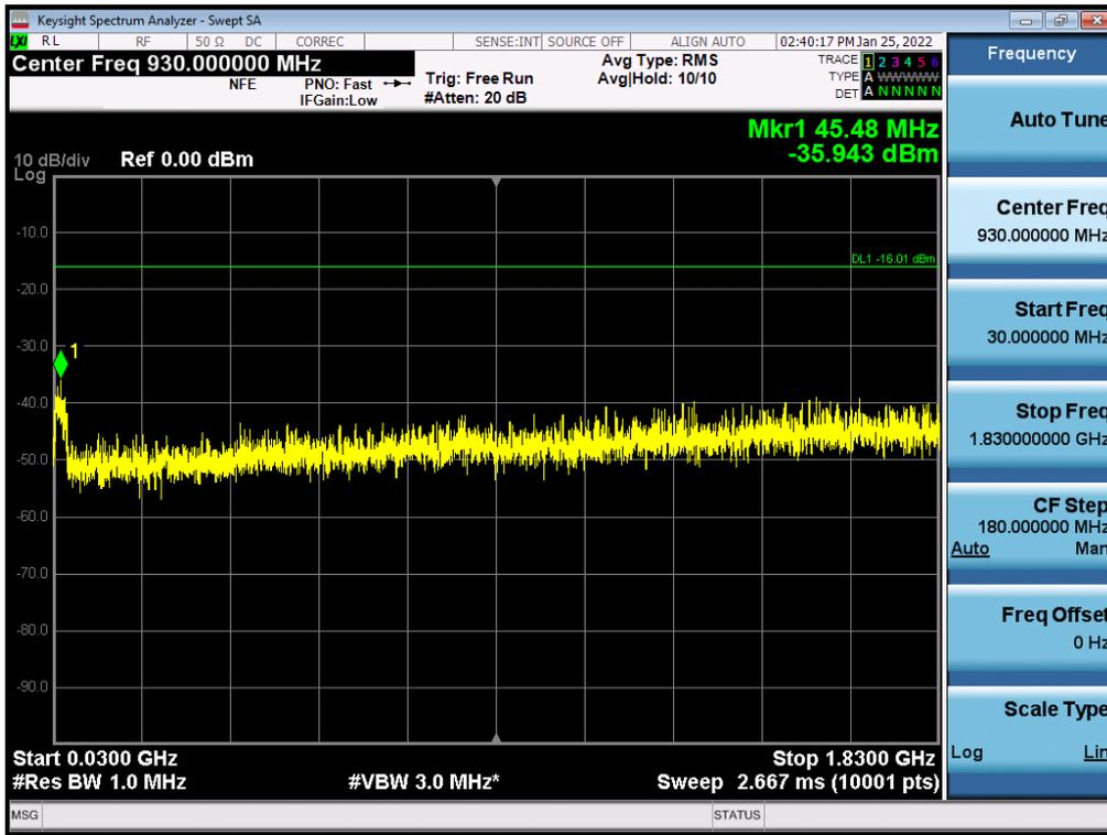
Antenna 1 / Low Edge - 100 MHz ~ Low Edge / (2 Port) LTE B2 5 MHz 1 Carrier + LTE B2 5 MHz 1 Carrier + 5G NR n2 20 MHz 1 Carrier [3 Carrier] (2C+1C) / Non-Contiguous / QPSK
