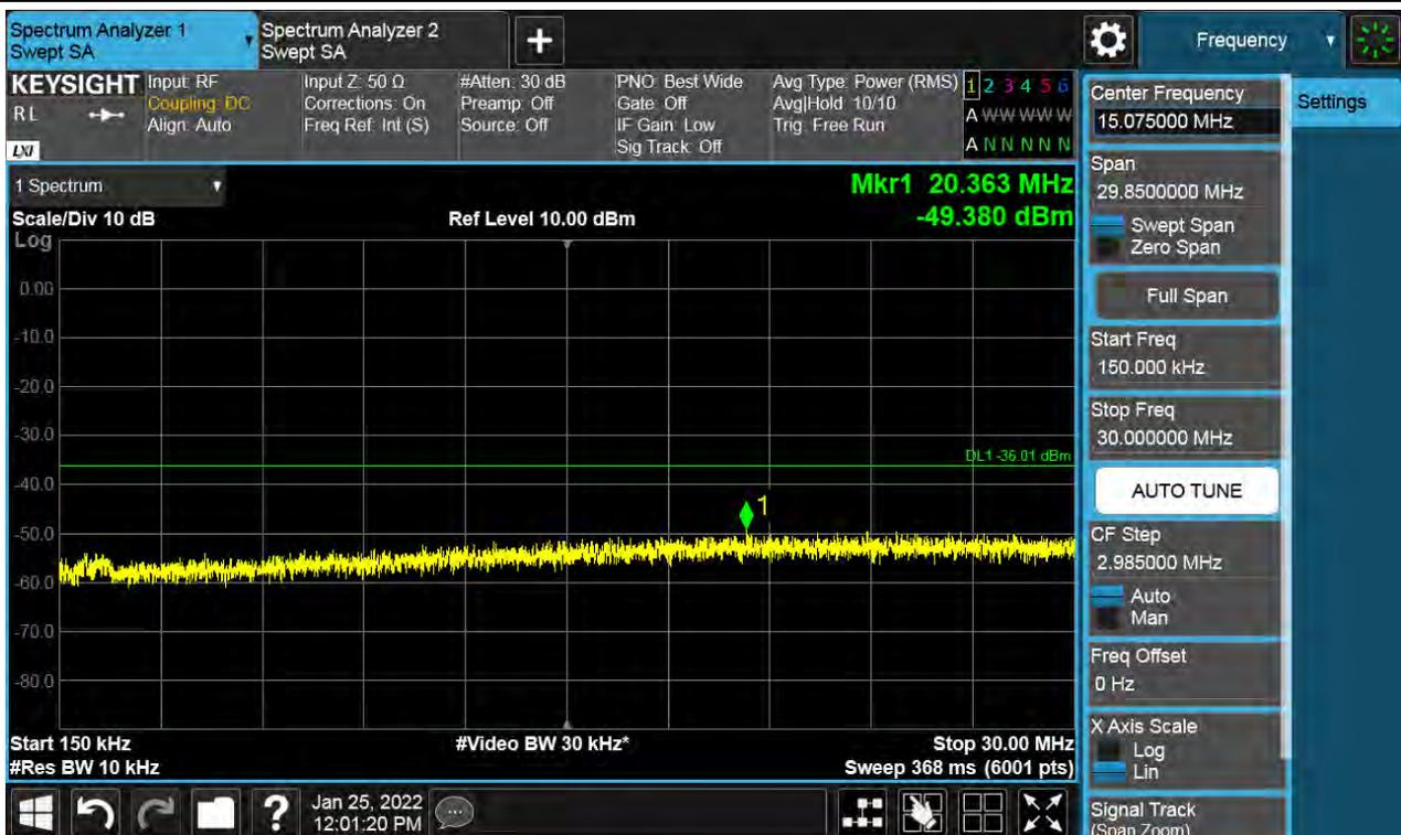
Antenna 1 / 30 MHz ~ Low Edge - 100 MHz / (2 Port) LTE B66 5 MHz 1 Carrier + LTE B66 5 MHz 1 Carrier + LTE B66 10 MHz 1 Carrier + 5G NR n66 20 MHz 1 Carrier [4 Carrier] (3C+1C) / Non-Contiguous / 64QAM
