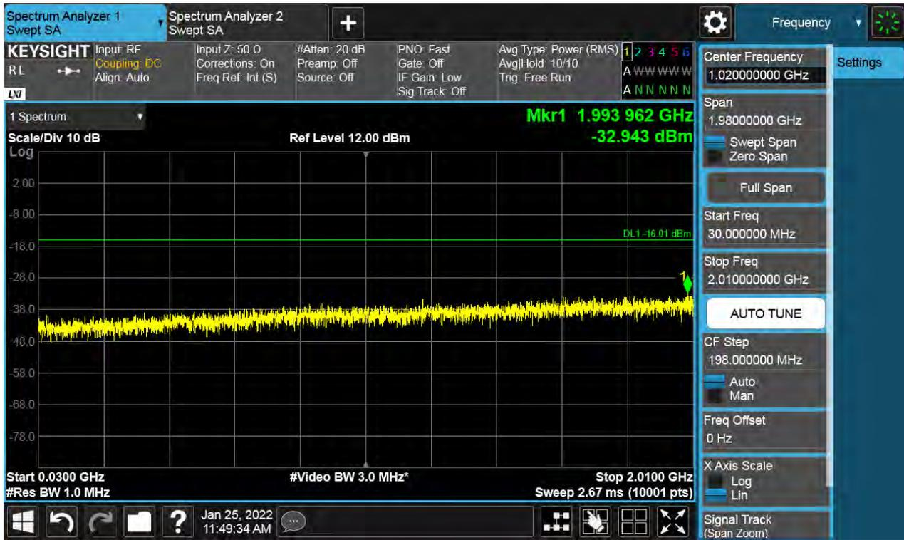
Antenna 1 / Low Edge - 100 MHz ~ Low Edge / (2 Port) LTE B66 5 MHz 1 Carrier + LTE B66 5 MHz 1 Carrier + LTE B66 10 MHz 1 Carrier + 5G NR n66 20 MHz 1 Carrier [4 Carrier] (3C+1C) / Non-Contiguous / 16QAM
