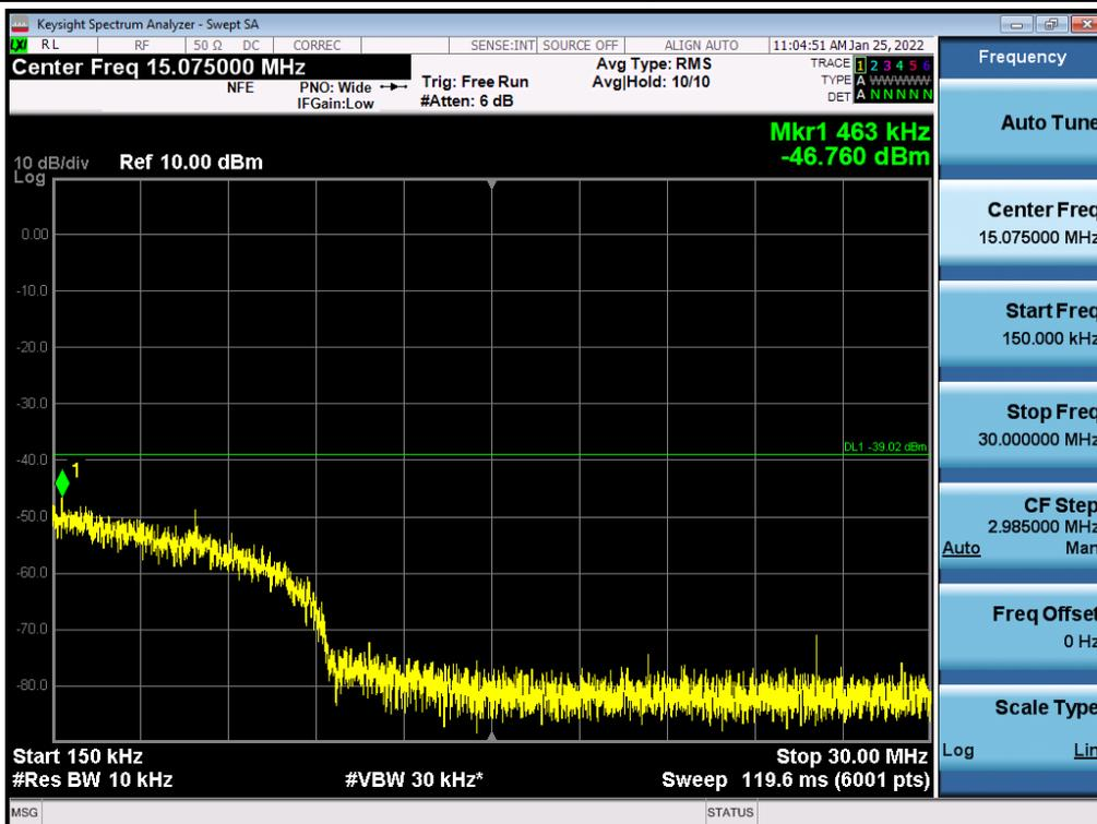
**Antenna 0 / 30 MHz ~ Low Edge - 100 MHz / (4 Port) LTE B2 5 MHz 1 Carrier + LTE B2 5 MHz 1 Carrier + 5G NR n2 5 MHz 1 Carrier [3 Carrier] (2C+1C) / Non-Contiguous / 16QAM**
