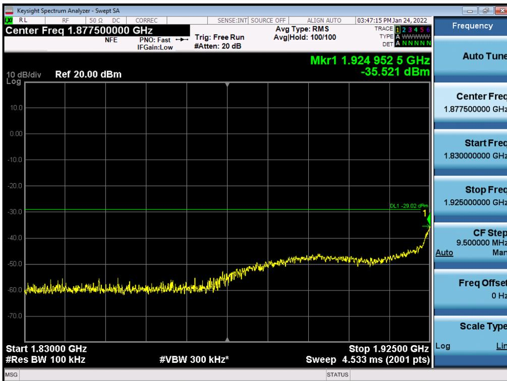
Antenna 0 / High Edge ~ High Edge + 100 MHz / (4 Port) LTE B2 5 MHz 1 Carrier + LTE B2 5 MHz 1 Carrier + 5G NR n2 20 MHz 1 Carrier [3 Carrier] (2C+1C) / Non-Contiguous / QPSK
