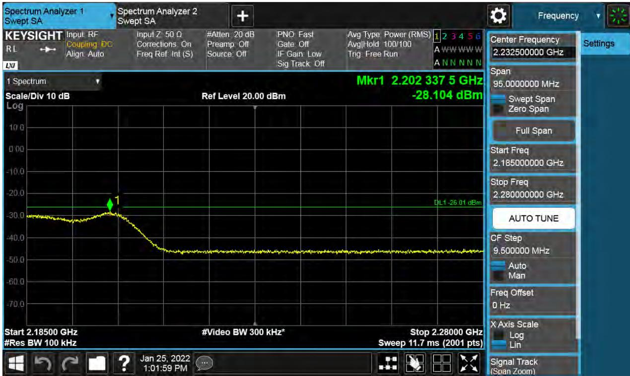
Antenna 1 / High Edge + 100 MHz ~ 10 GHz / (2 Port) LTE B66 5 MHz 1 Carrier + LTE B66 5 MHz 1 Carrier + LTE B66 10 MHz 1 Carrier + 5G NR n66 20 MHz 1 Carrier [4 Carrier] (1C+3C) / Non-Contiguous / 16QAM
