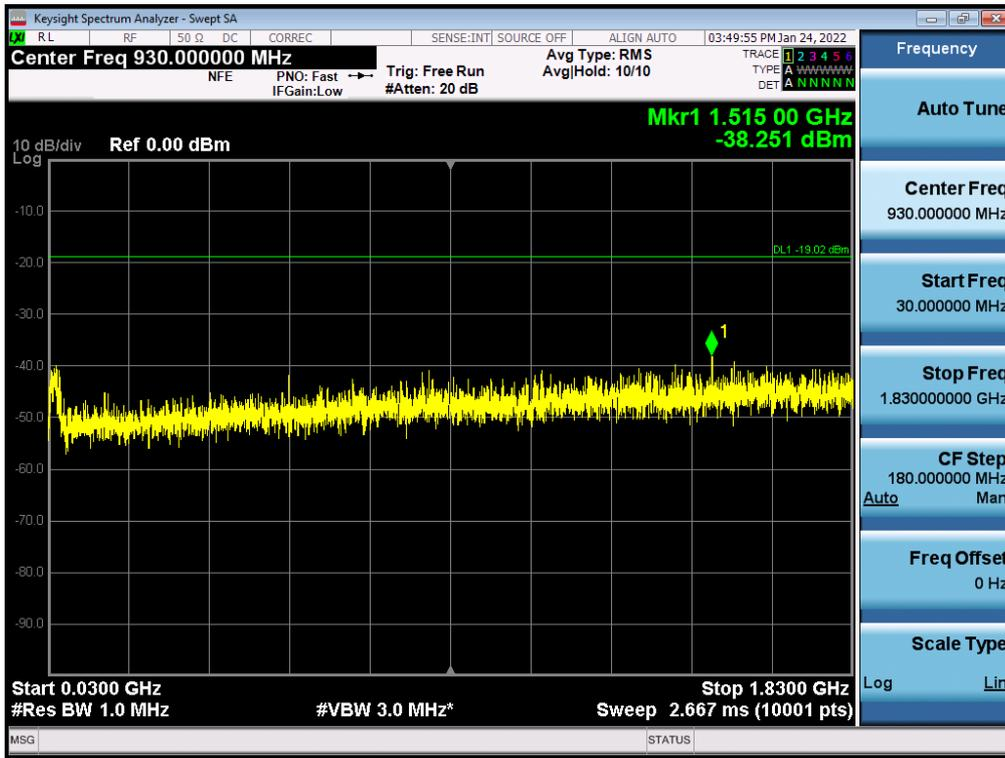
Antenna 1 / Low Edge - 100 MHz ~ Low Edge / (4 Port) LTE B2 5 MHz 1 Carrier + LTE B2 5 MHz 1 Carrier + 5G NR n2 20 MHz 1 Carrier [3 Carrier] (2C+1C) / Non-Contiguous / 16QAM
