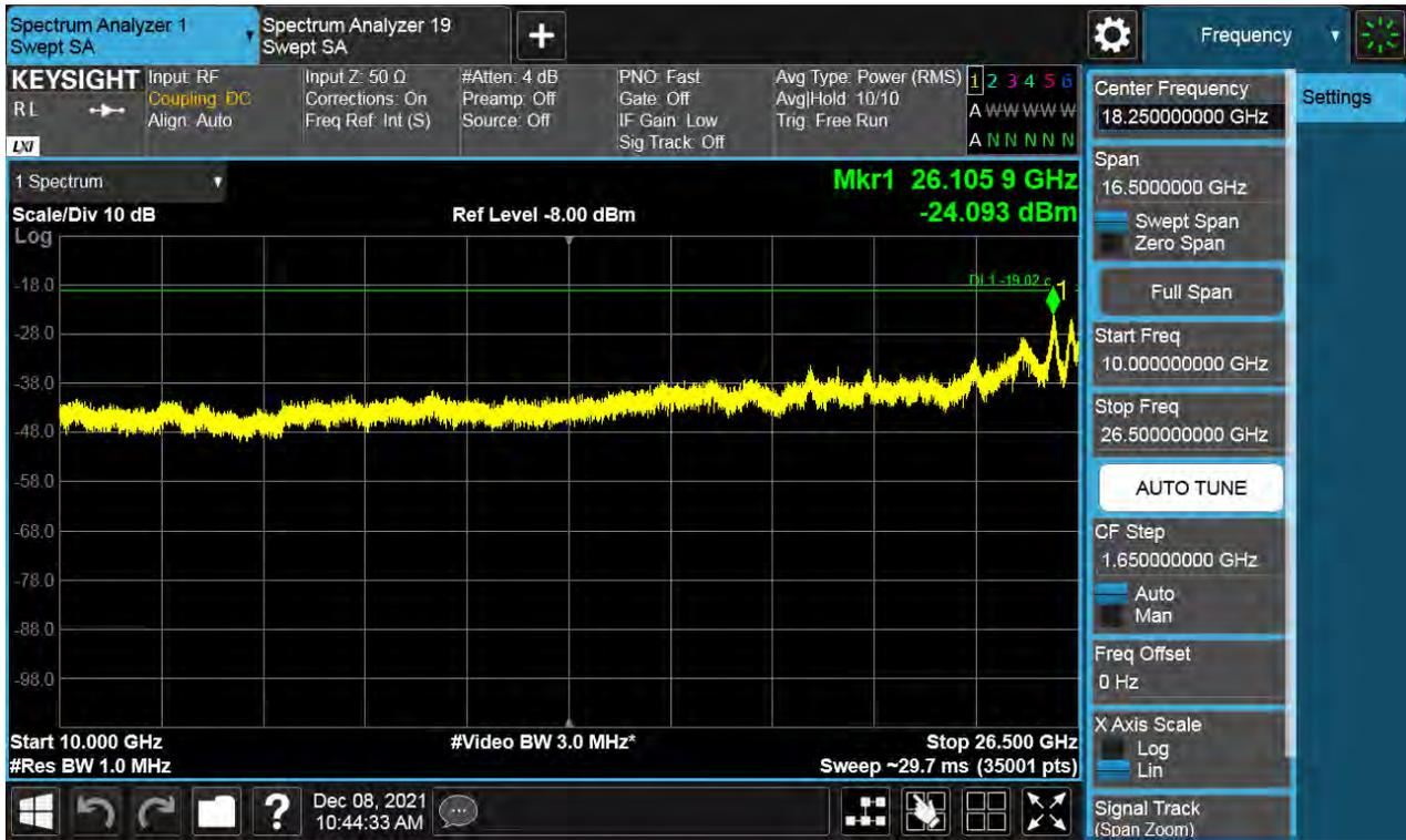
Antenna 1 / 9 kHz ~ 150 kHz / (2 Port) LTE B66 5 MHz 1 Carrier + LTE B66 5 MHz 1 Carrier + LTE B66 5 MHz 1 Carrier + 5G NR n66 5 MHz 1 Carrier [4 Carrier] (1C+3C) / Non-Contiguous / 16QAM
