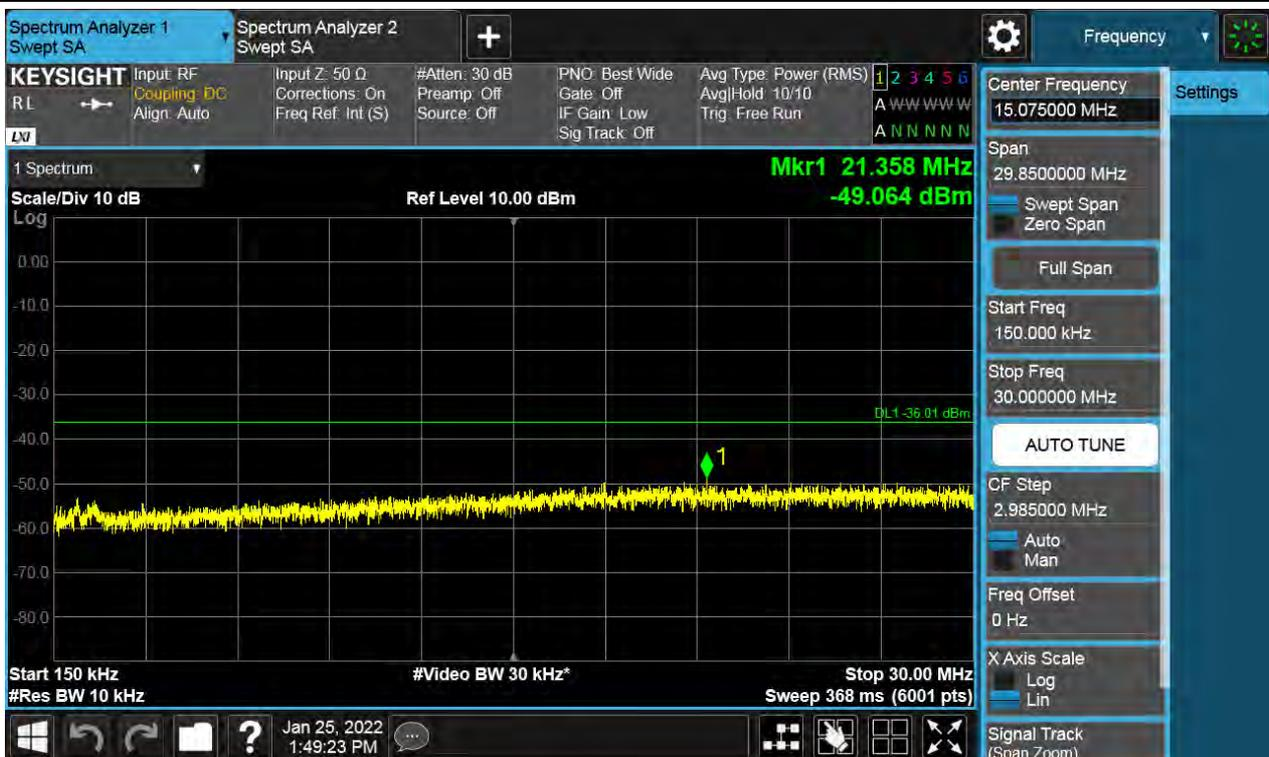
Antenna 1 / 30 MHz ~ Low Edge - 100 MHz / (2 Port) LTE B66 5 MHz 1 Carrier + LTE B66 5 MHz 1 Carrier + LTE B66 10 MHz 1 Carrier + 5G NR n66 20 MHz 1 Carrier [4 Carrier] (1C+3C) / Non-Contiguous / QPSK
