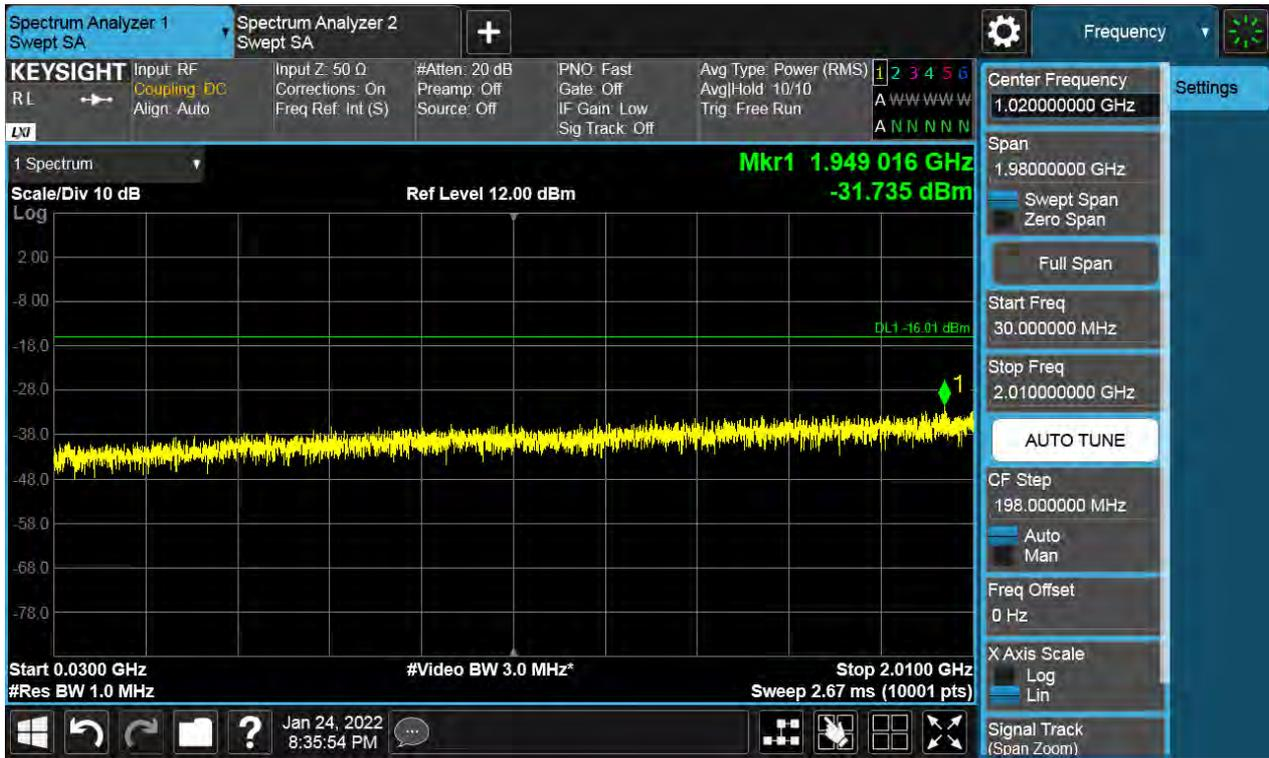
Antenna 1 / Low Edge - 100 MHz ~ Low Edge / (2 Port) LTE B66 5 MHz 1 Carrier + LTE B66 5 MHz 1 Carrier + LTE B66 5 MHz 1 Carrier + 5G NR n66 5 MHz 1 Carrier [4 Carrier] (1C+3C) / Non-Contiguous / QPSK
