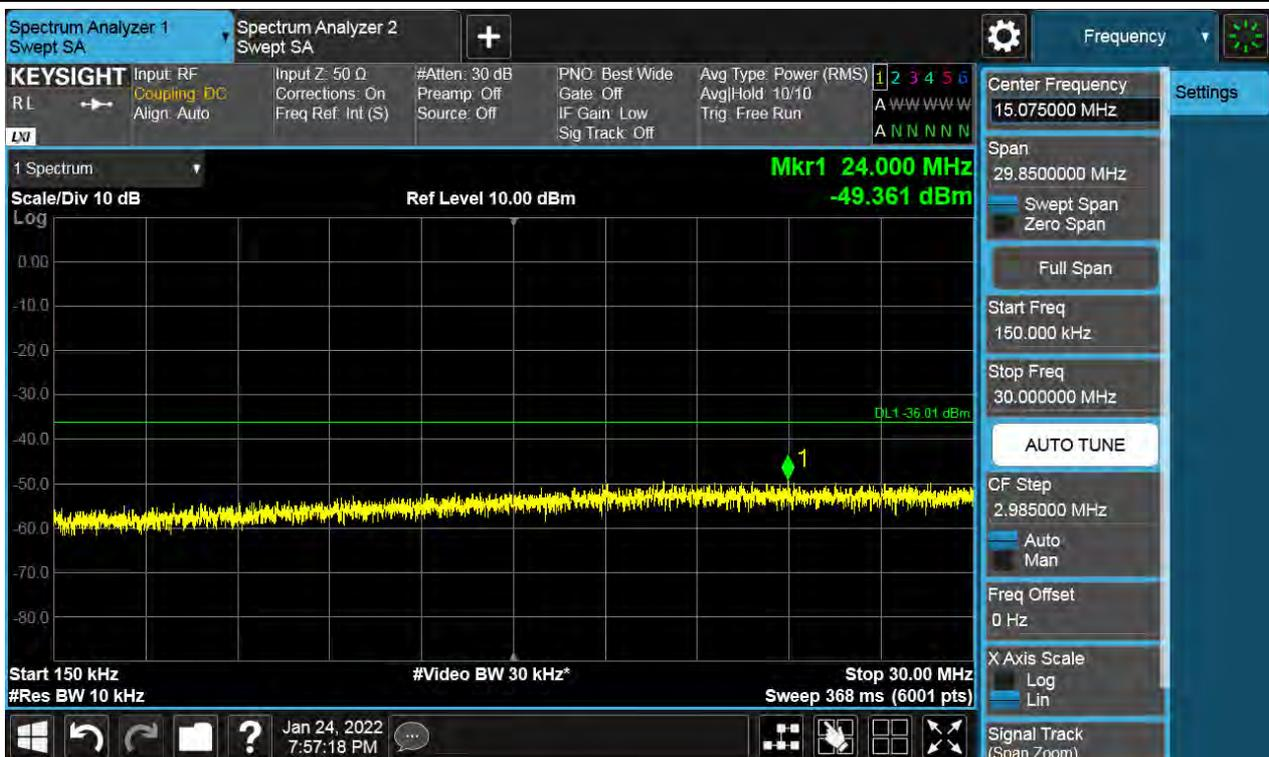
Antenna 1 / 30 MHz ~ Low Edge - 100 MHz / (2 Port) LTE B66 5 MHz 1 Carrier + LTE B66 5 MHz 1 Carrier + LTE B66 5 MHz 1 Carrier + 5G NR n66 5 MHz 1 Carrier [4 Carrier] (3C+1C) / Non-Contiguous / QPSK
