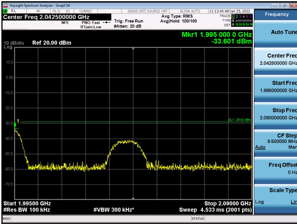
Antenna 1 / High Edge + 100 MHz ~ 10 GHz / (4 Port) LTE B2 5 MHz 1 Carrier + LTE B2 5 MHz 1 Carrier + 5G NR n2 5 MHz 1 Carrier [3 Carrier] (2C+1C) / Non-Contiguous / 16QAM
