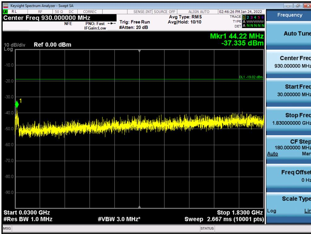
Antenna 1 / Low Edge - 100 MHz ~ Low Edge / (4 Port) LTE B2 5 MHz 1 Carrier + LTE B2 5 MHz 1 Carrier + 5G NR n2 20 MHz 1 Carrier [3 Carrier] (1C+2C) / Non-Contiguous / QPSK
