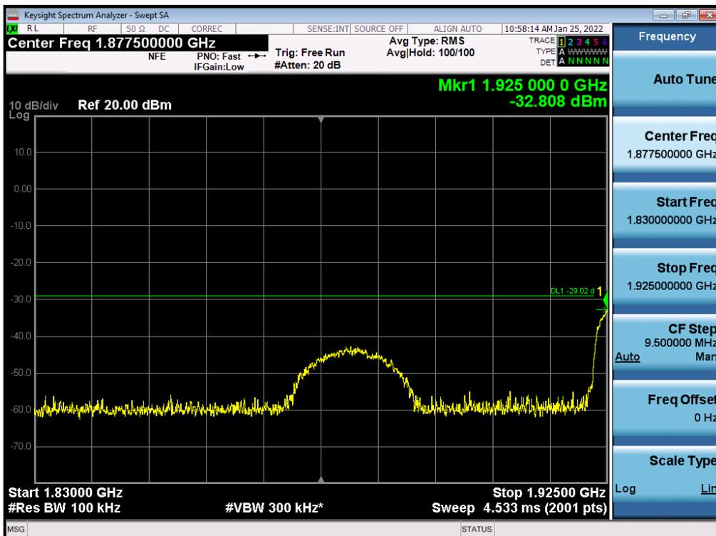
Antenna 3 / High Edge ~ High Edge + 100 MHz / (4 Port) LTE B2 5 MHz 1 Carrier + LTE B2 5 MHz 1 Carrier + 5G NR n2 5 MHz 1 Carrier [3 Carrier] (2C+1C) / Non-Contiguous / 16QAM
