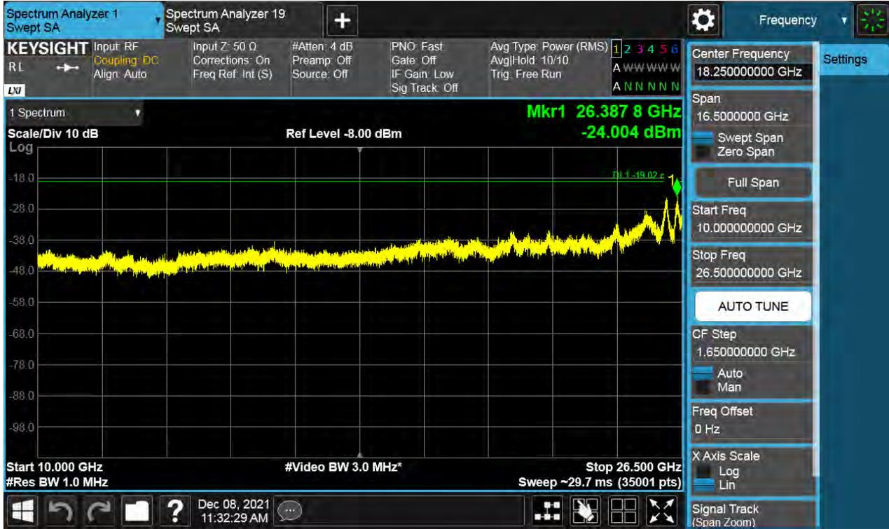
Antenna 3 / 9 kHz ~ 150 kHz / (4 Port) B66 DSS 20 MHz 9to1 1 Carrier + LTE B66 10 MHz 1 Carrier + LTE B66 5 MHz 1 Carrier + LTE B66 5 MHz 1 Carrier [4 Carrier] (3C+1C) / Non-Contiguous / QPSK
