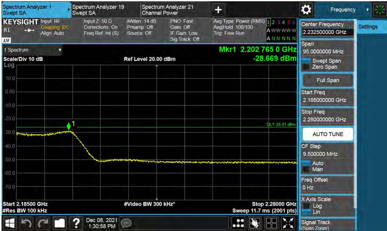
Antenna 0 / High Edge + 100 MHz ~ 10 GHz / (2 Port) B66 DSS 20 MHz 9to1 1 Carrier + LTE B66 10 MHz 1 Carrier + LTE B66 5 MHz 1 Carrier + LTE B66 5 MHz 1 Carrier [4 Carrier] (1C+3C) / Non-Contiguous / 16QAM
