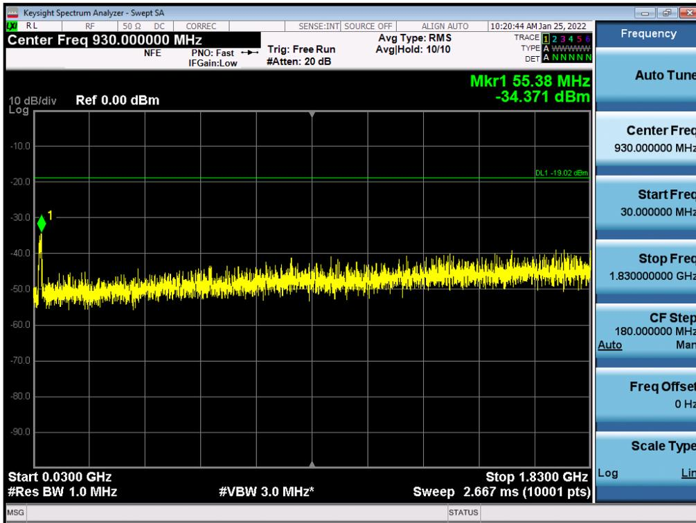
**Antenna 2 / Low Edge - 100 MHz ~ Low Edge / (4 Port) LTE B2 5 MHz 1 Carrier + LTE B2 5 MHz 1 Carrier + 5G NR n2 5 MHz 1 Carrier [3 Carrier] (1C+2C) / Non-Contiguous / 256QAM**
