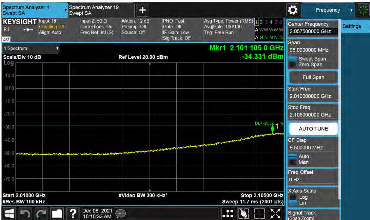
Antenna 0 / High Edge ~ High Edge + 100 MHz / (4 Port) B66 DSS 20 MHz 9to1 1 Carrier + LTE B66 10 MHz 1 Carrier + LTE B66 5 MHz 1 Carrier + LTE B66 5 MHz 1 Carrier [4 Carrier] (3C+1C) / Non-Contiguous / 64QAM
