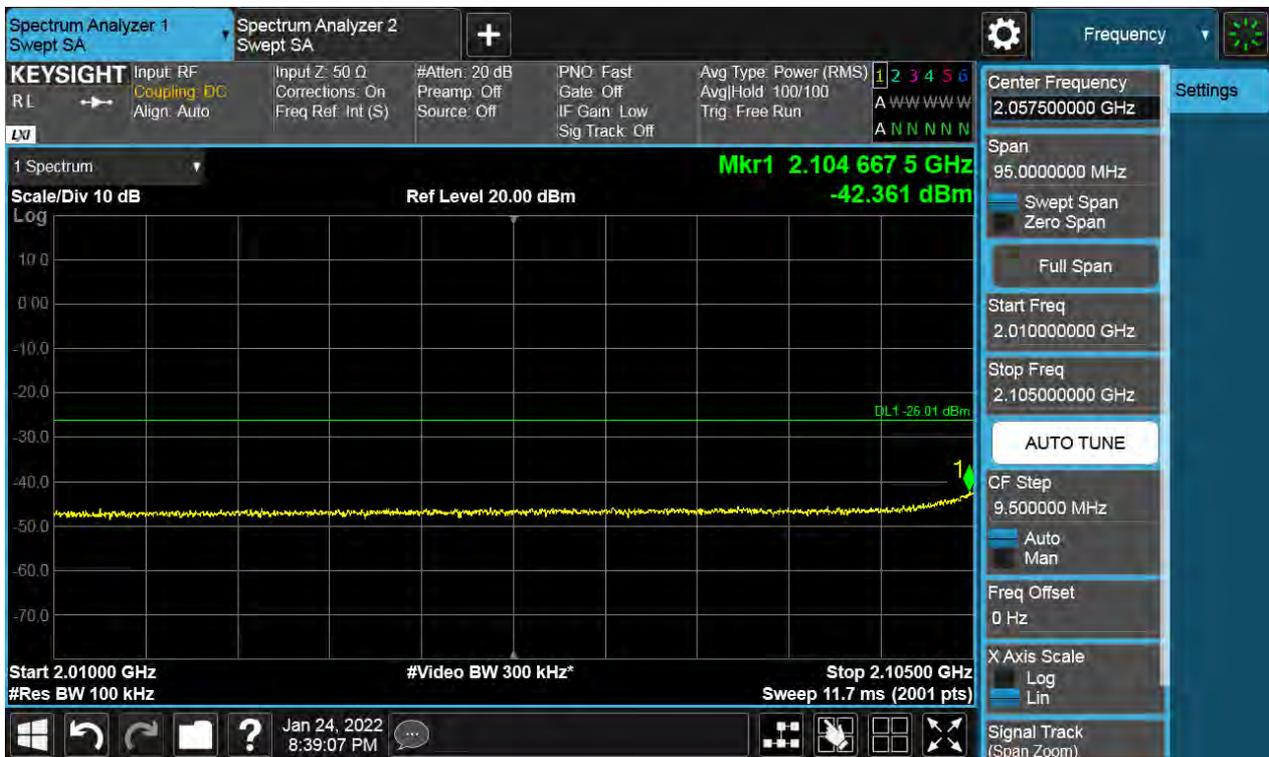
**Antenna 0 / High Edge ~ High Edge + 100 MHz / (2 Port) LTE B66 5 MHz 1 Carrier + LTE B66 5 MHz 1 Carrier + LTE B66 5 MHz 1 Carrier + 5G NR n66 5 MHz 1 Carrier [4 Carrier] (1C+3C) / Non-Contiguous / 16QAM**
