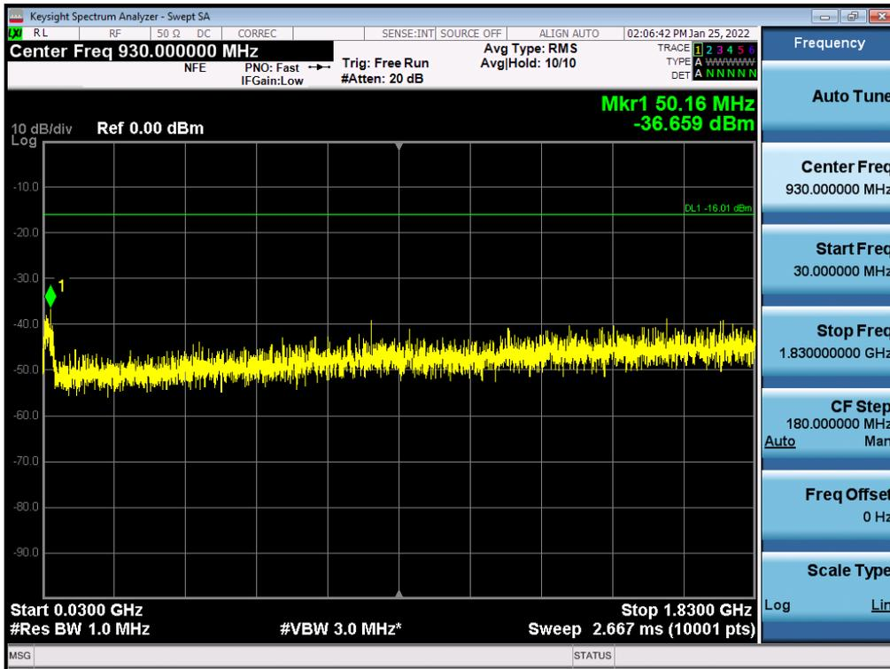
**Antenna 1 / Low Edge - 100 MHz ~ Low Edge / (2 Port) LTE B2 5 MHz 1 Carrier + LTE B2 5 MHz 1 Carrier + 5G NR n2 20 MHz 1 Carrier [3 Carrier] (1C+2C) / Non-Contiguous / 256QAM**
