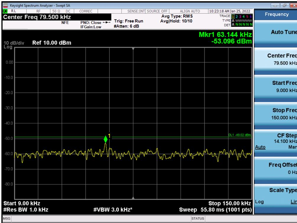
Antenna 2 / 150 kHz ~ 30 MHz / (4 Port) LTE B2 5 MHz 1 Carrier + LTE B2 5 MHz 1 Carrier + 5G NR n2 5 MHz 1 Carrier [3 Carrier] (1C+2C) / Non-Contiguous / 256QAM
