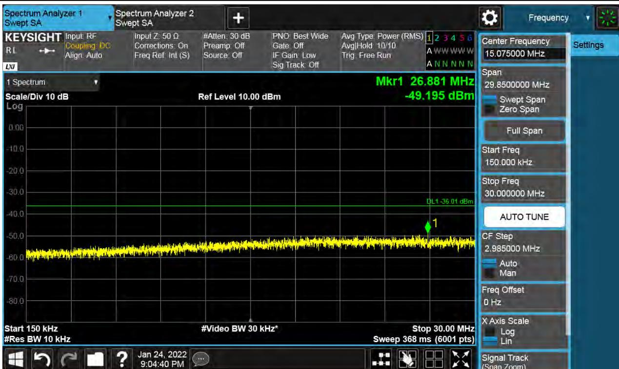
Antenna 0 / 30 MHz ~ Low Edge - 100 MHz / (2 Port) LTE B66 5 MHz 1 Carrier + LTE B66 5 MHz 1 Carrier + LTE B66 5 MHz 1 Carrier + 5G NR n66 5 MHz 1 Carrier [4 Carrier] (1C+3C) / Non-Contiguous / QPSK
