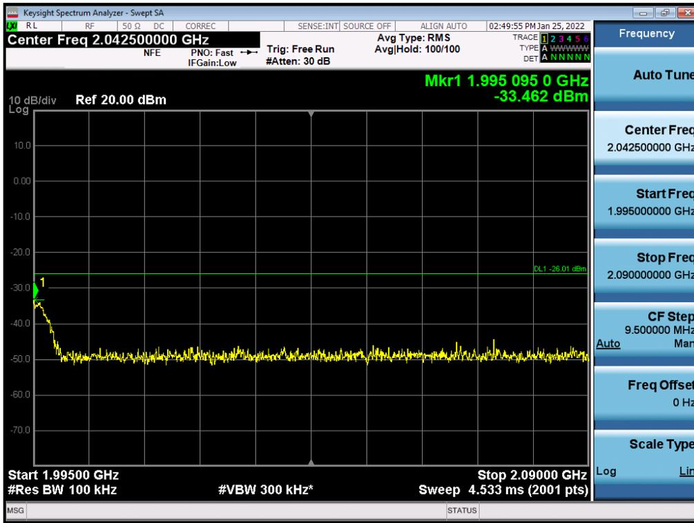
Antenna 0 / High Edge + 100 MHz ~ 10 GHz / (2 Port) LTE B2 5 MHz 1 Carrier + LTE B2 5 MHz 1 Carrier + 5G NR n2 20 MHz 1 Carrier [3 Carrier] (2C+1C) / Non-Contiguous / 16QAM
