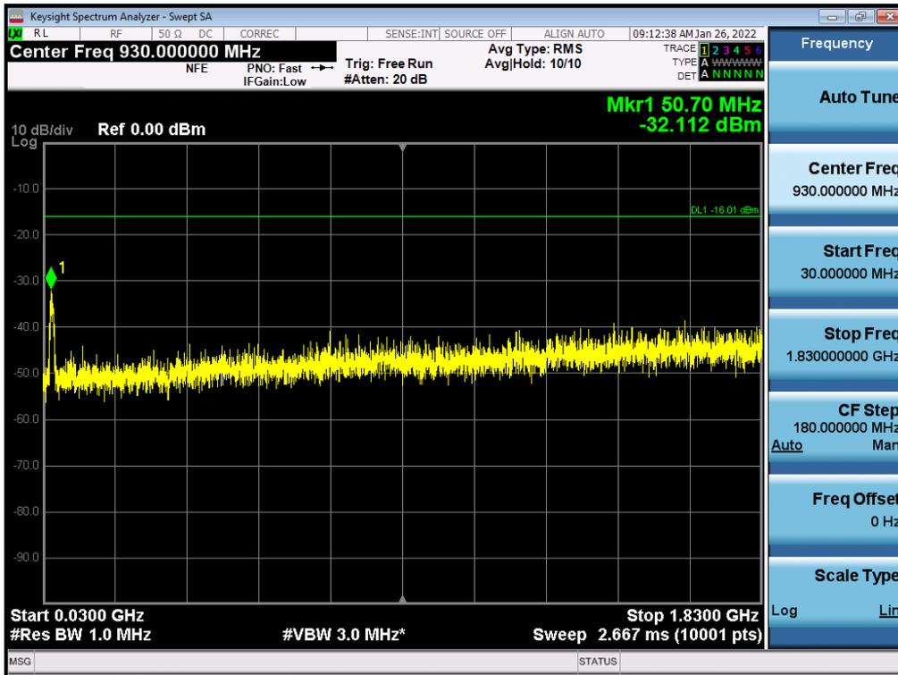
Antenna 1 / Low Edge - 100 MHz ~ Low Edge / (2 Port) LTE B2 5 MHz 1 Carrier + LTE B2 5 MHz 1 Carrier + 5G NR n2 5 MHz 1 Carrier [3 Carrier] (2C+1C) / Non-Contiguous / 256QAM
