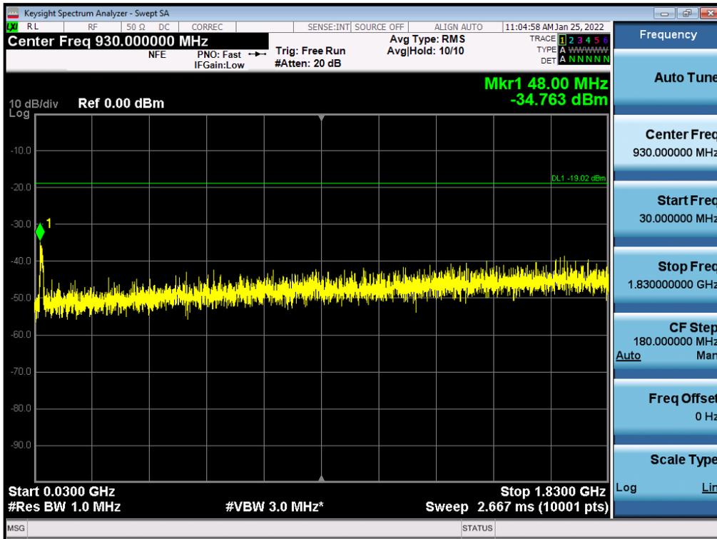
**Antenna 2 / Low Edge - 100 MHz ~ Low Edge / (4 Port) LTE B2 5 MHz 1 Carrier + LTE B2 5 MHz 1 Carrier + 5G NR n2 5 MHz 1 Carrier [3 Carrier] (2C+1C) / Non-Contiguous / QPSK**
