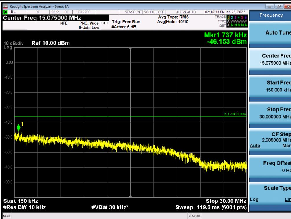
Antenna 0 / 30 MHz ~ Low Edge - 100 MHz / (2 Port) LTE B2 5 MHz 1 Carrier + LTE B2 5 MHz 1 Carrier + 5G NR n2 20 MHz 1 Carrier [3 Carrier] (2C+1C) / Non-Contiguous / QPSK
