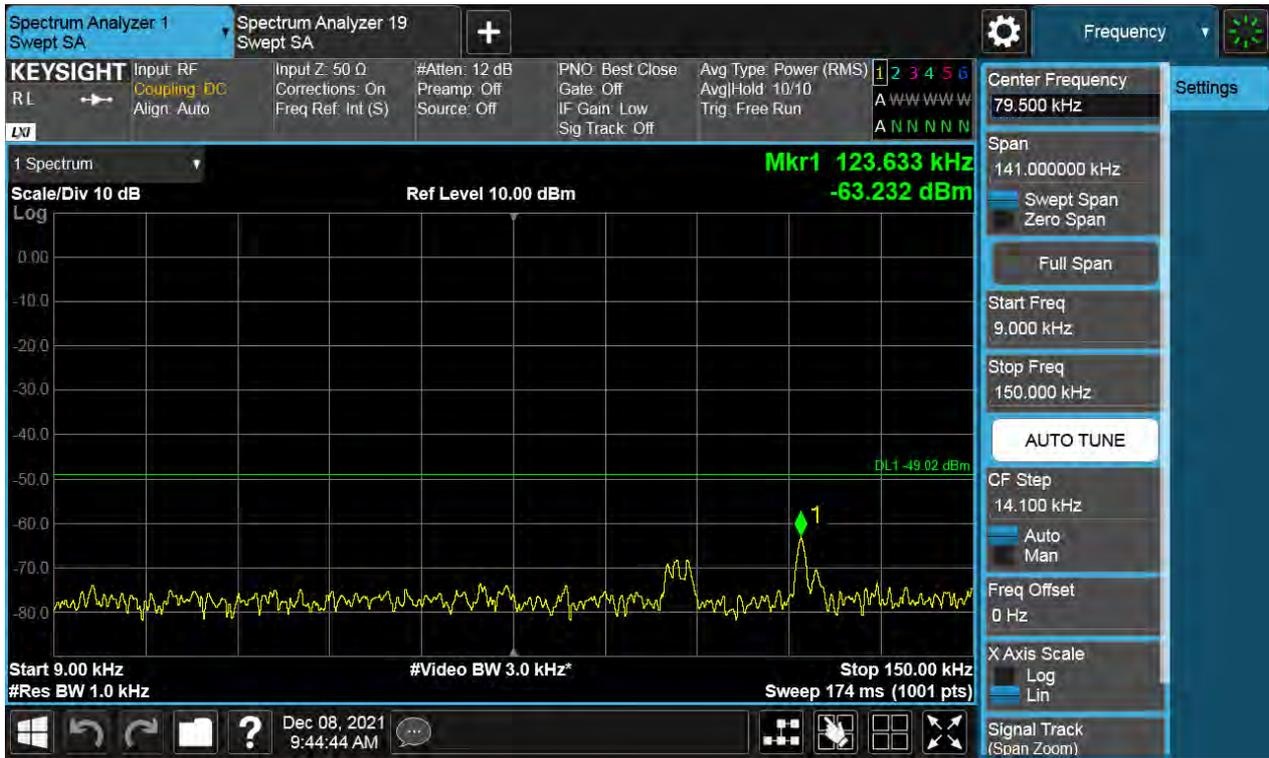
Antenna 3 / 150 kHz ~ 30 MHz / (4 Port) B66 DSS 20 MHz 9to1 1 Carrier + LTE B66 10 MHz 1 Carrier + LTE B66 5 MHz 1 Carrier + LTE B66 5 MHz 1 Carrier [4 Carrier] (3C+1C) / Non-Contiguous / 256QAM
