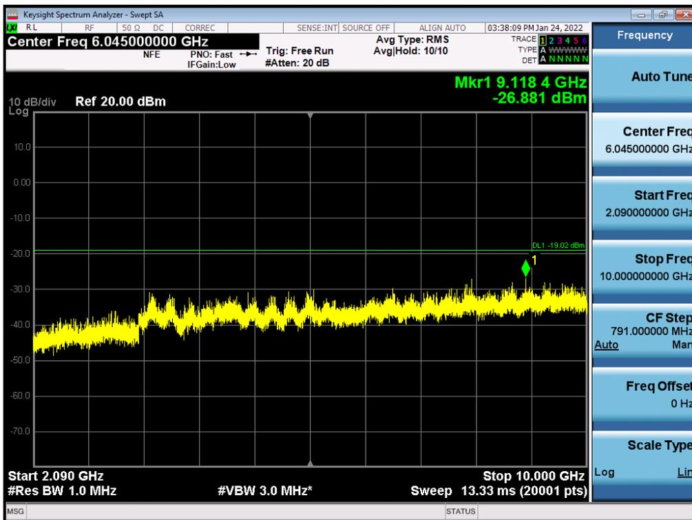
Antenna 1 / 10 GHz ~ 26.5 GHz / (4 Port) LTE B2 5 MHz 1 Carrier + LTE B2 5 MHz 1 Carrier + 5G NR n2 20 MHz 1 Carrier [3 Carrier] (2C+1C) / Non-Contiguous / 256QAM
