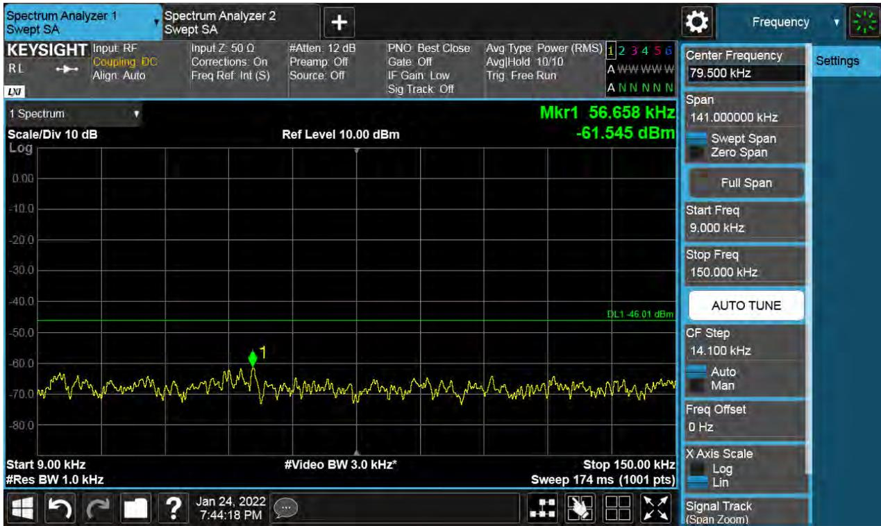
**Antenna 1 / 150 kHz ~ 30 MHz / (2 Port) LTE B66 5 MHz 1 Carrier + LTE B66 5 MHz 1 Carrier + LTE B66 5 MHz 1 Carrier + 5G NR n66 5 MHz 1 Carrier [4 Carrier] (3C+1C) / Non-Contiguous / 16QAM**
