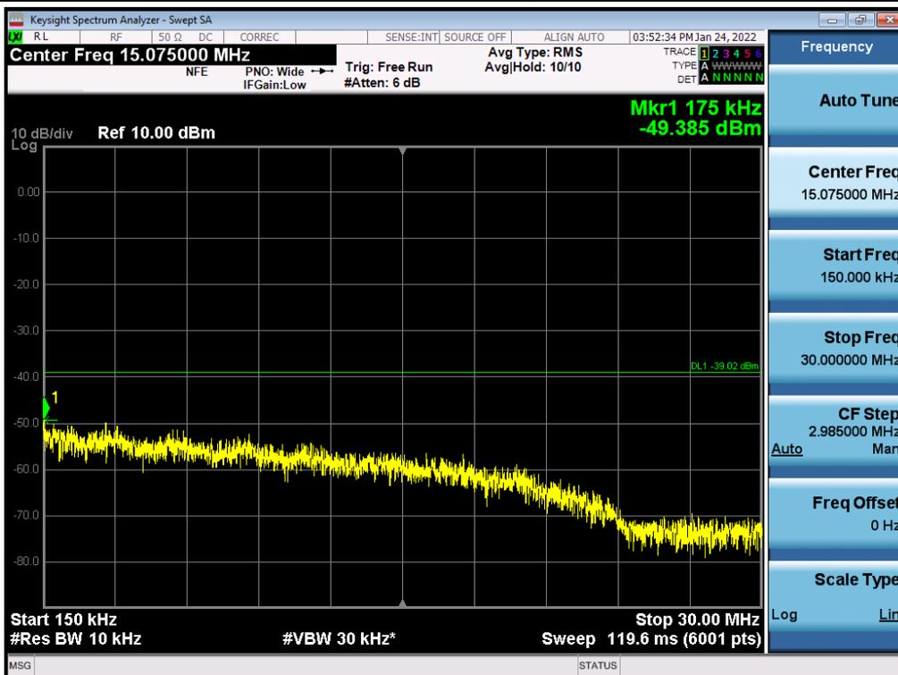
Antenna 2 / 30 MHz ~ Low Edge - 100 MHz / (4 Port) LTE B2 5 MHz 1 Carrier + LTE B2 5 MHz 1 Carrier + 5G NR n2 20 MHz 1 Carrier [3 Carrier] (2C+1C) / Non-Contiguous / 16QAM
