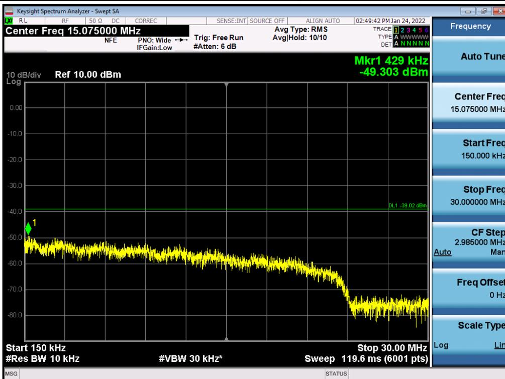
Antenna 2 / 30 MHz ~ Low Edge - 100 MHz / (4 Port) LTE B2 5 MHz 1 Carrier + LTE B2 5 MHz 1 Carrier + 5G NR n2 20 MHz 1 Carrier [3 Carrier] (1C+2C) / Non-Contiguous / 16QAM
