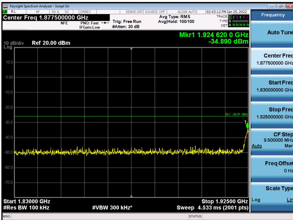
Antenna 1 / High Edge ~ High Edge + 100 MHz / (2 Port) LTE B2 5 MHz 1 Carrier + LTE B2 5 MHz 1 Carrier + 5G NR n2 20 MHz 1 Carrier [3 Carrier] (2C+1C) / Non-Contiguous / 16QAM
