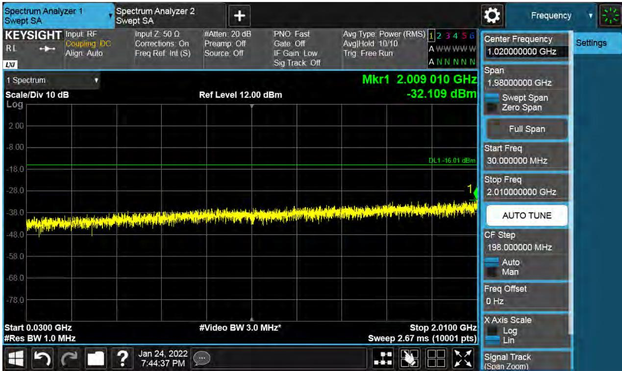
Antenna 1 / Low Edge - 100 MHz ~ Low Edge / (2 Port) LTE B66 5 MHz 1 Carrier + LTE B66 5 MHz 1 Carrier + LTE B66 5 MHz 1 Carrier + 5G NR n66 5 MHz 1 Carrier [4 Carrier] (3C+1C) / Non-Contiguous / 16QAM
