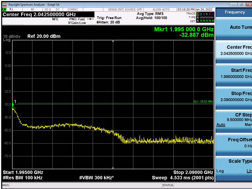
Antenna 0 / High Edge + 100 MHz ~ 10 GHz / (4 Port) LTE B2 5 MHz 1 Carrier + LTE B2 5 MHz 1 Carrier + 5G NR n2 20 MHz 1 Carrier [3 Carrier] (1C+2C) / Non-Contiguous / 64QAM
