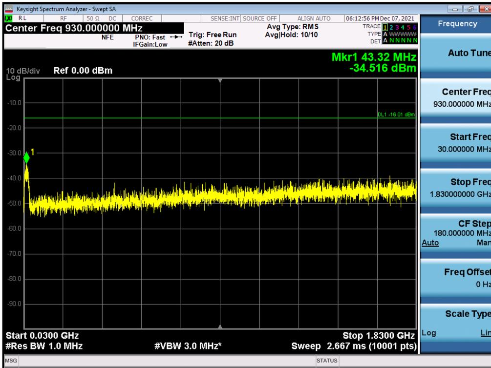
Antenna 1 / Low Edge - 100 MHz ~ Low Edge / (2 Port) B2 DSS 20 MHz 9to1 1 Carrier + LTE B2 5 MHz 1 Carrier + LTE B2 5 MHz 1 Carrier [3 Carrier] (2C+1C) / Non-Contiguous / QPSK
