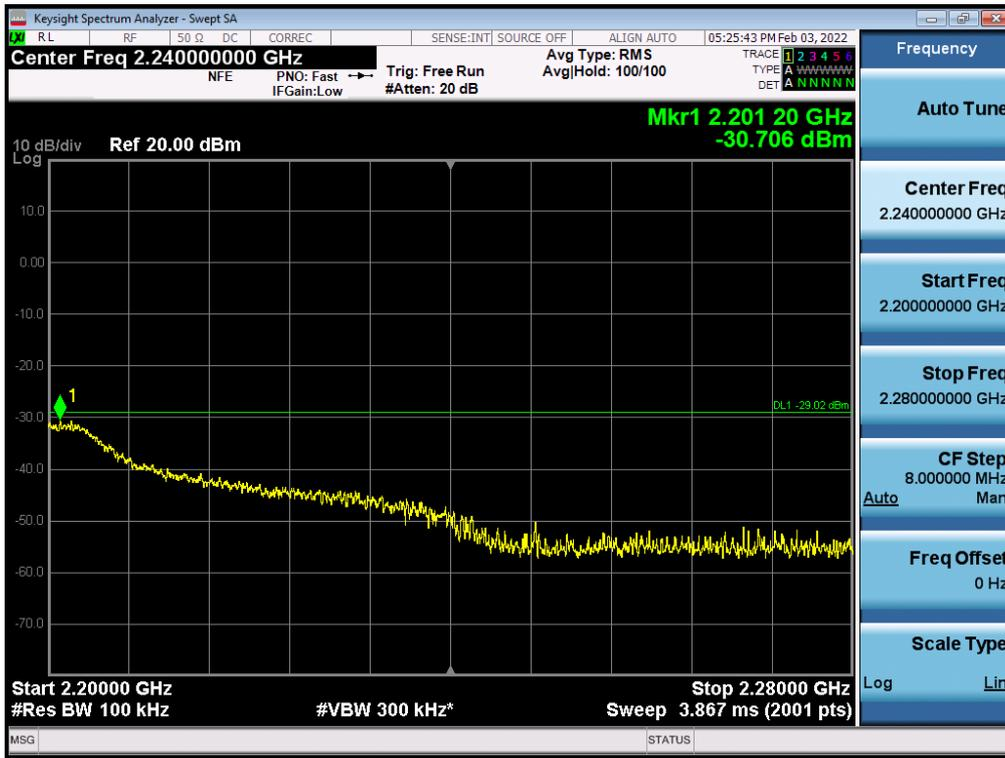
Antenna 3 / High Edge + 100 MHz ~ 10 GHz / (4 Port) LTE B66 20 MHz 1 Carrier + 5G NR n66 20 MHz 1 Carrier [2 Carrier] / Non-Contiguous / 16QAM
