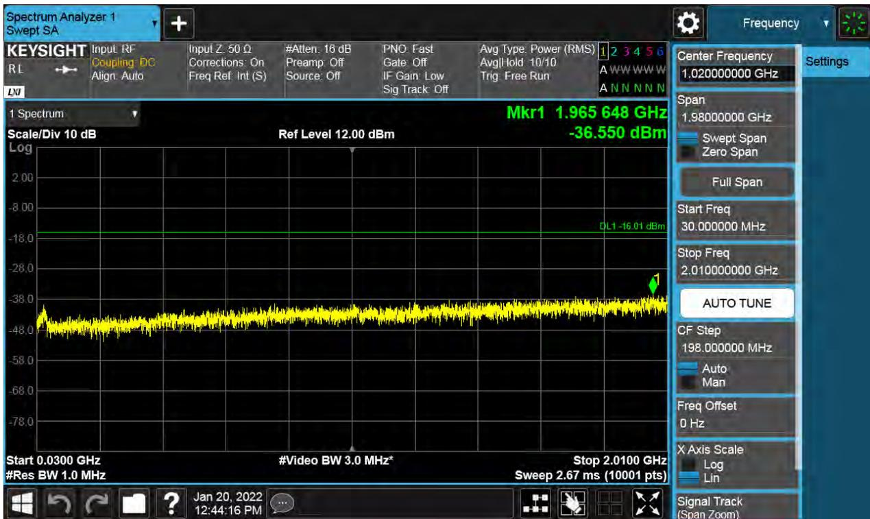
Antenna 0 / Low Edge - 100 MHz ~ Low Edge / (2 Port) LTE B66 20 MHz 1 Carrier + 5G NR n66 20 MHz 1 Carrier [2 Carrier] / Non-Contiguous / QPSK
