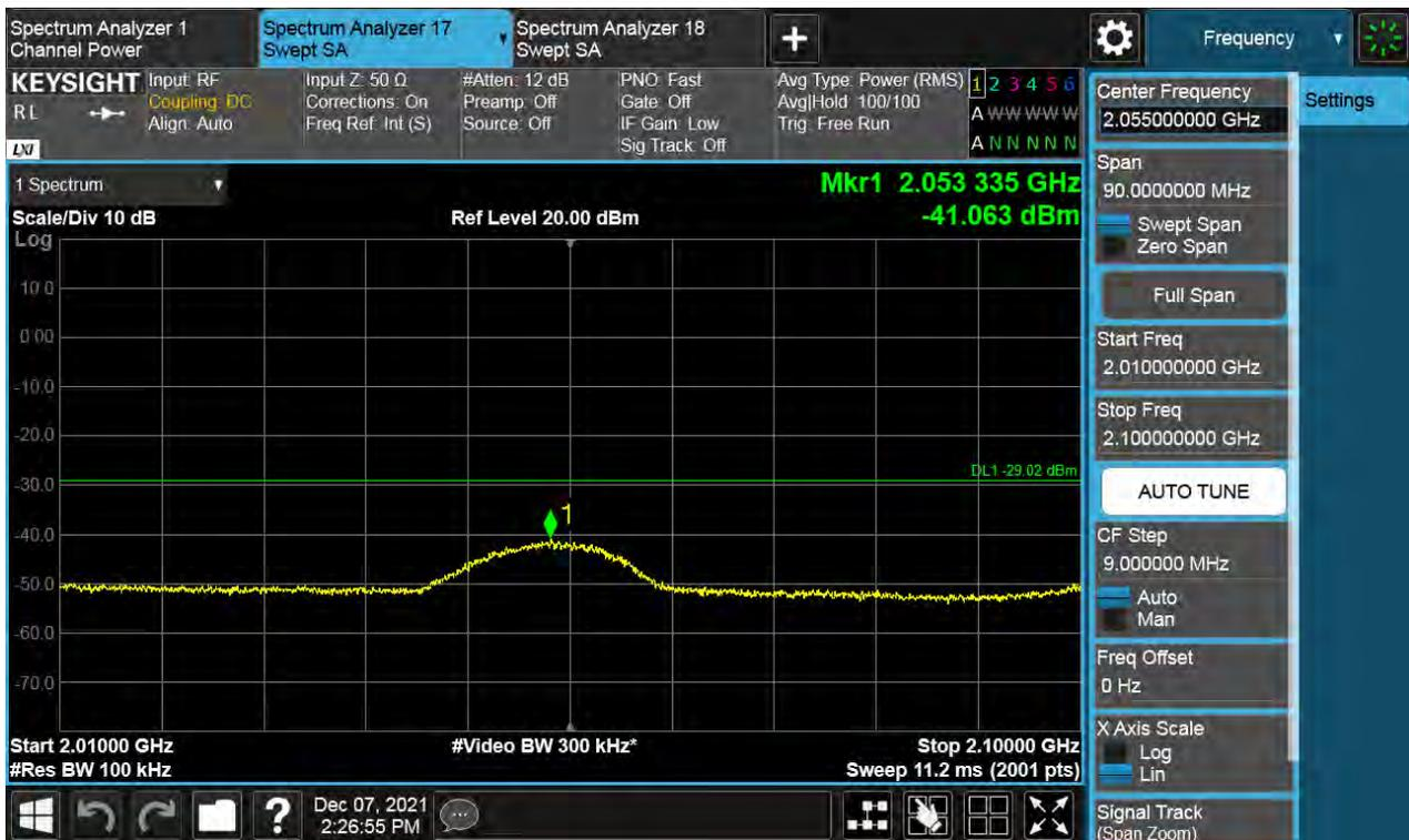
Antenna 0 / High Edge ~ High Edge + 100 MHz / (4 Port) B66 DSS 10 MHz 9to1 1 Carrier + LTE B66 5 MHz 1 Carrier [2 Carrier] / Non-Contiguous / 16QAM
