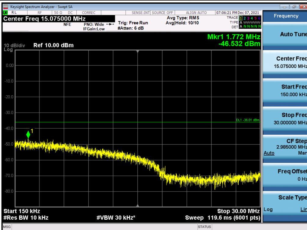
Antenna 0 / 30 MHz ~ Low Edge - 100 MHz / (2 Port) B2 DSS 20 MHz 9to1 1 Carrier + LTE B2 5 MHz 1 Carrier + LTE B2 5 MHz 1 Carrier [3 Carrier] (1C+2C) / Non-Contiguous / 64QAM
