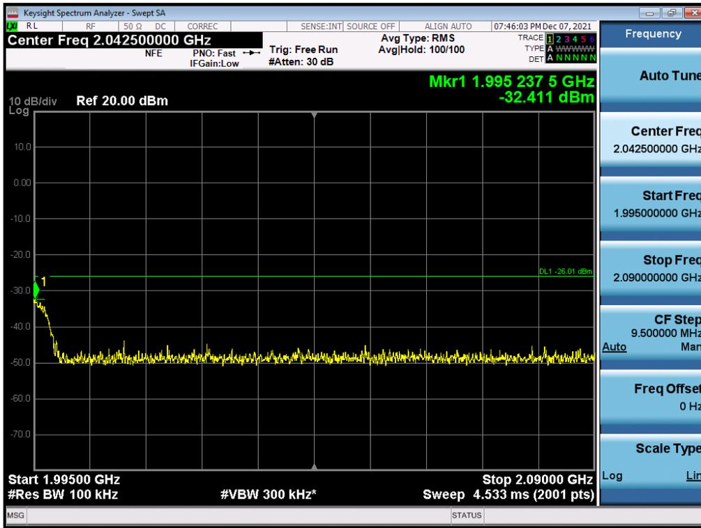
Antenna 0 / High Edge + 100 MHz ~ 10 GHz / (2 Port) B2 DSS 20 MHz 9to1 1 Carrier + LTE B2 5 MHz 1 Carrier + LTE B2 5 MHz 1 Carrier [3 Carrier] (1C+2C) / Non-Contiguous / 16QAM
