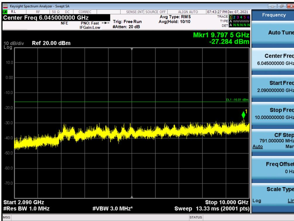
Antenna 0 / 10 GHz ~ 26.5 GHz / (2 Port) B2 DSS 20 MHz 9to1 1 Carrier + LTE B2 5 MHz 1 Carrier + LTE B2 5 MHz 1 Carrier [3 Carrier] (1C+2C) / Non-Contiguous / 16QAM
