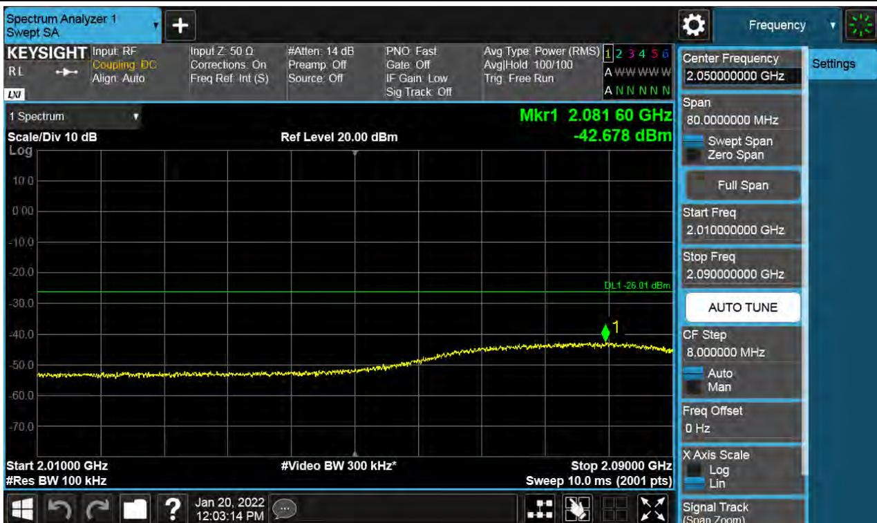
Antenna 0 / High Edge ~ High Edge + 100 MHz / (2 Port) LTE B66 20 MHz 1 Carrier + 5G NR n66 20 MHz 1 Carrier [2 Carrier] / Non-Contiguous / 16QAM
