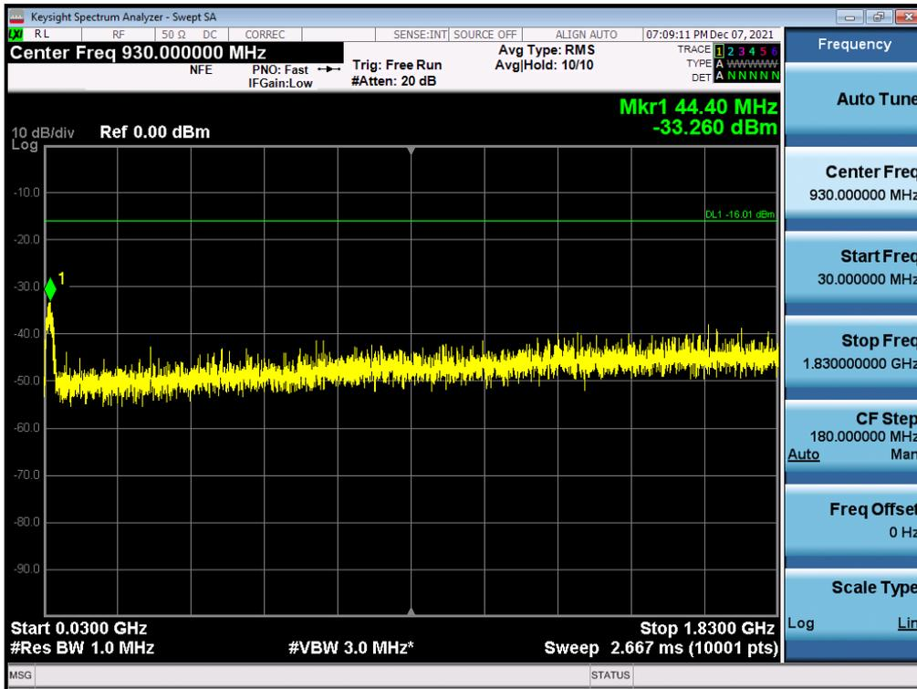
Antenna 1 / Low Edge - 100 MHz ~ Low Edge / (2 Port) B2 DSS 20 MHz 9to1 1 Carrier + LTE B2 5 MHz 1 Carrier + LTE B2 5 MHz 1 Carrier [3 Carrier] (1C+2C) / Non-Contiguous / 64QAM
