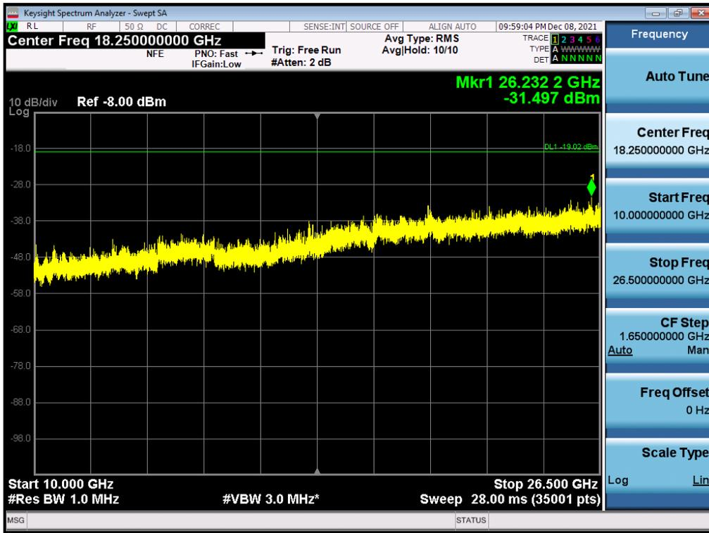
Antenna 3 / 9 kHz ~ 150 kHz / (4 Port) B2 DSS 20 MHz 9to1 1 Carrier + LTE B2 5 MHz 1 Carrier + LTE B2 5 MHz 1 Carrier [3 Carrier] (2C+1C) / Non-Contiguous / 16QAM
