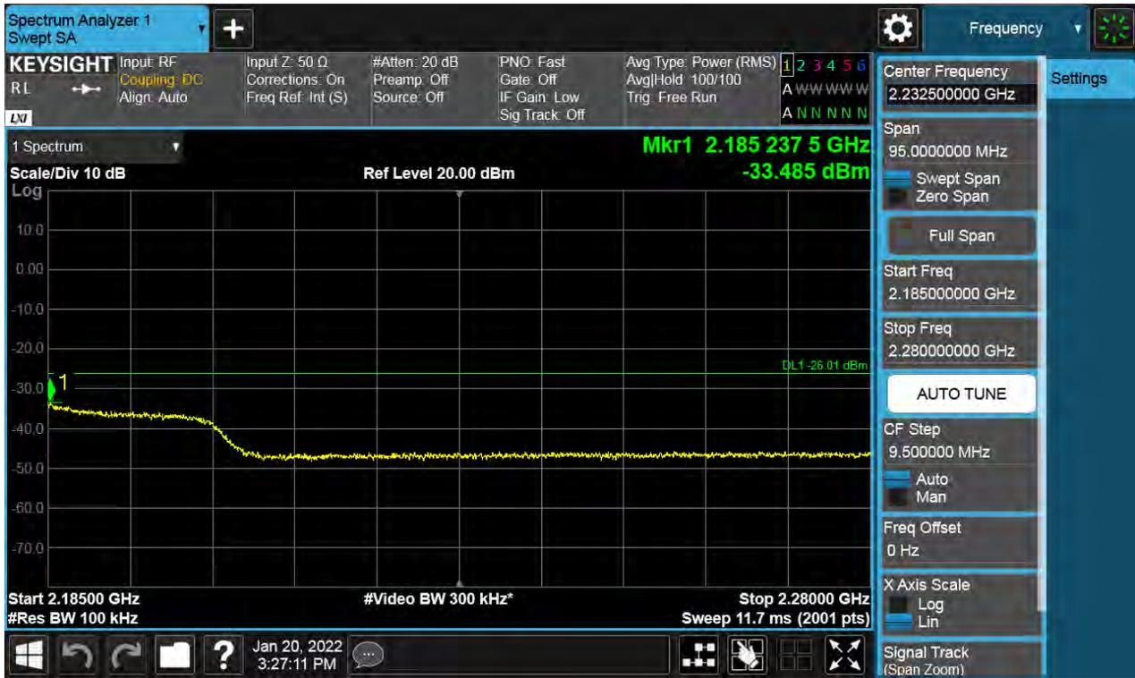
Antenna 1 / High Edge + 100 MHz ~ 10 GHz / (2 Port) LTE B66 5 MHz 1 Carrier + 5G NR n66 5 MHz 1 Carrier [2 Carrier] / Non-Contiguous / 256QAM
