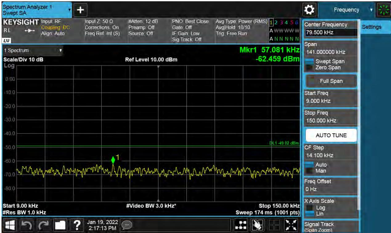
Antenna 3 / 150 kHz ~ 30 MHz / (4 Port) LTE B66 5 MHz 1 Carrier + 5G NR n66 10 MHz 1 Carrier [2 Carrier] / Non-Contiguous / QPSK
