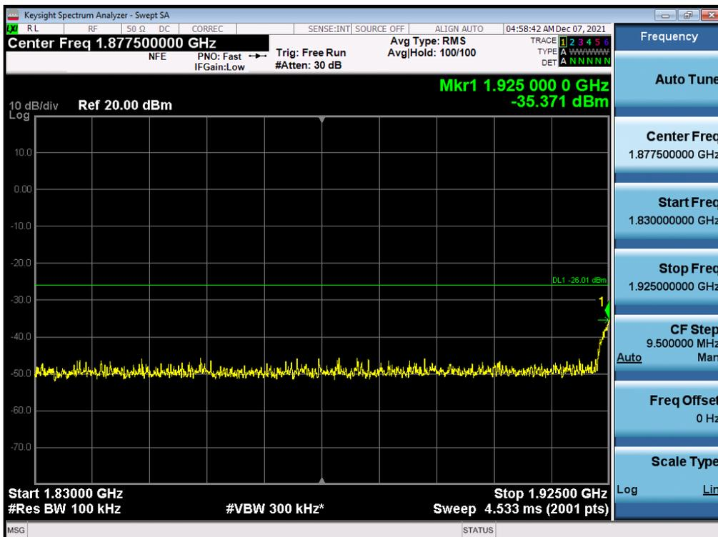
Antenna 1 / High Edge ~ High Edge + 100 MHz / (2 Port) B2 DSS 20 MHz 9to1 1 Carrier + LTE B2 5 MHz 1 Carrier + LTE B2 5 MHz 1 Carrier [3 Carrier] (2C+1C) / Non-Contiguous / QPSK
