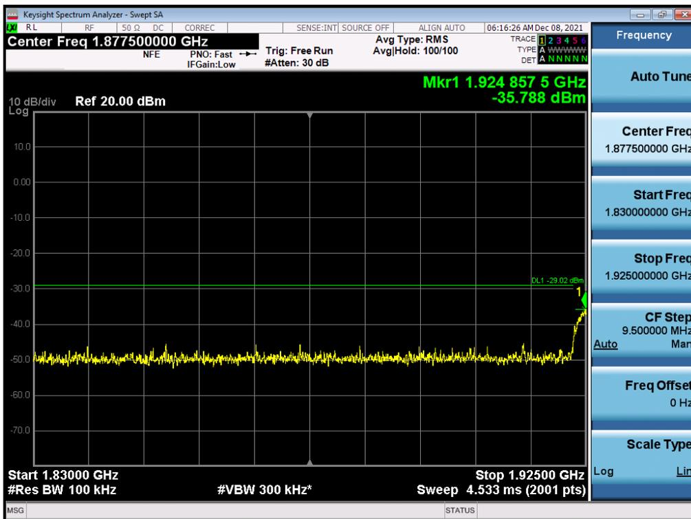
Antenna 1 / High Edge ~ High Edge + 100 MHz / (4 Port) B2 DSS 20 MHz 9to1 1 Carrier + LTE B2 5 MHz 1 Carrier + LTE B2 5 MHz 1 Carrier [3 Carrier] (2C+1C) / Non-Contiguous / QPSK
