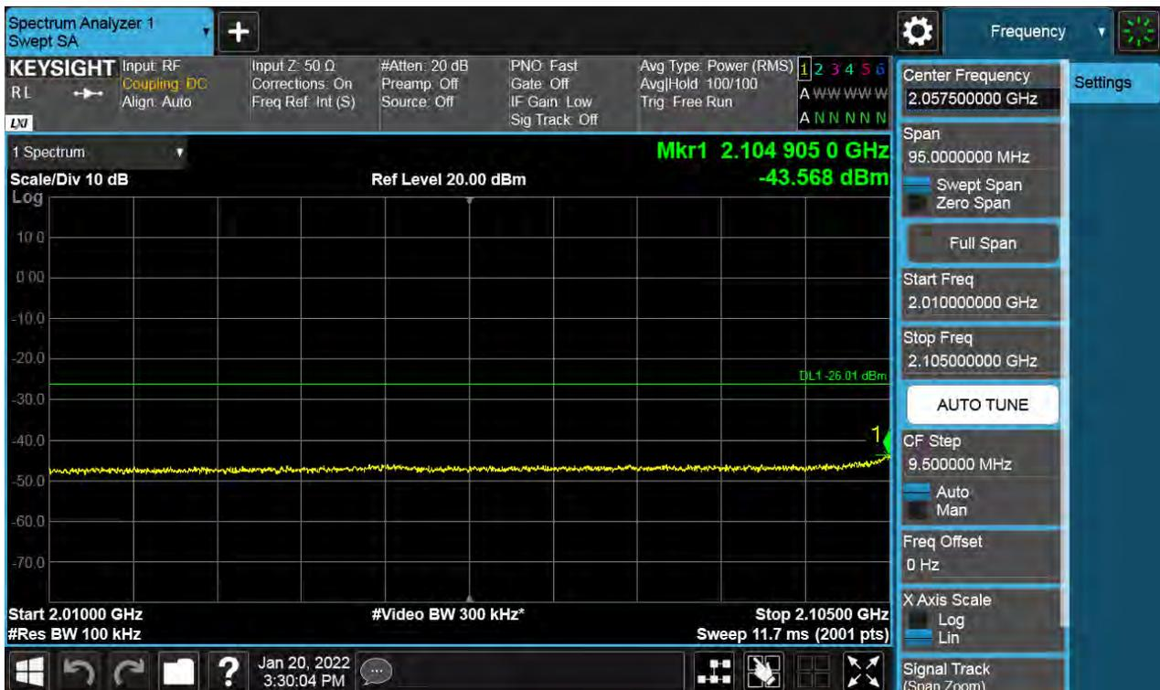
Antenna 0 / High Edge ~ High Edge + 100 MHz / (2 Port) LTE B66 5 MHz 1 Carrier + 5G NR n66 5 MHz 1 Carrier [2 Carrier] / Non-Contiguous / 16QAM
