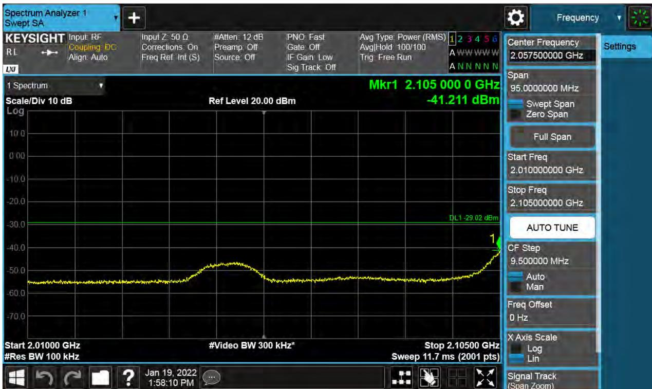
Antenna 0 / High Edge ~ High Edge + 100 MHz / (4 Port) LTE B66 5 MHz 1 Carrier + 5G NR n66 10 MHz 1 Carrier [2 Carrier] / Non-Contiguous / 64QAM
