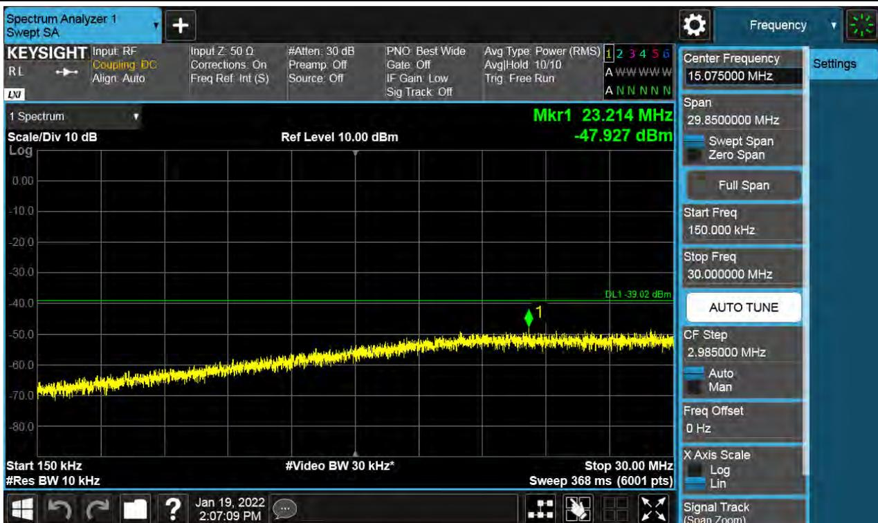
Antenna 0 / 30 MHz ~ Low Edge - 100 MHz / (4 Port) LTE B66 5 MHz 1 Carrier + 5G NR n66 10 MHz 1 Carrier [2 Carrier] / Non-Contiguous / 64QAM
