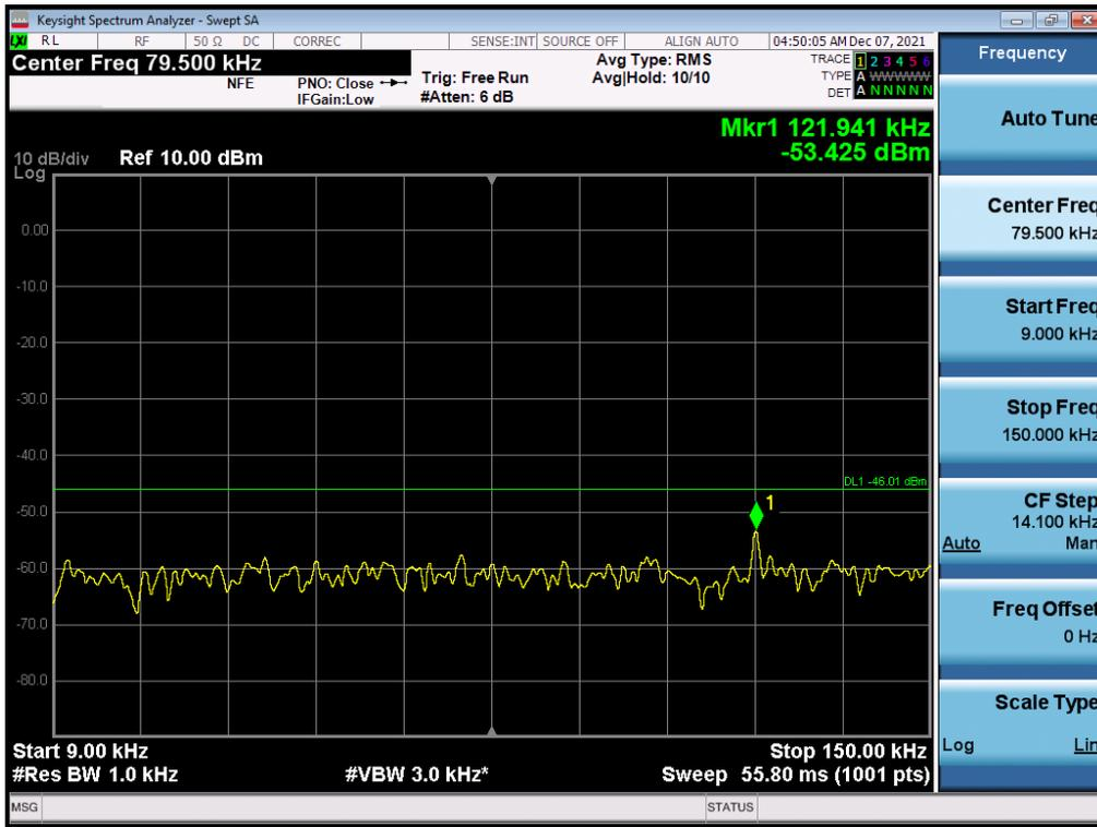
Antenna 1 / 150 kHz ~ 30 MHz / (2 Port) B2 DSS 20 MHz 9to1 1 Carrier + LTE B2 5 MHz 1 Carrier + LTE B2 5 MHz 1 Carrier [3 Carrier] (2C+1C) / Non-Contiguous / QPSK
