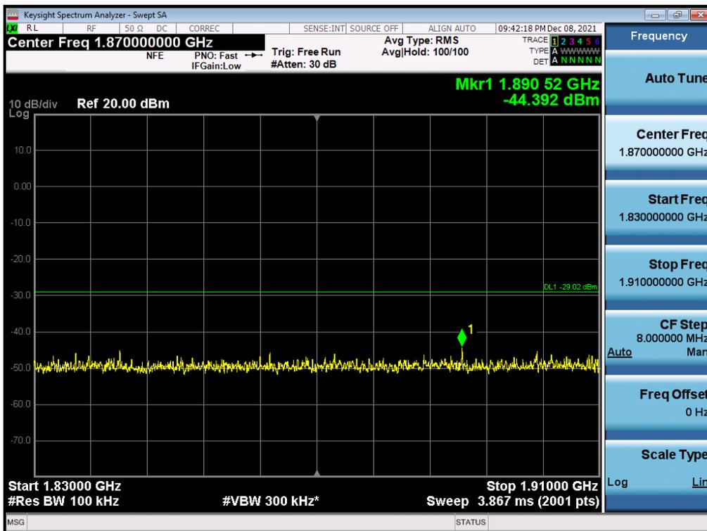
Antenna 2 / High Edge ~ High Edge + 100 MHz / (4 Port) B2 DSS 20 MHz 9to1 1 Carrier + LTE B2 5 MHz 1 Carrier + LTE B2 5 MHz 1 Carrier [3 Carrier] (1C+2C) / Non-Contiguous / 16QAM
