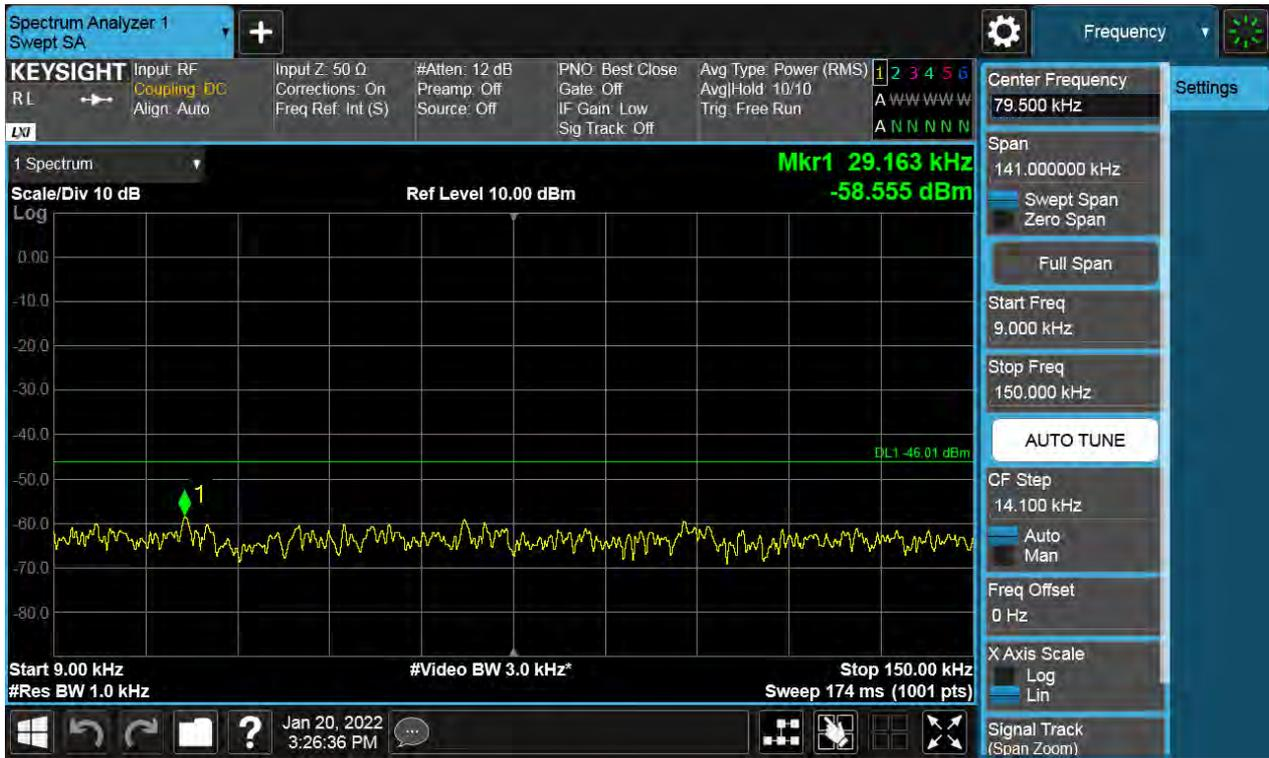
Antenna 1 / 150 kHz ~ 30 MHz / (2 Port) LTE B66 5 MHz 1 Carrier + 5G NR n66 5 MHz 1 Carrier [2 Carrier] / Non-Contiguous / 64QAM
