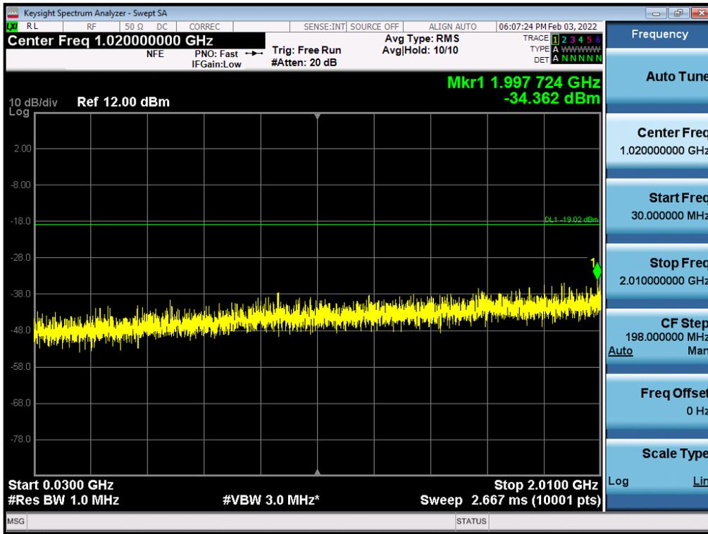
Antenna 0 / Low Edge - 100 MHz ~ Low Edge / (4 Port) LTE B66 20 MHz 1 Carrier + 5G NR n66 20 MHz 1 Carrier [2 Carrier] / Non-Contiguous / 16QAM
