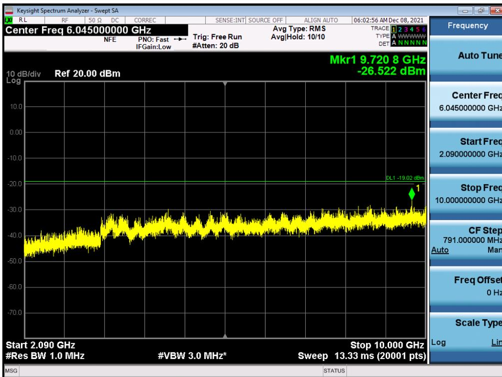
Antenna 3 / 10 GHz ~ 26.5 GHz / (4 Port) B2 DSS 20 MHz 9to1 1 Carrier + LTE B2 5 MHz 1 Carrier + LTE B2 5 MHz 1 Carrier [3 Carrier] (2C+1C) / Non-Contiguous / 64QAM
