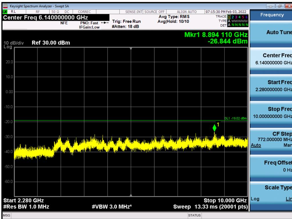
Antenna 3 / 10 GHz ~ 26.5 GHz / (4 Port) LTE B66 20 MHz 1 Carrier + 5G NR n66 20 MHz 1 Carrier [2 Carrier] / Non-Contiguous / 256QAM
