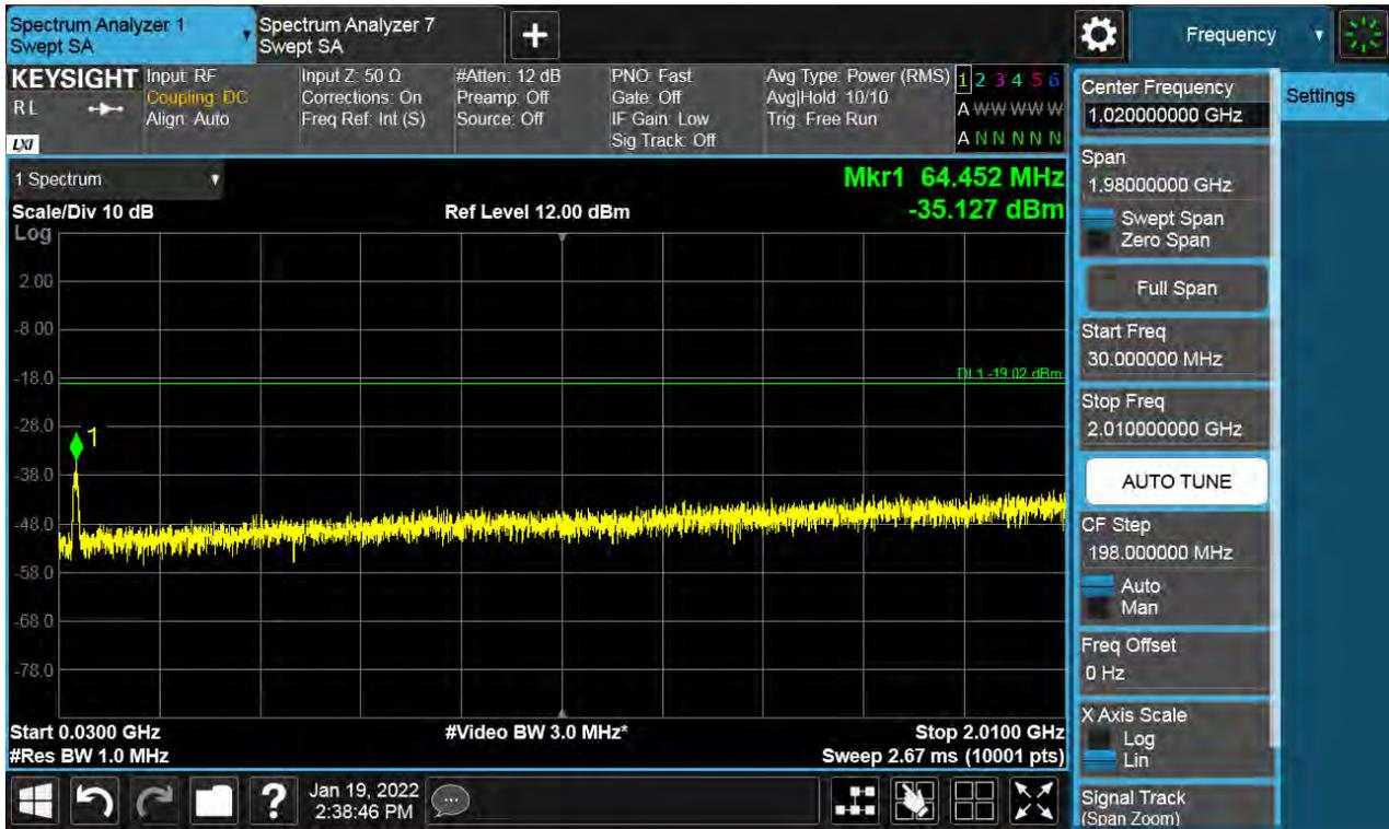
Antenna 0 / Low Edge - 100 MHz ~ Low Edge / (4 Port) LTE B66 5 MHz 1 Carrier + 5G NR n66 10 MHz 1 Carrier [2 Carrier] / Non-Contiguous / QPSK
