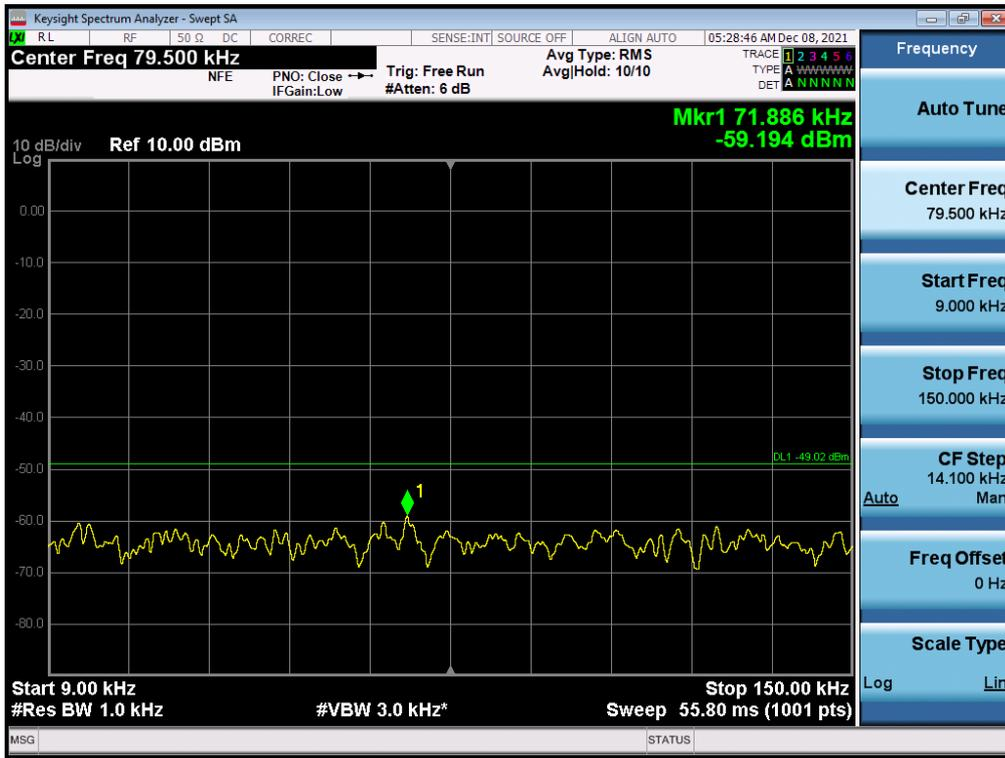
Antenna 2 / 150 kHz ~ 30 MHz / (4 Port) B2 DSS 20 MHz 9to1 1 Carrier + LTE B2 5 MHz 1 Carrier + LTE B2 5 MHz 1 Carrier [3 Carrier] (2C+1C) / Non-Contiguous / 256QAM
