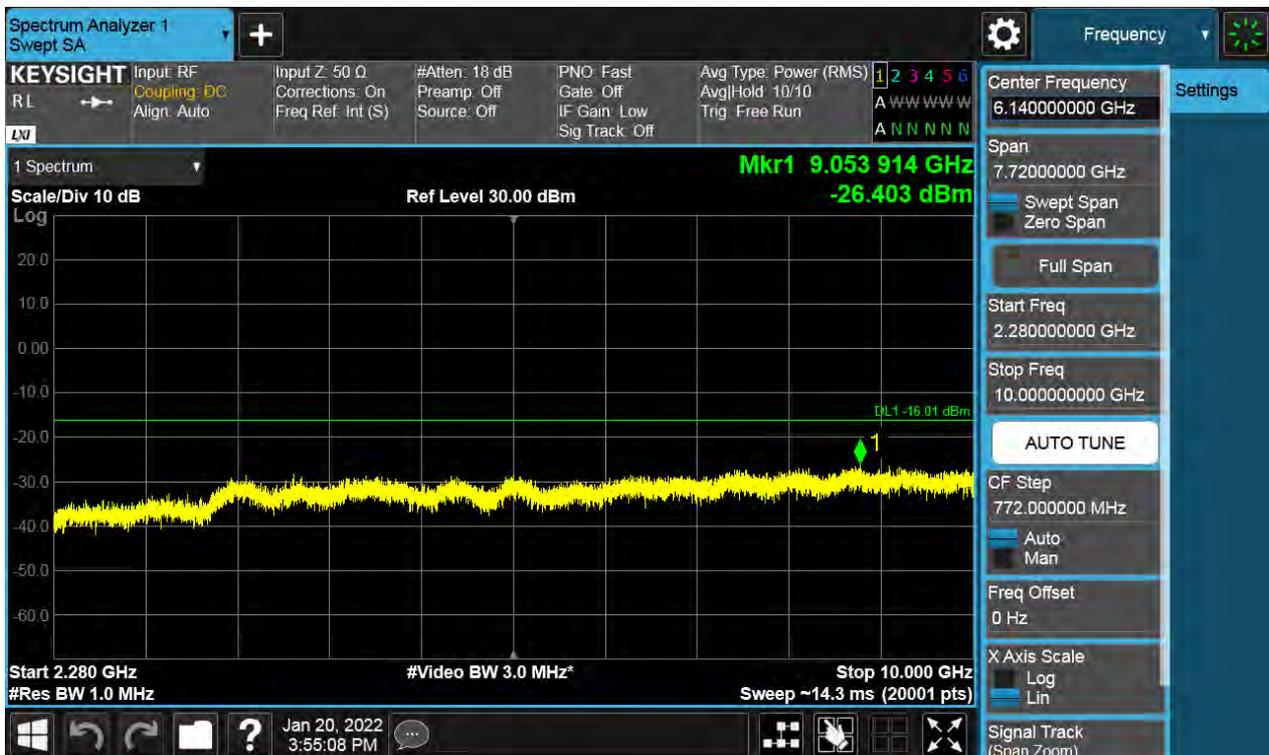
Antenna 1 / 10 GHz ~ 26.5 GHz / (2 Port) LTE B66 5 MHz 1 Carrier + 5G NR n66 5 MHz 1 Carrier [2 Carrier] / Non-Contiguous / 256QAM
