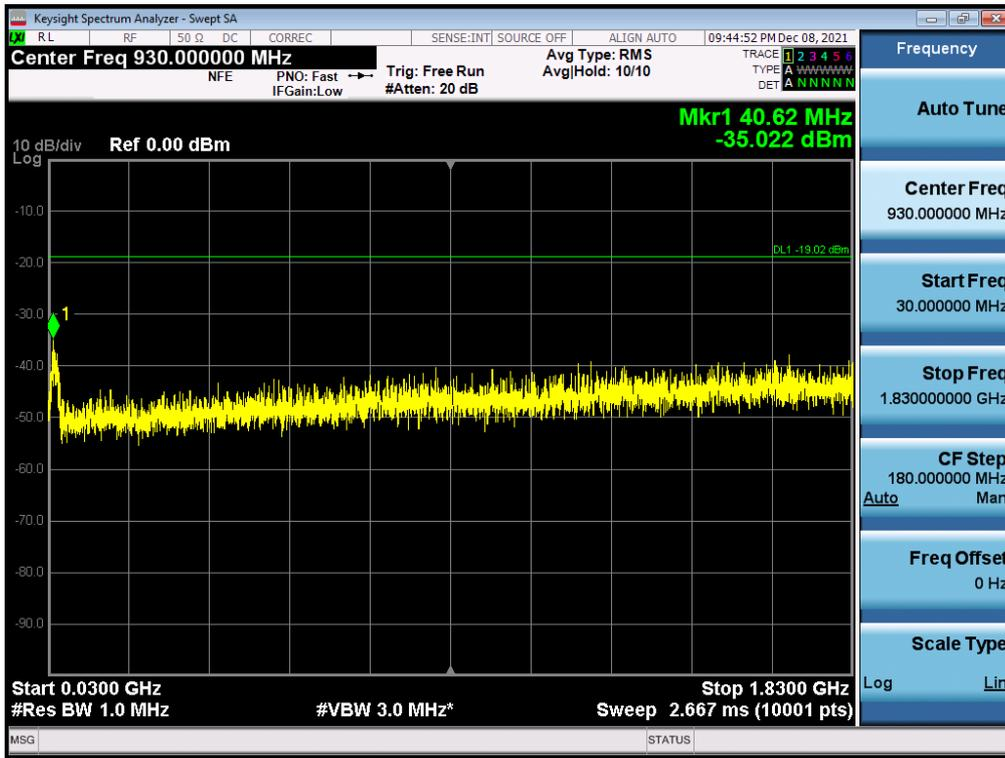
Antenna 1 / Low Edge - 100 MHz ~ Low Edge / (4 Port) B2 DSS 20 MHz 9to1 1 Carrier + LTE B2 5 MHz 1 Carrier + LTE B2 5 MHz 1 Carrier [3 Carrier] (1C+2C) / Non-Contiguous / 64QAM
