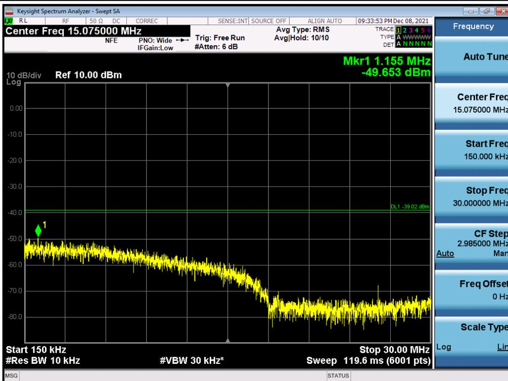
Antenna 1 / 30 MHz ~ Low Edge - 100 MHz / (4 Port) B2 DSS 20 MHz 9to1 1 Carrier + LTE B2 5 MHz 1 Carrier + LTE B2 5 MHz 1 Carrier [3 Carrier] (1C+2C) / Non-Contiguous / 256QAM
