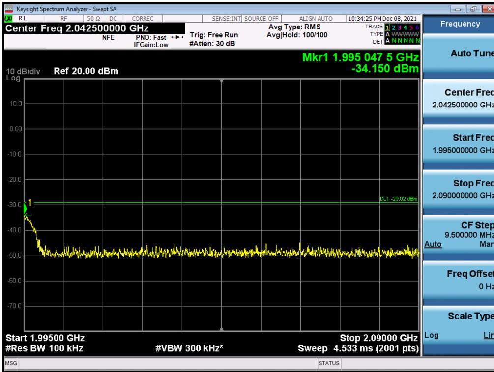
Antenna 0 / High Edge + 100 MHz ~ 10 GHz / (4 Port) B2 DSS 20 MHz 9to1 1 Carrier + LTE B2 5 MHz 1 Carrier + LTE B2 5 MHz 1 Carrier [3 Carrier] (1C+2C) / Non-Contiguous / QPSK
