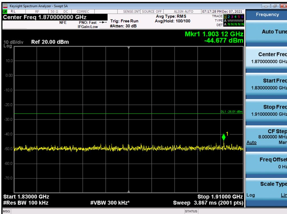
Antenna 1 / High Edge ~ High Edge + 100 MHz / (2 Port) B2 DSS 20 MHz 9to1 1 Carrier + LTE B2 5 MHz 1 Carrier + LTE B2 5 MHz 1 Carrier [3 Carrier] (1C+2C) / Non-Contiguous / 16QAM
