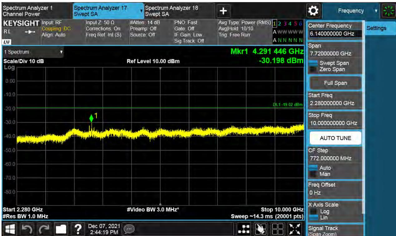
Antenna 1 / 10 GHz ~ 26.5 GHz / (4 Port) B66 DSS 10 MHz 9to1 1 Carrier + LTE B66 5 MHz 1 Carrier [2 Carrier] / Non-Contiguous / QPSK
