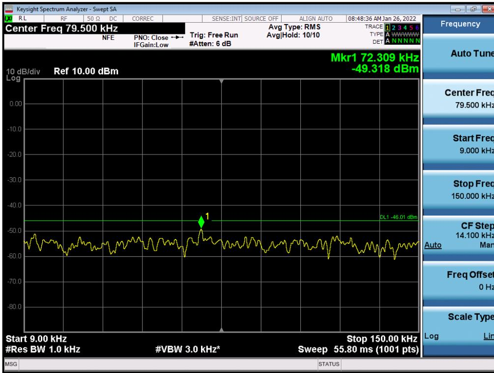
Antenna 0 / 150 kHz ~ 30 MHz / (2 Port) LTE B2 5 MHz 1 Carrier + LTE B2 5 MHz 1 Carrier + 5G NR n2 5 MHz 1 Carrier [3 Carrier] (1C+2C) / Non-Contiguous / 64QAM
