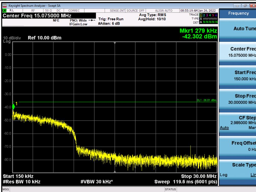
Antenna 0 / 30 MHz ~ Low Edge - 100 MHz / (2 Port) LTE B2 5 MHz 1 Carrier + LTE B2 5 MHz 1 Carrier + 5G NR n2 5 MHz 1 Carrier [3 Carrier] (1C+2C) / Non-Contiguous / 16QAM
