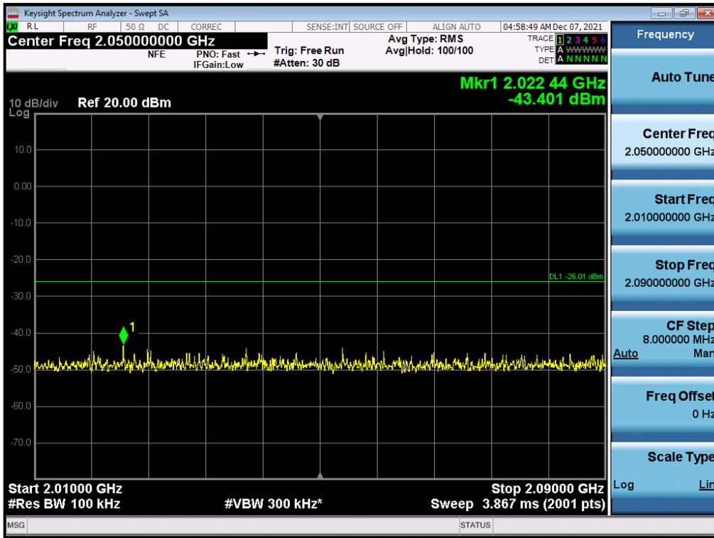
Antenna 1 / High Edge + 100 MHz ~ 10 GHz / (2 Port) B2 DSS 20 MHz 9to1 1 Carrier + LTE B2 5 MHz 1 Carrier + LTE B2 5 MHz 1 Carrier [3 Carrier] (2C+1C) / Non-Contiguous / 256QAM
