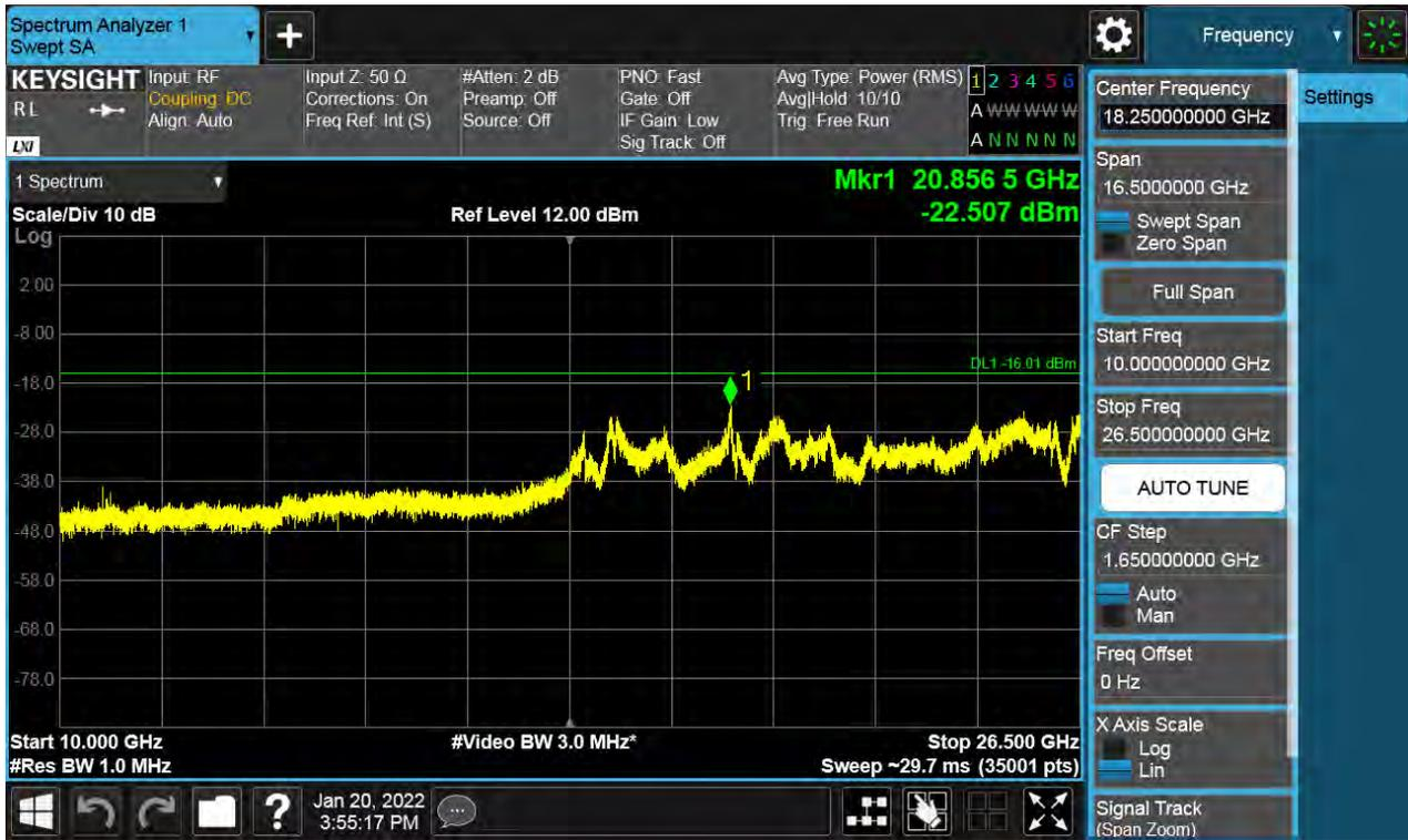
Antenna 1 / 30 MHz ~ Low Edge - 100 MHz / (2 Port) LTE B66 20 MHz 1 Carrier + 5G NR n66 20 MHz 1 Carrier [2 Carrier] / Non-Contiguous / 256QAM
