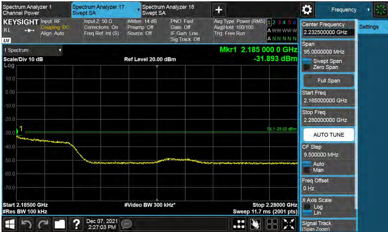
Antenna 0 / High Edge + 100 MHz ~ 10 GHz / (4 Port) B66 DSS 10 MHz 9to1 1 Carrier + LTE B66 5 MHz 1 Carrier [2 Carrier] / Non-Contiguous / 64QAM
