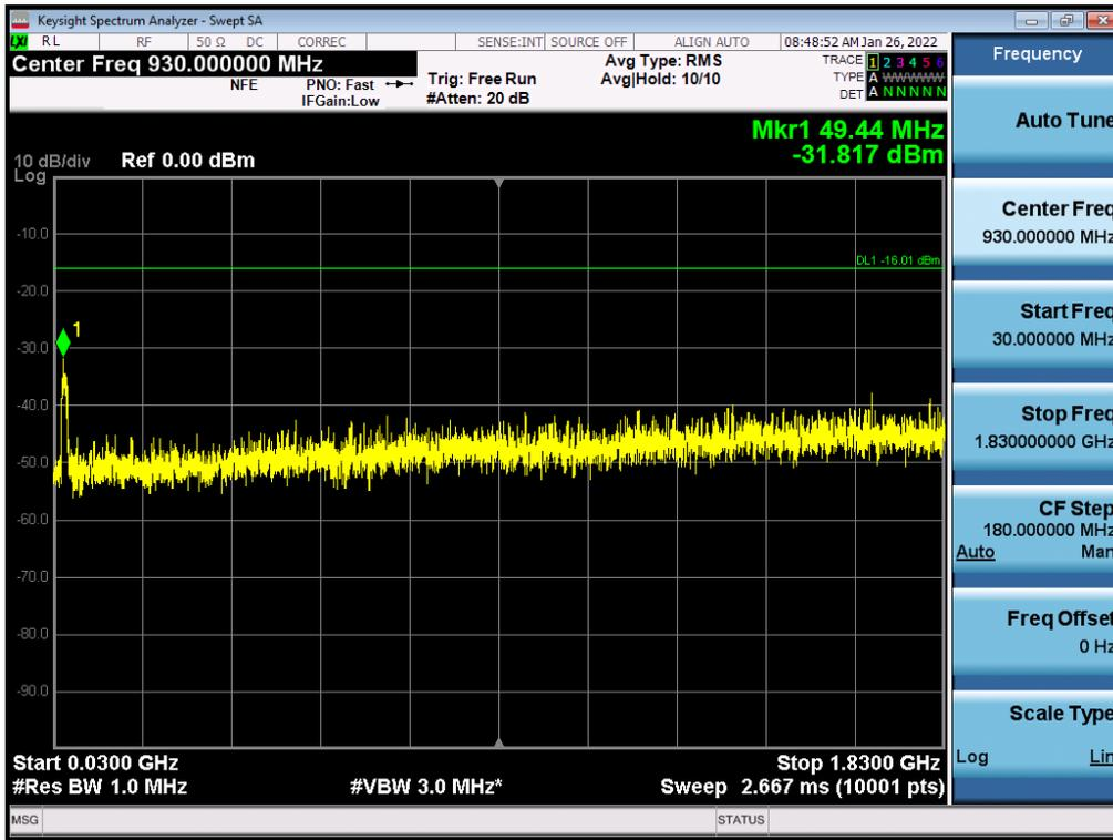
Antenna 1 / Low Edge - 100 MHz ~ Low Edge / (2 Port) LTE B2 5 MHz 1 Carrier + LTE B2 5 MHz 1 Carrier + 5G NR n2 5 MHz 1 Carrier [3 Carrier] (1C+2C) / Non-Contiguous / 64QAM
