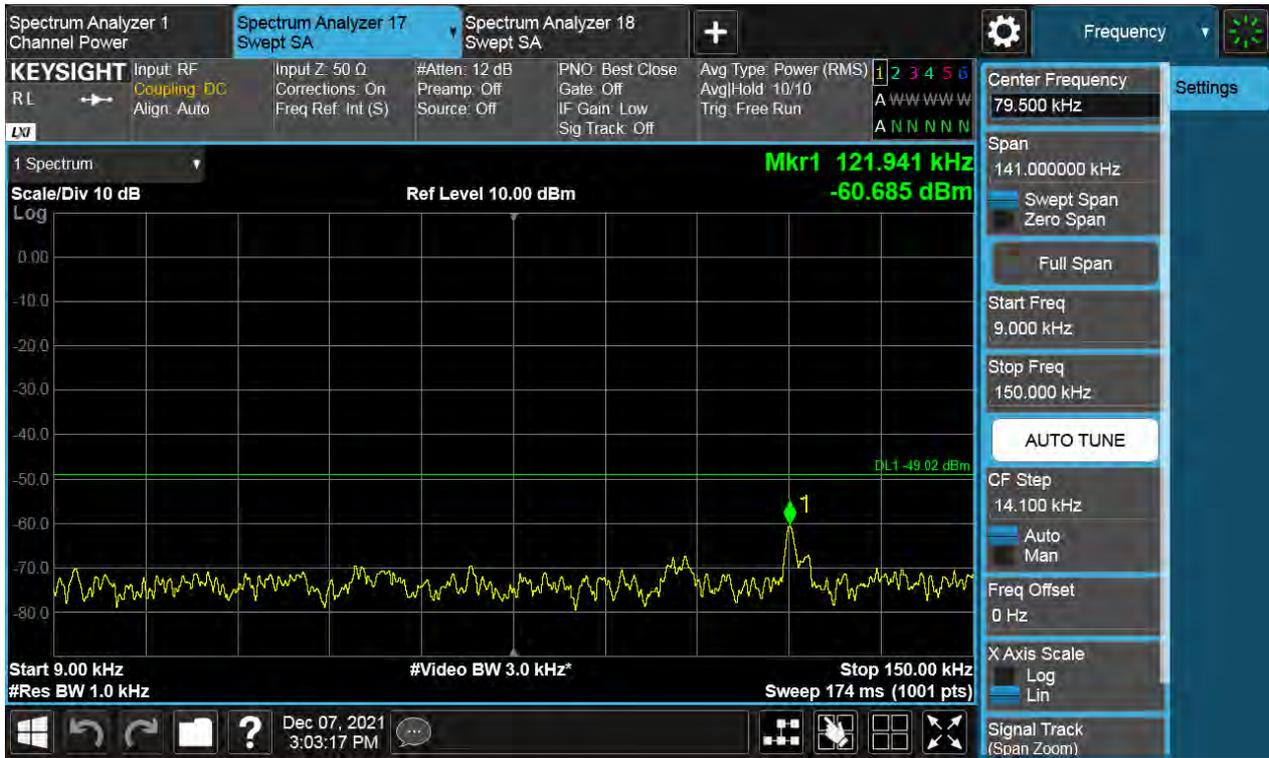
**Antenna 2 / 150 kHz ~ 30 MHz / (4 Port) B66 DSS 10 MHz 9to1 1 Carrier + LTE B66 5 MHz 1 Carrier [2 Carrier] / Non-Contiguous / 64QAM**
