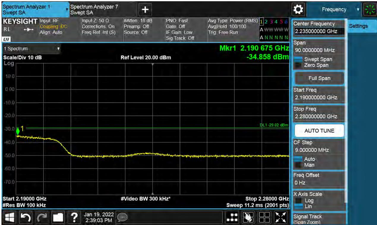
Antenna 2 / High Edge + 100 MHz ~ 10 GHz / (4 Port) LTE B66 5 MHz 1 Carrier + 5G NR n66 10 MHz 1 Carrier [2 Carrier] / Non-Contiguous / 256QAM
