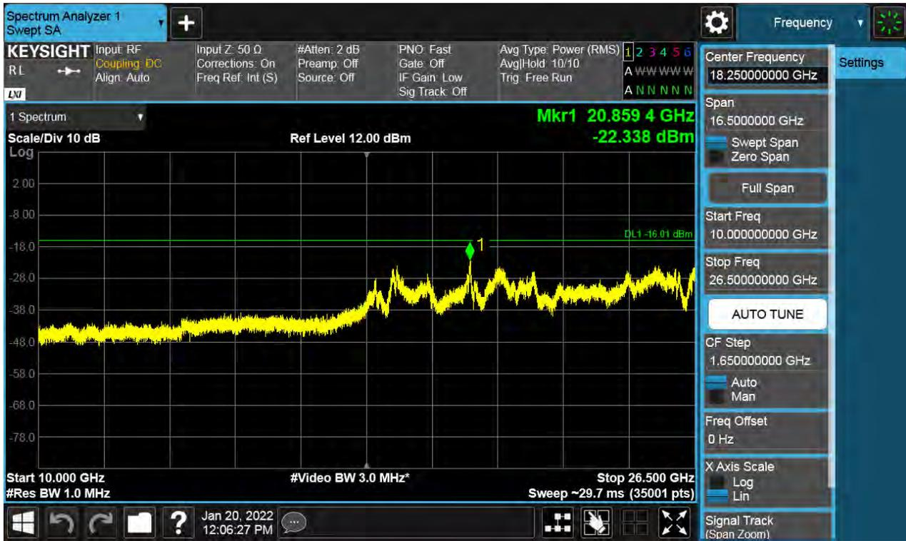
Antenna 0 / 9 kHz ~ 150 kHz / (4 Port) LTE B66 5 MHz 1 Carrier + 5G NR n66 10 MHz 1 Carrier [2 Carrier] / Non-Contiguous / 16QAM
