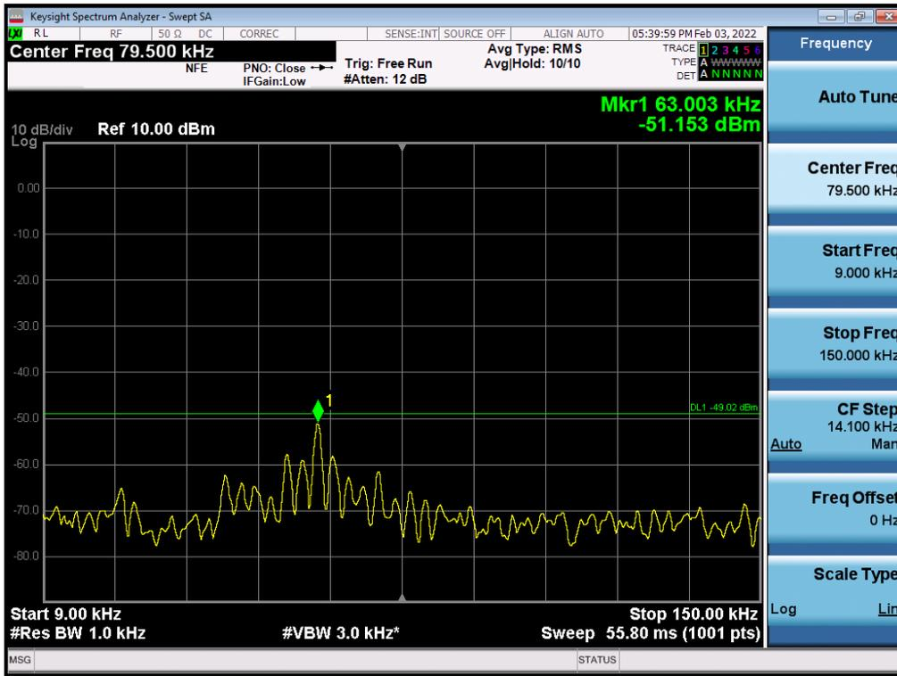
Antenna 2 / 150 kHz ~ 30 MHz / (4 Port) LTE B66 20 MHz 1 Carrier + 5G NR n66 20 MHz 1 Carrier [2 Carrier] / Non-Contiguous / 256QAM
