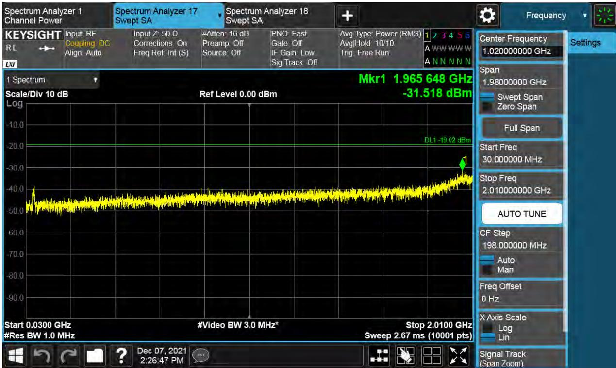
Antenna 0 / Low Edge - 100 MHz ~ Low Edge / (4 Port) B66 DSS 10 MHz 9to1 1 Carrier + LTE B66 5 MHz 1 Carrier [2 Carrier] / Non-Contiguous / 16QAM
