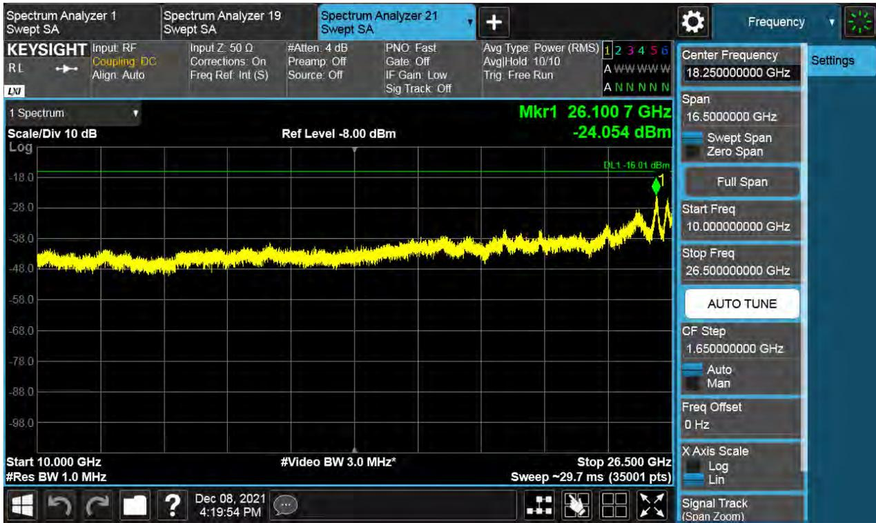
**Antenna 3 / 9 kHz ~ 150 kHz / (4 Port) B66 DSS 10 MHz 9to1 1 Carrier + LTE B66 5 MHz 1 Carrier [2 Carrier] / Non-Contiguous / 256QAM**
