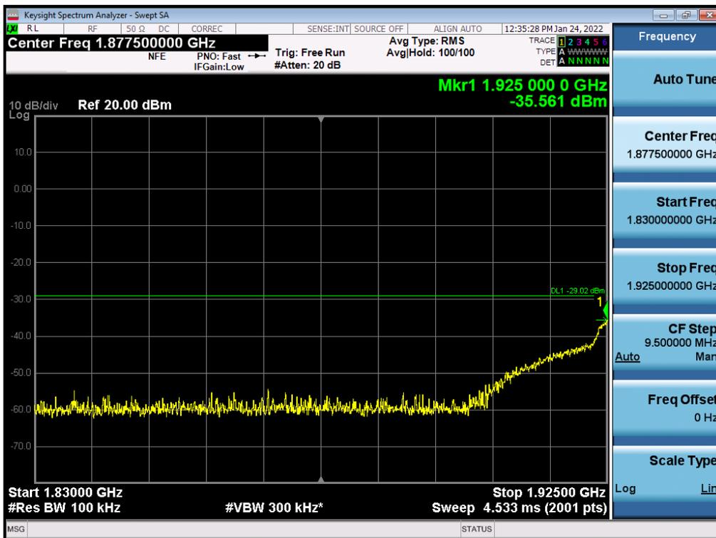
Antenna 1 / High Edge ~ High Edge + 100 MHz / (4 Port) LTE B2 5 MHz 1 Carrier + LTE B2 5 MHz 1 Carrier + 5G NR n2 20 MHz 1 Carrier [3 Carrier] / Contiguous / 16QAM / High
