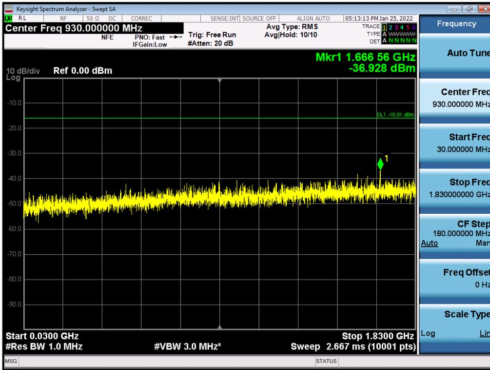
Antenna 1 / Low Edge - 100 MHz ~ Low Edge / (2 Port) LTE B2 5 MHz 1 Carrier + LTE B2 5 MHz 1 Carrier + 5G NR n2 5 MHz 1 Carrier [3 Carrier] / Contiguous / 256QAM / Low
