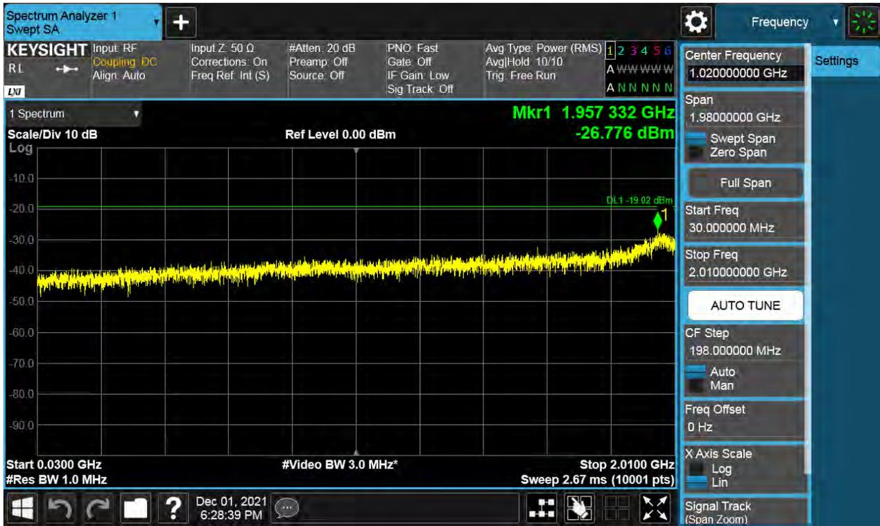
Antenna 0 / Low Edge - 100 MHz ~ Low Edge / (4 Port) B66 DSS 20 MHz 9to1 1 Carrier + LTE B66 10 MHz 1 Carrier + LTE B66 5 MHz 1 Carrier + LTE B66 5 MHz 1 Carrier [4 Carrier] / Contiguous / 16QAM / Middle
