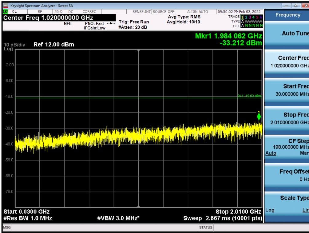
Antenna 2 / Low Edge - 100 MHz ~ Low Edge / (4 Port) LTE B66 5 MHz 1 Carrier + LTE B66 5 MHz 1 Carrier + LTE B66 10 MHz 1 Carrier + 5G NR n66 20 MHz 1 Carrier [4 Carrier] / Contiguous / 16QAM / Middle
