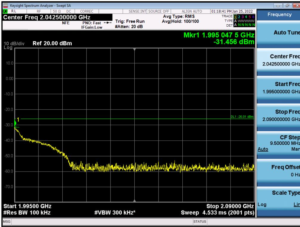
Antenna 0 / High Edge + 100 MHz ~ 10 GHz / (2 Port) LTE B2 5 MHz 1 Carrier + LTE B2 5 MHz 1 Carrier + 5G NR n2 20 MHz 1 Carrier [3 Carrier] / Contiguous / 64QAM / High
