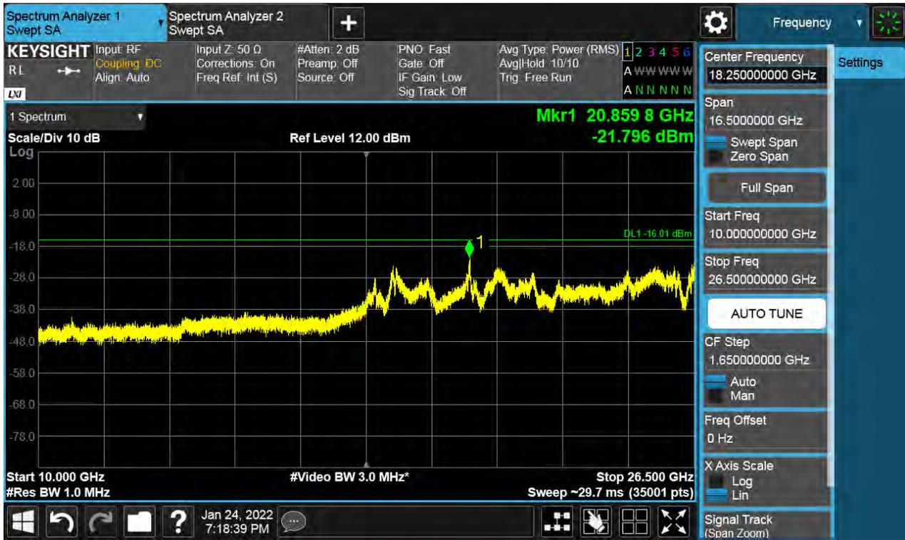
Antenna 1 / 9 kHz ~ 150 kHz / (2 Port) LTE B66 5 MHz 1 Carrier + LTE B66 5 MHz 1 Carrier + LTE B66 10 MHz 1 Carrier + 5G NR n66 20 MHz 1 Carrier [4 Carrier] / Contiguous / 256QAM / Middle
