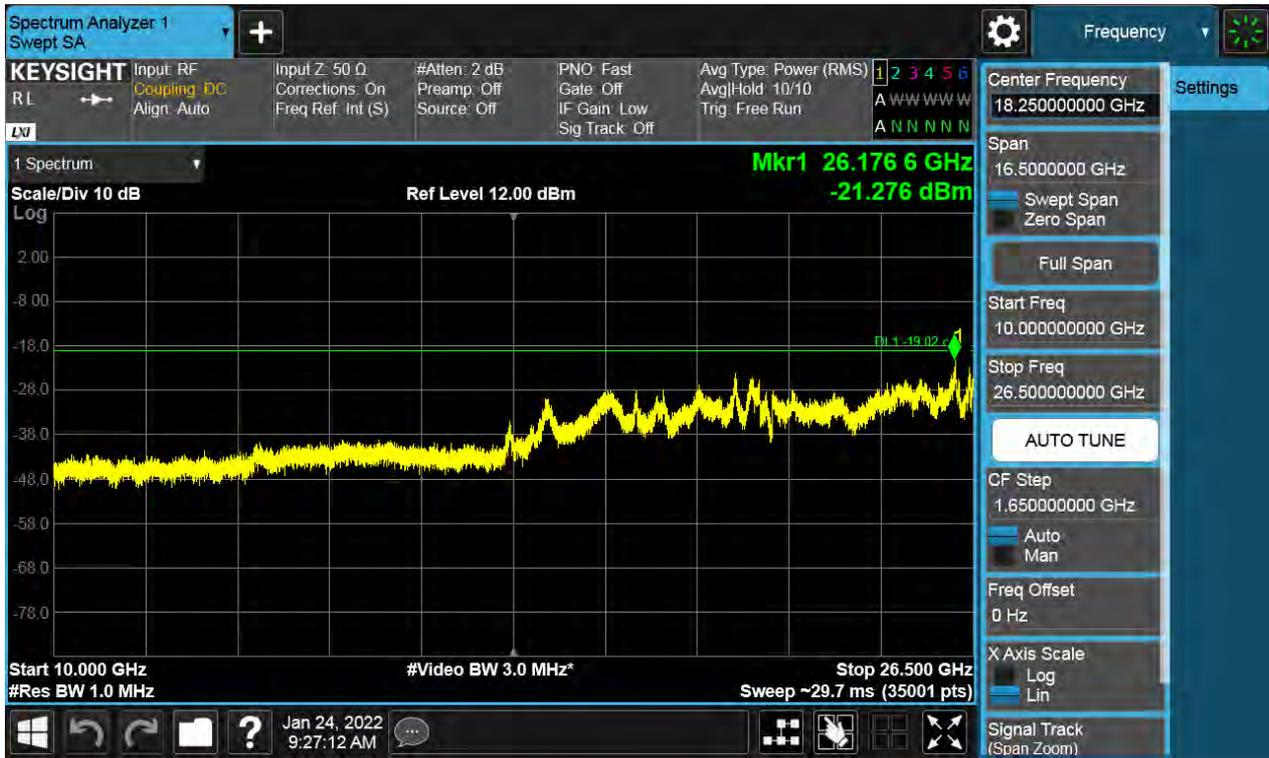
Antenna 2 / 9 kHz ~ 150 kHz / (4 Port) LTE B66 5 MHz 1 Carrier + LTE B66 5 MHz 1 Carrier + LTE B66 10 MHz 1 Carrier + 5G NR n66 20 MHz 1 Carrier [4 Carrier] / Contiguous / 256QAM / Middle
