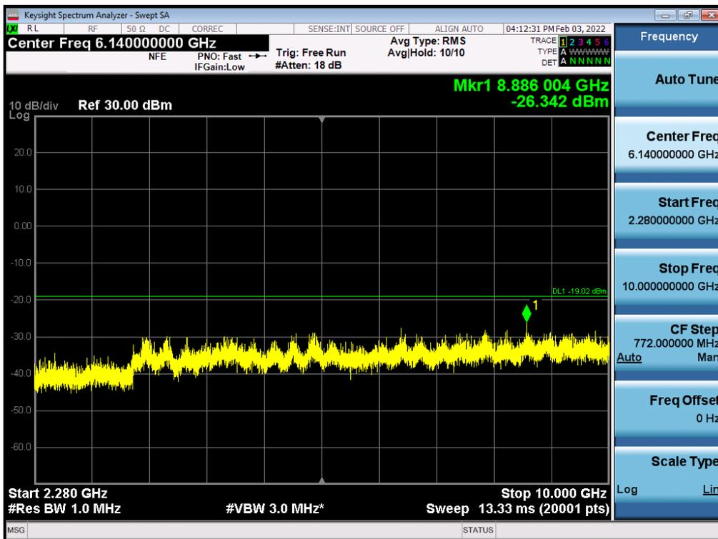
Antenna 2 / 10 GHz ~ 26.5 GHz / (4 Port) LTE B66 20 MHz 1 Carrier + 5G NR n66 20 MHz 1 Carrier [2 Carrier] / Contiguous / 256QAM / Low
