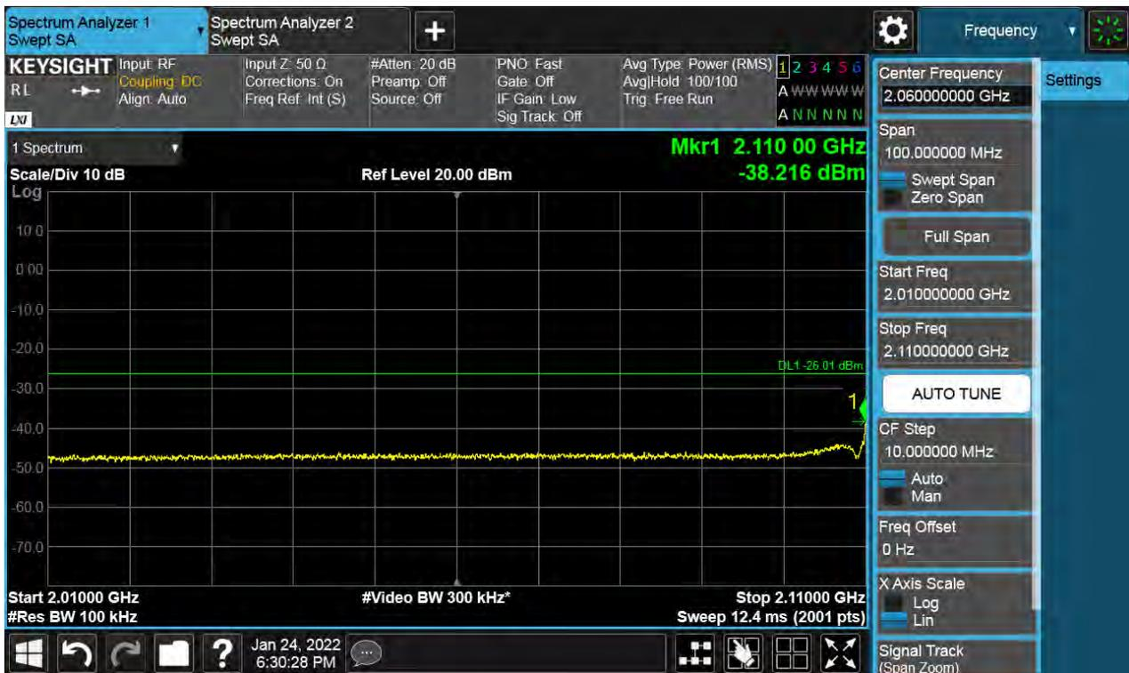
Antenna 1 / High Edge ~ High Edge + 100 MHz / (2 Port) LTE B66 5 MHz 1 Carrier + LTE B66 5 MHz 1 Carrier + LTE B66 5 MHz 1 Carrier + 5G NR n66 5 MHz 1 Carrier [4 Carrier] / Contiguous / 256QAM / High
