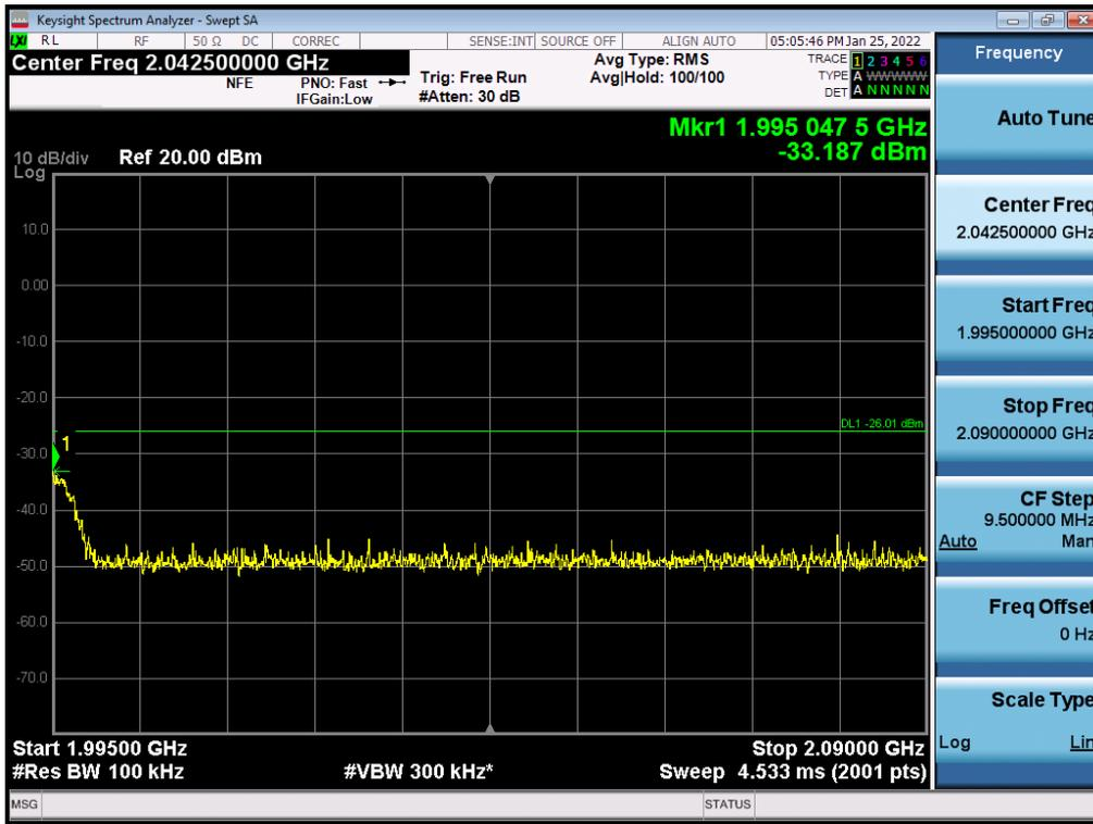
Antenna 0 / High Edge + 100 MHz ~ 10 GHz / (2 Port) LTE B2 5 MHz 1 Carrier + LTE B2 5 MHz 1 Carrier + 5G NR n2 5 MHz 1 Carrier [3 Carrier] / Contiguous / 16QAM / High
