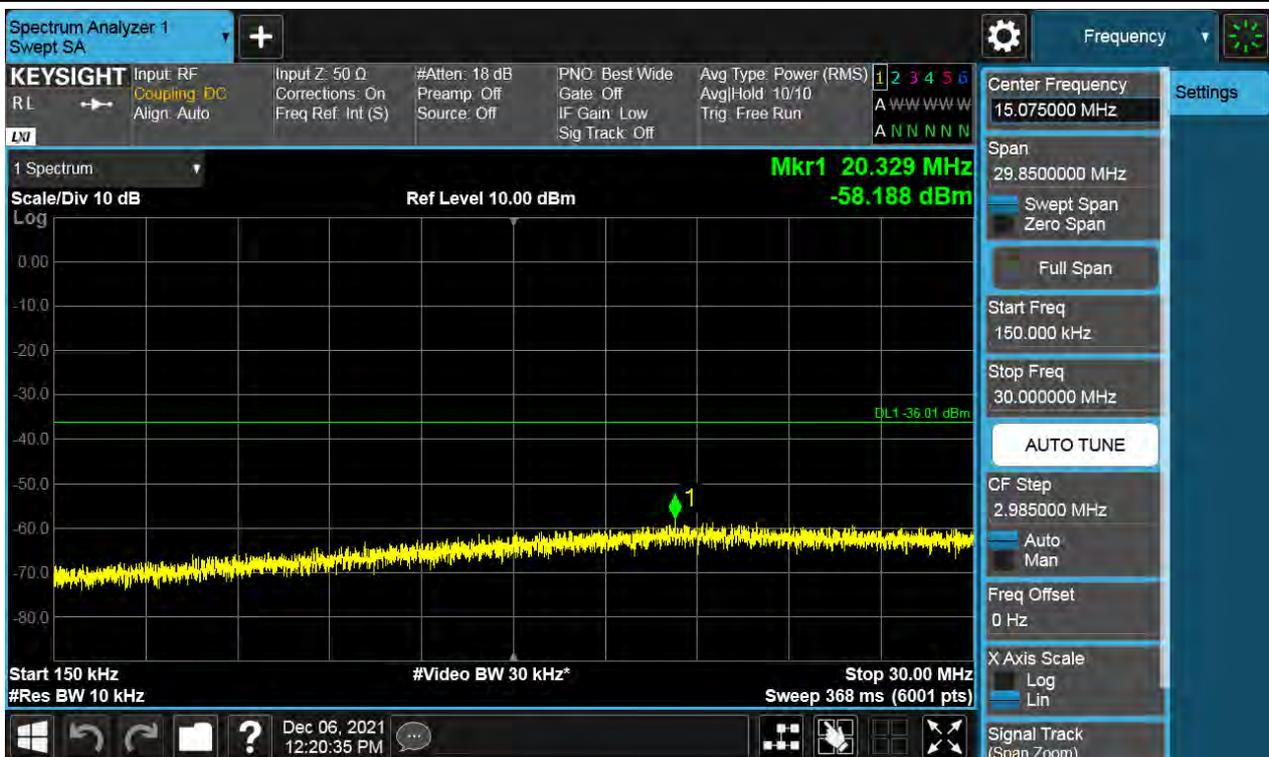
Antenna 0 / 30 MHz ~ Low Edge - 100 MHz / (2 Port) B66 DSS 20 MHz 9to1 1 Carrier + LTE B66 10 MHz 1 Carrier + LTE B66 5 MHz 1 Carrier + LTE B66 5 MHz 1 Carrier [4 Carrier] / Contiguous / 64QAM / Low
