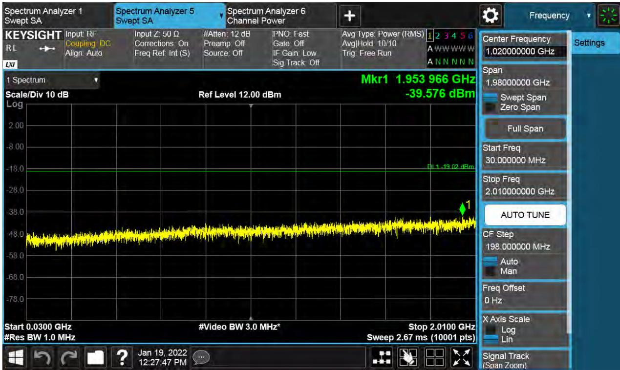
Antenna 0 / Low Edge - 100 MHz ~ Low Edge / (4 Port) LTE B66 5 MHz 1 Carrier + 5G NR n66 10 MHz 1 Carrier [2 Carrier] / Contiguous / QPSK / Middle
