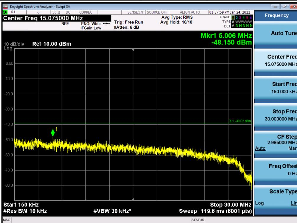
Antenna 1 / 30 MHz ~ Low Edge - 100 MHz / (4 Port) LTE B2 5 MHz 1 Carrier + LTE B2 5 MHz 1 Carrier + 5G NR n2 20 MHz 1 Carrier [3 Carrier] / Contiguous / 16QAM / Low
