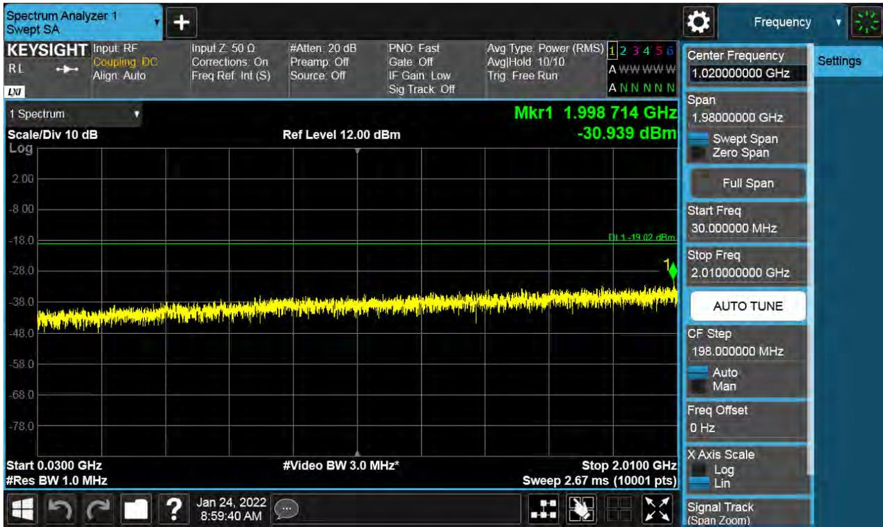
Antenna 0 / Low Edge - 100 MHz ~ Low Edge / (4 Port) LTE B66 5 MHz 1 Carrier + LTE B66 5 MHz 1 Carrier + LTE B66 5 MHz 1 Carrier + 5G NR n66 5 MHz 1 Carrier [4 Carrier] / Contiguous / 256QAM / Middle
