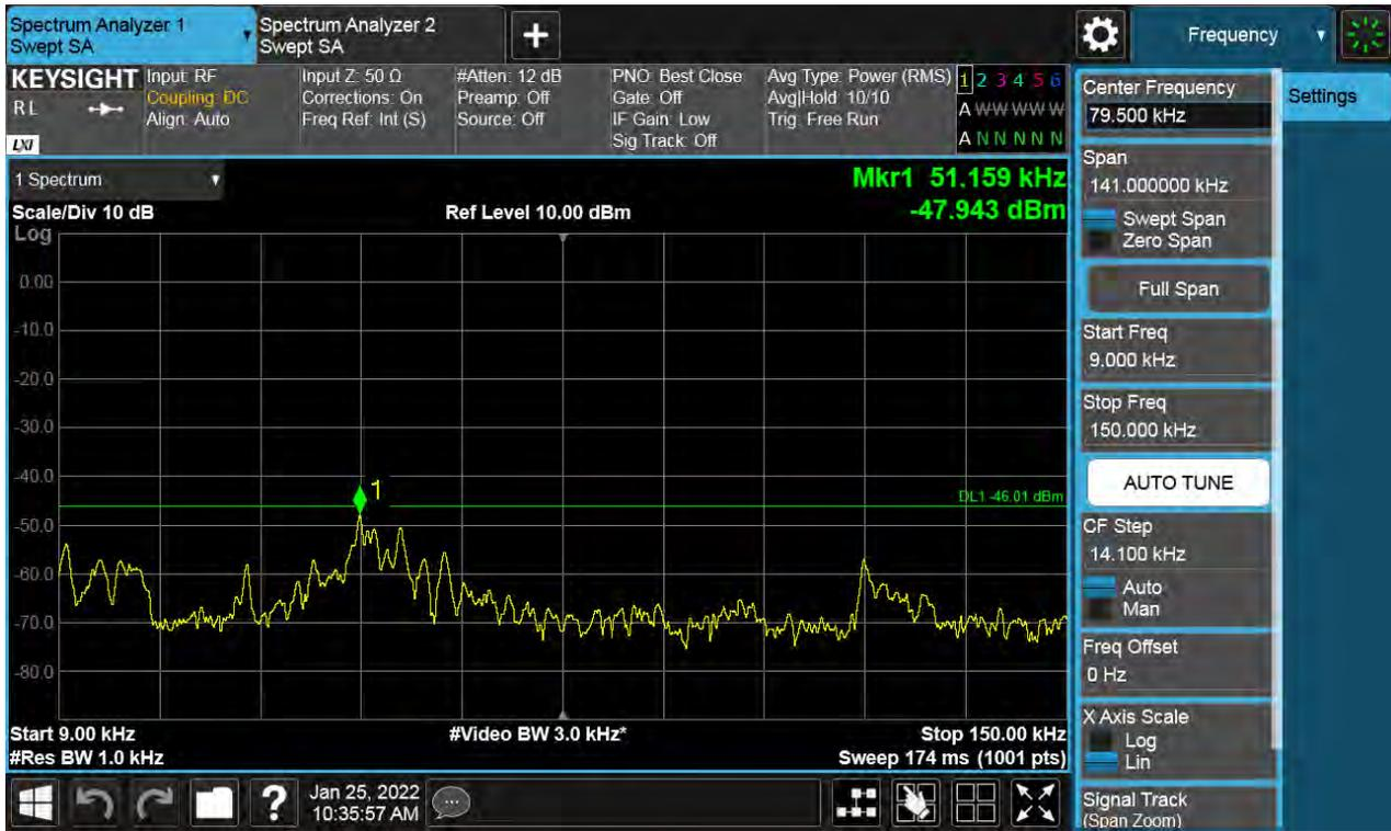
Antenna 1 / 150 kHz ~ 30 MHz / (2 Port) LTE B66 5 MHz 1 Carrier + LTE B66 5 MHz 1 Carrier + LTE B66 10 MHz 1 Carrier + 5G NR n66 20 MHz 1 Carrier [4 Carrier] / Contiguous / 256QAM / Middle
