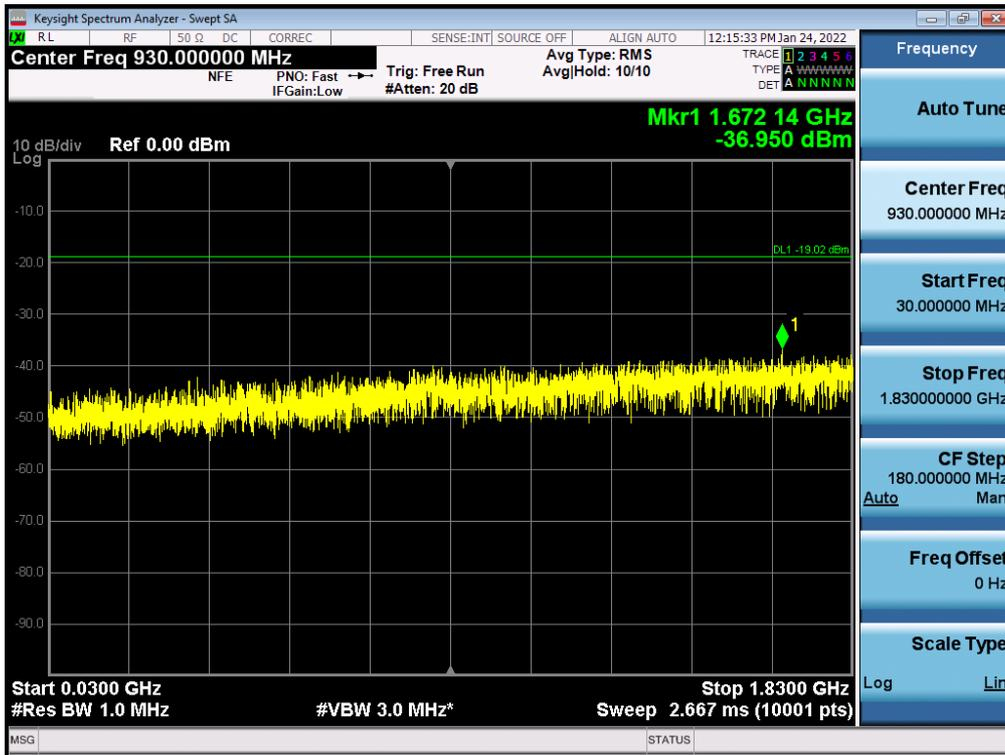
Antenna 2 / Low Edge - 100 MHz ~ Low Edge / (4 Port) LTE B2 5 MHz 1 Carrier + LTE B2 5 MHz 1 Carrier + 5G NR n2 20 MHz 1 Carrier [3 Carrier] / Contiguous / 256QAM / Low
