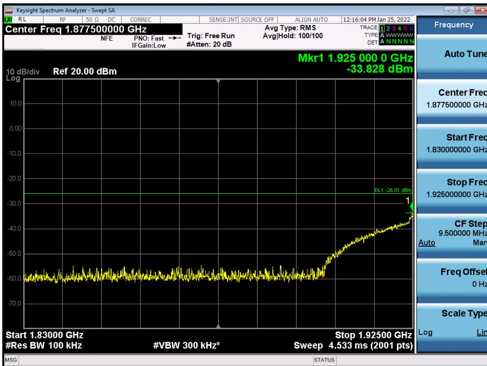
Antenna 1 / High Edge ~ High Edge + 100 MHz / (2 Port) LTE B2 5 MHz 1 Carrier + LTE B2 5 MHz 1 Carrier + 5G NR n2 20 MHz 1 Carrier [3 Carrier] / Contiguous / 64QAM / High
