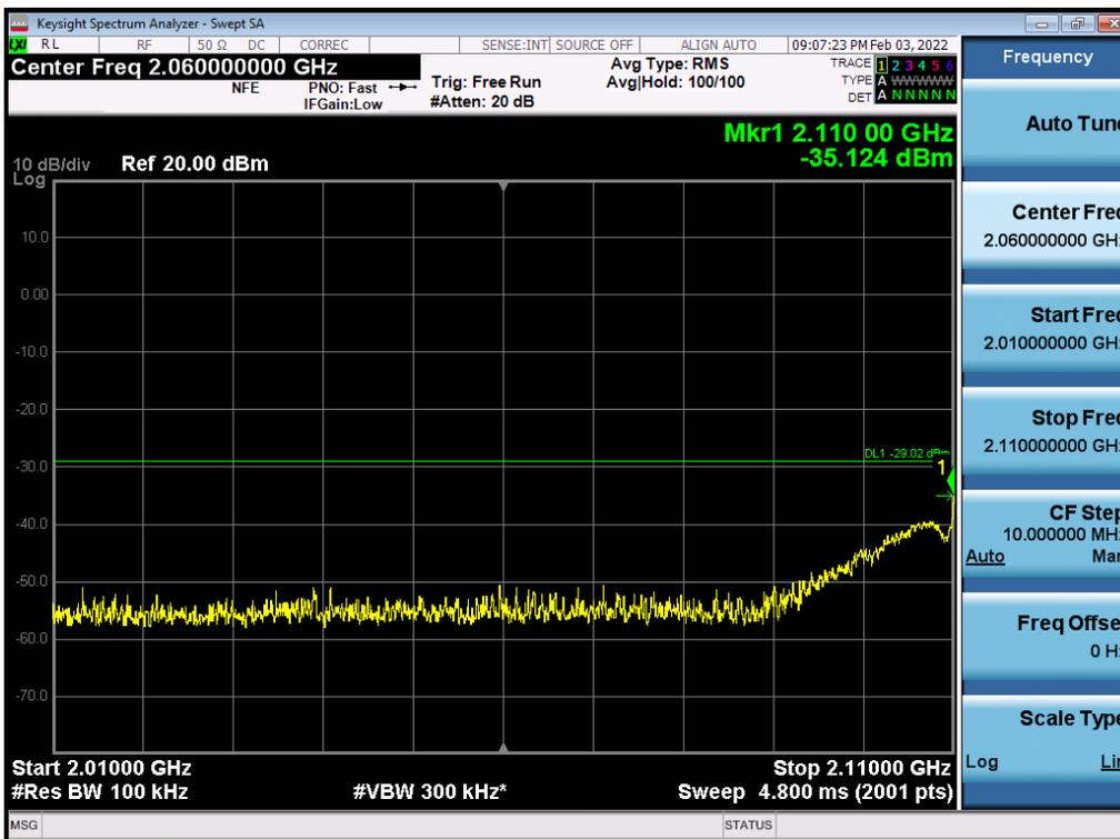
Antenna 2 / High Edge ~ High Edge + 100 MHz / (4 Port) LTE B66 5 MHz 1 Carrier + LTE B66 5 MHz 1 Carrier + LTE B66 10 MHz 1 Carrier + 5G NR n66 20 MHz 1 Carrier [4 Carrier] / Contiguous / 16QAM / High
