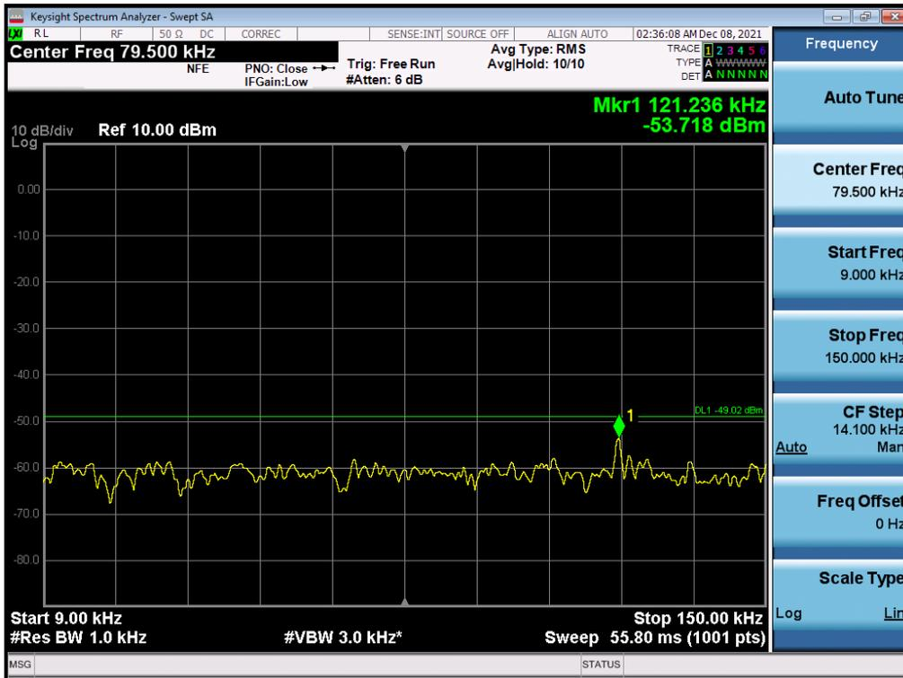
Antenna 3 / 150 kHz ~ 30 MHz / (4 Port) B2 DSS 10 MHz 9to1 1 Carrier + LTE B2 5 MHz 1 Carrier [2 Carrier] / Non-Contiguous / QPSK
