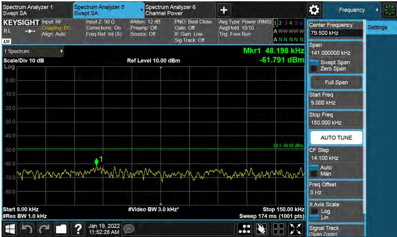
Antenna 3 / 150 kHz ~ 30 MHz / (4 Port) LTE B66 5 MHz 1 Carrier + 5G NR n66 10 MHz 1 Carrier [2 Carrier] / Contiguous / 64QAM / Low
