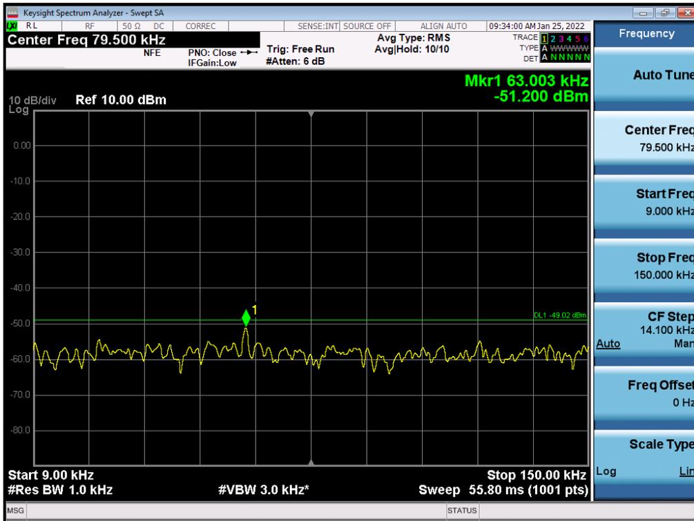
Antenna 3 / 150 kHz ~ 30 MHz / (4 Port) LTE B2 5 MHz 1 Carrier + LTE B2 5 MHz 1 Carrier + 5G NR n2 5 MHz 1 Carrier [3 Carrier] / Contiguous / 16QAM / High
