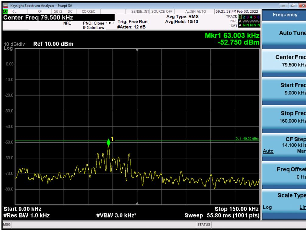
Antenna 3 / 150 kHz ~ 30 MHz / (4 Port) LTE B66 5 MHz 1 Carrier + LTE B66 5 MHz 1 Carrier + LTE B66 10 MHz 1 Carrier + 5G NR n66 20 MHz 1 Carrier [4 Carrier] / Contiguous / QPSK / Low
