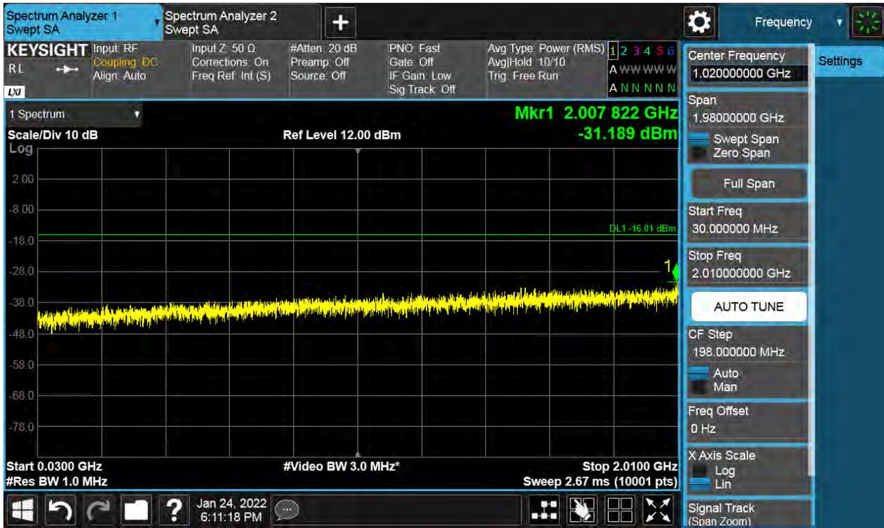
Antenna 0 / Low Edge - 100 MHz ~ Low Edge / (2 Port) LTE B66 5 MHz 1 Carrier + LTE B66 5 MHz 1 Carrier + LTE B66 5 MHz 1 Carrier + 5G NR n66 5 MHz 1 Carrier [4 Carrier] / Contiguous / 64QAM / Middle
