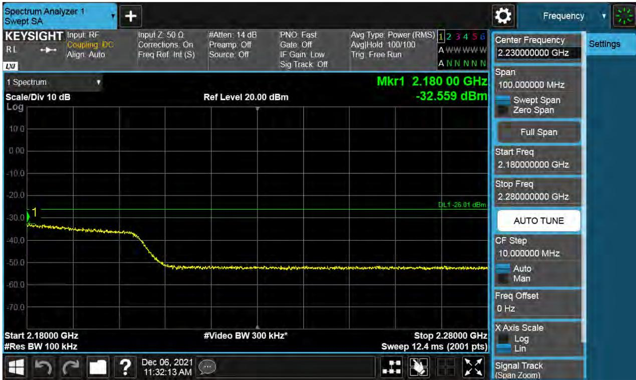
Antenna 0 / High Edge + 100 MHz ~ 10 GHz / (2 Port) B66 DSS 20 MHz 9to1 1 Carrier + LTE B66 10 MHz 1 Carrier + LTE B66 5 MHz 1 Carrier + LTE B66 5 MHz 1 Carrier [4 Carrier] / Contiguous / 16QAM / Middle
