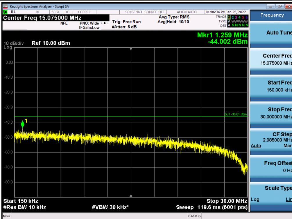
Antenna 0 / 30 MHz ~ Low Edge - 100 MHz / (2 Port) LTE B2 5 MHz 1 Carrier + LTE B2 5 MHz 1 Carrier + 5G NR n2 20 MHz 1 Carrier [3 Carrier] / Contiguous / QPSK / High
