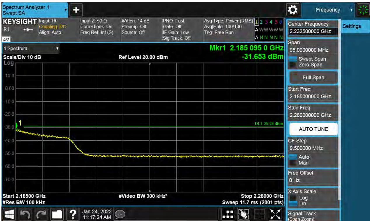
**Antenna 2 / High Edge + 100 MHz ~ 10 GHz / (4 Port) LTE B66 5 MHz 1 Carrier + LTE B66 5 MHz 1 Carrier + LTE B66 5 MHz 1 Carrier + 5G NR n66 5 MHz 1 Carrier [4 Carrier] / Contiguous / 64QAM / High**
