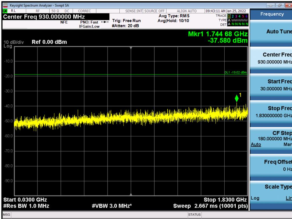
Antenna 2 / Low Edge - 100 MHz ~ Low Edge / (4 Port) LTE B2 5 MHz 1 Carrier + LTE B2 5 MHz 1 Carrier + 5G NR n2 5 MHz 1 Carrier [3 Carrier] / Contiguous / 256QAM / Low
