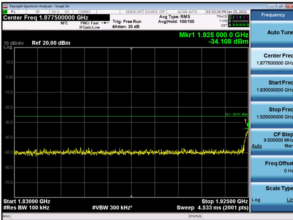
Antenna 1 / High Edge ~ High Edge + 100 MHz / (2 Port) LTE B2 5 MHz 1 Carrier + LTE B2 5 MHz 1 Carrier + 5G NR n2 5 MHz 1 Carrier [3 Carrier] / Contiguous / 16QAM / High
