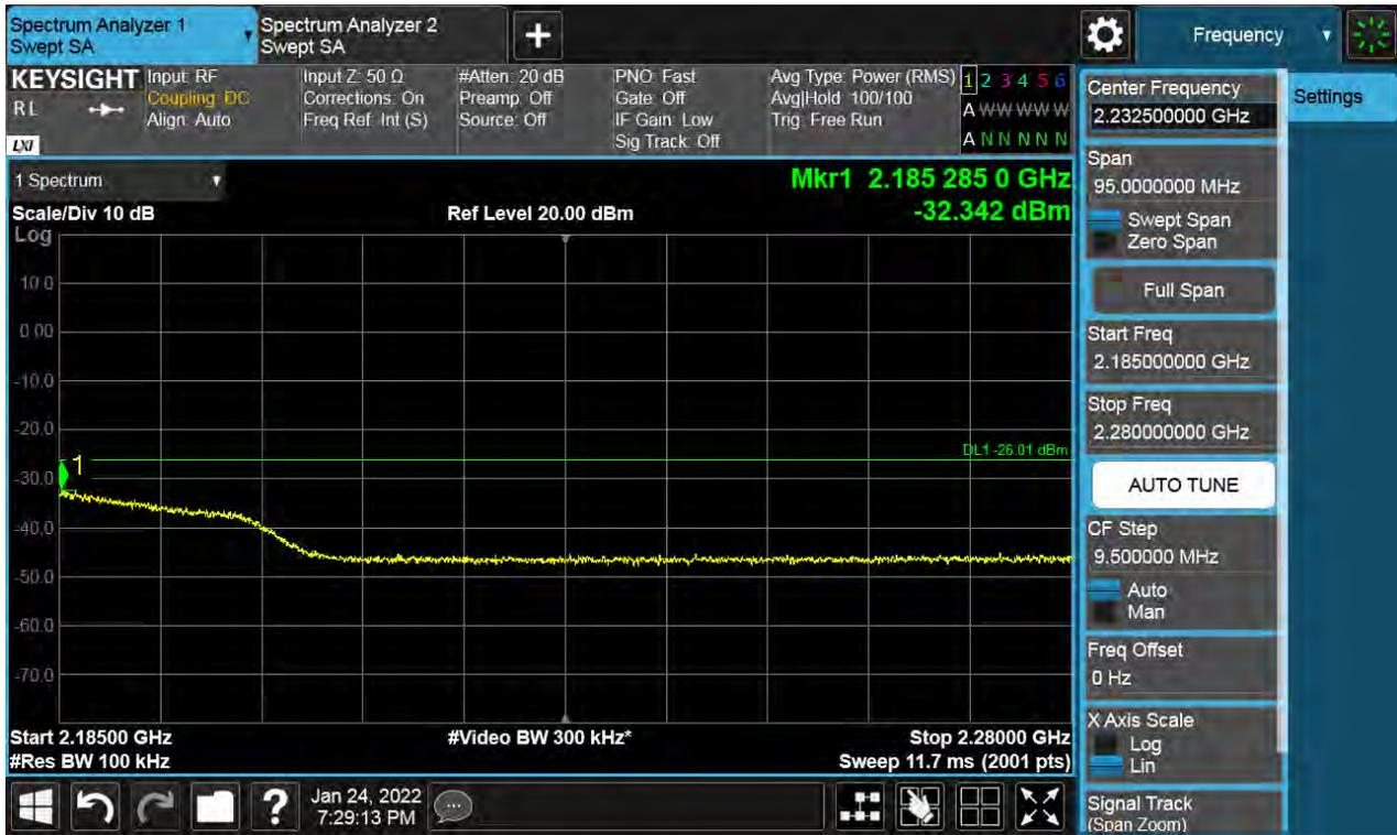
Antenna 1 / High Edge + 100 MHz ~ 10 GHz / (2 Port) LTE B66 5 MHz 1 Carrier + LTE B66 5 MHz 1 Carrier + LTE B66 5 MHz 1 Carrier + 5G NR n66 5 MHz 1 Carrier [4 Carrier] / Contiguous / 16QAM / High
