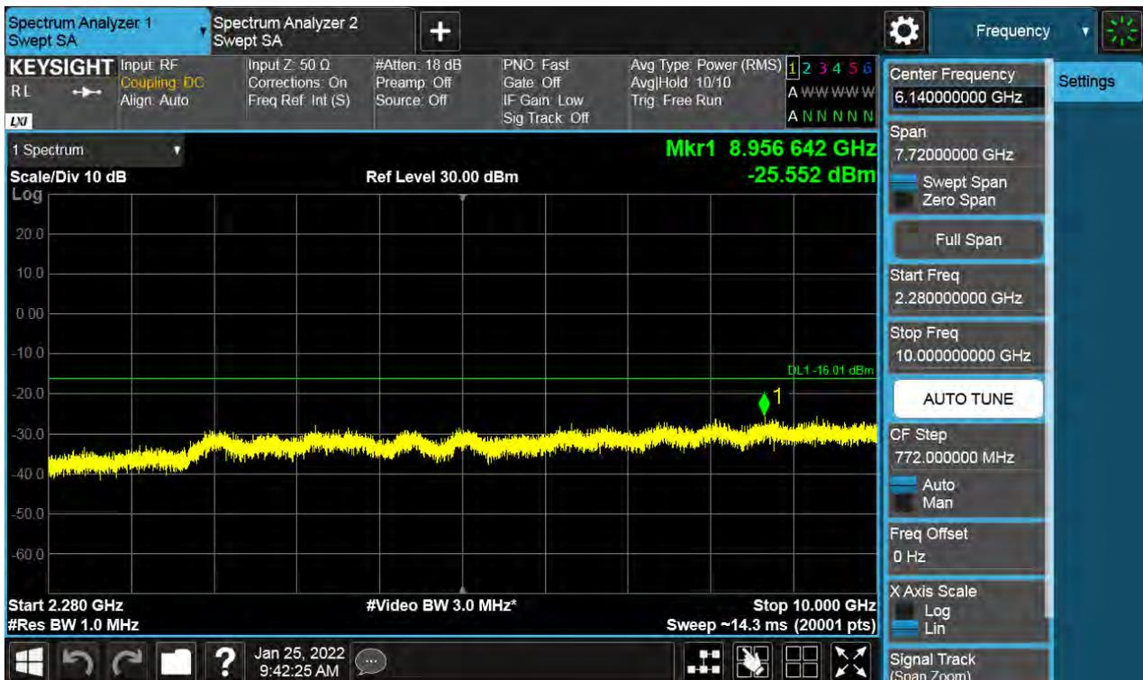
Antenna 1 / 10 GHz ~ 26.5 GHz / (2 Port) LTE B66 5 MHz 1 Carrier + LTE B66 5 MHz 1 Carrier + LTE B66 10 MHz 1 Carrier + 5G NR n66 20 MHz 1 Carrier [4 Carrier] / Contiguous / 256QAM / Middle
