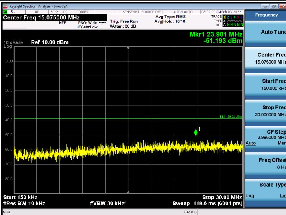
Antenna 3 / 30 MHz ~ Low Edge - 100 MHz / (4 Port) LTE B66 5 MHz 1 Carrier + LTE B66 5 MHz 1 Carrier + LTE B66 10 MHz 1 Carrier + 5G NR n66 20 MHz 1 Carrier [4 Carrier] / Contiguous / QPSK / High
