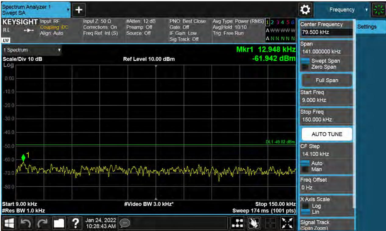
Antenna 3 / 150 kHz ~ 30 MHz / (4 Port) LTE B66 5 MHz 1 Carrier + LTE B66 5 MHz 1 Carrier + LTE B66 5 MHz 1 Carrier + 5G NR n66 5 MHz 1 Carrier [4 Carrier] / Contiguous / QPSK / Middle
