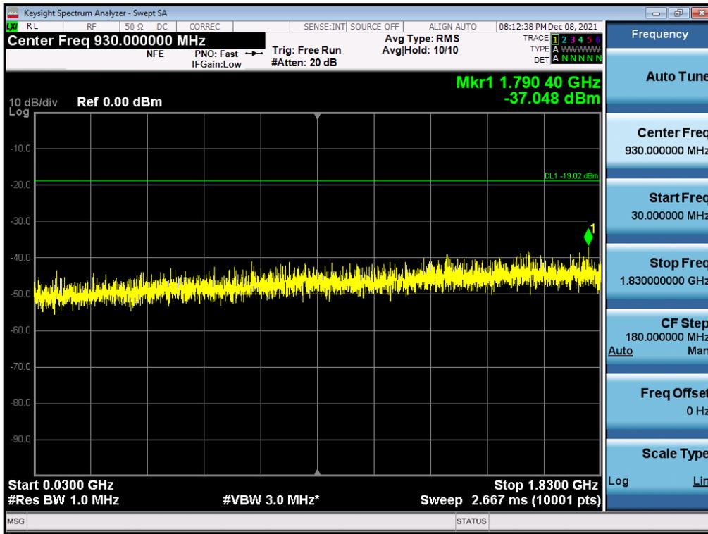
Antenna 0 / Low Edge - 100 MHz ~ Low Edge / (4 Port) B2 DSS 20 MHz 9to1 1 Carrier + LTE B2 5 MHz 1 Carrier + LTE B2 5 MHz 1 Carrier [3 Carrier] / Contiguous / QPSK / Middle
