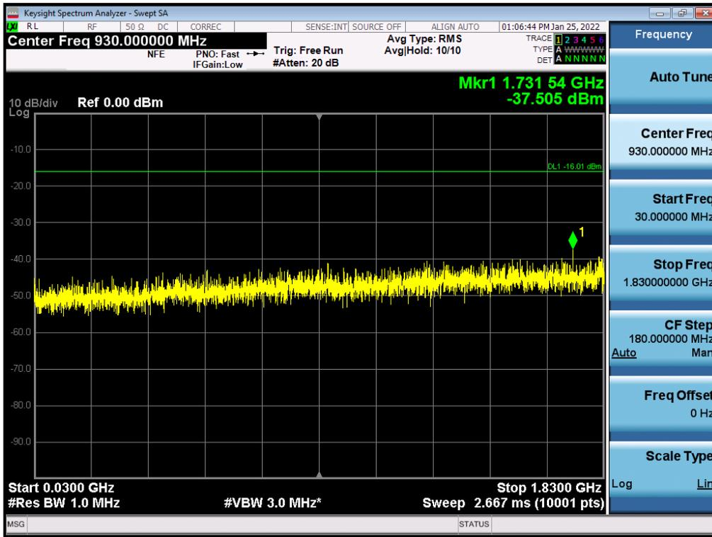
Antenna 1 / Low Edge - 100 MHz ~ Low Edge / (2 Port) LTE B2 5 MHz 1 Carrier + LTE B2 5 MHz 1 Carrier + 5G NR n2 20 MHz 1 Carrier [3 Carrier] / Contiguous / QPSK / Low
