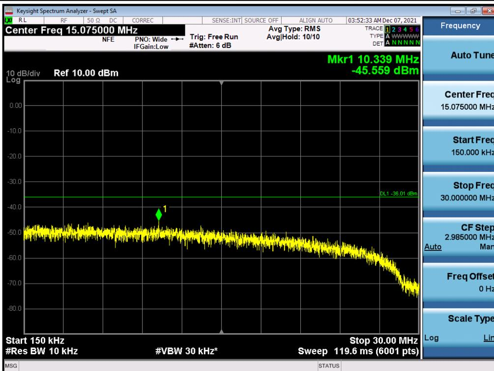
Antenna 1 / 30 MHz ~ Low Edge - 100 MHz / (2 Port) B2 DSS 20 MHz 9to1 1 Carrier + LTE B2 5 MHz 1 Carrier + LTE B2 5 MHz 1 Carrier [3 Carrier] / Contiguous / 64QAM / Middle
