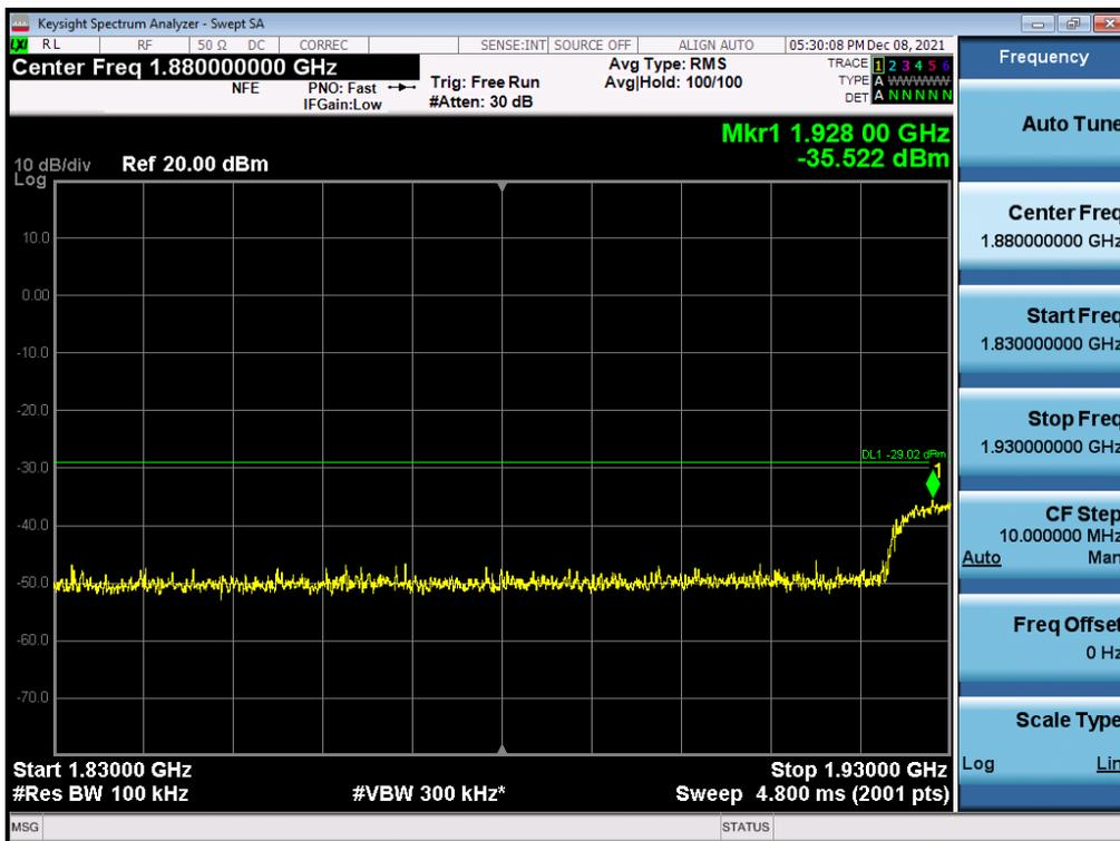
Antenna 0 / High Edge ~ High Edge + 100 MHz / (4 Port) B2 DSS 20 MHz 9to1 1 Carrier + LTE B2 5 MHz 1 Carrier + LTE B2 5 MHz 1 Carrier [3 Carrier] / Contiguous / QPSK / High
