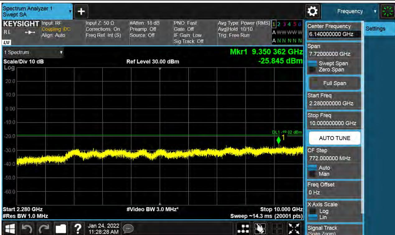
Antenna 2 / 10 GHz ~ 26.5 GHz / (4 Port) LTE B66 5 MHz 1 Carrier + LTE B66 5 MHz 1 Carrier + LTE B66 5 MHz 1 Carrier + 5G NR n66 5 MHz 1 Carrier [4 Carrier] / Contiguous / 256QAM / Low
