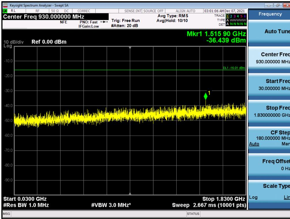
Antenna 0 / Low Edge - 100 MHz ~ Low Edge / (2 Port) B2 DSS 20 MHz 9to1 1 Carrier + LTE B2 5 MHz 1 Carrier + LTE B2 5 MHz 1 Carrier [3 Carrier] / Contiguous / QPSK / Middle
