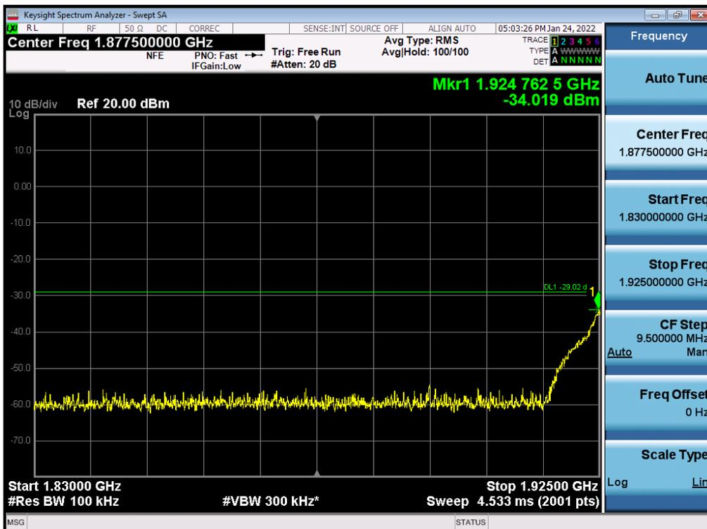
Antenna 1 / High Edge ~ High Edge + 100 MHz / (4 Port) LTE B2 5 MHz 1 Carrier + LTE B2 5 MHz 1 Carrier + 5G NR n2 5 MHz 1 Carrier [3 Carrier] / Contiguous / 64QAM / High
