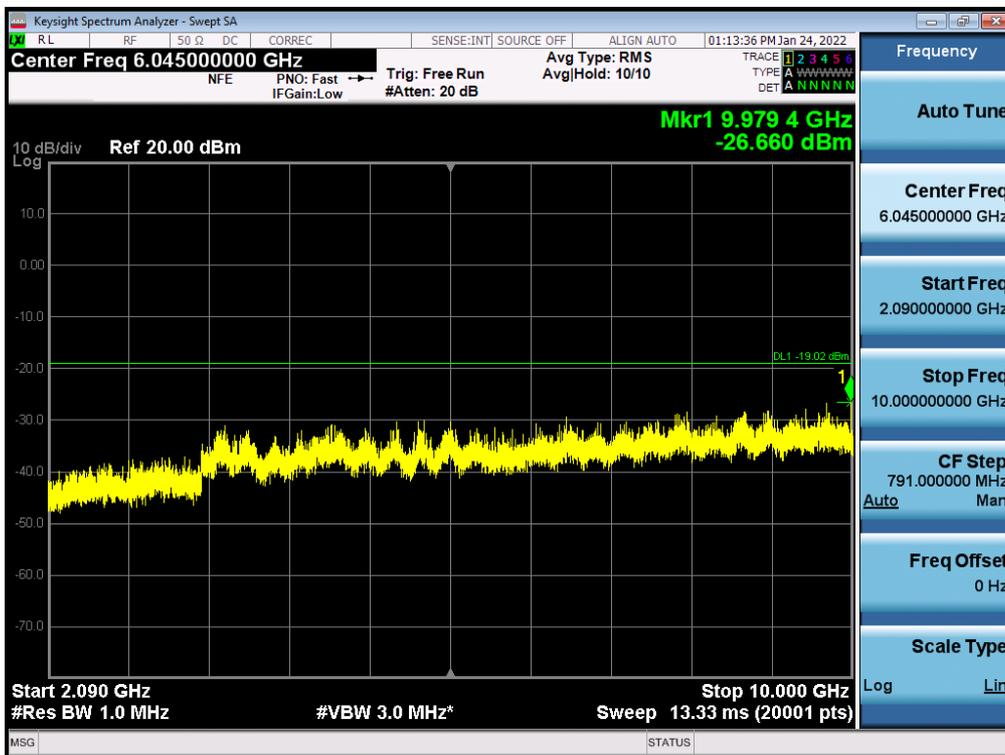
Antenna 2 / 10 GHz ~ 26.5 GHz / (4 Port) LTE B2 5 MHz 1 Carrier + LTE B2 5 MHz 1 Carrier + 5G NR n2 20 MHz 1 Carrier [3 Carrier] / Contiguous / 64QAM / Middle
