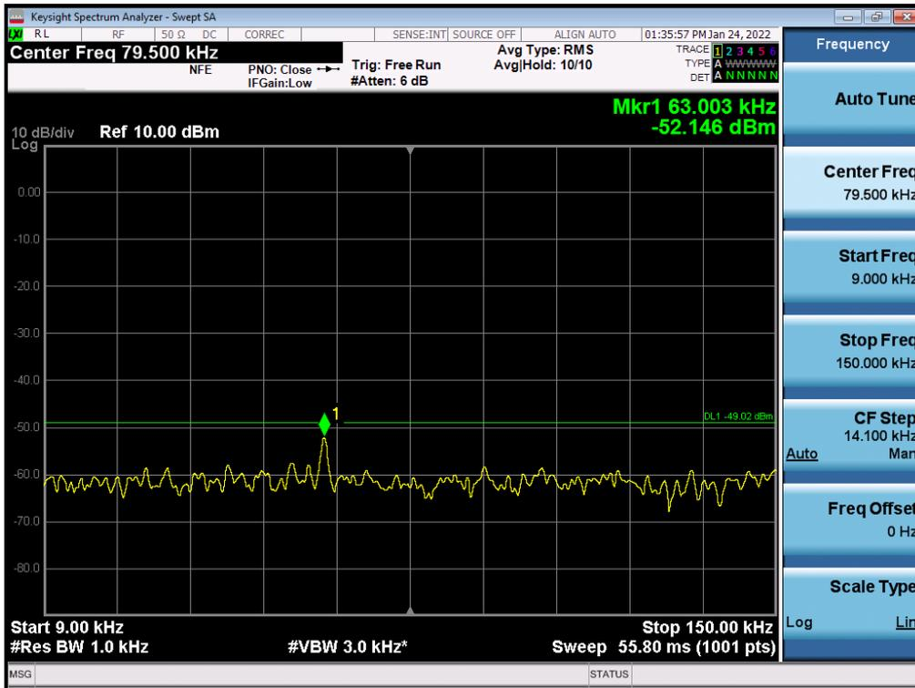
Antenna 2 / 150 kHz ~ 30 MHz / (4 Port) LTE B2 5 MHz 1 Carrier + LTE B2 5 MHz 1 Carrier + 5G NR n2 20 MHz 1 Carrier [3 Carrier] / Contiguous / 16QAM / High
