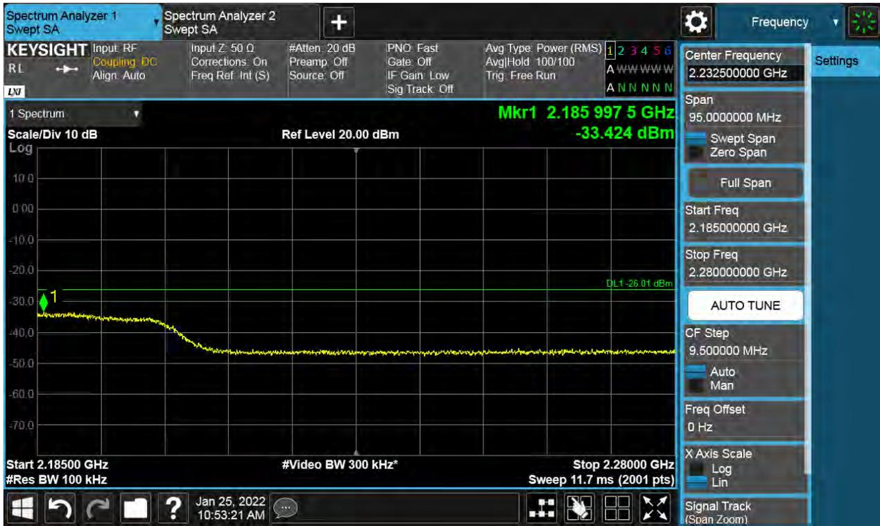
**Antenna 1 / High Edge + 100 MHz ~ 10 GHz / (2 Port) LTE B66 5 MHz 1 Carrier + LTE B66 5 MHz 1 Carrier + LTE B66 10 MHz 1 Carrier + 5G NR n66 20 MHz 1 Carrier [4 Carrier] / Contiguous / 64QAM / Low**
