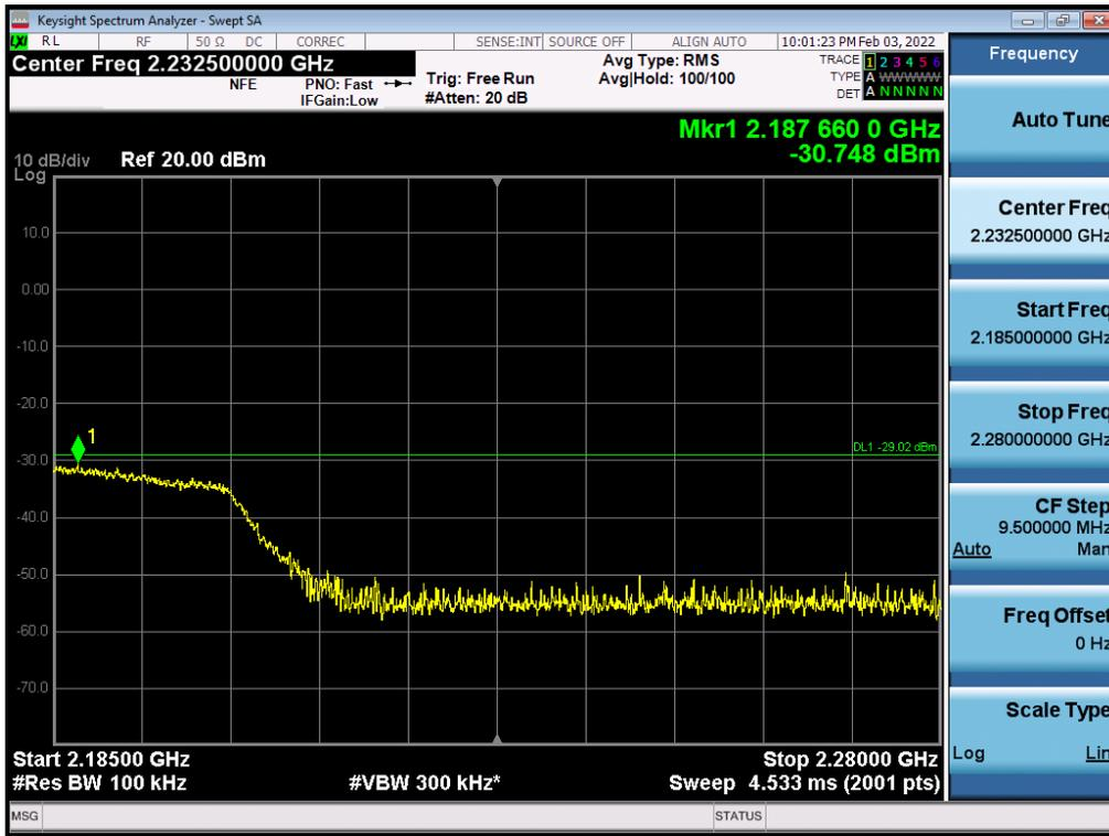
Antenna 3 / High Edge + 100 MHz ~ 10 GHz / (4 Port) LTE B66 5 MHz 1 Carrier + LTE B66 5 MHz 1 Carrier + LTE B66 10 MHz 1 Carrier + 5G NR n66 20 MHz 1 Carrier [4 Carrier] / Contiguous / 16QAM / Low
