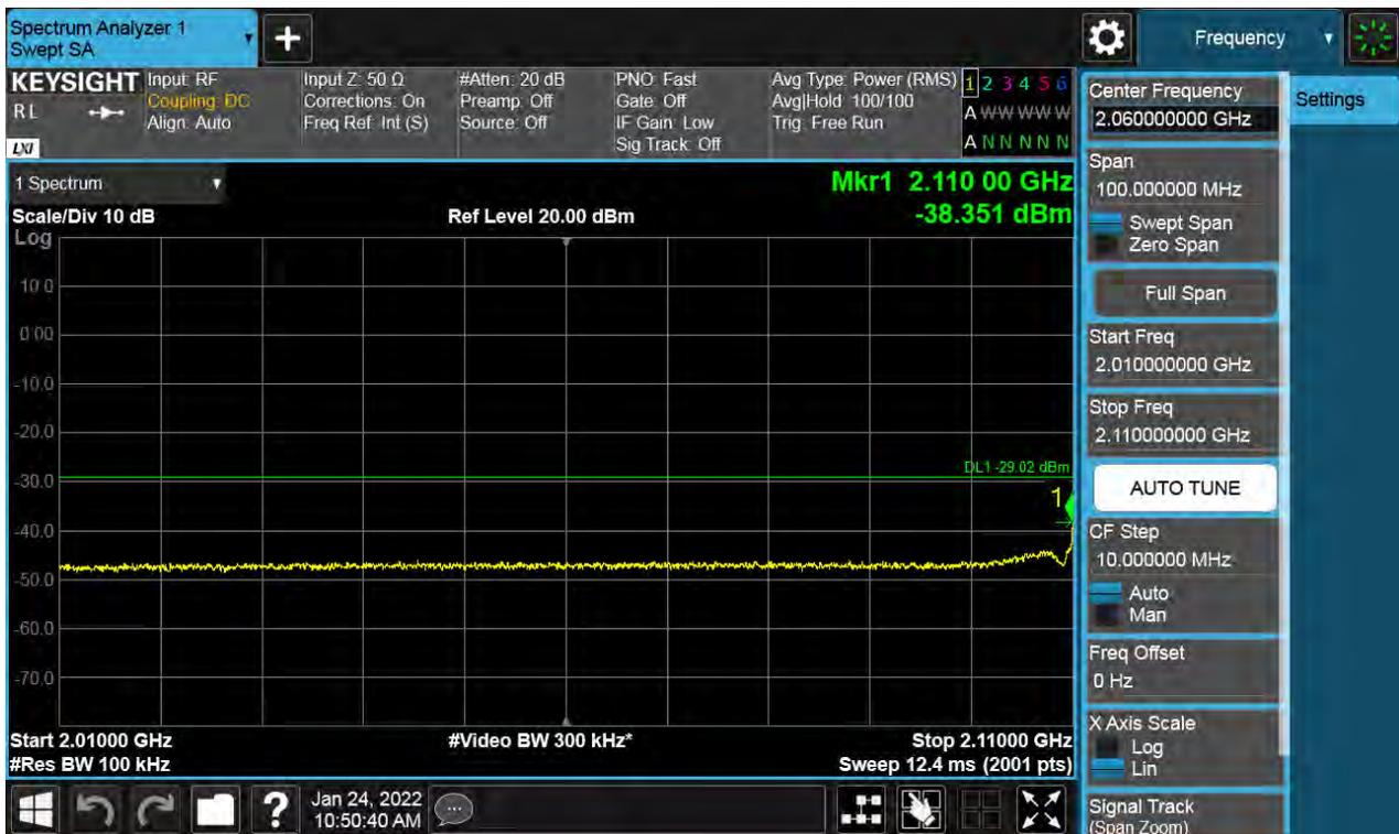
**Antenna 2 / High Edge ~ High Edge + 100 MHz / (4 Port) LTE B66 5 MHz 1 Carrier + LTE B66 5 MHz 1 Carrier + LTE B66 5 MHz 1 Carrier + 5G NR n66 5 MHz 1 Carrier [4 Carrier] / Contiguous / 16QAM / High**
