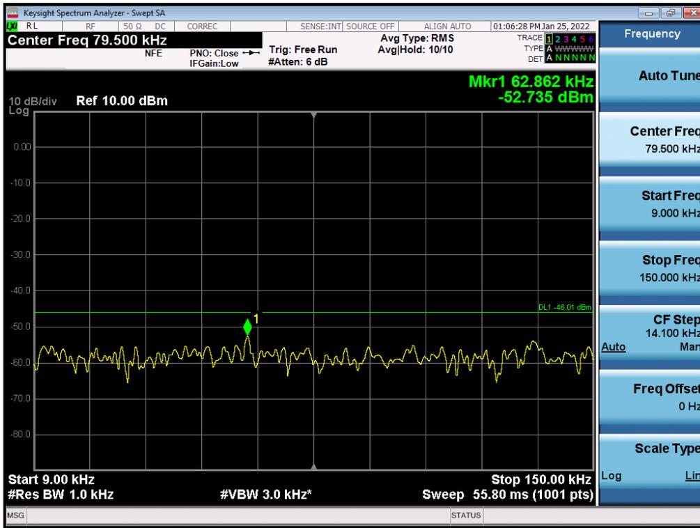
Antenna 0 / 150 kHz ~ 30 MHz / (2 Port) LTE B2 5 MHz 1 Carrier + LTE B2 5 MHz 1 Carrier + 5G NR n2 20 MHz 1 Carrier [3 Carrier] / Contiguous / QPSK / High
