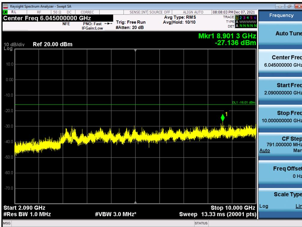
Antenna 0 / 10 GHz ~ 26.5 GHz / (2 Port) B2 DSS 10 MHz 9to1 1 Carrier + LTE B2 5 MHz 1 Carrier [2 Carrier] / Non-Contiguous / 64QAM
