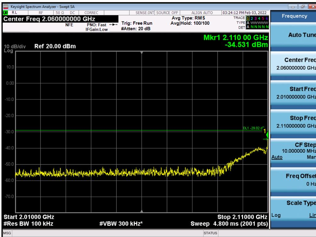
Antenna 2 / High Edge ~ High Edge + 100 MHz / (4 Port) LTE B66 20 MHz 1 Carrier + 5G NR n66 20 MHz 1 Carrier [2 Carrier] / Contiguous / 256QAM / Middle
