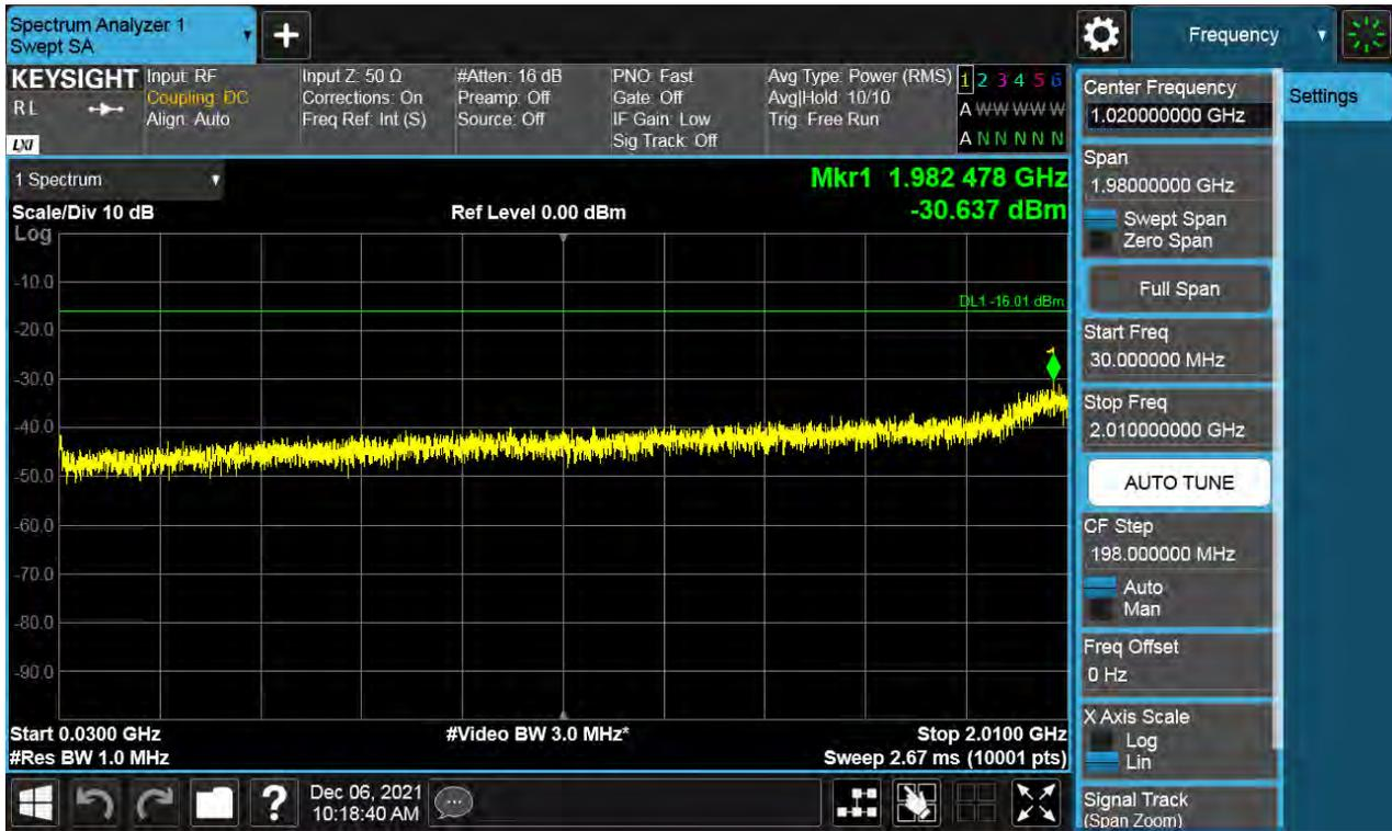
Antenna 0 / Low Edge - 100 MHz ~ Low Edge / (2 Port) B66 DSS 20 MHz 9to1 1 Carrier + LTE B66 10 MHz 1 Carrier + LTE B66 5 MHz 1 Carrier + LTE B66 5 MHz 1 Carrier [4 Carrier] / Contiguous / QPSK / Middle
