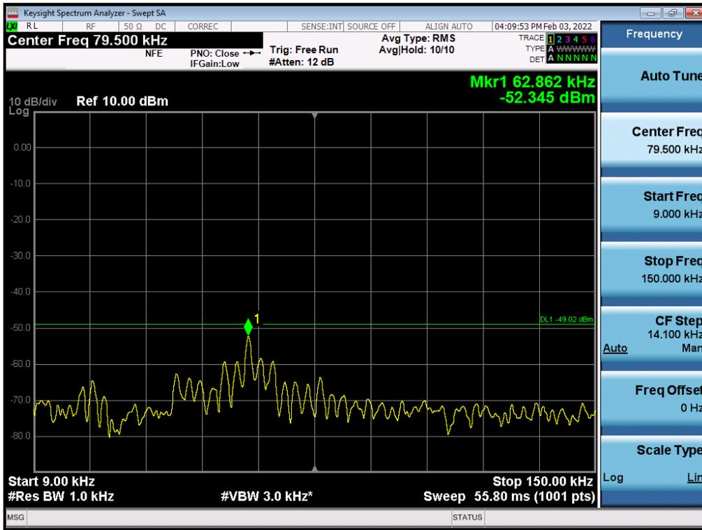
Antenna 1 / 150 kHz ~ 30 MHz / (4 Port) LTE B66 20 MHz 1 Carrier + 5G NR n66 20 MHz 1 Carrier [2 Carrier] / Contiguous / 64QAM / Middle
