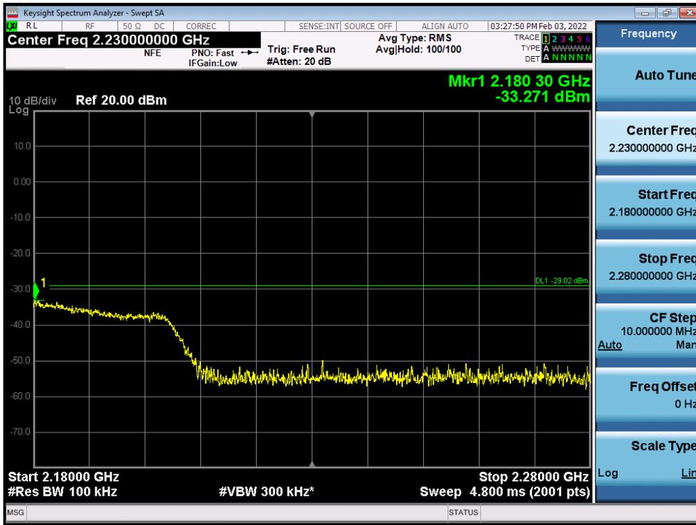
Antenna 3 / High Edge + 100 MHz ~ 10 GHz / (4 Port) LTE B66 20 MHz 1 Carrier + 5G NR n66 20 MHz 1 Carrier [2 Carrier] / Contiguous / QPSK / High
