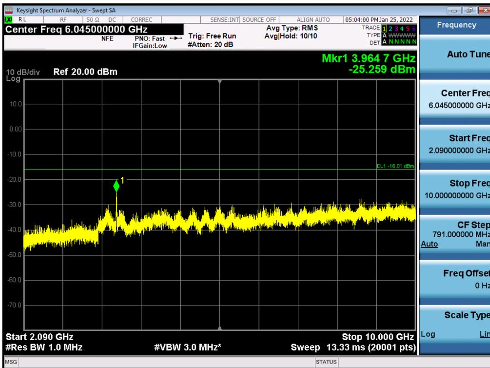
Antenna 1 / 10 GHz ~ 26.5 GHz / (2 Port) LTE B2 5 MHz 1 Carrier + LTE B2 5 MHz 1 Carrier + 5G NR n2 5 MHz 1 Carrier [3 Carrier] / Contiguous / 64QAM / Low
