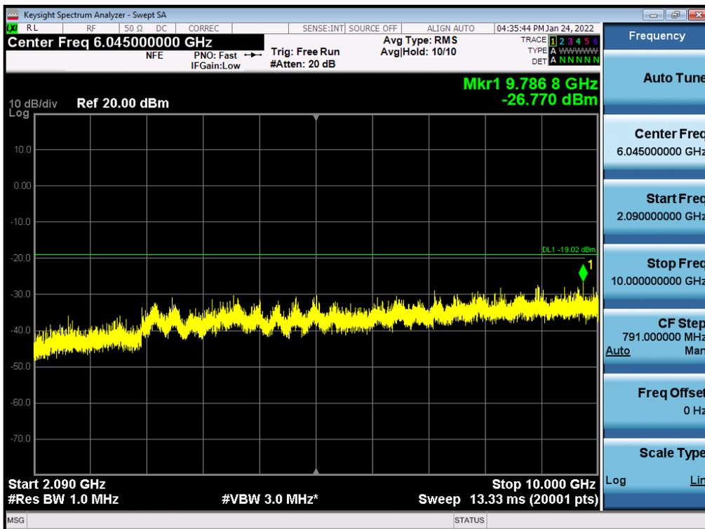
Antenna 2 / 10 GHz ~ 26.5 GHz / (4 Port) LTE B2 5 MHz 1 Carrier + LTE B2 5 MHz 1 Carrier + 5G NR n2 5 MHz 1 Carrier [3 Carrier] / Contiguous / 16QAM / High
