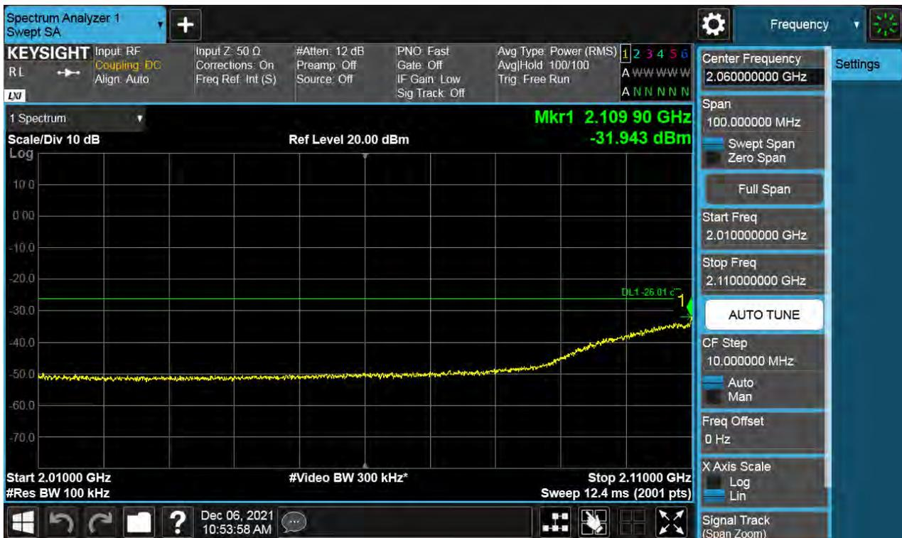
Antenna 0 / High Edge ~ High Edge + 100 MHz / (2 Port) B66 DSS 20 MHz 9to1 1 Carrier + LTE B66 10 MHz 1 Carrier + LTE B66 5 MHz 1 Carrier + LTE B66 5 MHz 1 Carrier [4 Carrier] / Contiguous / 256QAM / Middle
