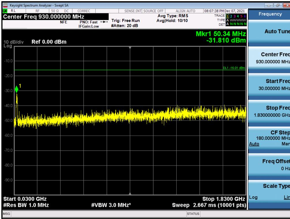
Antenna 1 / Low Edge - 100 MHz ~ Low Edge / (2 Port) B2 DSS 10 MHz 9to1 1 Carrier + LTE B2 5 MHz 1 Carrier [2 Carrier] / Non-Contiguous / QPSK
