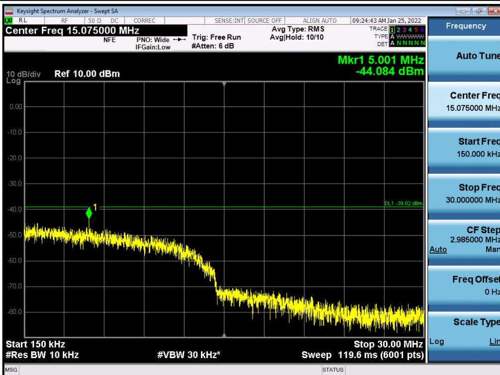
Antenna 2 / 30 MHz ~ Low Edge - 100 MHz / (4 Port) LTE B2 5 MHz 1 Carrier + LTE B2 5 MHz 1 Carrier + 5G NR n2 5 MHz 1 Carrier [3 Carrier] / Contiguous / 256QAM / High
