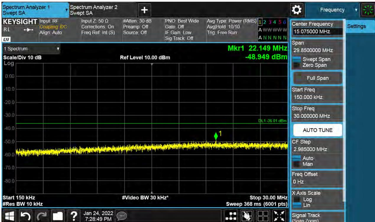
Antenna 1 / 30 MHz ~ Low Edge - 100 MHz / (2 Port) LTE B66 5 MHz 1 Carrier + LTE B66 5 MHz 1 Carrier + LTE B66 5 MHz 1 Carrier + 5G NR n66 5 MHz 1 Carrier [4 Carrier] / Contiguous / QPSK / Middle
