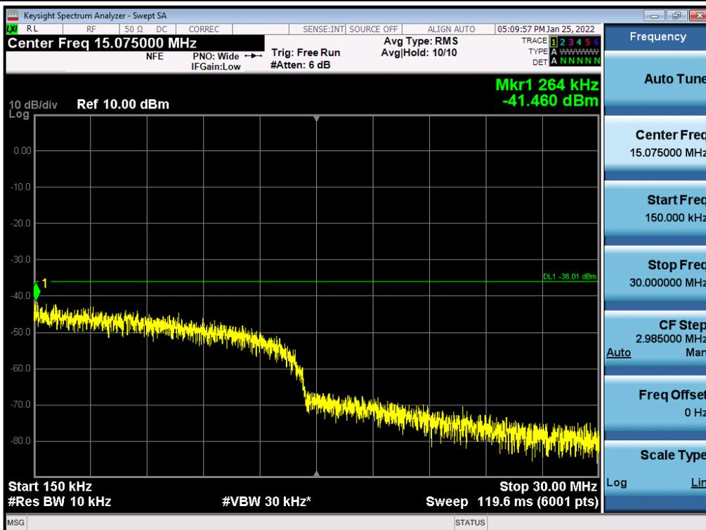
Antenna 0 / 30 MHz ~ Low Edge - 100 MHz / (2 Port) LTE B2 5 MHz 1 Carrier + LTE B2 5 MHz 1 Carrier + 5G NR n2 5 MHz 1 Carrier [3 Carrier] / Contiguous / 256QAM / High
