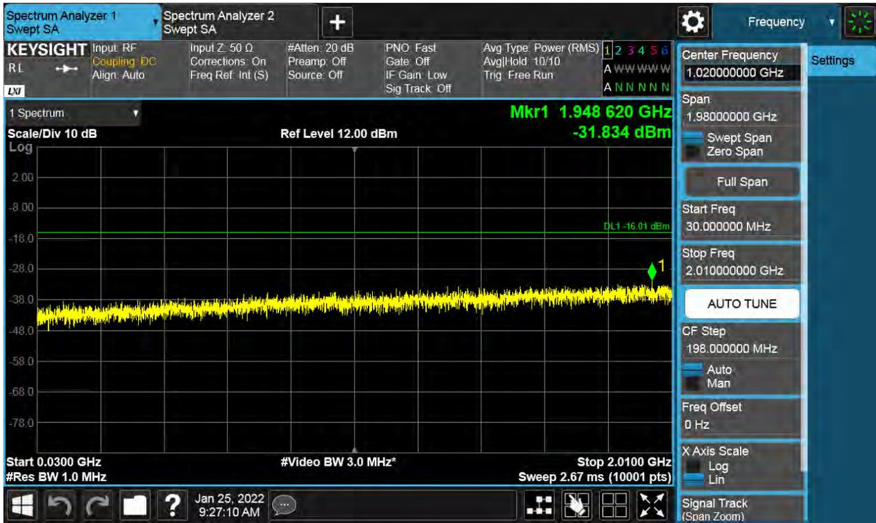
Antenna 0 / Low Edge - 100 MHz ~ Low Edge / (2 Port) LTE B66 5 MHz 1 Carrier + LTE B66 5 MHz 1 Carrier + LTE B66 10 MHz 1 Carrier + 5G NR n66 20 MHz 1 Carrier [4 Carrier] / Contiguous / 16QAM / Middle
