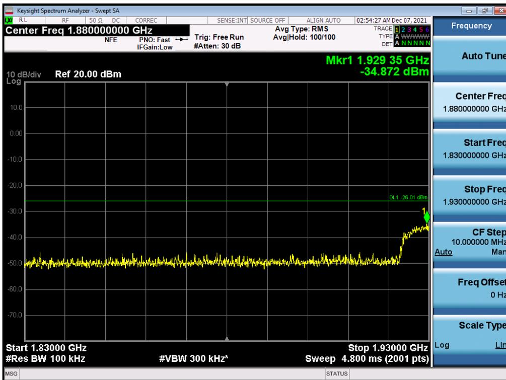
Antenna 1 / High Edge ~ High Edge + 100 MHz / (2 Port) B2 DSS 20 MHz 9to1 1 Carrier + LTE B2 5 MHz 1 Carrier + LTE B2 5 MHz 1 Carrier [3 Carrier] / Contiguous / 64QAM / High
