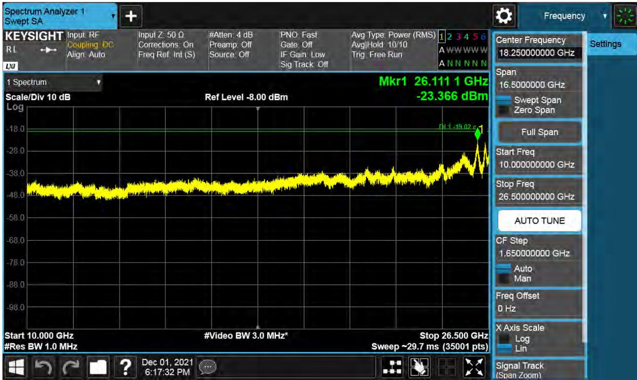
Antenna 0 / 9 kHz ~ 150 kHz / (2 Port) LTE B66 5 MHz 1 Carrier + LTE B66 5 MHz 1 Carrier + LTE B66 5 MHz 1 Carrier + 5G NR n66 5 MHz 1 Carrier [4 Carrier] / Contiguous / 16QAM / Middle
