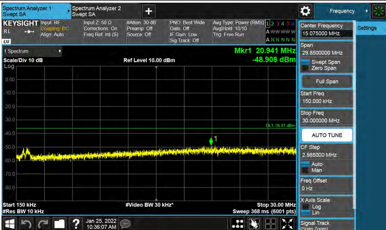
Antenna 1 / 30 MHz ~ Low Edge - 100 MHz / (2 Port) LTE B66 5 MHz 1 Carrier + LTE B66 5 MHz 1 Carrier + LTE B66 10 MHz 1 Carrier + 5G NR n66 20 MHz 1 Carrier [4 Carrier] / Contiguous / QPSK / Low
