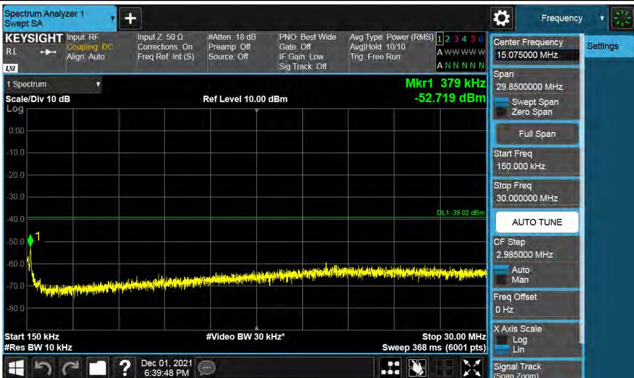
Antenna 0 / 30 MHz ~ Low Edge - 100 MHz / (4 Port) B66 DSS 20 MHz 9to1 1 Carrier + LTE B66 10 MHz 1 Carrier + LTE B66 5 MHz 1 Carrier + LTE B66 5 MHz 1 Carrier [4 Carrier] / Contiguous / 64QAM / Low
