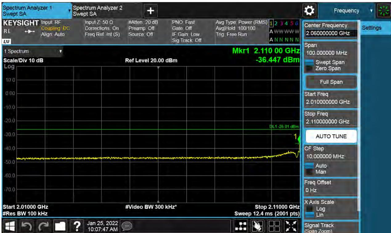
**Antenna 1 / High Edge ~ High Edge + 100 MHz / (2 Port) LTE B66 5 MHz 1 Carrier + LTE B66 5 MHz 1 Carrier + LTE B66 10 MHz 1 Carrier + 5G NR n66 20 MHz 1 Carrier [4 Carrier] / Contiguous / 16QAM / High**
