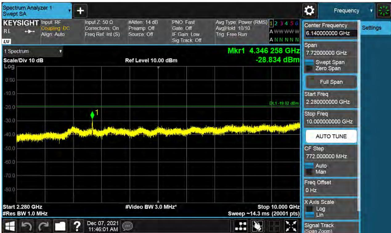
Antenna 1 / 10 GHz ~ 26.5 GHz / (4 Port) B66 DSS 10 MHz 9to1 1 Carrier + LTE B66 5 MHz 1 Carrier [2 Carrier] / Contiguous / 16QAM / Low
