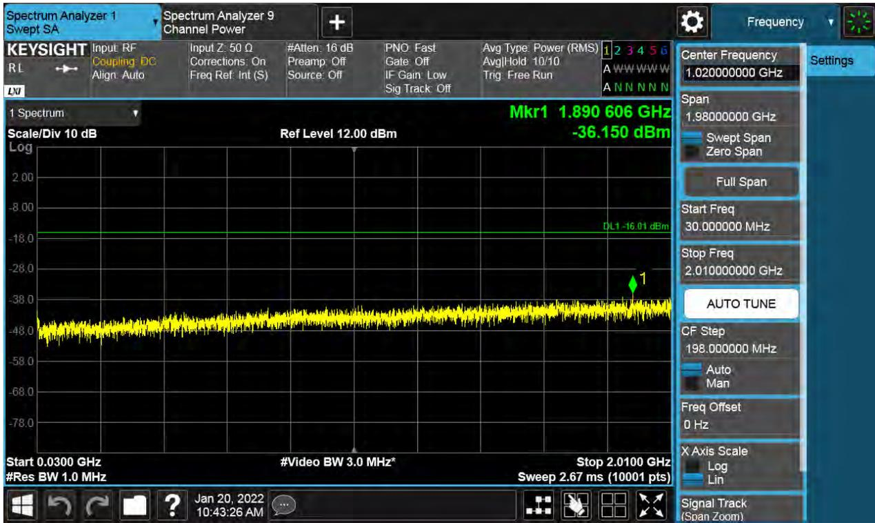
Antenna 0 / Low Edge - 100 MHz ~ Low Edge / (2 Port) LTE B66 20 MHz 1 Carrier + 5G NR n66 20 MHz 1 Carrier [2 Carrier] / Contiguous / 16QAM / Middle
