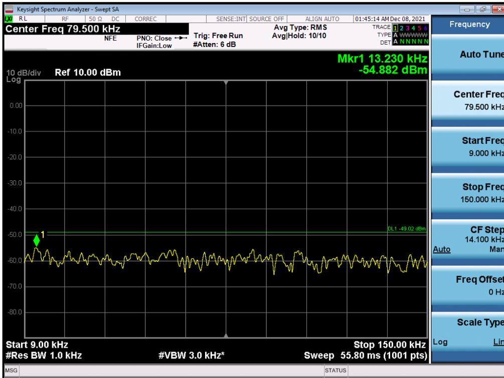
Antenna 3 / 150 kHz ~ 30 MHz / (4 Port) B2 DSS 10 MHz 9to1 1 Carrier + LTE B2 5 MHz 1 Carrier [2 Carrier] / Contiguous / QPSK / High
