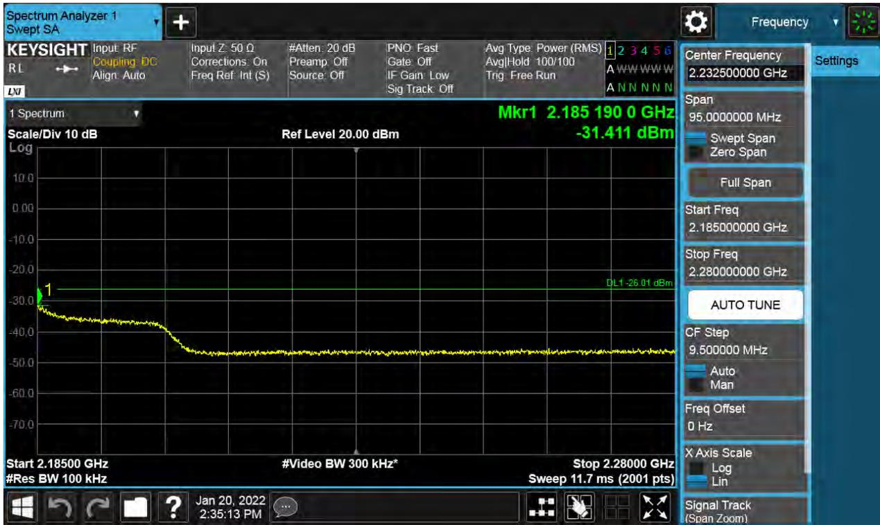
**Antenna 1 / High Edge + 100 MHz ~ 10 GHz / (2 Port) LTE B66 5 MHz 1 Carrier + 5G NR n66 5 MHz 1 Carrier [2 Carrier] / Contiguous / 16QAM / High**
