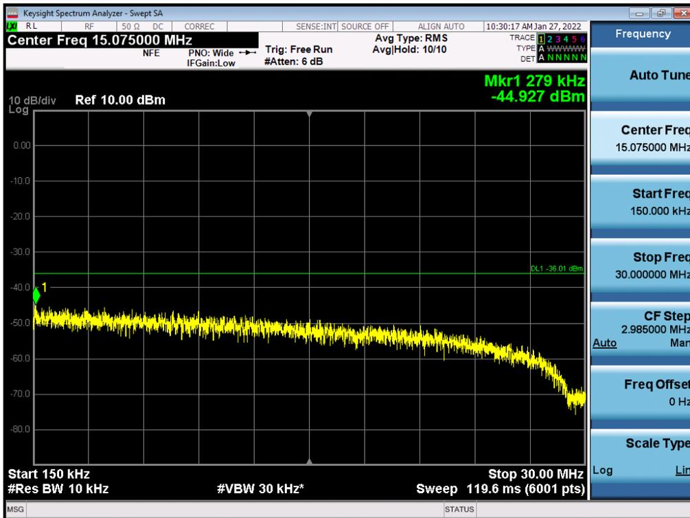
Antenna 0 / 30 MHz ~ Low Edge - 100 MHz / (2 Port) LTE B2 10 MHz 1 Carrier + 5G NR n2 20 MHz 1 Carrier [2 Carrier] / Contiguous / 64QAM / Middle
