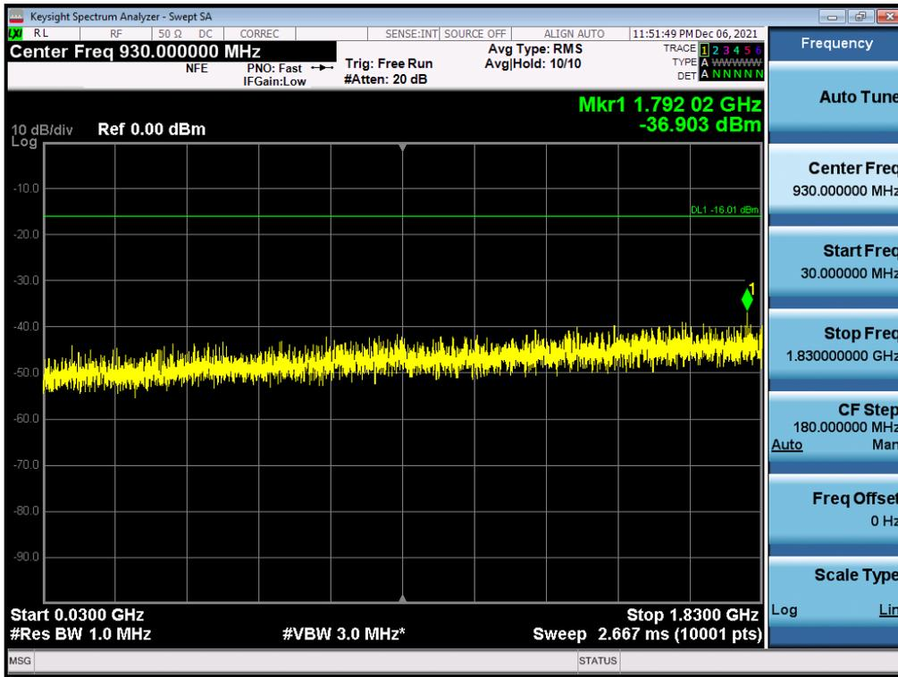
Antenna 1 / Low Edge - 100 MHz ~ Low Edge / (2 Port) B2 DSS 10 MHz 9to1 1 Carrier + LTE B2 5 MHz 1 Carrier [2 Carrier] / Contiguous / QPSK / Low
