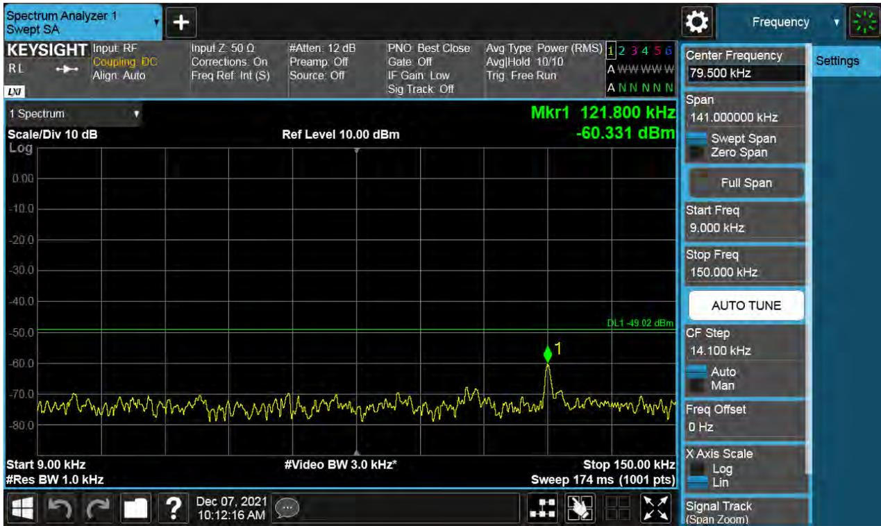
Antenna 1 / 150 kHz ~ 30 MHz / (4 Port) B66 DSS 10 MHz 9to1 1 Carrier + LTE B66 5 MHz 1 Carrier [2 Carrier] / Contiguous / 16QAM / High
