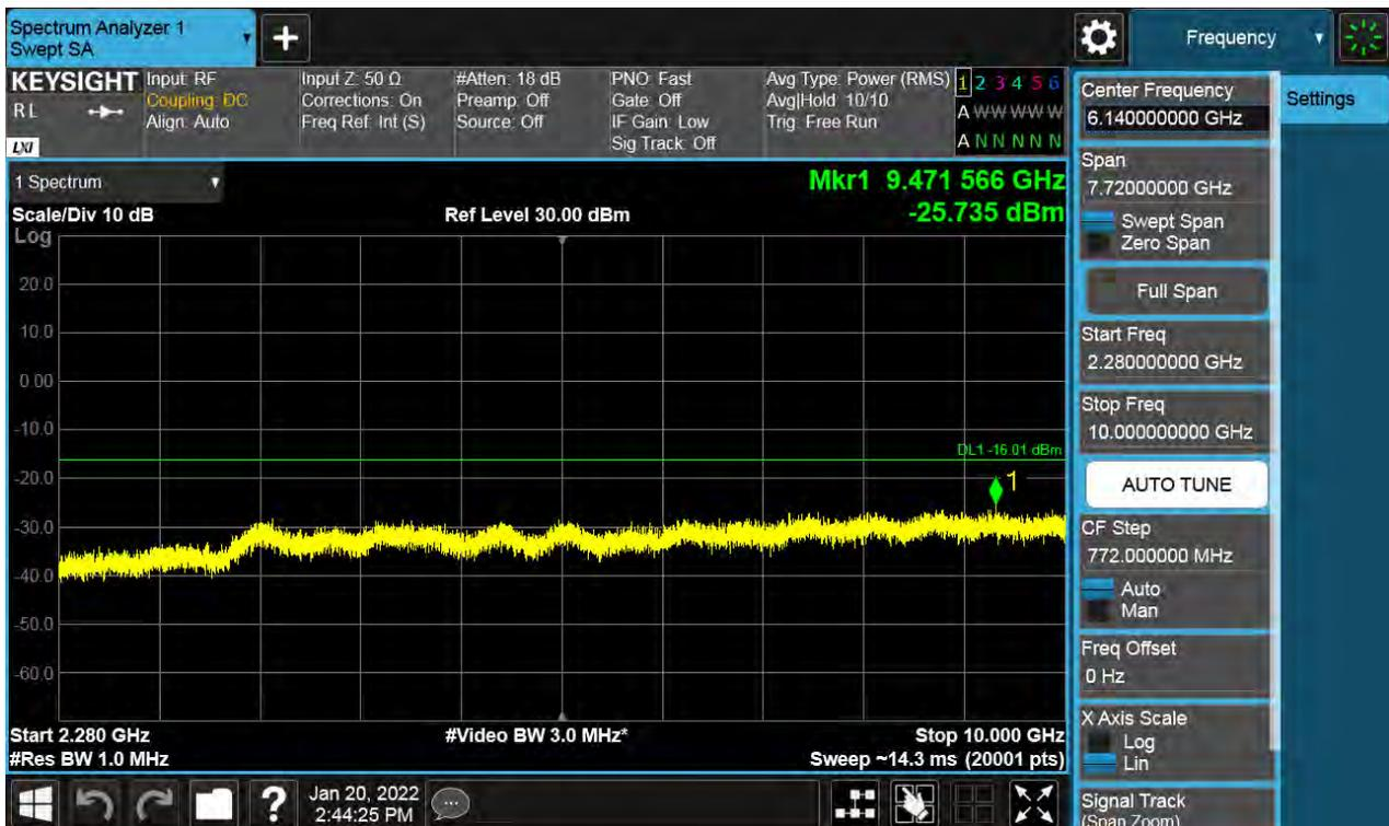
Antenna 1 / 10 GHz ~ 26.5 GHz / (2 Port) LTE B66 5 MHz 1 Carrier + 5G NR n66 5 MHz 1 Carrier [2 Carrier] / Contiguous / 64QAM / High
