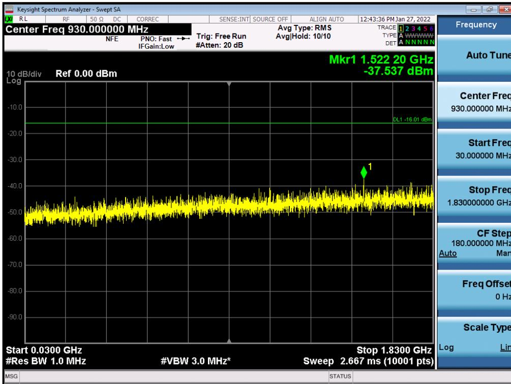
Antenna 1 / Low Edge - 100 MHz ~ Low Edge / (2 Port) LTE B2 5 MHz 1 Carrier + 5G NR n2 5 MHz 1 Carrier [2 Carrier] / Contiguous / QPSK / Low
