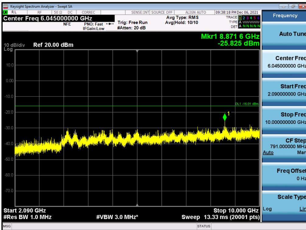
Antenna 0 / 10 GHz ~ 26.5 GHz / (2 Port) B2 DSS 10 MHz 9to1 1 Carrier + LTE B2 5 MHz 1 Carrier [2 Carrier] / Contiguous / 16QAM / Low
