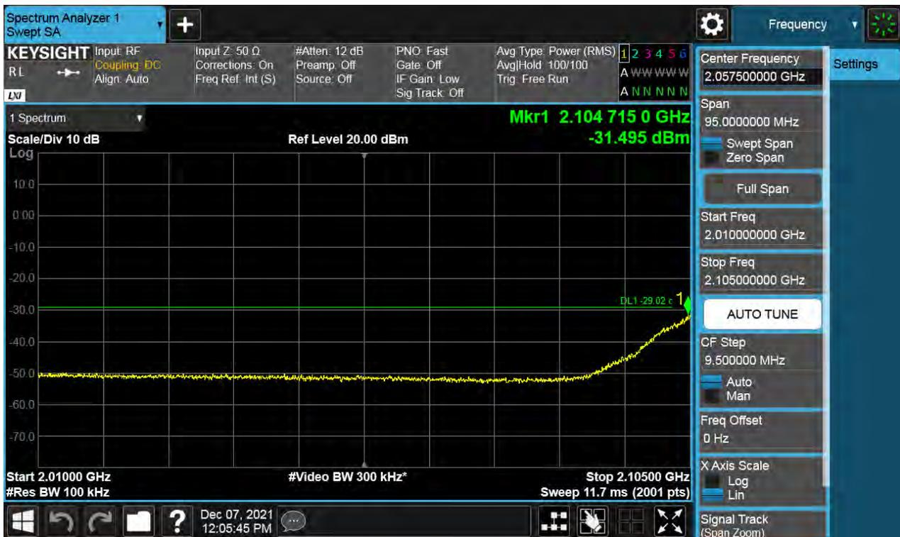
Antenna 2 / High Edge ~ High Edge + 100 MHz / (4 Port) B66 DSS 10 MHz 9to1 1 Carrier + LTE B66 5 MHz 1 Carrier [2 Carrier] / Contiguous / 64QAM / High
