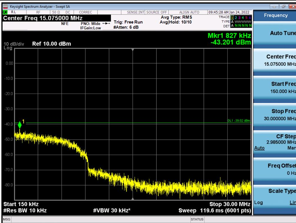
Antenna 2 / 30 MHz ~ Low Edge - 100 MHz / (4 Port) LTE B2 5 MHz 1 Carrier + 5G NR n2 5 MHz 1 Carrier [2 Carrier] / Contiguous / QPSK / Low
