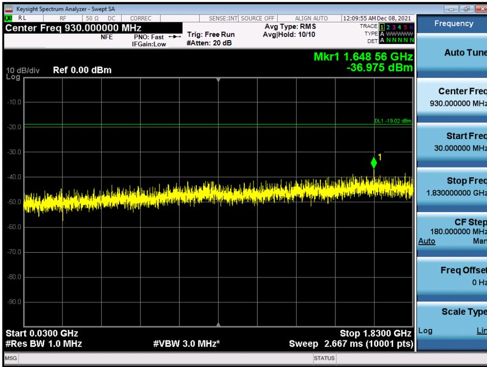
Antenna 2 / Low Edge - 100 MHz ~ Low Edge / (4 Port) B2 DSS 10 MHz 9to1 1 Carrier + LTE B2 5 MHz 1 Carrier [2 Carrier] / Contiguous / 64QAM / Low
