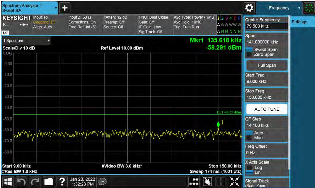
Antenna 1 / 150 kHz ~ 30 MHz / (2 Port) LTE B66 5 MHz 1 Carrier + 5G NR n66 5 MHz 1 Carrier [2 Carrier] / Contiguous / 16QAM / Low
