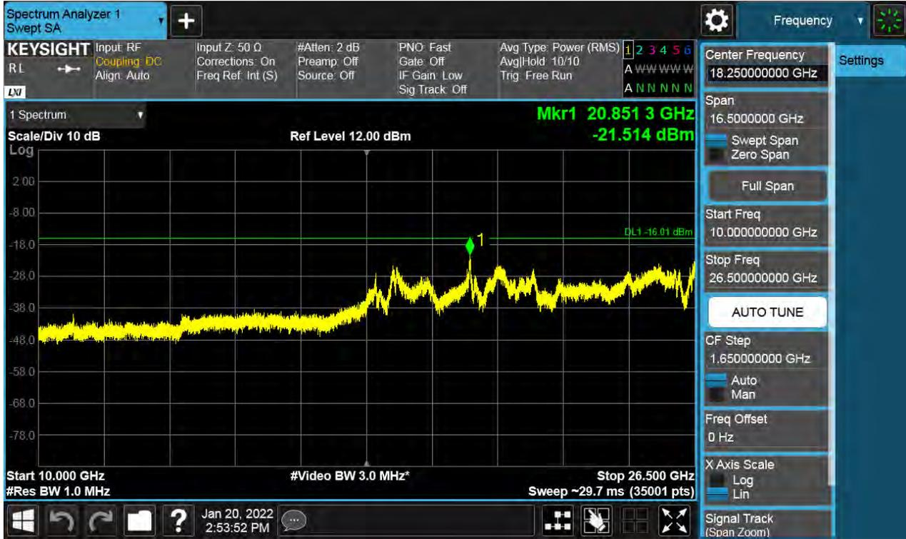
Antenna 0 / 9 kHz ~ 150 kHz / (2 Port) LTE B66 20 MHz 1 Carrier + 5G NR n66 20 MHz 1 Carrier [2 Carrier] / Contiguous / 16QAM / Middle
