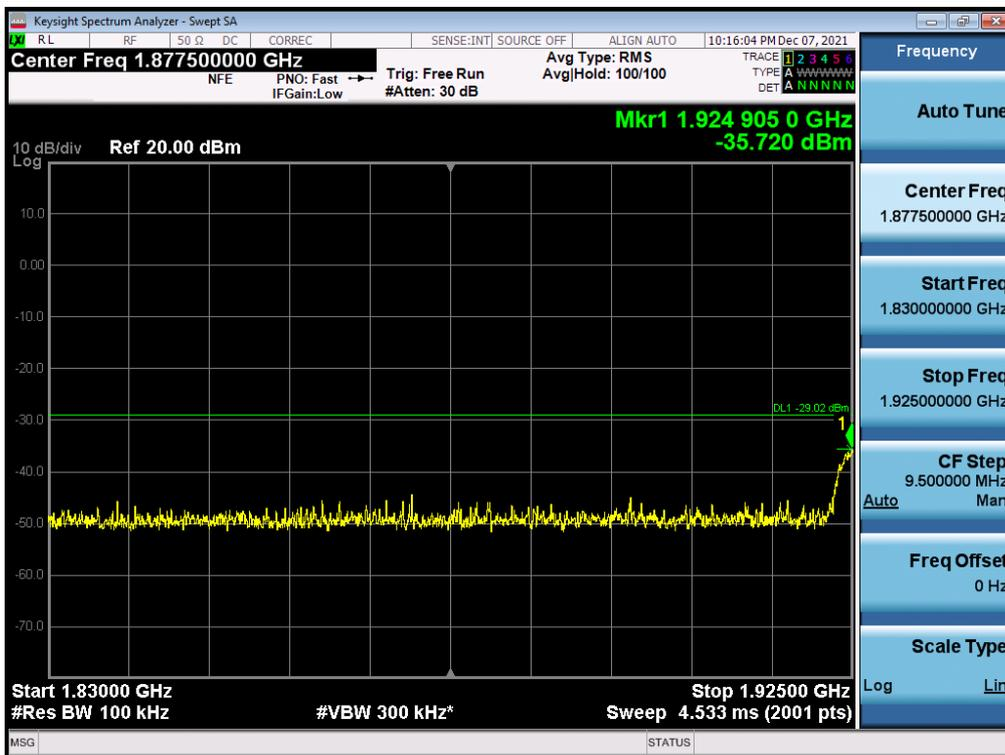
Antenna 0 / High Edge ~ High Edge + 100 MHz / (4 Port) B2 DSS 10 MHz 9to1 1 Carrier + LTE B2 5 MHz 1 Carrier [2 Carrier] / Contiguous / 16QAM / High
