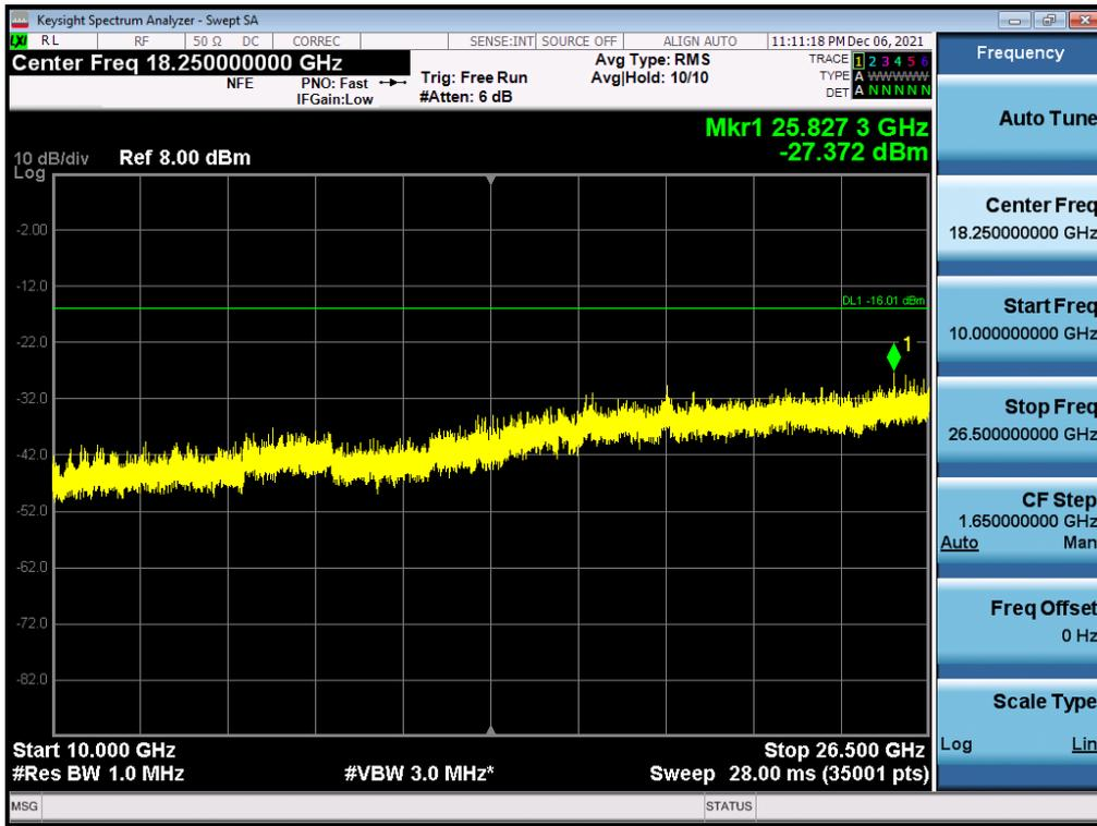
Antenna 2 / 9 kHz ~ 150 kHz / (4 Port) B2 DSS 10 MHz 9to1 1 Carrier + LTE B2 5 MHz 1 Carrier [2 Carrier] / Contiguous / 16QAM / High
