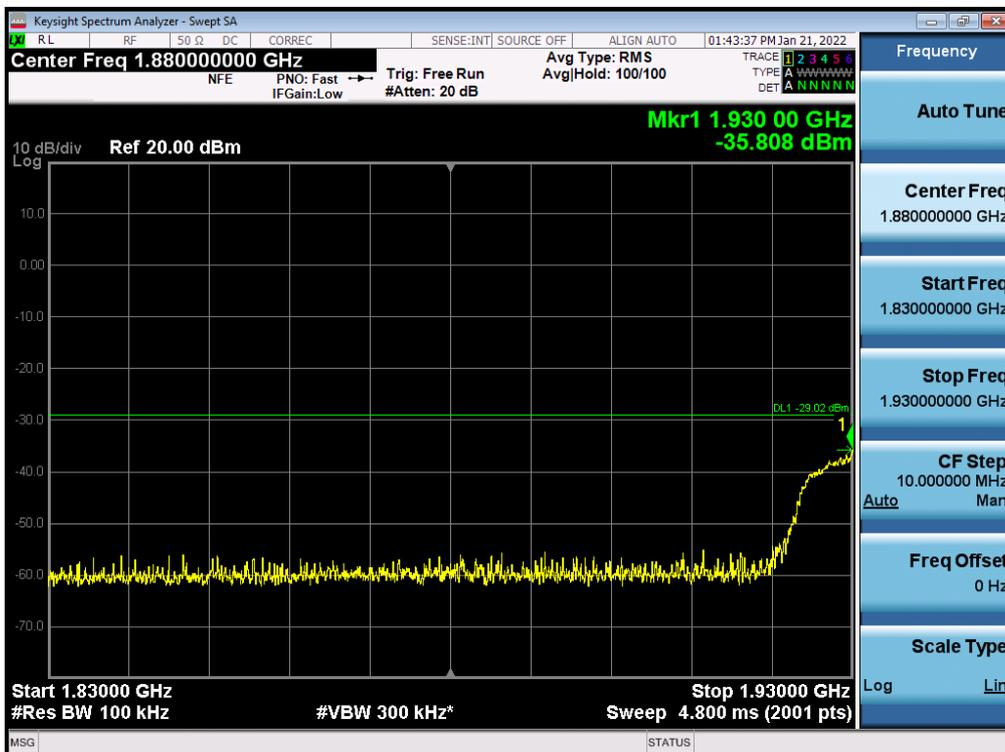
Antenna 1 / High Edge ~ High Edge + 100 MHz / (4 Port) LTE B2 10 MHz 1 Carrier + 5G NR n2 20 MHz 1 Carrier [2 Carrier] / Contiguous / 256QAM / Middle
