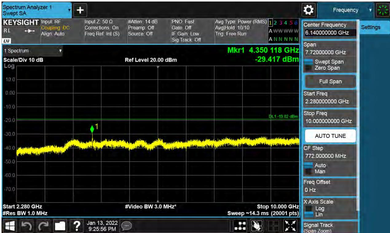
Antenna 2 / 10 GHz ~ 26.5 GHz / (4 Port) 5G NR n66 10 MHz 1 Carrier / 64QAM / Middle
