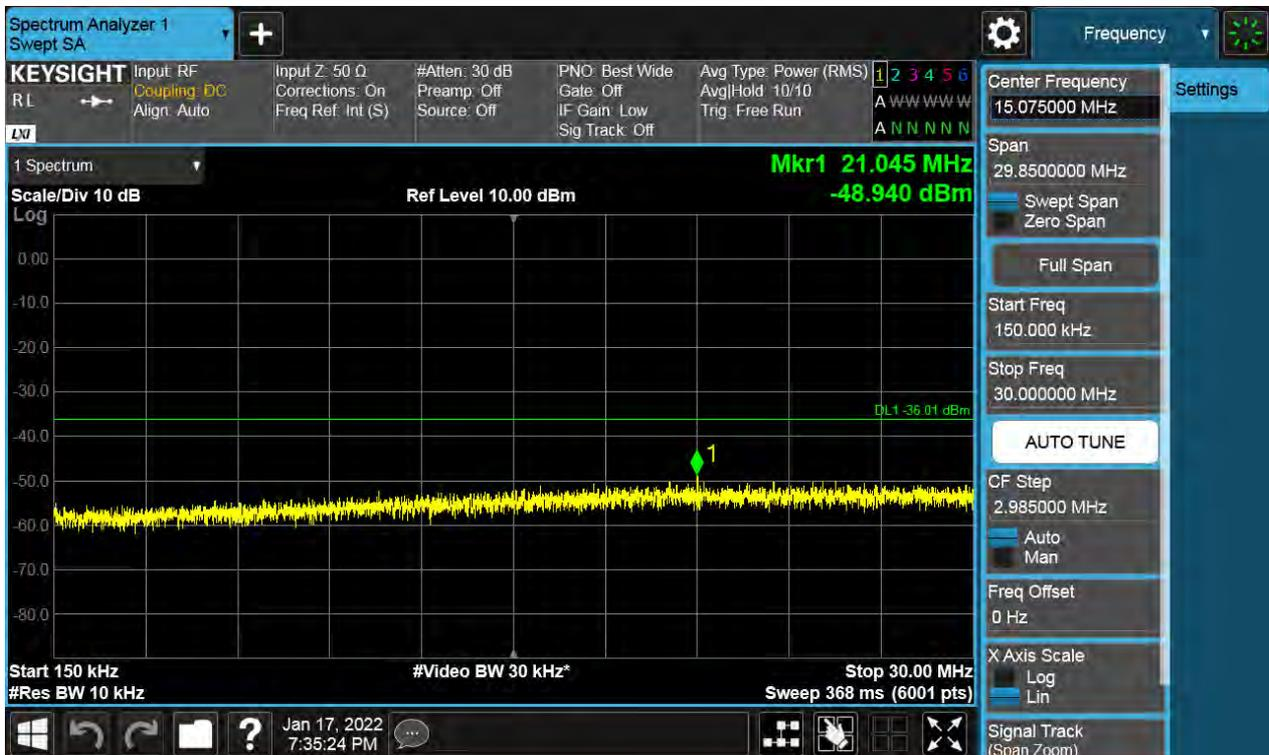
Antenna 1 / 30 MHz ~ Low Edge - 100 MHz / (2 Port) 5G NR n66 20 MHz 1 Carrier / 16QAM / High
