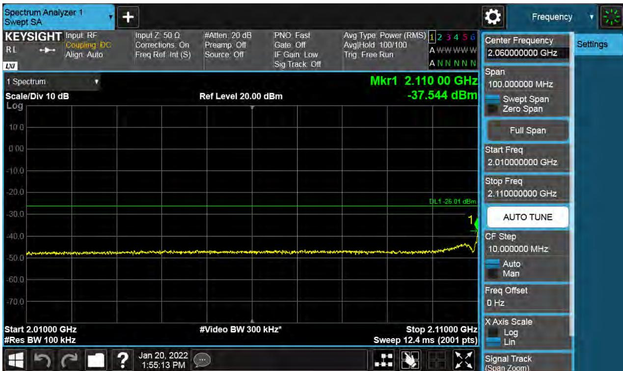
**Antenna 0 / High Edge ~ High Edge + 100 MHz / (2 Port) LTE B66 5 MHz 1 Carrier + 5G NR n66 5 MHz 1 Carrier [2 Carrier] / Contiguous / 16QAM / High**
