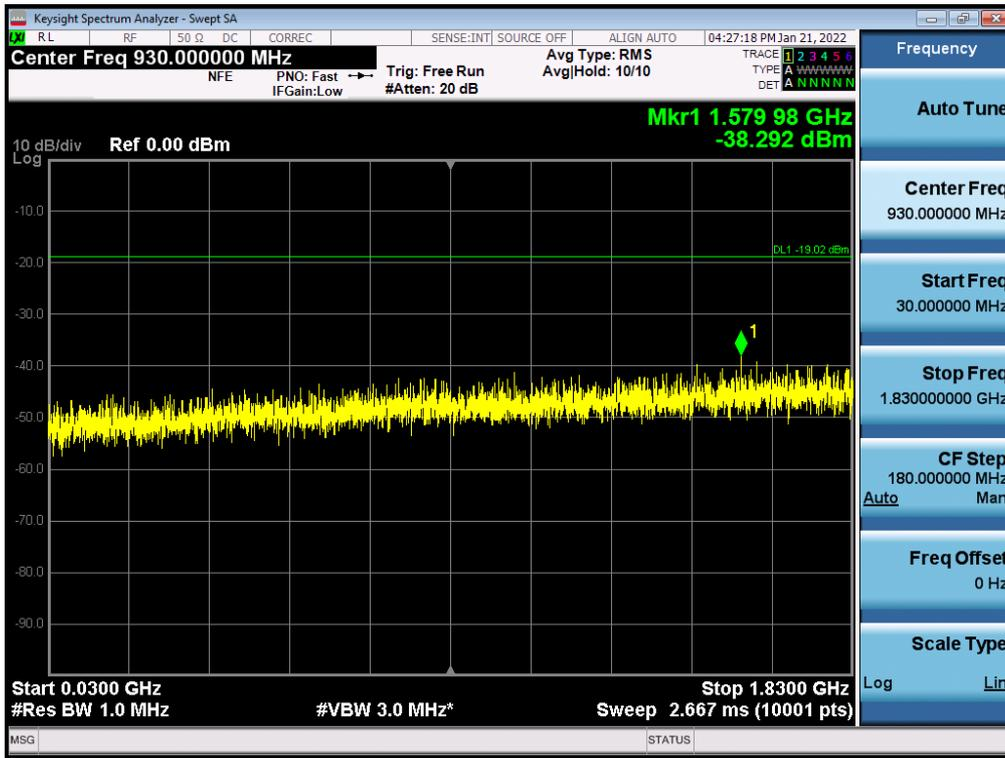
Antenna 3 / Low Edge - 100 MHz ~ Low Edge / (4 Port) LTE B2 5 MHz 1 Carrier + 5G NR n2 5 MHz 1 Carrier [2 Carrier] / Contiguous / QPSK / Low
