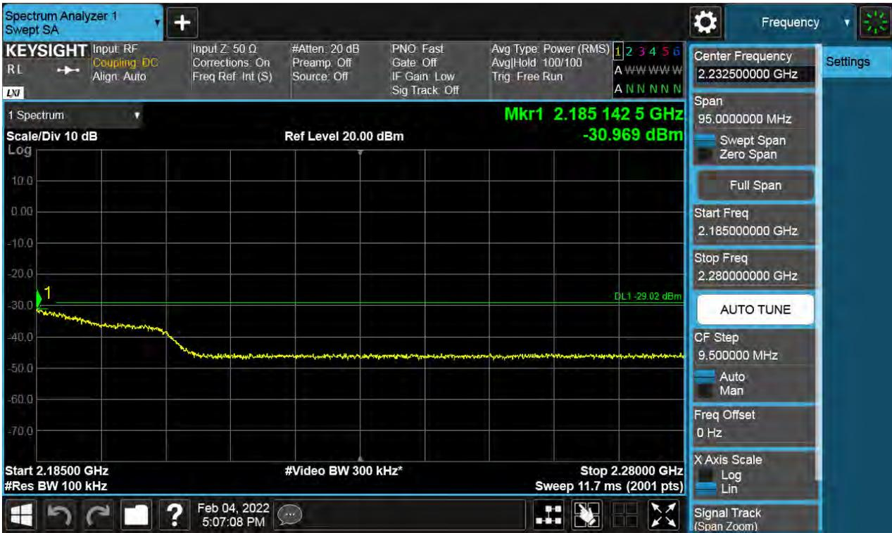
Antenna 0 / High Edge + 100 MHz ~ 10 GHz / (2 Port) B66 DSS 10 MHz 9to1 1 Carrier + LTE B66 5 MHz 1 Carrier [2 Carrier] / Contiguous / 256QAM / High
