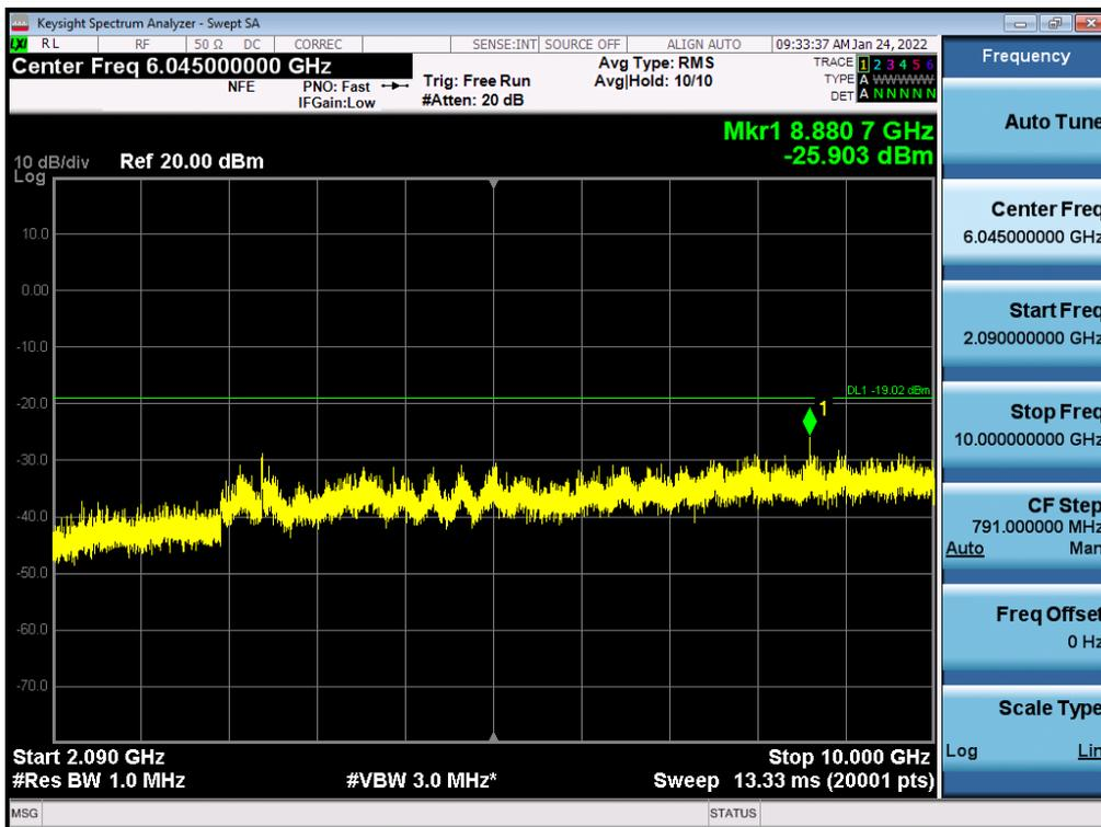
Antenna 1 / 10 GHz ~ 26.5 GHz / (4 Port) LTE B2 5 MHz 1 Carrier + 5G NR n2 5 MHz 1 Carrier [2 Carrier] / Contiguous / 256QAM / High
