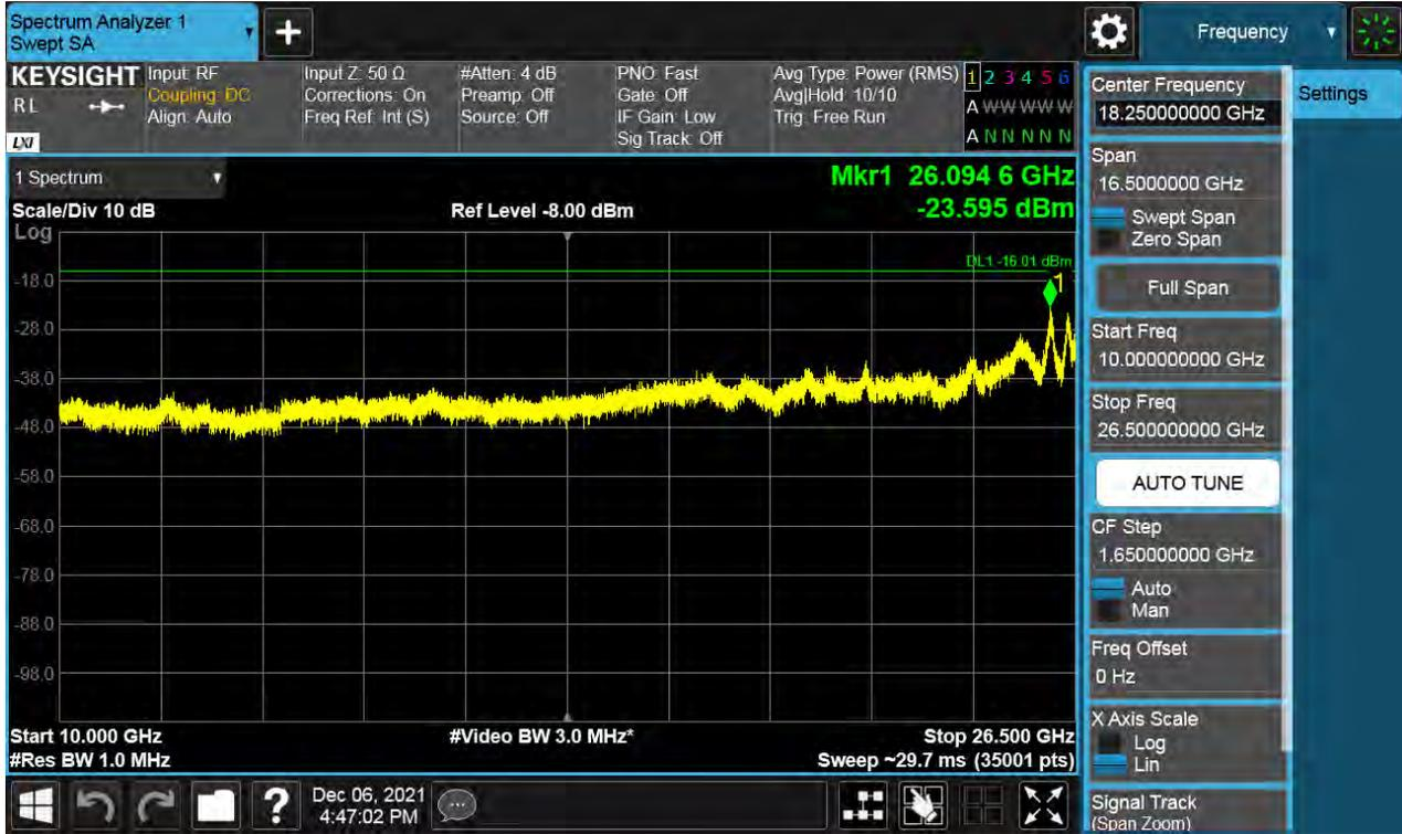
Antenna 3 / 9 kHz ~ 150 kHz / (4 Port) B66 DSS 10 MHz 9to1 1 Carrier + LTE B66 5 MHz 1 Carrier [2 Carrier] / Contiguous / 16QAM / Middle
