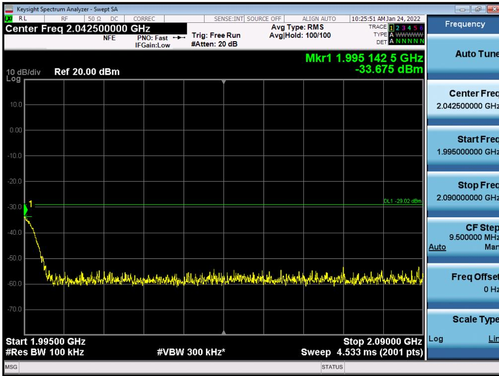
Antenna 1 / High Edge + 100 MHz ~ 10 GHz / (4 Port) LTE B2 5 MHz 1 Carrier + 5G NR n2 5 MHz 1 Carrier [2 Carrier] / Contiguous / QPSK / High
