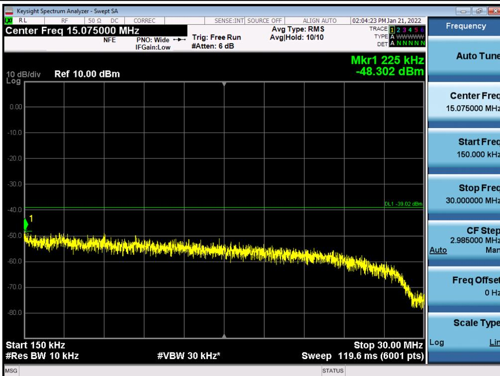
Antenna 1 / 30 MHz ~ Low Edge - 100 MHz / (4 Port) LTE B2 10 MHz 1 Carrier + 5G NR n2 20 MHz 1 Carrier [2 Carrier] / Contiguous / QPSK / High
