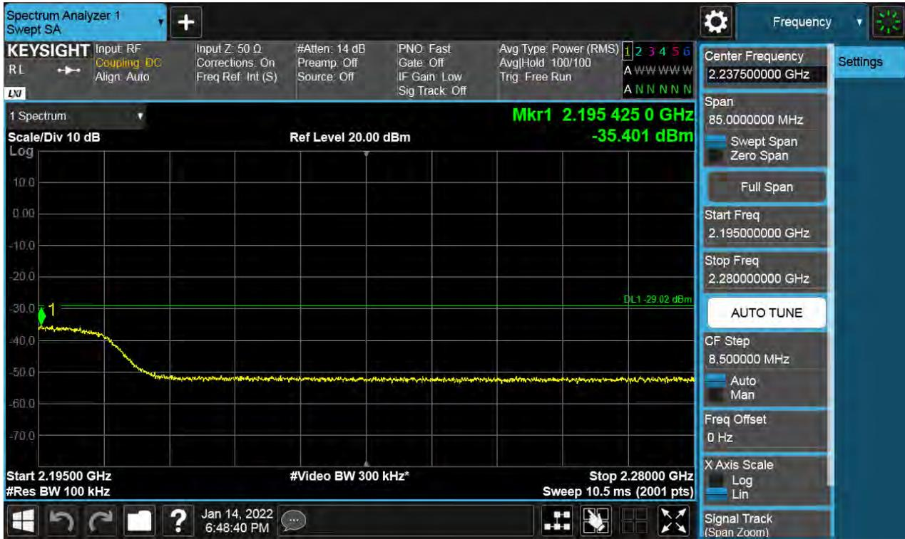
Antenna 2 / High Edge + 100 MHz ~ 10 GHz / (4 Port) 5G NR n66 15 MHz 1 Carrier / 16QAM / Middle
