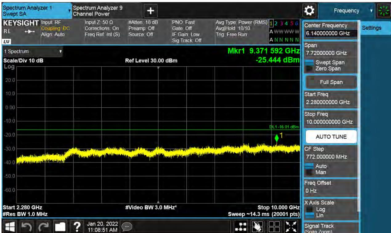
Antenna 1 / 10 GHz ~ 26.5 GHz / (2 Port) LTE B66 20 MHz 1 Carrier + 5G NR n66 20 MHz 1 Carrier [2 Carrier] / Contiguous / 64QAM / Middle
