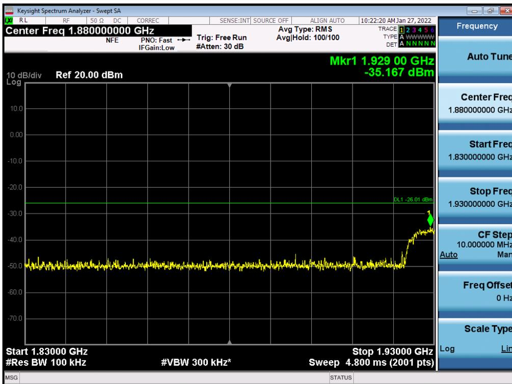
Antenna 0 / High Edge ~ High Edge + 100 MHz / (2 Port) LTE B2 10 MHz 1 Carrier + 5G NR n2 20 MHz 1 Carrier [2 Carrier] / Contiguous / 64QAM / Middle
