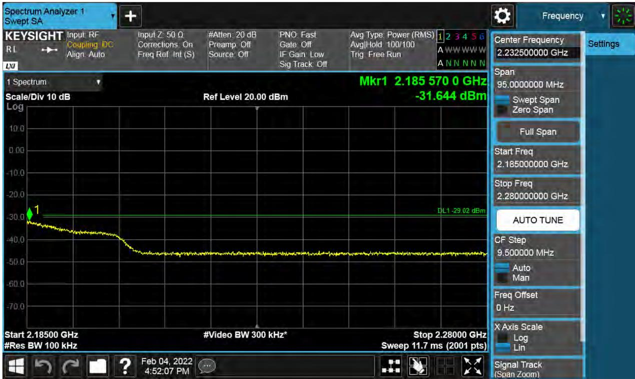
Antenna 0 / High Edge + 100 MHz ~ 10 GHz / (4 Port) B66 DSS 10 MHz 9to1 1 Carrier + LTE B66 5 MHz 1 Carrier [2 Carrier] / Contiguous / 256QAM / High
