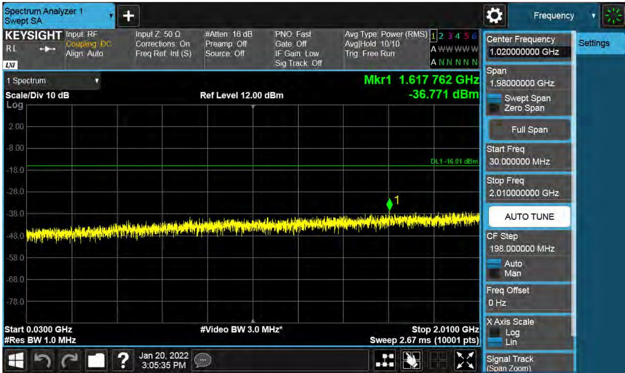
Antenna 0 / Low Edge - 100 MHz ~ Low Edge / (2 Port) LTE B66 5 MHz 1 Carrier + 5G NR n66 5 MHz 1 Carrier [2 Carrier] / Contiguous / 16QAM / Middle
