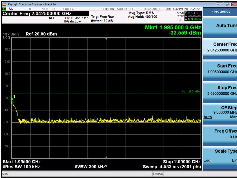
Antenna 0 / High Edge + 100 MHz ~ 10 GHz / (2 Port) LTE B2 5 MHz 1 Carrier + 5G NR n2 5 MHz 1 Carrier [2 Carrier] / Contiguous / 256QAM / High
