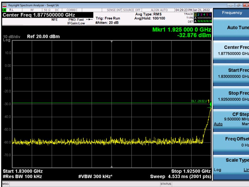
Antenna 0 / High Edge ~ High Edge + 100 MHz / (4 Port) LTE B2 5 MHz 1 Carrier + 5G NR n2 5 MHz 1 Carrier [2 Carrier] / Contiguous / 256QAM / High
