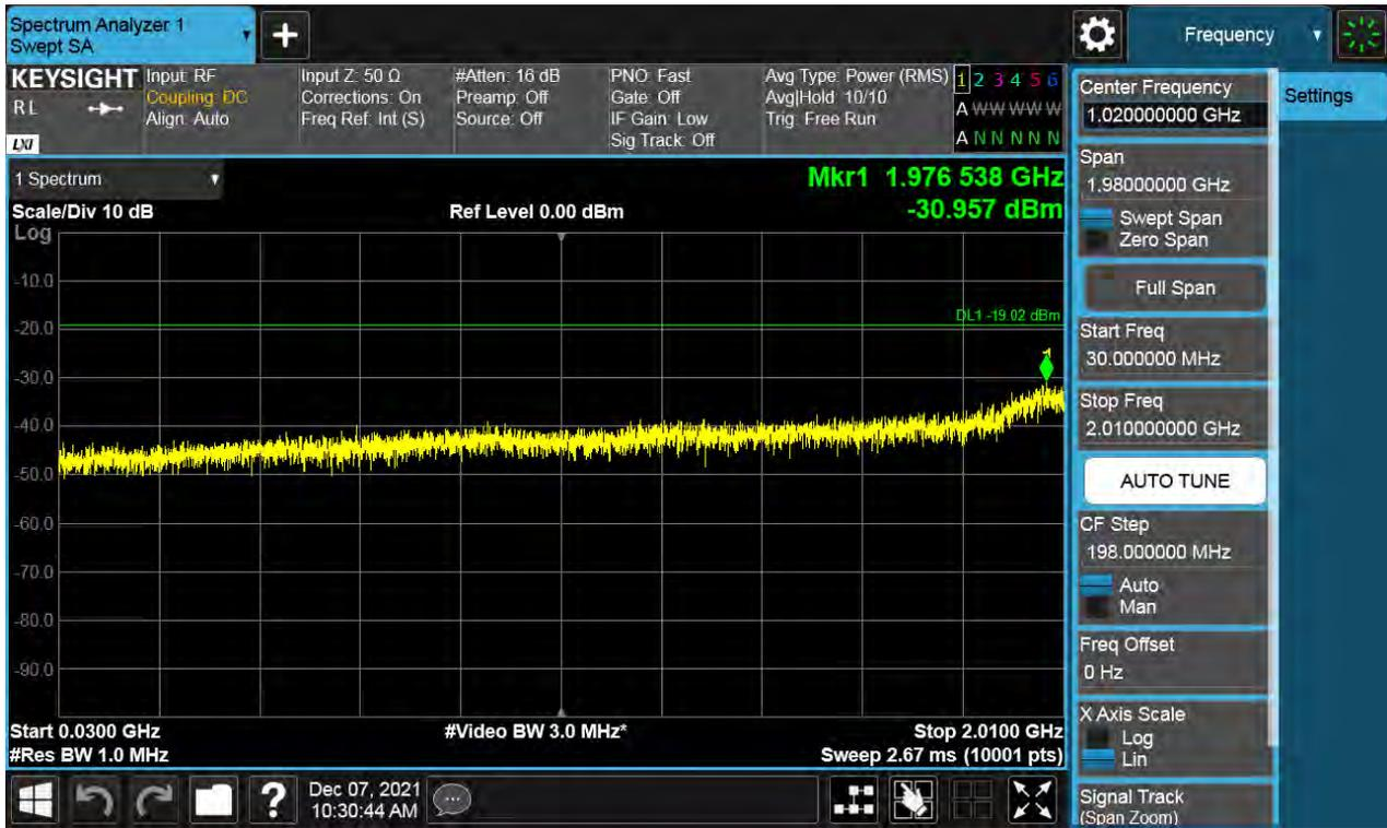
Antenna 0 / Low Edge - 100 MHz ~ Low Edge / (4 Port) B66 DSS 10 MHz 9to1 1 Carrier + LTE B66 5 MHz 1 Carrier [2 Carrier] / Contiguous / QPSK / Low
