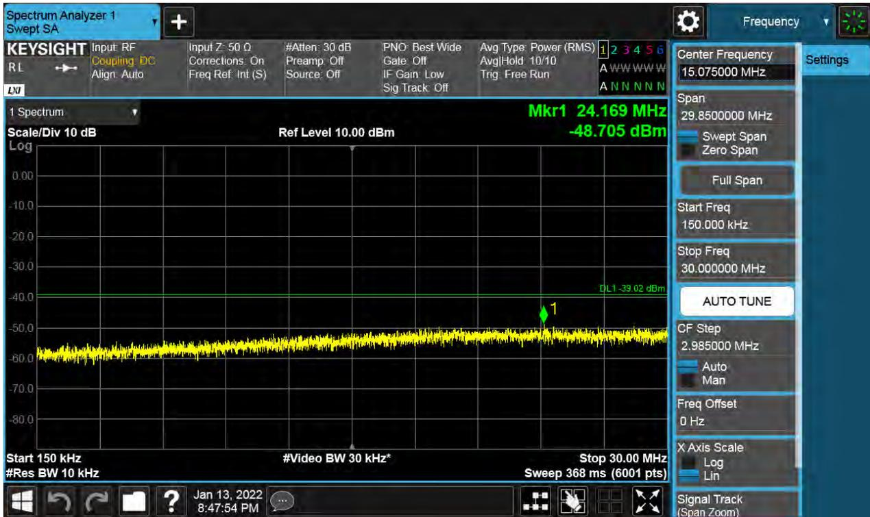
Antenna 3 / 30 MHz ~ Low Edge - 100 MHz / (4 Port) 5G NR n66 10 MHz 1 Carrier / 16QAM / Low
