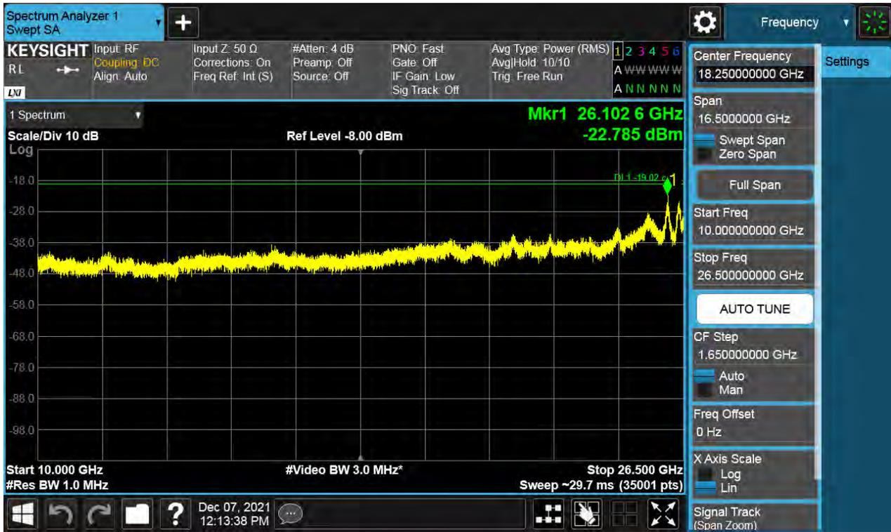
Antenna 0 / 9 kHz ~ 150 kHz / (2 Port) LTE B66 5 MHz 1 Carrier + 5G NR n66 5 MHz 1 Carrier [2 Carrier] / Contiguous / 256QAM / Low
