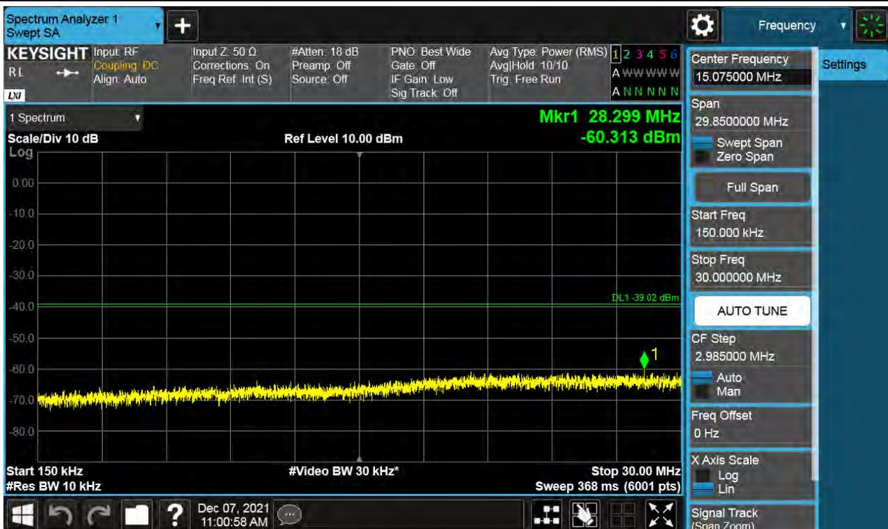
Antenna 0 / 30 MHz ~ Low Edge - 100 MHz / (4 Port) B66 DSS 10 MHz 9to1 1 Carrier + LTE B66 5 MHz 1 Carrier [2 Carrier] / Contiguous / 256QAM / Middle
