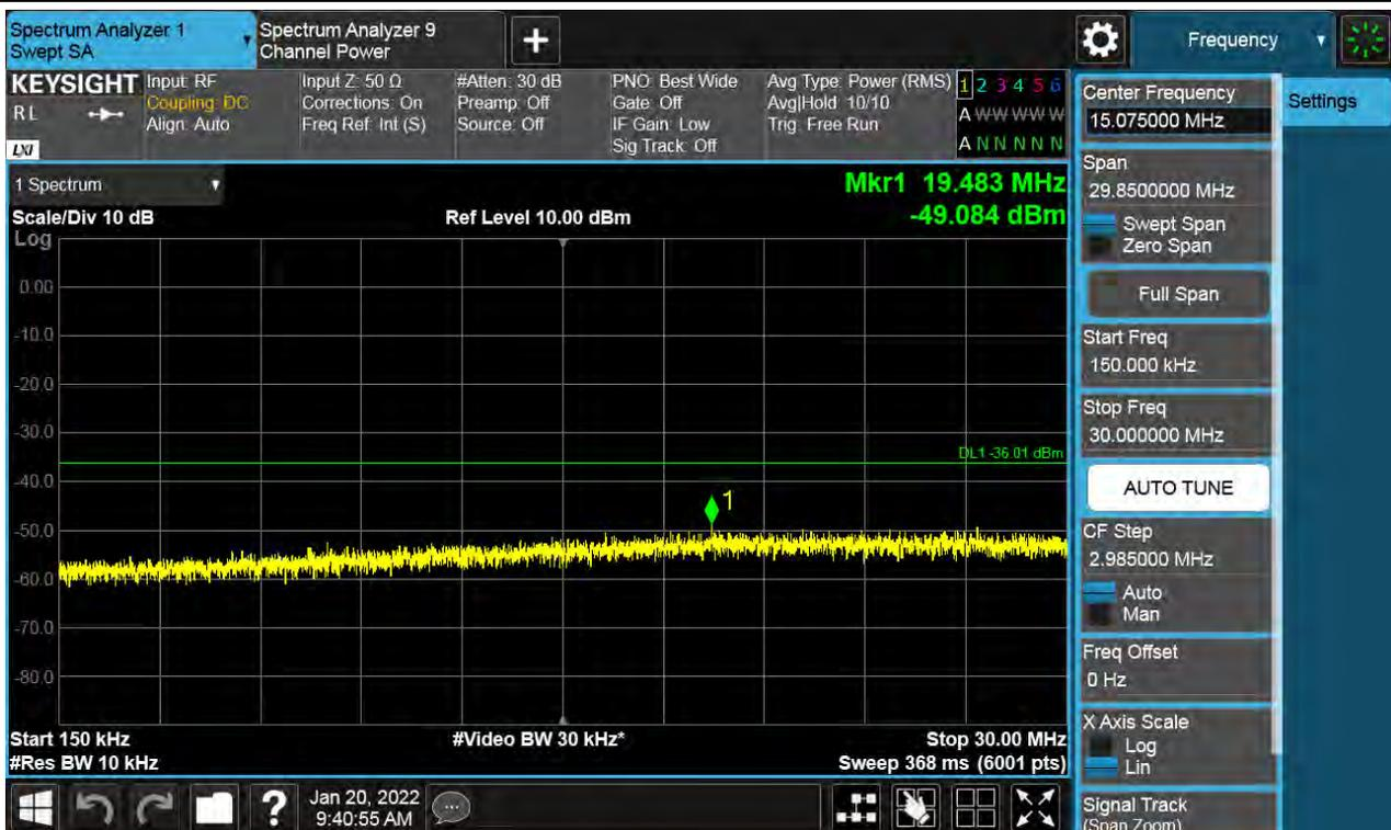
Antenna 1 / 30 MHz ~ Low Edge - 100 MHz / (2 Port) LTE B66 20 MHz 1 Carrier + 5G NR n66 20 MHz 1 Carrier [2 Carrier] / Contiguous / 256QAM / Middle
