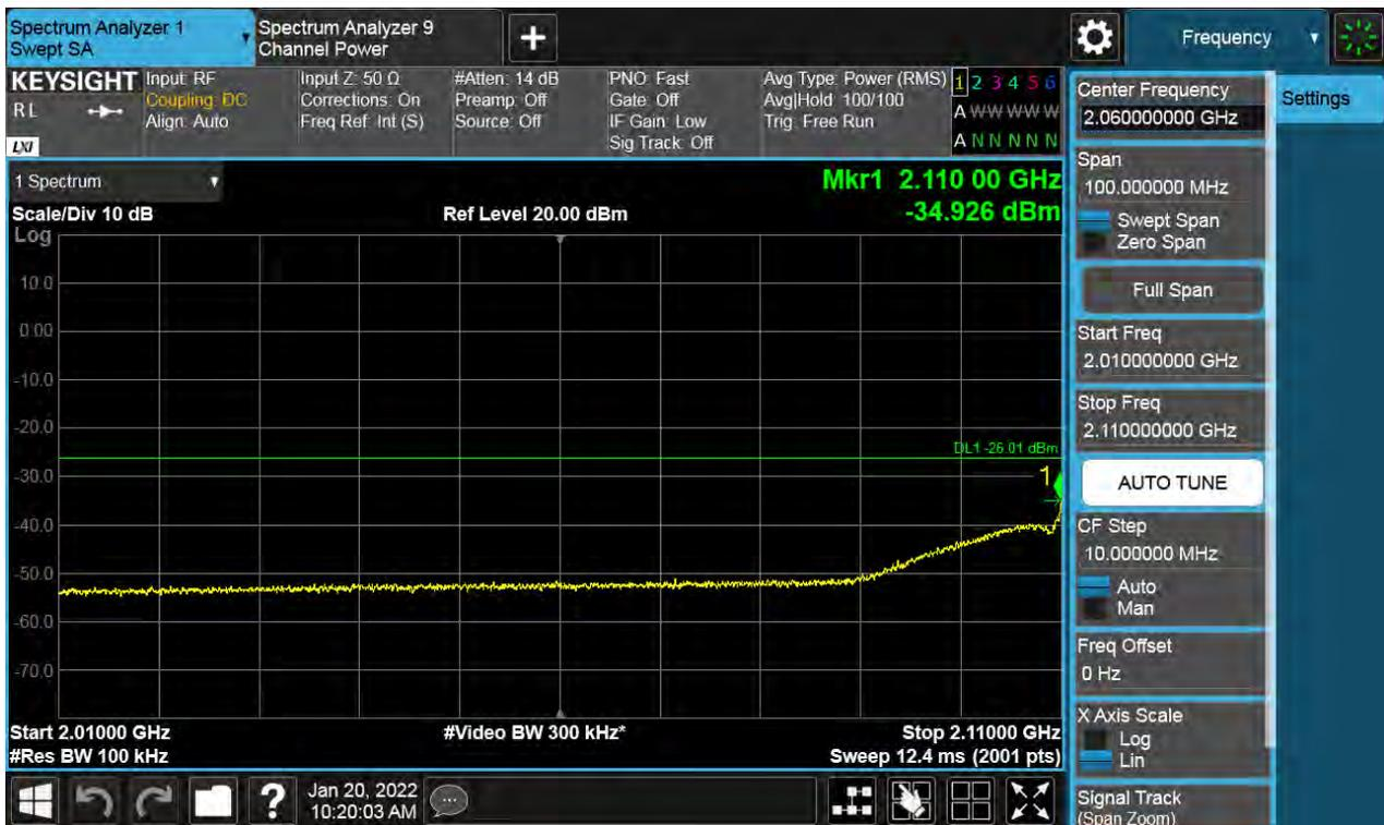
Antenna 0 / High Edge ~ High Edge + 100 MHz / (2 Port) LTE B66 20 MHz 1 Carrier + 5G NR n66 20 MHz 1 Carrier [2 Carrier] / Contiguous / 16QAM / Low
