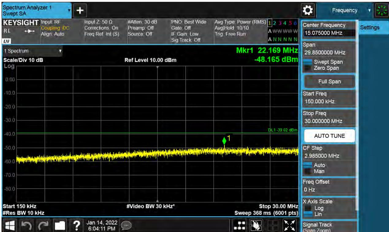
**Antenna 0 / 30 MHz ~ Low Edge - 100 MHz / (4 Port) 5G NR n66 15 MHz 1 Carrier / 16QAM / High**
