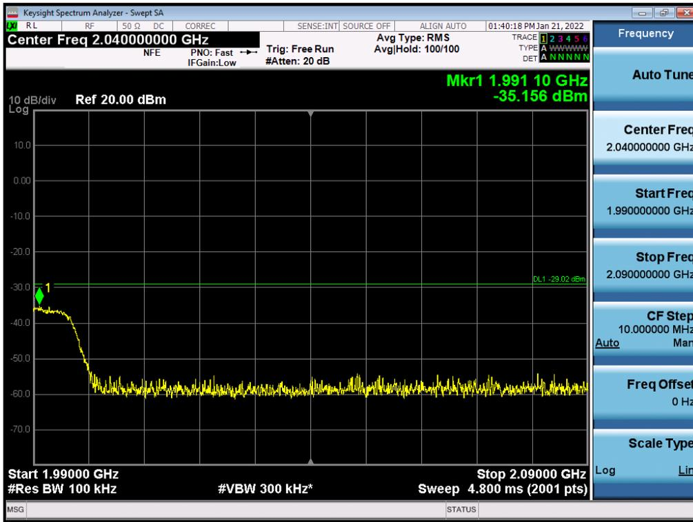
Antenna 1 / High Edge + 100 MHz ~ 10 GHz / (4 Port) LTE B2 10 MHz 1 Carrier + 5G NR n2 20 MHz 1 Carrier [2 Carrier] / Contiguous / 256QAM / Low
