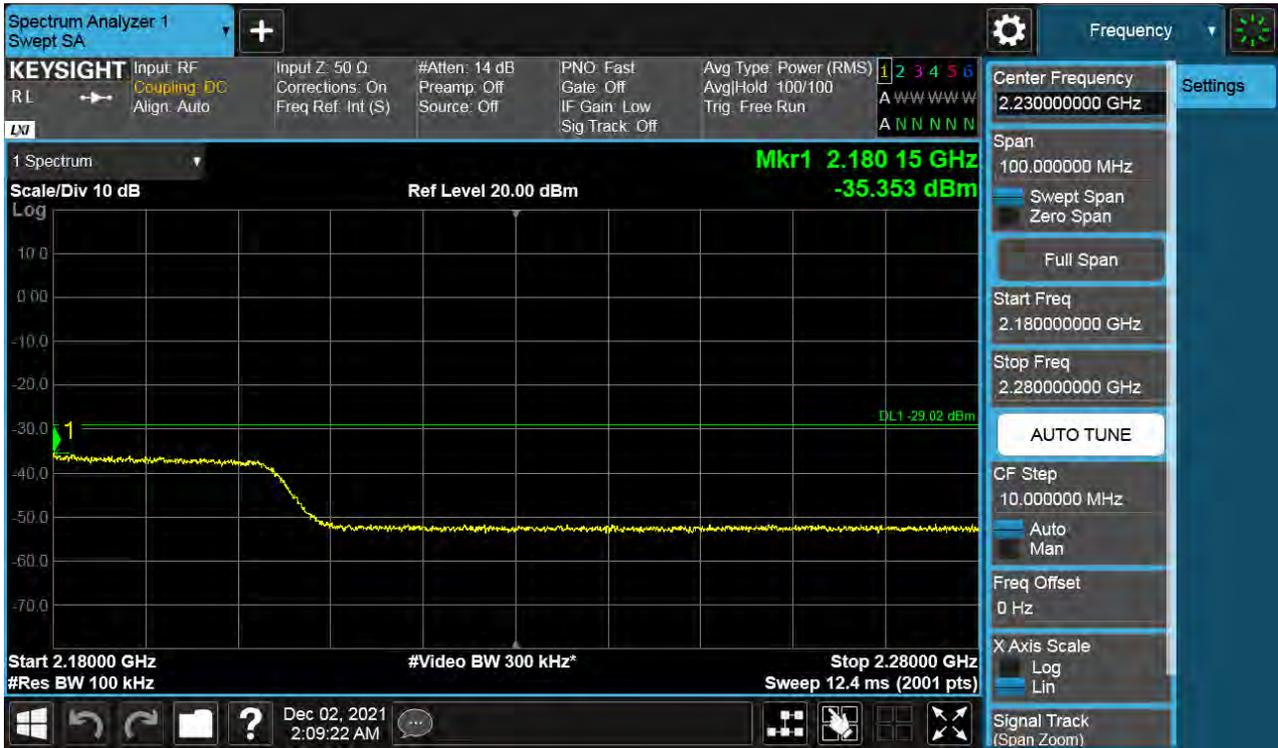
Antenna 0 / High Edge + 100 MHz ~ 10 GHz / (4 Port) B66 DSS 20 MHz 2to8 1 Carrier / 64QAM / High
