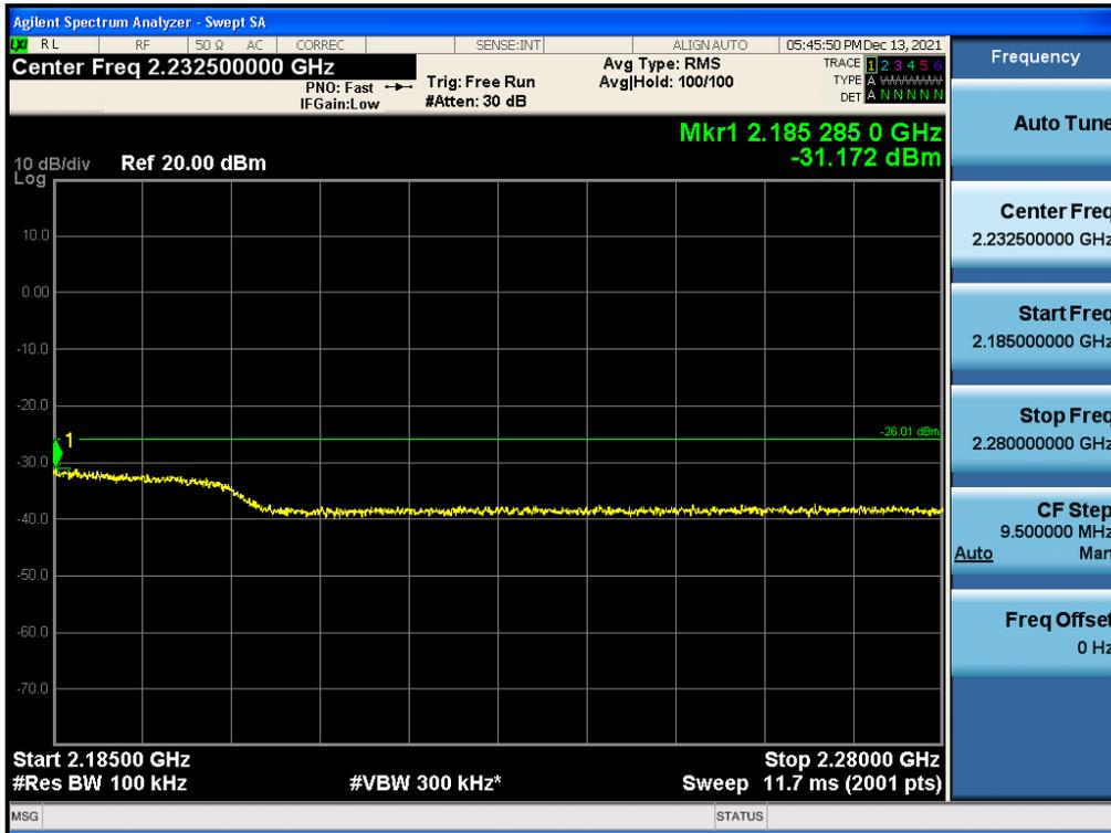
Antenna 1 / High Edge + 100 MHz ~ 10 GHz / (2 Port) LTE B66 5 MHz 1 Carrier / 16QAM / Middle
