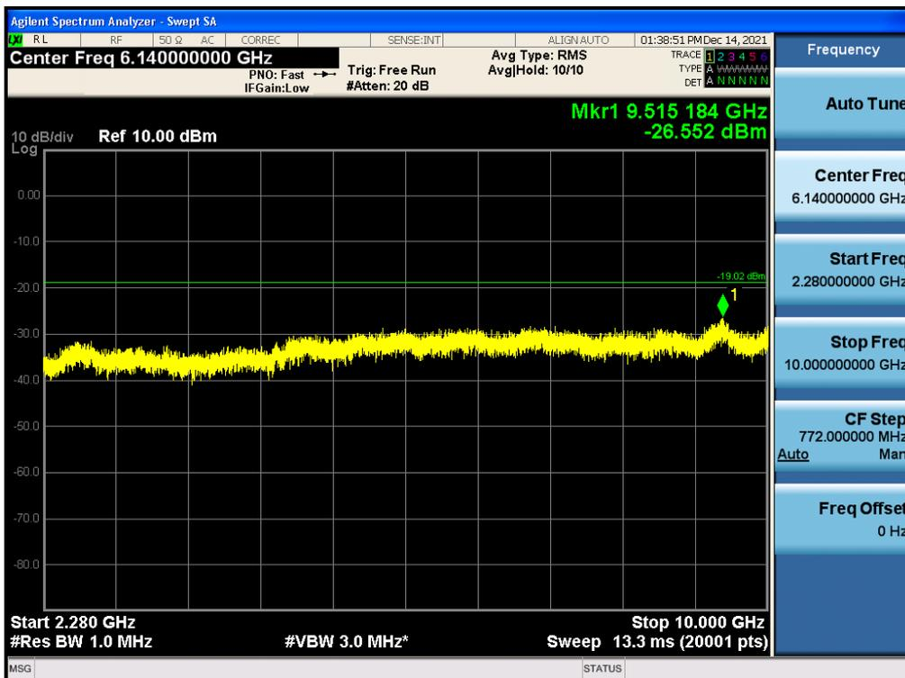
Antenna 0 / 10 GHz ~ 26.5 GHz / (4 Port) LTE B66 20 MHz 1 Carrier / 16QAM / High
