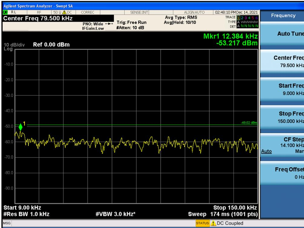
Antenna 3 / 150 kHz ~ 30 MHz / (4 Port) LTE B66 10 MHz 1 Carrier / 16QAM / Low
