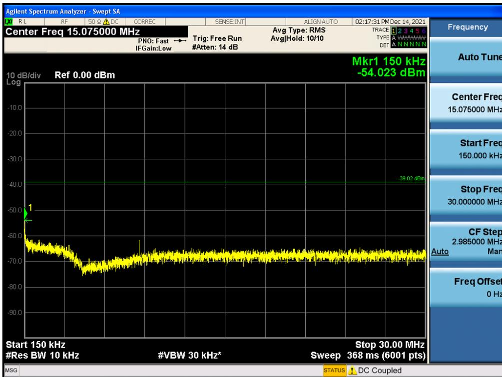
Antenna 0 / 30 MHz ~ Low Edge - 100 MHz / (4 Port) LTE B66 5 MHz 1 Carrier / QPSK / Middle
