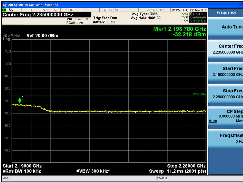
Antenna 1 / High Edge + 100 MHz ~ 10 GHz / (2 Port) LTE B66 10 MHz 1 Carrier / 16QAM / High
