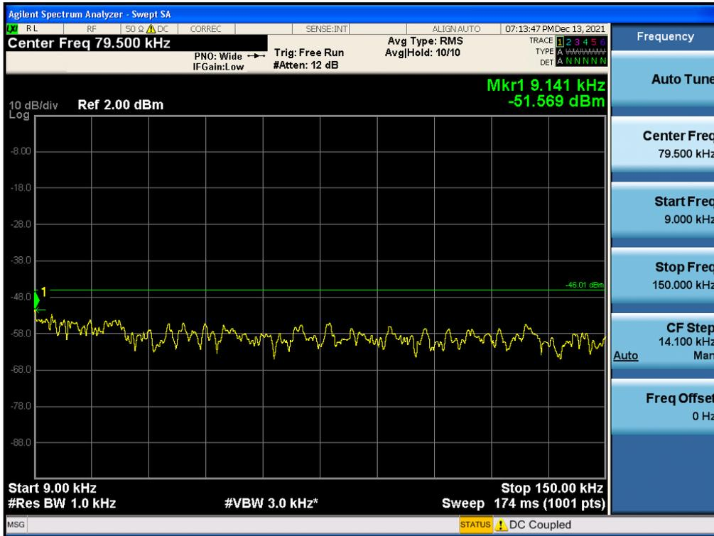
Antenna 1 / 150 kHz ~ 30 MHz / (2 Port) LTE B66 15 MHz 1 Carrier / QPSK / Middle
