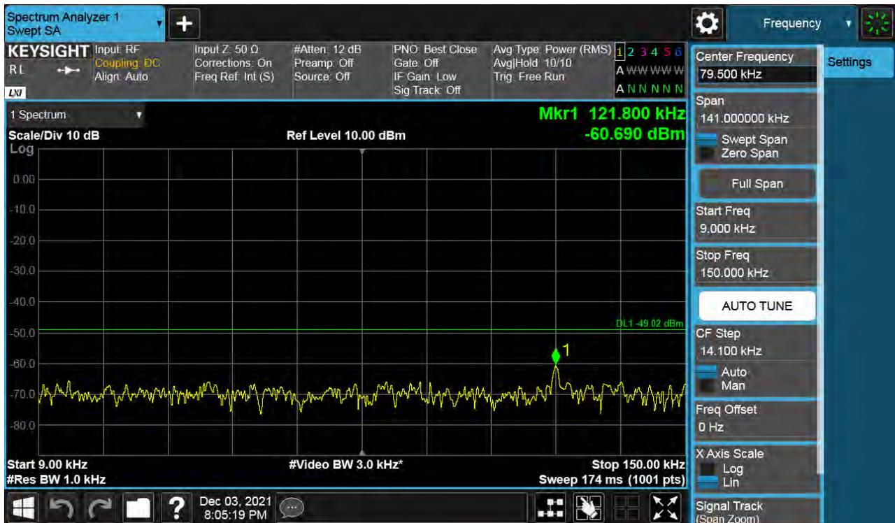
Antenna 1 / 150 kHz ~ 30 MHz / (2 Port) B66 DSS 10 MHz 2to8 1 Carrier / 16QAM / Low
