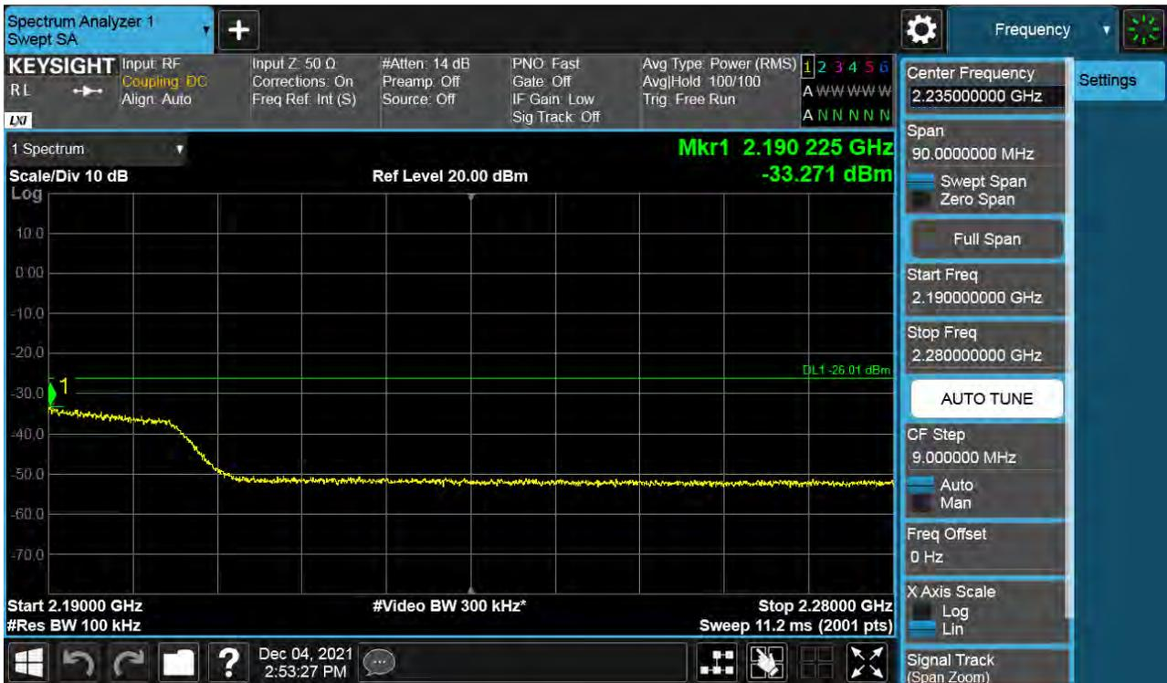
Antenna 0 / High Edge + 100 MHz ~ 10 GHz / (2 Port) B66 DSS 15 MHz 2to8 1 Carrier / 16QAM / High
