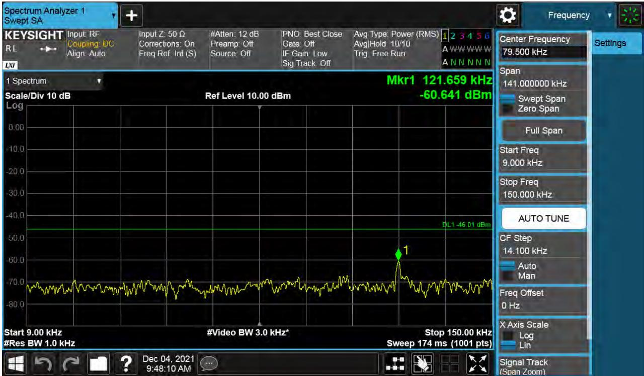
Antenna 1 / 150 kHz ~ 30 MHz / (2 Port) B66 DSS 15 MHz 9to1 1 Carrier / 64QAM / Middle
