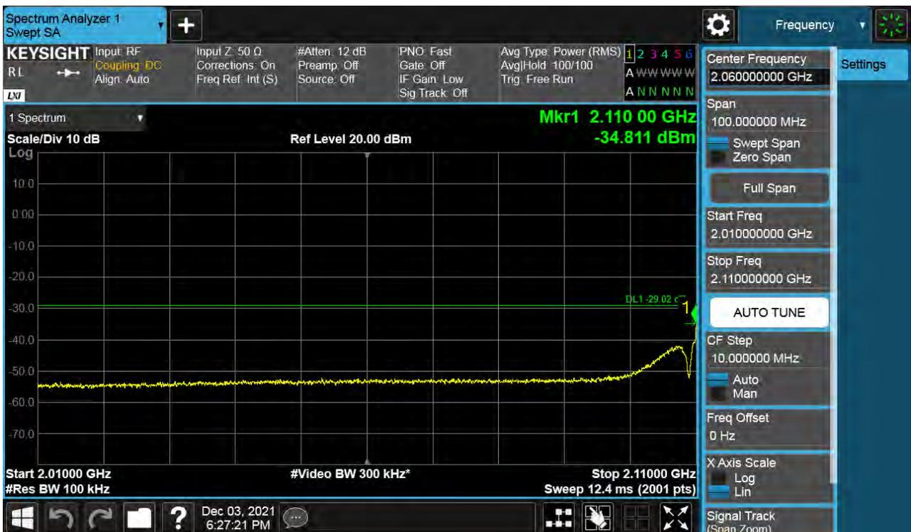
Antenna 1 / High Edge ~ High Edge + 100 MHz / (2 Port) B66 DSS 10 MHz 5to5 1 Carrier / QPSK / Middle
