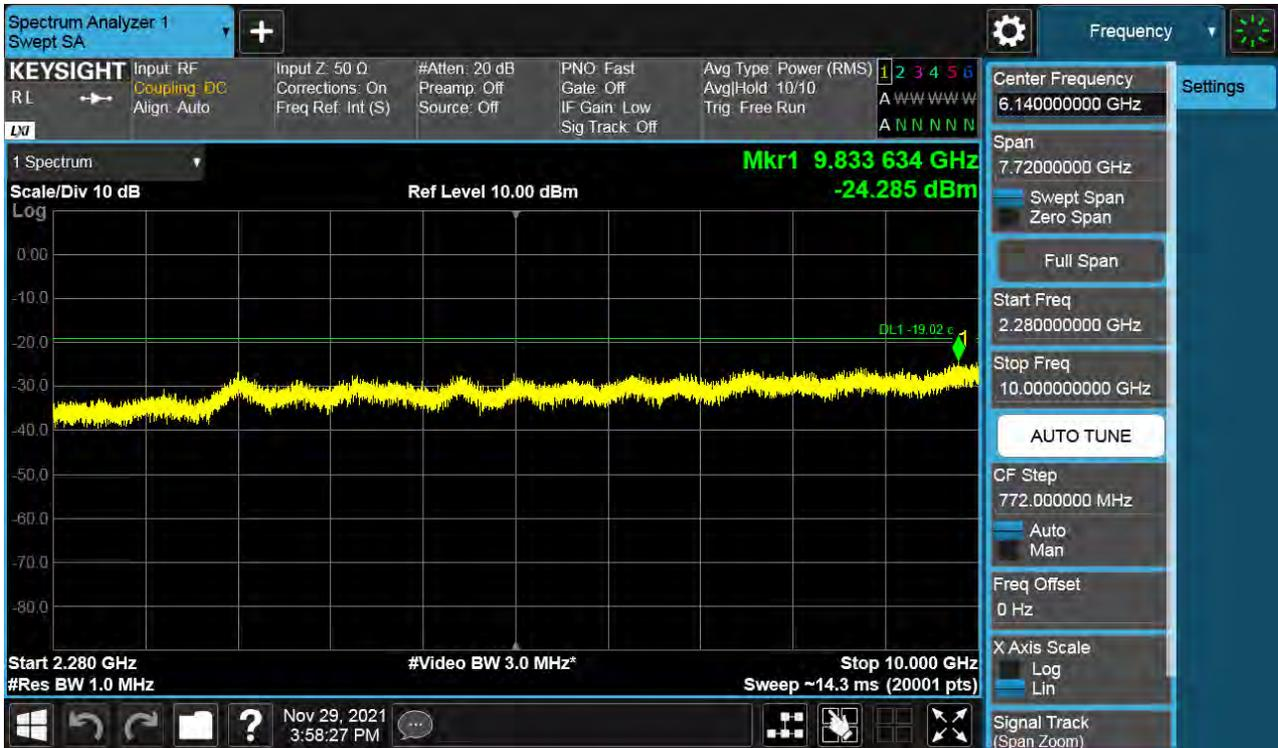
Antenna 1 / 10 GHz ~ 26.5 GHz / (4 Port) B66 DSS 10 MHz 9to1 1 Carrier / 64QAM / Middle
