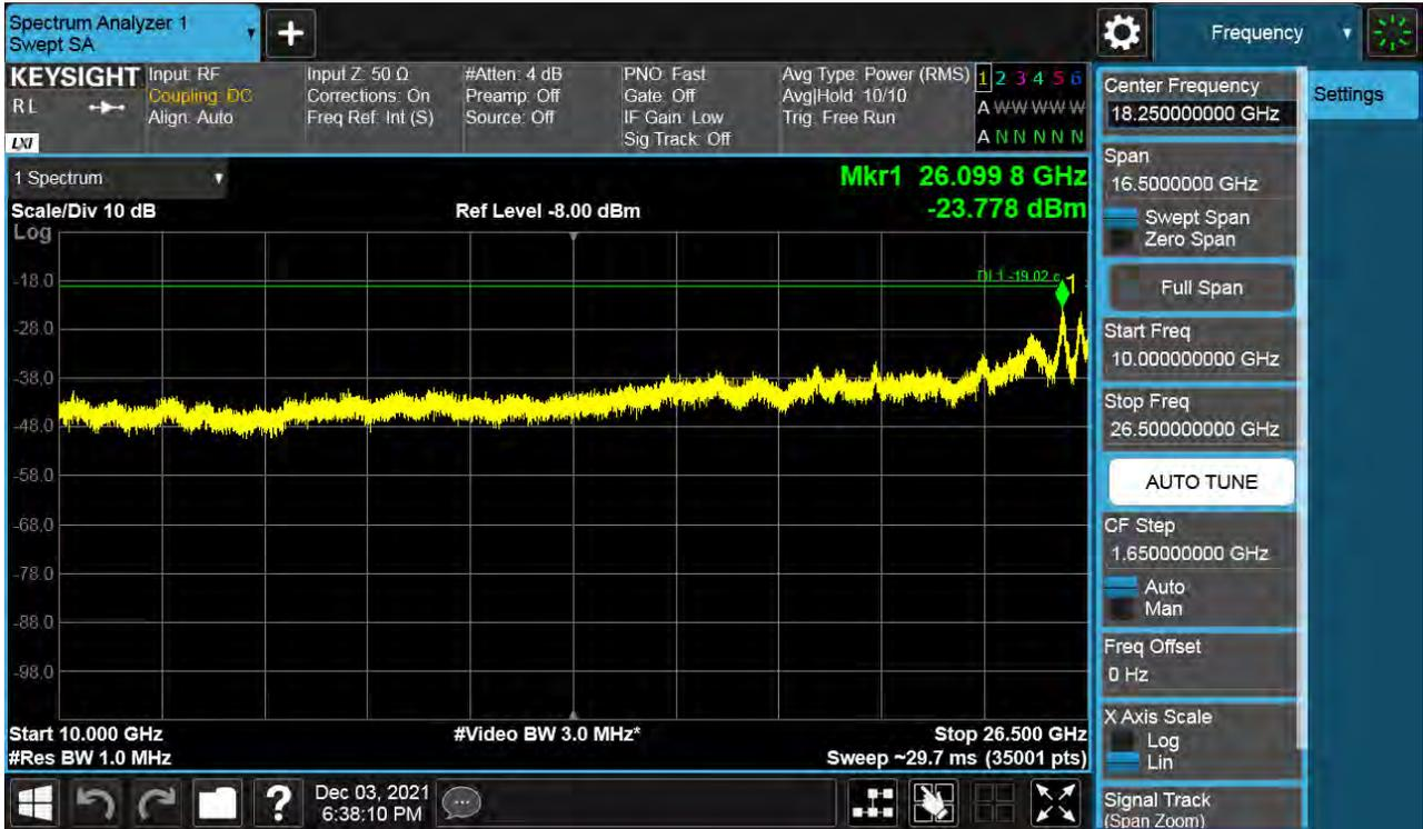
Antenna 1 / 9 kHz ~ 150 kHz / (2 Port) B66 DSS 10 MHz 9to1 1 Carrier / QPSK / Middle
