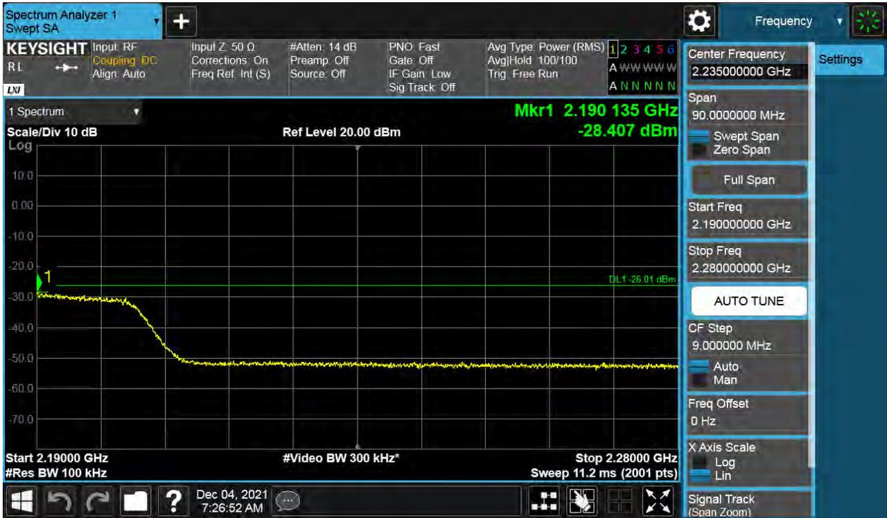
Antenna 0 / High Edge + 100 MHz ~ 10 GHz / (2 Port) B66 DSS 10 MHz 2to8 1 Carrier / QPSK / High
