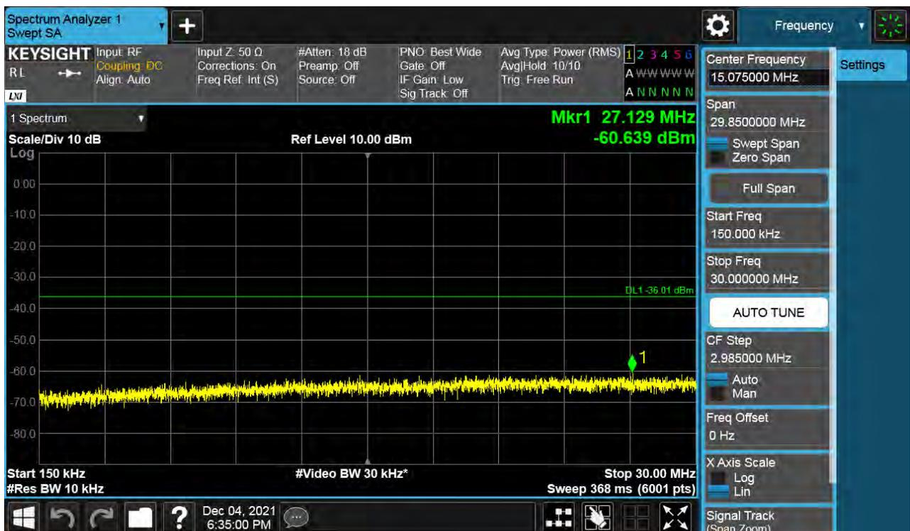
Antenna 0 / 30 MHz ~ Low Edge - 100 MHz / (2 Port) B66 DSS 20 MHz 5to5 1 Carrier / 64QAM / High
