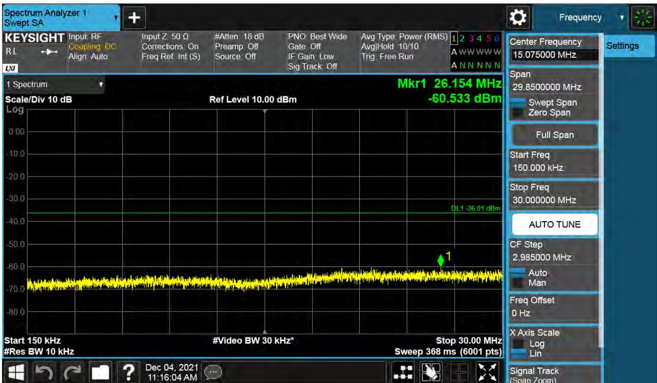
Antenna 0 / 30 MHz ~ Low Edge - 100 MHz / (2 Port) B66 DSS 15 MHz 5to5 1 Carrier / 256QAM / Low
