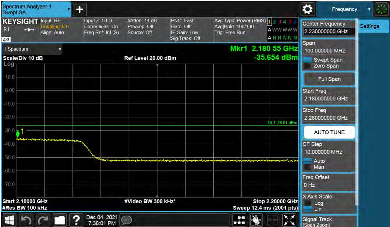
Antenna 0 / High Edge + 100 MHz ~ 10 GHz / (2 Port) B66 DSS 20 MHz 5to5 1 Carrier / 64QAM / High
