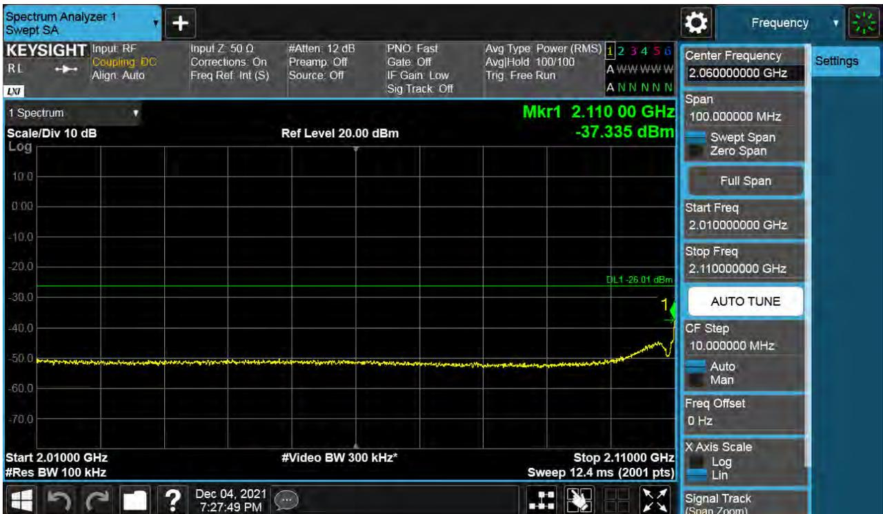
Antenna 0 / High Edge ~ High Edge + 100 MHz / (2 Port) B66 DSS 20 MHz 5to5 1 Carrier / 256QAM / Middle
