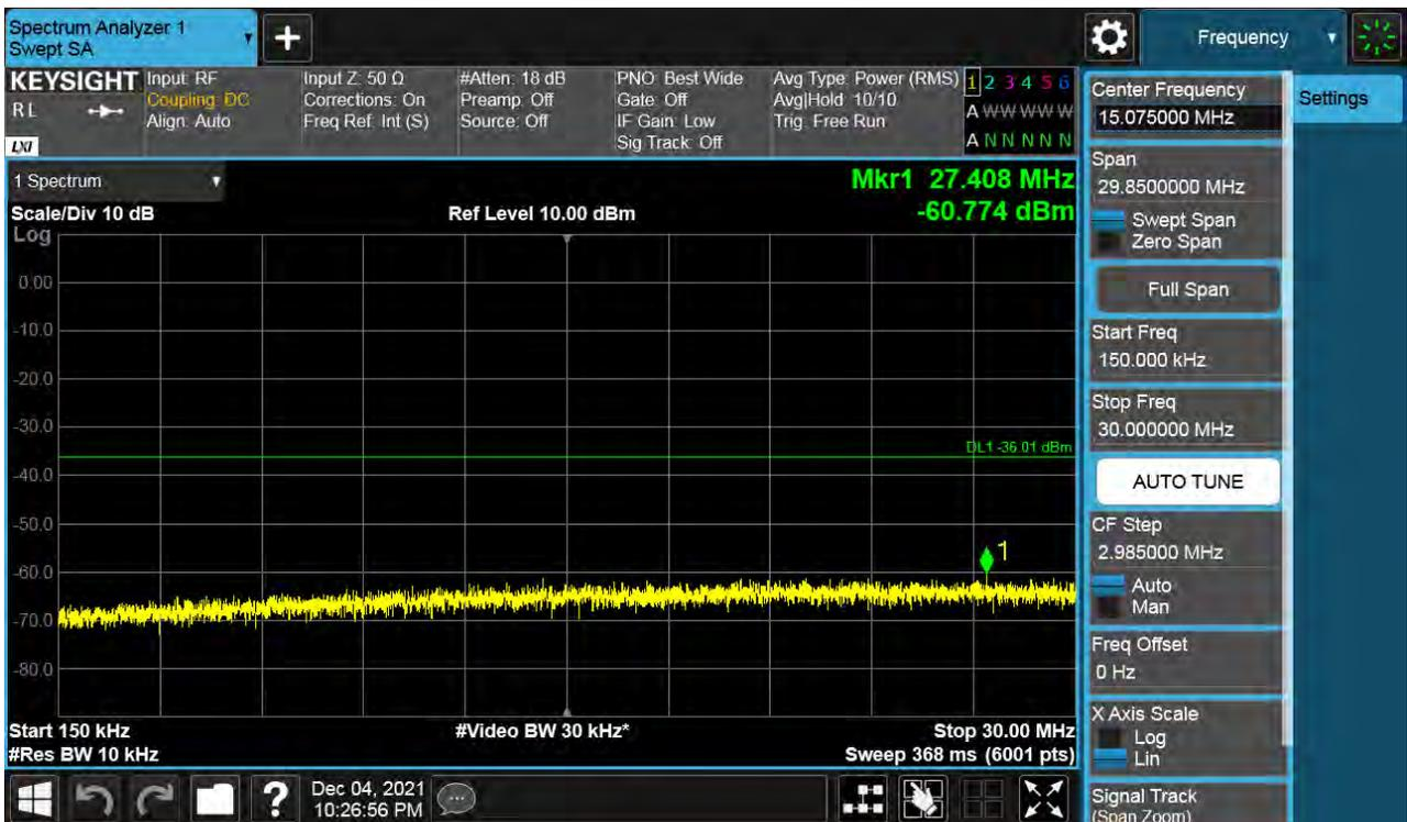
Antenna 0 / 30 MHz ~ Low Edge - 100 MHz / (2 Port) B66 DSS 20 MHz 2to8 1 Carrier / 64QAM / High
