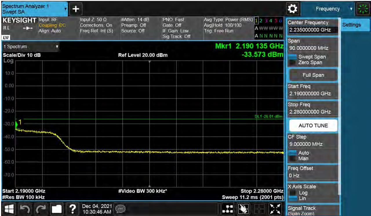
Antenna 0 / High Edge + 100 MHz ~ 10 GHz / (2 Port) B66 DSS 15 MHz 9to1 1 Carrier / QPSK / High
