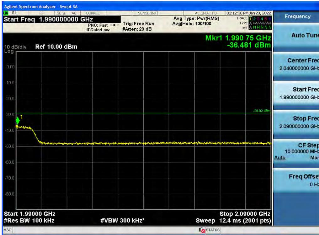
Antenna 2 / High Edge + 100 MHz ~ 10 GHz / (4 Port) 5G NR n2 15 MHz 1 Carrier / 64QAM / Middle
