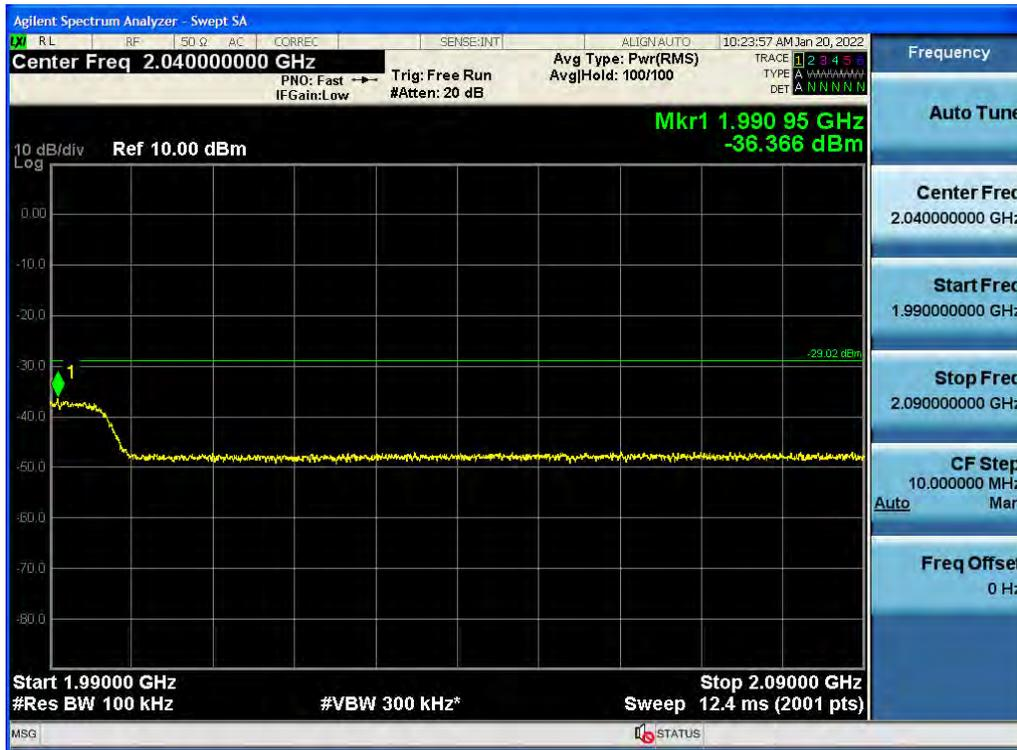
Antenna 2 / High Edge + 100 MHz ~ 10 GHz / (4 Port) 5G NR n2 20 MHz 1 Carrier / 64QAM / Low
