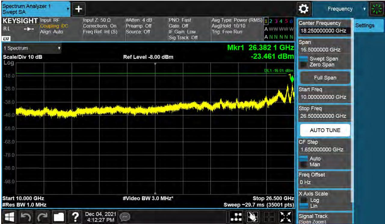
Antenna 3 / 9 kHz ~ 150 kHz / (4 Port) B66 DSS 10 MHz 2to8 1 Carrier / 256QAM / Middle
