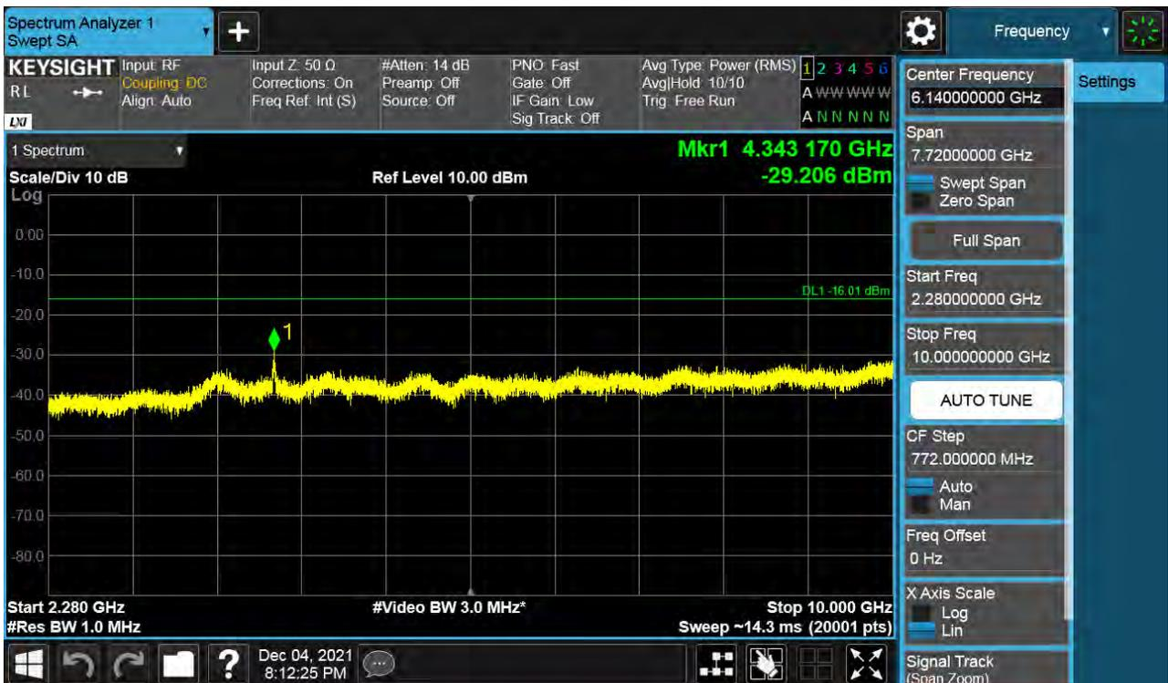
Antenna 1 / 10 GHz ~ 26.5 GHz / (2 Port) B66 DSS 20 MHz 5to5 1 Carrier / 64QAM / High
