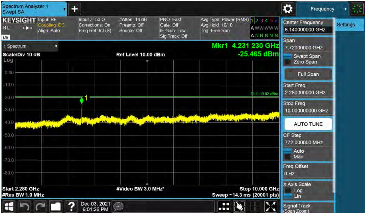
Antenna 1 / 10 GHz ~ 26.5 GHz / (2 Port) B66 DSS 10 MHz 5to5 1 Carrier / 16QAM / Middle
