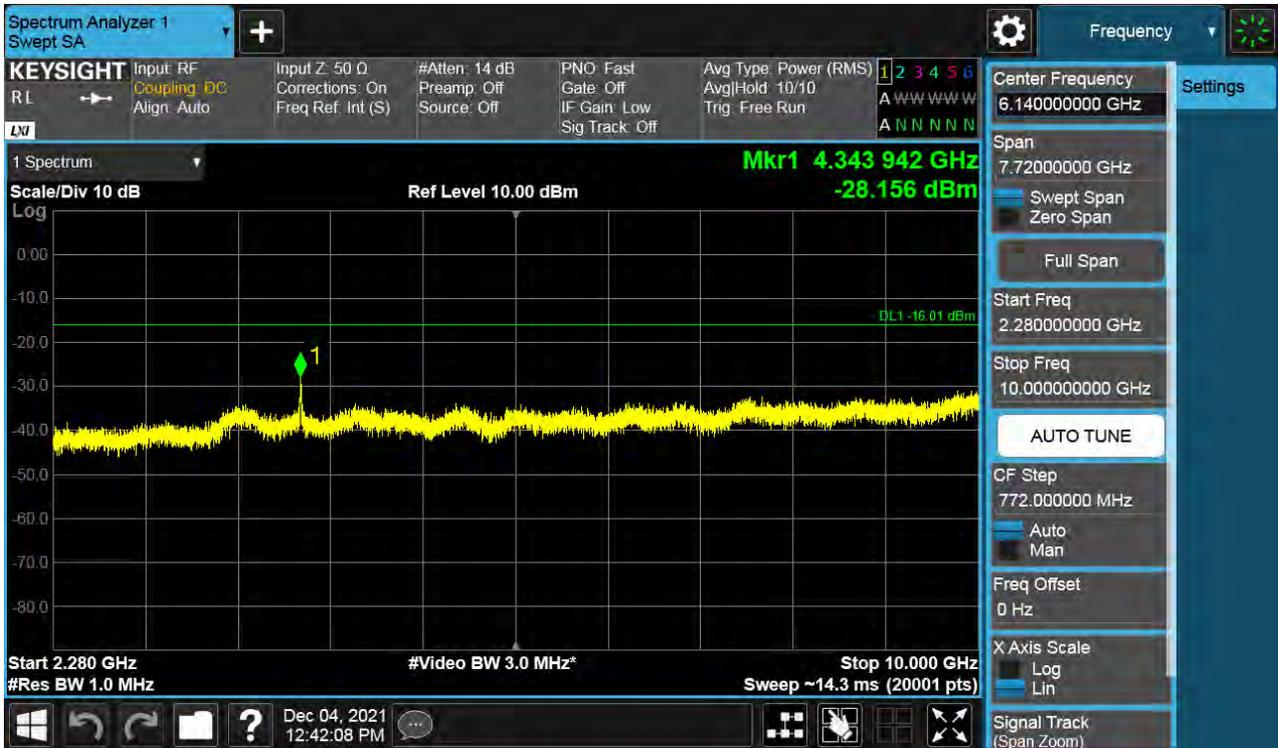
Antenna 1 / 10 GHz ~ 26.5 GHz / (2 Port) B66 DSS 15 MHz 5to5 1 Carrier / 16QAM / Low
