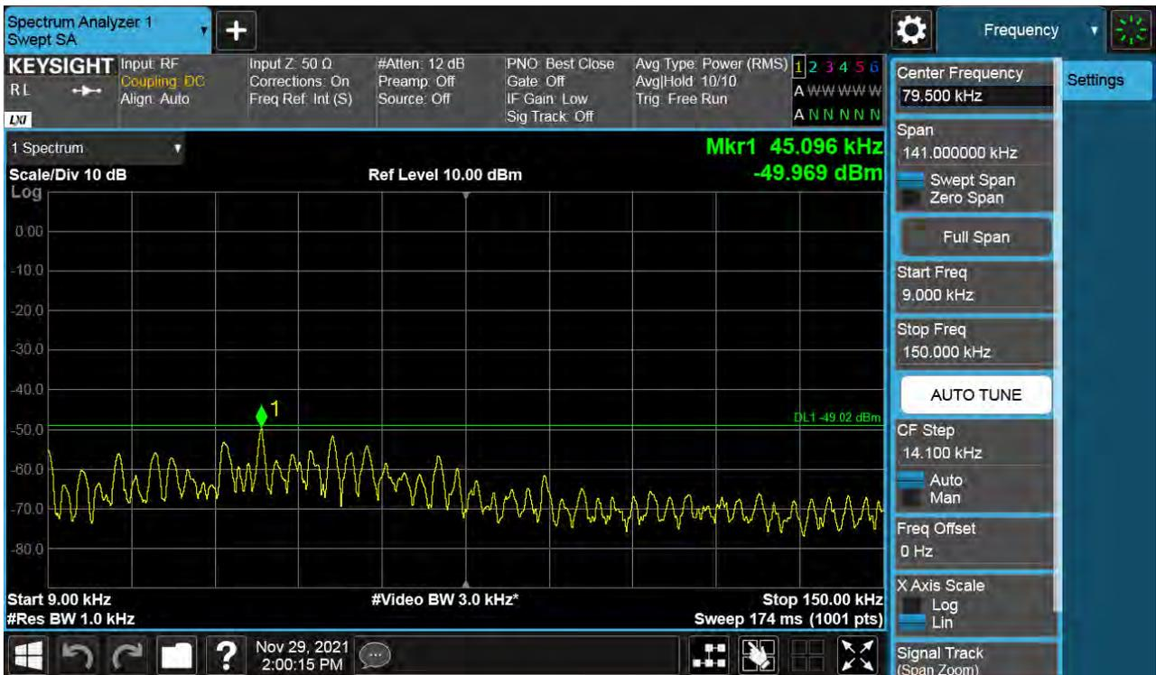
Antenna 3 / 150 kHz ~ 30 MHz / (4 Port) B66 DSS 10 MHz 5to5 1 Carrier / 64QAM / High
