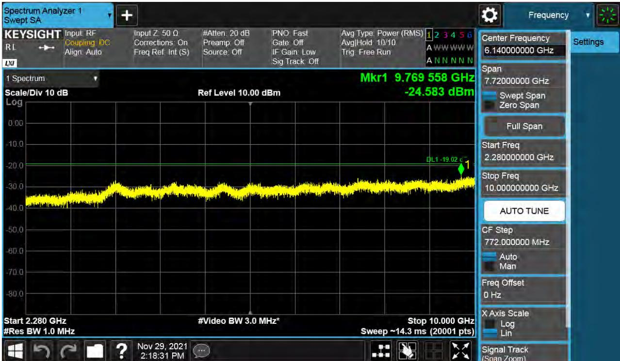
Antenna 1 / 10 GHz ~ 26.5 GHz / (4 Port) B66 DSS 10 MHz 5to5 1 Carrier / QPSK / Low
