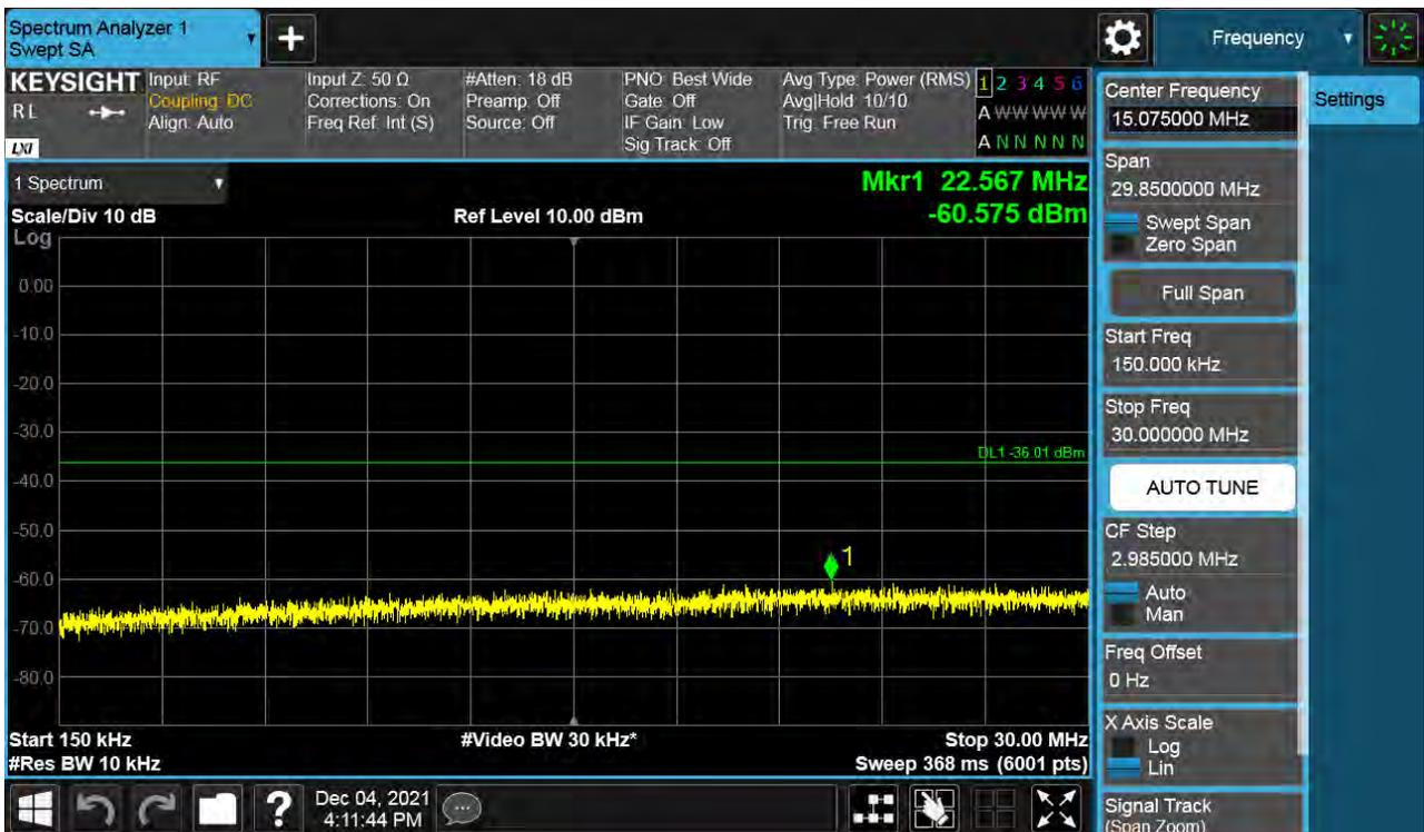
Antenna 0 / 30 MHz ~ Low Edge - 100 MHz / (2 Port) B66 DSS 20 MHz 9to1 1 Carrier / 256QAM / Middle
