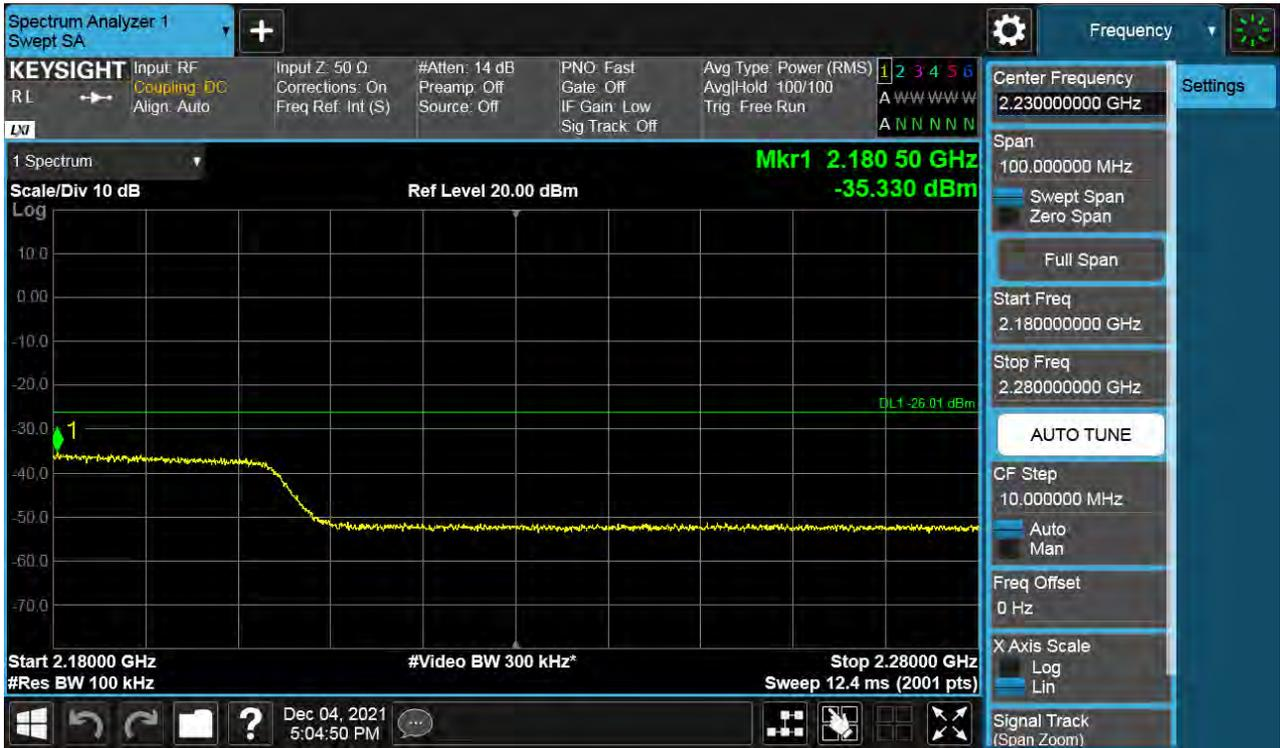
Antenna 0 / High Edge + 100 MHz ~ 10 GHz / (2 Port) B66 DSS 20 MHz 9to1 1 Carrier / QPSK / Middle
