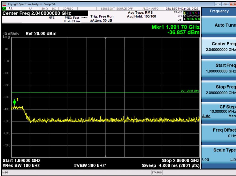
Antenna 0 / High Edge + 100 MHz ~ 10 GHz / (2 Port) 5G NR n2 10 MHz 1 Carrier / 16QAM / High
