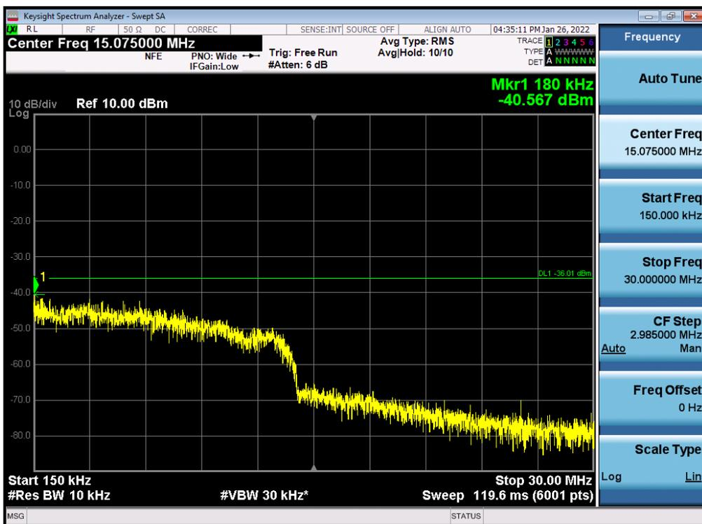
Antenna 0 / 30 MHz ~ Low Edge - 100 MHz / (2 Port) 5G NR n2 15 MHz 1 Carrier / QPSK / Middle
