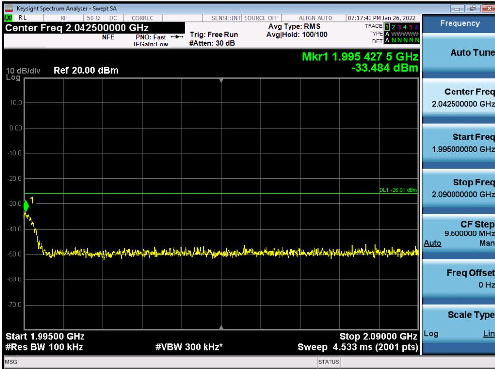
Antenna 0 / High Edge + 100 MHz ~ 10 GHz / (2 Port) 5G NR n2 5 MHz 1 Carrier / QPSK / High
