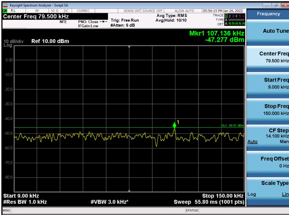
Antenna 0 / 150 kHz ~ 30 MHz / (2 Port) 5G NR n2 10 MHz 1 Carrier / 16QAM / High
