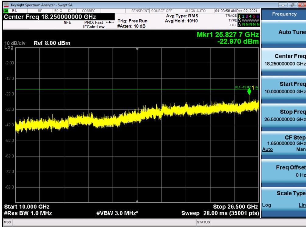
Antenna 0 / 9 kHz ~ 150 kHz / (4 Port) B2 DSS 20 MHz 9to1 1 Carrier / 64QAM / Low
