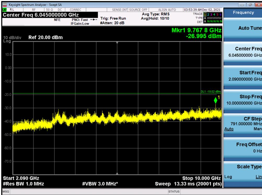
Antenna 0 / 10 GHz ~ 26.5 GHz / (4 Port) B2 DSS 20 MHz 5to5 1 Carrier / QPSK / Middle
