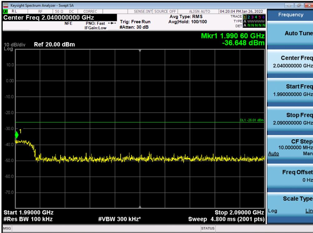
Antenna 0 / High Edge + 100 MHz ~ 10 GHz / (2 Port) 5G NR n2 15 MHz 1 Carrier / QPSK / High
