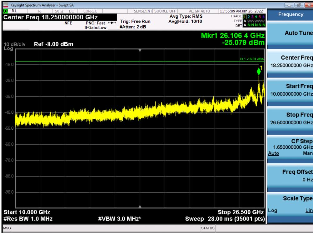
Antenna 3 / 9 kHz ~ 150 kHz / (4 Port) 5G NR n2 5 MHz 1 Carrier / 16QAM / Low
