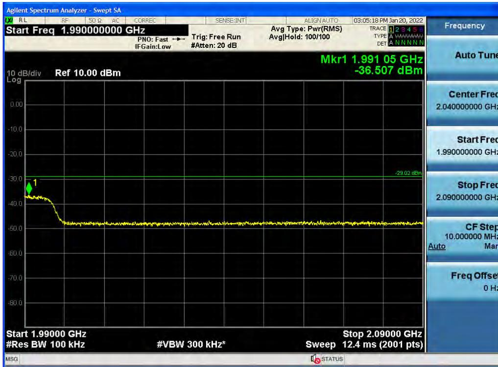
Antenna 1 / High Edge + 100 MHz ~ 10 GHz / (4 Port) 5G NR n2 10 MHz 1 Carrier / QPSK / High
