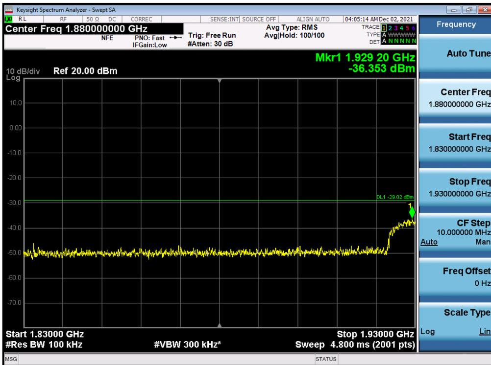
Antenna 0 / High Edge ~ High Edge + 100 MHz / (4 Port) B2 DSS 20 MHz 5to5 1 Carrier / 16QAM / Middle
