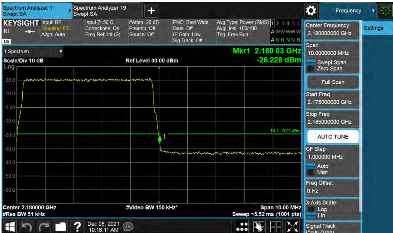
Antenna 0 / (2 Port) LTE B66 5 MHz 1 Carrier + LTE B66 5 MHz 1 Carrier + LTE B66 5 MHz 1 Carrier + 5G NR n66 5 MHz 1 Carrier [4 Carrier] (1C+3C) / Non-Contiguous / 64QAM / Low
