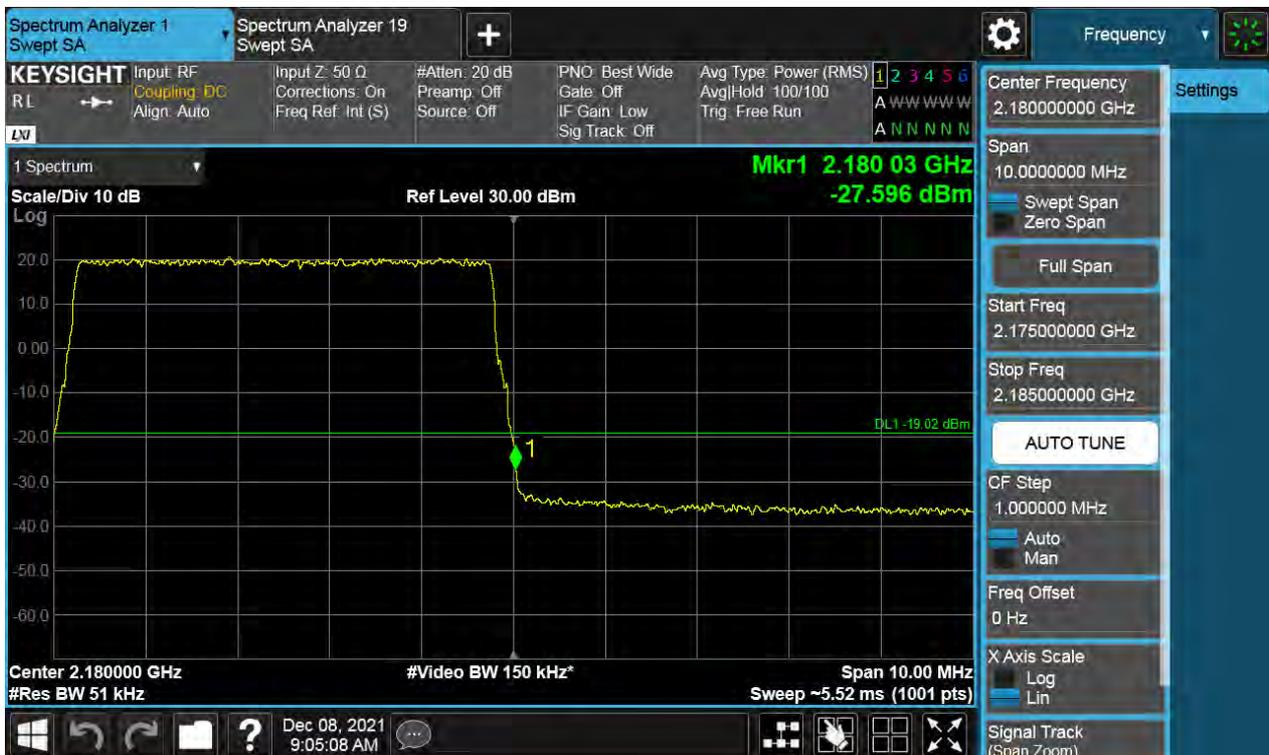
Antenna 0 / (4 Port) B66 DSS 20 MHz 9to1 1 Carrier + LTE B66 10 MHz 1 Carrier + LTE B66 5 MHz 1 Carrier + LTE B66 5 MHz 1 Carrier [4 Carrier] (3C+1C) / Non-Contiguous / 64QAM / Low
