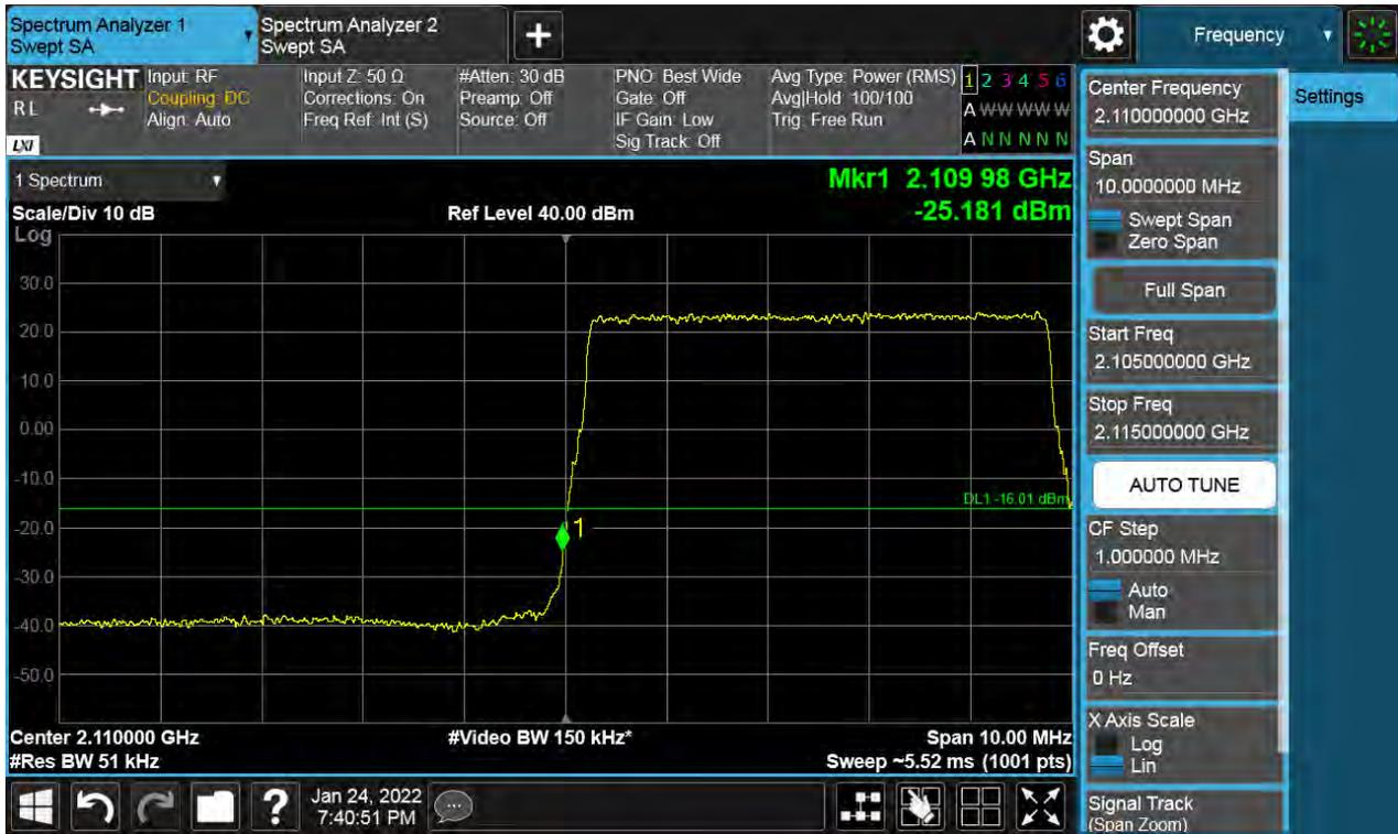
Antenna 1 / (2 Port) LTE B66 5 MHz 1 Carrier + LTE B66 5 MHz 1 Carrier + LTE B66 5 MHz 1 Carrier + 5G NR n66 5 MHz 1 Carrier [4 Carrier] (3C+1C) / Non-Contiguous / QPSK / High
