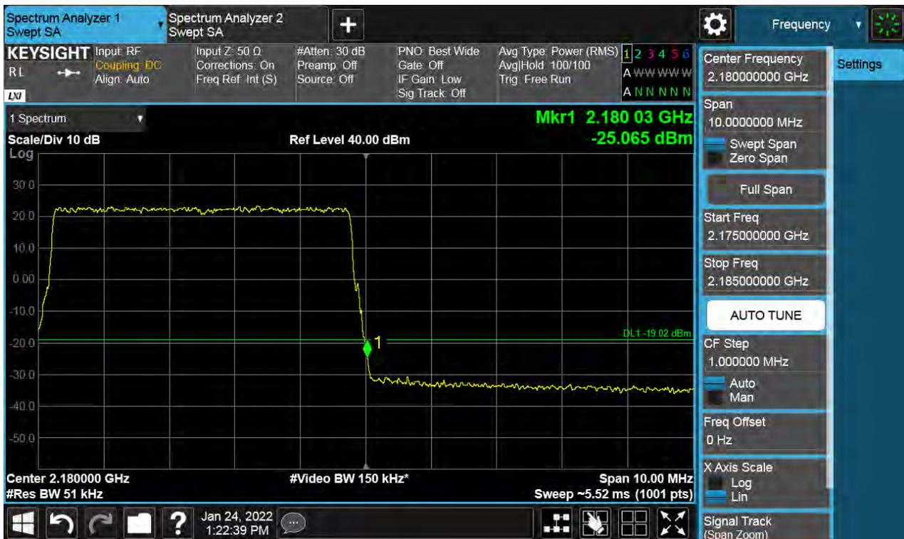
**Antenna 0 / (4 Port) LTE B66 5 MHz 1 Carrier + LTE B66 5 MHz 1 Carrier + LTE B66 5 MHz 1 Carrier + 5G NR n66 5 MHz 1 Carrier [4 Carrier] (3C+1C) / Non-Contiguous / 256QAM / Low**
