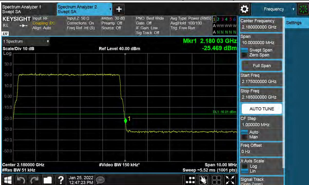
Antenna 0 / (2 Port) LTE B66 5 MHz 1 Carrier + LTE B66 5 MHz 1 Carrier + LTE B66 10 MHz 1 Carrier + 5G NR n66 20 MHz 1 Carrier [4 Carrier] (3C+1C) / Non-Contiguous / 256QAM / Low
