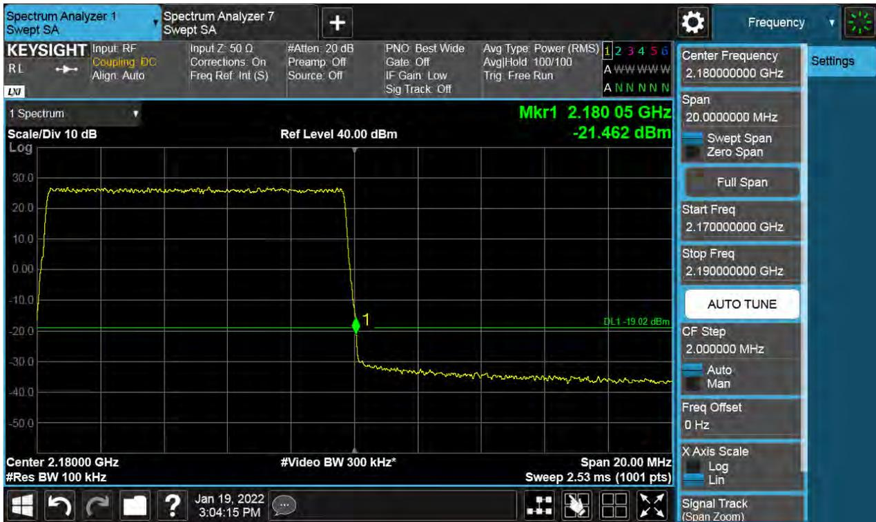
Antenna 3 / (4 Port) LTE B66 20 MHz 1 Carrier + 5G NR n66 20 MHz 1 Carrier [2 Carrier] / Non-Contiguous / QPSK / Low
