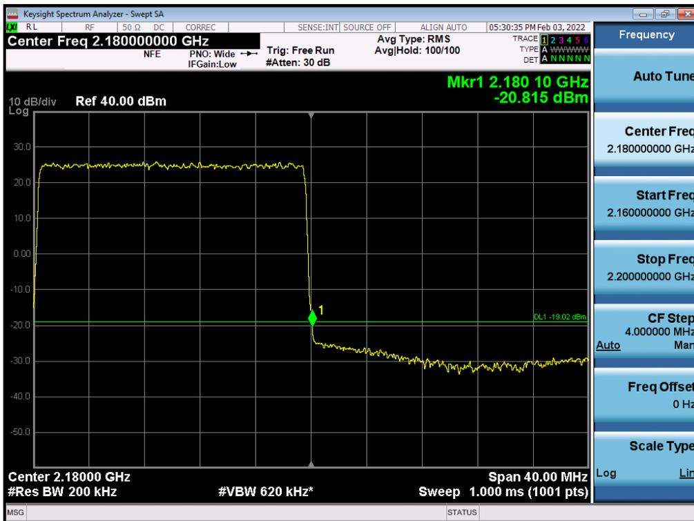
Antenna 1 / (2 Port) B2 DSS 20 MHz 9to1 1 Carrier + LTE B2 5 MHz 1 Carrier + LTE B2 5 MHz 1 Carrier [3 Carrier] (1C+2C) / Non-Contiguous / 256QAM / Low
