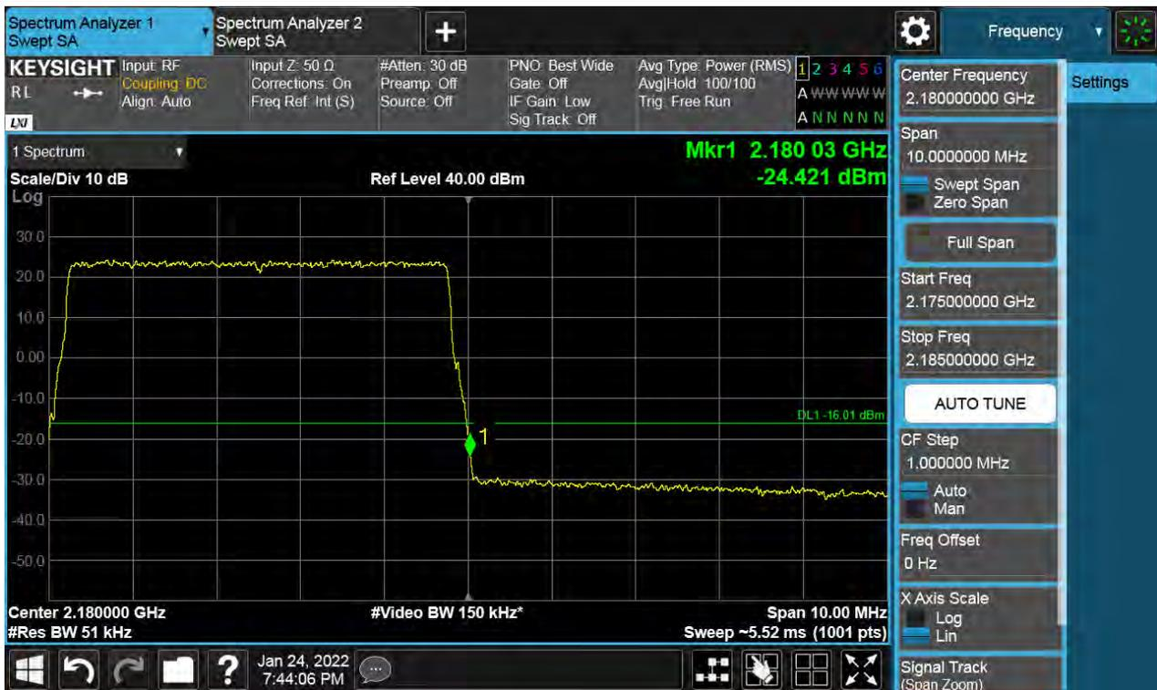
**Antenna 0 / (2 Port) LTE B66 5 MHz 1 Carrier + LTE B66 5 MHz 1 Carrier + LTE B66 10 MHz 1 Carrier + 5G NR n66 20 MHz 1 Carrier [4 Carrier] (1C+3C) / Non-Contiguous / QPSK / Low**
