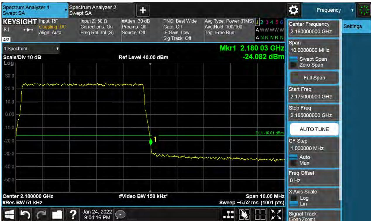
Antenna 0 / (2 Port) LTE B66 5 MHz 1 Carrier + LTE B66 5 MHz 1 Carrier + LTE B66 5 MHz 1 Carrier + 5G NR n66 5 MHz 1 Carrier [4 Carrier] (3C+1C) / Non-Contiguous / QPSK / Low
