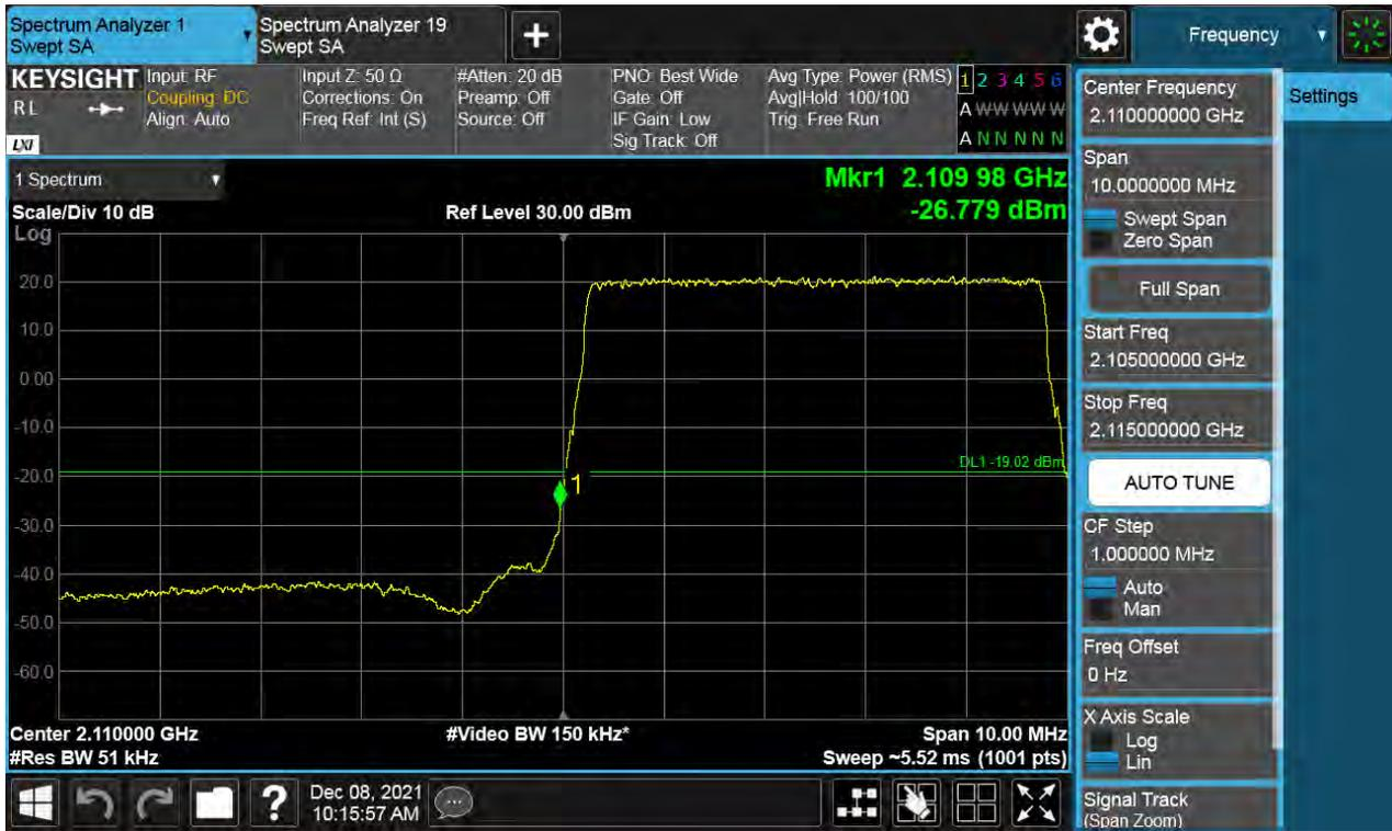
Antenna 0 / (4 Port) B66 DSS 20 MHz 9to1 1 Carrier + LTE B66 10 MHz 1 Carrier + LTE B66 5 MHz 1 Carrier + LTE B66 5 MHz 1 Carrier [4 Carrier] (3C+1C) / Non-Contiguous / 64QAM / High
