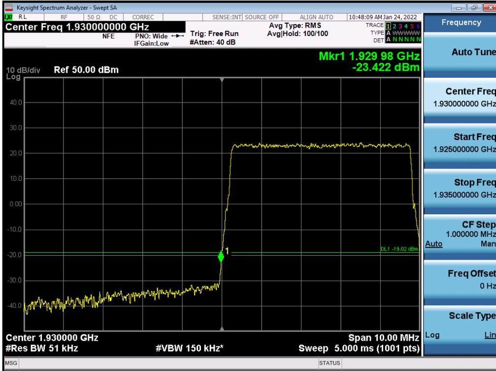
Antenna 0 / (4 Port) LTE B2 5 MHz 1 Carrier + 5G NR n2 5 MHz 1 Carrier [2 Carrier] / Non-Contiguous / 16QAM / High
