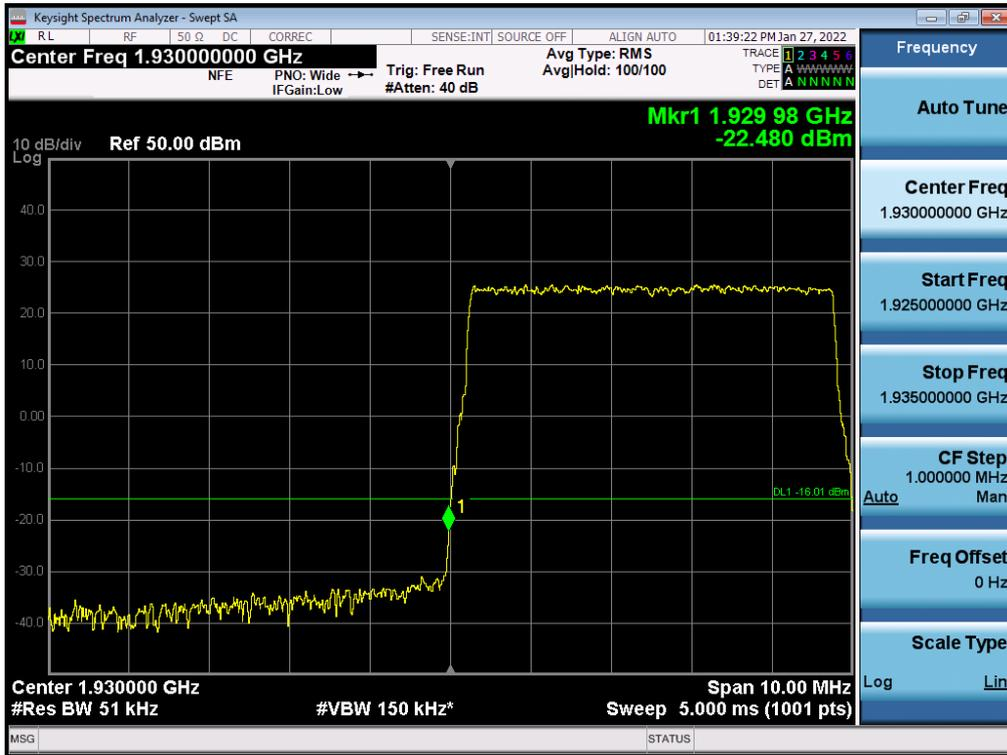
Antenna 0 / (2 Port) LTE B2 5 MHz 1 Carrier + 5G NR n2 5 MHz 1 Carrier [2 Carrier] / Non-Contiguous / 16QAM / High
