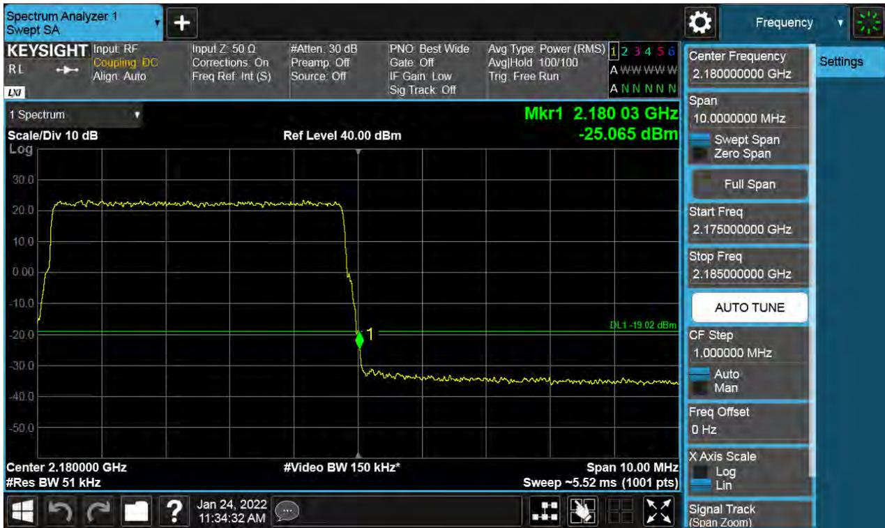
Antenna 0 / (4 Port) LTE B66 5 MHz 1 Carrier + LTE B66 5 MHz 1 Carrier + LTE B66 10 MHz 1 Carrier + 5G NR n66 20 MHz 1 Carrier [4 Carrier] / Contiguous / 256QAM / Low
