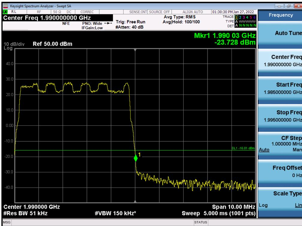
Antenna 1 / (2 Port) LTE B2 10 MHz 1 Carrier + 5G NR n2 20 MHz 1 Carrier [2 Carrier] / Non-Contiguous / QPSK / Low
