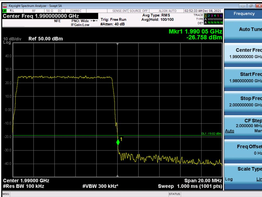
Antenna 1 / (2 Port) LTE B2 5 MHz 1 Carrier + 5G NR n2 5 MHz 1 Carrier [2 Carrier] / Non-Contiguous / 64QAM / Low
