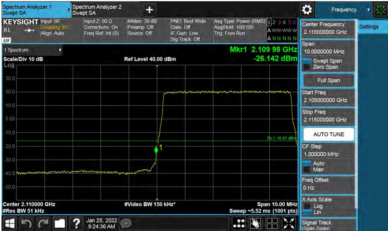
Antenna 1 / (2 Port) LTE B66 5 MHz 1 Carrier + LTE B66 5 MHz 1 Carrier + LTE B66 10 MHz 1 Carrier + 5G NR n66 20 MHz 1 Carrier [4 Carrier] / Contiguous / 256QAM / High
