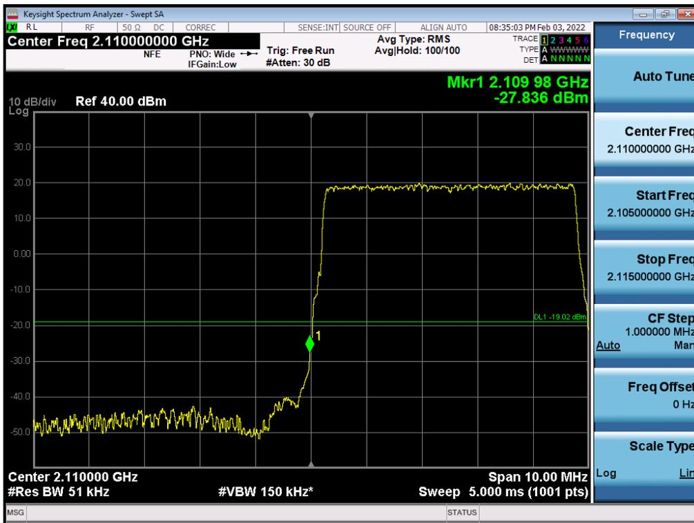
Antenna 3 / (4 Port) LTE B66 5 MHz 1 Carrier + LTE B66 5 MHz 1 Carrier + LTE B66 10 MHz 1 Carrier + 5G NR n66 20 MHz 1 Carrier [4 Carrier] / Contiguous / 64QAM / High
