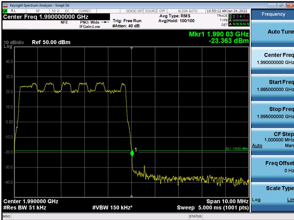
Antenna 3 / (4 Port) LTE B2 10 MHz 1 Carrier + 5G NR n2 20 MHz 1 Carrier [2 Carrier] / Non-Contiguous / 64QAM / Low
