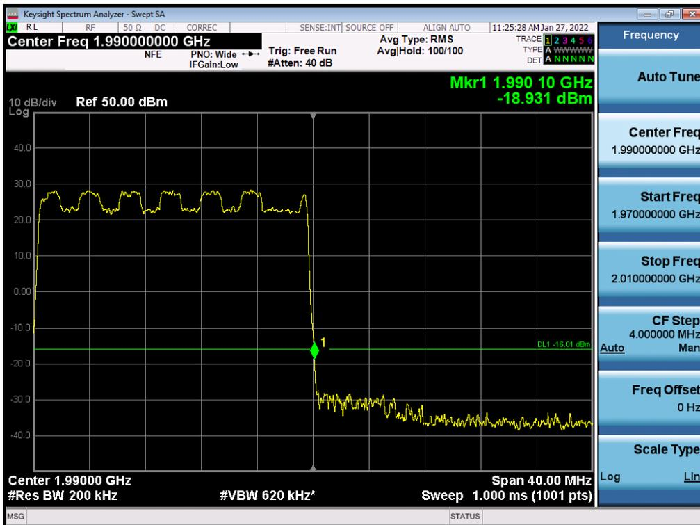
Antenna 2 / (4 Port) LTE B2 5 MHz 1 Carrier + 5G NR n2 5 MHz 1 Carrier [2 Carrier] / Non-Contiguous / QPSK / Low
