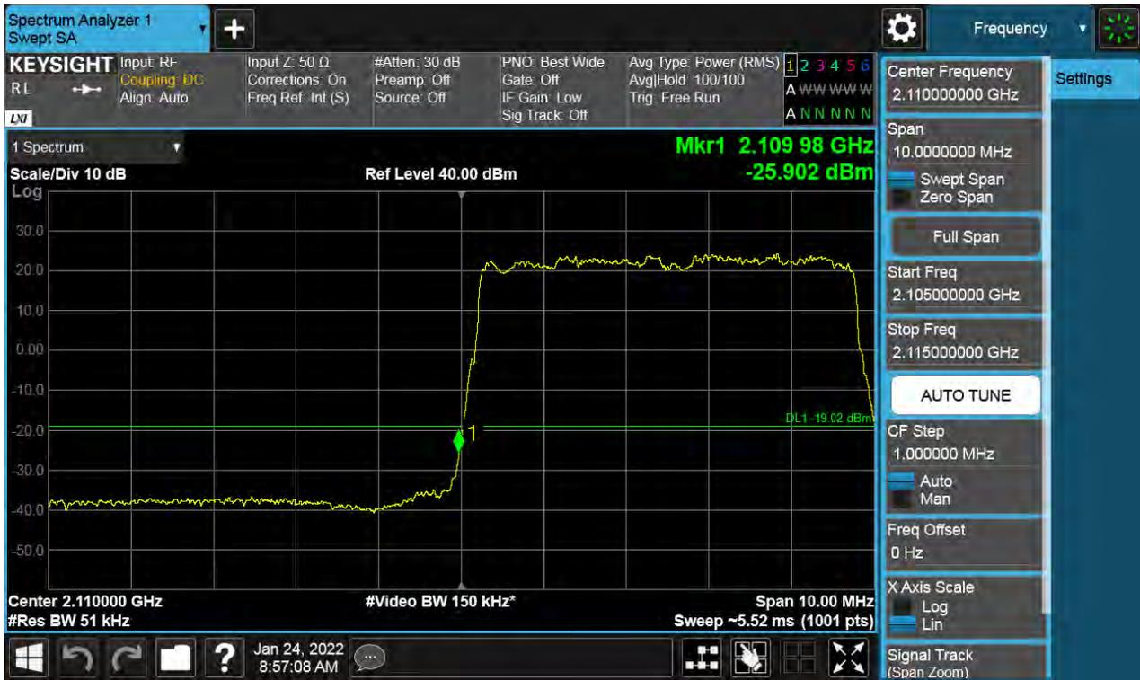
Antenna 0 / (4 Port) LTE B66 5 MHz 1 Carrier + LTE B66 5 MHz 1 Carrier + LTE B66 5 MHz 1 Carrier + 5G NR n66 5 MHz 1 Carrier [4 Carrier] / Contiguous / 256QAM / High
