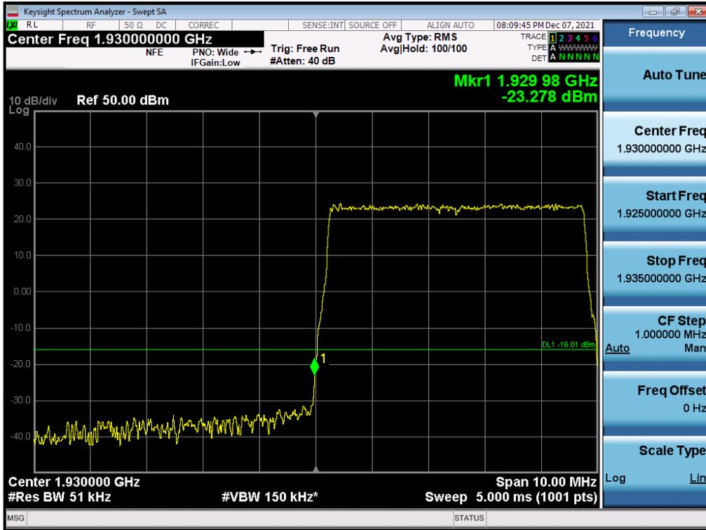
Antenna 1 / (2 Port) B2 DSS 10 MHz 9to1 1 Carrier + LTE B2 5 MHz 1 Carrier [2 Carrier] / Non-Contiguous / 64QAM / High
