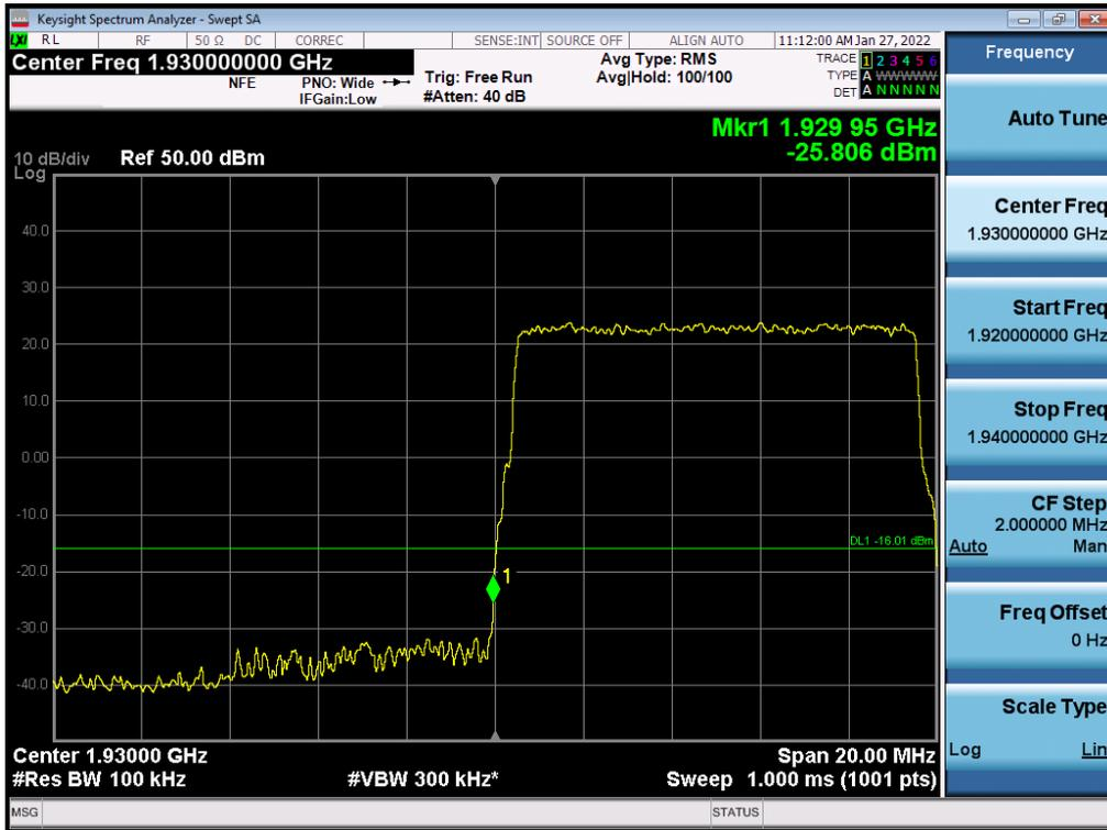
Antenna 1 / (2 Port) LTE B2 10 MHz 1 Carrier + 5G NR n2 20 MHz 1 Carrier [2 Carrier] / Non-Contiguous / 16QAM / High
