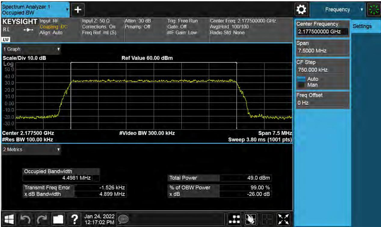
Antenna 1 / (4 Port) LTE B66 5 MHz 1 Carrier + LTE B66 5 MHz 1 Carrier + LTE B66 10 MHz 1 Carrier + 5G NR n66 20 MHz 1 Carrier [4 Carrier] (1C+3C) / Non-Contiguous / LTE B66 5 MHz / 256QAM / Low
