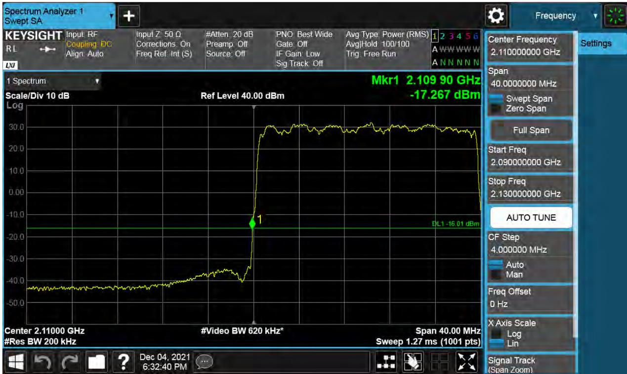
Antenna 1 / (2 Port) B66 DSS 20 MHz 5to5 1 Carrier / 256QAM / High
