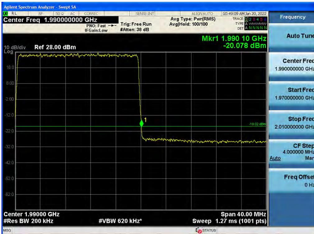
Antenna 1 / (2 Port) B66 DSS 10 MHz 2to8 1 Carrier / 256QAM / Low
