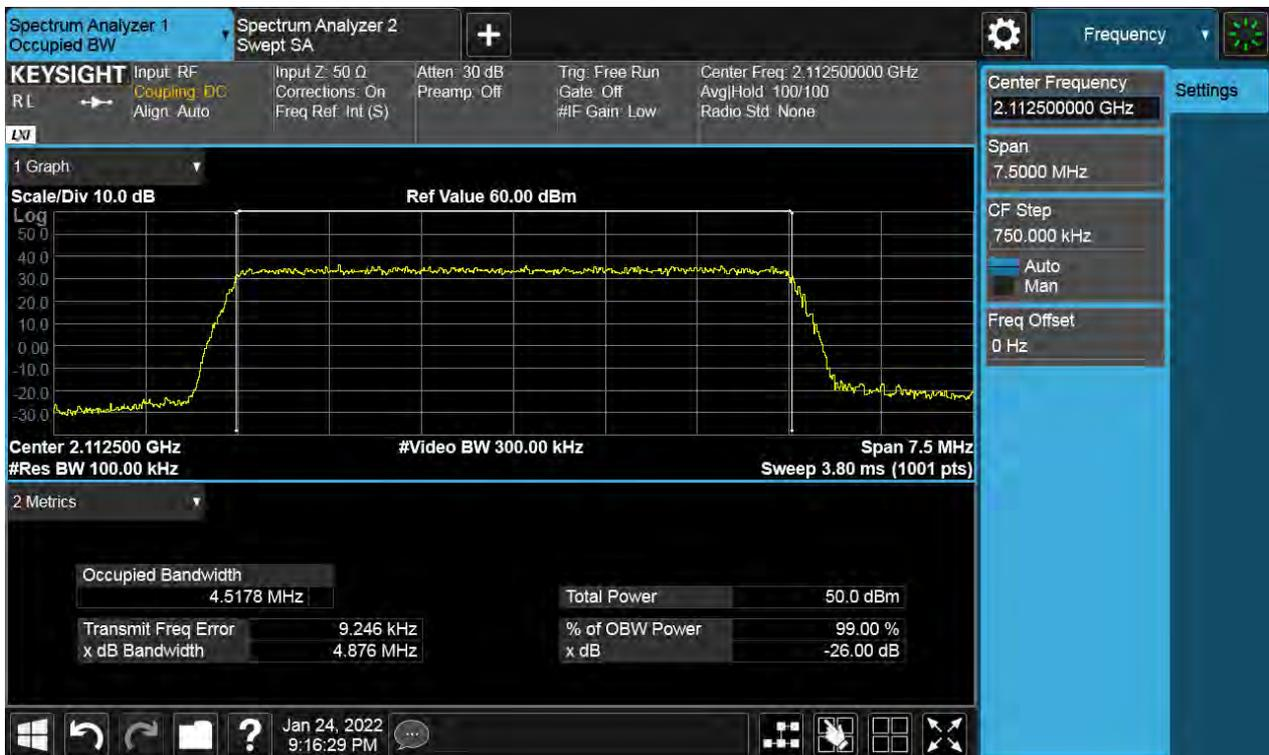
**Antenna 1 / (2 Port) LTE B66 5 MHz 1 Carrier + LTE B66 5 MHz 1 Carrier + LTE B66 5 MHz 1 Carrier + 5G NR n66 5 MHz 1 Carrier [4 Carrier] (1C+3C) / Non-Contiguous / LTE B66 5 MHz + LTE B66 5 MHz + 5G NR n66 5 MHz / 256QAM / High**
