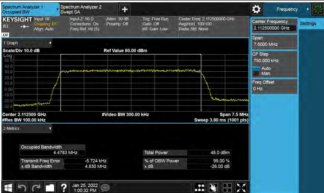
**Antenna 1 / (2 Port) LTE B66 5 MHz 1 Carrier + LTE B66 5 MHz 1 Carrier + LTE B66 10 MHz 1 Carrier + 5G NR n66 20 MHz 1 Carrier [4 Carrier] (1C+3C) / Non-Contiguous / LTE B66 5 MHz + LTE B66 10 MHz + 5G NR n66 20 MHz / 16QAM / High**
