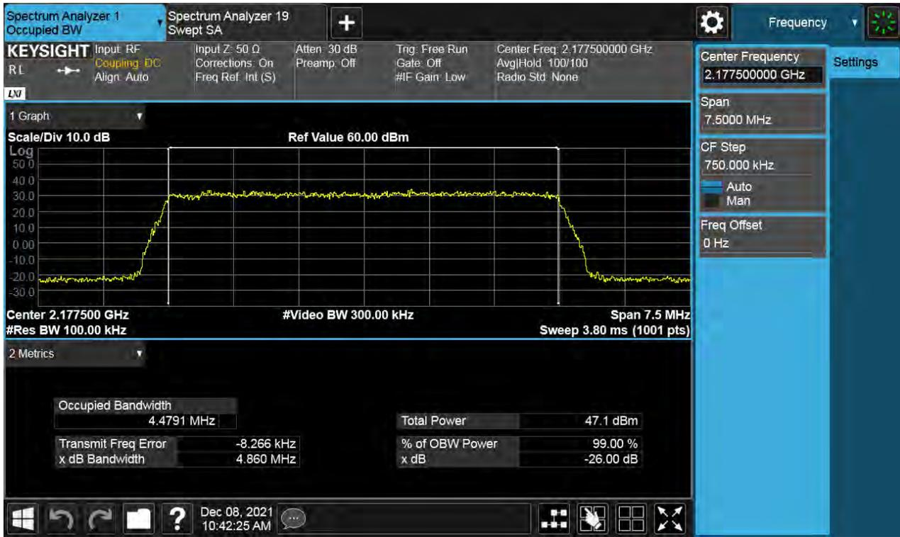
**Antenna 1 / (2 Port) LTE B66 5 MHz 1 Carrier + LTE B66 5 MHz 1 Carrier + LTE B66 5 MHz 1 Carrier + 5G NR n66 5 MHz 1 Carrier [4 Carrier] (1C+3C) / Non-Contiguous / LTE B66 5 MHz / 256QAM / Low**
