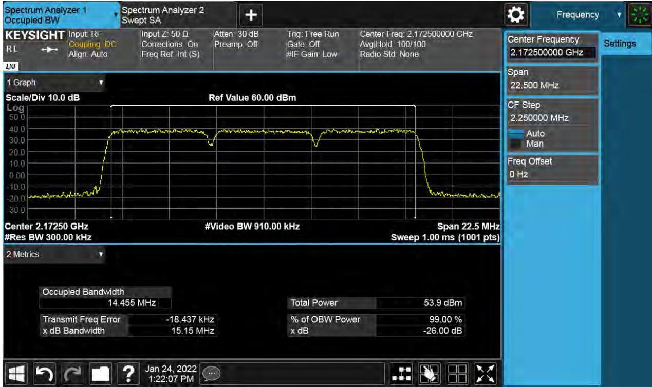
**Antenna 0 / (4 Port) LTE B66 5 MHz 1 Carrier + LTE B66 5 MHz 1 Carrier + LTE B66 5 MHz 1 Carrier + 5G NR n66 5 MHz 1 Carrier [4 Carrier] (3C+1C) / Non-Contiguous / LTE B66 5 MHz + LTE B66 5 MHz + LTE B66 5 MHz / QPSK / Low**
