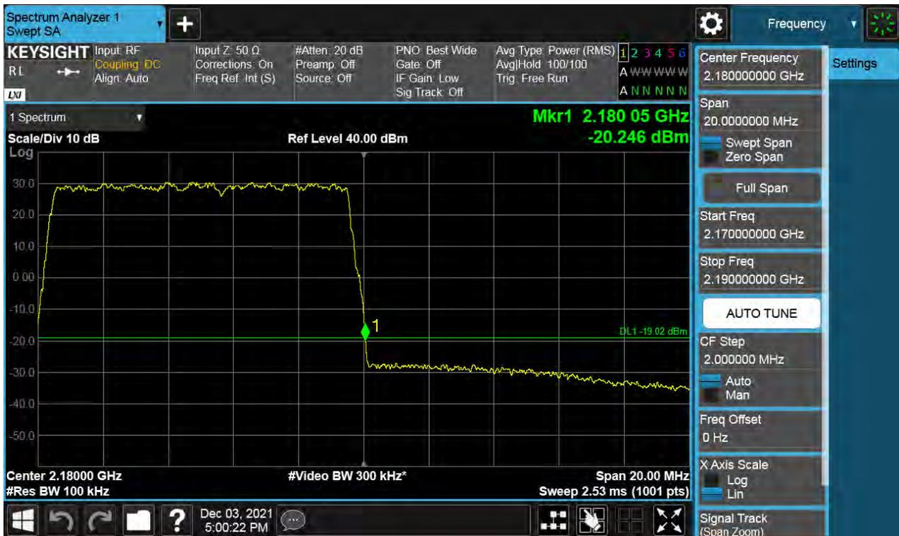
**Antenna 0 / (2 Port) B66 DSS 15 MHz 2to8 1 Carrier / QPSK / Low**
