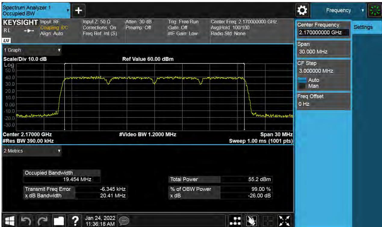
Antenna 1 / (4 Port) LTE B66 5 MHz 1 Carrier + LTE B66 5 MHz 1 Carrier + LTE B66 10 MHz 1 Carrier + 5G NR n66 20 MHz 1 Carrier [4 Carrier] / Contiguous / 64QAM / High
