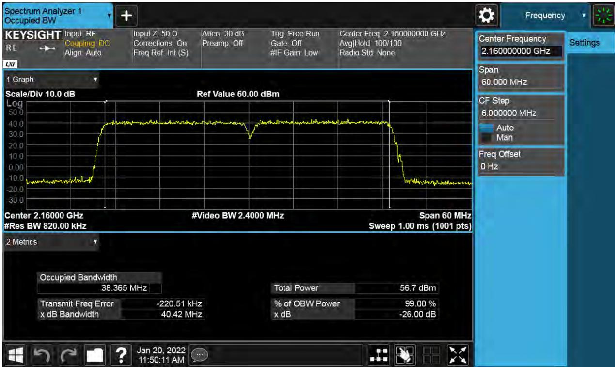
**Antenna 1 / (4 Port) LTE B66 5 MHz 1 Carrier + 5G NR n66 10 MHz 1 Carrier [2 Carrier] / Contiguous / 16QAM / High**
