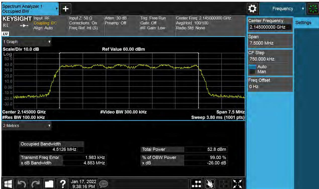
Antenna 1 / (2 Port) 5G NR n66 10 MHz 1 Carrier / 64QAM / Middle
