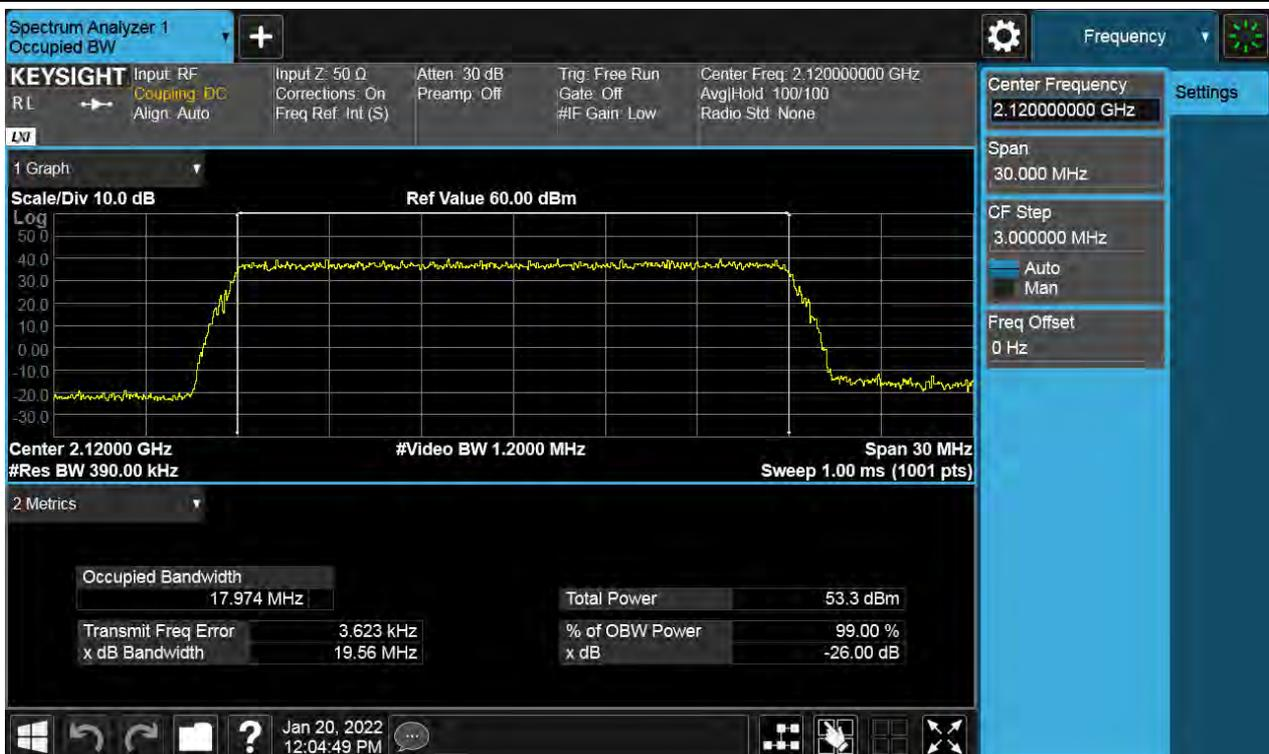
**Antenna 1 / (2 Port) LTE B66 20 MHz 1 Carrier + 5G NR n66 20 MHz 1 Carrier [2 Carrier] / Non-Contiguous / 5G NR n66 20 MHz / QPSK / High**
