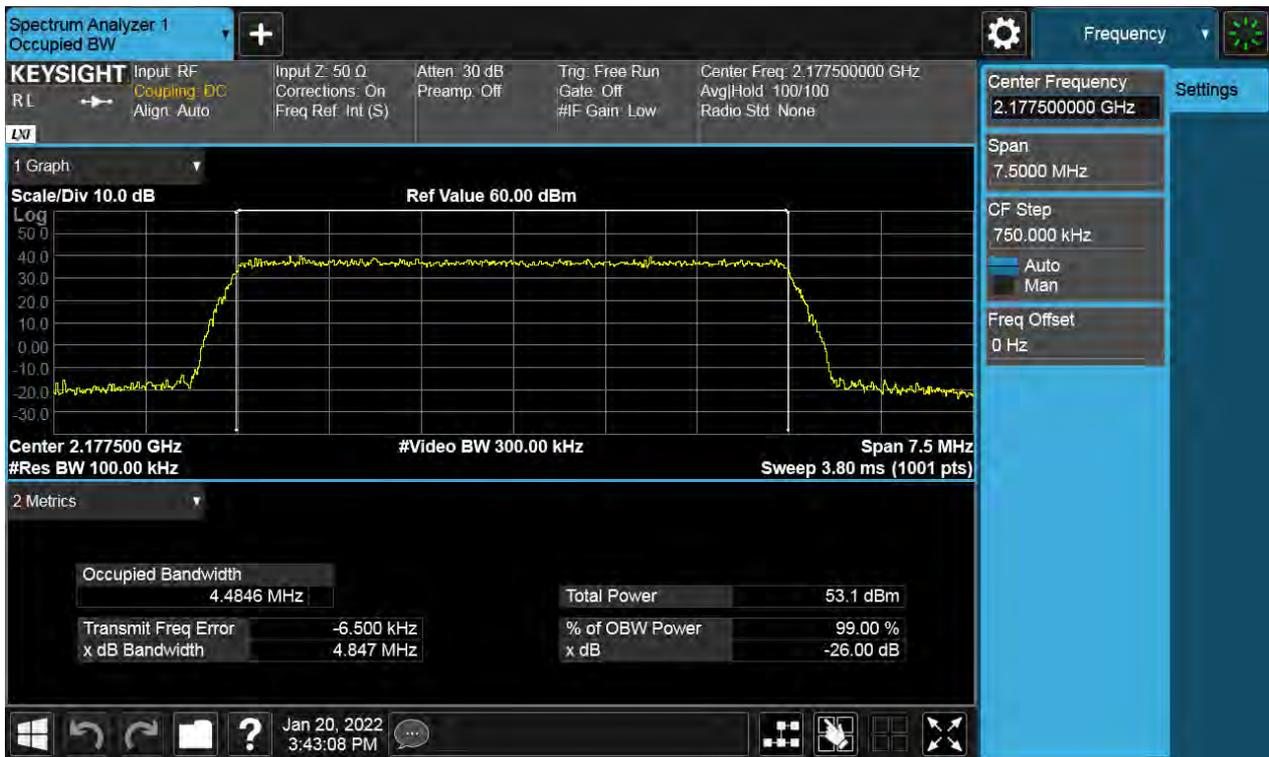
**Antenna 1 / (2 Port) LTE B66 20 MHz 1 Carrier + 5G NR n66 20 MHz 1 Carrier [2 Carrier] / Non-Contiguous / LTE B66 20 MHz / QPSK / Low**
