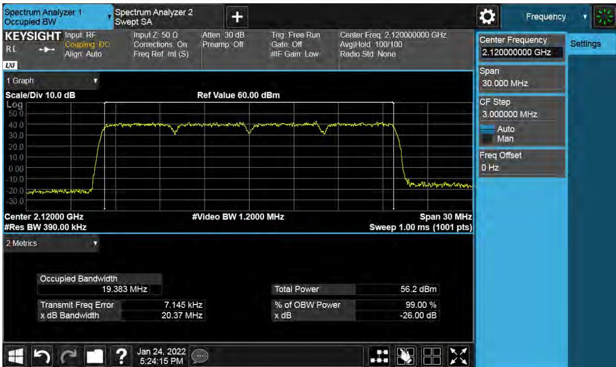
**Antenna 1 / (2 Port) LTE B66 5 MHz 1 Carrier + LTE B66 5 MHz 1 Carrier + LTE B66 10 MHz 1 Carrier + 5G NR n66 20 MHz 1 Carrier [4 Carrier] / Contiguous / QPSK / Middle**
