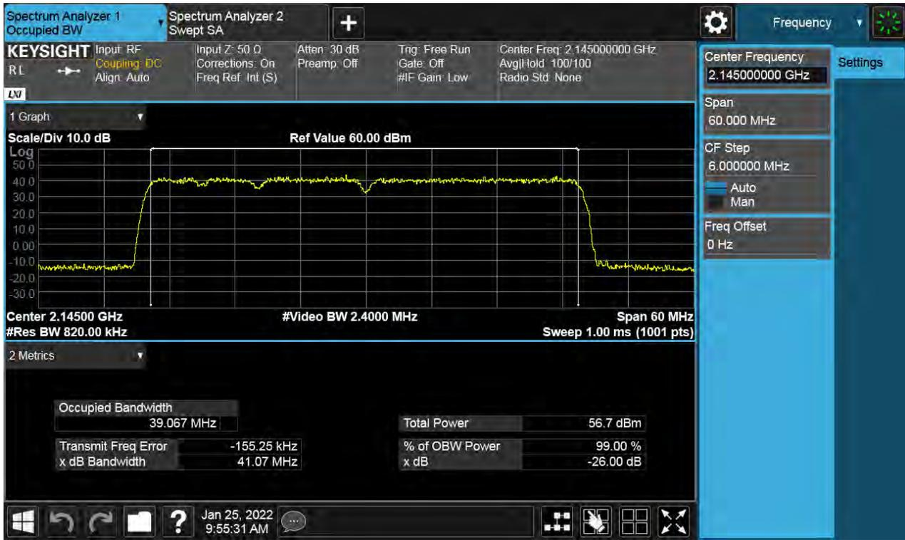
**Antenna 1 / (4 Port) LTE B66 5 MHz 1 Carrier + LTE B66 5 MHz 1 Carrier + LTE B66 5 MHz 1 Carrier + 5G NR n66 5 MHz 1 Carrier [4 Carrier] / Contiguous / 256QAM / High**
