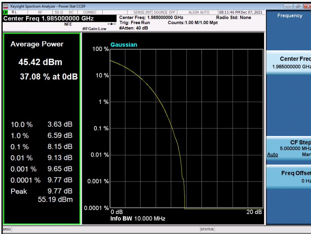
Antenna 1 / (4 Port) B2 DSS 10 MHz 9to1 1 Carrier + LTE B2 5 MHz 1 Carrier [2 Carrier] / Non-Contiguous / B2 DSS 10 MHz 9to1 / 256QAM / Low
