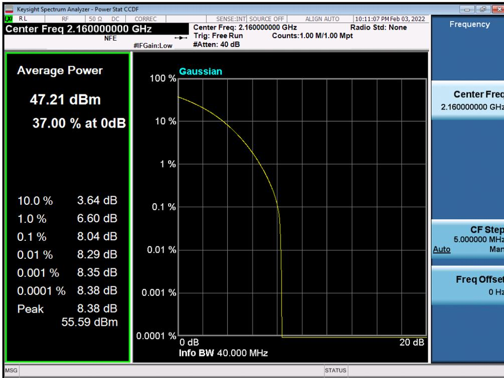
**Antenna 0 / (2 Port) B2 DSS 10 MHz 9to1 1 Carrier + LTE B2 5 MHz 1 Carrier [2 Carrier] / Non-Contiguous / B2 DSS 10 MHz 9to1 / 256QAM / Low**
