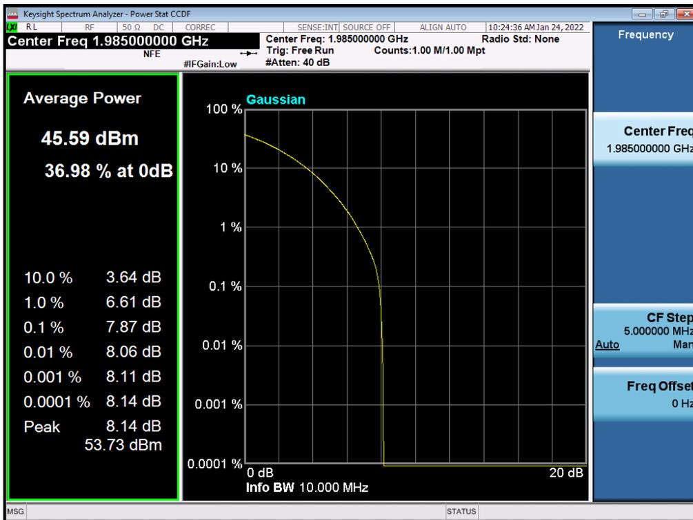
Antenna 0 / (4 Port) LTE B2 10 MHz 1 Carrier + 5G NR n2 20 MHz 1 Carrier [2 Carrier] / Contiguous / 64QAM / High
