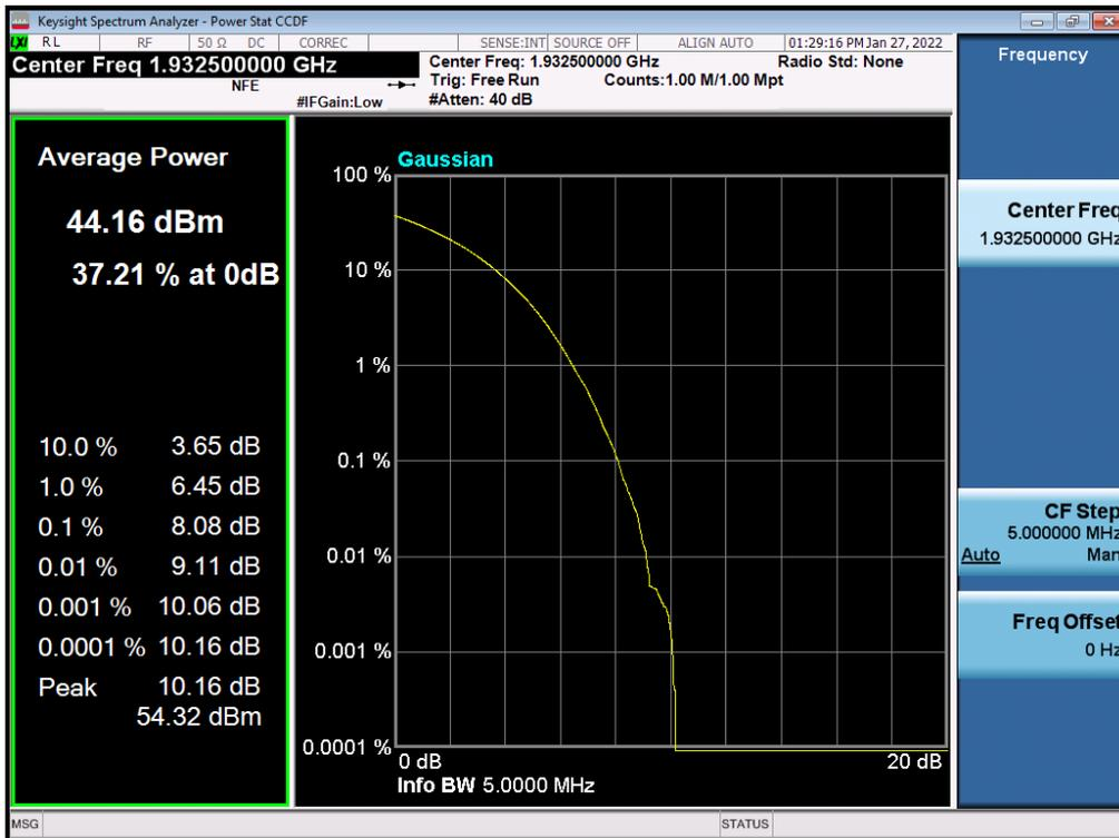
Antenna 0 / (2 Port) LTE B2 5 MHz 1 Carrier + 5G NR n2 5 MHz 1 Carrier [2 Carrier] / Non-Contiguous / 5G NR n2 5 MHz / 16QAM / High
