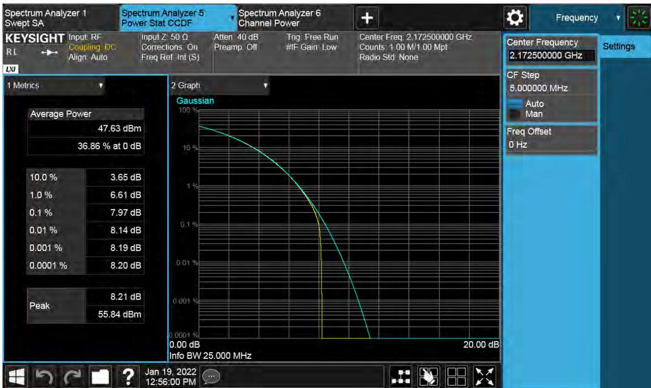
Antenna 1 / (4 Port) LTE B66 20 MHz 1 Carrier + 5G NR n66 20 MHz 1 Carrier [2 Carrier] / Contiguous / QPSK / Low
