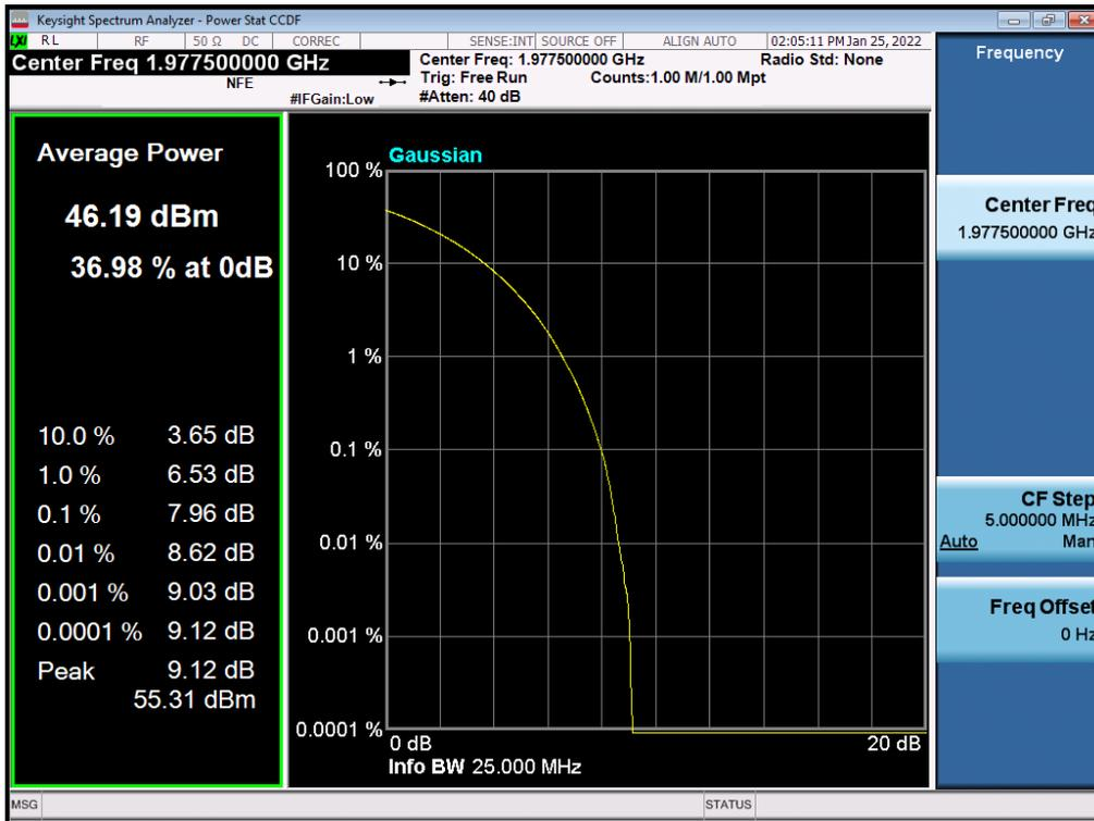
Antenna 0 / (2 Port) LTE B2 5 MHz 1 Carrier + LTE B2 5 MHz 1 Carrier + 5G NR n2 20 MHz 1 Carrier [3 Carrier] (2C+1C) / Non-Contiguous / LTE B2 5 MHz + LTE B2 5 MHz / 16QAM / Low
