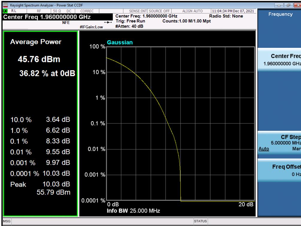
Antenna 0 / (2 Port) LTE B2 5 MHz 1 Carrier + 5G NR n2 5 MHz 1 Carrier [2 Carrier] / Contiguous / 256QAM / High
