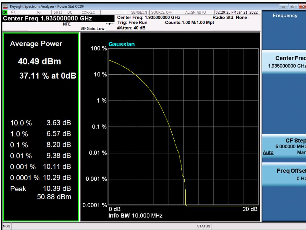
Antenna 0 / (4 Port) LTE B2 10 MHz 1 Carrier + 5G NR n2 20 MHz 1 Carrier [2 Carrier] / Non-Contiguous / 5G NR n2 20 MHz / QPSK / High
