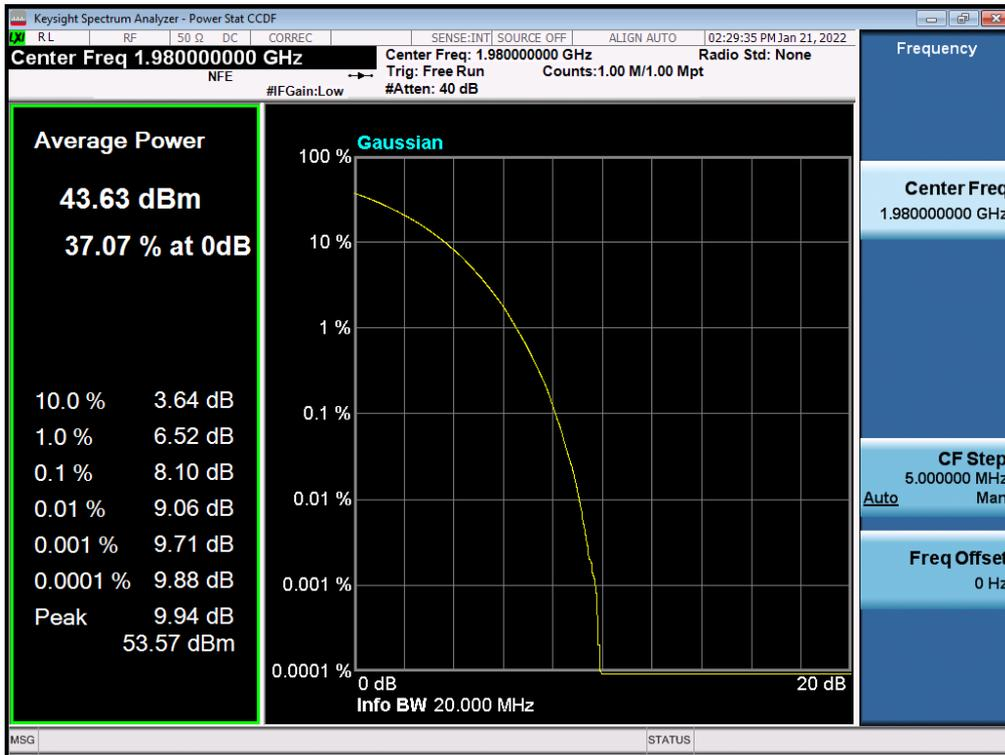
Antenna 0 / (2 Port) B66 DSS 10 MHz 9to1 1 Carrier + LTE B66 5 MHz 1 Carrier [2 Carrier] / Non-Contiguous / B66 DSS 10 MHz 9to1 / 256QAM / Low
