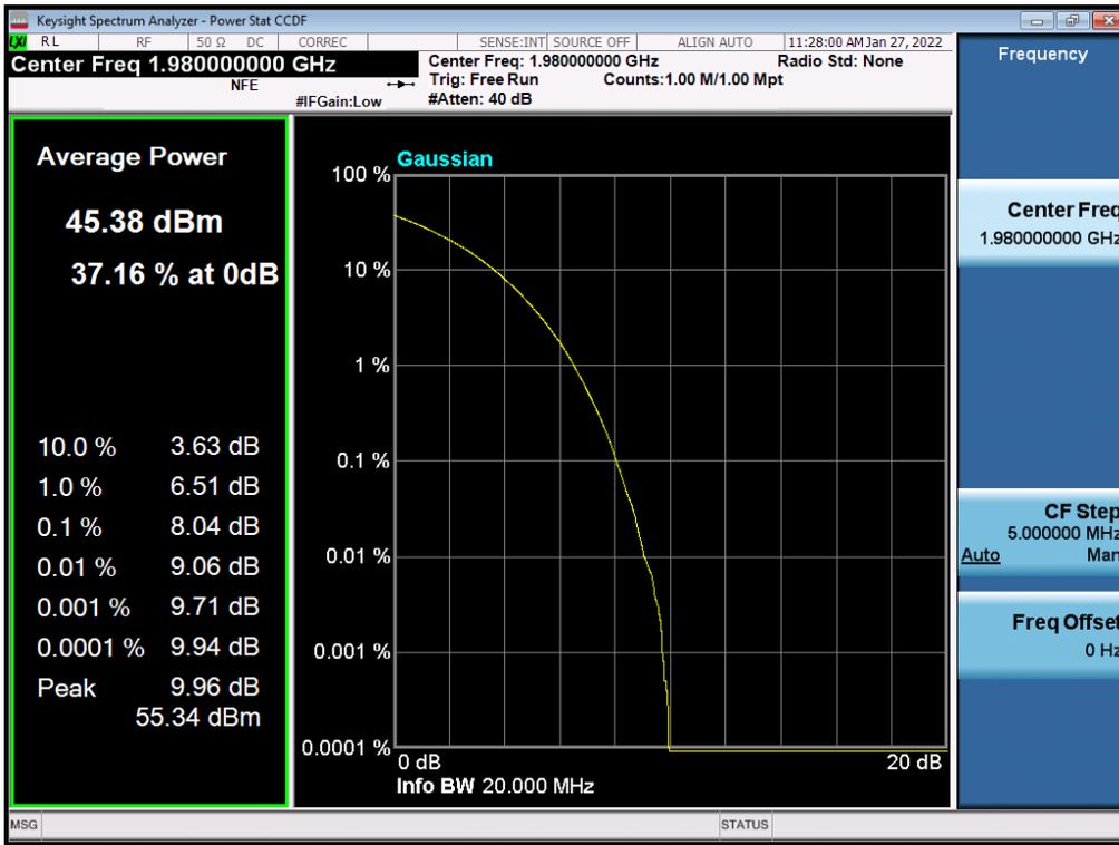
Antenna 0 / (4 Port) LTE B2 5 MHz 1 Carrier + 5G NR n2 5 MHz 1 Carrier [2 Carrier] / Non-Contiguous / LTE B2 5 MHz / 64QAM / Low
