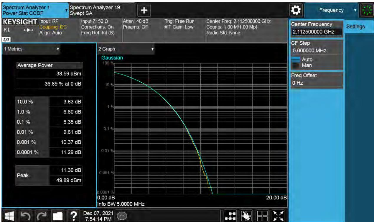
**Antenna 3 / (4 Port) B66 DSS 20 MHz 9to1 1 Carrier + LTE B66 10 MHz 1 Carrier + LTE B66 5 MHz 1 Carrier + LTE B66 5 MHz 1 Carrier [4 Carrier] (1C+3C) / Non-Contiguous / LTE B66 10 MHz + LTE B66 5 MHz + LTE B66 5 MHz / QPSK / High**
