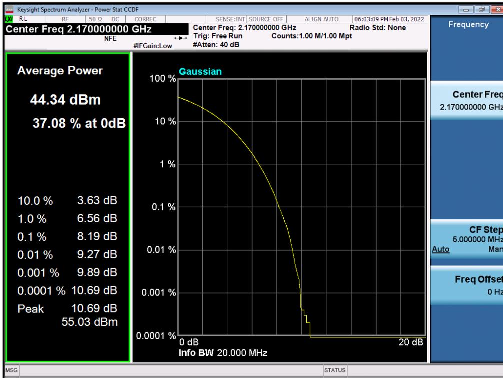
**Antenna 0 / (2 Port) B2 DSS 20 MHz 9to1 1 Carrier + LTE B2 5 MHz 1 Carrier + LTE B2 5 MHz 1 Carrier [3 Carrier] (1C+2C) / Non-Contiguous / B2 DSS 20 MHz 9to1 / 16QAM / Low**
