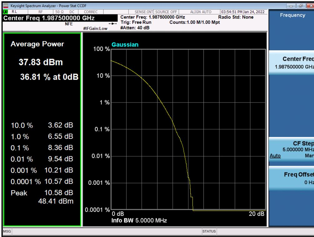
Antenna 1 / (2 Port) B66 DSS 20 MHz 9to1 1 Carrier + LTE B66 10 MHz 1 Carrier + LTE B66 5 MHz 1 Carrier + LTE B66 5 MHz 1 Carrier [4 Carrier] (1C+3C) / Non-Contiguous / B66 DSS 20 MHz 9to1 / 64QAM / Low
