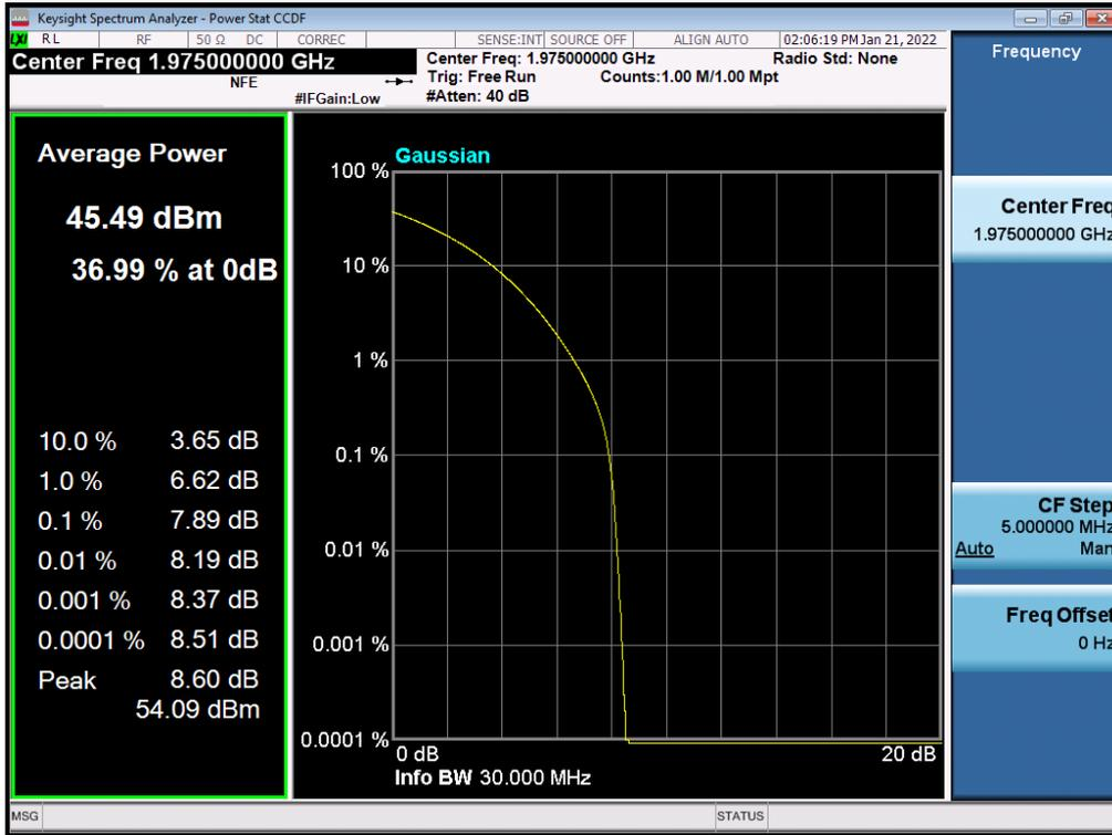
Antenna 0 / (2 Port) B66 DSS 10 MHz 9to1 1 Carrier + LTE B66 5 MHz 1 Carrier [2 Carrier] / Contiguous / QPSK / High
