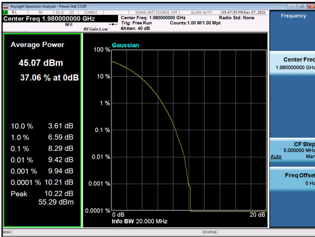
Antenna 0 / (4 Port) B2 DSS 20 MHz 9to1 1 Carrier + LTE B2 5 MHz 1 Carrier + LTE B2 5 MHz 1 Carrier [3 Carrier] (1C+2C) / Non-Contiguous / B2 DSS 20 MHz 9to1 / 16QAM / Low
