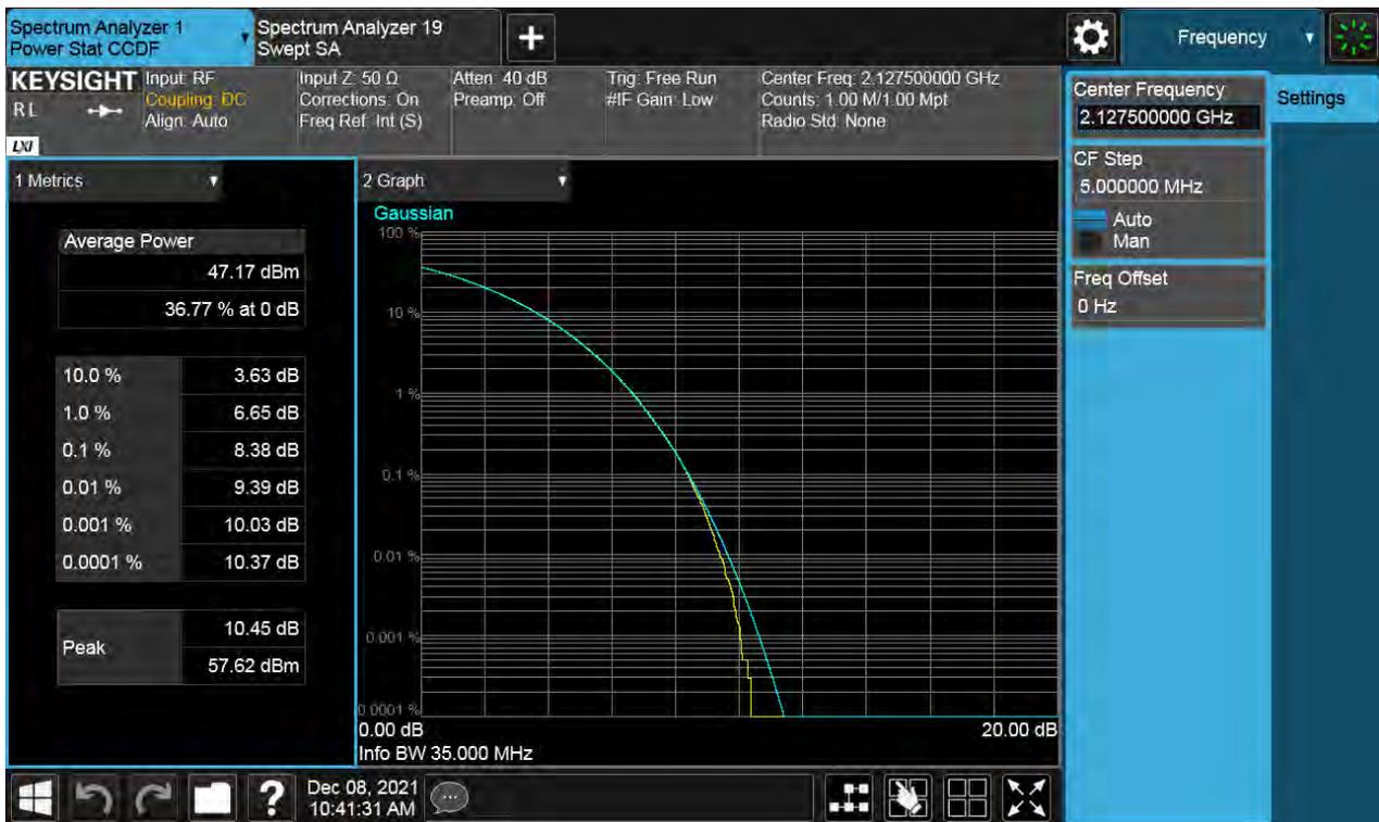
**Antenna 1 / (4 Port) B66 DSS 20 MHz 9to1 1 Carrier + LTE B66 10 MHz 1 Carrier + LTE B66 5 MHz 1 Carrier + LTE B66 5 MHz 1 Carrier [4 Carrier] (3C+1C) / Non-Contiguous / LTE B66 5 MHz / 16QAM / High**
