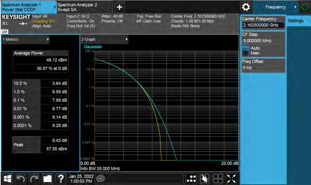
Antenna 1 / (2 Port) LTE B66 5 MHz 1 Carrier + LTE B66 5 MHz 1 Carrier + LTE B66 10 MHz 1 Carrier + 5G NR n66 20 MHz 1 Carrier [4 Carrier] (3C+1C) / Non-Contiguous / LTE B66 5 MHz + LTE B66 5 MHz + LTE B66 10 MHz / QPSK / Low
