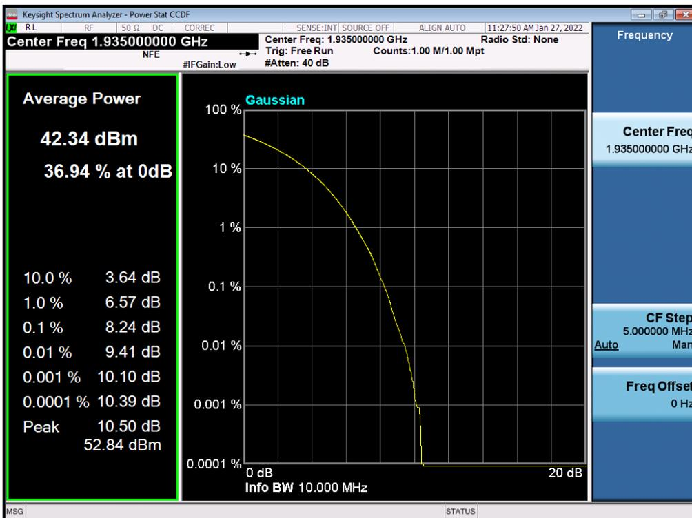
Antenna 0 / (2 Port) LTE B2 10 MHz 1 Carrier + 5G NR n2 20 MHz 1 Carrier [2 Carrier] / Non-Contiguous / 5G NR n2 20 MHz / 64QAM / High
