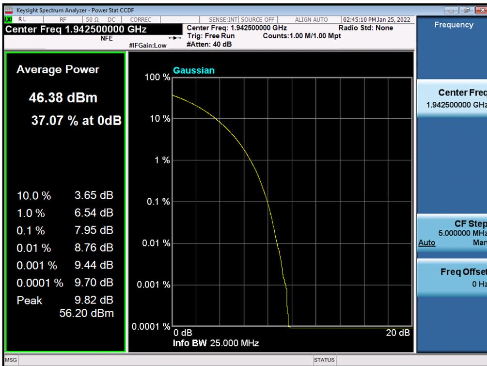
Antenna 0 / (2 Port) LTE B2 5 MHz 1 Carrier + LTE B2 5 MHz 1 Carrier + 5G NR n2 20 MHz 1 Carrier [3 Carrier] (2C+1C) / Non-Contiguous / 5G NR n2 20 MHz / 16QAM / High
