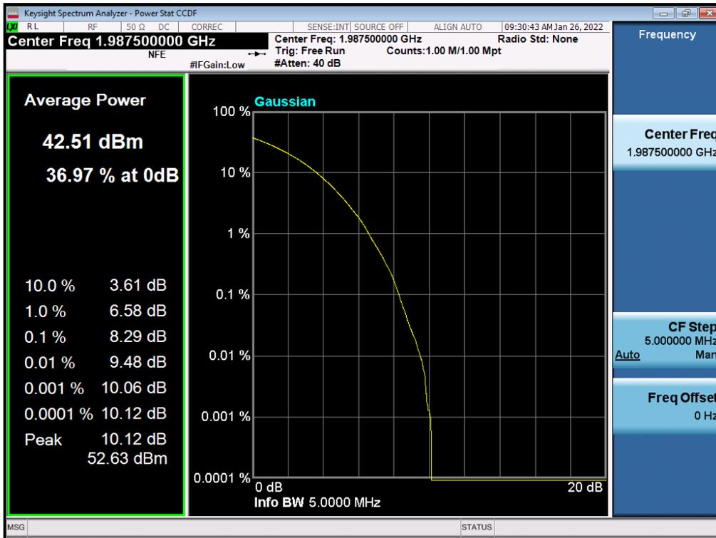
Antenna 0 / (2 Port) LTE B2 5 MHz 1 Carrier + LTE B2 5 MHz 1 Carrier + 5G NR n2 20 MHz 1 Carrier [3 Carrier] (1C+2C) / Non-Contiguous / LTE B2 5 MHz / QPSK / Low
