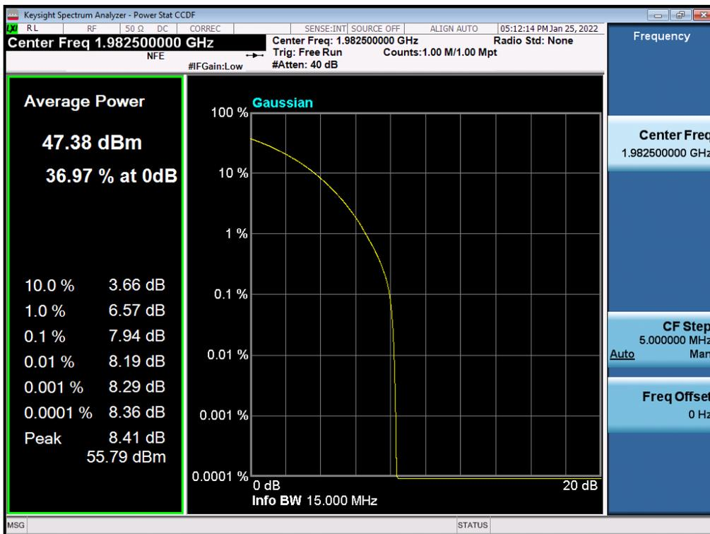
Antenna 0 / (2 Port) LTE B2 5 MHz 1 Carrier + LTE B2 5 MHz 1 Carrier + 5G NR n2 20 MHz 1 Carrier [3 Carrier] / Contiguous / 64QAM / High
