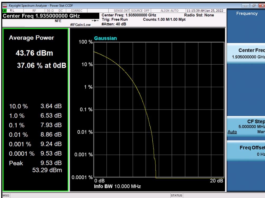
Antenna 0 / (4 Port) LTE B2 5 MHz 1 Carrier + LTE B2 5 MHz 1 Carrier + 5G NR n2 5 MHz 1 Carrier [3 Carrier] (2C+1C) / Non-Contiguous / 5G NR n2 5 MHz / 64QAM / High
