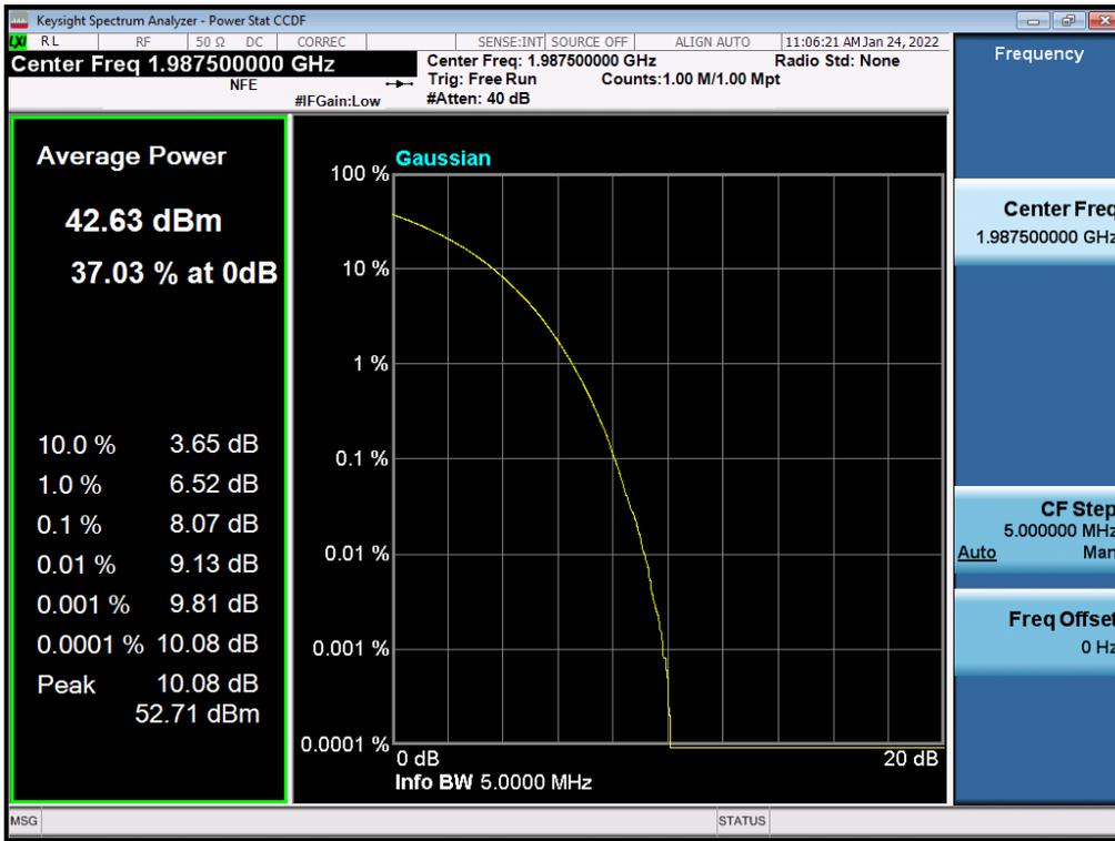
Antenna 0 / (4 Port) LTE B2 10 MHz 1 Carrier + 5G NR n2 20 MHz 1 Carrier [2 Carrier] / Non-Contiguous / LTE B2 10 MHz / QPSK / Low
