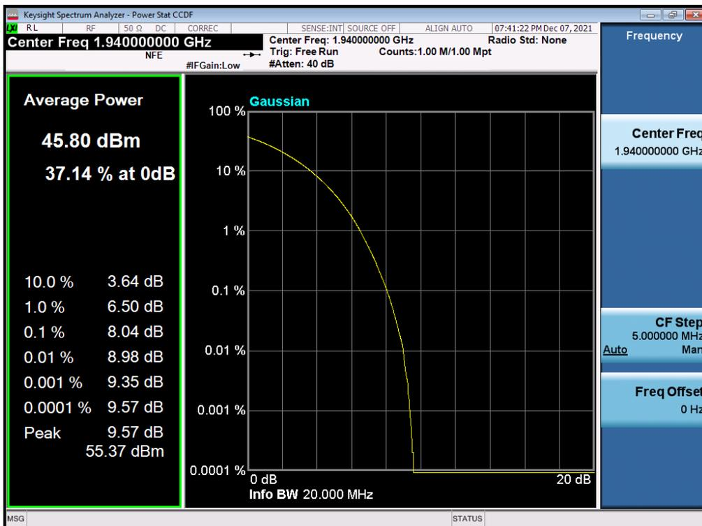
Antenna 0 / (2 Port) B2 DSS 20 MHz 9to1 1 Carrier + LTE B2 5 MHz 1 Carrier + LTE B2 5 MHz 1 Carrier [3 Carrier] (1C+2C) / Non-Contiguous / LTE B2 5 MHz + LTE B2 5 MHz / 16QAM / High
