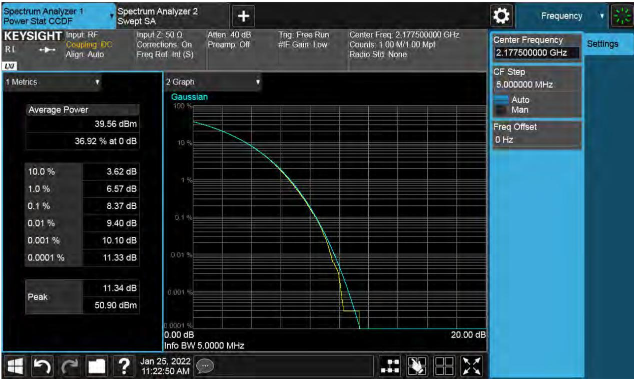
**Antenna 1 / (4 Port) LTE B66 5 MHz 1 Carrier + LTE B66 5 MHz 1 Carrier + LTE B66 5 MHz 1 Carrier + 5G NR n66 5 MHz 1 Carrier [4 Carrier] (1C+3C) / Non-Contiguous / LTE B66 5 MHz / QPSK / Low**
