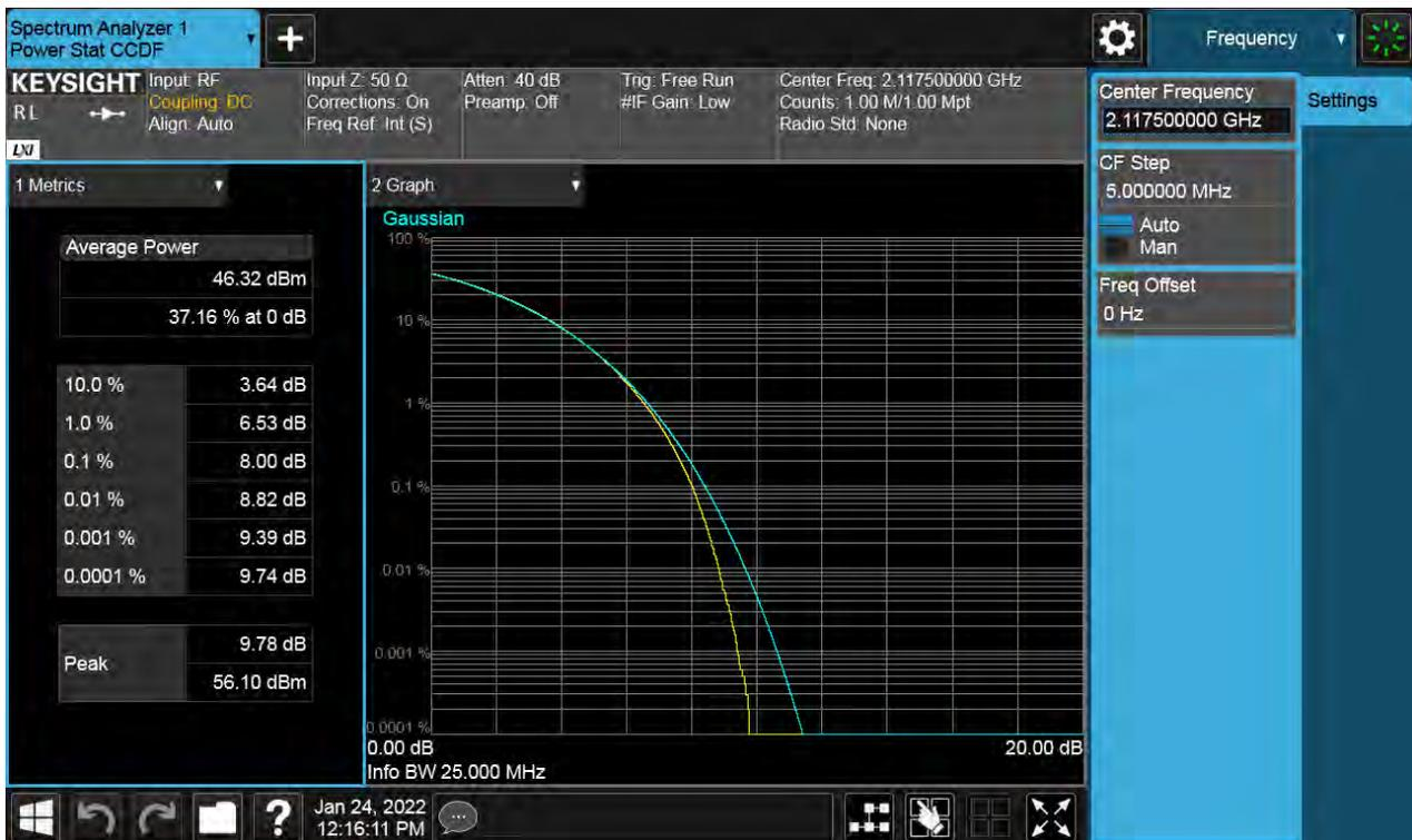
**Antenna 0 / (4 Port) LTE B66 5 MHz 1 Carrier + LTE B66 5 MHz 1 Carrier + LTE B66 5 MHz 1 Carrier + 5G NR n66 5 MHz 1 Carrier [4 Carrier] (3C+1C) / Non-Contiguous / 5G NR n66 5 MHz / QPSK / High**
