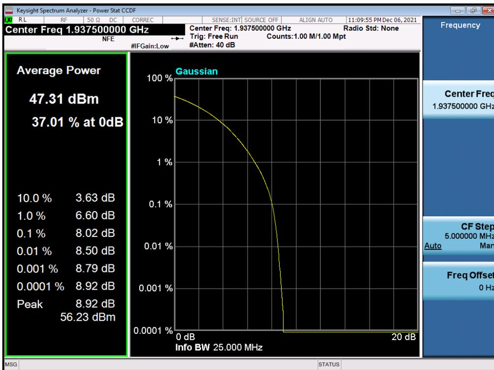
Antenna 0 / (4 Port) B2 DSS 10 MHz 9to1 1 Carrier + LTE B2 5 MHz 1 Carrier [2 Carrier] / Contiguous / QPSK / Middle
