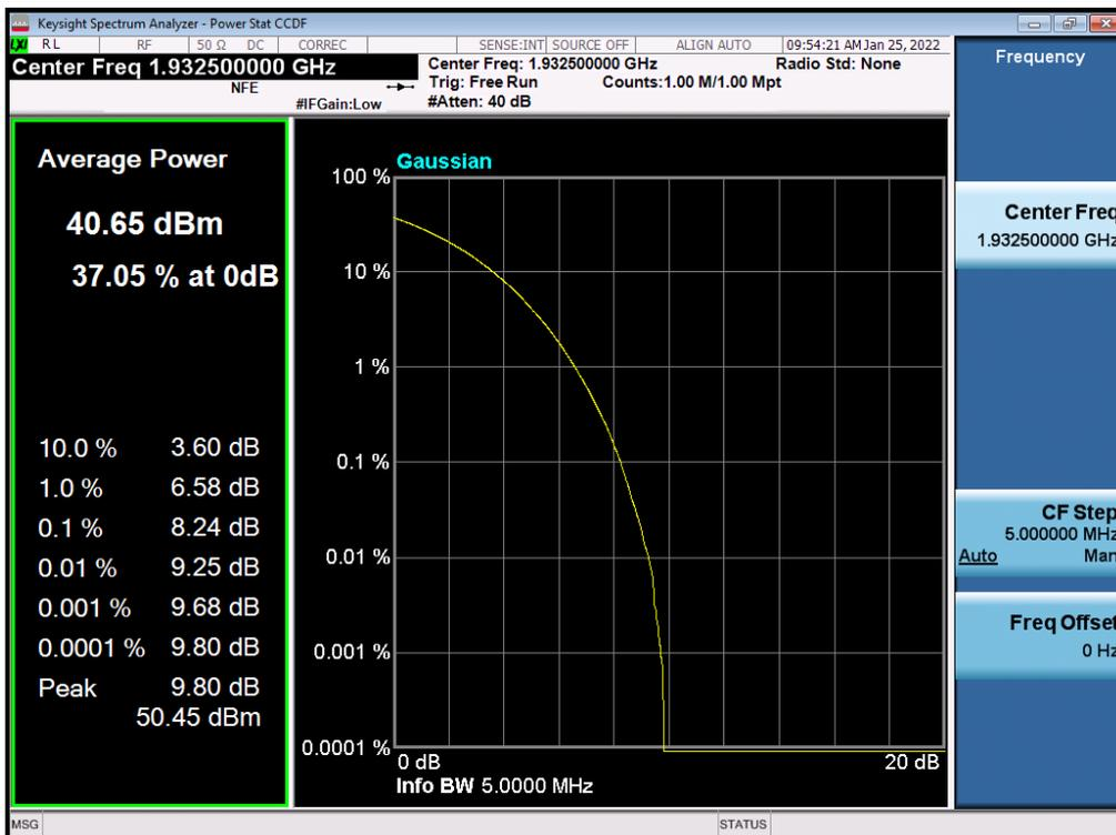
Antenna 0 / (4 Port) LTE B2 5 MHz 1 Carrier + LTE B2 5 MHz 1 Carrier + 5G NR n2 5 MHz 1 Carrier [3 Carrier] (1C+2C) / Non-Contiguous / LTE B2 5 MHz + 5G NR n2 5 MHz / QPSK / High
