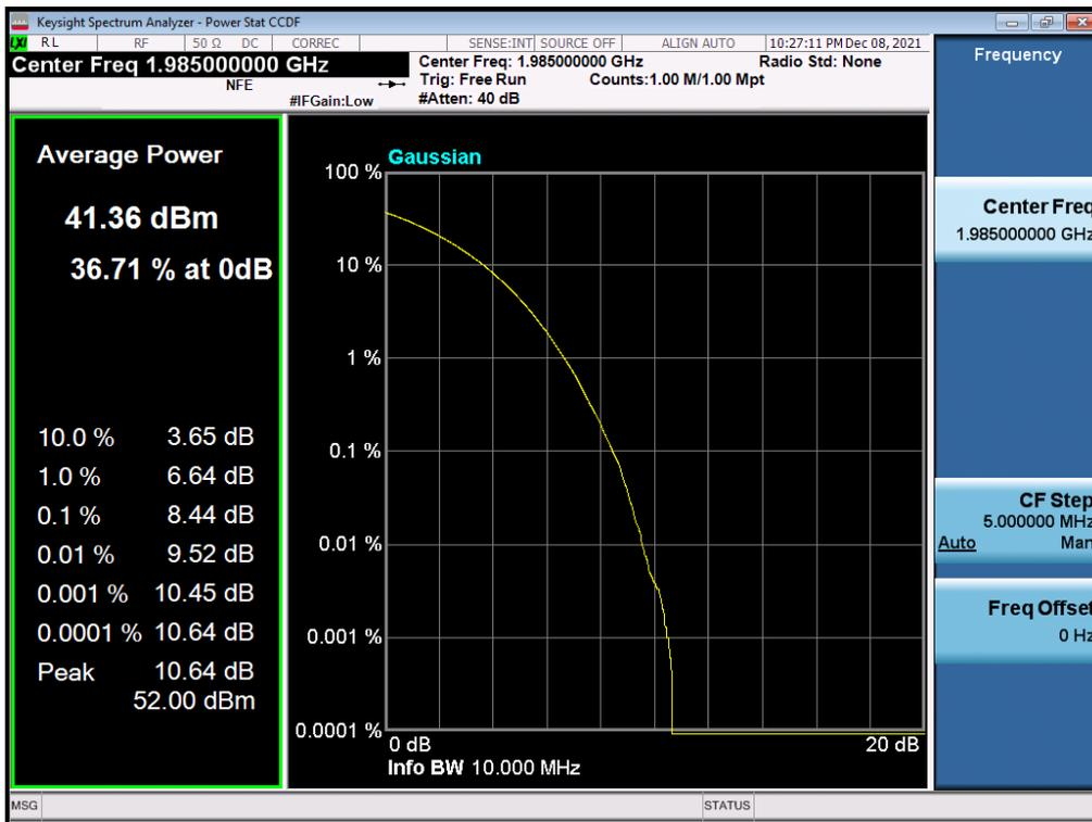
Antenna 1 / (4 Port) B2 DSS 20 MHz 9to1 1 Carrier + LTE B2 5 MHz 1 Carrier + LTE B2 5 MHz 1 Carrier [3 Carrier] (2C+1C) / Non-Contiguous / B2 DSS 20 MHz 9to1 + LTE B2 5 MHz / QPSK / Low
