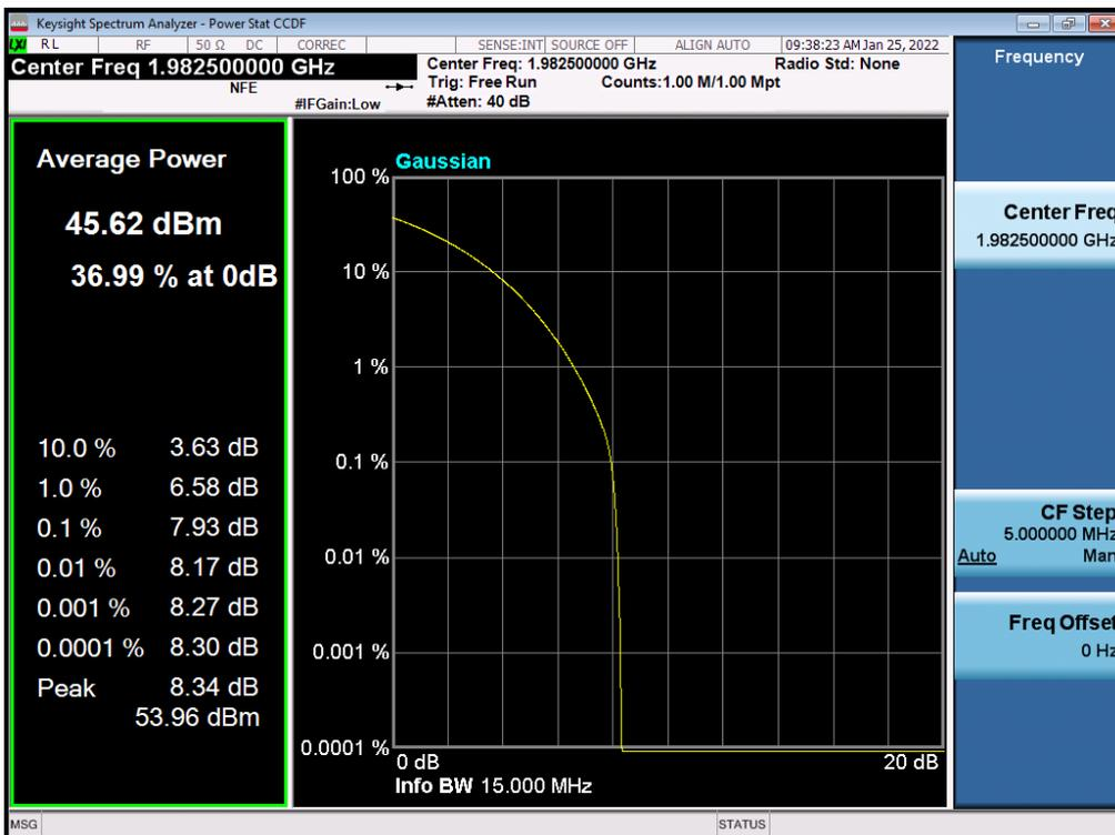
Antenna 0 / (4 Port) LTE B2 5 MHz 1 Carrier + LTE B2 5 MHz 1 Carrier + 5G NR n2 20 MHz 1 Carrier [3 Carrier] / Contiguous / 16QAM / High
