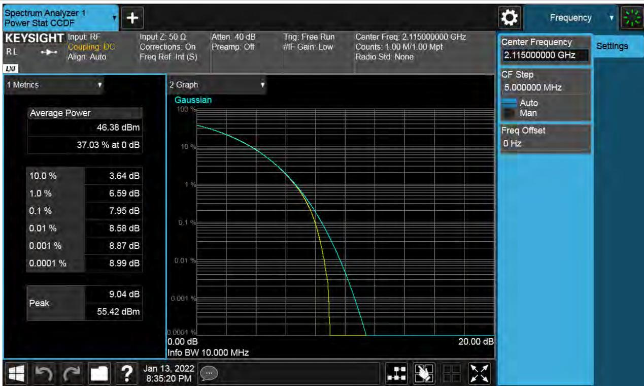
**Antenna 3 / (4 Port) 5G NR n66 15 MHz 1 Carrier / QPSK / Low**
