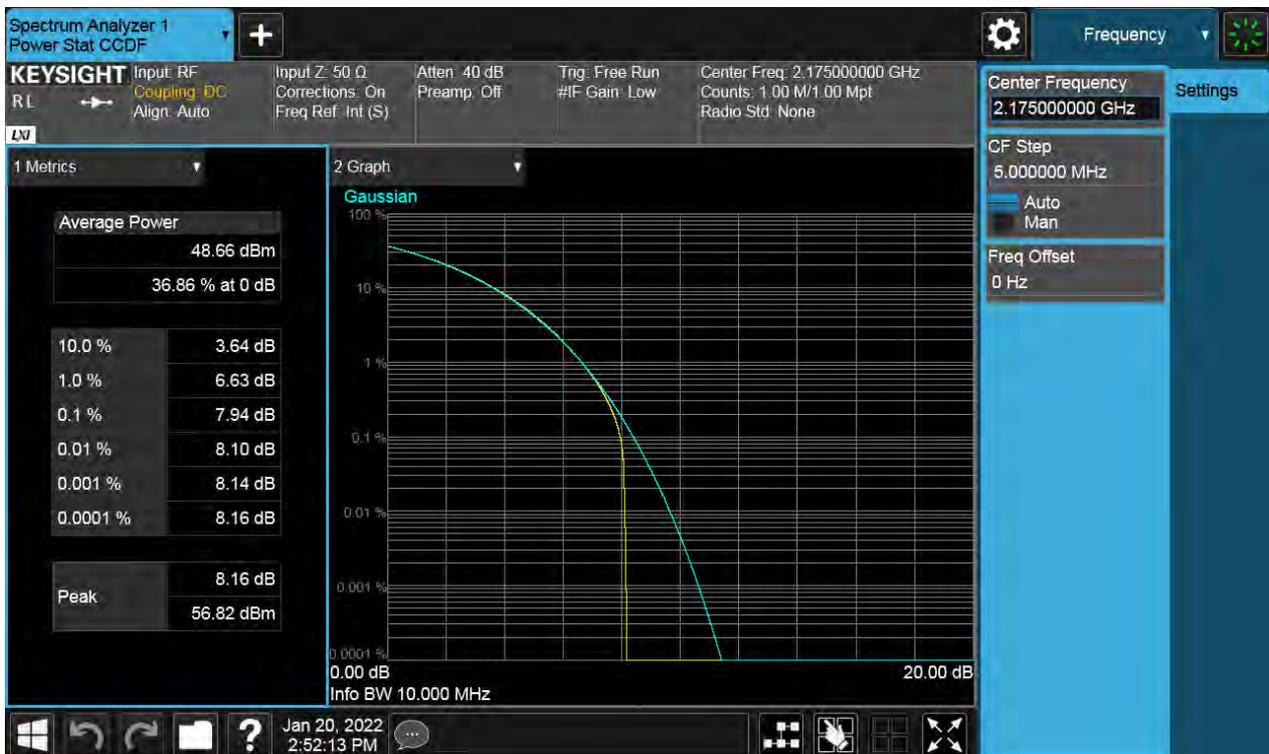
**Antenna 1 / (2 Port) LTE B66 20 MHz 1 Carrier + 5G NR n66 20 MHz 1 Carrier [2 Carrier] / Contiguous / 256QAM / High**
