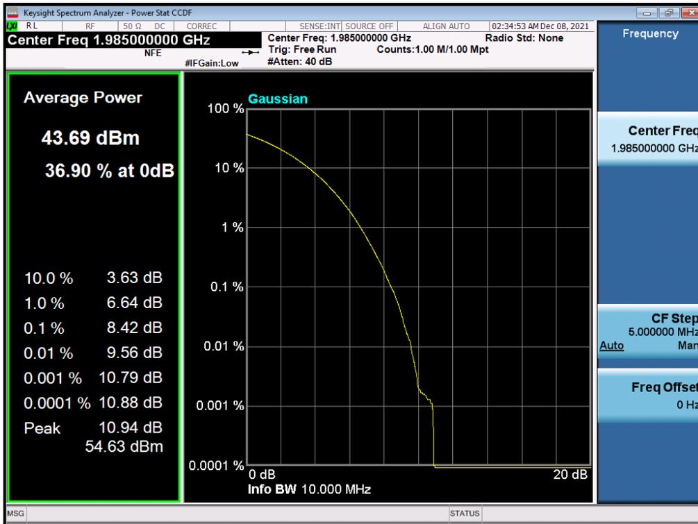
Antenna 0 / (2 Port) LTE B2 5 MHz 1 Carrier + 5G NR n2 5 MHz 1 Carrier [2 Carrier] / Non-Contiguous / LTE B2 5 MHz / 16QAM / Low
