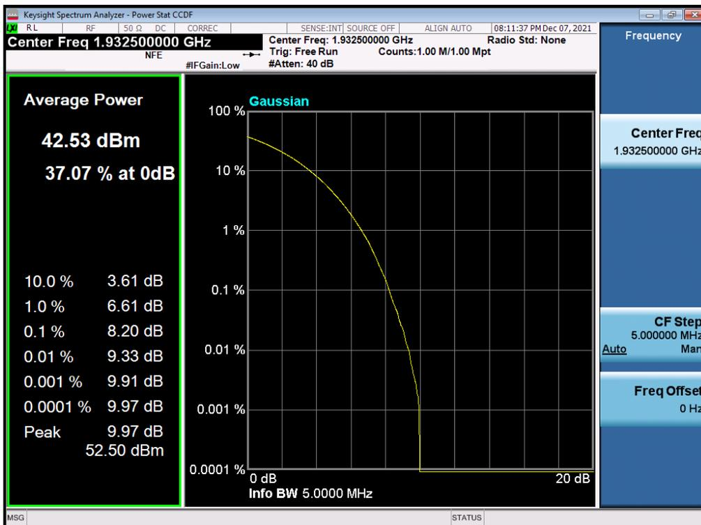
Antenna 0 / (2 Port) B2 DSS 10 MHz 9to1 1 Carrier + LTE B2 5 MHz 1 Carrier [2 Carrier] / Non-Contiguous / LTE B2 5 MHz / 256QAM / High
