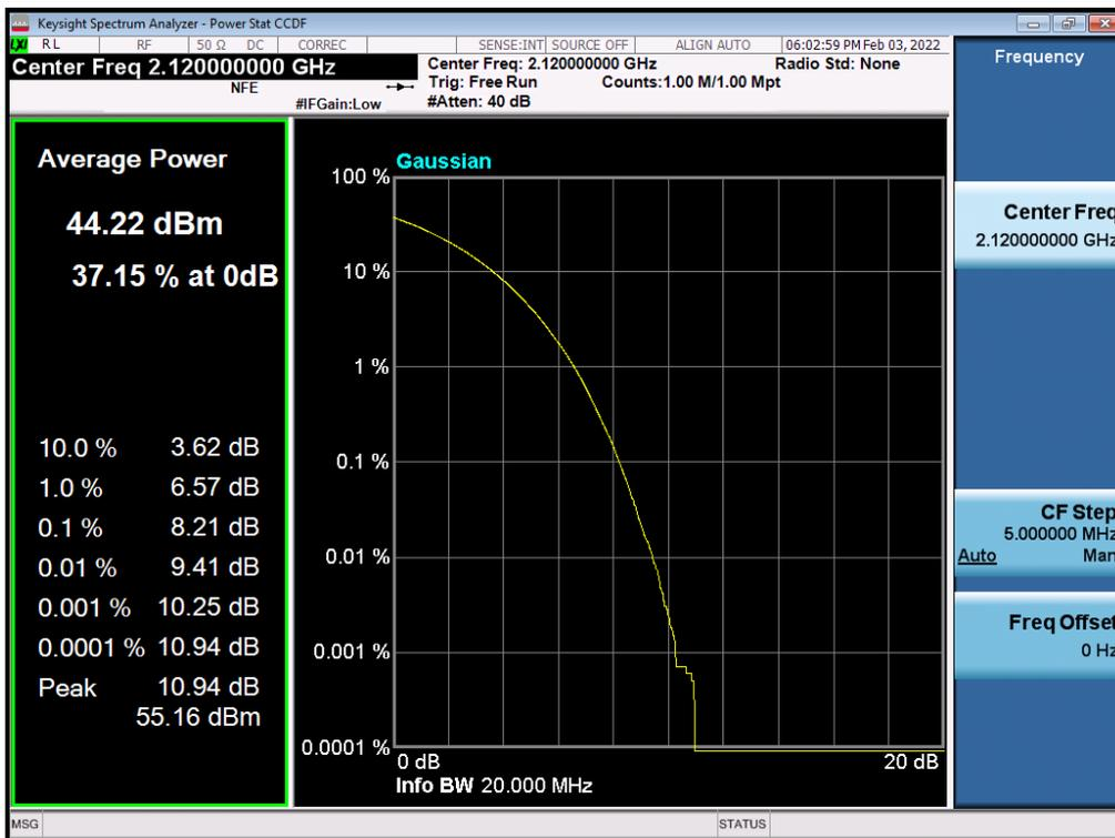
**Antenna 2 / (4 Port) LTE B66 20 MHz 1 Carrier + 5G NR n66 20 MHz 1 Carrier [2 Carrier] / Non-Contiguous / 5G NR n66 20 MHz / 256QAM / High**
