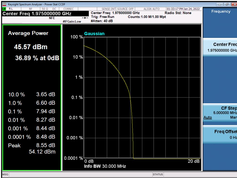
Antenna 0 / (2 Port) B66 DSS 20 MHz 9to1 1 Carrier + LTE B66 10 MHz 1 Carrier + LTE B66 5 MHz 1 Carrier + LTE B66 5 MHz 1 Carrier [4 Carrier] / Contiguous / QPSK / Low
