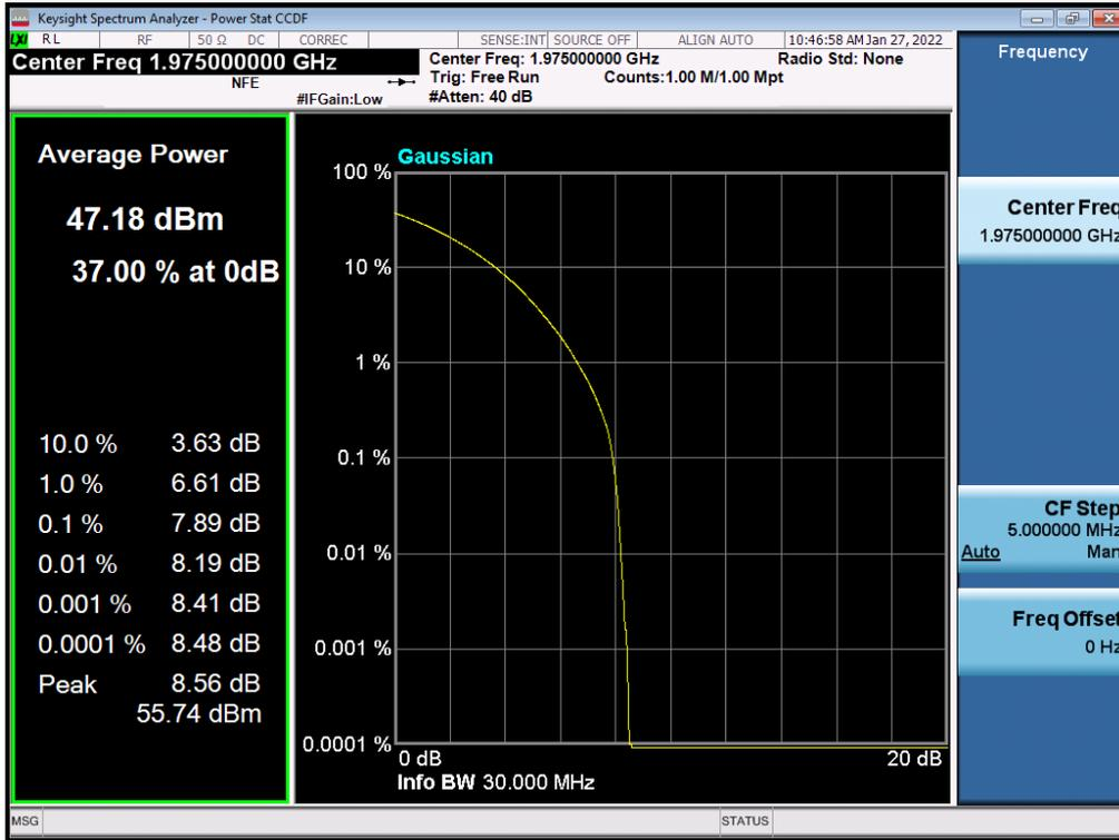
Antenna 0 / (4 Port) LTE B2 5 MHz 1 Carrier + 5G NR n2 5 MHz 1 Carrier [2 Carrier] / Contiguous / 256QAM / High
