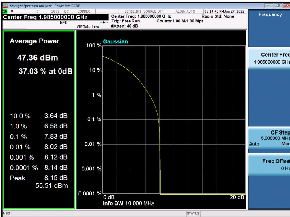
Antenna 0 / (2 Port) LTE B2 10 MHz 1 Carrier + 5G NR n2 20 MHz 1 Carrier [2 Carrier] / Contiguous / 64QAM / High
