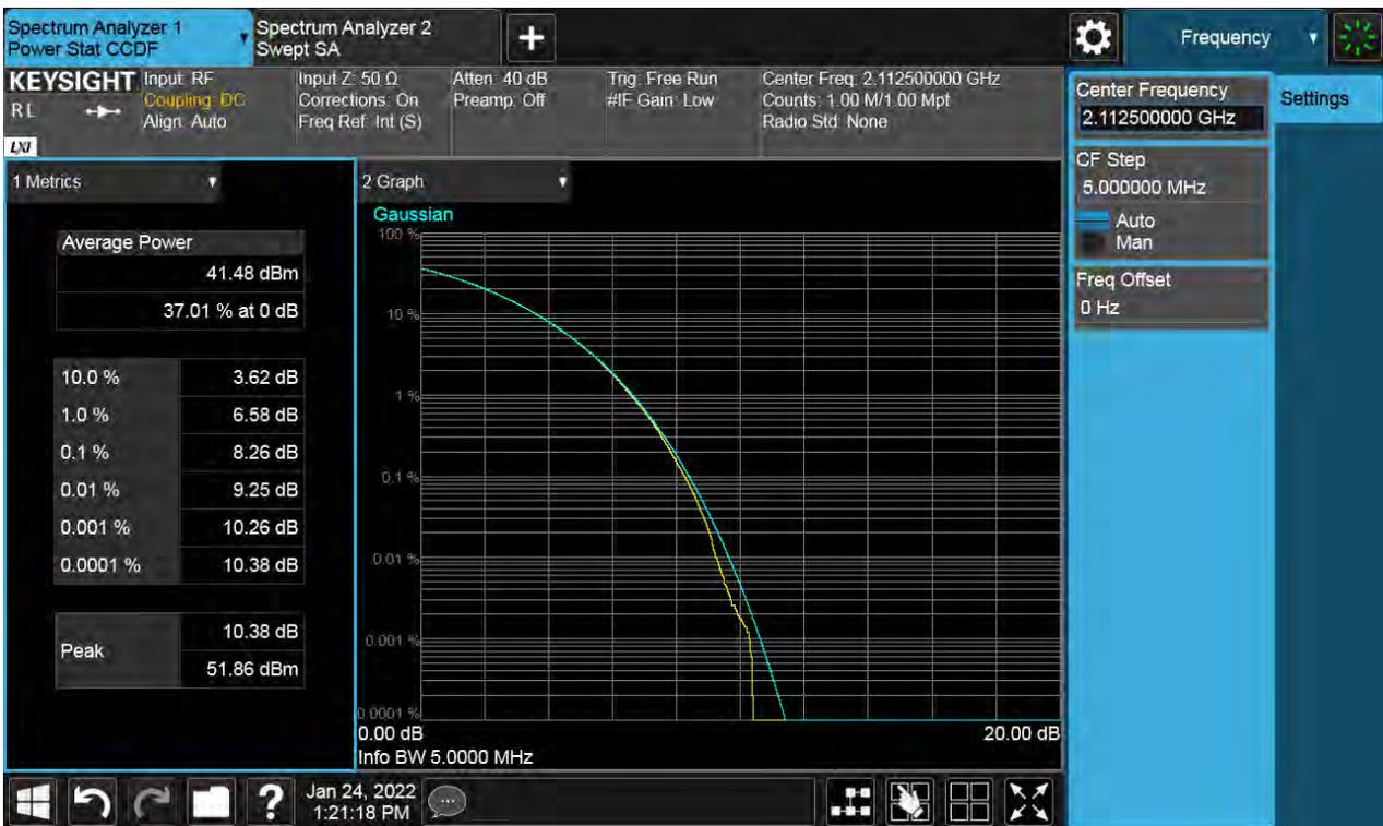
**Antenna 1 / (4 Port) LTE B66 5 MHz 1 Carrier + LTE B66 5 MHz 1 Carrier + LTE B66 5 MHz 1 Carrier + 5G NR n66 5 MHz 1 Carrier [4 Carrier] (1C+3C) / Non-Contiguous / LTE B66 5 MHz + LTE B66 5 MHz + 5G NR n66 5 MHz / QPSK / High**
