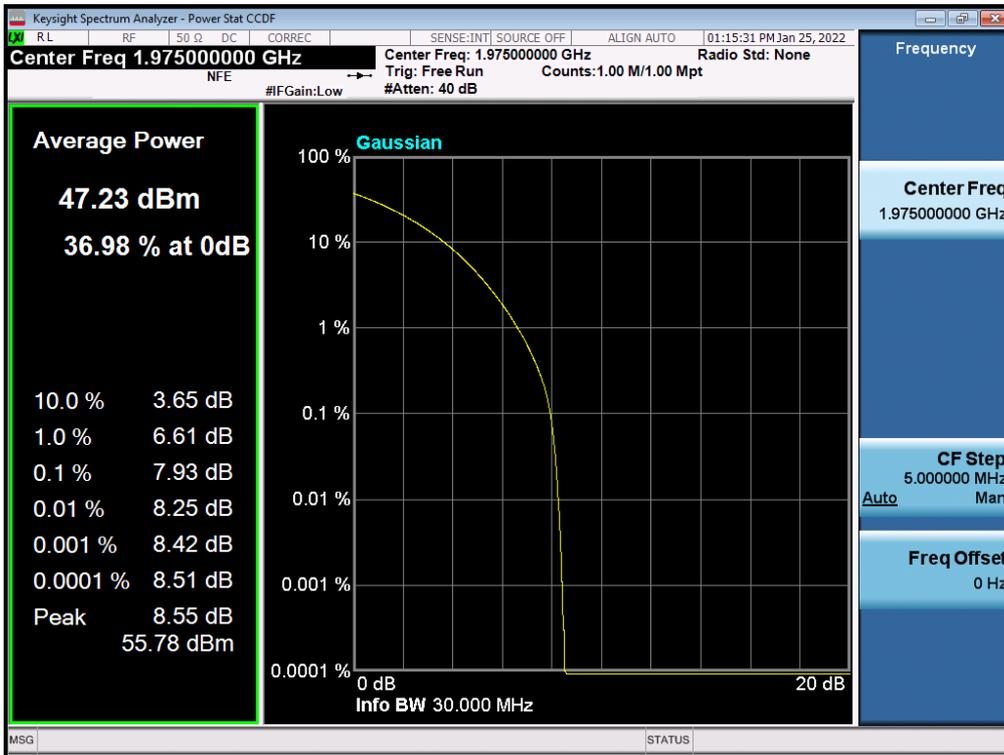
Antenna 0 / (4 Port) LTE B2 5 MHz 1 Carrier + LTE B2 5 MHz 1 Carrier + 5G NR n2 5 MHz 1 Carrier [3 Carrier] / Contiguous / 256QAM / High
