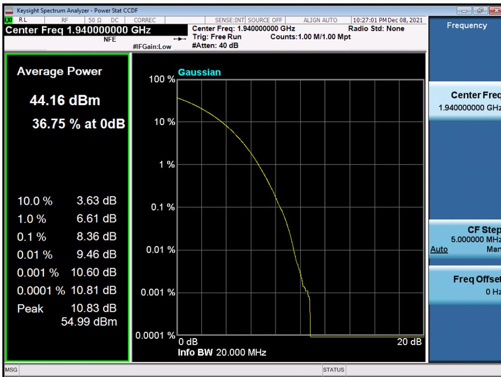
Antenna 0 / (4 Port) B2 DSS 20 MHz 9to1 1 Carrier + LTE B2 5 MHz 1 Carrier + LTE B2 5 MHz 1 Carrier [3 Carrier] (1C+2C) / Non-Contiguous / LTE B2 5 MHz + LTE B2 5 MHz / 16QAM / High
