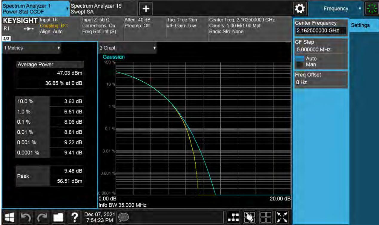
**Antenna 1 / (4 Port) B66 DSS 20 MHz 9to1 1 Carrier + LTE B66 10 MHz 1 Carrier + LTE B66 5 MHz 1 Carrier + LTE B66 5 MHz 1 Carrier [4 Carrier] (3C+1C) / Non-Contiguous / B66 DSS 20 MHz 9to1 + LTE B66 10 MHz + LTE B66 5 MHz / 16QAM / Low**
