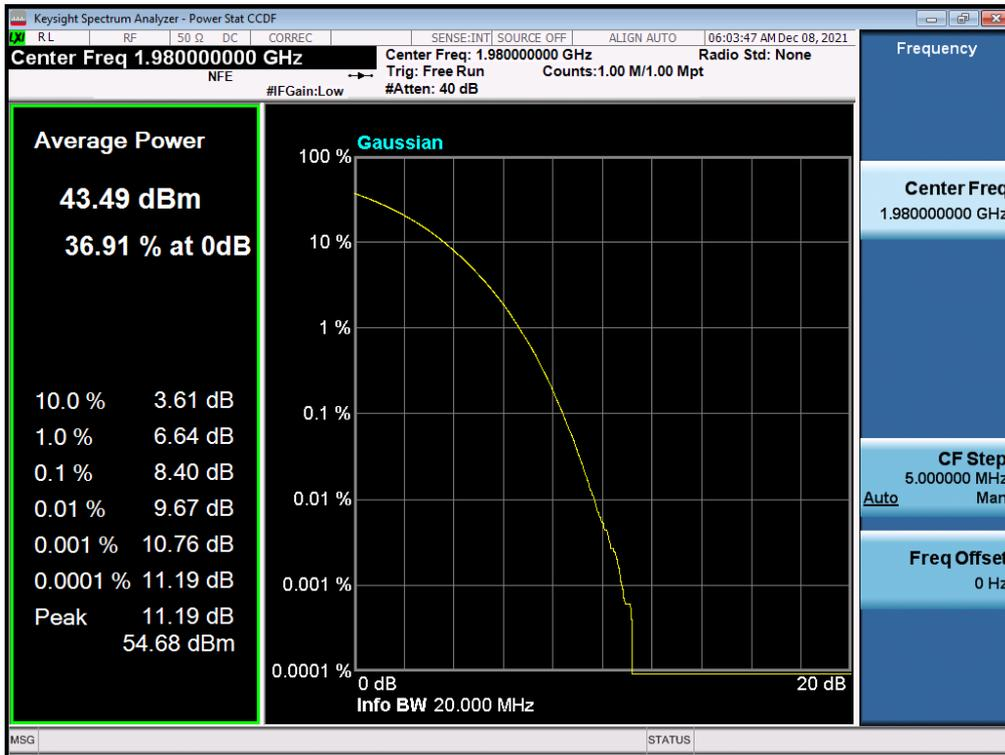
Antenna 0 / (2 Port) LTE B2 5 MHz 1 Carrier + LTE B2 5 MHz 1 Carrier + 5G NR n2 5 MHz 1 Carrier [3 Carrier] (1C+2C) / Non-Contiguous / LTE B2 5 MHz / 256QAM / Low
