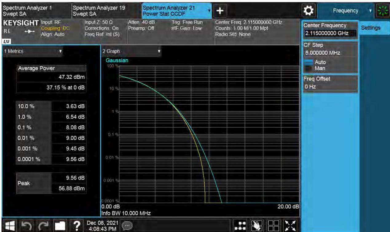
**Antenna 0 / (2 Port) B66 DSS 10 MHz 9to1 1 Carrier + LTE B66 5 MHz 1 Carrier [2 Carrier] / Non-Contiguous / LTE B66 5 MHz / 256QAM / High**
