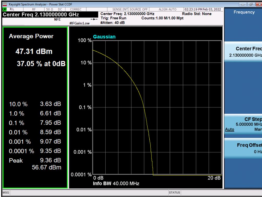
Antenna 0 / (2 Port) B2 DSS 20 MHz 9to1 1 Carrier + LTE B2 5 MHz 1 Carrier + LTE B2 5 MHz 1 Carrier [3 Carrier] / Contiguous / QPSK / High
