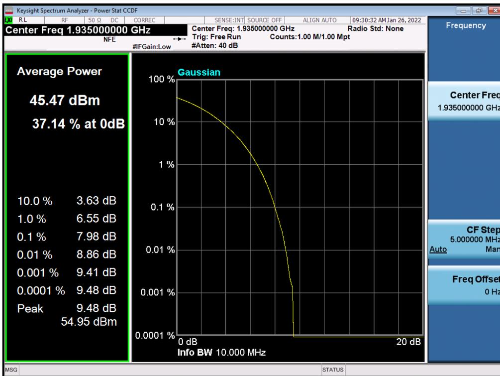
Antenna 0 / (2 Port) LTE B2 5 MHz 1 Carrier + LTE B2 5 MHz 1 Carrier + 5G NR n2 5 MHz 1 Carrier [3 Carrier] (2C+1C) / Non-Contiguous / 5G NR n2 5 MHz / 256QAM / High
