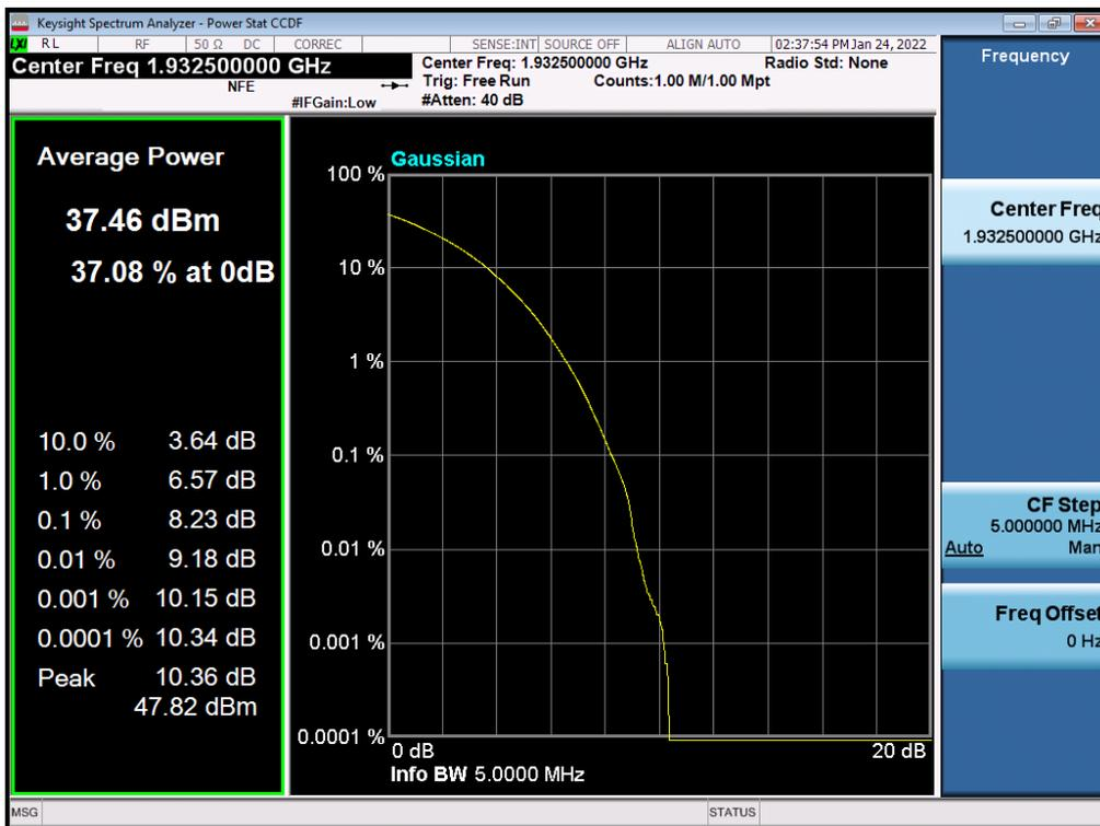
Antenna 0 / (4 Port) LTE B2 5 MHz 1 Carrier + LTE B2 5 MHz 1 Carrier + 5G NR n2 20 MHz 1 Carrier [3 Carrier] (1C+2C) / Non-Contiguous / LTE B2 5 MHz + 5G NR n2 20 MHz / 16QAM / High
