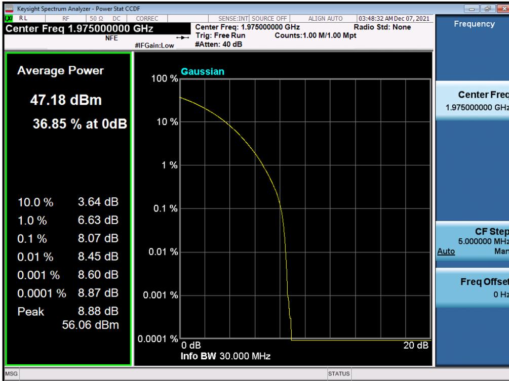
Antenna 0 / (4 Port) B2 DSS 20 MHz 9to1 1 Carrier + LTE B2 5 MHz 1 Carrier + LTE B2 5 MHz 1 Carrier [3 Carrier] / Contiguous / 16QAM / High
