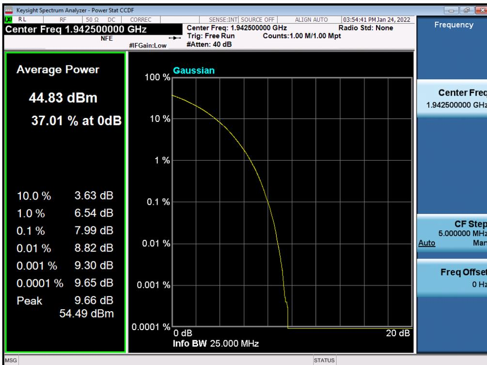
Antenna 0 / (4 Port) LTE B2 5 MHz 1 Carrier + LTE B2 5 MHz 1 Carrier + 5G NR n2 20 MHz 1 Carrier [3 Carrier] (2C+1C) / Non-Contiguous / 5G NR n2 20 MHz / 64QAM / High
