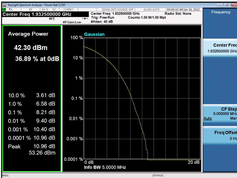
Antenna 0 / (2 Port) LTE B2 5 MHz 1 Carrier + LTE B2 5 MHz 1 Carrier + 5G NR n2 5 MHz 1 Carrier [3 Carrier] (1C+2C) / Non-Contiguous / LTE B2 5 MHz + 5G NR n2 5 MHz / 256QAM / High
