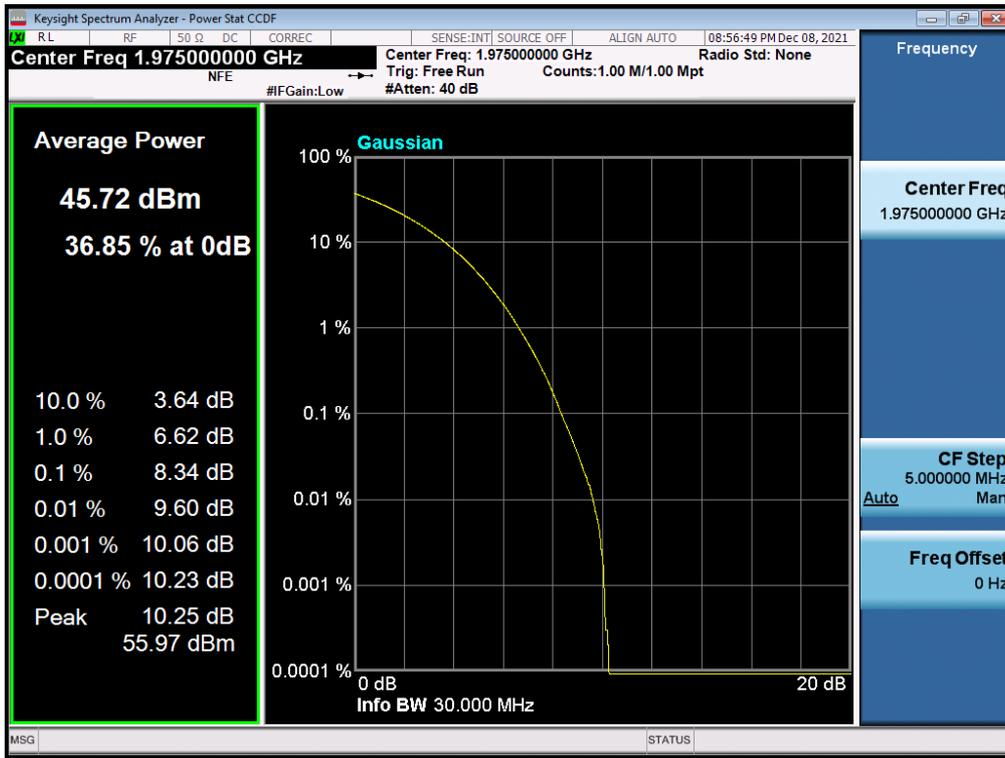
Antenna 0 / (2 Port) LTE B2 5 MHz 1 Carrier + LTE B2 5 MHz 1 Carrier + 5G NR n2 5 MHz 1 Carrier [3 Carrier] / Contiguous / 256QAM / High
