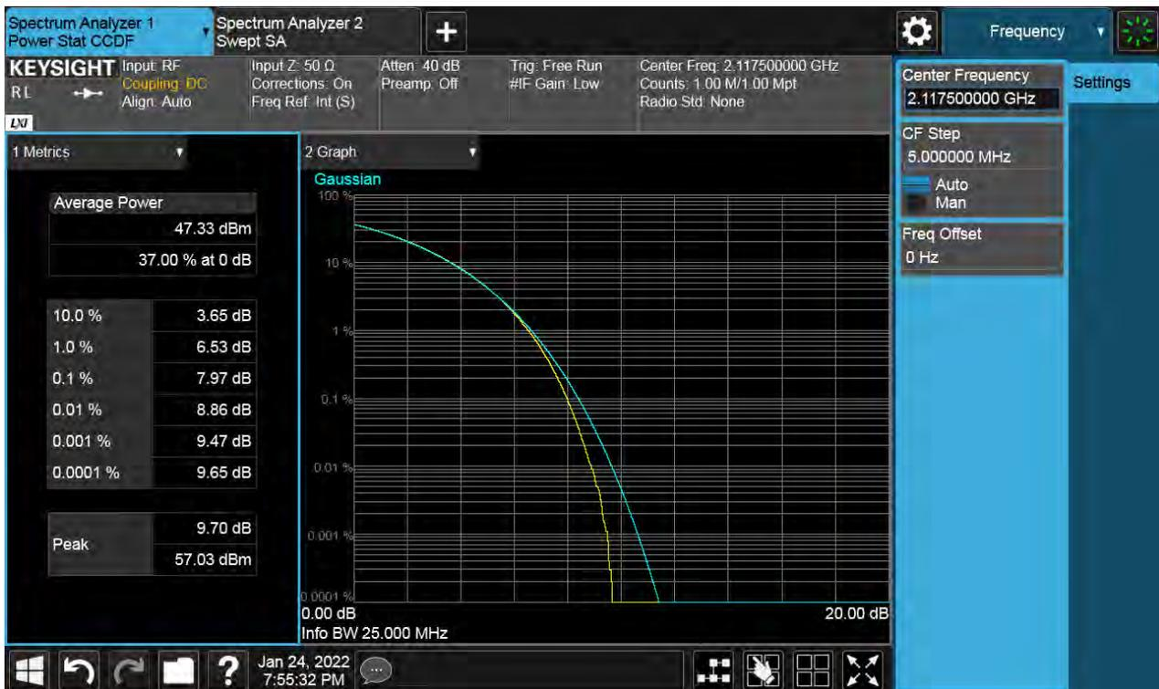
**Antenna 1 / (2 Port) LTE B66 5 MHz 1 Carrier + LTE B66 5 MHz 1 Carrier + LTE B66 5 MHz 1 Carrier + 5G NR n66 5 MHz 1 Carrier [4 Carrier] (3C+1C) / Non-Contiguous / 5G NR n66 5 MHz / 16QAM / High**
