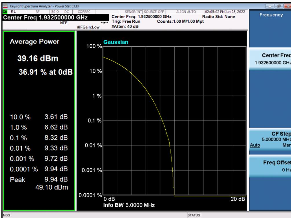
Antenna 0 / (2 Port) LTE B2 5 MHz 1 Carrier + LTE B2 5 MHz 1 Carrier + 5G NR n2 20 MHz 1 Carrier [3 Carrier] (1C+2C) / Non-Contiguous / LTE B2 5 MHz + 5G NR n2 20 MHz / QPSK / High
