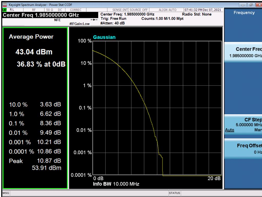
Antenna 1 / (2 Port) B2 DSS 20 MHz 9to1 1 Carrier + LTE B2 5 MHz 1 Carrier + LTE B2 5 MHz 1 Carrier [3 Carrier] (2C+1C) / Non-Contiguous / B2 DSS 20 MHz 9to1 + LTE B2 5 MHz / 256QAM / Low
