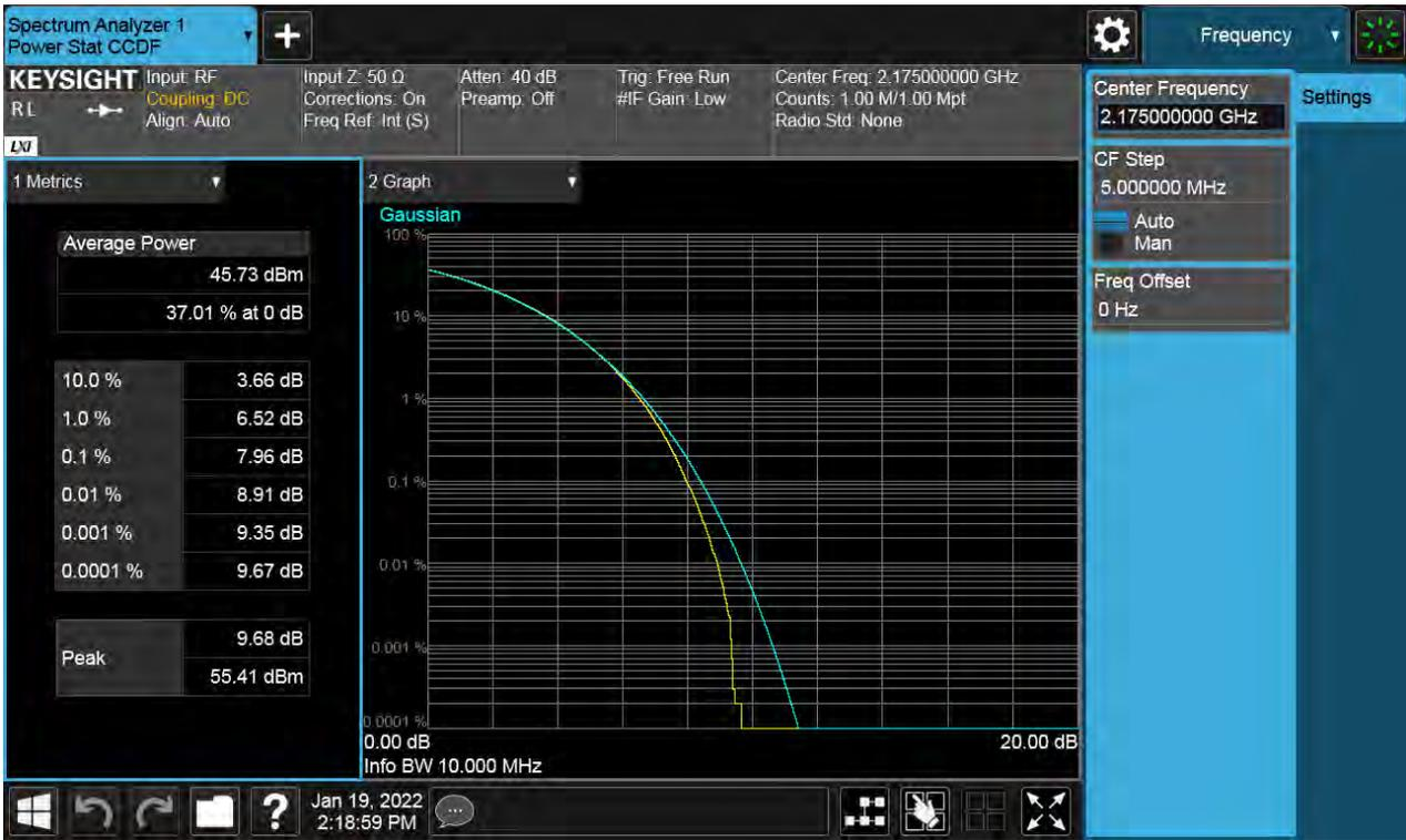
Antenna 2 / (4 Port) LTE B66 20 MHz 1 Carrier + 5G NR n66 20 MHz 1 Carrier [2 Carrier] / Non-Contiguous / LTE B66 20 MHz / 256QAM / Low
