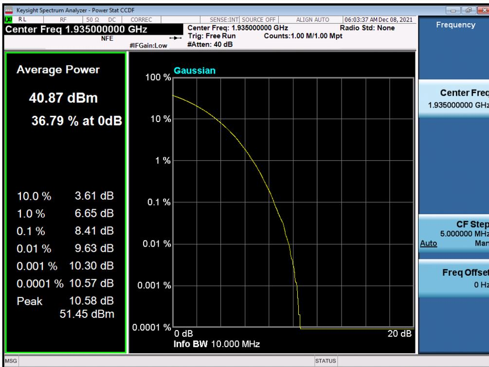
Antenna 1 / (4 Port) B2 DSS 20 MHz 9to1 1 Carrier + LTE B2 5 MHz 1 Carrier + LTE B2 5 MHz 1 Carrier [3 Carrier] (2C+1C) / Non-Contiguous / LTE B2 5 MHz / QPSK / High
