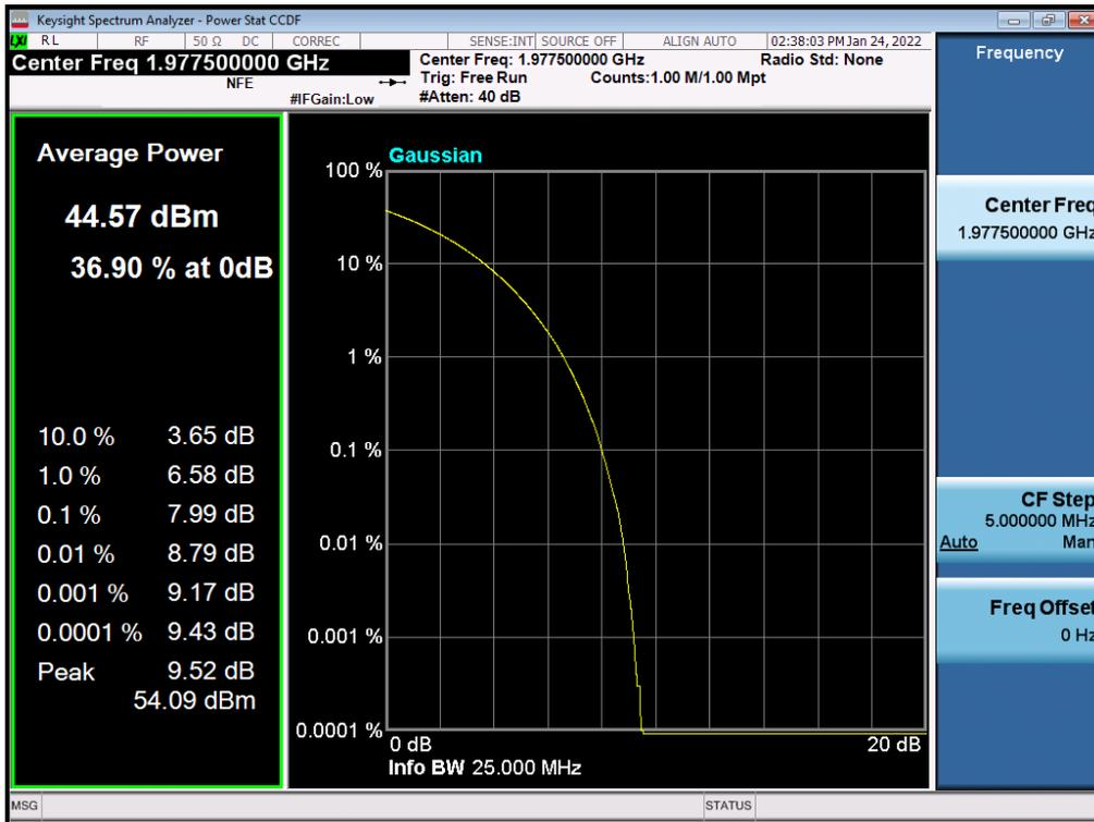
Antenna 0 / (4 Port) LTE B2 5 MHz 1 Carrier + LTE B2 5 MHz 1 Carrier + 5G NR n2 20 MHz 1 Carrier [3 Carrier] (2C+1C) / Non-Contiguous / LTE B2 5 MHz + LTE B2 5 MHz / 64QAM / Low
