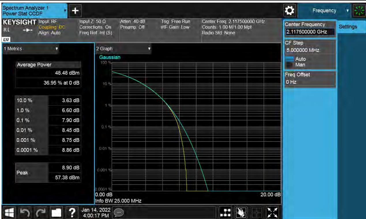
Antenna 2 / (4 Port) 5G NR n66 20 MHz 1 Carrier / QPSK / Low
