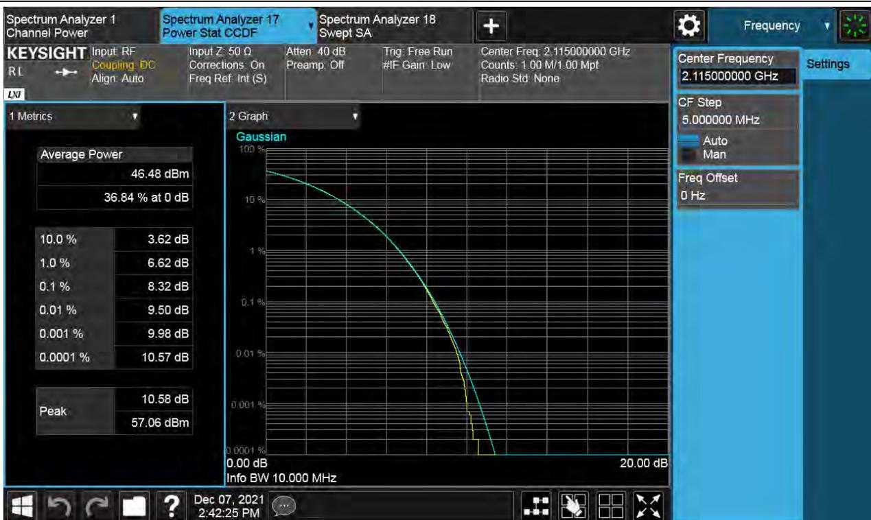
**Antenna 0 / (4 Port) B66 DSS 10 MHz 9to1 1 Carrier + LTE B66 5 MHz 1 Carrier [2 Carrier] / Non-Contiguous / LTE B66 5 MHz / 64QAM / High**
