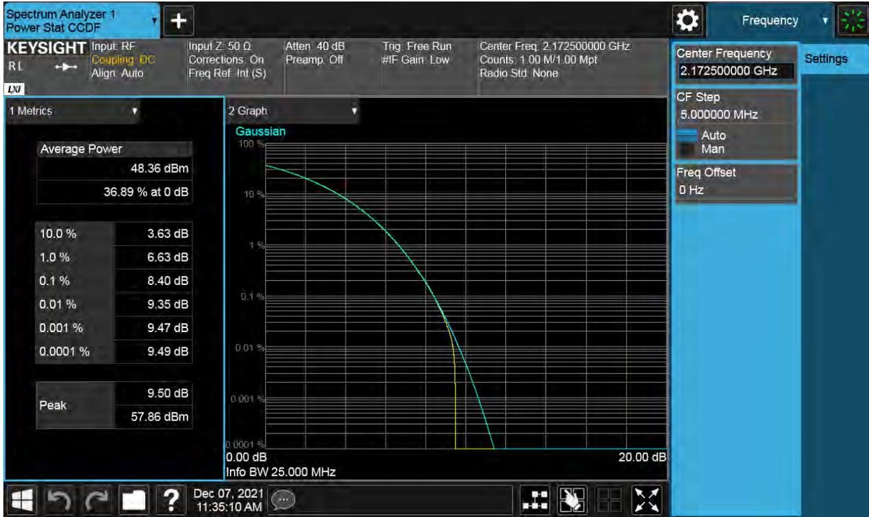
**Antenna 1 / (2 Port) LTE B66 5 MHz 1 Carrier + 5G NR n66 5 MHz 1 Carrier [2 Carrier] / Contiguous / 64QAM / High**
