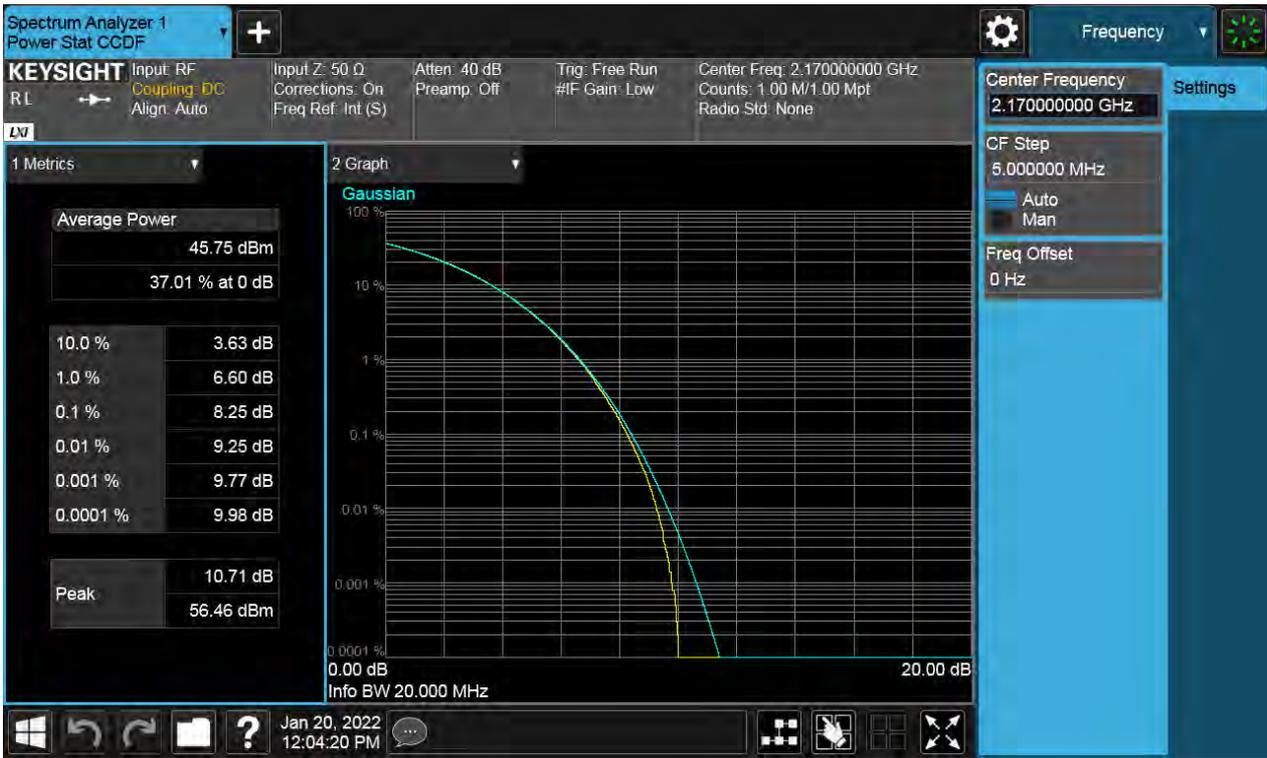
**Antenna 1 / (4 Port) LTE B66 5 MHz 1 Carrier + 5G NR n66 10 MHz 1 Carrier [2 Carrier] / Non-Contiguous / LTE B66 5 MHz / 16QAM / Low**
