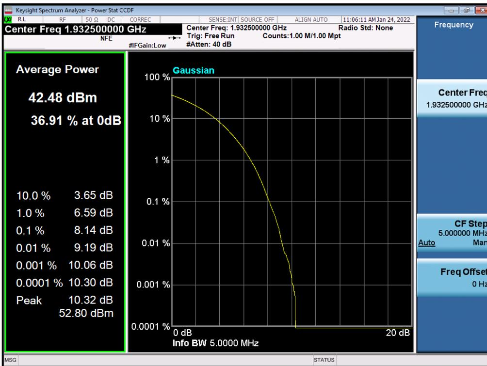
Antenna 0 / (4 Port) LTE B2 5 MHz 1 Carrier + 5G NR n2 5 MHz 1 Carrier [2 Carrier] / Non-Contiguous / 5G NR n2 5 MHz / 64QAM / High
