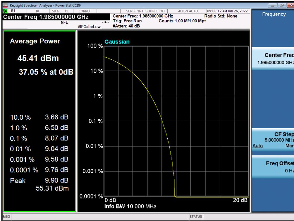
Antenna 0 / (2 Port) LTE B2 5 MHz 1 Carrier + LTE B2 5 MHz 1 Carrier + 5G NR n2 5 MHz 1 Carrier [3 Carrier] (2C+1C) / Non-Contiguous / LTE B2 5 MHz + LTE B2 5 MHz / 256QAM / Low
