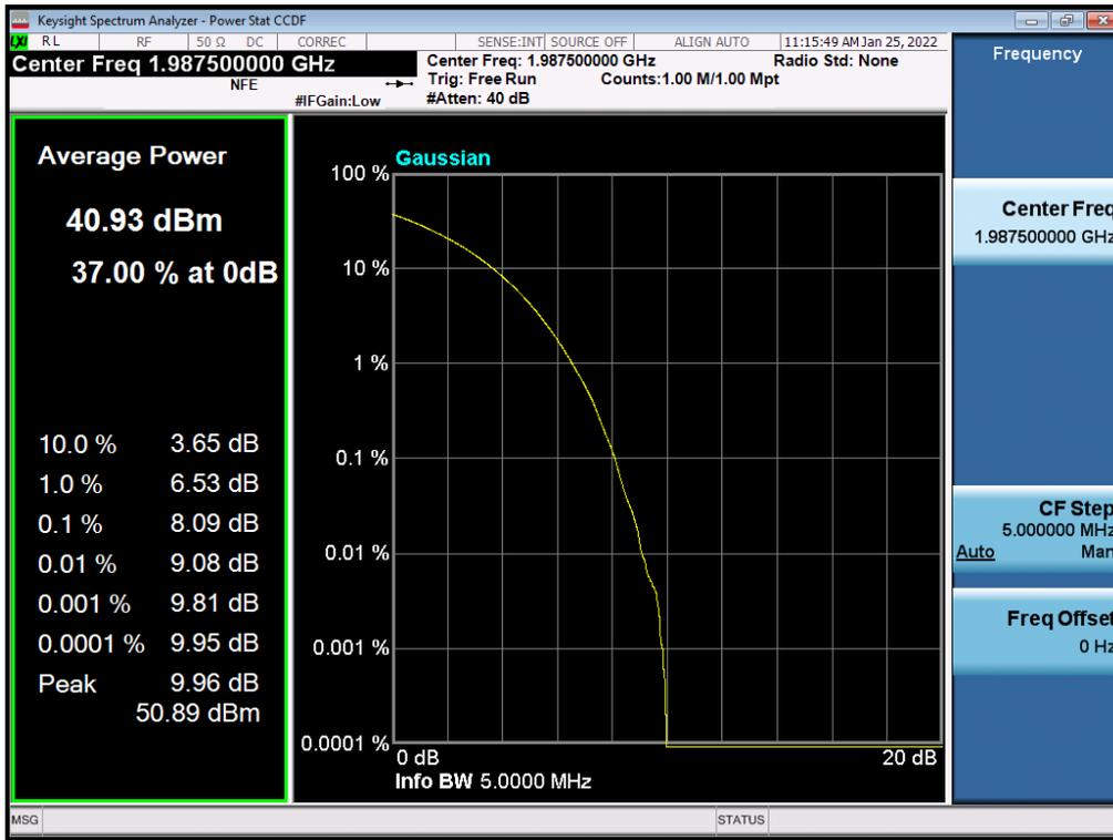
Antenna 0 / (4 Port) LTE B2 5 MHz 1 Carrier + LTE B2 5 MHz 1 Carrier + 5G NR n2 20 MHz 1 Carrier [3 Carrier] (1C+2C) / Non-Contiguous / LTE B2 5 MHz / 16QAM / Low
