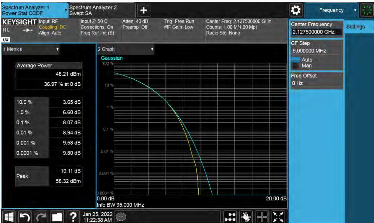
**Antenna 1 / (2 Port) LTE B66 5 MHz 1 Carrier + LTE B66 5 MHz 1 Carrier + LTE B66 10 MHz 1 Carrier + 5G NR n66 20 MHz 1 Carrier [4 Carrier] (3C+1C) / Non-Contiguous / 5G NR n66 20 MHz / QPSK / High**
