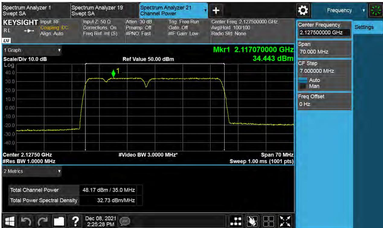
**Antenna 1 / (2 Port) B66 DSS 20 MHz 9to1 1 Carrier + LTE B66 10 MHz 1 Carrier + LTE B66 5 MHz 1 Carrier + LTE B66 5 MHz 1 Carrier [4 Carrier] (3C+1C) / Non-Contiguous / LTE B66 5 MHz / 16QAM / High**
