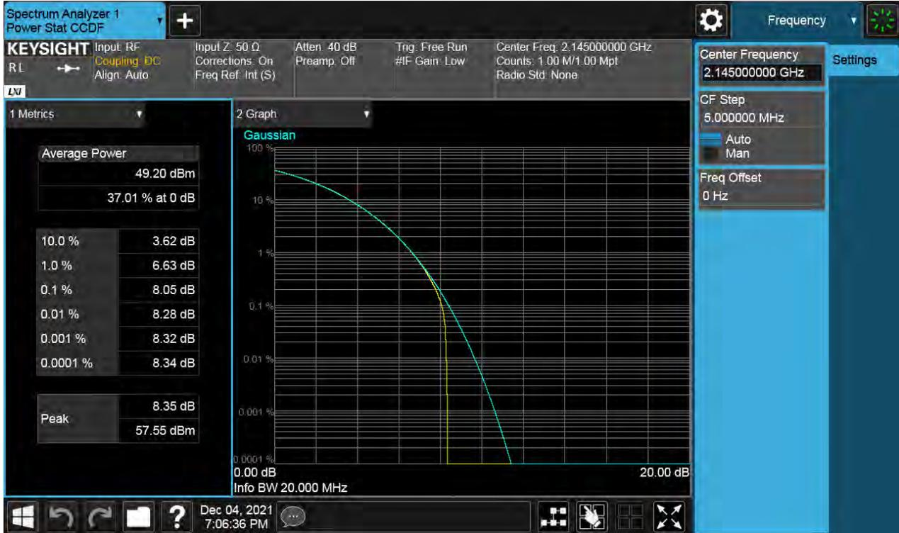
**Antenna 0 / (2 Port) B66 DSS 20 MHz 9to1 1 Carrier / QPSK / Middle**
