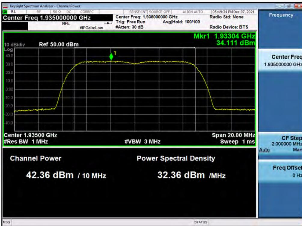
Antenna 1 / (2 Port) B2 DSS 20 MHz 9to1 1 Carrier + LTE B2 5 MHz 1 Carrier + LTE B2 5 MHz 1 Carrier [3 Carrier] (2C+1C) / Non-Contiguous / LTE B2 5 MHz / 256QAM / High
