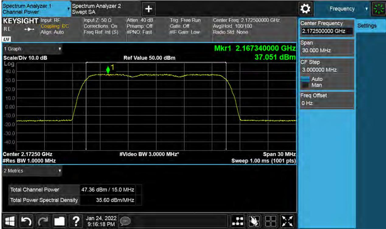
**Antenna 1 / (2 Port) LTE B66 5 MHz 1 Carrier + LTE B66 5 MHz 1 Carrier + LTE B66 5 MHz 1 Carrier + 5G NR n66 5 MHz 1 Carrier [4 Carrier] (3C+1C) / Non-Contiguous / LTE B66 5 MHz + LTE B66 5 MHz + LTE B66 5 MHz / 16QAM / Low**
