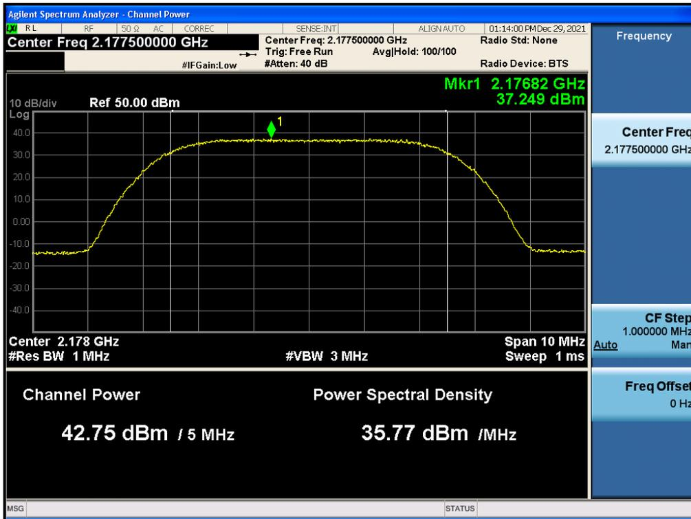
**Antenna 1 / (2 Port) LTE B66 5 MHz 1 Carrier + 5G NR n66 5 MHz 1 Carrier [2 Carrier] / Non-Contiguous / LTE B66 5 MHz / 64QAM / Low**
