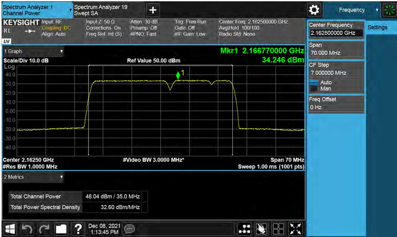
Antenna 1 / (2 Port) B66 DSS 20 MHz 9to1 1 Carrier + LTE B66 10 MHz 1 Carrier + LTE B66 5 MHz 1 Carrier + LTE B66 5 MHz 1 Carrier [4 Carrier] (3C+1C) / Non-Contiguous / B66 DSS 20 MHz 9to1 + LTE B66 10 MHz + LTE B66 5 MHz / 16QAM / Low
