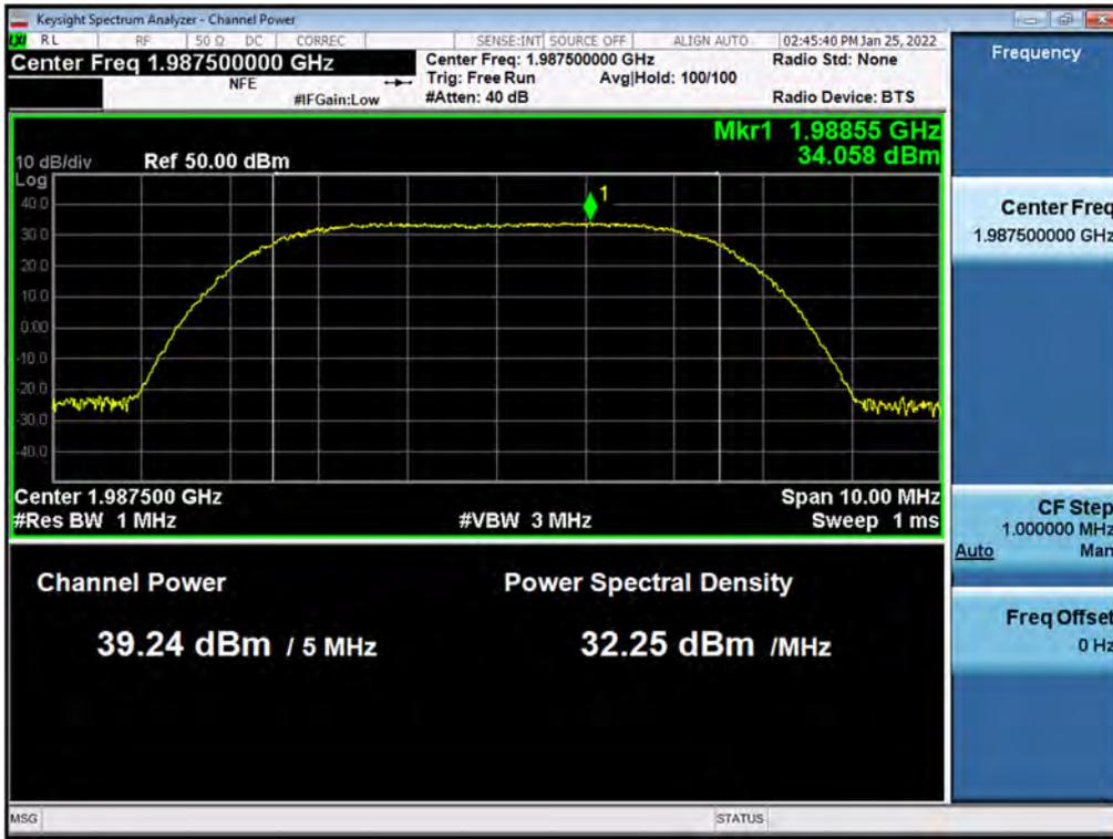
Antenna 0 / (4 Port) LTE B2 5 MHz 1 Carrier + LTE B2 5 MHz 1 Carrier + 5G NR n2 5 MHz 1 Carrier [3 Carrier] (1C+2C) / Non-Contiguous / LTE B2 5 MHz / QPSK / Low
