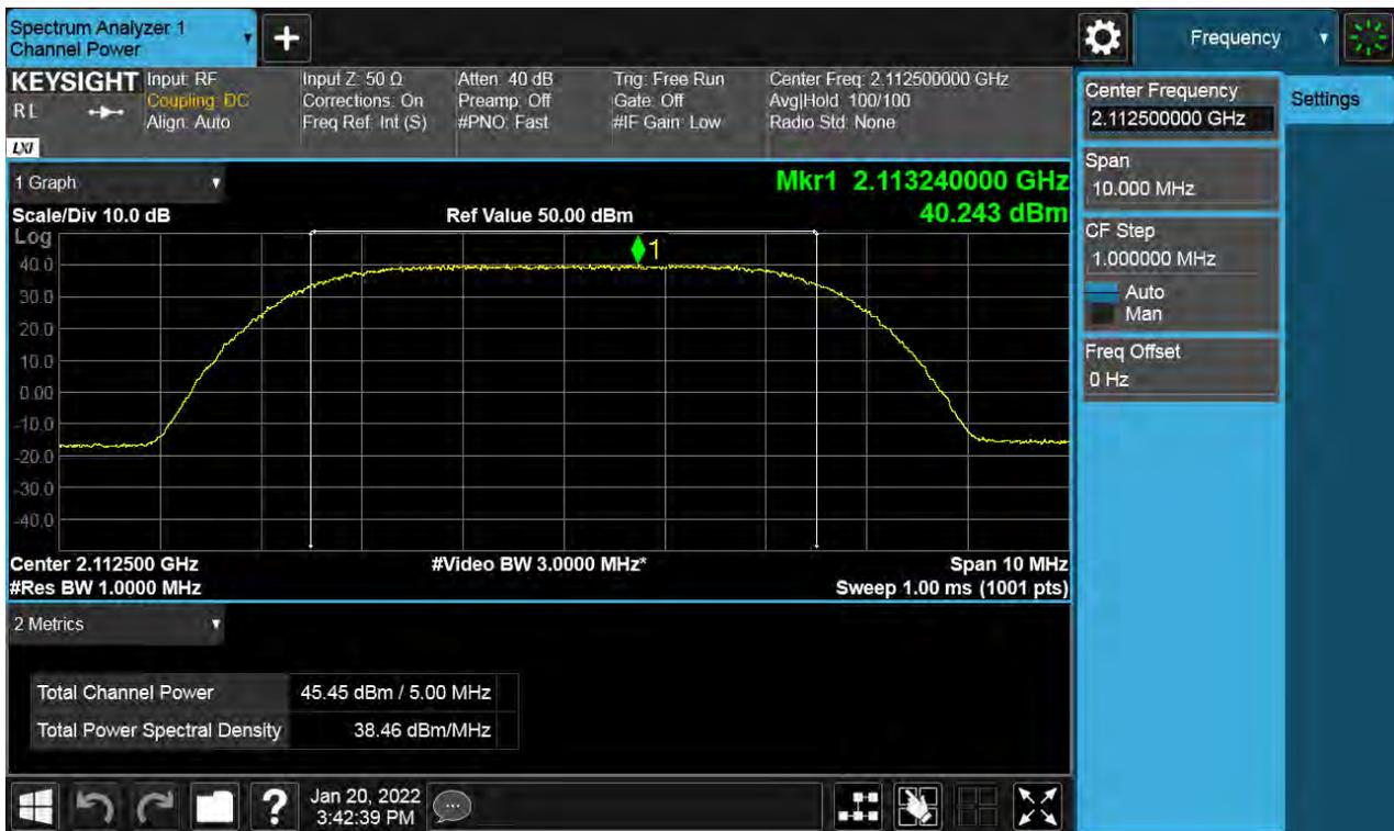
**Antenna 1 / (2 Port) LTE B66 5 MHz 1 Carrier + 5G NR n66 5 MHz 1 Carrier [2 Carrier] / Non-Contiguous / 5G NR n66 5 MHz / 64QAM / High**
