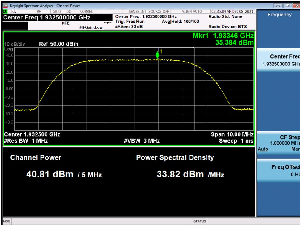
Antenna 1 / (4 Port) B2 DSS 10 MHz 9to1 1 Carrier + LTE B2 5 MHz 1 Carrier [2 Carrier] / Non-Contiguous / LTE B2 5 MHz / 256QAM / High
