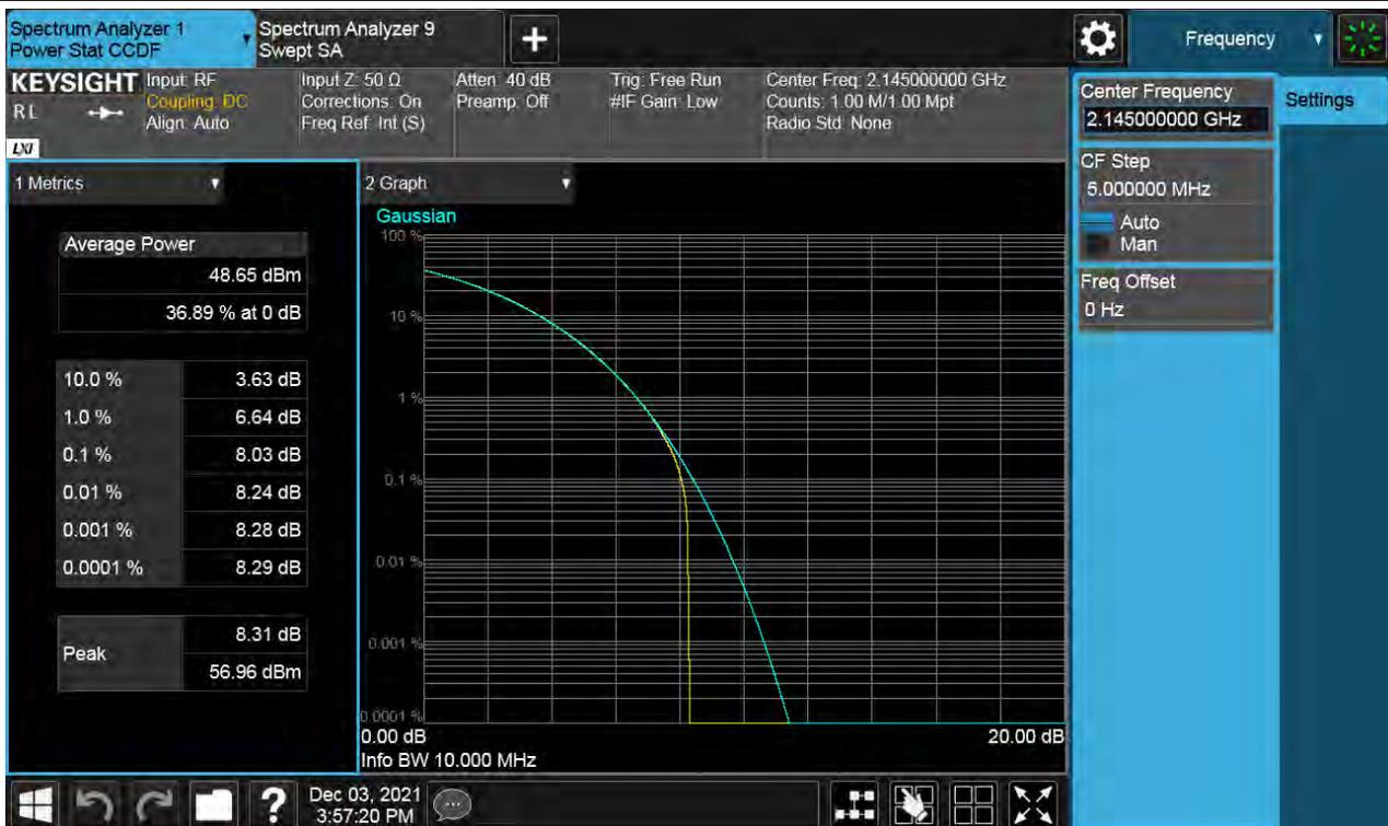
Antenna 0 / (2 Port) B66 DSS 15 MHz 2to8 1 Carrier / QPSK / Middle
