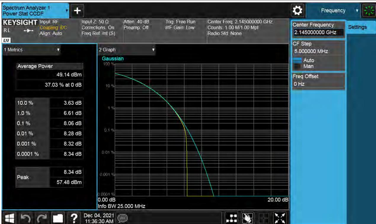
Antenna 0 / (2 Port) B66 DSS 15 MHz 9to1 1 Carrier / QPSK / Middle
