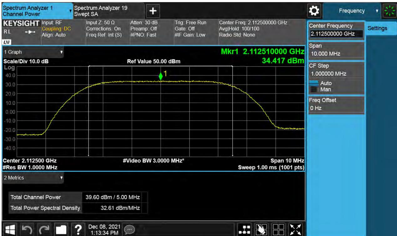
Antenna 1 / (2 Port) B66 DSS 20 MHz 9to1 1 Carrier + LTE B66 10 MHz 1 Carrier + LTE B66 5 MHz 1 Carrier + LTE B66 5 MHz 1 Carrier [4 Carrier] (1C+3C) / Non-Contiguous / LTE B66 10 MHz + LTE B66 5 MHz + LTE B66 5 MHz / 64QAM / High
