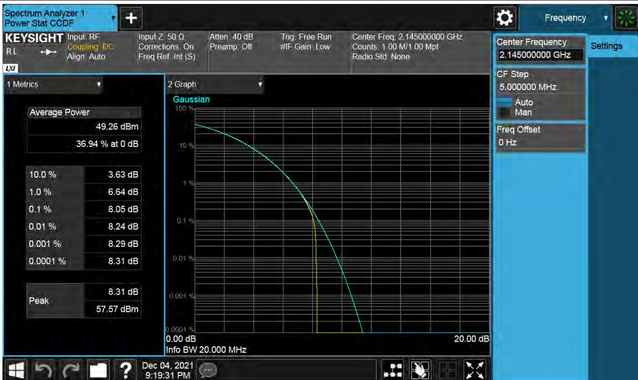
**Antenna 0 / (2 Port) B66 DSS 20 MHz 5to5 1 Carrier / QPSK / Middle**
