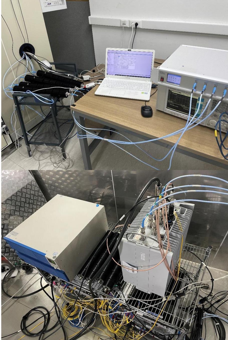
**2. Radiated Test Setup Photo(Antenna Mast : above 1 GHz Horizontal)**
