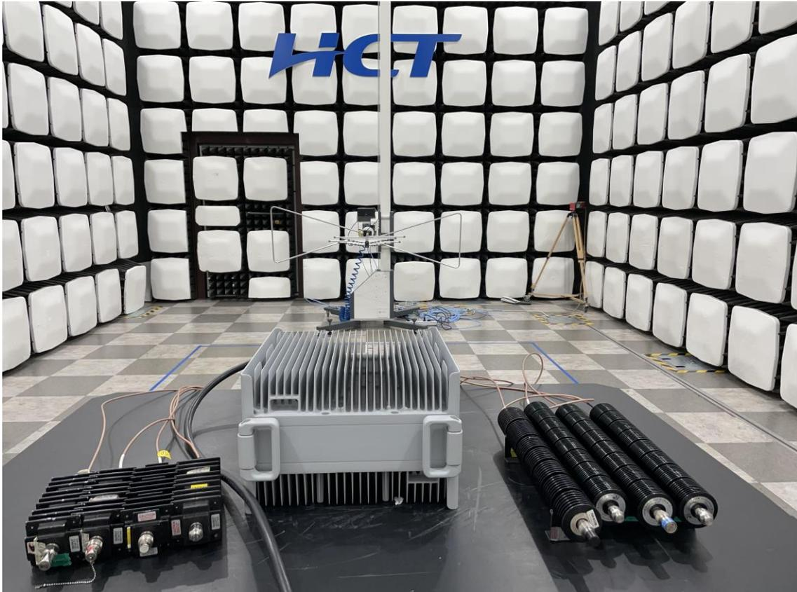
**5. Radiated Test Setup Photo(Antenna Mast : below 1 GHz Vertical)**
