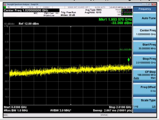
Antenna 2 / Low Edge - 100 MHz ~ Low Edge / (4 Port) LTE B66 5 MHz 1 Carrier + LTE B66 5 MHz 1 Carrier + LTE B66 10 MHz 1 Carrier + 5G NR n66 20 MHz 1 Carrier [4 Carrier] (1C+3C) / Non-Contiguous / QPSK
