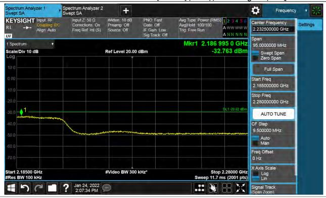
Antenna 3 / High Edge + 100 MHz ~ 10 GHz / (4 Port) LTE B66 5 MHz 1 Carrier + LTE B66 5 MHz 1 Carrier + LTE B66 5 MHz 1 Carrier + LTE B66 5 MHz 1 Carrier [4 Carrier] (1C+3C) / Non-Contiguous / QPSK
