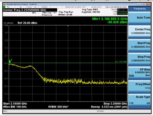
Antenna 3 / High Edge + 100 MHz ~ 10 GHz / (4 Port) LTE B66 5 MHz 1 Carrier + LTE B66 5 MHz 1 Carrier + LTE B66 10 MHz 1 Carrier + 5G NR n66 20 MHz 1 Carrier [4 Carrier] (3C+1C) / Non-Contiguous / 64QAM
