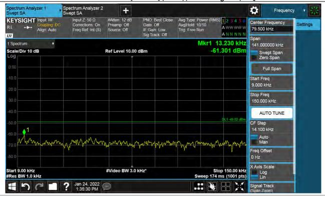
Antenna 3 / 150 kHz ~ 30 MHz / (4 Port) LTE B66 5 MHz 1 Carrier + LTE B66 5 MHz 1 Carrier + LTE B66 5 MHz 1 Carrier + 5G NR n66 5 MHz 1 Carrier [4 Carrier] (1C+3C) / Non-Contiguous / QPSK
