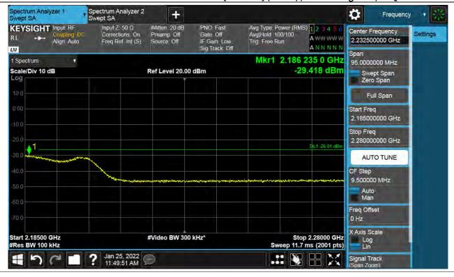
Antenna 1 / High Edge + 100 MHz ~ 10 GHz / (2 Port) LTE B66 5 MHz 1 Carrier + LTE B66 5 MHz 1 Carrier + LTE B66 10 MHz 1 Carrier + 5G NR n66 20 MHz 1 Carrier [4 Carrier] (3C+1C) / Non-Contiguous / QPSK
