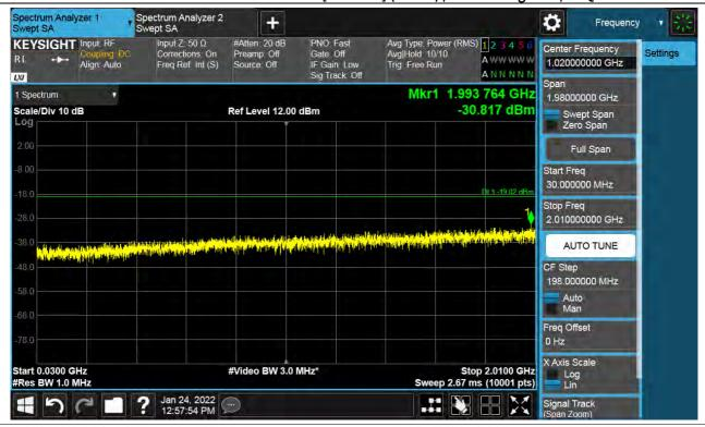
Antenna 2 / Low Edge - 100 MHz ~ Low Edge / (4 Port) LTE B66 5 MHz 1 Carrier + LTE B66 5 MHz 1 Carrier + LTE B66 5 MHz 1 Carrier + 5G NR n66 5 MHz 1 Carrier [4 Carrier] (3C+1C) / Non-Contiguous / QPSK
