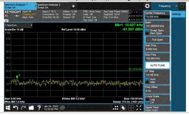
Antenna 3 / 150 kHz ~ 30 MHz / (4 Port) LTE B66 5 MHz 1 Carrier + LTE B66 5 MHz 1 Carrier + LTE B66 5 MHz 1 Carrier + 5G NR n66 5 MHz 1 Carrier [4 Carrier] (3C+1C) / Non-Contiguous / 16QAM
