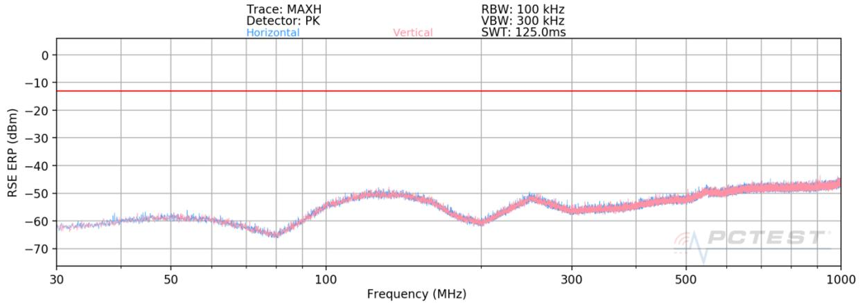
**Plot 7-1299. Radiated spurious emission\_30 MHz to 1000 MHz
