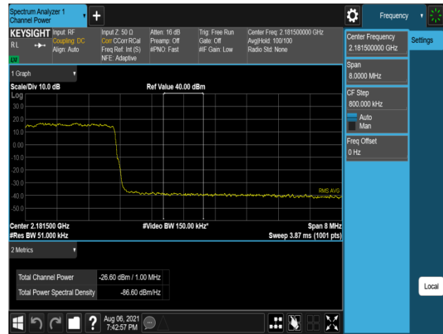
Plot 7-958. Band Edge Emission (2181MHz to 2182MHz) Plot (B66_5M+5M+5M+5M_4C_16QAM - High Channel, Port 3)
