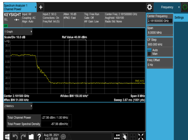
Plot 7-954. Band Edge Emission (2181MHz to 2182MHz) Plot (B66_5M+15M+20M_3C_16QAM - High Channel, Port 3)
