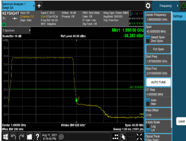
Plot 7-913. Band Edge Emission (1990MHz to 1991MHz) Plot (B2_5M+5M+20M_3C_64QAM - High Channel, Port 0)
