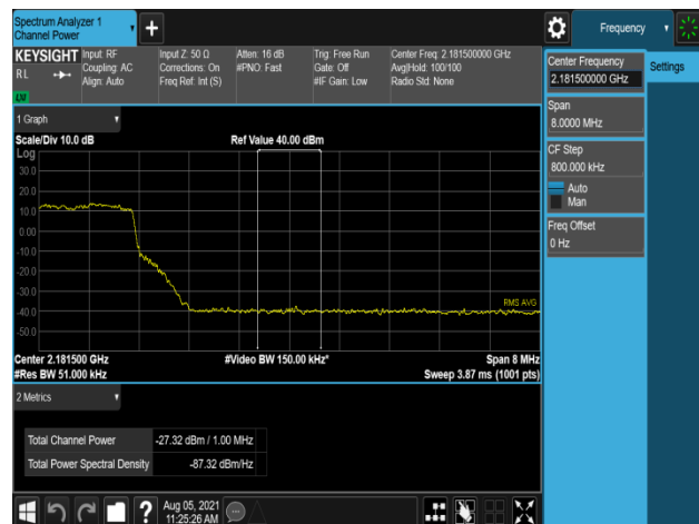
Plot 7-942. Band Edge Emission (2181MHz to 2182MHz) Plot (B66_20M+20M_2C_16QAM - High Channel, Port 3)
