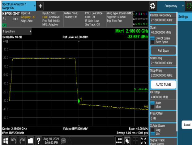
Plot 7-961. Band Edge Emission (2180MHz to 2181MHz) Plot (B66_5M+5M+5M+20M_4C_256QAM - High Channel, Port 3)
