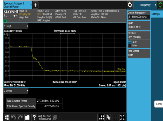
Plot 7-962. Band Edge Emission (2181MHz to 2182MHz) Plot (B66_5M+5M+5M+20M_4C_256QAM - High Channel, Port 2)
