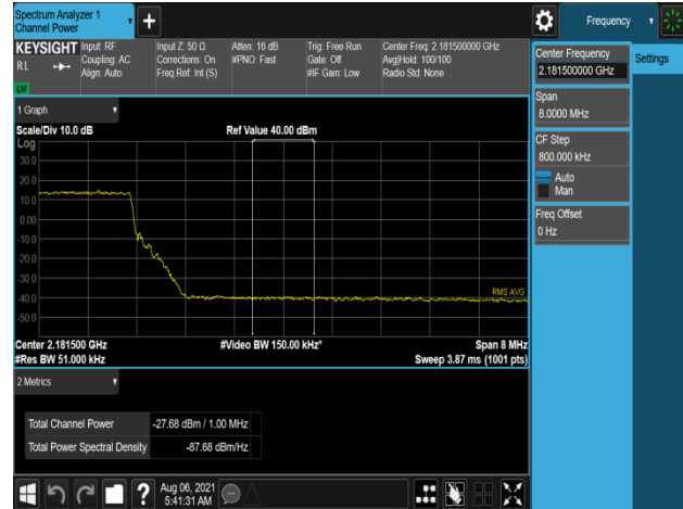
Plot 7-950. Band Edge Emission (2181MHz to 2182MHz) Plot (B66_5M+5M+20M_3C_64QAM - High Channel, Port 0)
