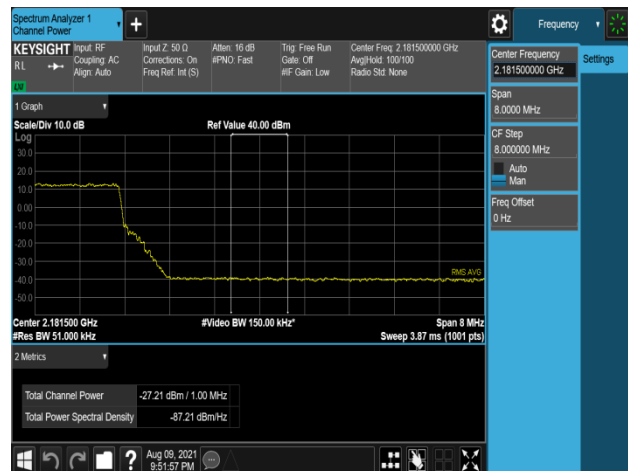
Plot 7-966. Band Edge Emission (2181MHz to 2182MHz) Plot (B66_5M+5M+10M+20M_4C_64QAM - High Channel, Port 3)
