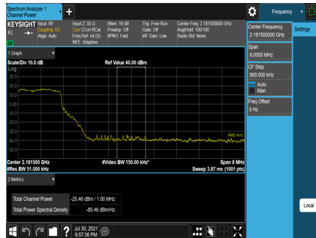
Plot 7-930. Band Edge Emission (2181MHz to 2182MHz) Plot (B66_20M_1C_16QAM - High Channel, Port 2)
