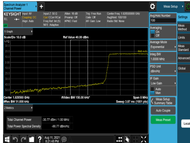
Plot 7-908. Band Edge Emission (2108MHz to 2109MHz) Plot (B2_5M+5M+5M_3C_QPSK - Low Channel, Port 3)
