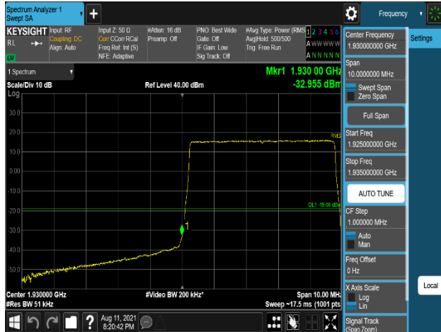
Plot 7-907. Band Edge Emission (1929MHz to 1930MHz) Plot (B2_5M+5M+5M_3C_QPSK - Low Channel, Port 3)
