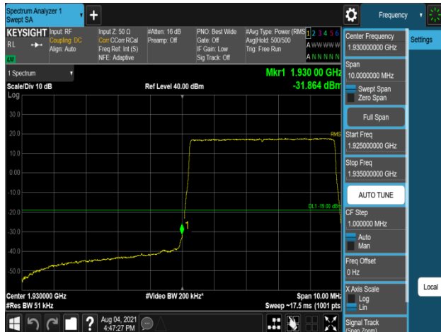
Plot 7-875. Band Edge Emission (1929MHz to 1930MHz) Plot (B2_5M+5M_2C_QPSK - Low Channel, Port 0)
