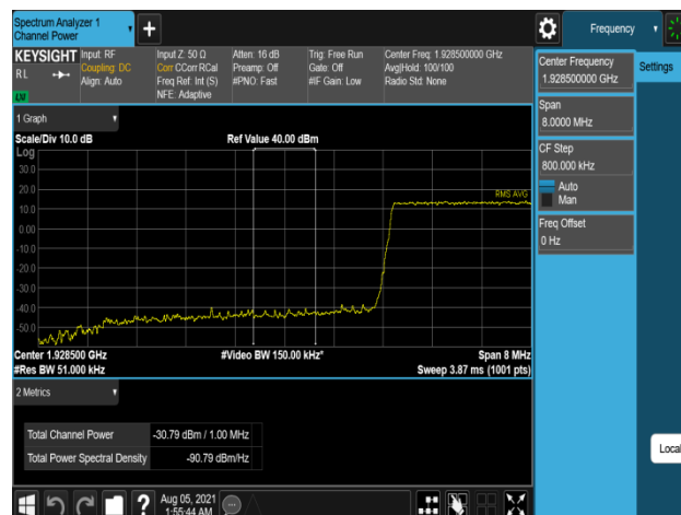
Plot 7-880. Band Edge Emission (1928MHz to 1929MHz) Plot (B2_5M+20M_2C_QPSK - Low Channel, Port 0)
