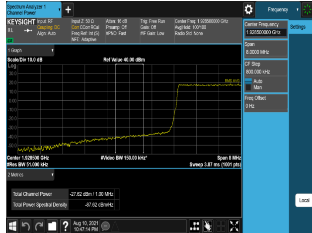
Plot 7-896. Band Edge Emission (2108MHz to 2109MHz) Plot (B2_5M+5M_2C_64QAM - Low Channel, Port 3)
