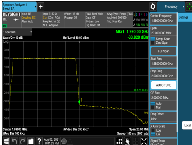
Plot 7-865. Band Edge Emission (1990MHz to 1991MHz) Plot (B2_10M_1C_64QAM - High Channel, Port 0)
