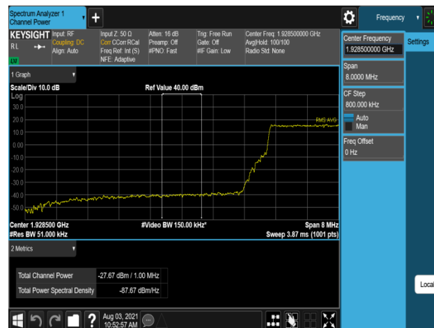
Plot 7-868. Band Edge Emission (1928MHz to 1929MHz) Plot (B2_15M_1C_64QAM - Low Channel, Port 2)
