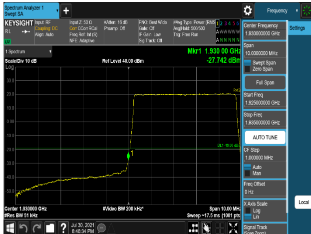
Plot 7-859. Band Edge Emission (1929MHz to 1930MHz) Plot (B2_5M_1C_QPSK - Low Channel, Port 2)
