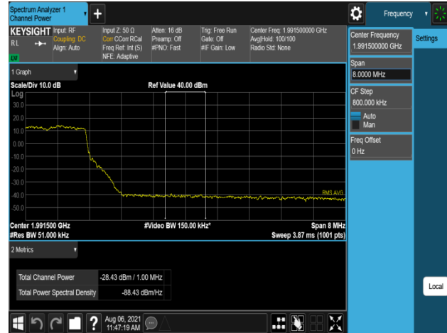
Plot 7-894. Band Edge Emission (1991MHz to 1992MHz) Plot (B2_5M+5M+20M_3C_16QAM - High Channel, Port 2)
