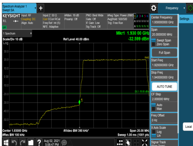
Plot 7-863. Band Edge Emission (1929MHz to 1930MHz) Plot (B2_10M_1C_64QAM - Low Channel, Port 1)
