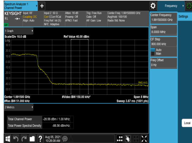
Plot 7-882. Band Edge Emission (1991MHz to 1992MHz) Plot (B2_5M+20M_2C_16QAM - High Channel, Port 1)
