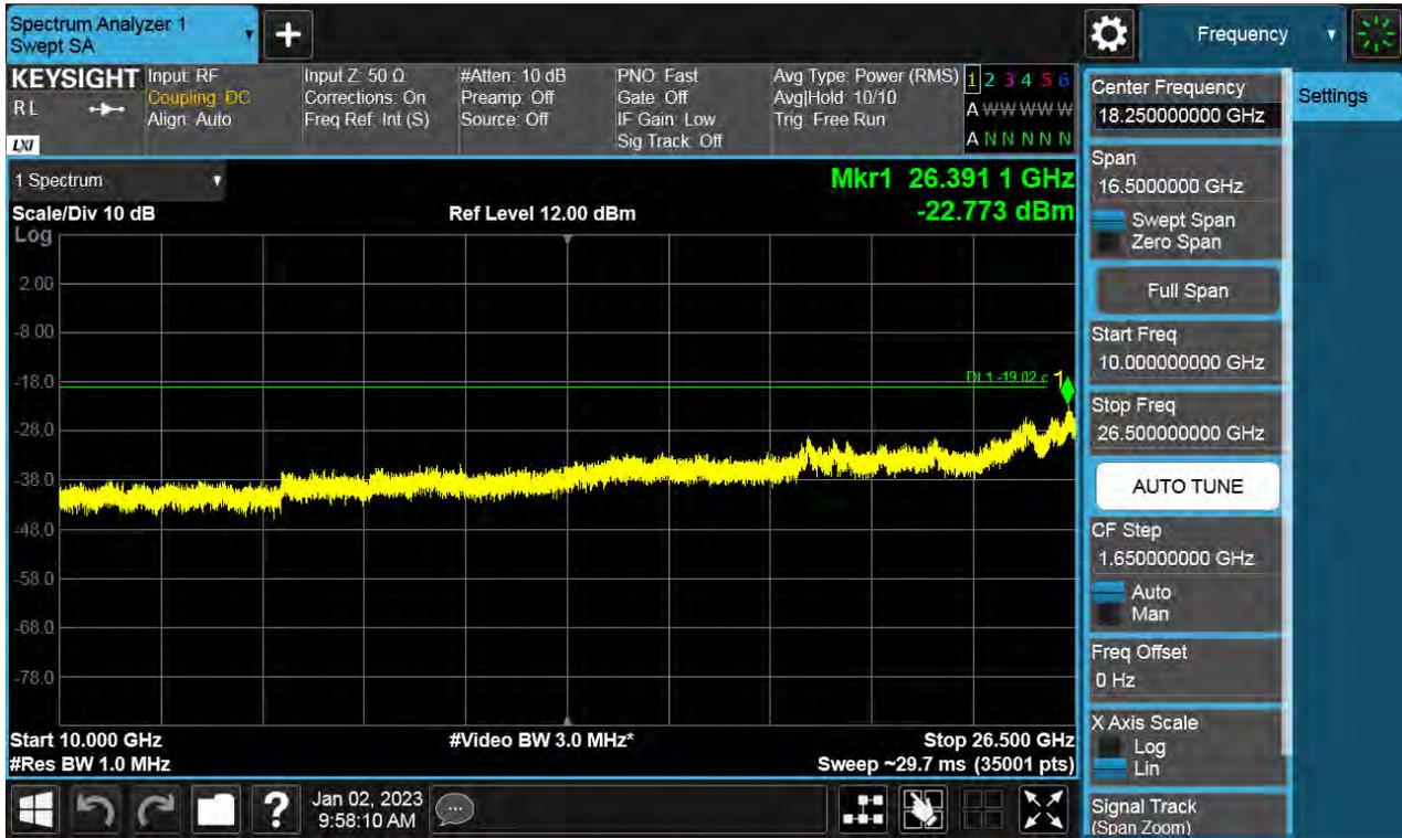
Antenna 0 / (4 Port) DSS B2 15 MHz 5t5 [1 Carrier] / 9 kHz ~ 150 kHz / 16QAM / MIDDLE
