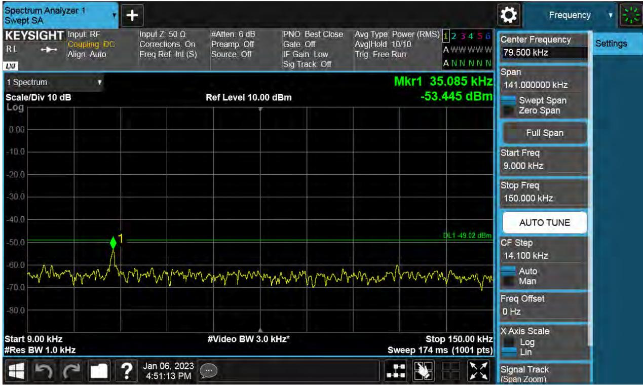
Antenna 2 / (4 Port) 5G NR n2 5 MHz 1 Carrier / 150 kHz ~ 30 MHz / 16QAM / HIGH
