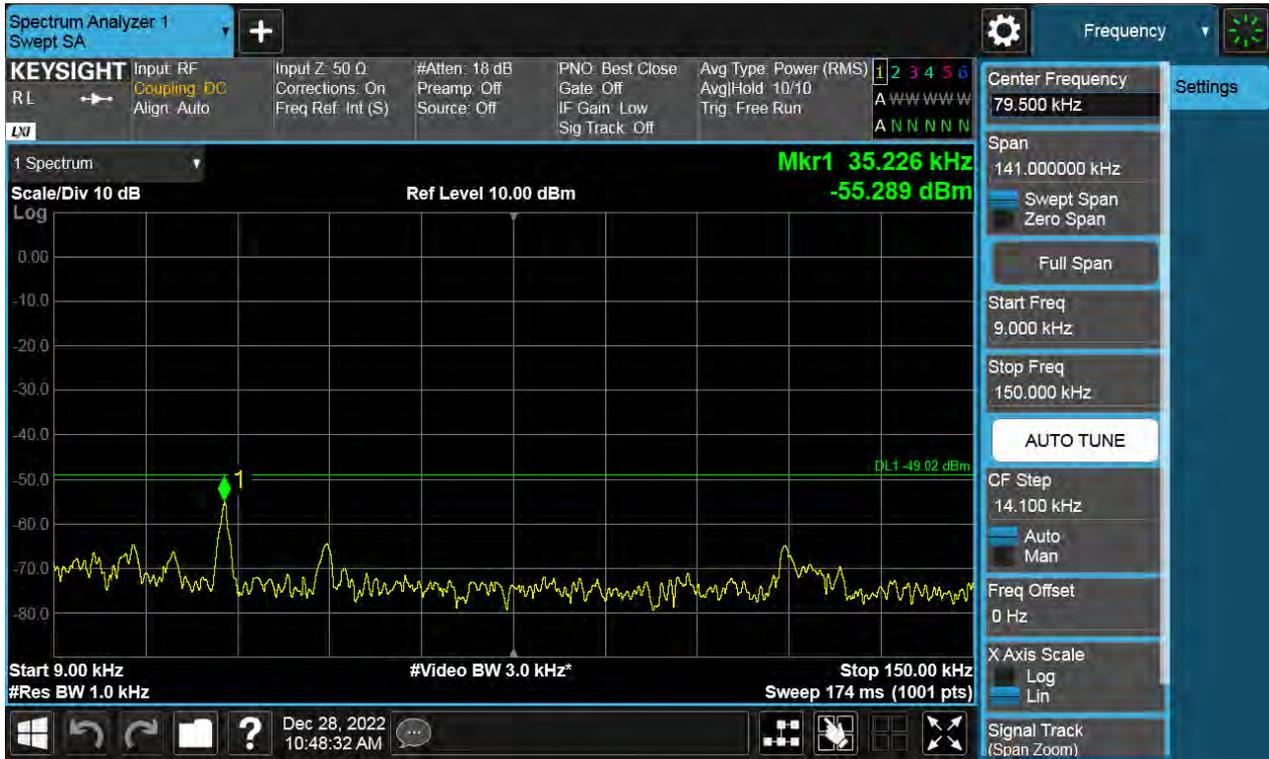
Antenna 2 / (4 Port) DSS B2 10 MHz 2t8 [1 Carrier] / 150 kHz ~ 30 MHz / 16QAM / MIDDLE
