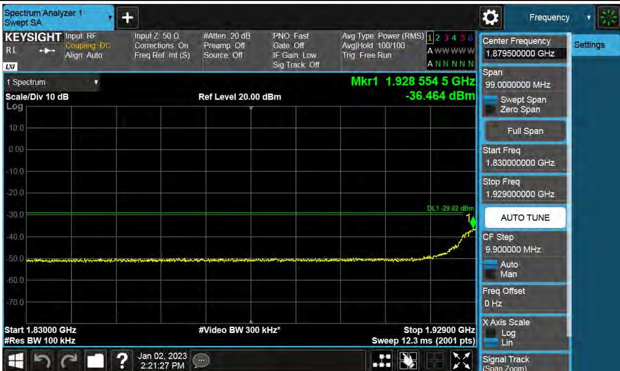
Antenna 1 / (4 Port) DSS B2 15 MHz 2t8 [1 Carrier] / High Edge ~ High Edge + 100 MHz / QPSK / HIGH
