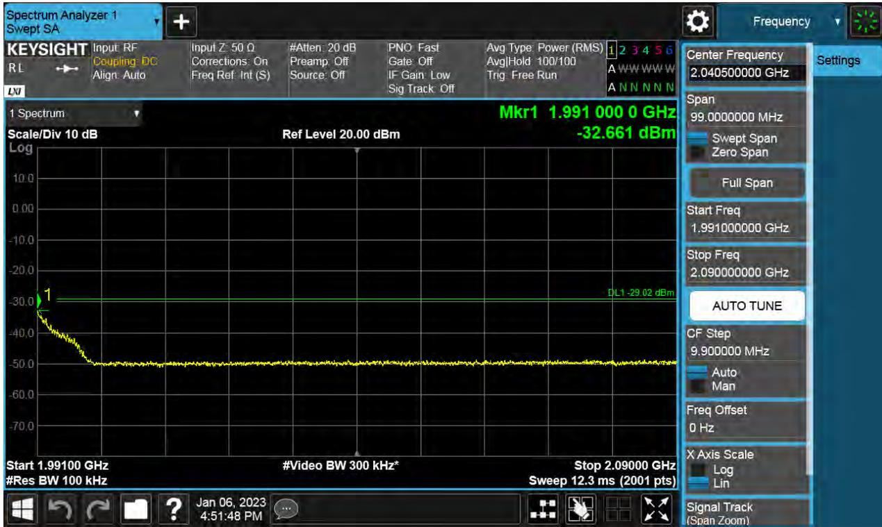
Antenna 2 / (4 Port) 5G NR n2 5 MHz 1 Carrier / High Edge + 100 MHz ~ 10 GHz / 256QAM / HIGH
