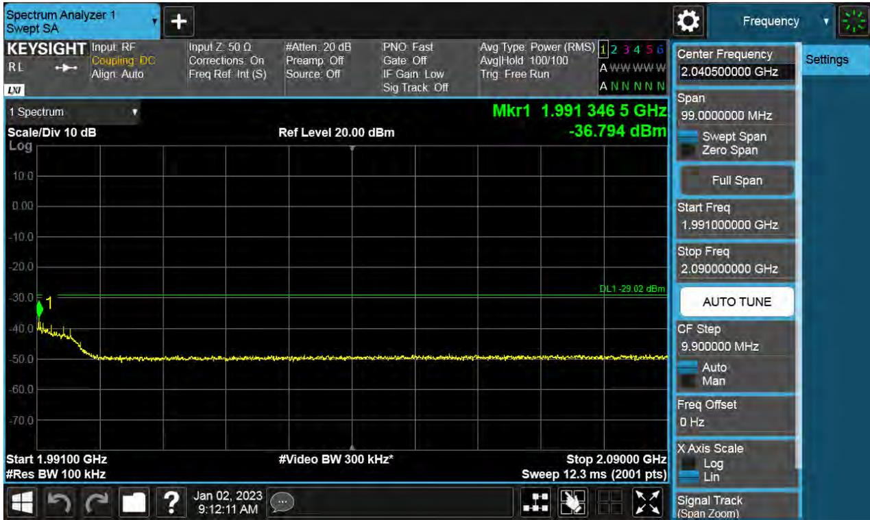
Antenna 2 / (4 Port) DSS B2 15 MHz 5t5 [1 Carrier] / High Edge + 100 MHz ~ 10 GHz / QPSK / HIGH
