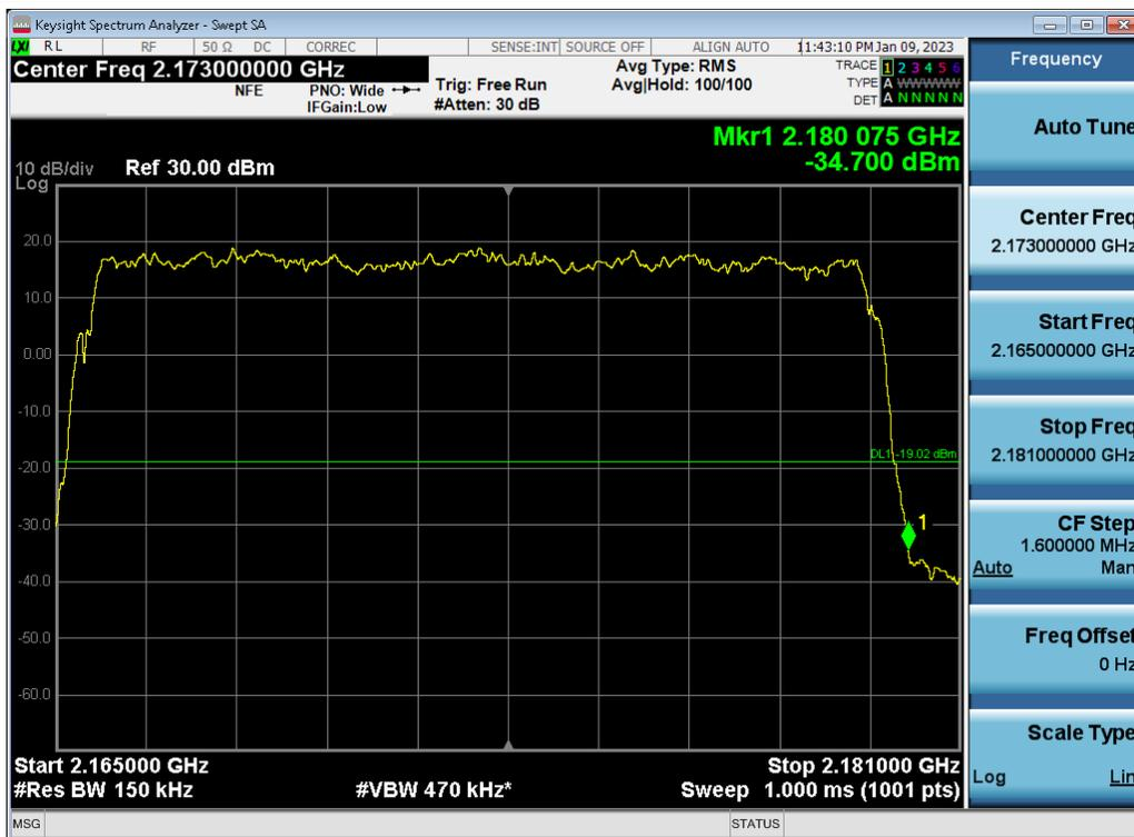
Antenna 0 / (4 Port) LTE B66 5 MHz 1 Carrier + DSS B66 10 MHz 1 Carrier + DSS B66 10 MHz 1 Carrier + DSS B66 15 MHz 1 Carrier [4 Carrier] [3C+1C] / QPSK / Low / Non-Contiguous
