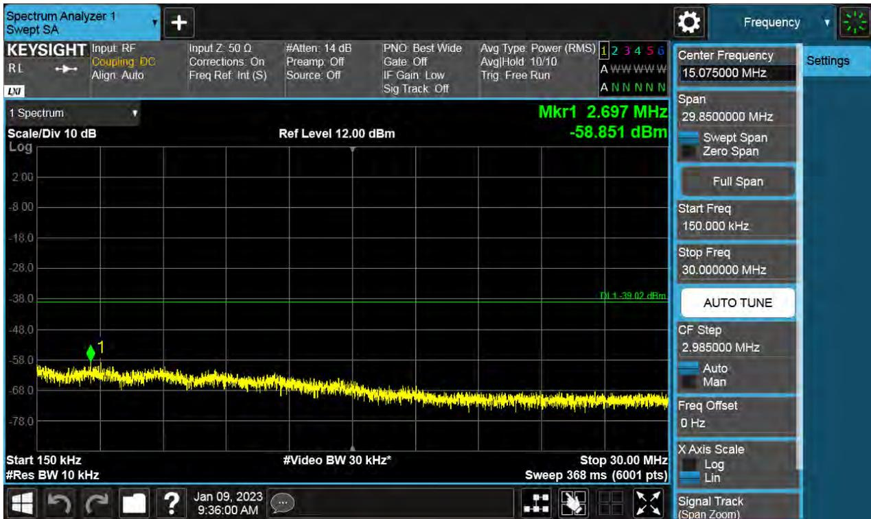
Antenna 3 / (4 Port) 5G NR n2 20 MHz 1 Carrier / 30 MHz ~ Low Edge - 100 MHz / 256QAM / LOW
