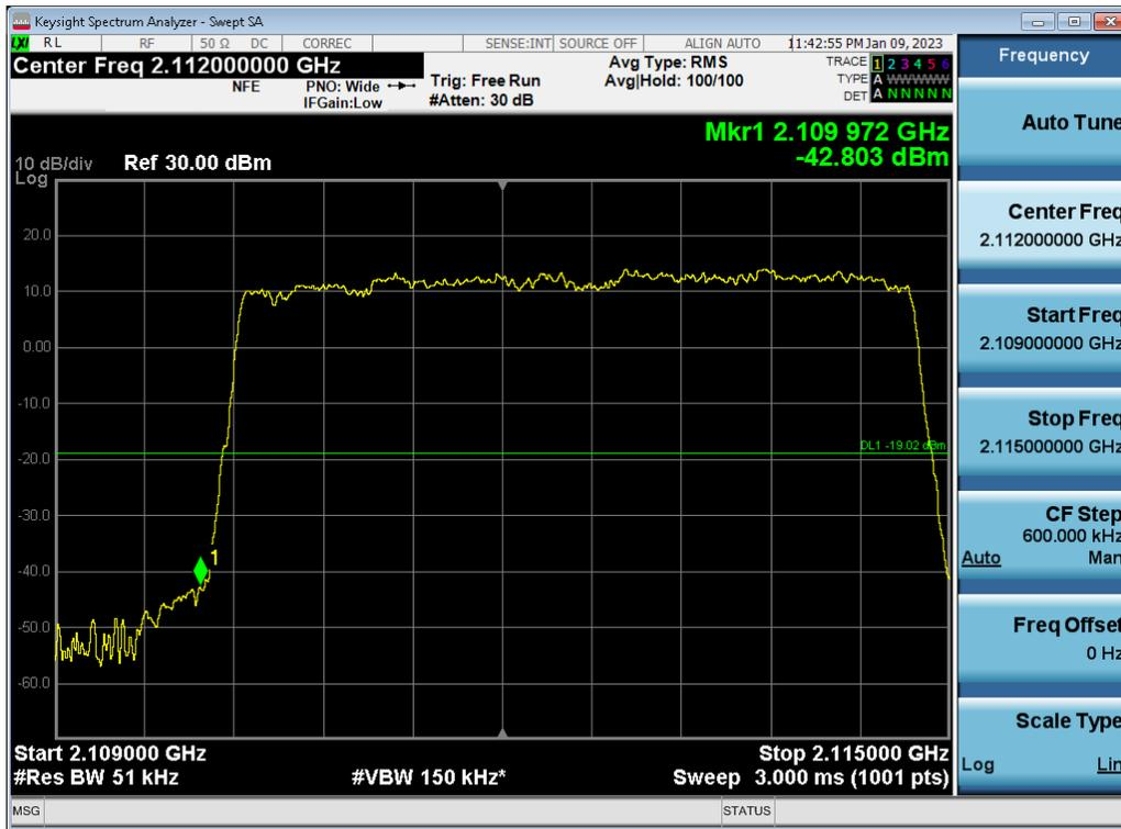
Antenna 0 / (4 Port) LTE B66 5 MHz 1 Carrier + DSS B66 10 MHz 1 Carrier + DSS B66 10 MHz 1 Carrier + DSS B66 15 MHz 1 Carrier [4 Carrier] [1C+3C] / 16QAM / High / Non-Contiguous
