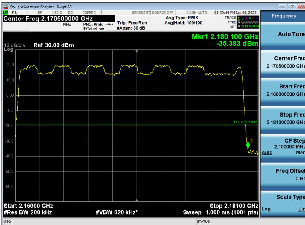
Antenna 1 / (4 Port) DSS B66 5 MHz 1 Carrier + LTE B66 5 MHz 1 Carrier + LTE B66 5 MHz 1 Carrier + LTE B66 10 MHz 1 Carrier [4 Carrier] [1C+3C] / 64QAM / Low / Non-Contiguous
