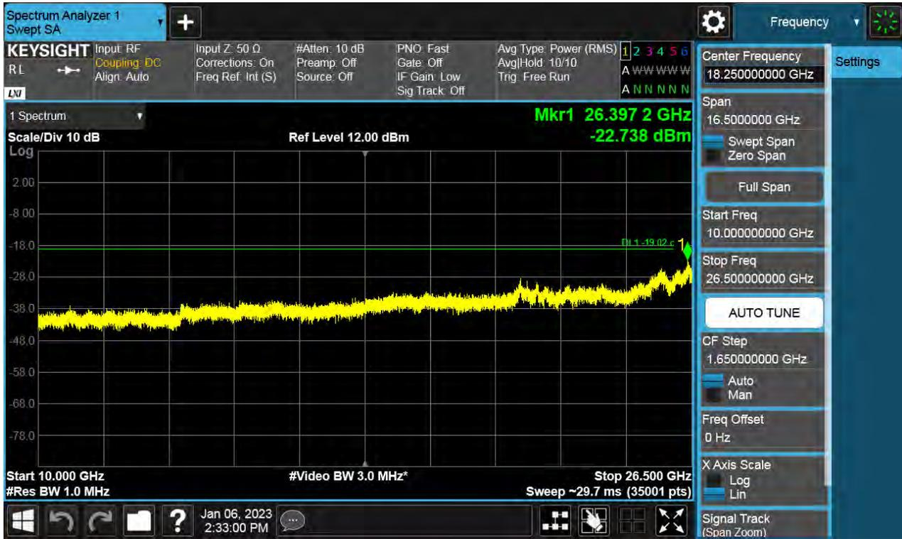
Antenna 0 / (4 Port) 5G NR n2 10 MHz 1 Carrier / 9 kHz ~ 150 kHz / 64QAM / LOW
