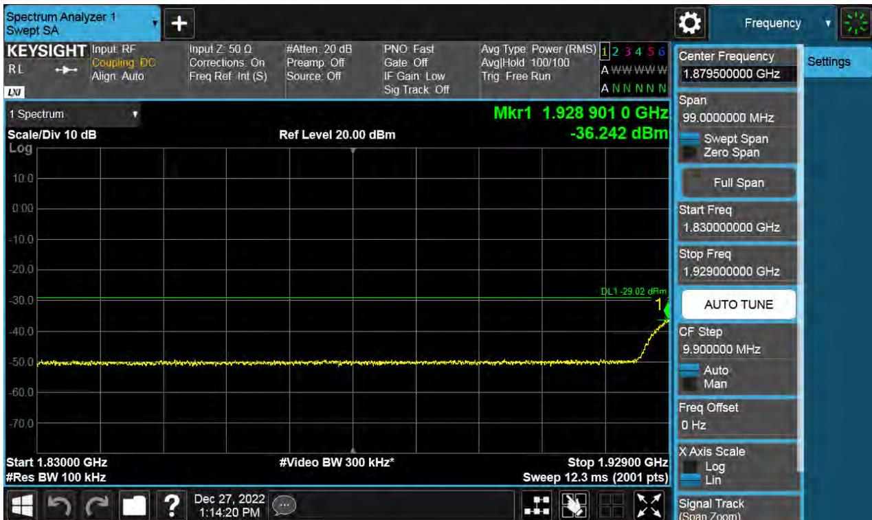
Antenna 0 / (4 Port) DSS B2 10 MHz 9t1 [1 Carrier] / High Edge ~ High Edge + 100 MHz / 16QAM / HIGH
