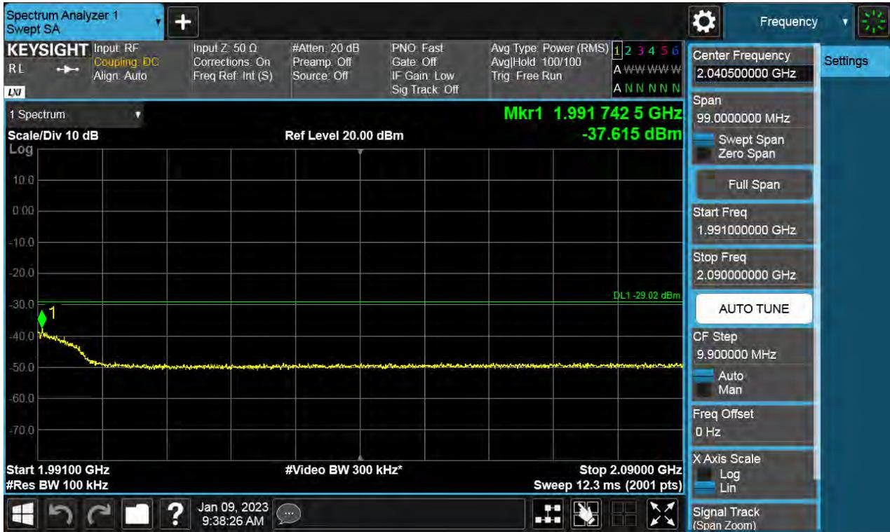
Antenna 2 / (4 Port) 5G NR n2 20 MHz 1 Carrier / High Edge + 100 MHz ~ 10 GHz / 16QAM / HIGH
