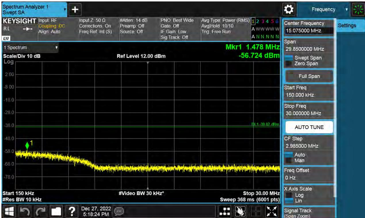
Antenna 3 / (4 Port) DSS B2 10 MHz 5t5 [1 Carrier] / 30 MHz ~ Low Edge - 100 MHz / 16QAM / HIGH
