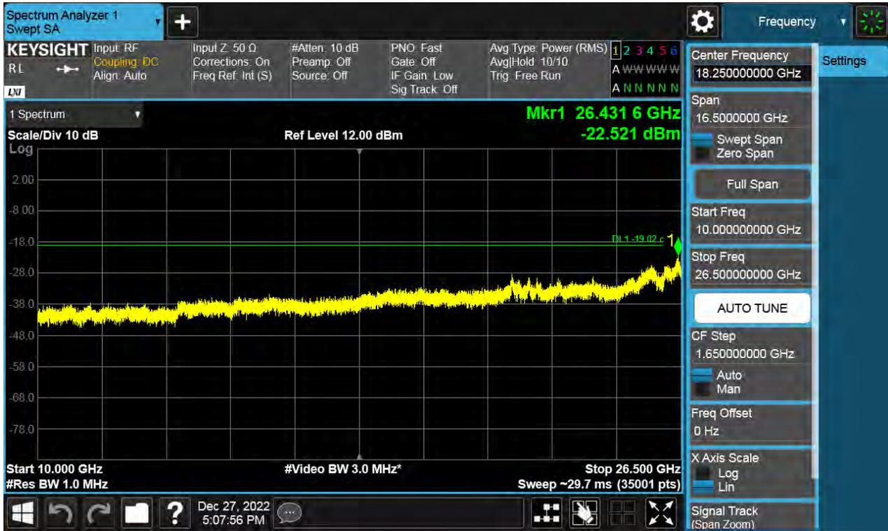
Antenna 0 / (4 Port) DSS B2 10 MHz 9t1 [1 Carrier] / 9 kHz ~ 150 kHz / 256QAM / MIDDLE
