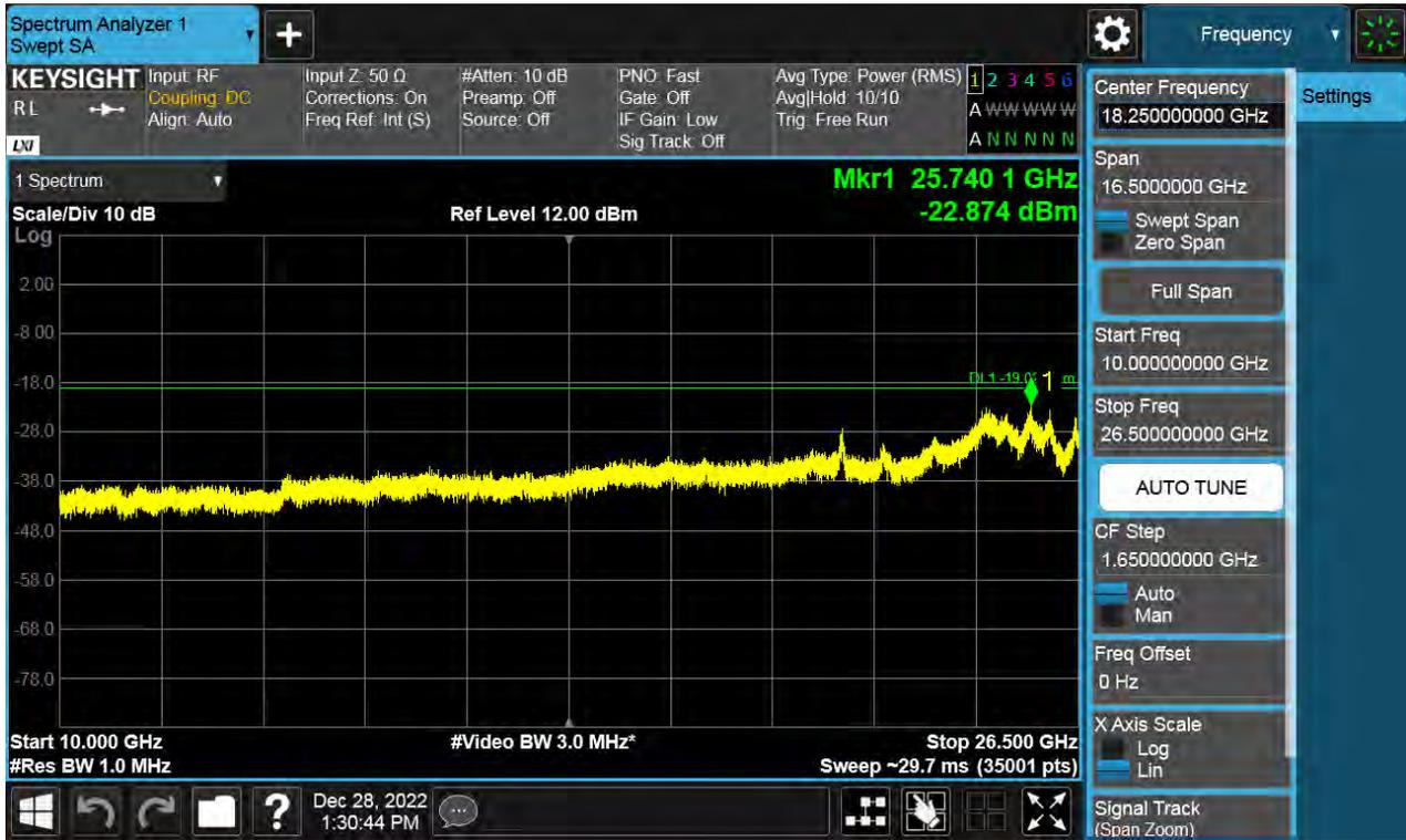
Antenna 0 / (4 Port) DSS B2 10 MHz 5t5 [1 Carrier] / 9 kHz ~ 150 kHz / 256QAM / MIDDLE
