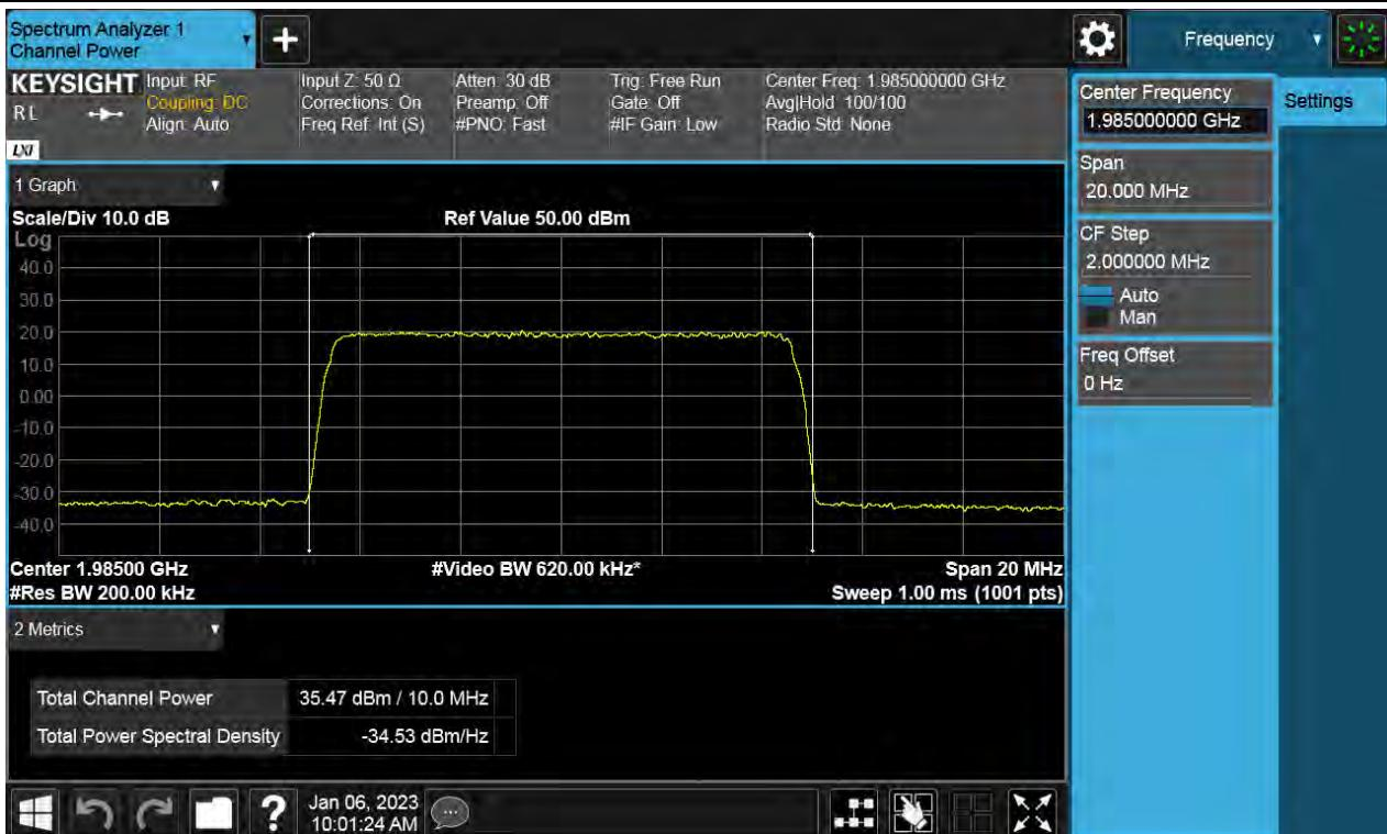
**Antenna 1 / (4 Port) 5G NR n66 5 MHz 1 Carrier + 5G NR n66 5 MHz 1 Carrier + 5G NR n66 5 MHz 1 Carrier [3 Carrier]
