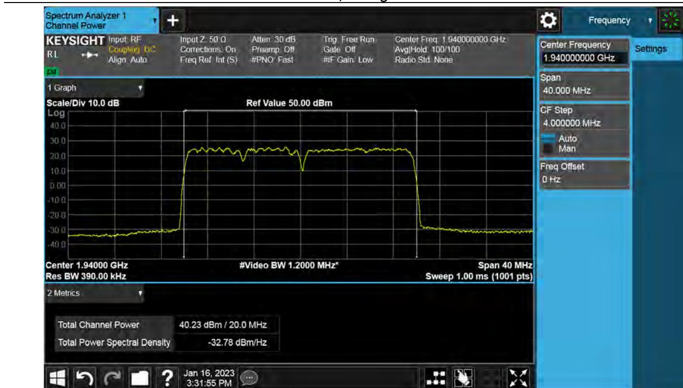
**Antenna 0 / (4 Port) DSS B2 10 MHz 1 Carrer + 5G NR n2 5 MHz 1 Carrier + 5G NR n2 15 MHz 1 Carrer [3 Carrier] / 64QAM / Middle / Contiguous**
