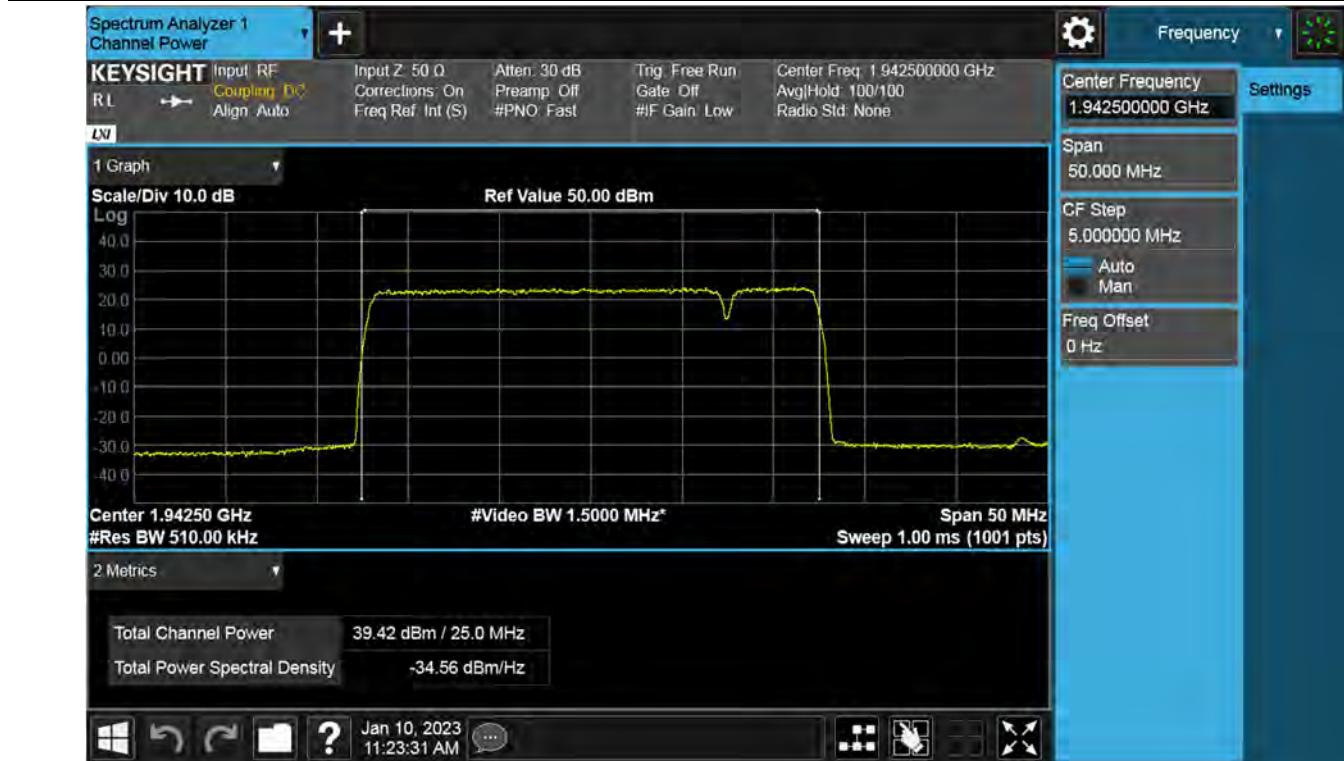
**Antenna 3 / (4 Port) 5G NR n2 20 MHz 1 Carrier + 5G NR n2 5 MHz 1 Carrier + 5G NR n2 5 MHz 1 Carrier [3 Carrier][2C+1C]
