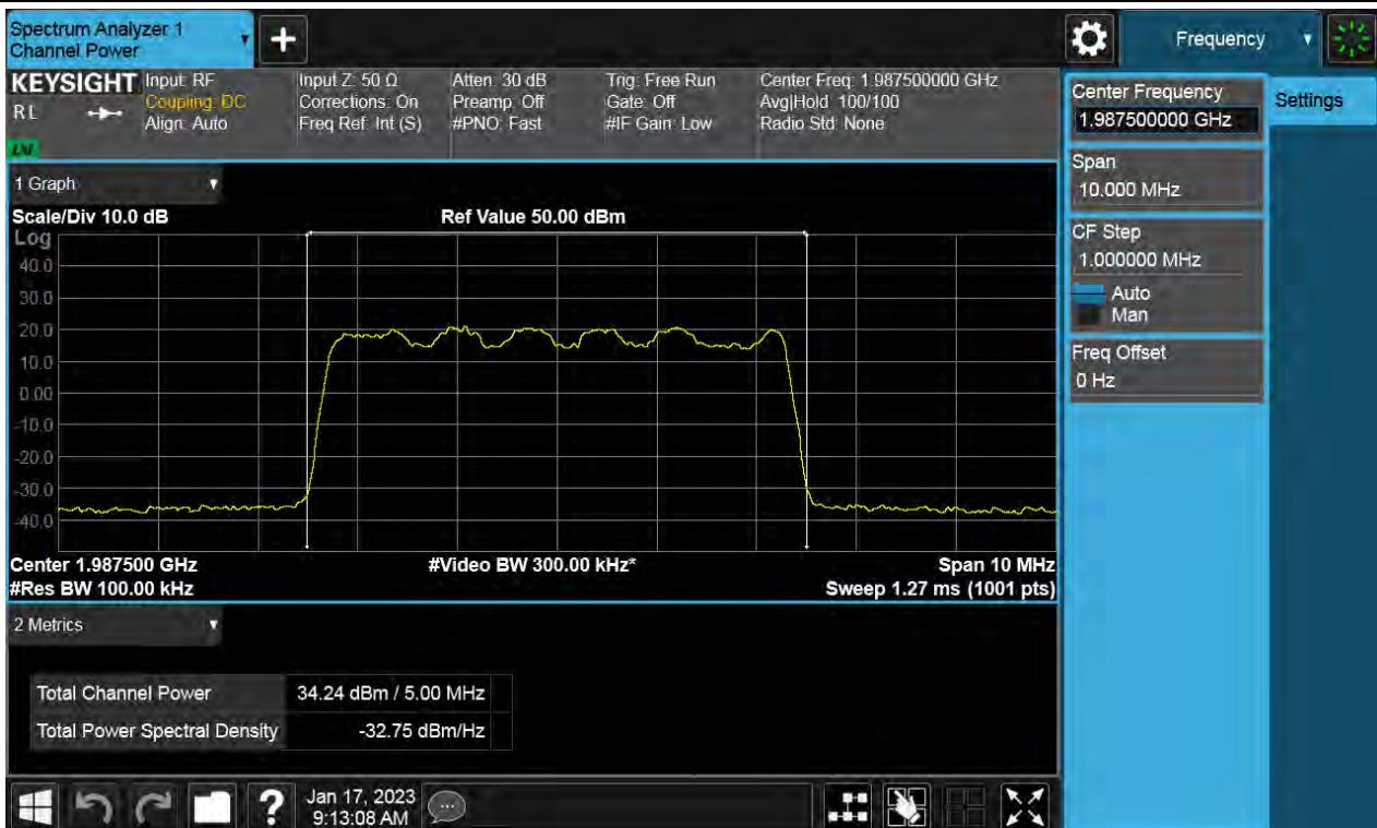
**Antenna 0 / (4 Port) DSS B2 10 MHz 1 Carrer + 5G NR n2 5 MHz 1 Carrier + 5G NR n2 15 MHz 1 Carrer [3 Carrier][1C+2C] / Non-Contiguous / DSS B2 10 MHz 1 Carrier / 64QAM / Low**
