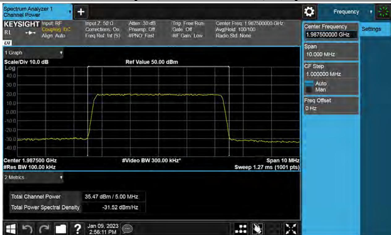
**Antenna 0 / (4 Port) 5G NR n2 20 MHz 1 Carrier + 5G NR n2 5 MHz 1 Carrier + 5G NR n2 5 MHz 1 Carrier [3 Carrier][1C+2C]
