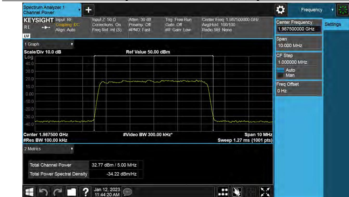
**Antenna 0 / (4 Port) DSS B2 10 MHz 1 Carrier + 5G NR n2 5 MHz 1 Carrier + 5G NR n2 5 MHz 1 Carrer [3 Carrier][1C+2C] / Non-Contiguous / 5G NR n2 5 MHz 1 Carrier / QPSK / Low**
