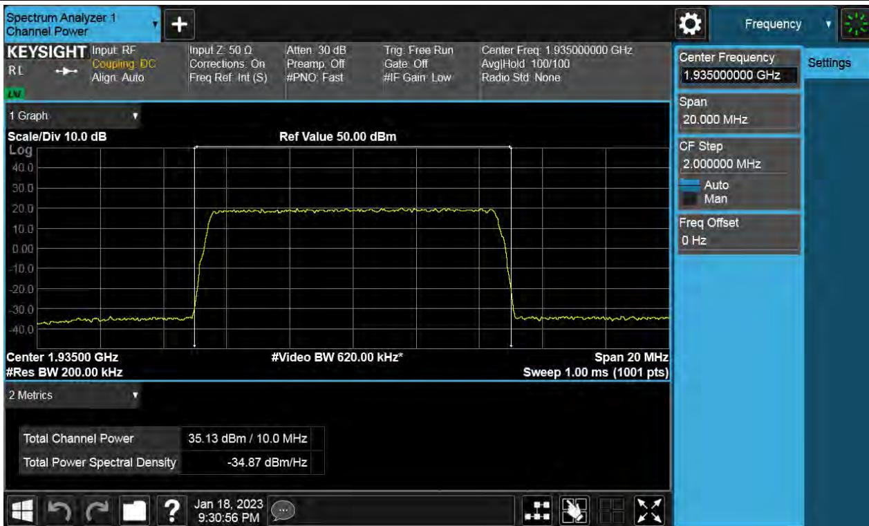
**Antenna 0 / (4 Port) DSS B2 10 MHz 1 Carrier + 5G NR n2 15 MHz 1 Carrier + LTE B2 5 MHz 1 Carrer [3 Carrier][1C+2C] / Non-Contiguous / LTE B2 5 MHz + 5G NR n2 15 MHz 1 Carrier / 64QAM / High**
