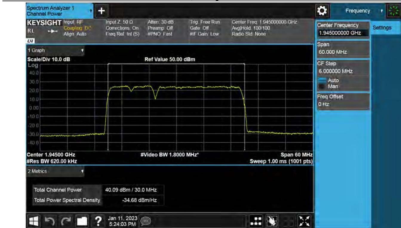
**Antenna 0 / (4 Port) DSS B2 10 MHz 1 Carrier + 5G NR n2 5 MHz 1 Carrier + 5G NR n2 5 MHz 1 Carrer [3 Carrier] / 16QAM / Low / Contiguous**
