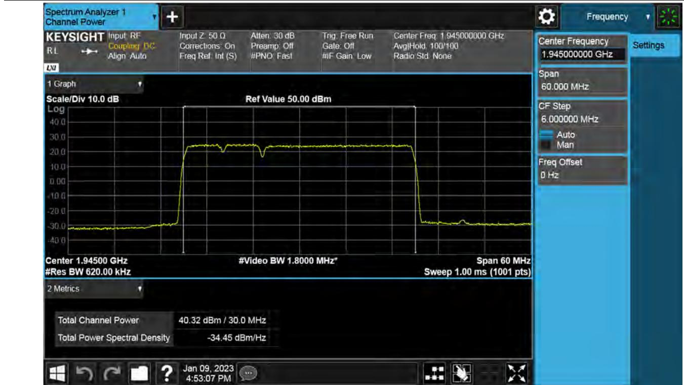
**Antenna 0 / (4 Port) 5G NR n2 5 MHz 1 Carrier + 5G NR n2 5 MHz 1 Carrier + LTE B2 5 MHz 1 Carrier [3 Carrier] / 64QAM / High / Contiguous**
