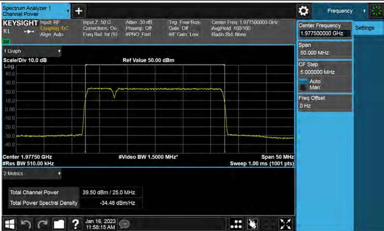
**Antenna 0 / (4 Port) 5G NR n2 5 MHz 1 Carrier + 5G NR n2 20 MHz 1 Carrier + LTE B2 5 MHz 1 Carrier [3 Carrier][2C+1C] / Non-Contiguous / 5G NR n2 20 MHz 1 Carrier + 5G NR n2 5 MHz 1 Carrier / 64QAM / Low**
