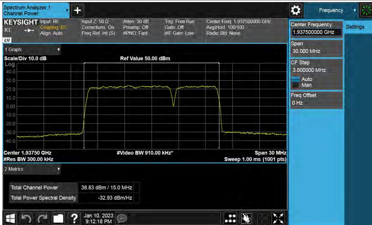
**Antenna 3 / (4 Port) DSS B2 10 MHz 1 Carrier + LTE B2 5 MHz 1 Carrier + LTE B2 5 MHz 1 Carrier [3 Carrier][2C+1C] / Non-Contiguous / LTE B2 5 MHz 1 Carrier / 16QAM / High**
