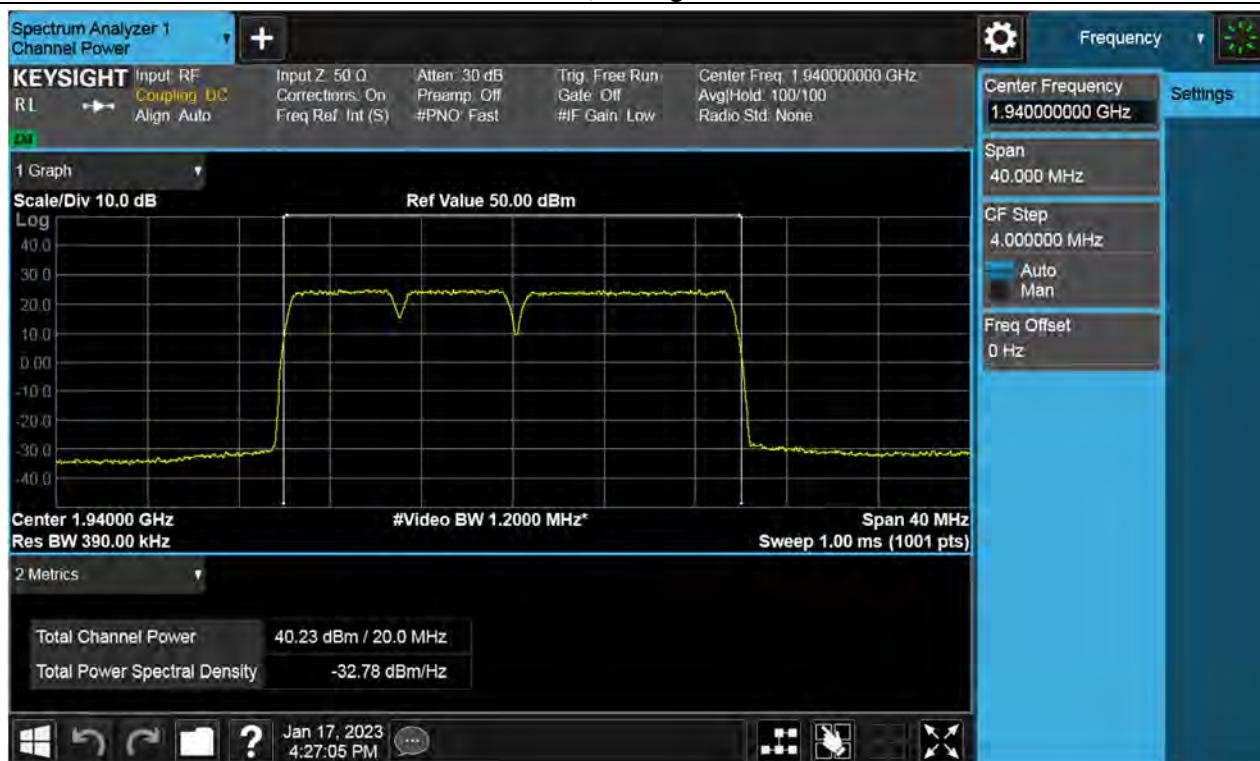
**Antenna 0 / (4 Port) DSS B2 10 MHz 1 Carrier + 5G NR n2 15 MHz 1 Carrier + LTE B2 5 MHz 1 Carrer [3 Carrier] / 16QAM / High / Contiguous**
