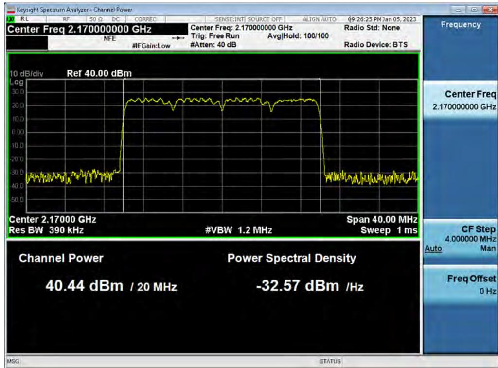
**Antenna 2 / (4 Port) LTE B66 5 MHz 1 Carrier + 5G NR n66 5 MHz 1 Carrier + 5G NR n66 10 MHz 1 Carrier + 5G NR n66 20 MHz 1 Carrier [4 Carrier] / 64QAM / Low / Contiguous**
