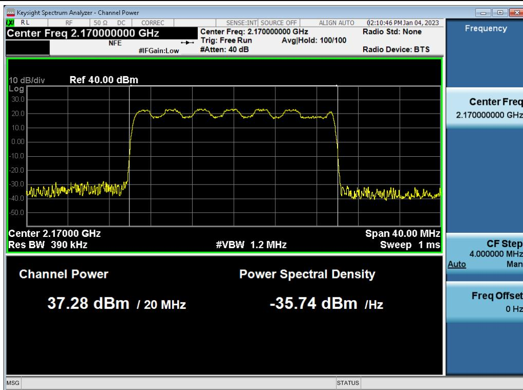
**Antenna 1 / (4 Port) 5G NR n66 5 MHz 1 Carrier + 5G NR n66 5 MHz 1 Carrier + DSS B66 10 MHz 1 Carrier [3 Carrier] [1C+2C] / 5G NR n66 5 MHz 1 Carrier / QPSK / Low / Non-Contiguous**
