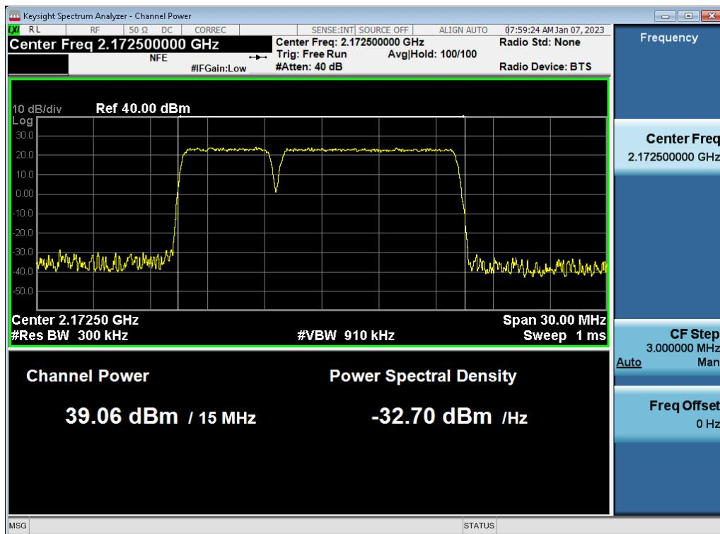
**Antenna 1 / (4 Port) 5G NR n66 5 MHz 1 Carrier + 5G NR n66 5 MHz 1 Carrier + DSS B66 10 MHz 1 Carrier [3 Carrier]
