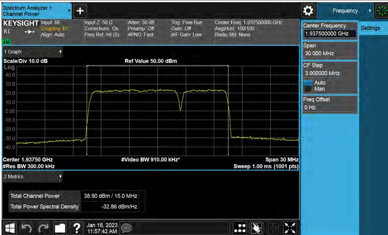
**Antenna 0 / (4 Port) DSS B2 10 MHz 1 Carrier + 5G NR n2 5 MHz 1 Carrier + LTE B2 5 MHz 1 Carrer [3 Carrier][2C+1C] / Non-Contiguous / LTE B2 5 MHz 1 Carrier / 16QAM / High**
