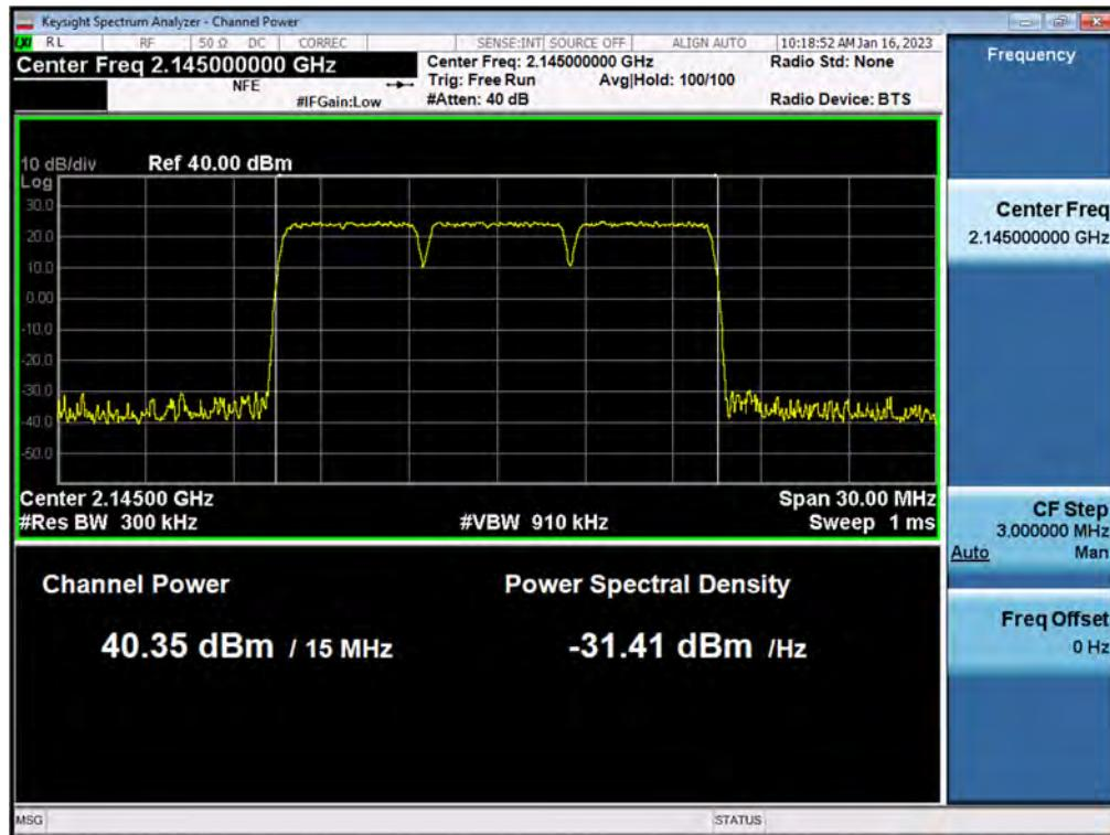
Antenna 1 / (4 Port) 5G NR n66 5 MHz 1 Carrier + 5G NR n66 15 MHz 1 Carrier + 5G NR n66 20 MHz 1 Carrier [3 Carrier] / 16QAM / High / Contiguous
