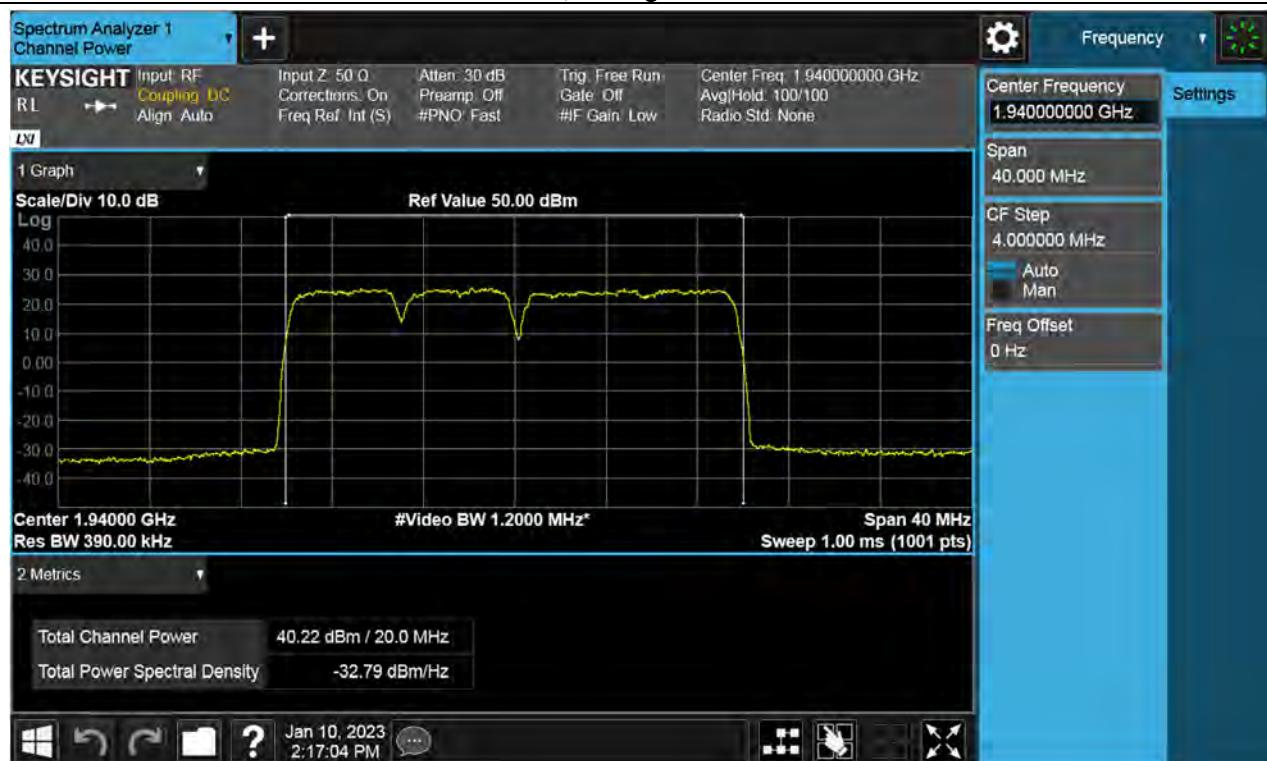
**Antenna 0 / (4 Port) DSS B2 20 MHz 1 Carrier + LTE B2 5 MHz 1 Carrier + LTE B2 5 MHz 1 Carrier [3 Carrier] / 16QAM / Low / Contiguous**
