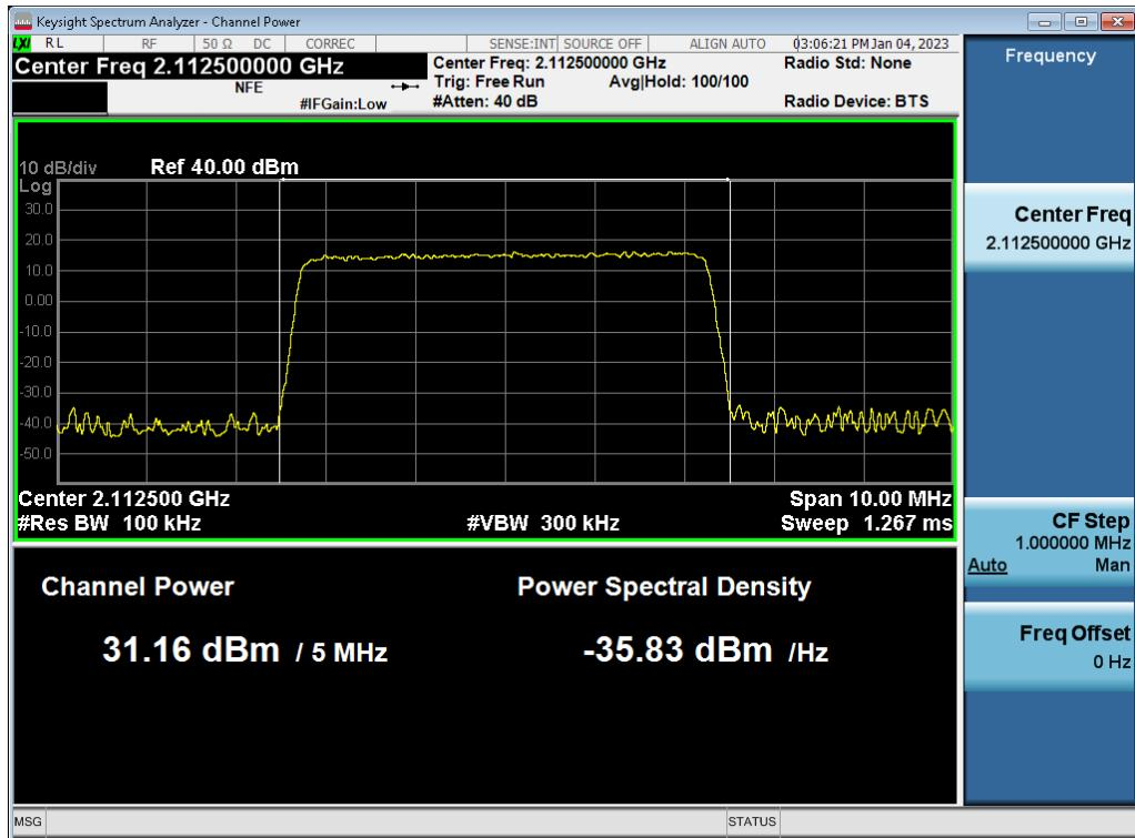
**Antenna 1 / (4 Port) 5G NR n66 5 MHz 1 Carrier + 5G NR n66 15 MHz 1 Carrier + 5G NR n66 20 MHz 1 Carrier [3 Carrier]
