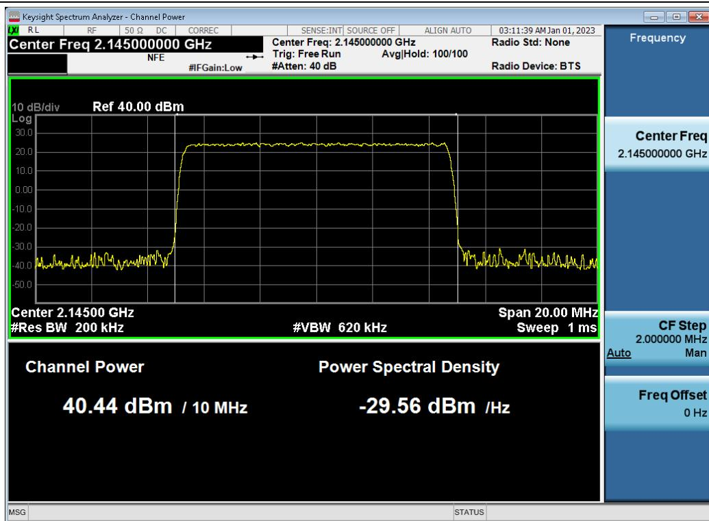
**Antenna 1 / (4 Port) 5G NR n66 15 MHz [1 Carrier] / 16QAM / Middle**
