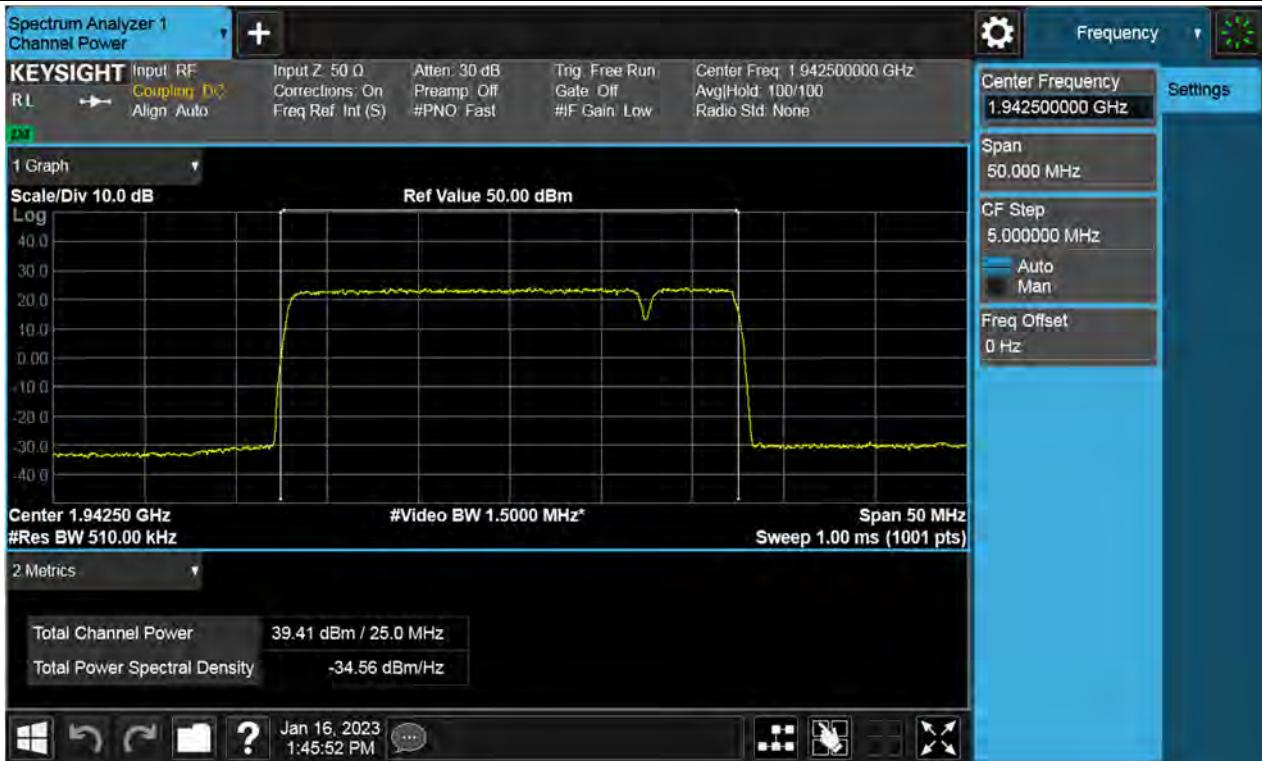
**Antenna 0 / (4 Port) 5G NR n2 5 MHz 1 Carrier + 5G NR n2 20 MHz 1 Carrier + LTE B2 5 MHz 1 Carrier [3 Carrier][2C+1C] / Non-Contiguous / LTE B2 5 MHz 1 Carrier / 64QAM / High**
