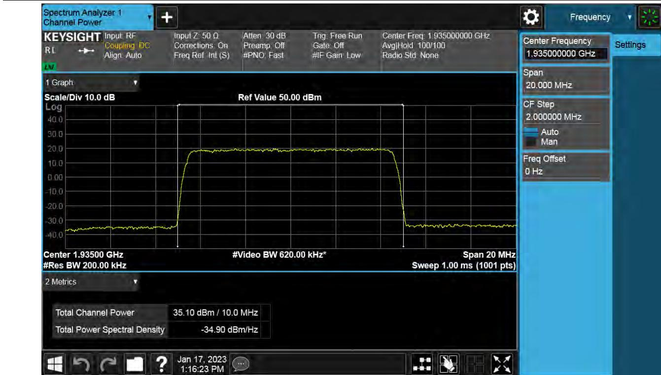
**Antenna 0 / (4 Port) DSS B2 10 MHz 1 Carrer + 5G NR n2 5 MHz 1 Carrier + 5G NR n2 15 MHz 1 Carrer [3 Carrier][1C+2C] / Non-Contiguous / 5G NR n2 5 MHz 1 Carrier + 5G NR n2 15 MHz 1 Carrier / 64QAM / High**
