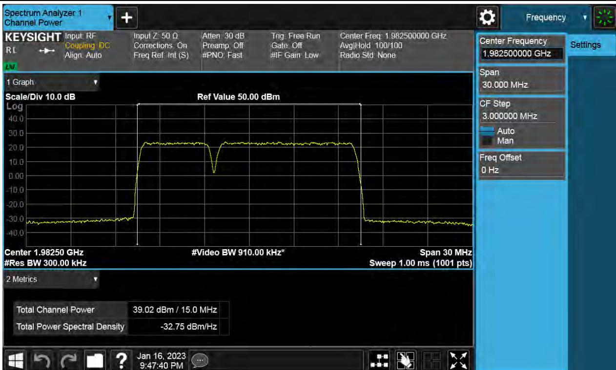
**Antenna 0 / (4 Port) DSS B2 10 MHz 1 Carrier + 5G NR n2 5 MHz 1 Carrier + 5G NR n2 5 MHz 1 Carrer [3 Carrier][2C+1C] / Non-Contiguous / DSS B2 10 MHz 1 Carrier + 5G NR n2 5 MHz 1 Carrier / 16QAM / Low**
