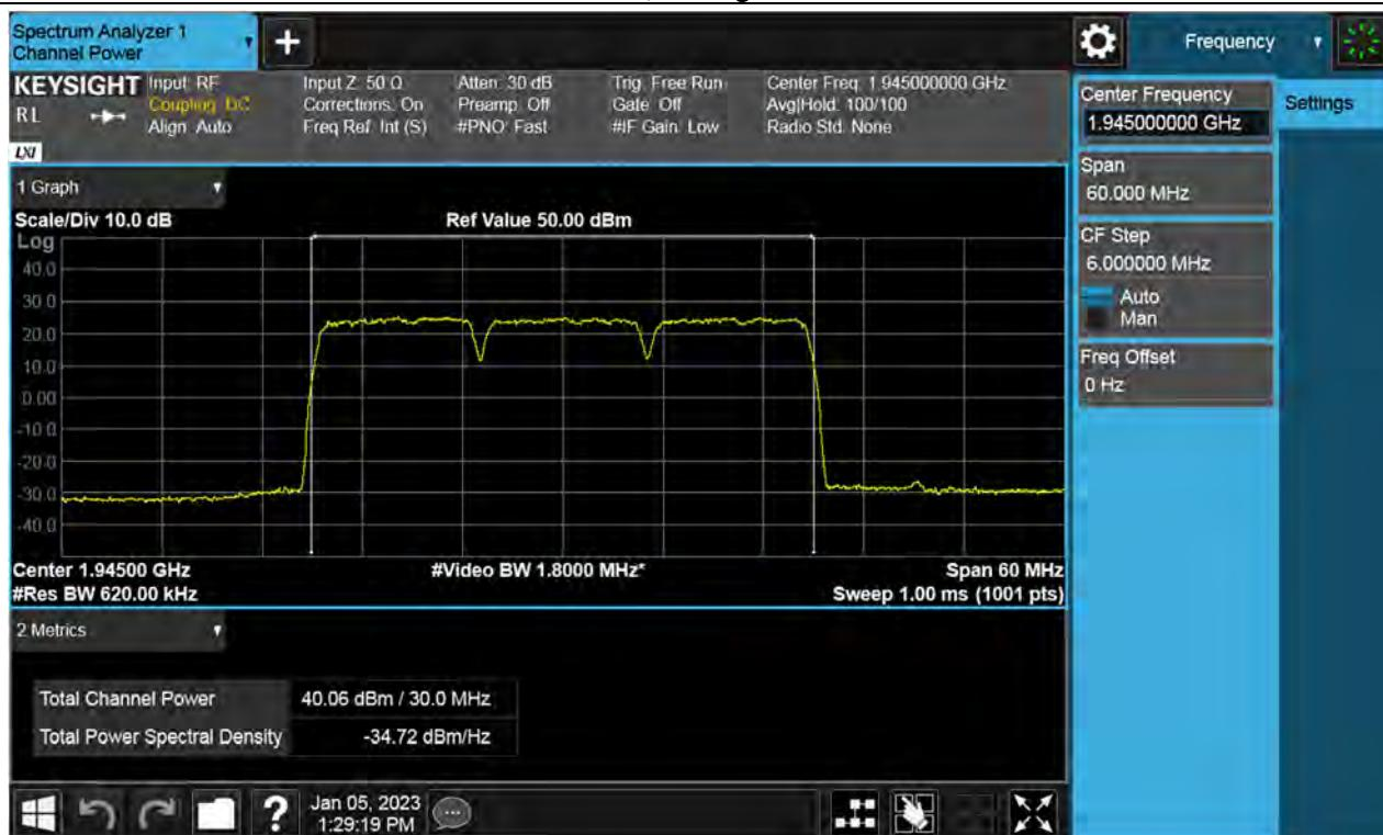
Antenna 1 / (4 Port) 5G NR n66 5 MHz 1 Carrier + 5G NR n66 5 MHz 1 Carrier + 5G NR n66 5 MHz 1 Carrier [3 Carrier] / 256QAM / Middle / Contiguous
