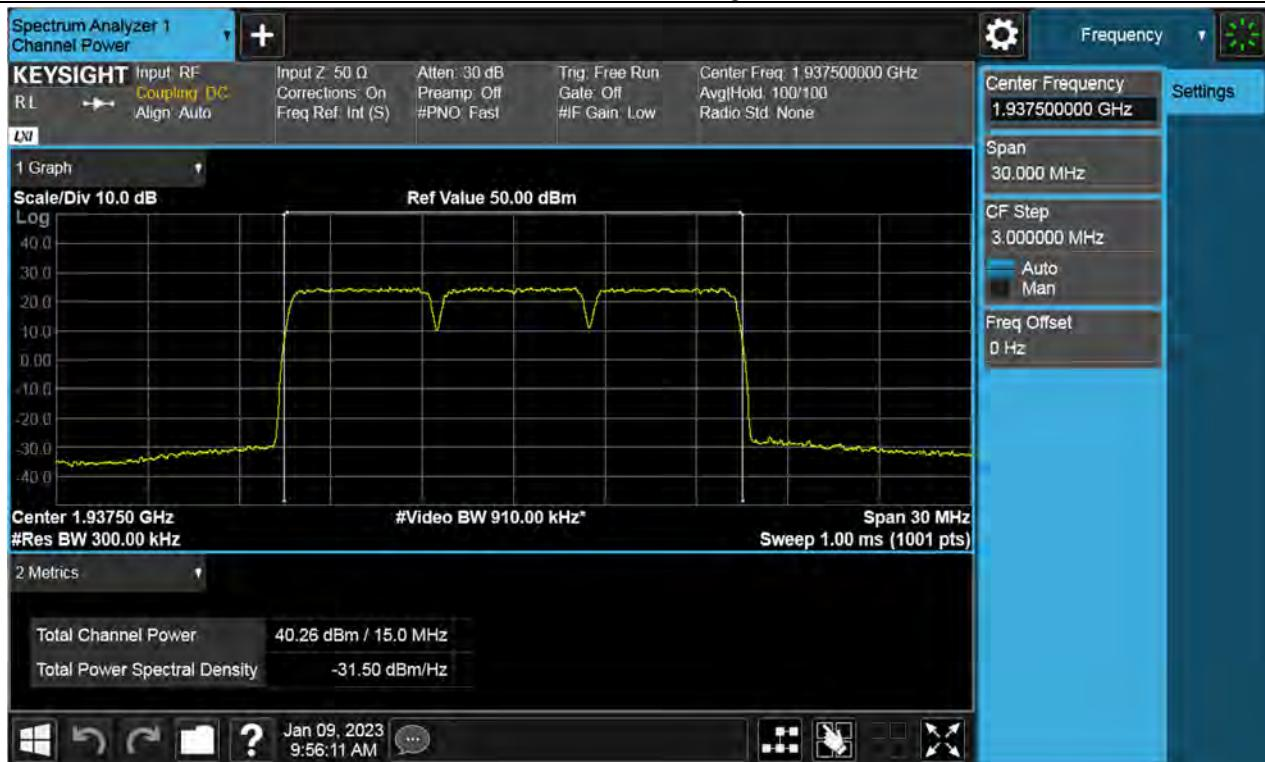
**Antenna 3 / (4 Port) 5G NR n2 20 MHz 1 Carrier + 5G NR n2 5 MHz 1 Carrier + 5G NR n2 5 MHz 1 Carrier [3 Carrier] / QPSK / Low / Contiguous**
