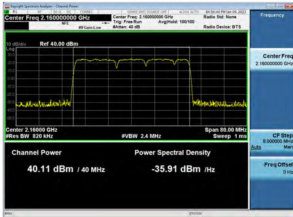
**Antenna 0 / (4 Port) DSS B2 10 MHz 1 Carrier + DSS B2 10 MHz 1 Carrier [2 Carrier] / Non-Contiguous / DSS B2 10 MHz 1 Carrier / 16QAM / Low**
