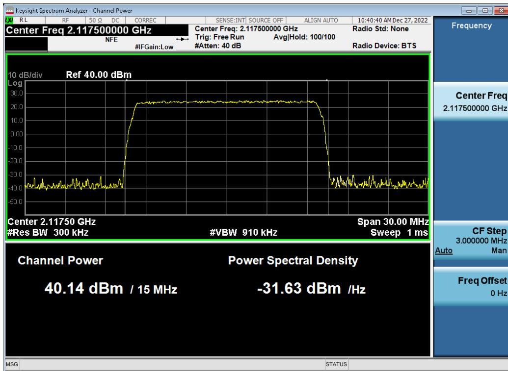
**Antenna 1 / (4 Port) DSS B66 20 MHz 2to8 [1 Carrier] / 256QAM / Low**
