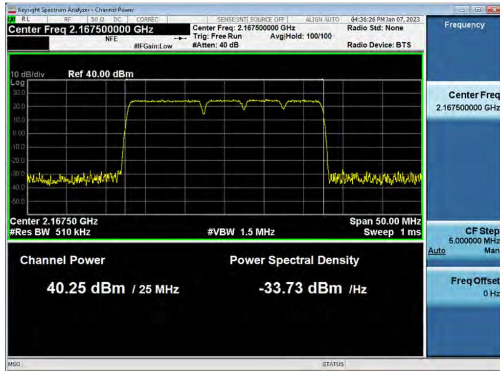
**Antenna 1 / (4 Port) LTE B66 5 MHz 1 Carrier + 5G NR n66 5 MHz 1 Carrier + DSS B66 10 MHz 1 Carrier + 5G NR n66 20 MHz 1 Carrier [4 Carrier] / QPSK / Low / Contiguous**
