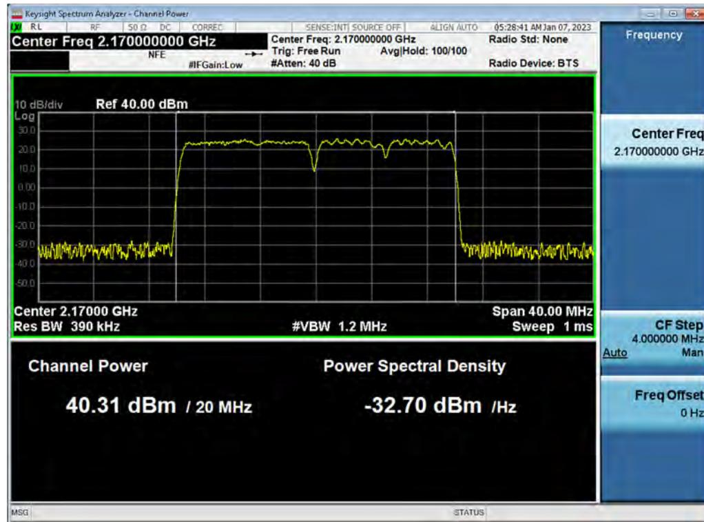
**Antenna 1 / (4 Port) DSS B66 10 MHz 1 Carrier + 5G NR n66 10 MHz 1 Carrier + 5G NR n66 20 MHz 1 Carrier [3 Carrier] / 16QAM / High / Contiguous**
