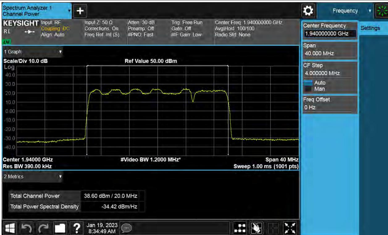
**Antenna 0 / (4 Port) DSS B2 10 MHz 1 Carrier + 5G NR n2 15 MHz 1 Carrier + LTE B2 5 MHz 1 Carrer [3 Carrier][2C+1C] / Non-Contiguous / DSS B2 10 MHz 1 Carrier / 16QAM / High**
