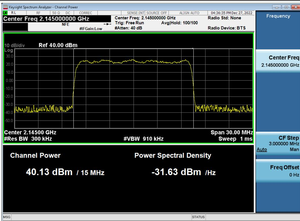
**Antenna 1 / (4 Port) DSS B66 15 MHz 9to1 [1 Carrier] / 256QAM / Low**
