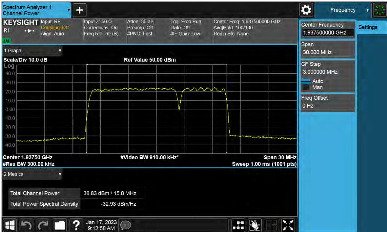
**Antenna 0 / (4 Port) DSS B2 10 MHz 1 Carrier + 5G NR n2 5 MHz 1 Carrier + 5G NR n2 5 MHz 1 Carrer [3 Carrier][2C+1C] / Non-Contiguous / 5G NR n2 5 MHz 1 Carrier / 16QAM / High**
