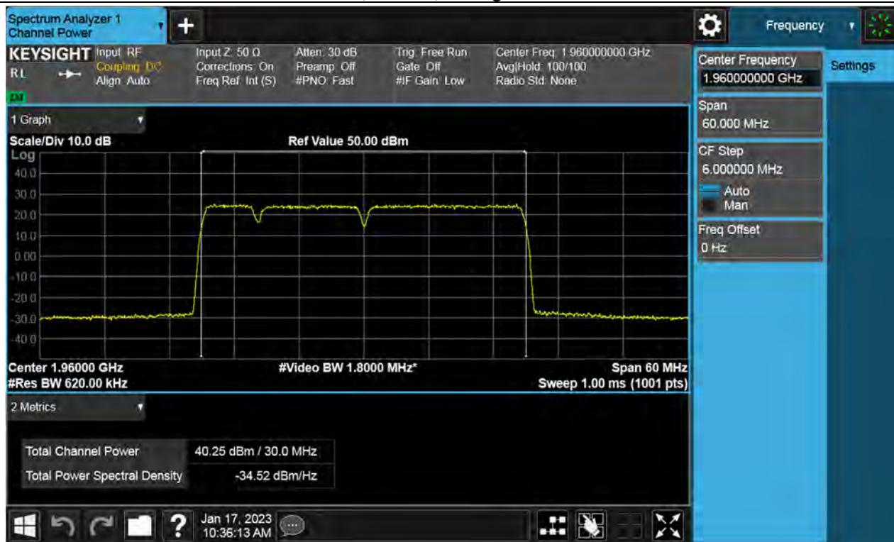
**Antenna 0 / (4 Port) DSS B2 10 MHz 1 Carrier + 5G NR n2 5 MHz 1 Carrier + LTE B2 5 MHz 1 Carrer [3 Carrier] / 256QAM / Low / Contiguous**
