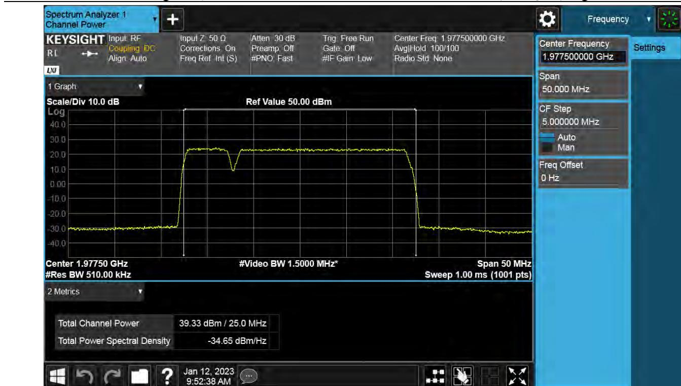
**Antenna 0 / (4 Port) DSS B2 20 MHz 1 Carrier + LTE B2 5 MHz 1 Carrier + LTE B2 5 MHz 1 Carrier [3 Carrier][2C+1C] / Non-Contiguous / DSS B2 20 MHz 1 Carrier + LTE B2 5 MHz 1 Carrier / 16QAM / Low**
