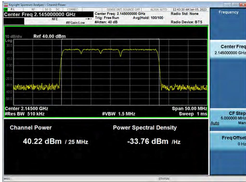
**Antenna 1 / (4 Port) LTE B66 5 MHz 1 Carrier + DSS B66 10 MHz 1 Carrier + DSS B66 10 MHz 1 Carrier + DSS B66 15 MHz 1 Carrier [4 Carrier] / 16QAM / High / Contiguous**
