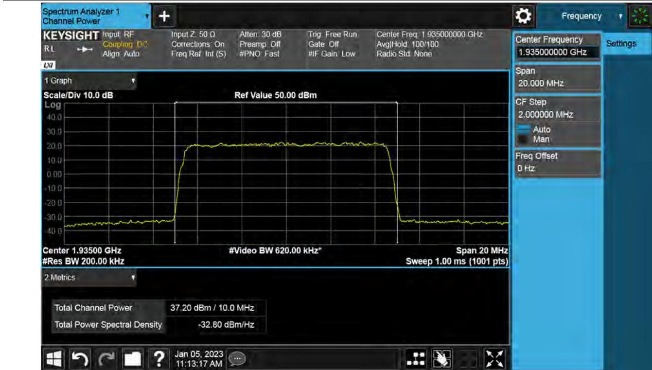
**Antenna 0 / (4 Port) DSS B2 10 MHz 1 Carrier + DSS B2 10 MHz 1 Carrier [2 Carrier] / Non-Contiguous / DSS B2 10 MHz 1 Carrier / 16QAM / High**
