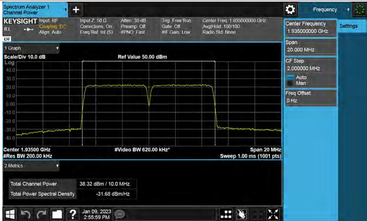
**Antenna 0 / (4 Port) 5G NR n2 5 MHz 1 Carrier + 5G NR n2 5 MHz 1 Carrier + 5G NR n2 5 MHz 1 Carrier [3 Carrier] [2C+1C]
