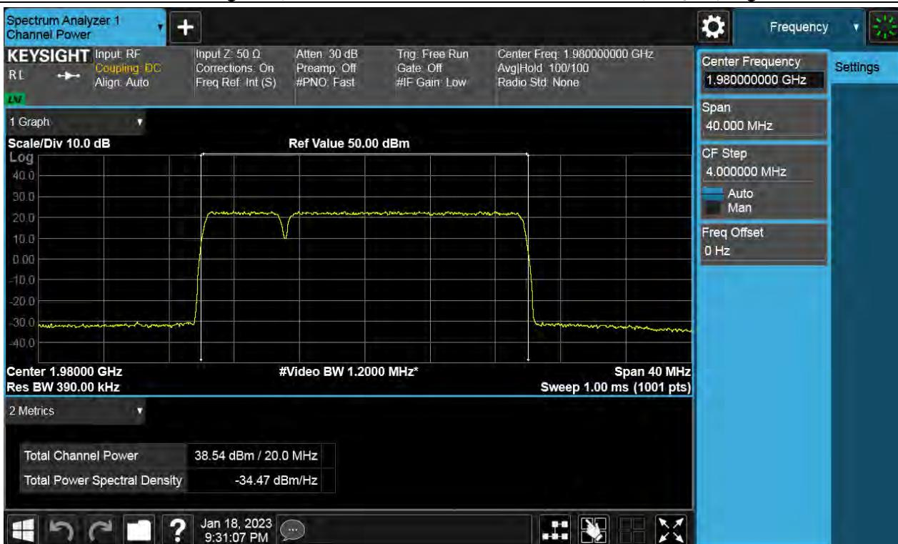
**Antenna 0 / (4 Port) DSS B2 10 MHz 1 Carrier + 5G NR n2 15 MHz 1 Carrier + LTE B2 5 MHz 1 Carrer [3 Carrier][2C+1C] / Non-Contiguous / 5G NR n2 15 MHz 1 Carrier + LTE B2 5 MHz 1 Carrier/ 16QAM / Low**
