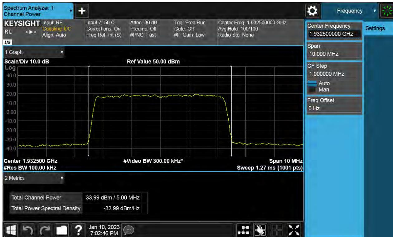
**Antenna 3 / (4 Port) DSS B2 10 MHz 1 Carrier + LTE B2 5 MHz 1 Carrier + LTE B2 5 MHz 1 Carrier [3 Carrier][1C+2C] / Non-Contiguous / LTE B2 5 MHz 1 Carrier + DSS B2 10 MHz 1 Carrier / 16QAM / High**
