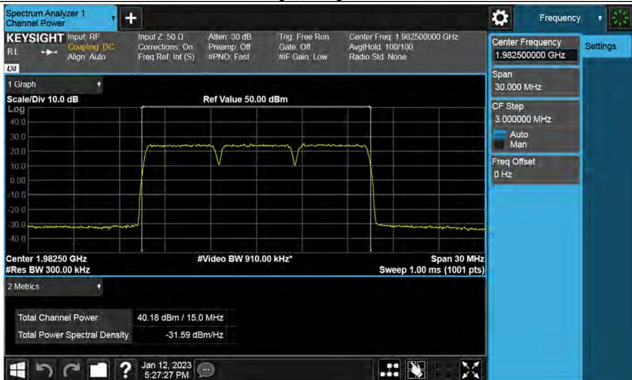
**Antenna 0 / (4 Port) 5G NR n2 5 MHz 1 Carrier + 5G NR n2 20 MHz 1 Carrier + LTE B2 5 MHz 1 Carrier [3 Carrier] / 64QAM / Middle / Contiguous**
