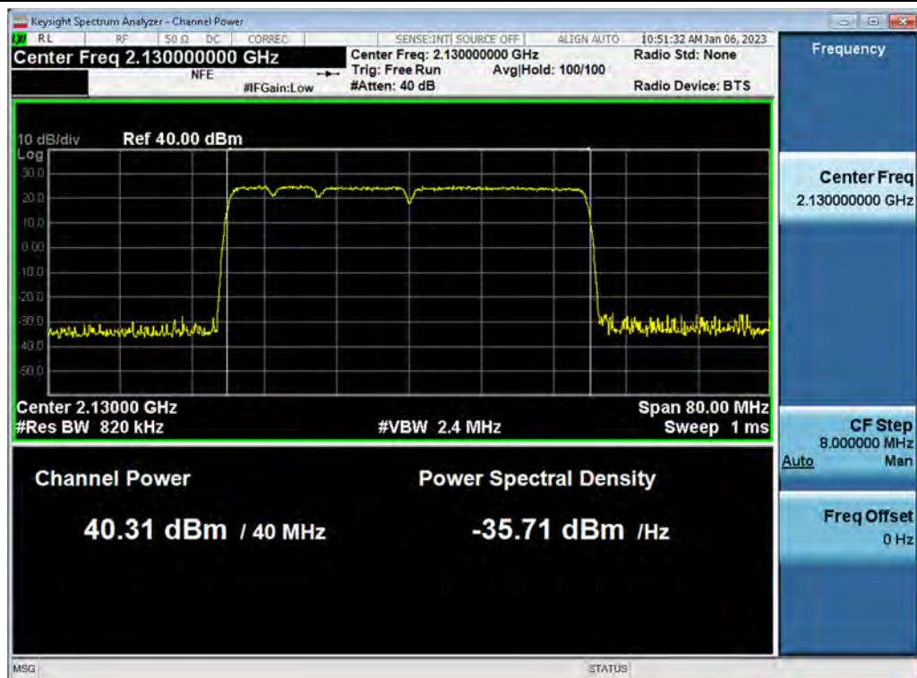
**Antenna 1 / (4 Port) LTE B66 5 MHz 1 Carrier + 5G NR n66 5 MHz 1 Carrier + 5G NR n66 5 MHz 1 Carrier + DSS B66 10 MHz 1 Carrier [4 Carrier] / QPSK / High / Contiguous**
