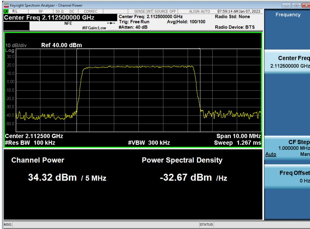
**Antenna 1 / (4 Port) 5G NR n66 5 MHz 1 Carrier + 5G NR n66 5 MHz 1 Carrier + DSS B66 10 MHz 1 Carrier [3 Carrier] [1C+2C] / 5G NR n66 5 MHz 1 Carrier + DSS B66 10 MHz 1 Carrier / QPSK / High / Non-Contiguous**
