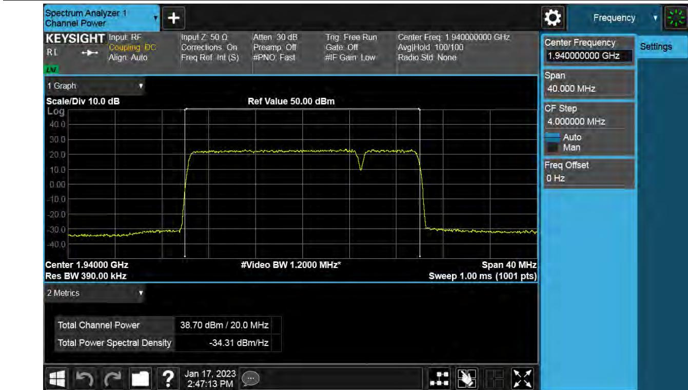
**Antenna 0 / (4 Port) DSS B2 10 MHz 1 Carrer + 5G NR n2 5 MHz 1 Carrier + 5G NR n2 15 MHz 1 Carrer [3 Carrier][2C+1C] / Non-Contiguous / DSS B2 10 MHz 1 Carrier / 256QAM / High**
