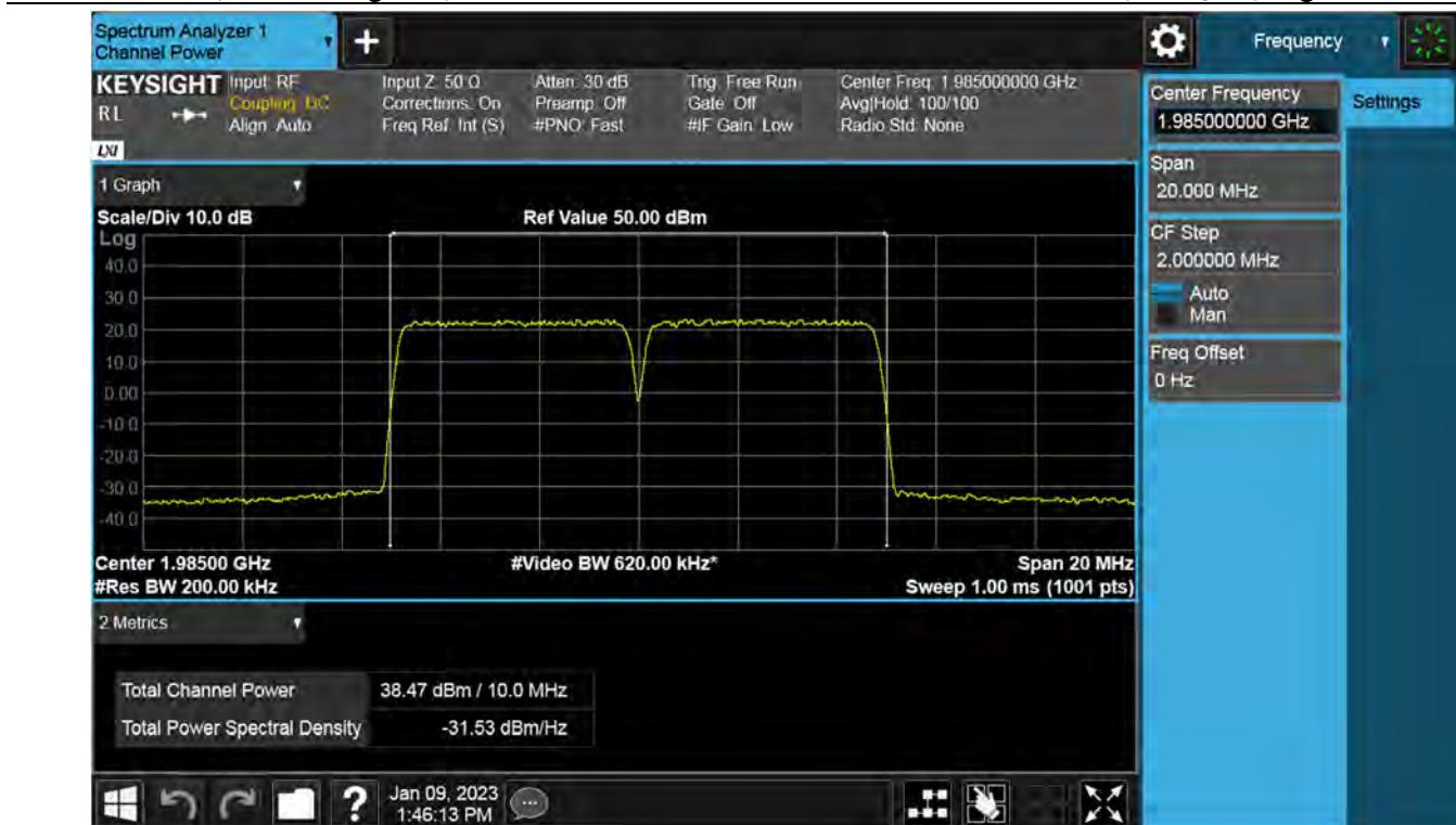
**Antenna 0 / (4 Port) 5G NR n2 5 MHz 1 Carrier + 5G NR n2 5 MHz 1 Carrier + 5G NR n2 5 MHz 1 Carrier [3 Carrier] [2C+1C]
