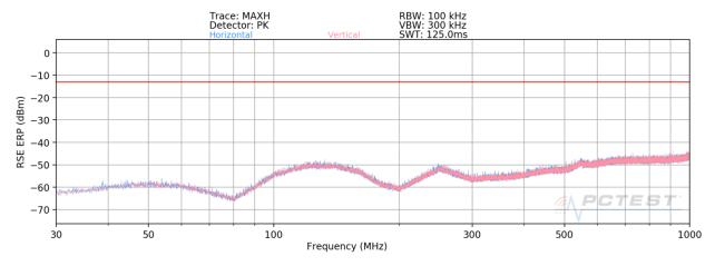
Plot 7-1299. Radiated spurious emission\_30 MHz to 1000 MHz (Multi Band\_B2\_5M+5M+5M\_3C\_High + B66\_5M+5M+5M\_3C\_Low)
