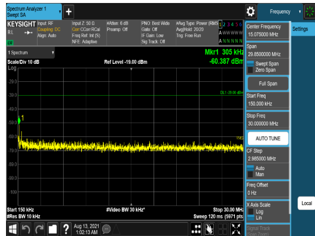
Plot 7-1241. Conducted Spurious Emission Plot 150 kHz to 30 MHz
