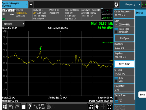
Plot 7-1247. Conducted Spurious Emission Plot 9 kHz to 150 kHz Multi Band_B2_5M+5M+5M_3C - Non-contiguous + B66_5M+5M+5M_3C - Non-contiguous_QPSK - Port 2
