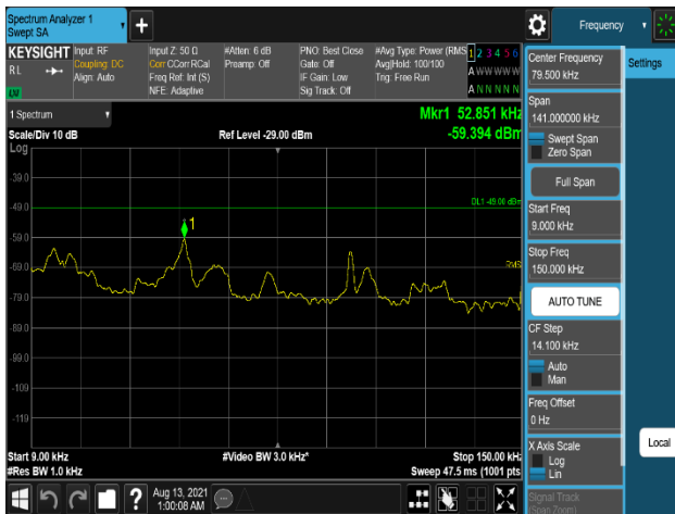
Plot 7-1240. Conducted Spurious Emission Plot 9 kHz to 150 kHz
