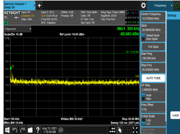
Plot 7-1248. Conducted Spurious Emission Plot 150 kHz to 30 MHz Multi Band_B2_5M+5M+5M_3C - Non-contiguous + B66_5M+5M+5M_3C - Non-contiguous_QPSK - Port 1
