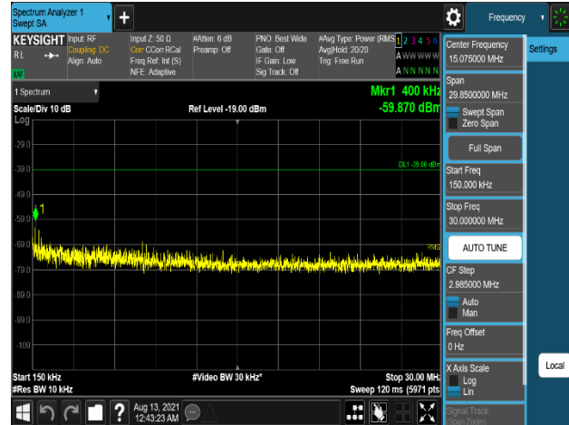
Plot 7-1234. Conducted Spurious Emission Plot 150 kHz to 30 MHz
