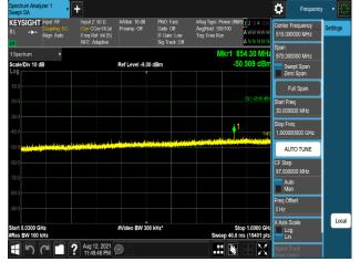
Plot 7-1228. Conducted Spurious Emission Plot 30 MHz to 1 GHz (Multi Band\_B2\_5M\_1C\_High + B66\_5M\_1C\_Low\_QPSK - Port 3)
