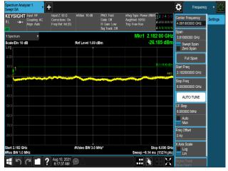
Plot 7-1187. Conducted Spurious Emission Plot 2.182 GHz to 6 GHz (B66\_5M+5M\_2C\_QPSK - Port 3)
