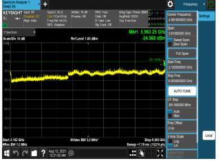
Plot 7-1217. Conducted Spurious Emission Plot 2.182 GHz to 6 GHz (B66\_5M+5M+10M+20M\_4C\_64QAM - Port 2)
