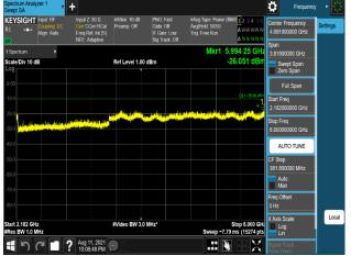
Plot 7-1205. Conducted Spurious Emission Plot 2.182 GHz to 6 GHz (B66\_5M+5M+5M+5M\_4C\_64QAM - Port 2)
