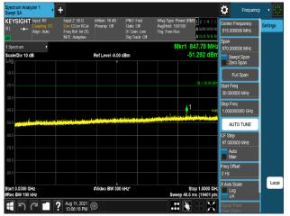
Plot 7-1203. Conducted Spurious Emission Plot 30 MHz to 1 GHz (B66\_5M+5M+5M+5M\_4C\_64QAM - Port 3)
