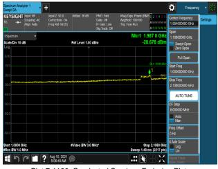
Plot 7-1180. Conducted Spurious Emission Plot 1 GHz to 2.108 GHz (B66\_20M+20M\_2C\_QPSK - Port 0)
