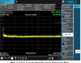
Plot 7-1214. Conducted Spurious Emission Plot 150 kHz to 30 MHz (B66\_5M+5M+10M+20M\_4C\_64QAM - Port 1)
