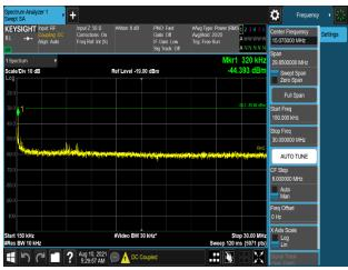
Plot 7-1166. Conducted Spurious Emission Plot 150 kHz to 30 MHz (B66\_5M+5M\_2C\_QPSK - Port 3)
