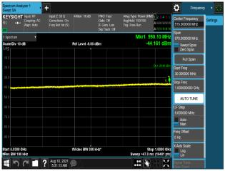
Plot 7-1167. Conducted Spurious Emission Plot 30 MHz to 1 GHz (B66\_5M+5M\_2C\_QPSK - Port 2)
