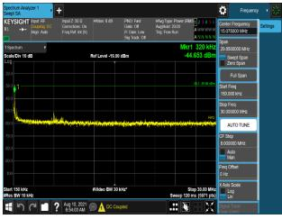
Plot 7-1190. Conducted Spurious Emission Plot 150 kHz to 30 MHz (B66\_5M+5M+20M\_3C\_16QAM - Port 1)
