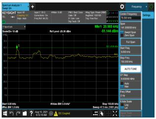
Plot 7-1183. Conducted Spurious Emission Plot 9 kHz to 150 kHz (B66\_5M+5M+5M\_3C\_64QAM - Port 3)
