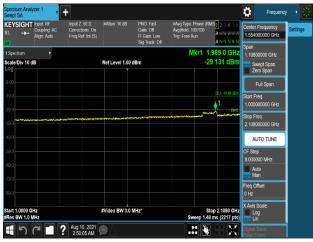
Plot 7-1174. Conducted Spurious Emission Plot 1 GHz to 2.108 GHz (B66\_5M+20M\_2C\_64QAM - Port 1)
