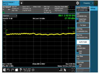
Plot 7-1175. Conducted Spurious Emission Plot 2.182 GHz to 6 GHz (B66\_5M+20M\_2C\_64QAM - Port 1)
