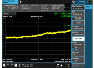
Plot 7-1176. Conducted Spurious Emission Plot 6 GHz to 22 GHz (B66\_5M+20M\_2C\_64QAM - Port 2)
