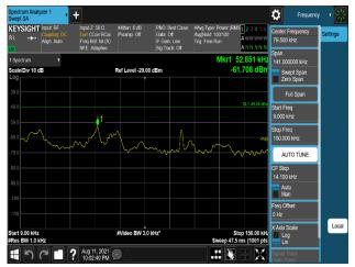
Plot 7-1201. Conducted Spurious Emission Plot 9 kHz to 150 kHz (B66\_5M+5M+5M+5M\_4C\_64QAM - Port 1)
