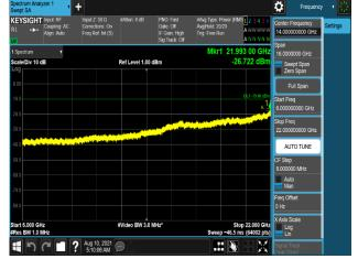
Plot 7-1182. Conducted Spurious Emission Plot 6 GHz to 22 GHz (B66\_20M+20M\_2C\_QPSK - Port 2)
