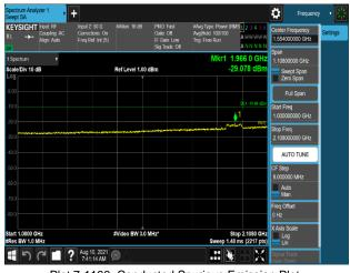
Plot 7-1198. Conducted Spurious Emission Plot 1 GHz to 2.108 GHz (B66\_5M+15M+20M\_3C\_64QAM - Port 3)
