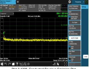
Plot 7-1208. Conducted Spurious Emission Plot 150 kHz to 30 MHz (B66\_5M+5M+5M+20M\_4C\_64QAM - Port 1)
