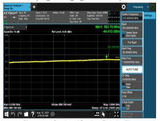
Plot 7-1173. Conducted Spurious Emission Plot 30 MHz to 1 GHz (B66\_5M+20M\_2C\_64QAM - Port 0)
