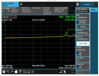
Plot 7-1192. Conducted Spurious Emission Plot 1 GHz to 2.108 GHz (B66\_5M+5M+20M\_3C\_16QAM - Port 3)
