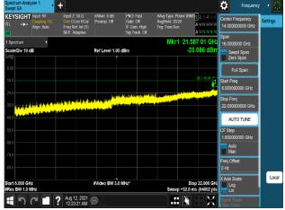
Plot 7-1218. Conducted Spurious Emission Plot 6 GHz to 22 GHz (B66\_5M+15M+20M\_3C\_64QAM - Port 2)
