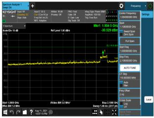
Plot 7-1204. Conducted Spurious Emission Plot 1 GHz to 2.108 GHz (B66\_5M+5M+5M+5M\_4C\_64QAM - Port 2)
