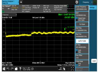
Plot 7-1211. Conducted Spurious Emission Plot 2.182 GHz to 6 GHz (B66\_5M+5M+5M+20M\_4C\_64QAM - Port 2)
