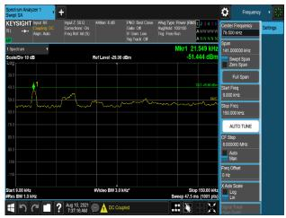
Plot 7-1195. Conducted Spurious Emission Plot 9 kHz to 150 kHz (B66\_5M+15M+20M\_3C\_64QAM - Port 3)
