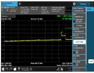
Plot 7-1216. Conducted Spurious Emission Plot 1 GHz to 2.108 GHz (B66\_5M+5M+10M+20M\_4C\_64QAM - Port 0)
