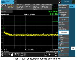
150 kHz to 30 MHz (Multi Band\_B2\_5M\_1C\_Low + B66\_5M\_1C\_High\_QPSK - Port 0)
