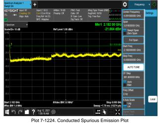
2.182 GHz to 6 GHz  $(Multi\ Band\_B2\_5M\_1C\_Low + B66\_5M\_1C\_High\_QPSK - Port\ 3)$
