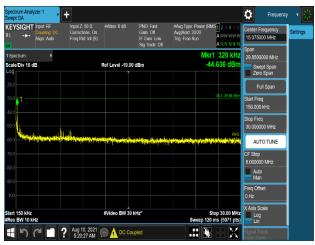
Plot 7-1178. Conducted Spurious Emission Plot 150 kHz to 30 MHz (B66\_20M+20M\_2C\_QPSK - Port 3)
