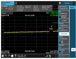
Plot 7-1210. Conducted Spurious Emission Plot 1 GHz to 2.108 GHz (B66\_5M+5M+5M+20M\_4C\_64QAM - Port 3)
