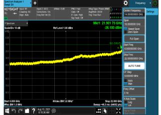
Plot 7-1188. Conducted Spurious Emission Plot 6 GHz to 22 GHz (B66\_5M+5M\_2C\_QPSK - Port 2)
