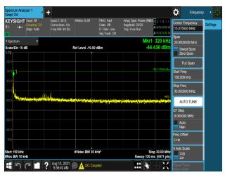
Plot 7-1172. Conducted Spurious Emission Plot 150 kHz to 30 MHz (B66\_5M+20M\_2C\_64QAM - Port 3)
