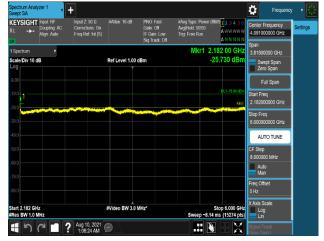
Plot 7-1169. Conducted Spurious Emission Plot 2.182 GHz to 6 GHz (B66\_5M+5M\_2C\_QPSK - Port 2)
