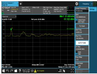
Plot 7-1165. Conducted Spurious Emission Plot 9 kHz to 150 kHz (B66\_5M+5M\_2C\_QPSK - Port 1)
