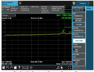
Plot 7-1186. Conducted Spurious Emission Plot 1 GHz to 2.108 GHz (B66\_5M+5M\_2C\_QPSK - Port 3)
