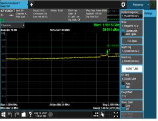
Plot 7-1168. Conducted Spurious Emission Plot 1 GHz to 2.108 GHz (B66\_5M+5M\_2C\_QPSK - Port 0)
