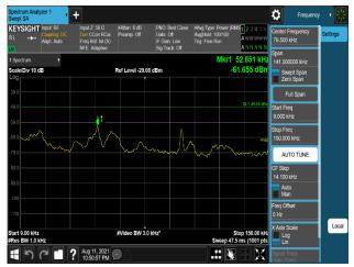
Plot 7-1207. Conducted Spurious Emission Plot 9 kHz to 150 kHz (B66\_5M+5M+5M+20M\_4C\_64QAM - Port 1)
