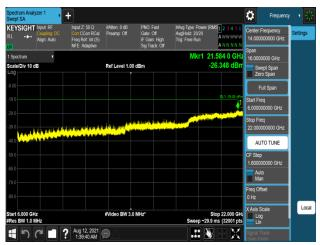
Plot 7-1225. Conducted Spurious Emission Plot 6 GHz to 22 GHz (Multi Band\_B2\_5M\_1C\_Low + B66\_5M\_1C\_High\_QPSK - Port 3)
