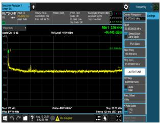
Plot 7-1184. Conducted Spurious Emission Plot 150 kHz to 30 MHz (B66\_5M+5M\_2C\_QPSK - Port 1)
