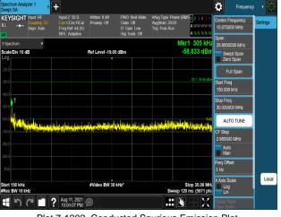
Plot 7-1202. Conducted Spurious Emission Plot 150 kHz to 30 MHz (B66\_5M+5M+5M+5M\_4C\_64QAM - Port 1)
