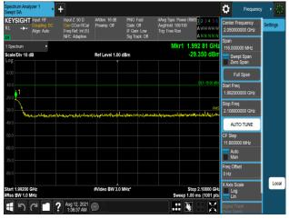
Plot 7-1223. Conducted Spurious Emission Plot 1.992 GHz to 2.108 GHz (Multi Band\_B2\_5M\_1C\_Low + B66\_5M\_1C\_High\_QPSK - Port 0)
