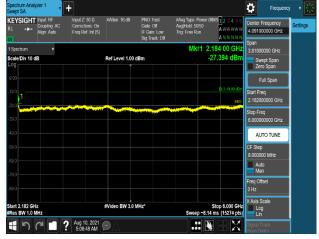
Plot 7-1181. Conducted Spurious Emission Plot 2.182 GHz to 6 GHz (B66\_20M+20M\_2C\_QPSK - Port 2)
