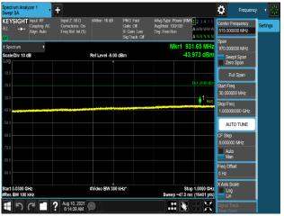
Plot 7-1185. Conducted Spurious Emission Plot 30 MHz to 1 GHz (B66\_5M+5M\_2C\_QPSK - Port 2)
