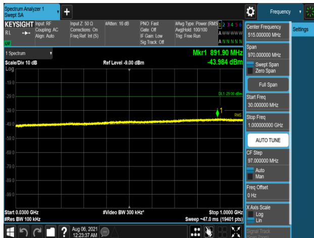
Plot 7-1131. Conducted Spurious Emission Plot 30 MHz to 1 GHz (B66_5M+5M+5M_3C_QPSK - High Channel, Port 0)
