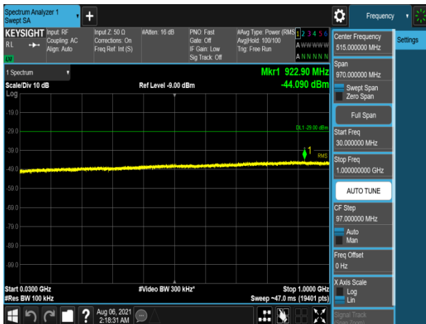
Plot 7-1137. Conducted Spurious Emission Plot 30 MHz to 1 GHz (B66_5M+5M+20M_3C_QPSK - Low Channel, Port 0)
