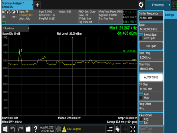
Plot 7-1117. Conducted Spurious Emission Plot 9 kHz to 150 kHz (B66_5M+20M_2C_64QAM - Low Channel, Port 3)
