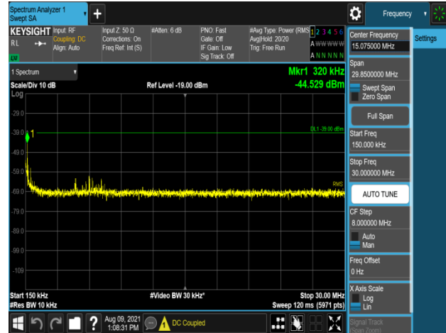
Plot 7-1160. Conducted Spurious Emission Plot 150 kHz to 30 MHz (B66_5M+5M+10M+20M_4C_QPSK - Mid Channel, Port 3)
