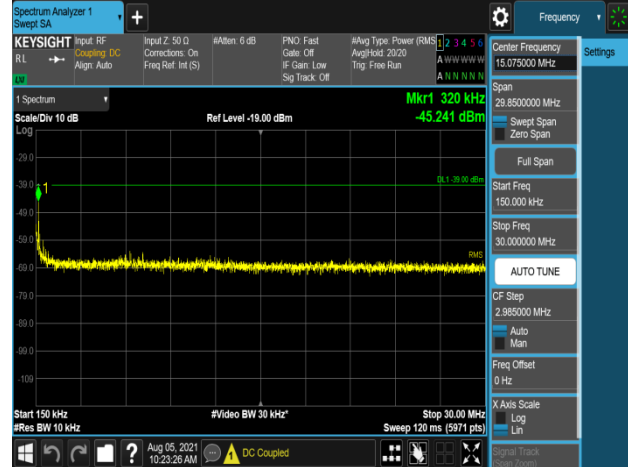
Plot 7-1124. Conducted Spurious Emission Plot 150 kHz to 30 MHz (B66_20M+20M_2C_64QAM - Mid Channel, Port 1)
