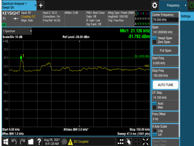
Plot 7-1123. Conducted Spurious Emission Plot 9 kHz to 150 kHz (B66_20M+20M_2C_16QAM - Low Channel, Port 1)
