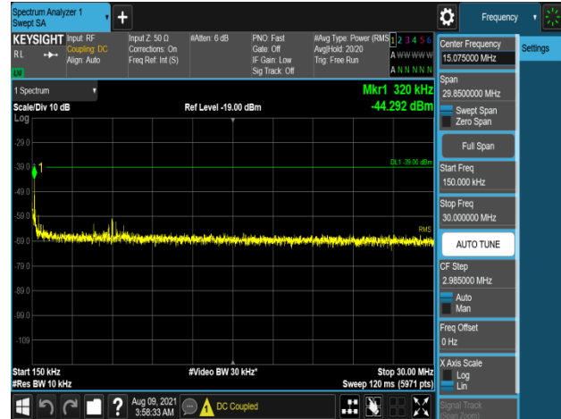
Plot 7-1142. Conducted Spurious Emission Plot 150 kHz to 30 MHz (B66_5M+15M+20M_3C_256QAM - Mid Channel, Port 3)
