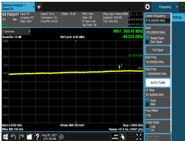
Plot 7-1119. Conducted Spurious Emission Plot 30 MHz to 1 GHz (B66_5M+20M_2C_QPSK - Low Channel, Port 2)
