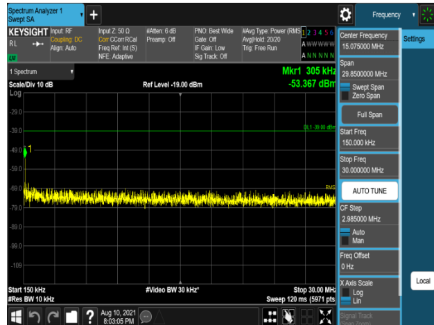
Plot 7-1154. Conducted Spurious Emission Plot 150 kHz to 30 MHz (B66_5M+5M+5M+20M_4C_64QAM - Mid Channel, Port 1)
