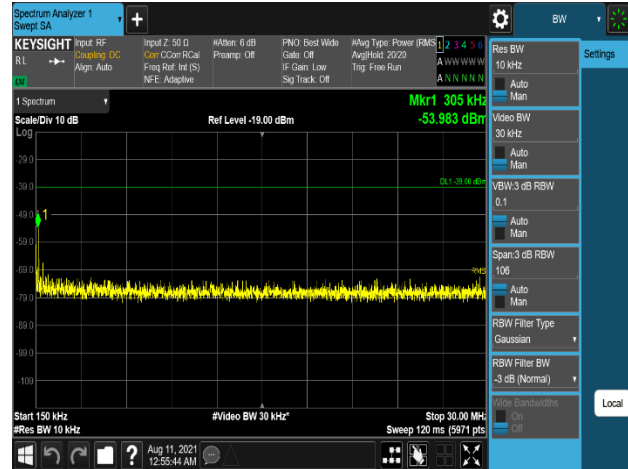
Plot 7-1070. Conducted Spurious Emission Plot 150 kHz to 30 MHz (B2_10M+20M_2C_QPSK - Port 3)
