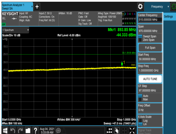
Plot 7-1113. Conducted Spurious Emission Plot 30 MHz to 1 GHz (B66_5M+5M_2C_QPSK - Low Channel, Port 0)
