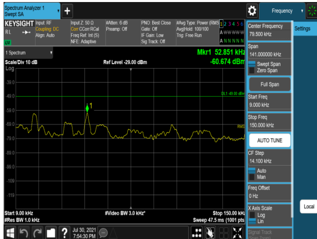
Plot 7-1105. Conducted Spurious Emission Plot 9 kHz to 150 kHz (B66_20M_1C_256QAM - High Channel, Port 1)
