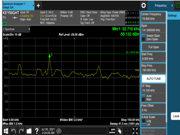
Plot 7-1099. Conducted Spurious Emission Plot 9 kHz to 150 kHz (B66_15M_1C_64QAM - Mid Channel, Port 1)
