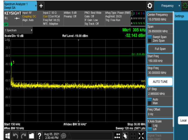
Plot 7-1040. Conducted Spurious Emission Plot 150 kHz to 30 MHz (B2_10M+20M_2C_64QAM - Mid Channel, Port 1)
