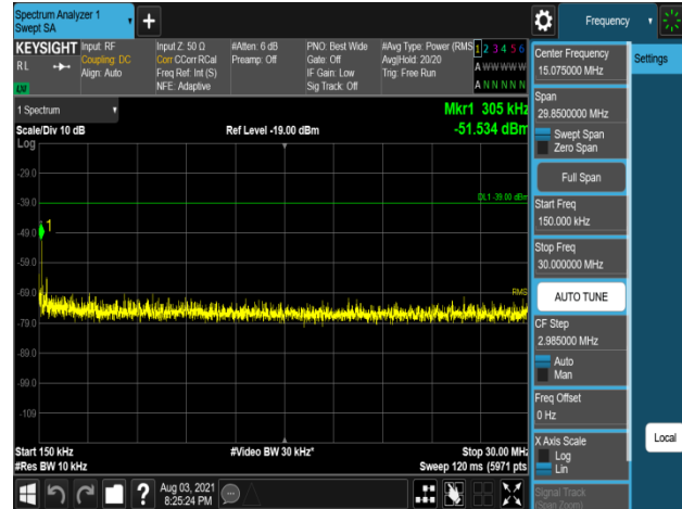
Plot 7-1022. Conducted Spurious Emission Plot 150 kHz to 30 MHz (B2_20M_1C_64QAM - High Channel, Port 1)
