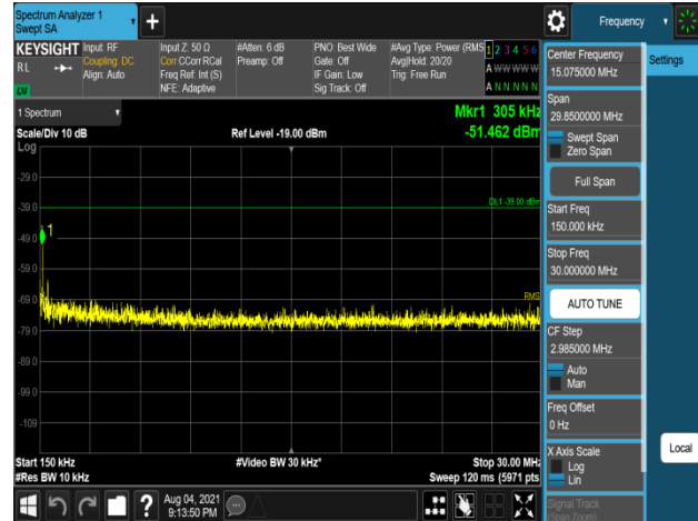
Pot 7-1028. Conducted Spurious Emission Plot 150 kHz to 30 MHz (B2_5M+5M_2C_QPSK - High Channel, Port 1)
