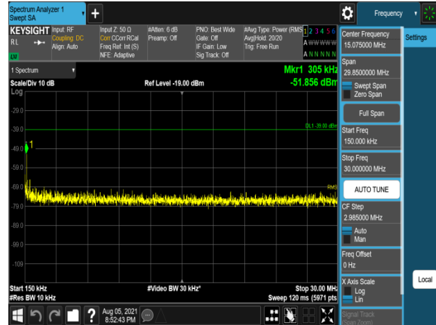
Pot 7-1046. Conducted Spurious Emission Plot 150 kHz to 30 MHz (B2_5M+5M+5M_3C_QPSK - Low Channel, Port 1)
