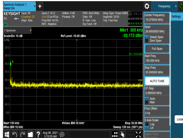
Plot 7-1052. Conducted Spurious Emission Plot 150 kHz to 30 MHz (B2_5M+5M+20M_3C_256QAM - Low Channel, Port 1)
