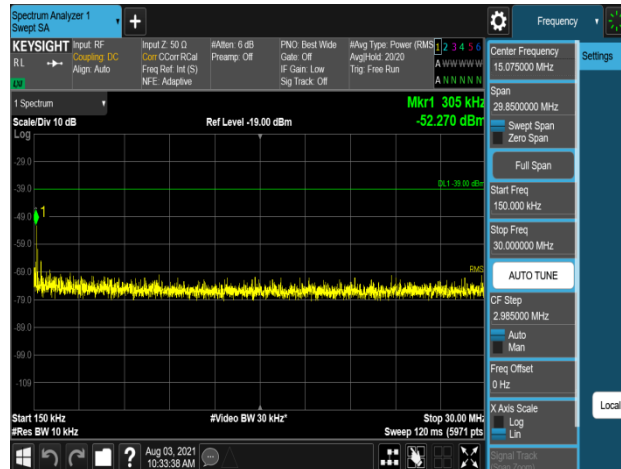
Plot 7-1016. Conducted Spurious Emission Plot 150 kHz to 30 MHz (B2_15M_1C_16QAM - Low Channel, Port 1)
