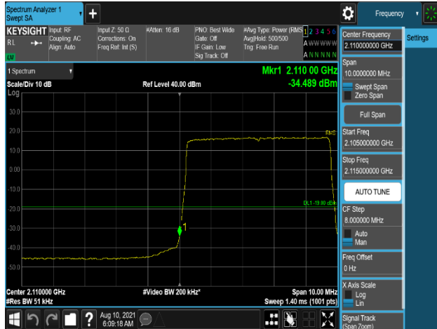
Plot 7-979. Band Edge Emission (2109MHz to 2110MHz) Plot (B66_5M+5M+5M_3C_64QAM - Low Channel, Port 2)
