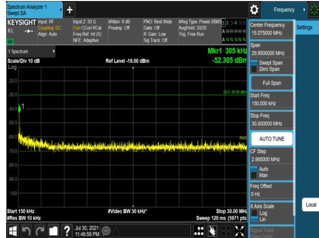
Plot 7-1004. Conducted Spurious Emission Plot 150 kHz to 30 MHz (B2_5M_1C_256QAM - Mid Channel, Port 1)
