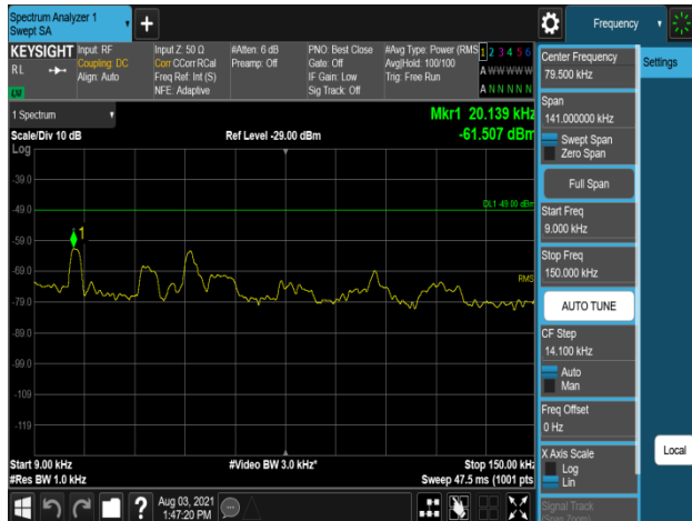
Plot 7-1015. Conducted Spurious Emission Plot 9 kHz to 150 kHz (B2_15M_1C_64QAM - High Channel, Port 1)
