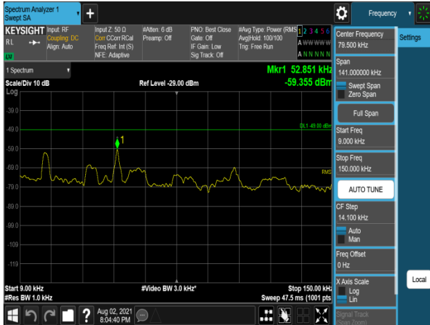
Plot 7-1009. Conducted Spurious Emission Plot 9 kHz to 150 kHz (B2_10M_1C_64QAM - High Channel, Port 1)
