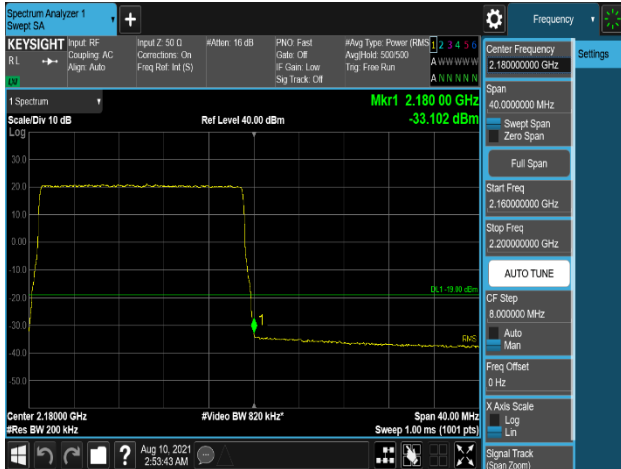
Plot 7-973. Band Edge Emission (2180MHz to 2181MHz) Plot (B66_5M+20M_2C_64QAM - High Channel, Port 0)
