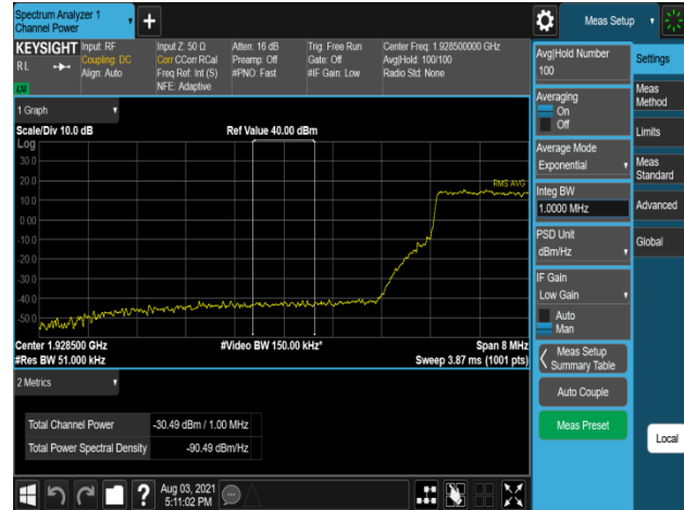
Plot 7-872. Band Edge Emission (1928MHz to 1929MHz) Plot (B2_20M_1C_16QAM - Low Channel, Port 3)
