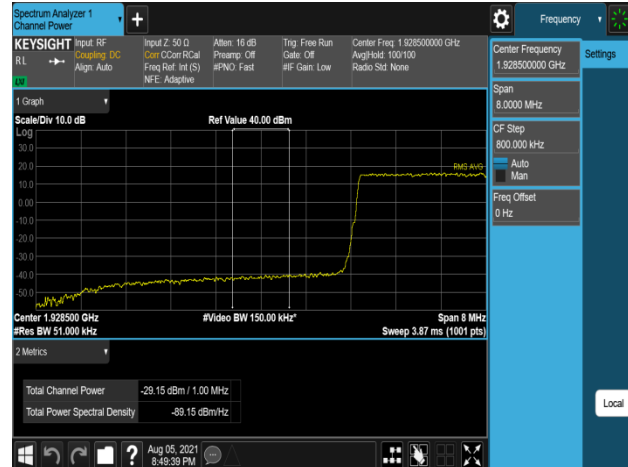
Plot 7-888. Band Edge Emission (1928MHz to 1929MHz) Plot (B2_5M+5M+5M_3C_QPSK - Low Channel, Port 3)
