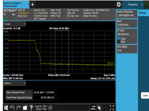
Plot 7-866. Band Edge Emission (1991MHz to 1992MHz) Plot (B2_10M_1C_64QAM - High Channel, Port 2)
