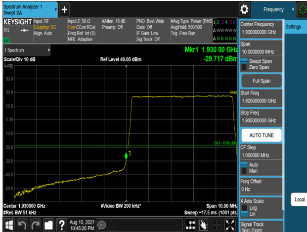
Plot 7-895. Band Edge Emission (1929MHz to 1930MHz) Plot (B2_5M+5M_2C_64QAM - Low Channel, Port 2)
