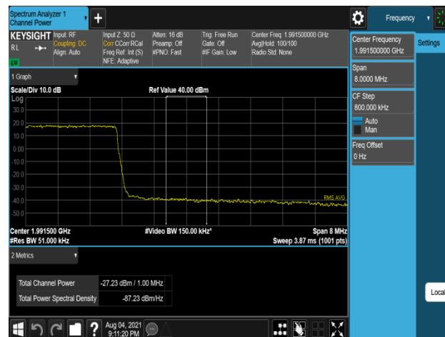
Plot 7-878. Band Edge Emission (1991MHz to 1992MHz) Plot (B2_5M+5M_2C_16QAM - High Channel, Port 2)
