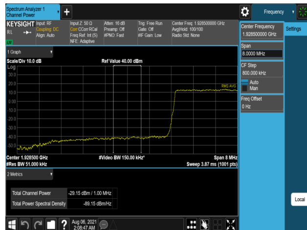
Plot 7-892. Band Edge Emission (1928MHz to 1929MHz) Plot (B2_5M+5M+20M_3C_QPSK - Low Channel, Port 3)
