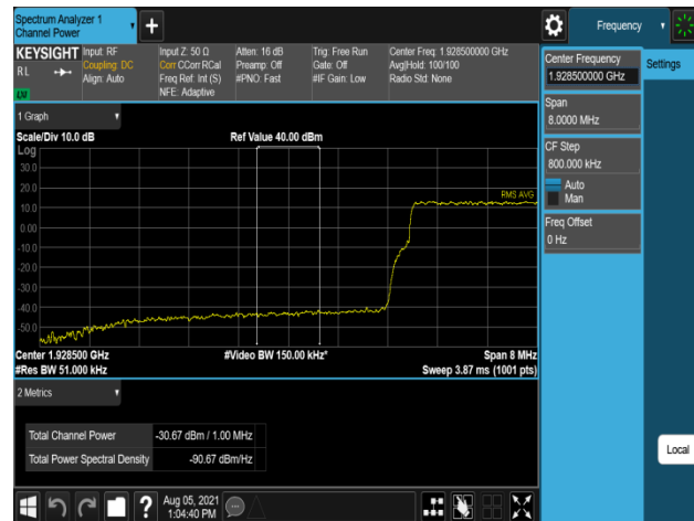
Plot 7-884. Band Edge Emission (1928MHz to 1929MHz) Plot (B2_10M+20M_2C_64QAM - Low Channel, Port 0)
