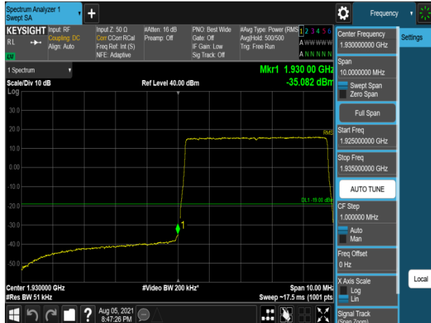
Plot 7-887. Band Edge Emission (1929MHz to 1930MHz) Plot (B2_5M+5M+5M_3C_QPSK - Low Channel, Port 0)
