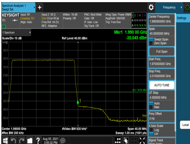
Plot 7-885. Band Edge Emission (1990MHz to 1991MHz) Plot (B2_10M+20M_2C_64QAM - High Channel, Port 0)
