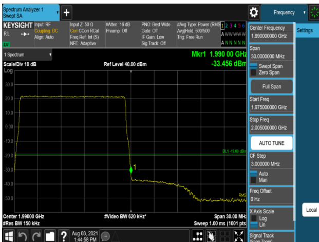
Plot 7-869. Band Edge Emission (1990MHz to 1991MHz) Plot (B2_15M_1C_64QAM - High Channel, Port 2)
