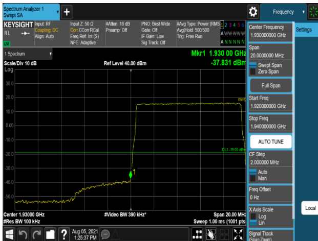
Plot 7-883. Band Edge Emission (1929MHz to 1930MHz) Plot (B2_10M+20M_2C_256QAM - Low Channel, Port 2)
