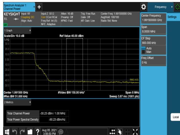
Plot 7-886. Band Edge Emission (1991MHz to 1992MHz) Plot (B2_10M+20M_2C_64QAM - High Channel, Port 0)
