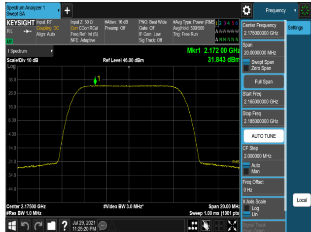
Plot 7-658. Peak Power Spectral Density Plot (B66_10M_1C_256QAM - High Channel, Port 1)
