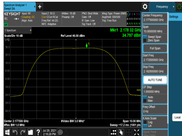
Plot 7-646. Peak Power Spectral Density Plot (B66_5M_1C_16QAM – High Channel, Port 1)
