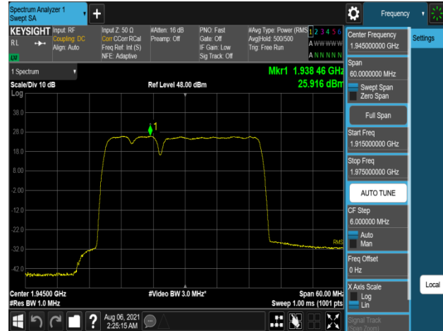
Plot 7-626. Peak Power Spectral Density Plot (B2_5M+5M+20M_3C_16QAM - Low Channel, Port 1)
