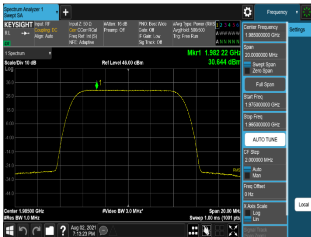
Plot 7-551. Peak Power Spectral Density Plot (B2_10M_1C_QPSK - High Channel, Port 2)
