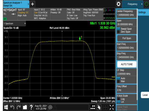
Plot 7-542. Peak Power Spectral Density Plot (B2_10M_1C_16QAM - Low Channel, Port 1)
