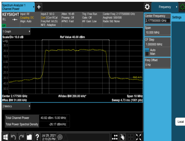
Plot 7-381. Conducted Average Output Power Plot (B66_5M_1C_16QAM - High Channel, Port 0)
