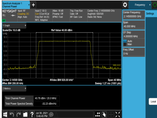
Plot 7-415. Conducted Average Output Power Plot (B66_20M_1C_64QAM - Mid Channel, Port 2)
