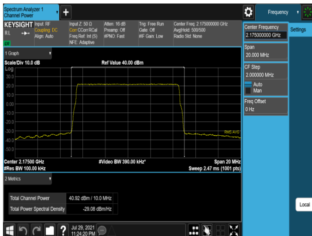
Plot 7-395. Conducted Average Output Power Plot (B66_10M_1C_256QAM – High Channel, Port 2)
