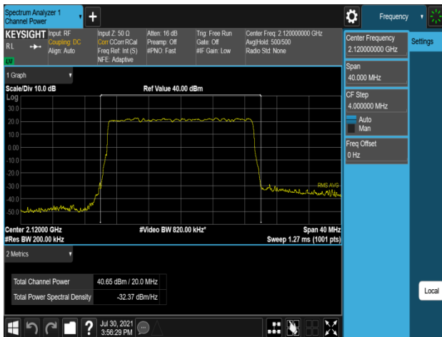
Plot 7-411. Conducted Average Output Power Plot (B66_20M_1C_16QAM - Low Channel, Port 2)
