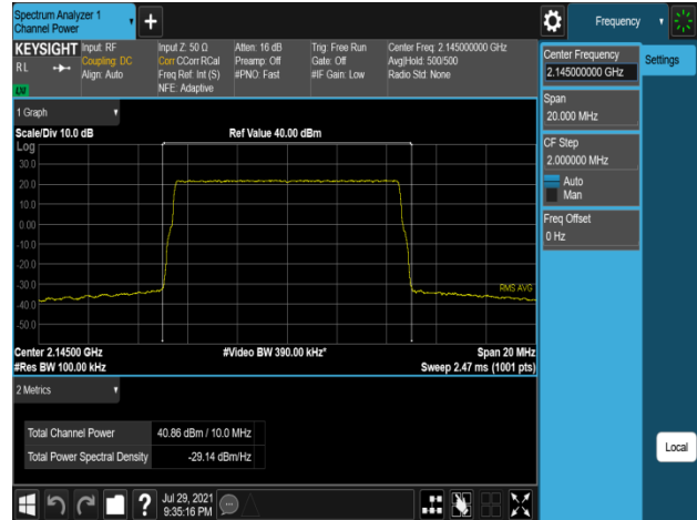
Plot 7-392. Conducted Average Output Power Plot (B66_10M_1C_64QAM - Mid Channel, Port 3)
