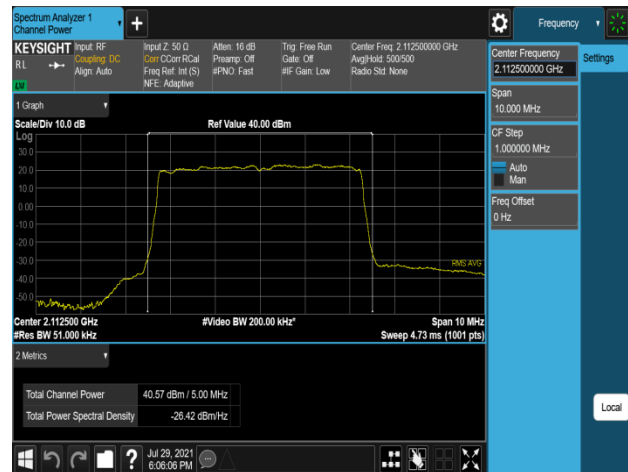
Plot 7-376. Conducted Average Output Power Plot (B66_5M_1C_16QAM - Low Channel, Port 3)
