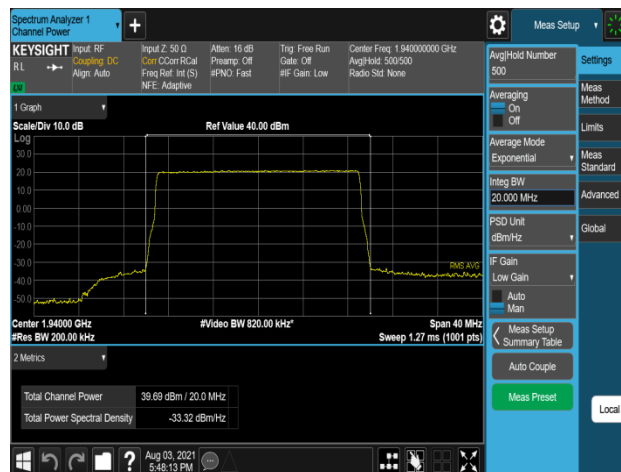
Plot 7-304. Conducted Average Output Power Plot (B2_20M_1C_256QAM - Low Channel, Port 3)
