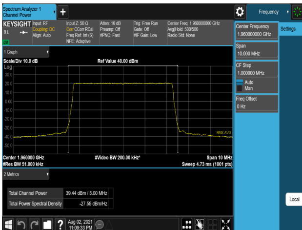
Plot 7-269. Conducted Average Output Power Plot (B2_5M_1C_QPSK - Mid Channel, Port 0)
