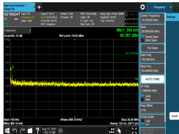
Plot 7-1241. Conducted Spurious Emission Plot 150 kHz to 30 MHz (Multi Band_B2_5M+5M+5M_3C_High + B66_5M+5M+5M_3C_Low_QPSK - Port 3)
