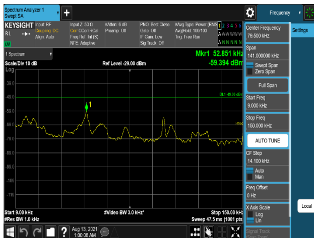
Plot 7-1240. Conducted Spurious Emission Plot 9 kHz to 150 kHz (Multi Band_B2_5M+5M+5M_3C_High + B66_5M+5M+5M_3C_Low_QPSK - Port 1)
