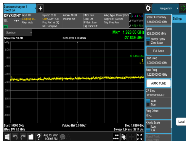
Plot 7-1243. Conducted Spurious Emission Plot 1 GHz to 1.928 GHz (Multi Band_B2_5M+5M+5M_3C_High + B66_5M+5M+5M_3C_Low_QPSK - Port 3)
