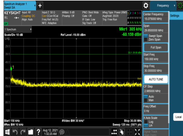
Plot 7-1220. Conducted Spurious Emission Plot 150 kHz to 30 MHz (Multi Band_B2_5M_1C_Low + B66_5M_1C_High_QPSK - Port 0)
