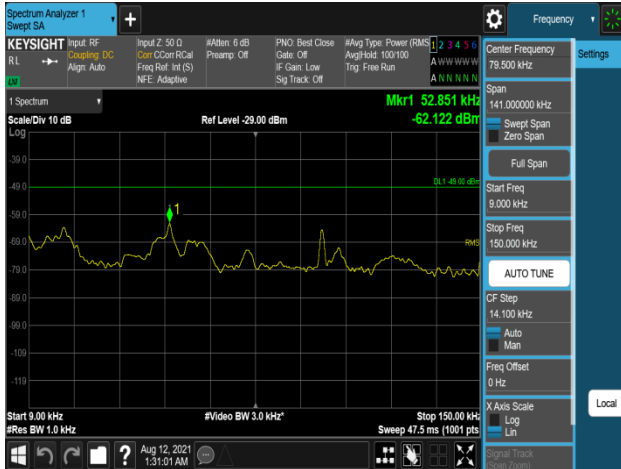
Plot 7-1219. Conducted Spurious Emission Plot 9 kHz to 150 kHz (Multi Band_B2_5M_1C_Low + B66_5M_1C_High_QPSK - Port 2)
