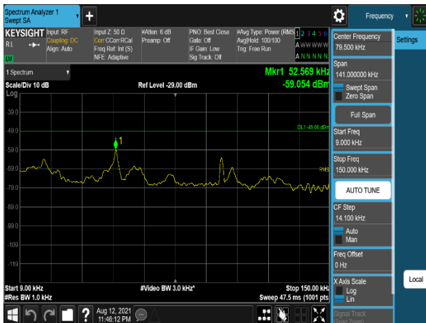
Plot 7-1226. Conducted Spurious Emission Plot 9 kHz to 150 kHz (Multi Band_B2_5M_1C_High + B66_5M_1C_Low_QPSK - Port 1)
