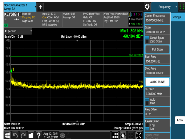
Plot 7-1227. Conducted Spurious Emission Plot 150 kHz to 30 MHz (Multi Band_B2_5M_1C_High + B66_5M_1C_Low_QPSK - Port 1)
