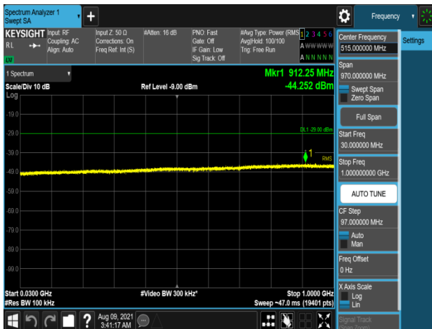
Plot 7-1143. Conducted Spurious Emission Plot 30 MHz to 1 GHz (B66_5M+15M+20M_3C_64QAM - Mid Channel, Port 2)
