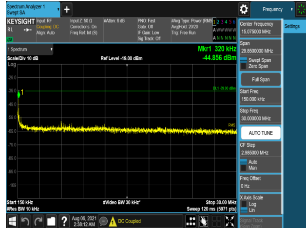
Plot 7-1136. Conducted Spurious Emission Plot 150 kHz to 30 MHz (B66_5M+5M+20M_3C_16QAM - Low Channel, Port 1)
