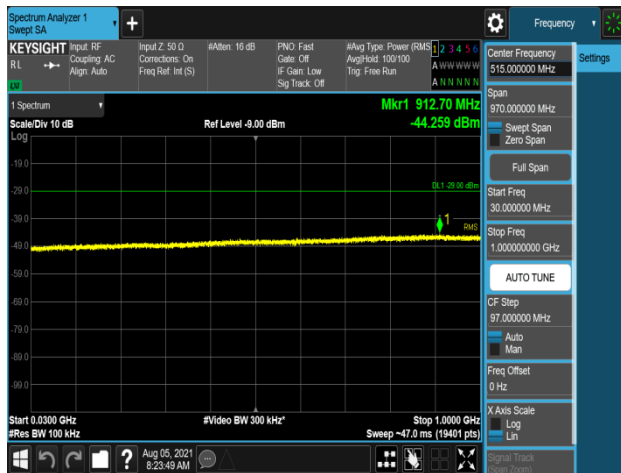
Plot 7-1125. Conducted Spurious Emission Plot 30 MHz to 1 GHz (B66_20M+20M_2C_QPSK - Low Channel, Port 2)
