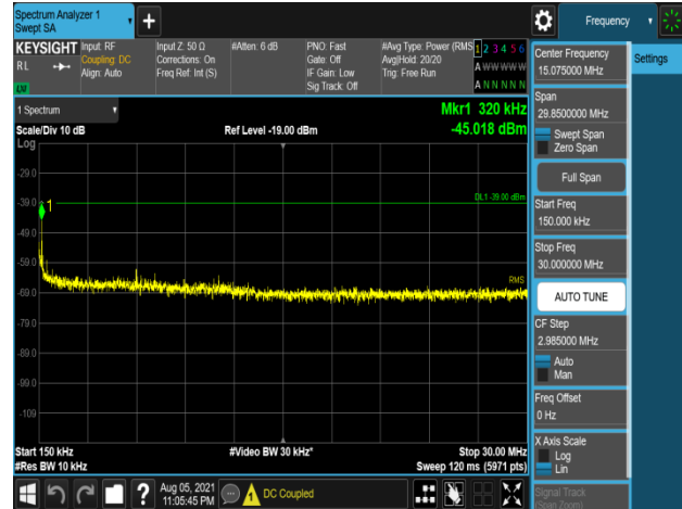
Pot 7-1130. Conducted Spurious Emission Plot 150 kHz to 30 MHz (B66_5M+5M+5M_3C_16QAM - Mid Channel, Port 1)
