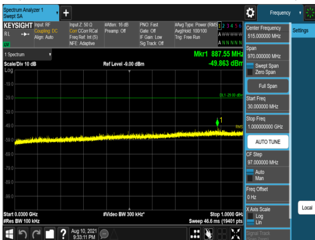
Plot 7-1155. Conducted Spurious Emission Plot 30 MHz to 1 GHz (B66_5M+5M+5M+20M_4C_64QAM - High Channel, Port 2)
