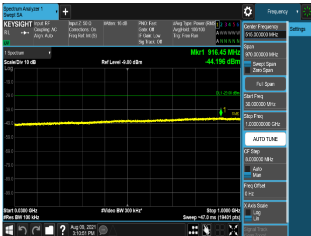
Plot 7-1161. Conducted Spurious Emission Plot 30 MHz to 1 GHz (B66_5M+5M+10M+20M_4C_64QAM - High Channel, Port 0)
