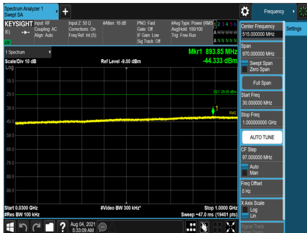
Plot 7-1113. Conducted Spurious Emission Plot 30 MHz to 1 GHz (B66_5M+5M_2C_QPSK - Low Channel, Port 0)
