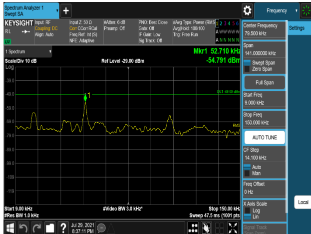
Plot 7-1093. Conducted Spurious Emission Plot 9 kHz to 150 kHz (B66_10M_1C_256QAM - Low Channel, Port 1)
