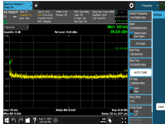
Pot 7-1076. Conducted Spurious Emission Plot 150 kHz to 30 MHz (B2_5M+5M+5M_3C_64QAM – Port 1)
