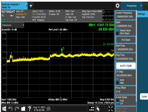
Plot 7-1085. Conducted Spurious Emission Plot 1.992 GHz to 6 GHz (B2_5M+5M+20M_3C_16QAM - Port 2)
