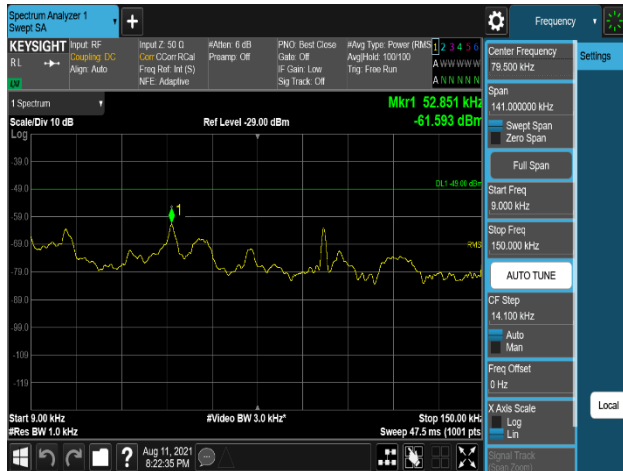
Plot 7-1075. Conducted Spurious Emission Plot 9 kHz to 150 kHz (B2_5M+5M+5M_3C_64QAM – Port 1)
