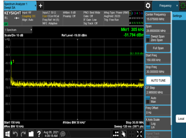
Plot 7-1034. Conducted Spurious Emission Plot 150 kHz to 30 MHz (B2_5M+20M_2C_64QAM - Mid Channel, Port 1)
