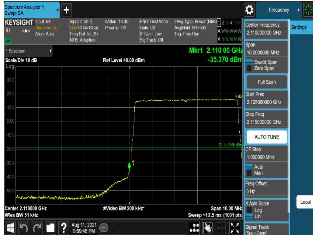
Plot 7-991. Band Edge Emission (2109MHz to 2110MHz) Plot (B66_5M+5M+5M+5M_4C_64QAM - Low Channel, Port 2)
