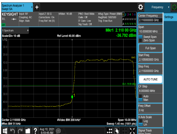
Plot 7-983. Band Edge Emission (2109MHz to 2110MHz) Plot (B66_5M+5M+20M_3C_16QAM - Low Channel, Port 0)
