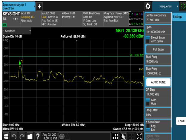
Plot 7-1021. Conducted Spurious Emission Plot 9 kHz to 150 kHz (B2_20M_1C_QPSK - Low Channel, Port 1)
