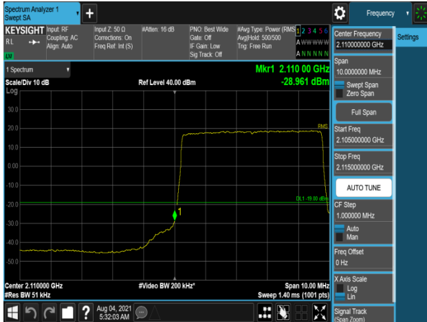
Plot 7-931. Band Edge Emission (2109MHz to 2110MHz) Plot (B66_5M+5M_2C_QPSK - Low Channel, Port 0)
