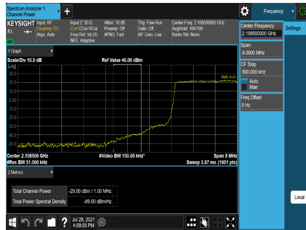
Plot 7-916. Band Edge Emission (2108MHz to 2109MHz) Plot (B66_5M_1C_64QAM - Low Channel, Port 3)
