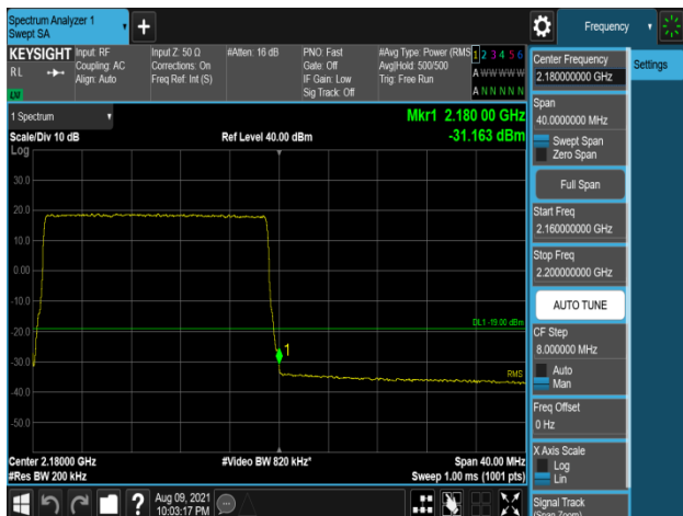
Plot 7-965. Band Edge Emission (2180MHz to 2181MHz) Plot (B66_5M+5M+10M+20M_4C_256QAM - High Channel, Port 2)
