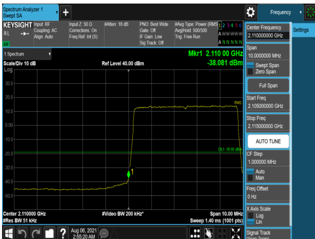
Plot 7-947. Band Edge Emission (2109MHz to 2110MHz) Plot (B66_5M+5M+20M_3C_64QAM - Low Channel, Port 2)
