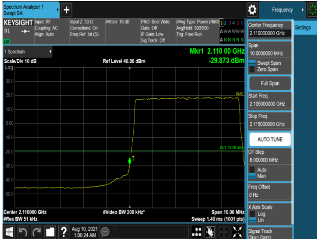
Plot 7-967. Band Edge Emission (2109MHz to 2110MHz) Plot (B66_5M+5M_2C_QPSK - Low Channel, Port 2)
