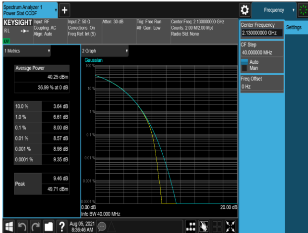
Plot 7-838. Peak To Average Power Ratio Plot (B66_20M+20M_2C_16QAM – Low Channel, Port 1)
