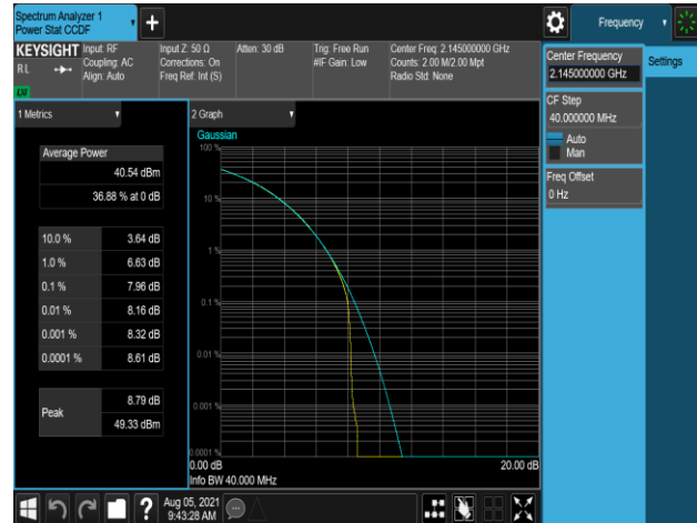
Plot 7-839. Peak To Average Power Ratio Plot (B66_20M+20M_2C_QPSK – Mid Channel, Port 3)
