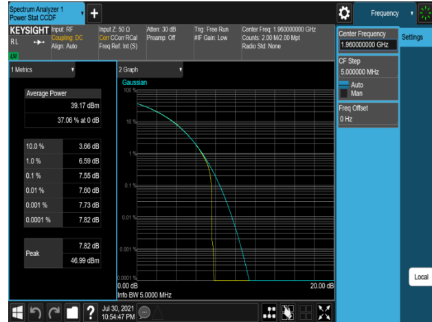
Plot 7-794. Peak To Average Power Ratio Plot (B2_5M_1C_16QAM - Mid Channel, Port 1)
