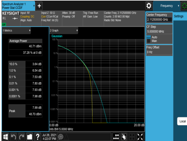
Plot 7-820. Peak To Average Power Ratio Plot (B66_5M_1C_16QAM - Low Channel, Port 0)
