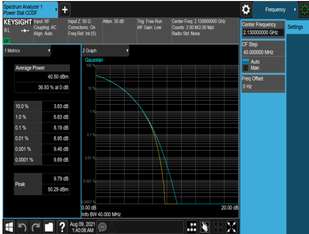
Plot 7-847. Peak To Average Power Ratio Plot (B66_5M+15M+20M_3C_16QAM – Low Channel, Port 0)
