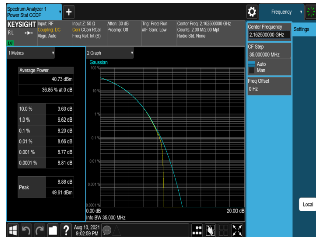
Plot 7-853. Peak To Average Power Ratio Plot (B66_5M+5M+5M+20M_4C_16QAM - Low Channel, Port 0)
