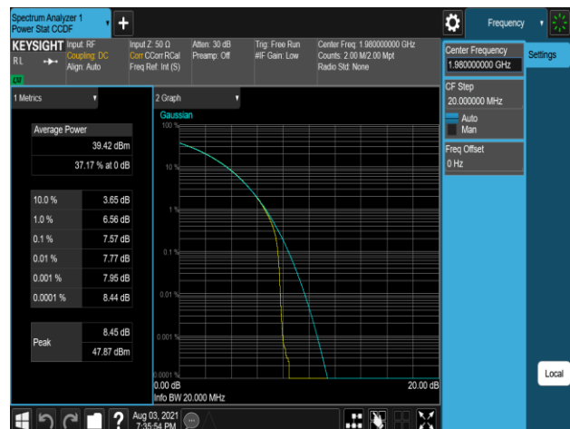
Plot 7-804. Peak To Average Power Ratio Plot (B2_20M_1C_QPSK – High Channel, Port 2)
