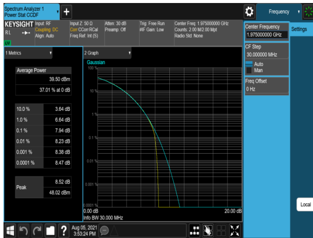
Plot 7-813. Peak To Average Power Ratio Plot (B2_10M+20M_2C_64QAM – High Channel, Port 0)
