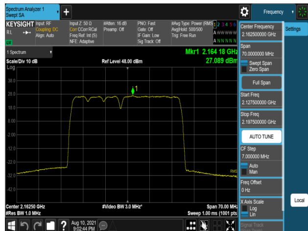
Plot 7-780. Peak Power Spectral Density Plot (B66_5M+5M+5M+20M_4C_16QAM - High Channel, Port 3)
