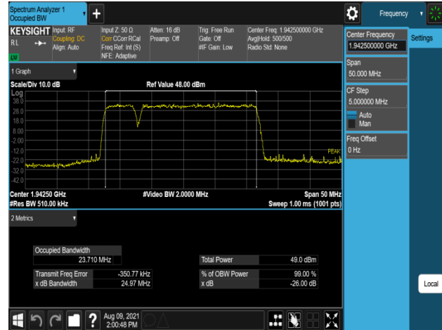
Plot 7-62. Occupied Bandwidth Plot (B2_5M+20M_2C_16QAM - Low Channel, Port 2)
