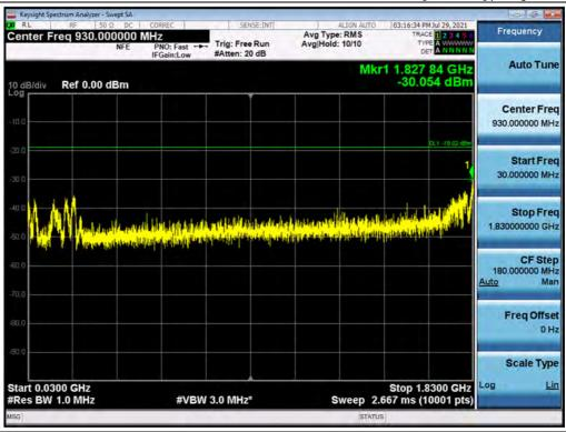
Antenna 1 / Low Edge - 100 MHz ~ Low Edge / B25 LTE 5 MHz 1 Carrier + B25 LTE 20 MHz 1 Carrier + B25 LTE 20 MHz 1 Carrier + B66 LTE 10 MHz 1 Carrier + B66 LTE 10 MHz 1 Carrier [5 Carrier] / 16QAM
