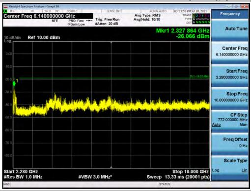
Antenna 3 / 10 GHz ~ 26.5 GHz / B25 LTE 5 MHz 1 Carrier + B25 LTE 20 MHz 1 Carrier + B25 LTE 5 MHz 1 Carrier + B66 LTE 10 MHz 1 Carrier + B66 LTE 10 MHz 1 Carrier [5 Carrier] / 256QAM
