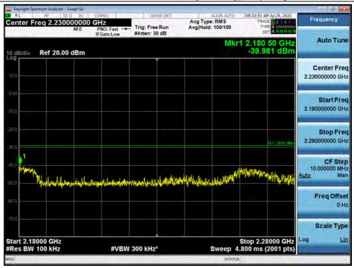
Antenna 1 / High Edge ~ High Edge + 100 MHz / B25 LTE 5 MHz 1 Carrier + B25 LTE 20 MHz 1 Carrier + B25 LTE 5 MHz 1 Carrier + B66 LTE 10 MHz 1 Carrier [4 Carrier]\_Low / QPSK
