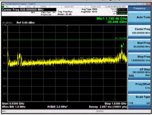
Antenna 1 / Low Edge - 100 MHz ~ Low Edge / B25 LTE 5 MHz 1 Carrier + B25 LTE 20 MHz 1 Carrier + B25 LTE 5 MHz 1 Carrier + B66 LTE 10 MHz 1 Carrier [4 Carrier]\_High / QPSK
