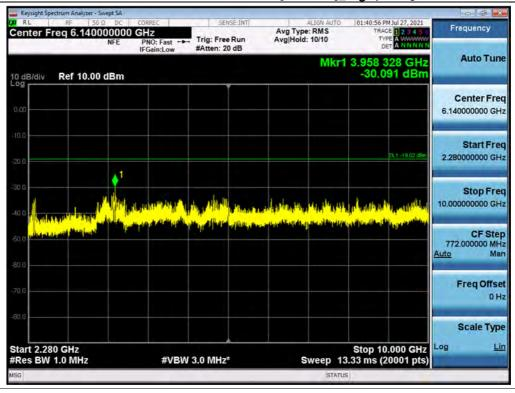
Antenna 1 / 10 GHz ~ 26.5 GHz / B25 LTE 5 MHz 1 Carrier + B25 LTE 15 MHz 1 Carrier + B25 LTE 5 MHz 1 Carrier + B66 LTE 5 MHz 1 Carrier [4 Carrier]\_High / 16QAM
