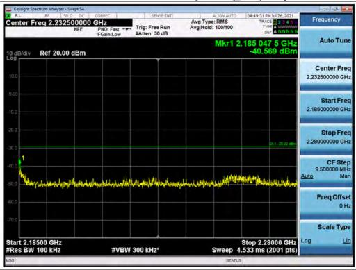
Antenna 1 / High Edge ~ High Edge + 100 MHz / B25 LTE 5 MHz 1 Carrier + B25 LTE 15 MHz 1 Carrier + B25 LTE 5 MHz 1 Carrier + B66 LTE 5 MHz 1 Carrier [4 Carrier]\_Low / QPSK
