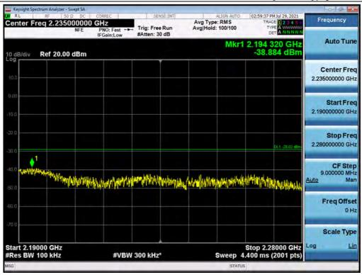
Antenna 3 / High Edge ~ High Edge + 100 MHz / B25 LTE 5 MHz 1 Carrier + B25 LTE 20 MHz 1 Carrier + B25 LTE 20 MHz 1 Carrier + B66 LTE 10 MHz 1 Carrier + B66 LTE 10 MHz 1 Carrier | 64QAM
