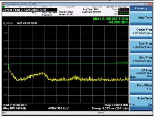
Antenna 2 / High Edge ~ High Edge + 100 MHz / B25 LTE 5 MHz 1 Carrier + B25 LTE 15 MHz 1 Carrier + B25 LTE 5 MHz 1 Carrier + B66 LTE 5 MHz 1 Carrier [4 Carrier]\_High / 16QAM
