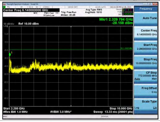
Antenna 2 / 10 GHz ~ 26.5 GHz / B25 LTE 5 MHz 1 Carrier + B25 LTE 20 MHz 1 Carrier + B25 LTE 5 MHz 1 Carrier + B66 LTE 5 MHz 1 Carrier + B66 LTE 10 MHz 1 Carrier [5 Carrier] / 16QAM
