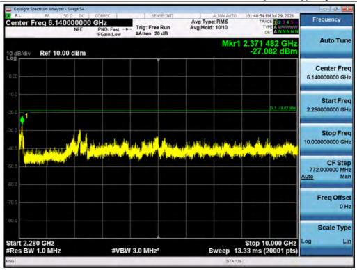
Antenna 3 / 10 GHz ~ 26.5 GHz / B25 LTE 5 MHz 1 Carrier + B25 LTE 20 MHz 1 Carrier + B25 LTE 20 MHz 1 Carrier + B66 LTE 5 MHz 1 Carrier + B66 LTE 20 MHz 1 Carrier [5 Carrier] / 256QAM
