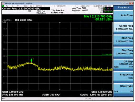
Antenna 1 / High Edge ~ High Edge + 100 MHz / B25 LTE 5 MHz 1 Carrier + B25 LTE 20 MHz 1 Carrier + B25 LTE 5 MHz 1 Carrier + B66 LTE 5 MHz 1 Carrier + B66 LTE 10 MHz 1 Carrier [5 Carrier] / 256QAM
