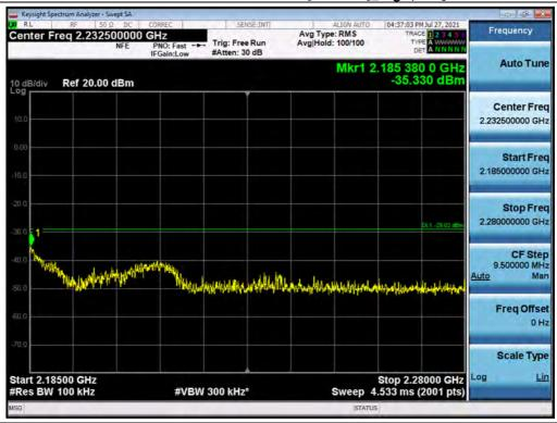
Antenna 1 / High Edge ~ High Edge + 100 MHz / B25 LTE 5 MHz 1 Carrier + B25 LTE 20 MHz 1 Carrier + B25 LTE 5 MHz 1 Carrier + B66 LTE 5 MHz 1 Carrier [4 Carrier]\_High / 16QAM
