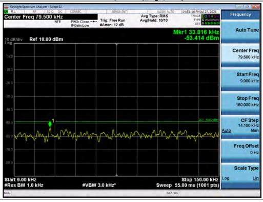
Antenna 0 / 150 kHz ~ 30 MHz / B25 LTE 5 MHz 1 Carrier + B25 LTE 20 MHz 1 Carrier + B25 LTE 5 MHz 1 Carrier + B66 LTE 5 MHz 1 Carrier [4 Carrier]\_High / 64QAM
