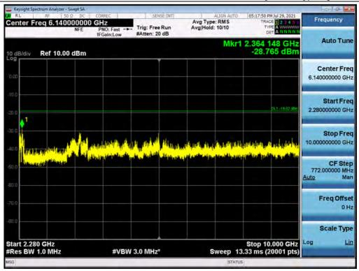
Antenna 1 / 10 GHz ~ 26.5 GHz / B25 LTE 5 MHz 1 Carrier + B25 LTE 20 MHz 1 Carrier + B25 LTE 20 MHz 1 Carrier + B66 LTE 5 MHz 1 Carrier + B66 LTE 10 MHz 1 Carrier [5 Carrier] / 256QAM
