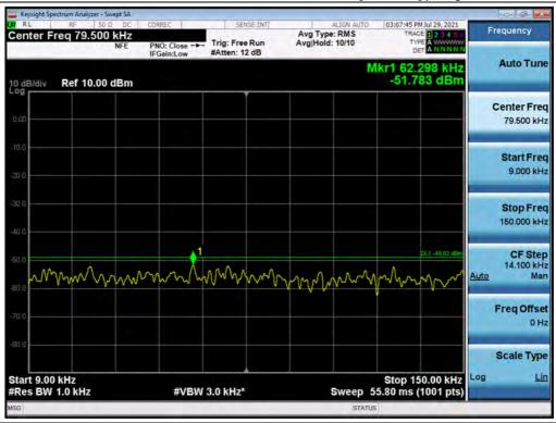
Antenna 0 / 150 kHz ~ 30 MHz / B25 LTE 5 MHz 1 Carrier + B25 LTE 20 MHz 1 Carrier + B25 LTE 20 MHz 1 Carrier + B66 LTE 10 MHz 1 Carrier | F25 LTE 20 MHz 1 C
