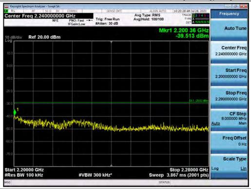
Antenna 1 / High Edge ~ High Edge + 100 MHz / B25 LTE 5 MHz 1 Carrier + B25 LTE 20 MHz 1 Carrier + B25 LTE 5 MHz 1 Carrier + B66 LTE 5 MHz 1 Carrier + B66 LTE 20 MHz 1 Carrier [5 Carrier] / 16QAM
