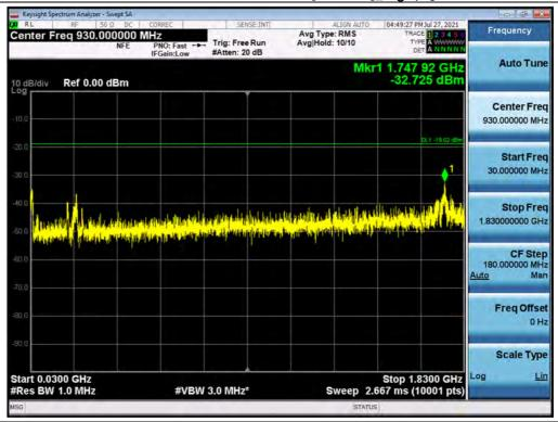
Antenna 1 / Low Edge - 100 MHz ~ Low Edge / B25 LTE 5 MHz 1 Carrier + B25 LTE 20 MHz 1 Carrier + B25 LTE 5 MHz 1 Carrier + B66 LTE 5 MHz 1 Carrier [4 Carrier]\_High / 16QAM
