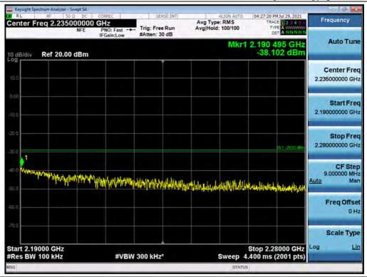
Antenna 2 / High Edge ~ High Edge + 100 MHz / B25 LTE 5 MHz 1 Carrier + B25 LTE 20 MHz 1 Carrier + B25 LTE 20 MHz 1 Carrier + B66 LTE 5 MHz 1 Carrier + B66 LTE 10 MHz 1 Carrier [5 Carrier] / 256QAM
