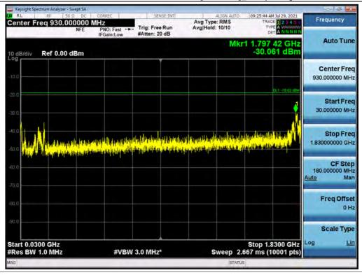
Antenna 1 / Low Edge - 100 MHz ~ Low Edge / B25 LTE 5 MHz 1 Carrier + B25 LTE 20 MHz 1 Carrier + B25 LTE 5 MHz 1 Carrier + B66 LTE 10 MHz 1 Carrier [4 Carrier]\_Low / QPSK
