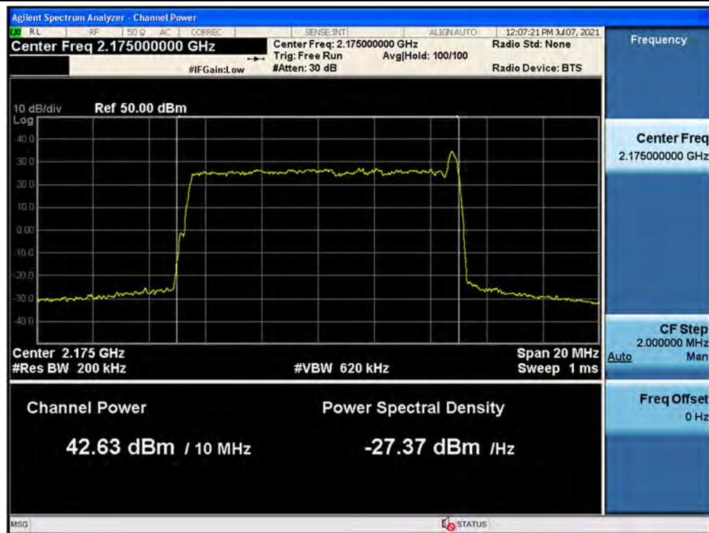
**Antenna 0 / B66 LTE 5 MHz 1 Carrier + B66 LTE 20 MHz 1 Carrier [2 Carrier] / Non-Contiguous / B66 LTE 5 MHz / 64QAM / Low**
