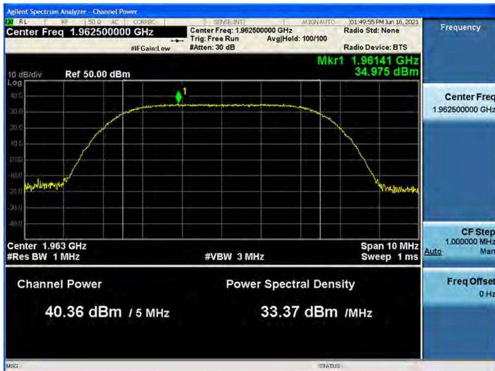
**Antenna 1 / B25 LTE 10 MHz 1 Carrier / QPSK / Low**
